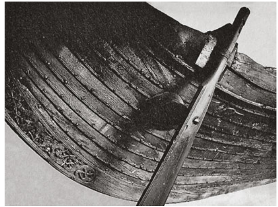
138 Every plank on the stern of the Oseberg ship has been decorated using a geitsfuss in exactly the same way as many log buildings. – Viking Ship Museum, Oslo, Norway
