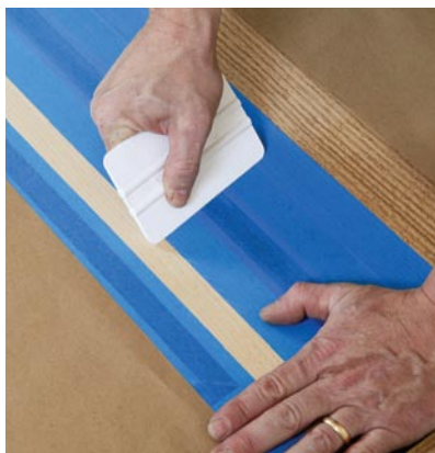
1. Burnish 3M blue painter's tape tight to the wood to prevent paints and stains from bleeding. You can use auto body spatulas, the back of a spoon, or a roller.
