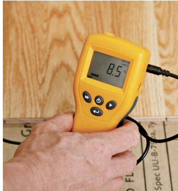
Check the moisture content of the floor between coats of waterborne finish. Re-coat when it's within 1% of the reading before finishing.
