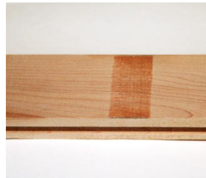
Sticker stain: Cross-grain stripes about 1 in. wide found at regular intervals on boards.
