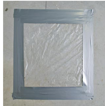
A common test for concrete slab moisture is to tape plastic to the slab and watch for condensation to develop. This test isn't of much value, however, because a lack of condensation doesn't guarantee the slab is at an acceptable moisture level.
