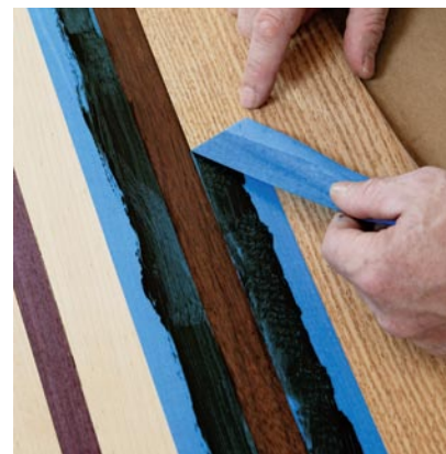
3. Pull the tape off at a 45° angle while the stain is still wet.
