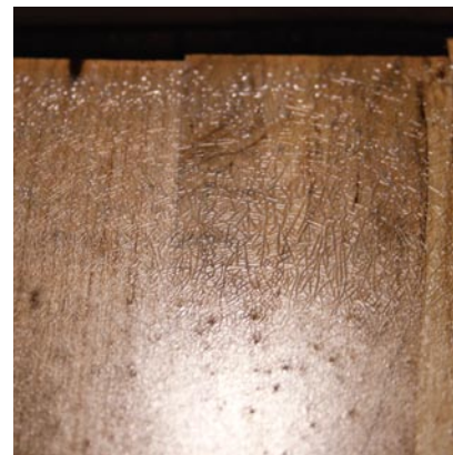
An alligator finish pulls away from itself, gathering into a series of ridges as it dries, and is rough to the touch.
