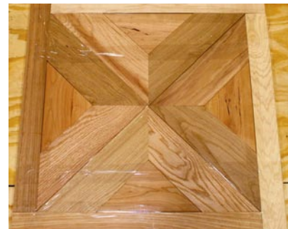
Parquet tiles can be made from \frac{3}{4} -in. flooring temporarily held together with tape or glue. When gluing the tiles to the subfloor, remove the tape.
