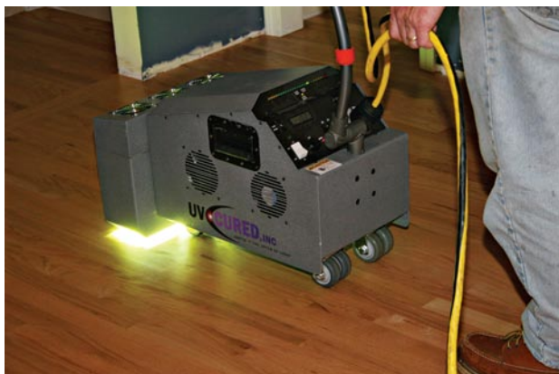
UV-cured urethanes harden instantly with exposure to UV light. This professional finish allows the room to go back into service immediately.
