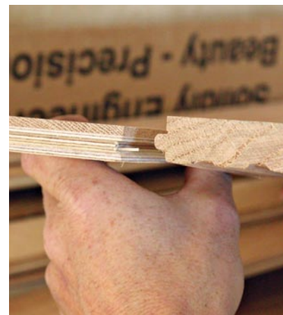
Engineered flooring, like plywood, is composed of multiple layers with a hardwood face veneer. The multiple layers create more stable flooring.
