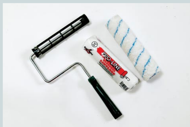
The author prefers rolling on all finishes, using solvent-resistant roller covers for oil-based finishes. Look for roller frames with straight ribs that won't distort the covers.
