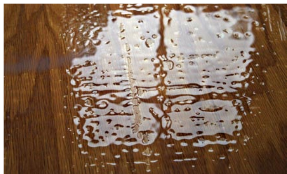
Crawling occurs when the finish pulls, or "crawls," away from itself.
