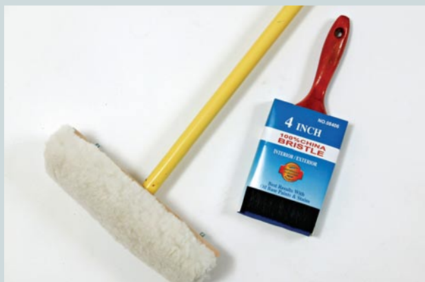
The traditional tools for applying oil-based finishes are a lamb's wool pad and a China bristle brush.
