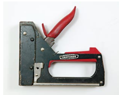
A stapler to tack down the moisture retarder.
