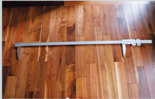
A vernier caliper is used to measure a group of boards.
