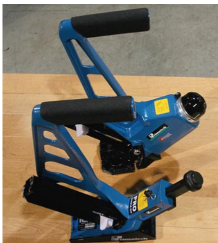
Whether manual (bottom) or pneumatic (top), both kinds of nailer beat doing it by hand—and either kind is available to rent.
