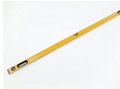
A 6-ft.- or 10-ft.-long straightedge to check the flatness of the subfloor.
