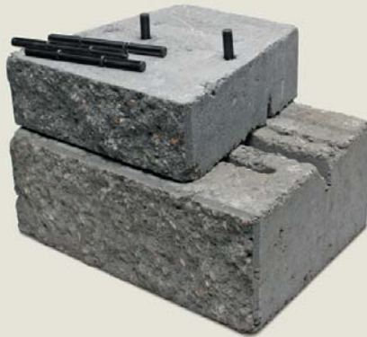
VERSA-LOK® MOSAIC. A top-down pinning system lets you push a pin through a hole in one course and into a groove in the course below ( www.versa-lok.com ; 800-770-4525).
