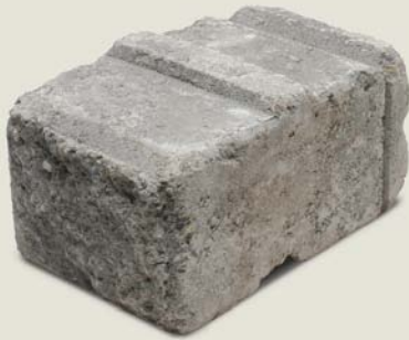
UNILOCK ROMAN PISA. A ridge on the top of one course fits into a groove on the bottom of the next ( www.unilock.com ; 800-864-5625).
