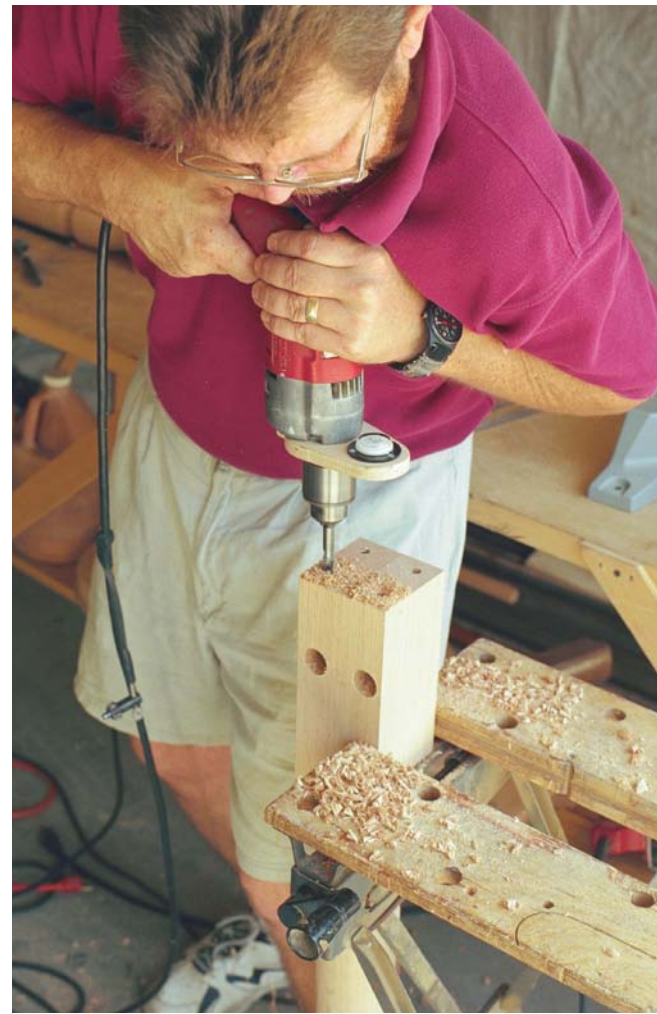
Bubble level keeps the drill straight. After drilling access holes in the newel, the author clamps the post plumb and drills four bolt holes that must be true. The bubble level's plywood base fits tightly onto the drill's motor housing.
