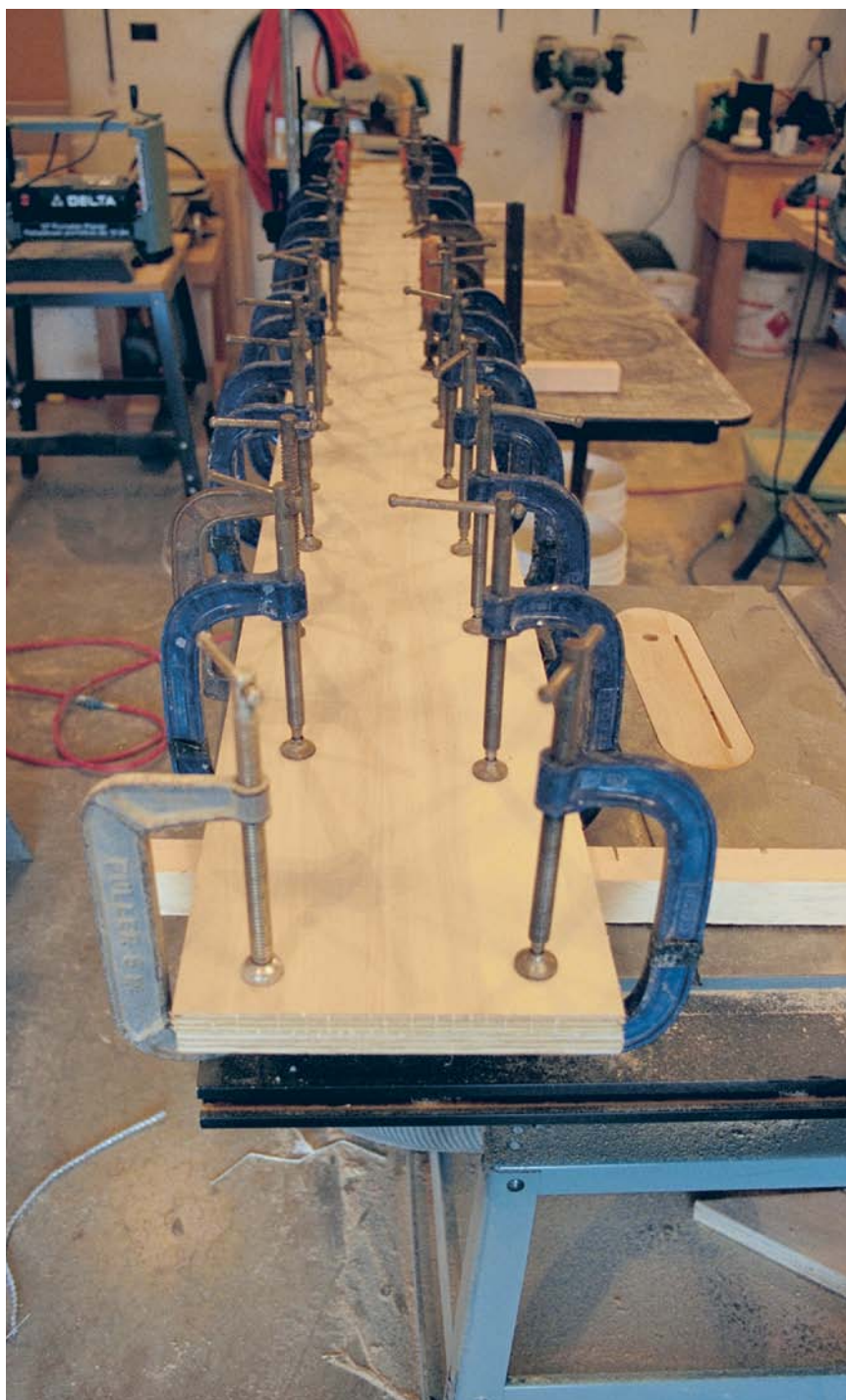
Laminated stringers won't shrink or warp. Two layers of \frac{3}{4} -in. plywood are glued together for stringer stock that will remain stable and true for the life of the stair.
