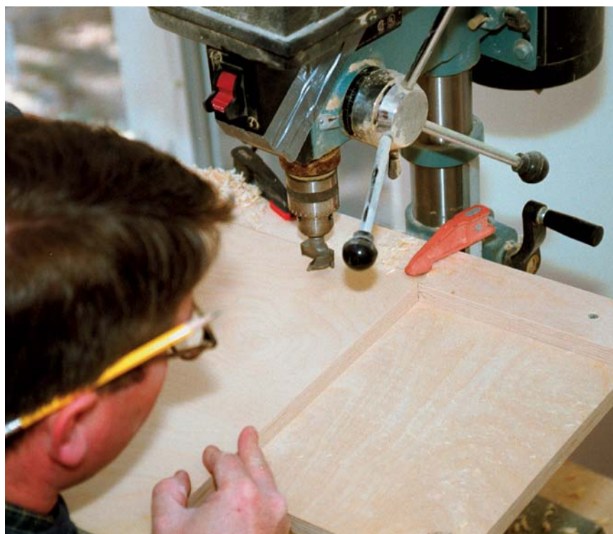
After testing the layout on scrap , the author drills 32mm holes in the backs of cabinet doors. Pencil marks on the drill-press fence indicate the door-edge alignment.
