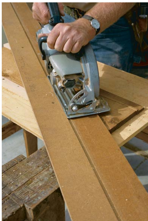
Shooting board for acute angles. A straightedge screwed to a pair of fences guides a circular saw through repetitive cuts that are beyond the swing of the sliding compound saw.
