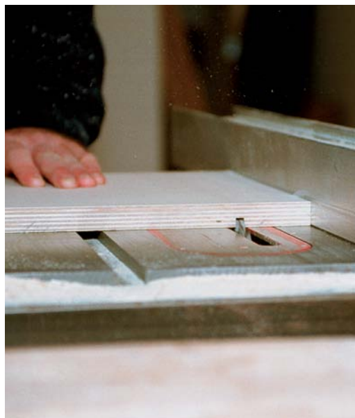
Grooving cabinet sides 2 in. from their bottoms creates space to hide over-the-counter lights.
