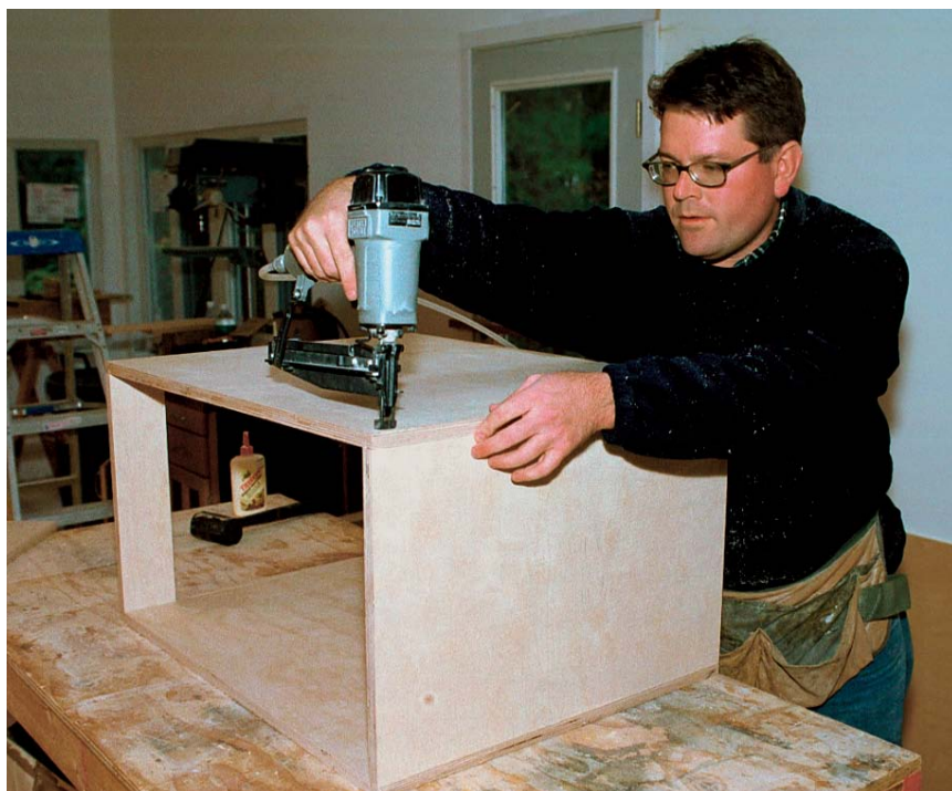
Nails secure cabinet boxes while the glue dries. Check for square by comparing diagonal measurements before the glue sets.
