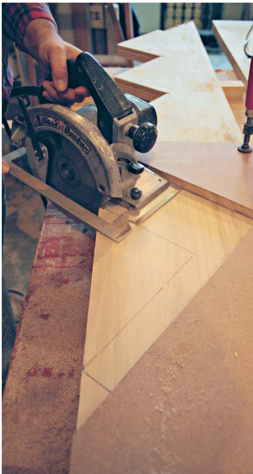
MDF jig for perfect sawcuts. The table of the circular saw registers against the edge of a simple jig made from MDF to eliminate freehand sawing. The cuts are finished with a jigsaw and fine-tuned with a chisel.
