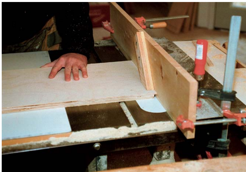
When cutting the tongues , a featherboard attached to an auxiliary fence makes the process safer and the tongues more consistent in thickness.
