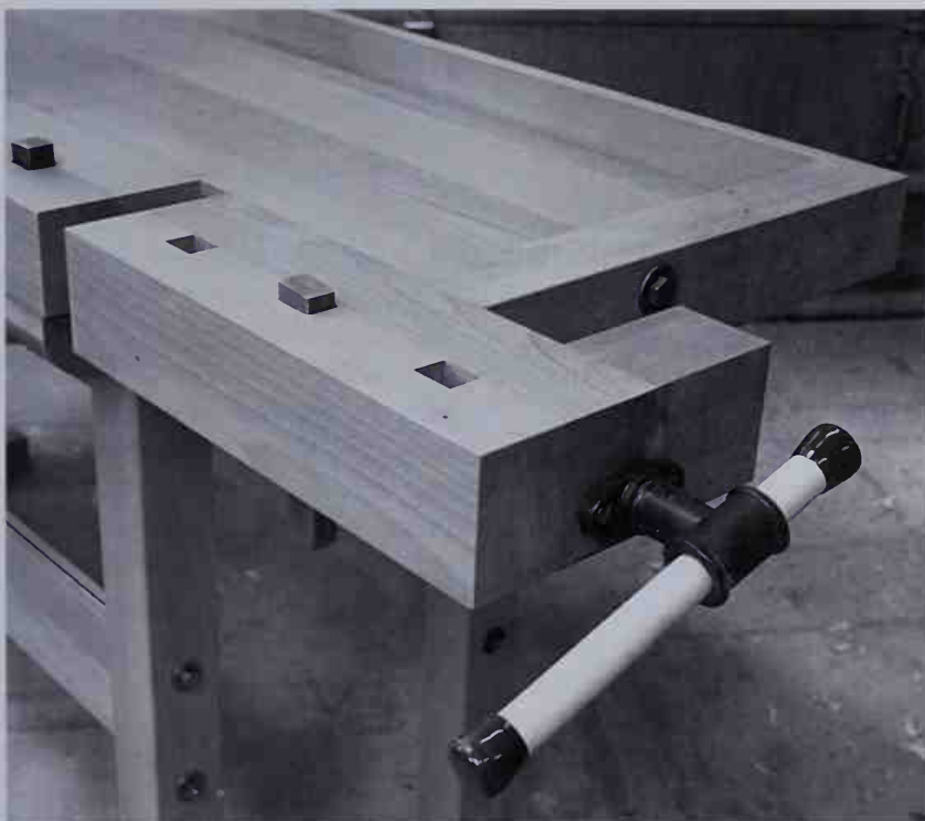
Bench dogs with a tail vise hold wood flat upon the workbench.
