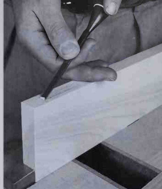
Use a chisel to pare back to the knife lines at each end of the mortise.
