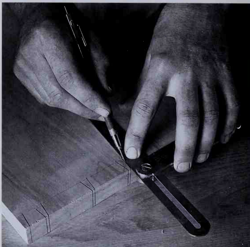
Use a sliding Tbevel to lay out the tails.
