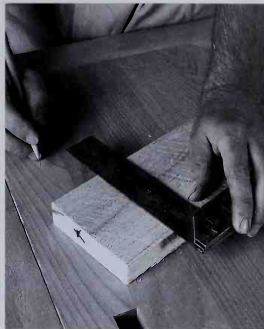
The correct way to use a try square is to hold the stock firmly against the work.
