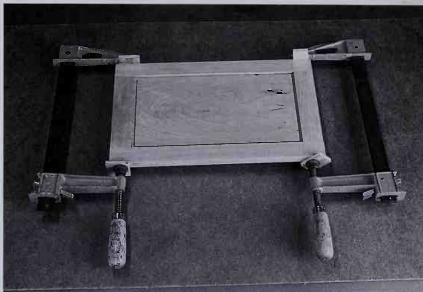
The cabinet door, glued and clamped.
