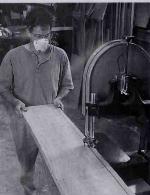
Cut the roughsawn board to approximate length on the radial-arm saw (top), then bandsaw the board to approximate width (above).
