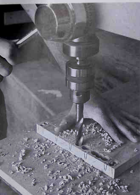
Drill out the bulk of the waste between the pins.
