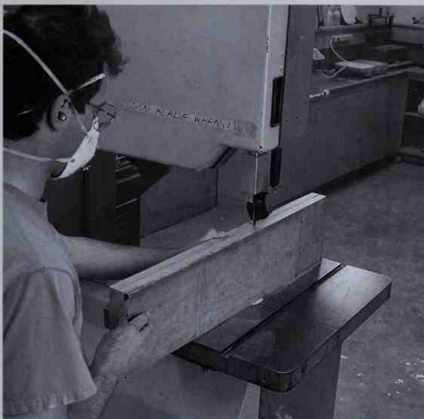
The author resaws a piece of 8/4 cherry for the carcass of the cabinet.
