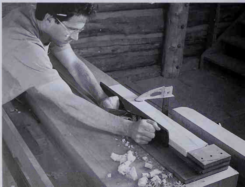
With the board clamped to the shooting board, plane along the entire length of the protruding edge.
