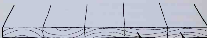
ALTERNATING GROWTH-RING CURVES
