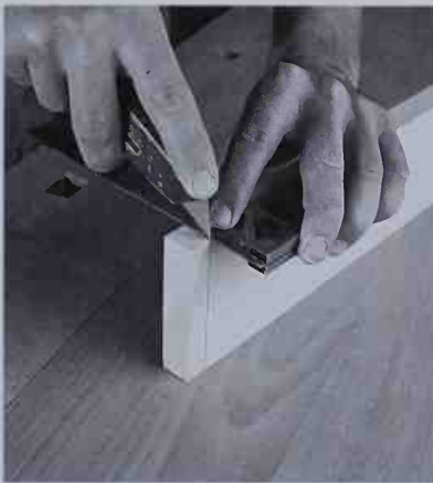
Use the first cut to register the knife for the second cut on the side of the board.
