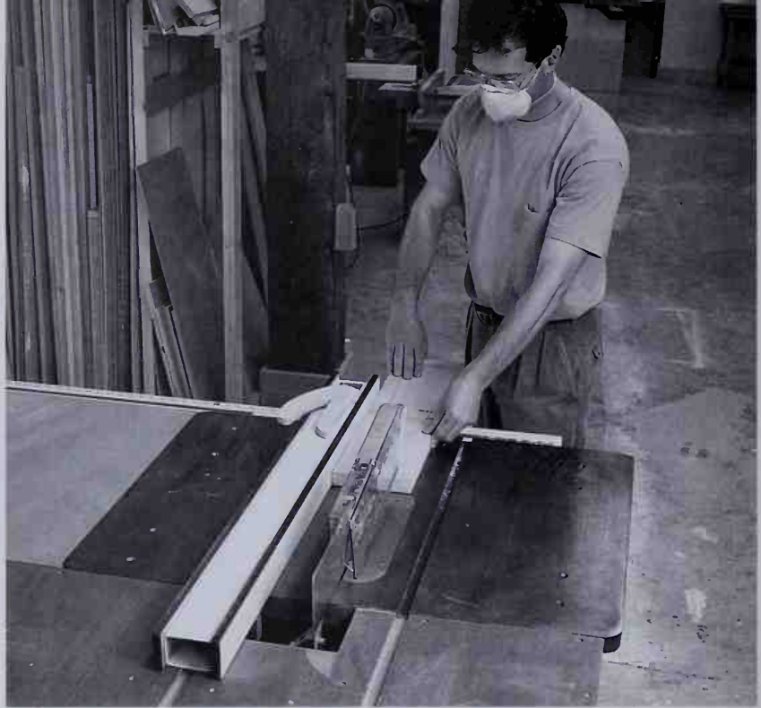
A rip fence is used when sawing a board along its length.
