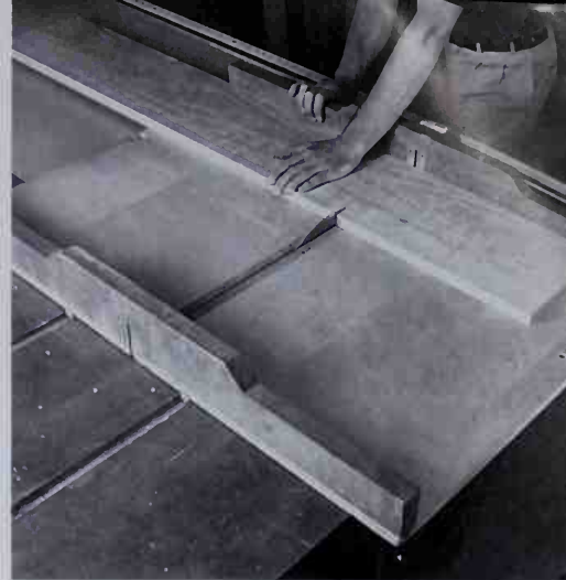
Crosscut the board to finished length using a sliding table on the table saw.
