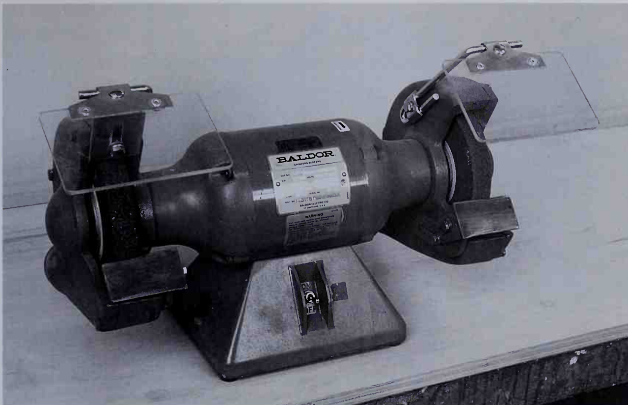
An electric grinder is used for reshaping chisels, plane irons and other tools.
