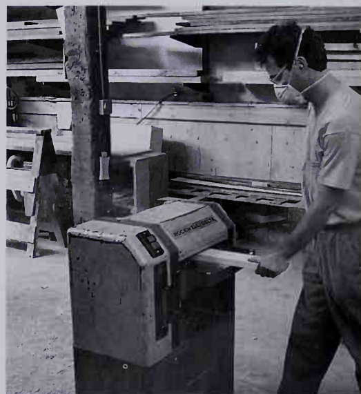
Feed the board through the thickness planer to achieve the desired thickness.
