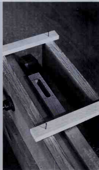
The rounded ends of the router-cut mortise can be chiseled square, or the tenons can be filed round to fit. ↑
