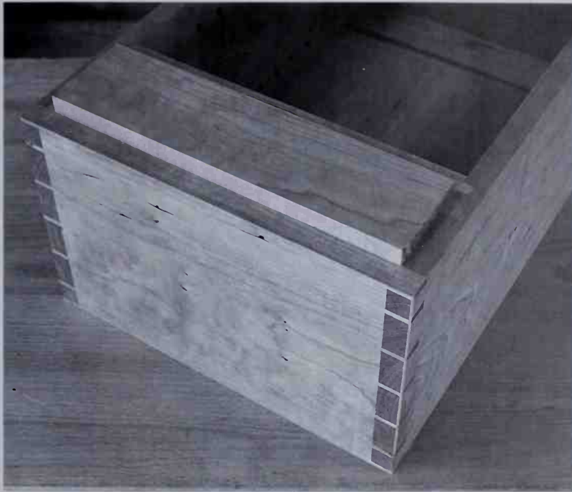
The drawer front should be cut to fit the opening tightly.
