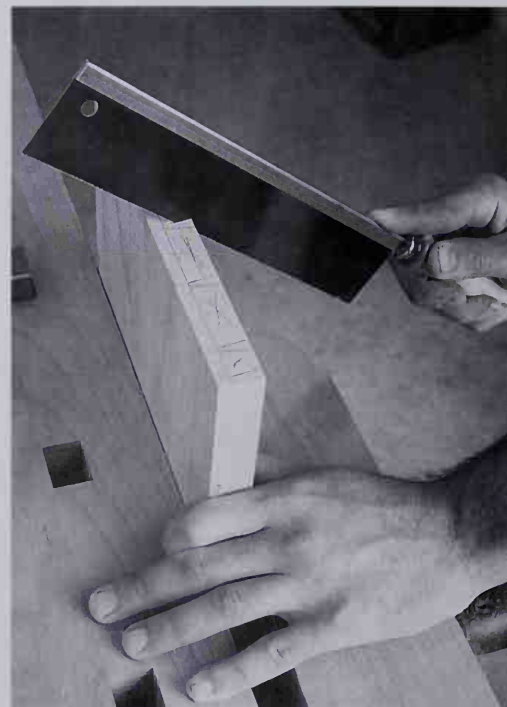
Saw the pins on the diagonal.
