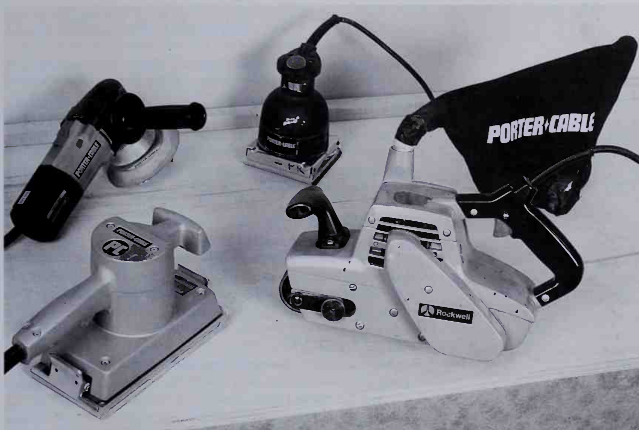
Common electric sanders include (clockwise from front left) a half-sheet orbital sander, a random orbital disc sander, a palm sander and a hand-held belt sander.
