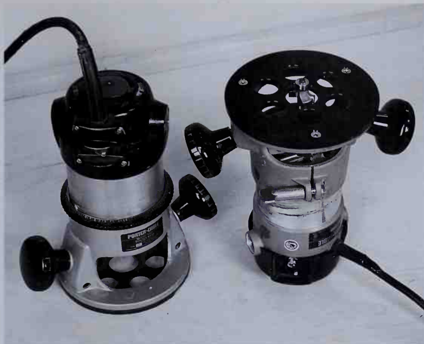
Routers are used for a wide variety of woodworking operations, including edge shaping, flush trimming and mortising.
