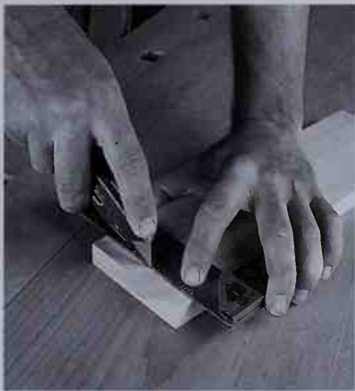
Mark the tenon shoulder across one face of the board with a knife.
