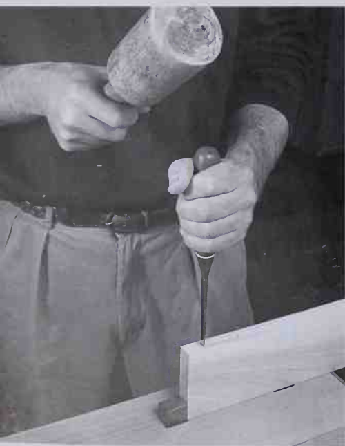
Chop down into the wood just shy of the mortise ends.
