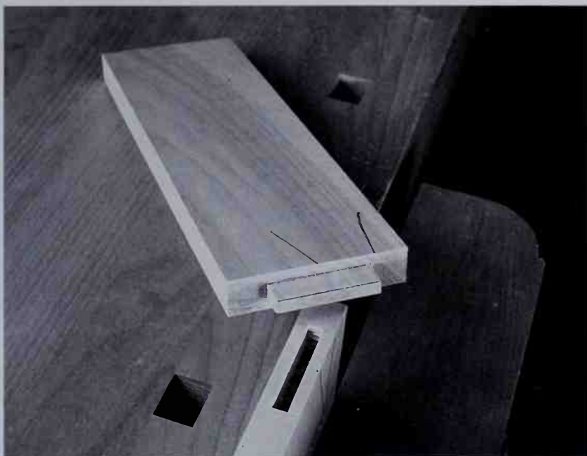
The completed mortise and tenon.
