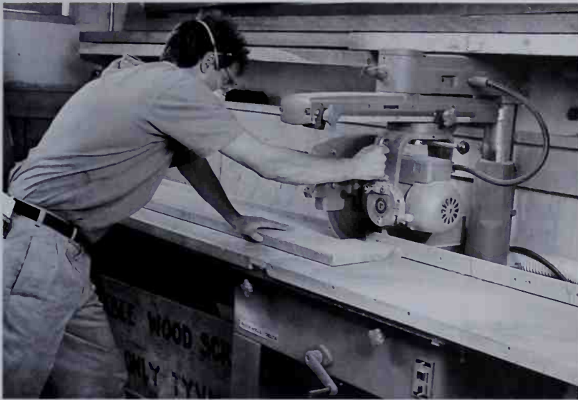
Side-extension tables make the radial-arm saw safer and easier to use.
