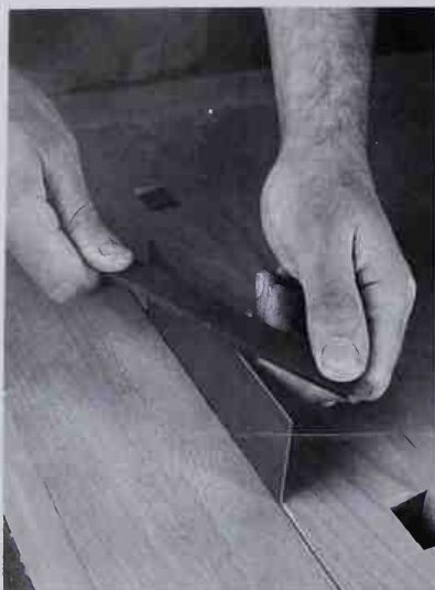
With the scraper held firmly in the shoulder vise, file the edge with a mill bastard file.
