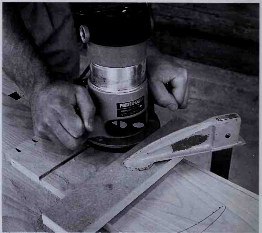
To cut the shelf groove with a router, run the router against a clamped fence.
