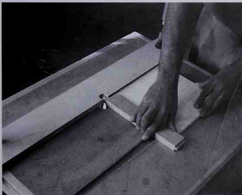
The tongue on the end of the mounting piece can be made on a router table. The square push block keeps the narrow mounting piece steady as it passes the cutter.
