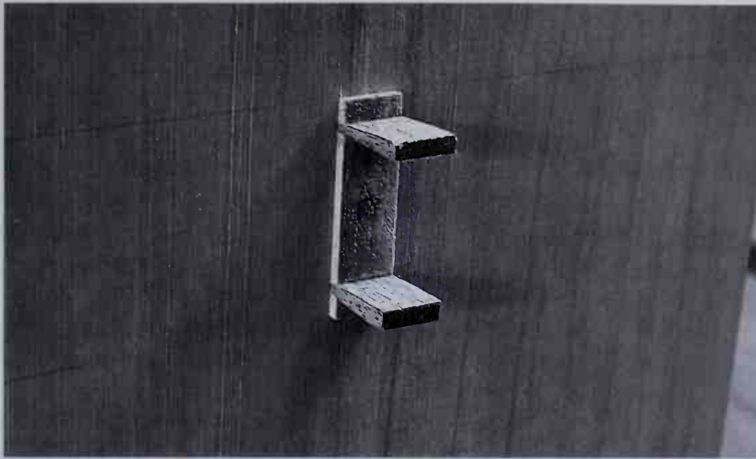
The wedged tenon will be trimmed flush once the glue has dried.
