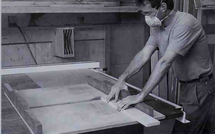
A miter gauge (left) or a sliding table (above) should always be used when crosscutting on the table saw.
