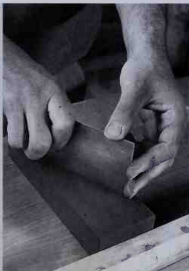
Smooth the edges of the scraper on a medium-grit stone first (as shown) and then on a fine stone.
