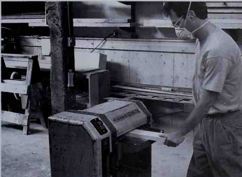
A thickness planer creates a second face parallel to the first.
