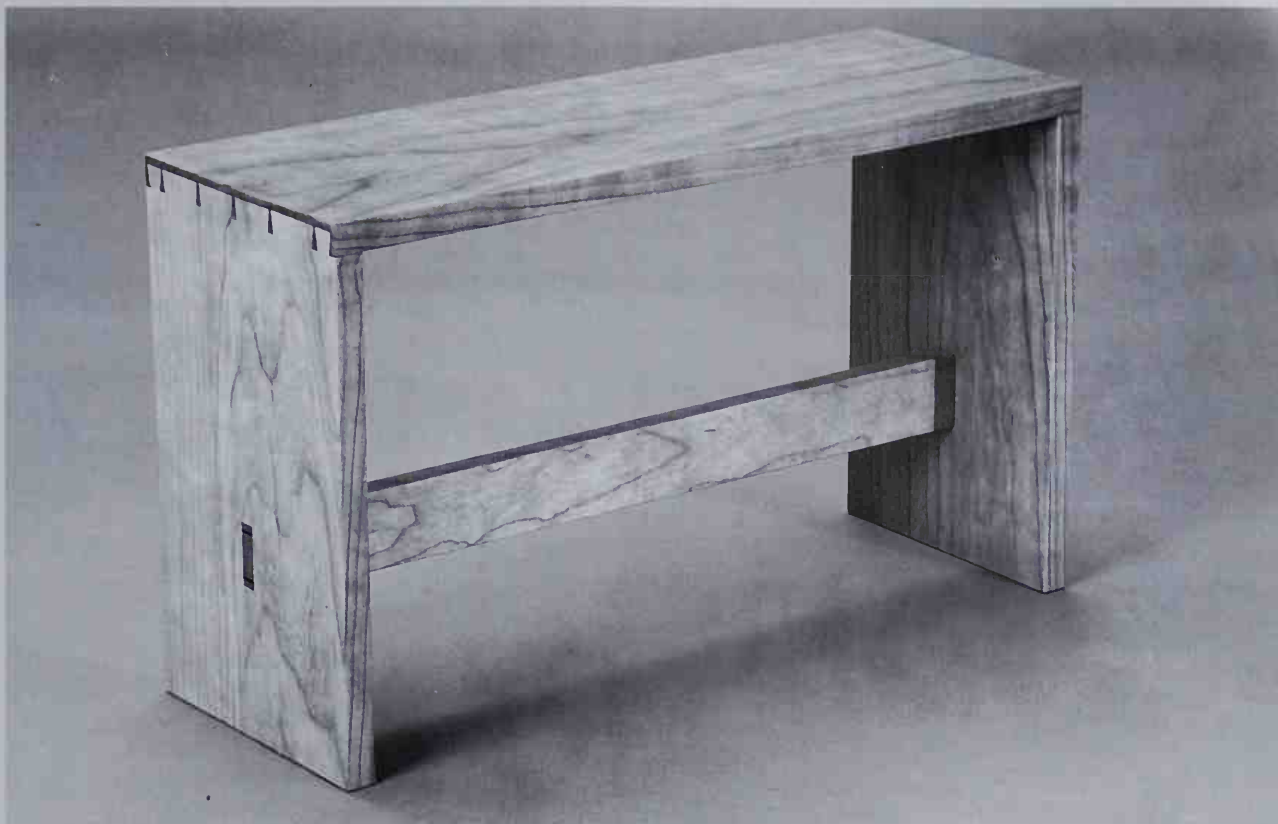
The completed bench.
