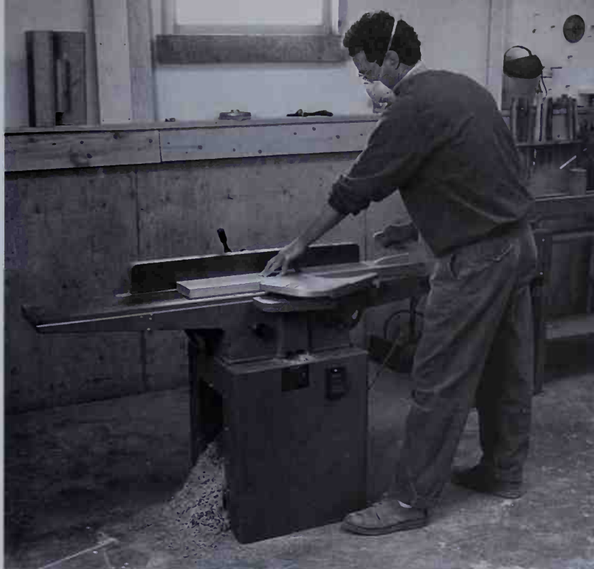
The jointer is used to establish a flat face and perpendicular edge.
