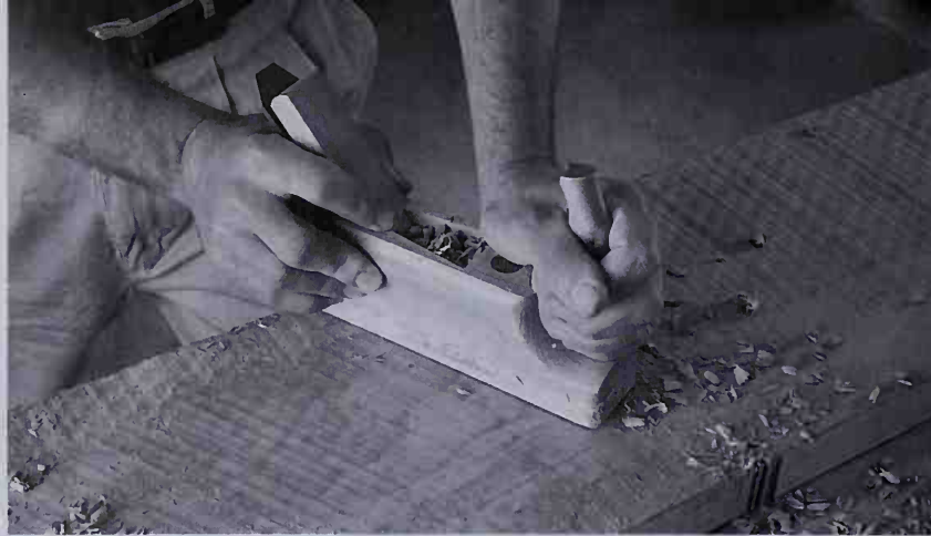
Plane the first face flat, starting with a scrub plane, if necessary (as shown).
