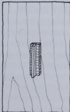
Wrong way: Wedge exerts pressure against edge grain of mortise.
