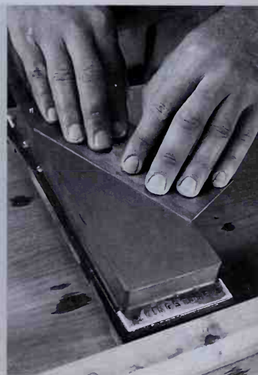
Polish the sides of the scraper on a fine stone.
