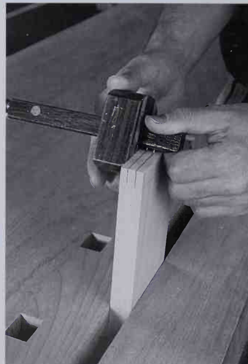
Scribe the tenon thickness from shoulder to shoulder with the mortising gauge.
