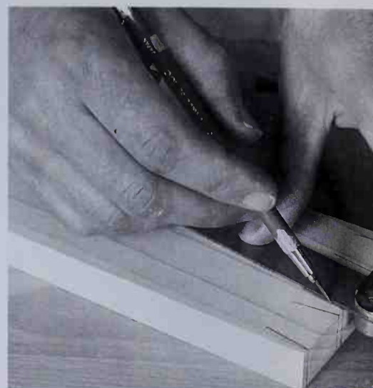
Use a sliding T-bevel and pencil to lay out the tails.
