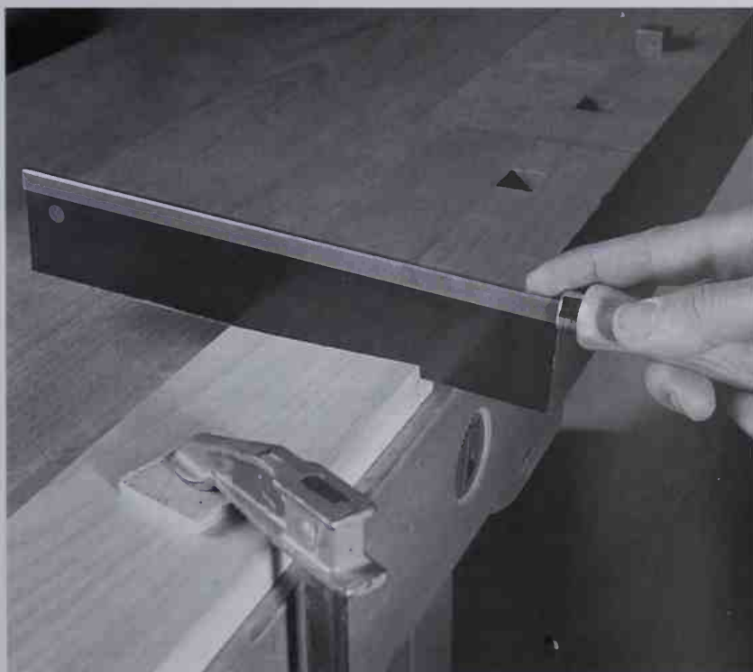
Starting at the near corner, saw the tenon shoulders on the diagonal.
