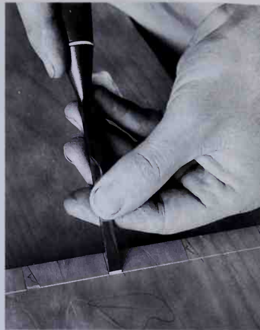
Pare back to the shoulders between the tails.
