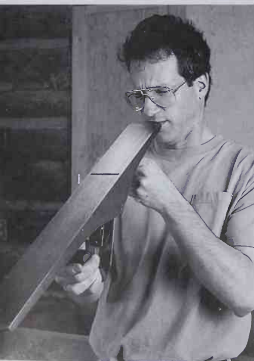
Sight down the jointer plane and set the blade parallel to the sole.
