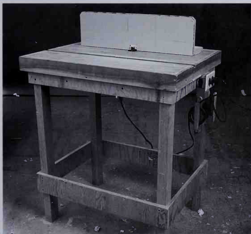
Router table with fence. A table-mounted router allows greater control than a hand-held router.
