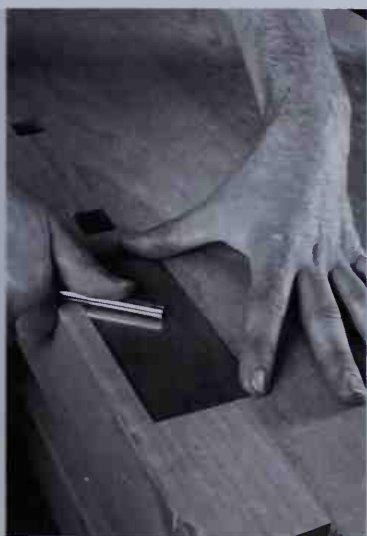
Pull off the burr with a burnisher held flat on the scraper.
