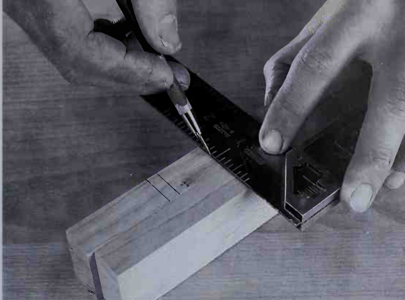
Transfer the mortise locations from one door stile to the other.
