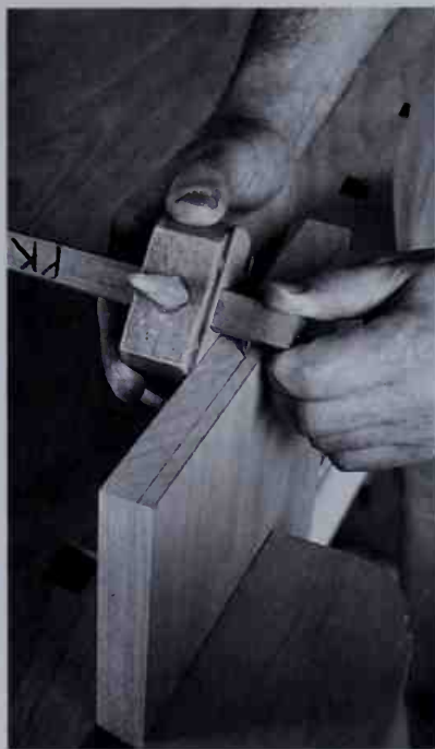
Scribe pin depth with the marking gauge.
