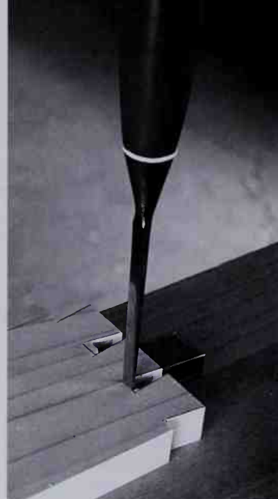
With a sharp chisel, chop the tail shoulders square.
