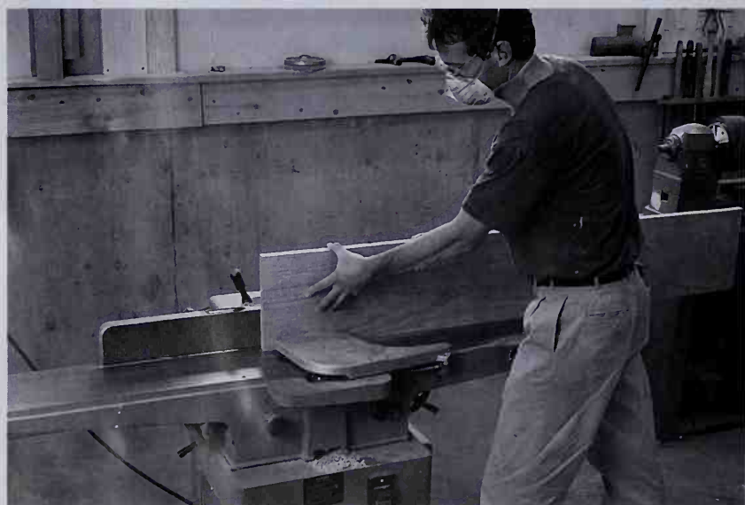
Joint one edge of the board square to the first face.
