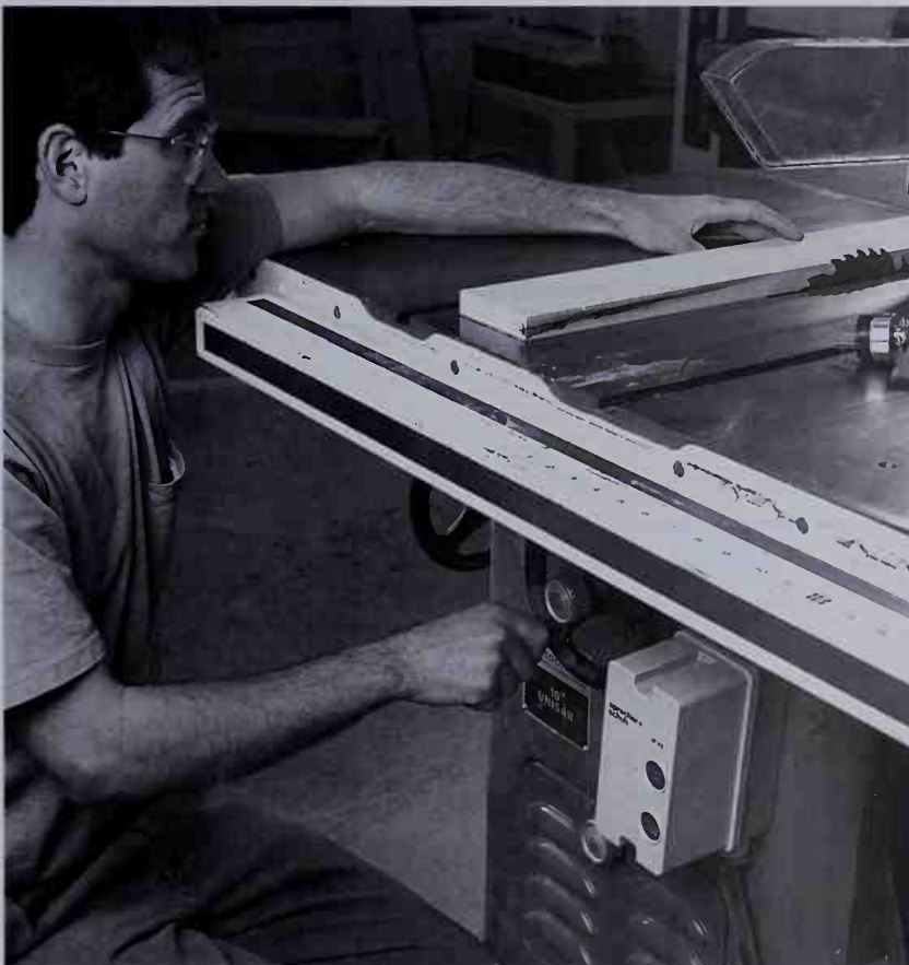
Set the sawblade a tooth higher than the thickness of the wood.
