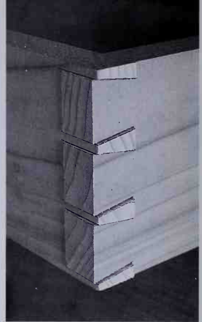
The assembled dovetail joint, before being trimmed flush.
