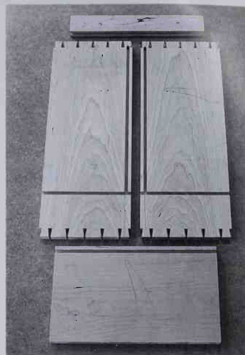
The cabinet mounting piece, sides and shelf with grooves cut.
