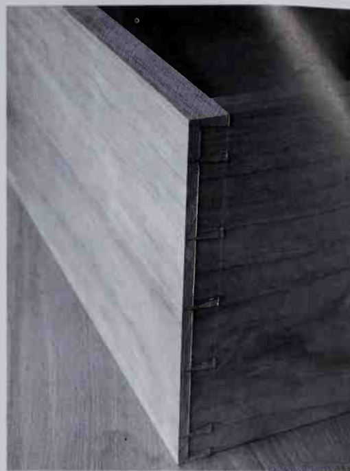
The assembled joint will be cleaned up after the bench components have been glued together.
