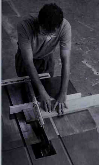
A miter gauge (left) or a sliding table (above) should always be used when crosscutting on the table saw.
