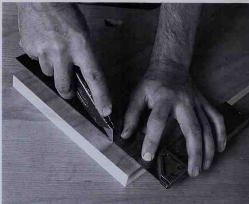
Mark the shoulders for the pins on the bottom side of the bench.
