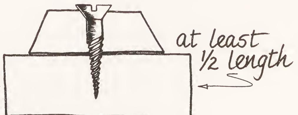
ness. (Not a full range, though; #2 screws come in  $\frac{1}{4}$ - and  $\frac{1}{2}$ -inch lengths, and #7 in  $\frac{1}{2}$ -to- $1\frac{1}{2}$ -inch lengths, and #16 in  $1\frac{1}{4}$ -to-3-inch lengths, for example.)
