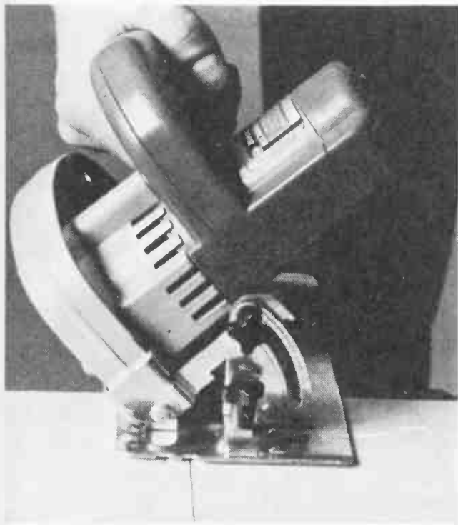
You can make angled cuts simply by tilting the sole plate
