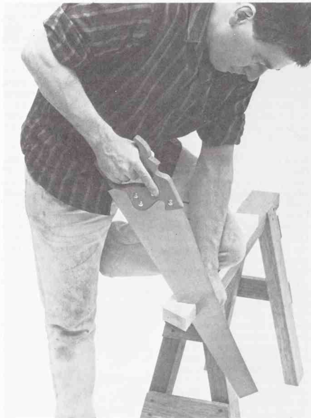
Left: the coarseness of a saw blade is measured by the number of teeth per inch of blade
