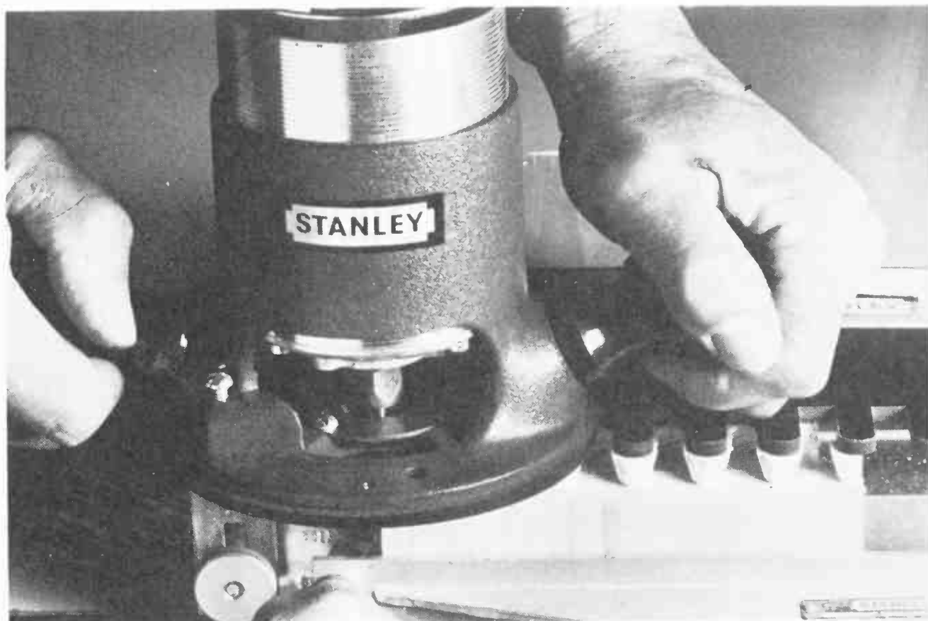
Using its special dovetailing attachment, the router makes light work of cutting perfectly matched dovetail joints
