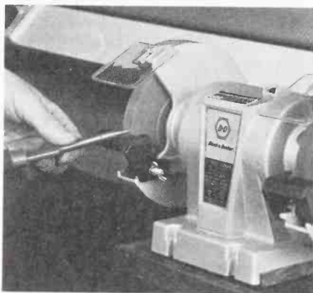
Right: regrinding chisel and plane blades is easy with a bench mounted power grinder
