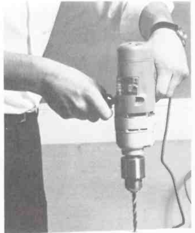
Use the detachable side handle to keep the drill vertical here
