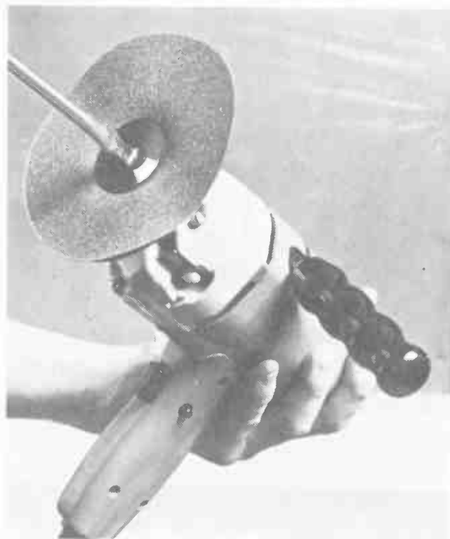
Circular sanding disks are held in place by a washer and screw
