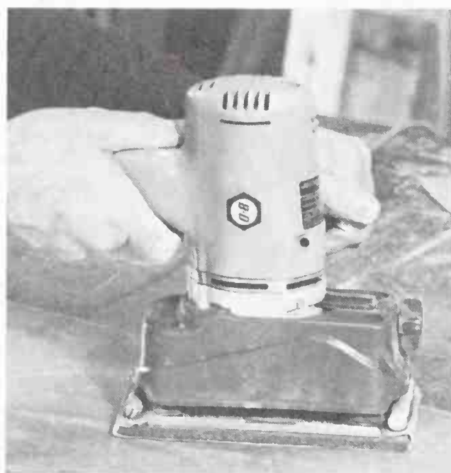
You can fit an orbital sander attachment to your power drill . . .
