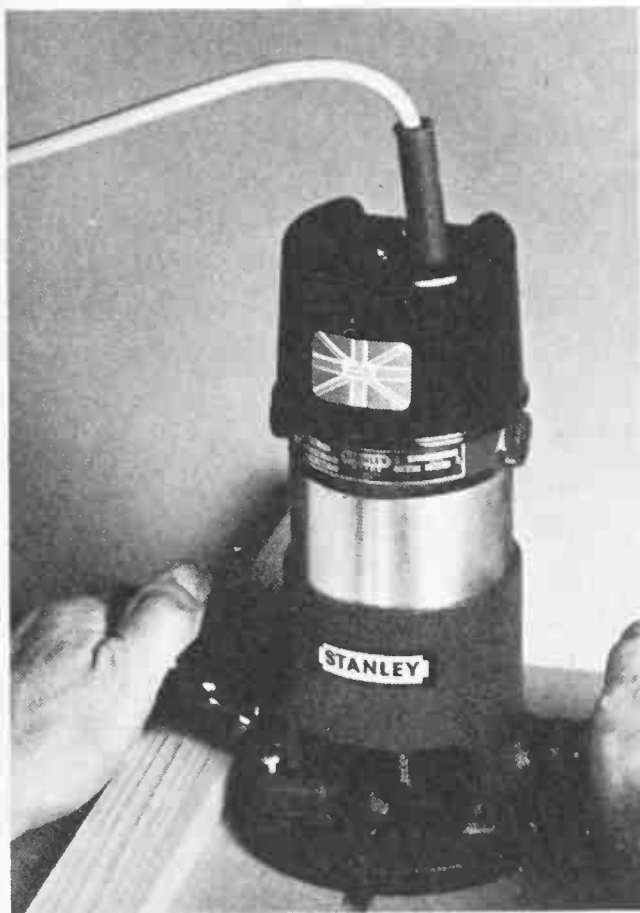
The power router will cut grooves in a variety of shapes and sizes
