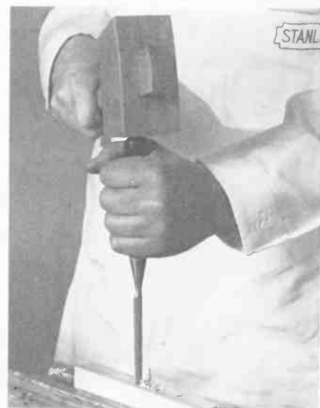
Using a wooden mallet and chisel to chop out a mortise
