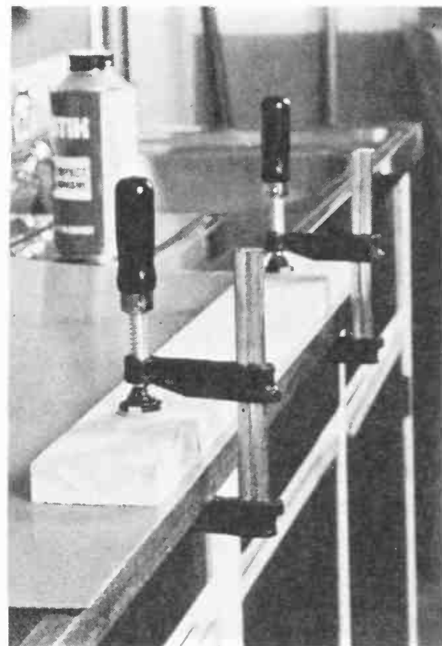
These quick action clamps are perfect for clamping plastic laminate in place on a worktop, and also for holding workpieces on the bench. The movable jaw slides freely along the stem, but is locked against it when the turn screw is tightened on the surface of the workpiece
