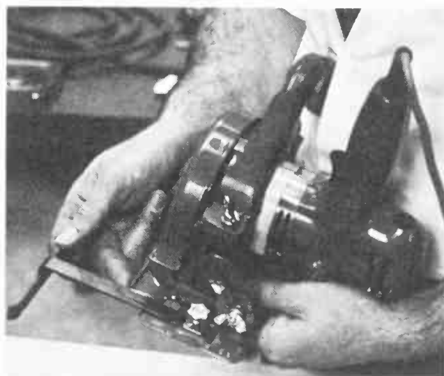
An adjustable fence makes accurate cutting much easier
