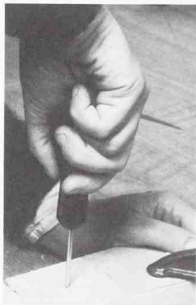
The bradawl is used to make starting holes for screws too small to warrant the drilling of pilot and clearance holes (page 89). It is used with a side to side twisting action
