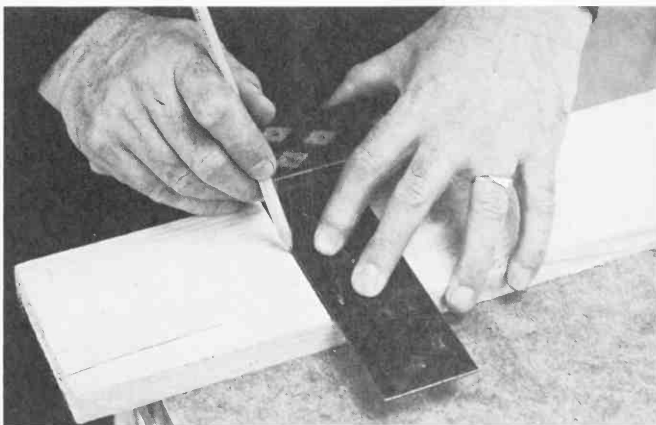
Use a try square with the stock pressed firmly against the edge of the wood and the fingers pressing down on the blade
