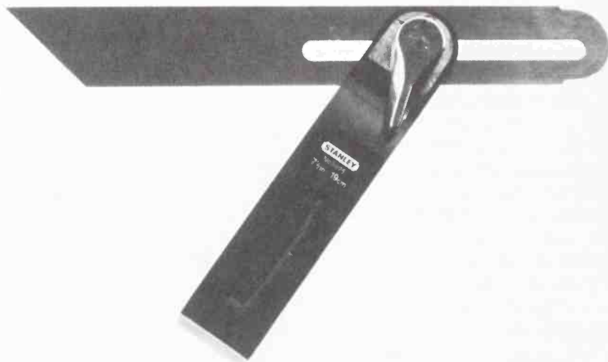
The sliding bevel is an adjustable square used for marking angles of any size
