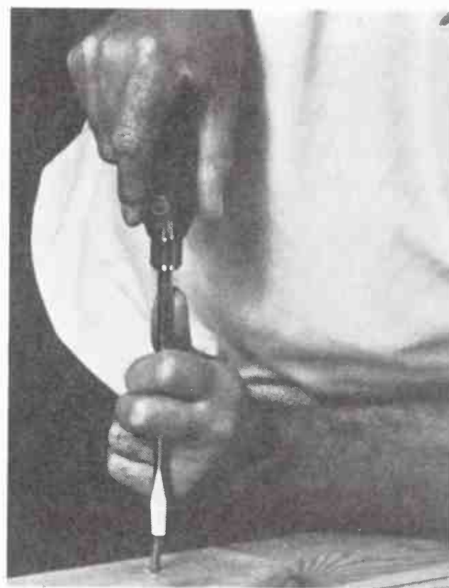
Hold the blade with one hand while the other turns the screw
