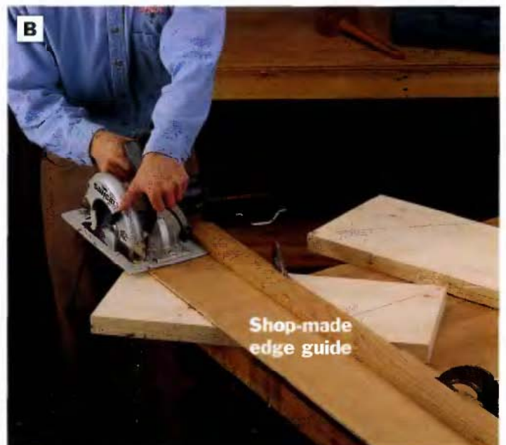
PHOTO B: Gang-cut the carcass top and bottom panels to size, then gang-cut the fixed shelves. Use an edge guide clamped to the workpiece and your workbench to ensure straight cuts.
