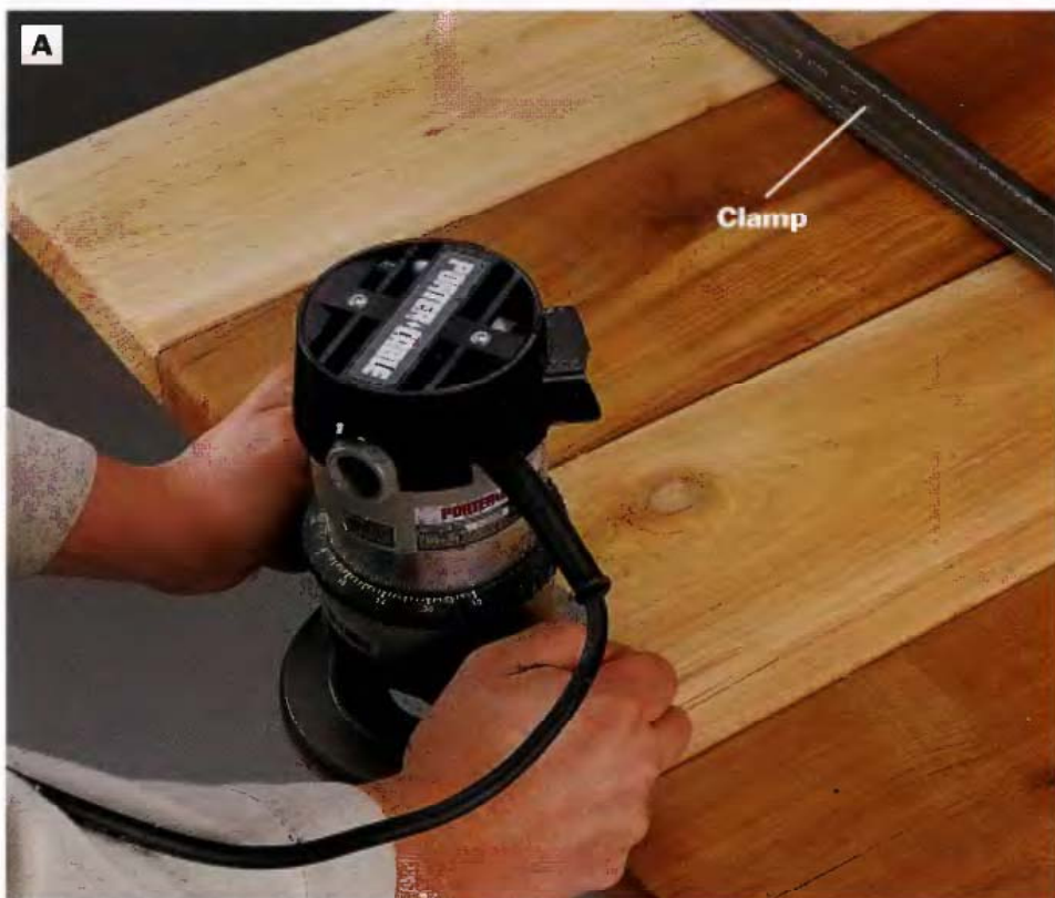
PHOTO A: Clamp the tabletop slats together and rout the ends and edges with a 1/2-in. roundover bit. Clamping the slats together will produce an even profile on the ends of the slats.
