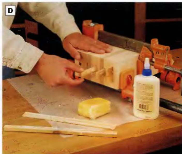
PHOTO D: After your clamps have squeezed the excess glue from the assembly, but before the glue starts to set, remove the wax-coated filler strips in the knife slots. Once the glue dries, sand the block smooth.
