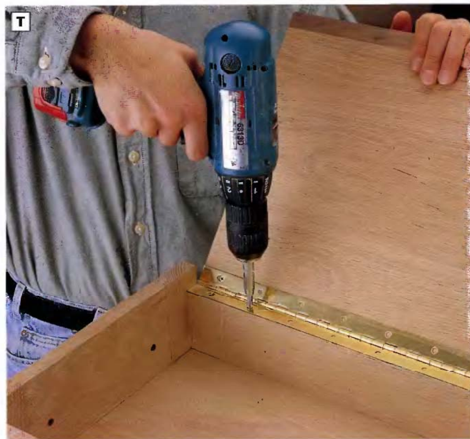
PHOTO T: Dry-fit the lid by attaching the piano hinge with one or two screws in each end and another in the middle. Remove the hinge, once you're satisfied that everything fits together, and reattach it after the finish is applied.
