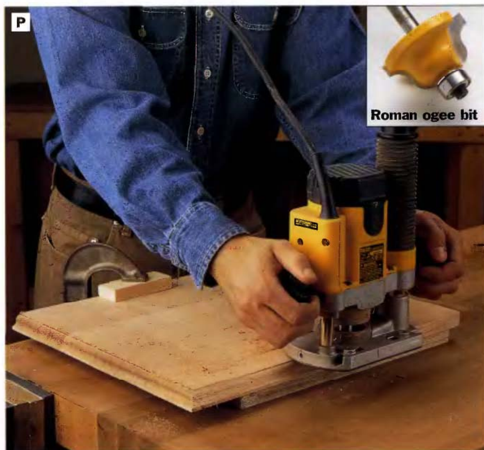
PHOTO P: Clamp the top panel to the workbench and use a Roman ogee bit to rout a profile around the side and front edges. Insert scrap plywood between the benchtop and the top panel to give clearance for the bit's pilot bearing.
