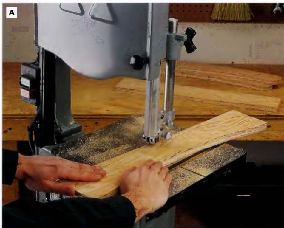
PHOTO A: Lay out and cut the four table legs on the band saw or with a jlg saw. Since the profiles of the legs match, mark and cut one to serve as a template for tracing the profiles onto the other three leg blanks.
