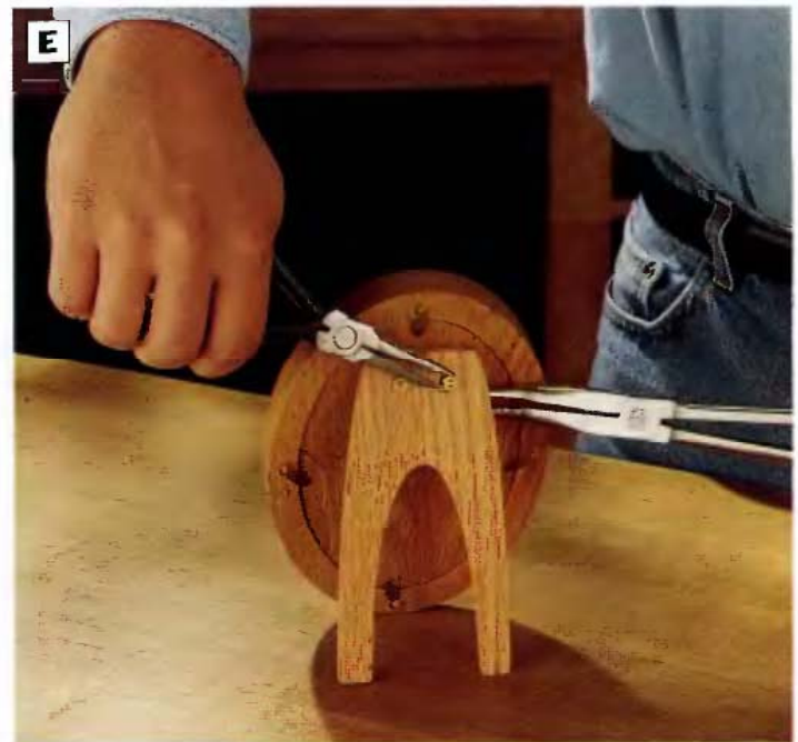
PHOTO E: After locating the hinge position, mount the hinge to the frame back with #4 × 1/4-in. brass flathead wood screws. Fasten the hinge to the stand with bolts and nuts. Arrange the bolts so you can thread the nuts on from the back of the stand. Tighten the nuts and bolts with a pair of needle-nose pliers.
