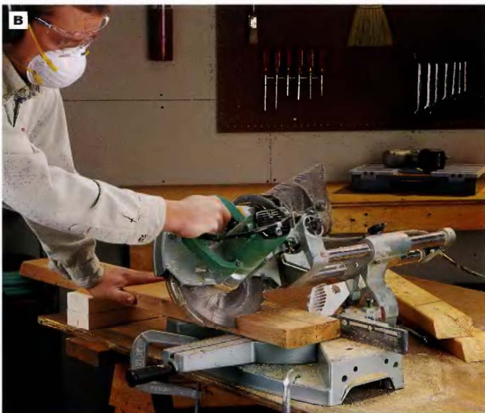
PHOTO B: Bevel-cut the ends of the outer and center table stretchers at 30° angles. We used a power miter box, but you could also make these cuts with a circular saw or a table saw.
