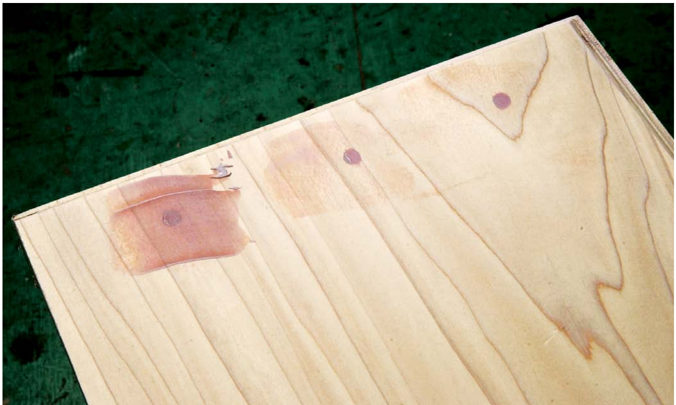
Properly sanded filler (right) shows a sharp delineation between the filled spot and surrounding wood. The hole on the left hasn't been sanded at all; the one in the middle hasn't been sanded enough.
