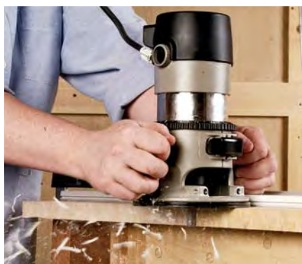
Straighten a wavy edge.
