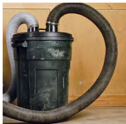
A trash can with a special lid keeps big chips and debris from damaging the fan blade.
