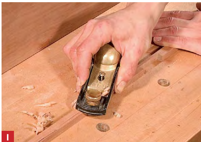
I Planed to perfection. Don't try to get a perfect-fitting strip straight off the tablesaw. Rip the strip slightly wider than you need, then plane to fit.
