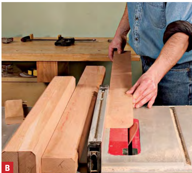
B Precut corners. Instead of overworking your router, or wasting time repositioning the bit or fence to make multiple cuts, set your tablesaw to 45° and slice off the outside corner before routing.
