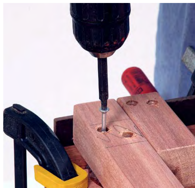
A simple jig made from leftover 2×2s (on the right) accurately positions the uprights (on the left) and holds them in place while driving the screws.
