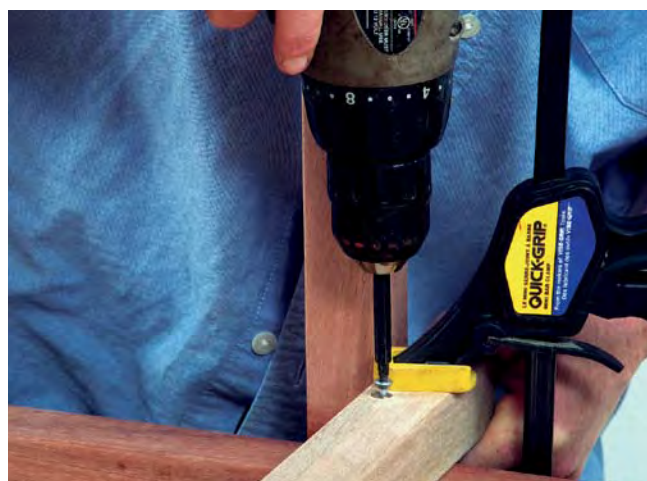
Glue-and-screw joints are easy to construct and make this chair redundantly strong.
