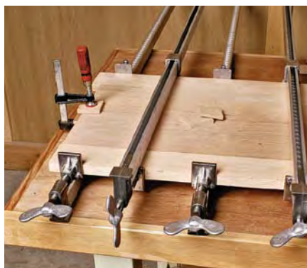
Panel clamps help keep glue-ups flat.
