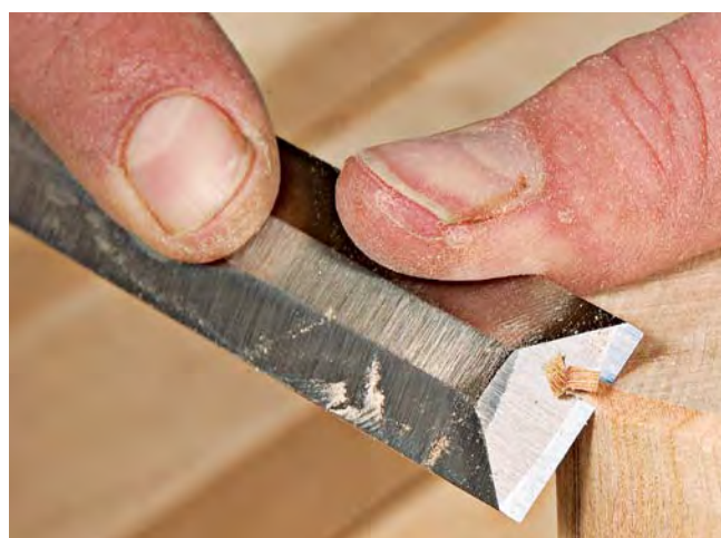
Make your own mark. Hand-cut details, like chamfered edges, add visual and tactile interest that you can't get from power tools.
