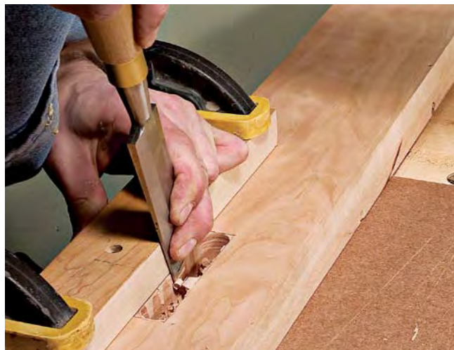
Chop to it. Drilling out most of the mortise and paring up to the line is easy to master, and easier on your chisel than chopping with a mallet.
