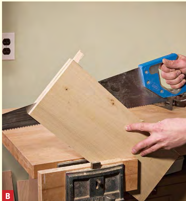
B Finish by hand. A handsaw is a safer and more controllable way to finish narrower boards. Insert a wedge in the kerf so the board doesn't pinch the blade.
