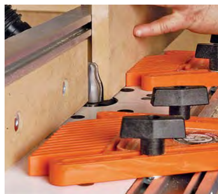
A vertical bit creates the raised field of a raised panel.
