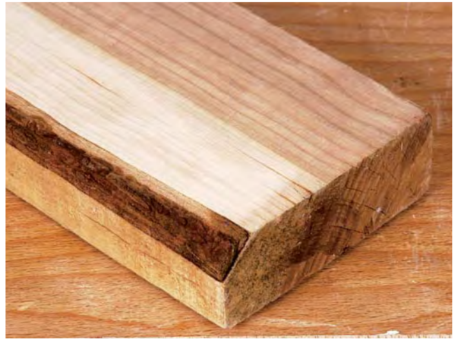
The sapwood near the edge of this cherry board is not only different in color but also less stable.
