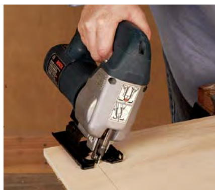
Tilt the blade to the right or left.
