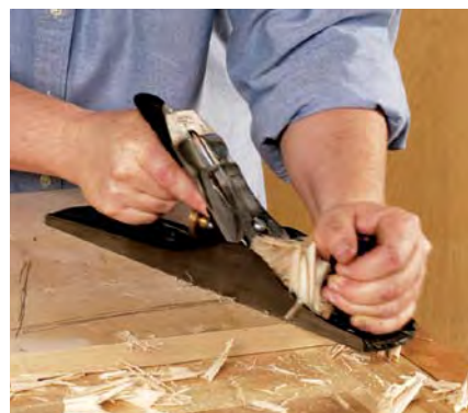
Remove bumps and hollows to make a surface level.
