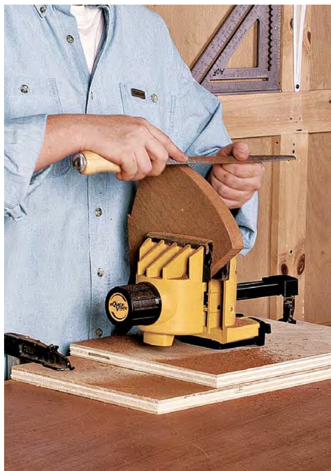
A portable vise can be easily clamped in place to hold small complex workpieces at a convenient height for fine work.
