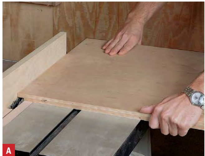
Rabbet the top and bottom. To rabbet the edges of the top and bottom, install a dado head set to \frac{3}{4} " and run the auxiliary tablesaw fence almost flush to the blade.
