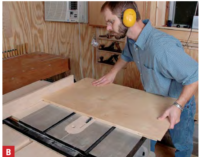
Dado for the divider. Shift the fence and set it to cut a dado down the center of both the top and the bottom.
