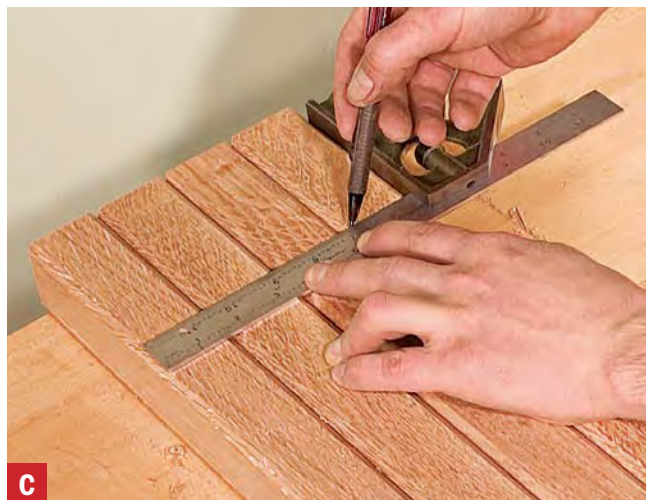
C Measure once, then mark all four at once. When marked off in one swipe, the legs won't be off even the width of a pencil line.
