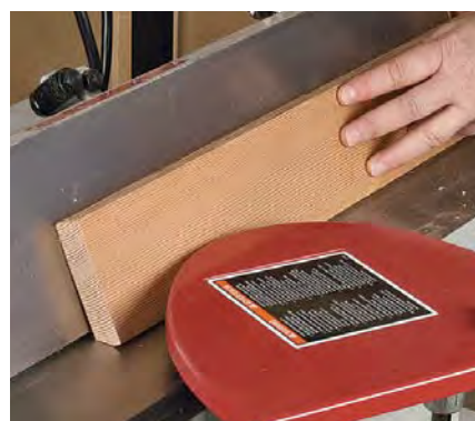
Angle the fence to bevel the edge of a board.
