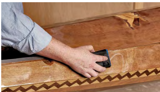
A sanding block helps retain flatness.
