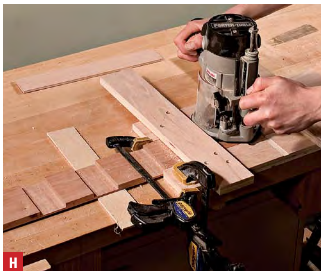
Mortises made easy. Make the "mortises" for all four rails at once by using your router and the wide dado jig.
