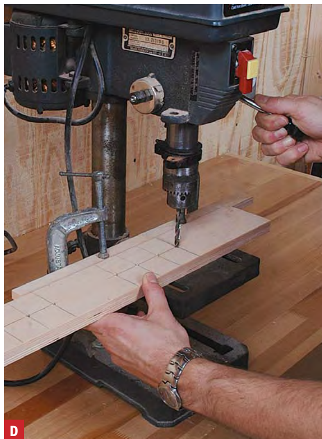
D Make the guide. Use either a drilling guide or a drill press to drill 90° holes spaced 1\frac{1}{2} " apart and centered on the guide.
