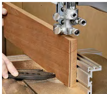
Cut thick pieces to thin.
