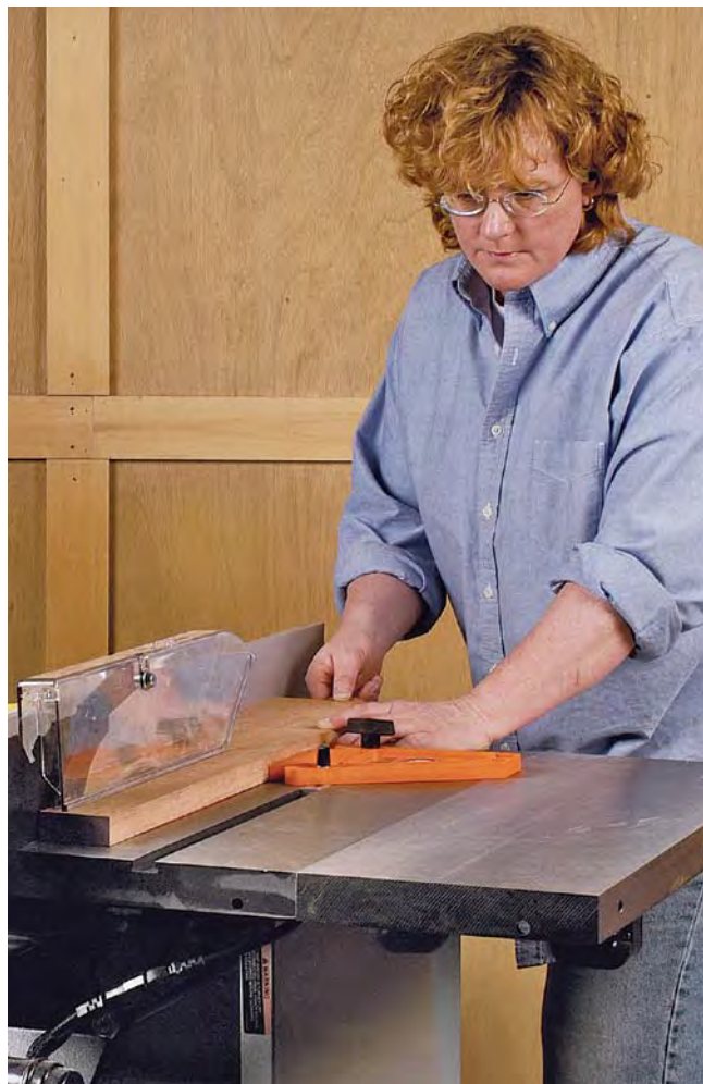
Stand to the left of the blade when ripping and use featherboards to hold the board against the fence. Feed the board steadily, pushing against the fence just behind the blade.
