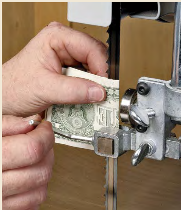
Set the guides. A folded dollar bill is an inexpensive alternative to a feeler gauge for setting the correct distance between guides and the blade.
