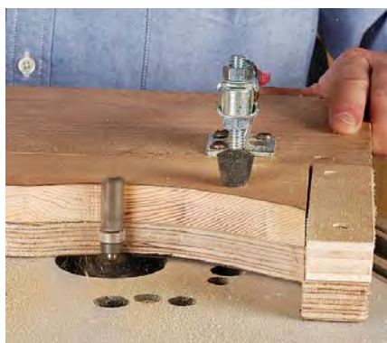
Cut to a template using a bearing-guided router bit.
