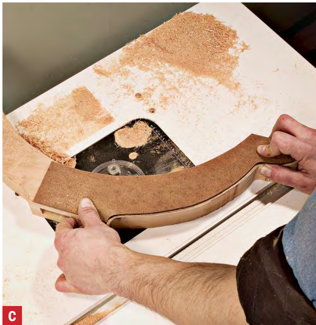
C Double-duty template. Made from \frac{1}{4} "-thick hardboard, the template used to trace the legs can also serve to guide a bearing-topped 1\frac{1}{2} "-long flush trimming bit. When routing, make only light cuts.
