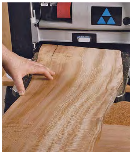
With the jointed face down, plane the top smooth.
