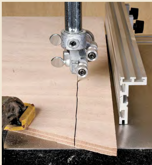
Reset the rip fence. Each time you change the blade, you'll have to adjust your rip fence to match the blade's cut.
