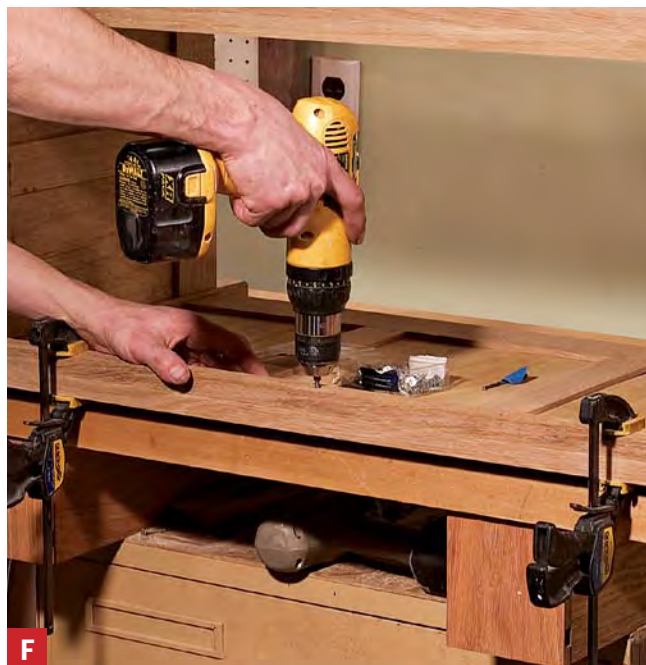
F A cleat to hold on to. Screw a pair of cleats to the bottom edge of the lower front and back rails. Use clamps to hold the cleat flush to the bottom edge as you screw it in place.
