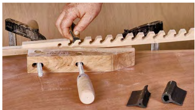
Profiled rubber sanding forms aid sanding in tight spots.
