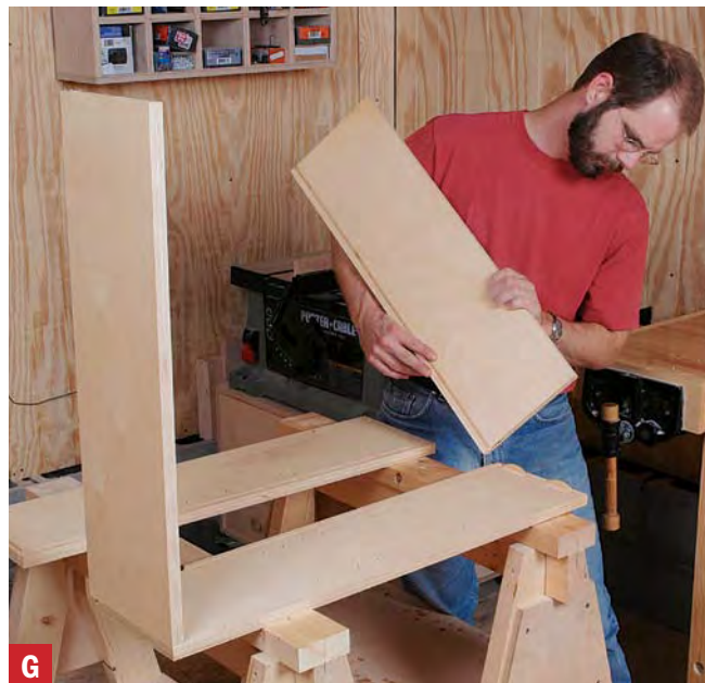
G Set the ends in place. With one side of the cabinet laying across sawhorses, add glue and biscuits, then set the top and bottom in place.
