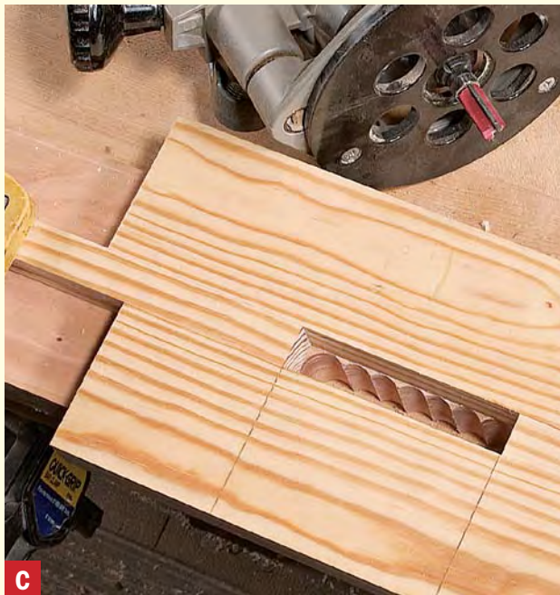
A solution for multiple mortises. When you have more than a few mortises, consider using your router and this simple jig. The bit's bearing rides against the wood while the carbide cutters clean out the mortise underneath.
