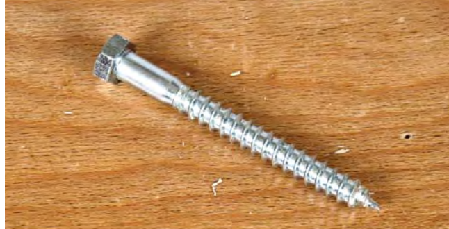
Lag screws are like coarse, long wood screws installed with a wrench. Always use a washer under the head to keep the wood around it from being crushed.
