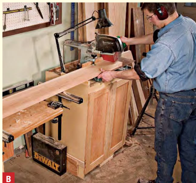
Double-duty workbench. Quick-clamping roller supports grab onto your bench or a sawhorse to support oversize stock. Use a 4' level to set the supports to the same level as the saw.
