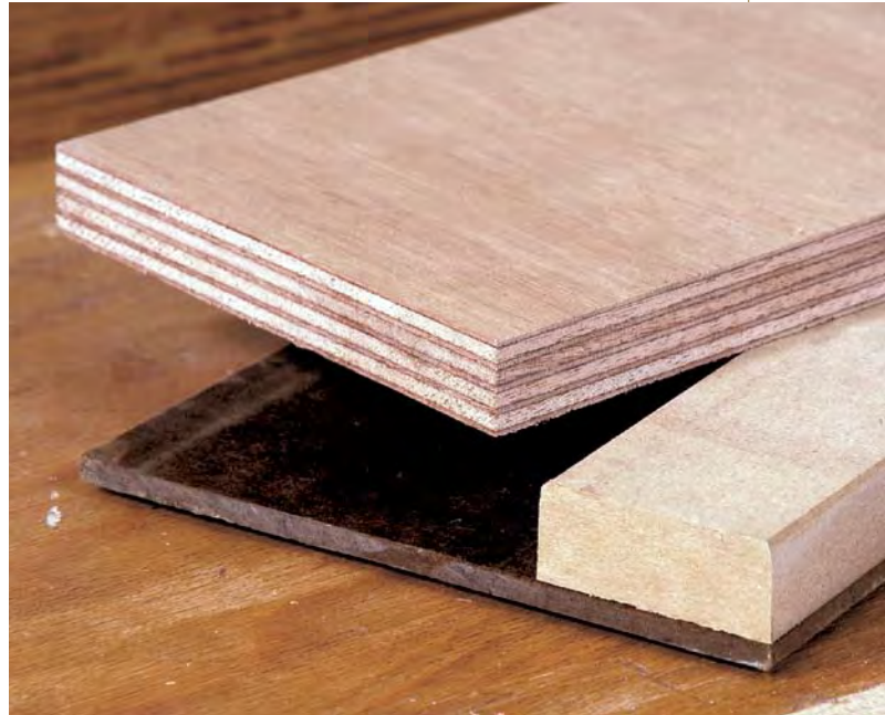
Sheet materials are dimensionally stable. Shown are a high-end plywood with many plies (top), MDF (right), and hardboard (bottom).
