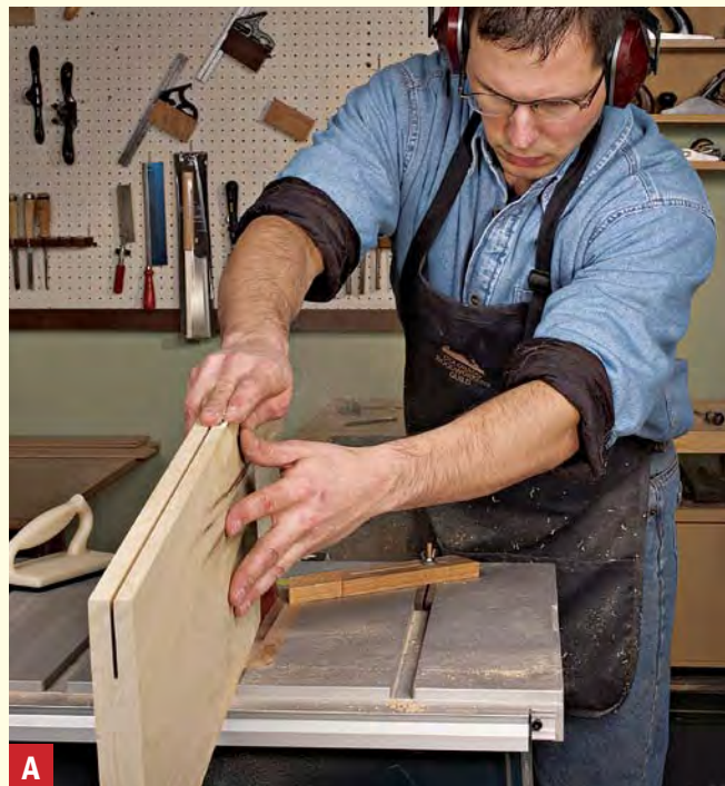
A Slicing two boards from one. Resawing on a tablesaw is slower than with a bandsaw, but with a thin-kerf rip blade, you can slice wide boards easily, even with a smaller saw.
