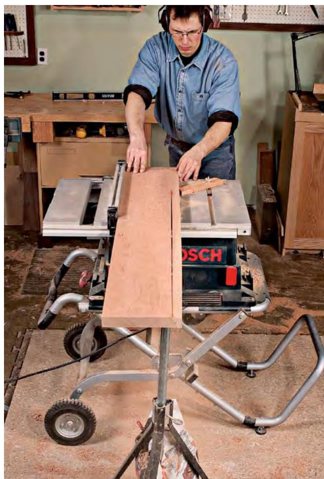
Balancing acts with benchtop tools. Learn how to safely manage long boards on small saws by providing support before, during, and after the cut.
