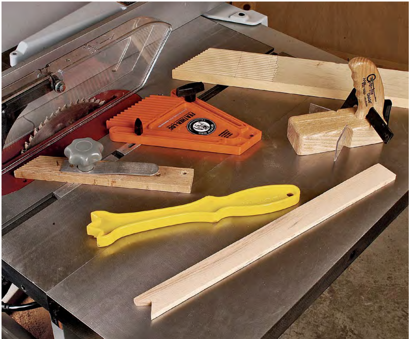
Featherboards and push sticks guide the board and keep hands from getting too close to the blade. At the far right is a shopmade push stick. To its left is a plastic push stick. Aligned in the slot are a selection of featherboards: a wooden single-lock featherboard, a more secure double-lock variety, a shopmade featherboard that clamps to the table, and a magnetic featherboard.
