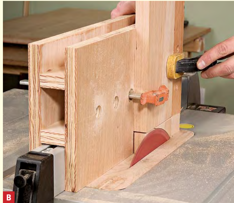
B Cutting the cheeks. The tenoning jig rides on your saw's rip fence so that the board is completely supported through the cut. For big boards, two clamps are better than one.
