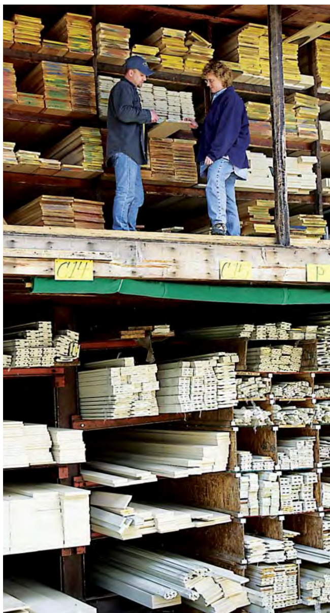
Whereas structural lumber is piled outside in the weather, dimensional lumber is kept dry and out of the sun.
