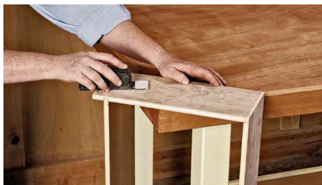
A corner can serve as a vise for sanding or light planing.
