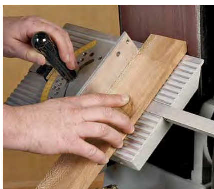
Tilt the table to sand a bevel with disk or belt.
