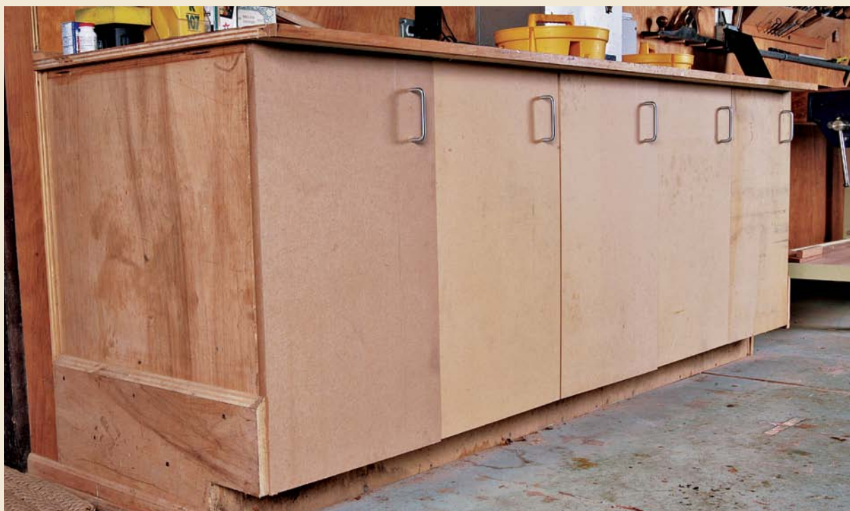
Made from \frac{3}{4} " shop-grade plywood with MDF doors, these cabinets are serviceable and sturdy. You might say they have a rugged and functional handsomeness.
