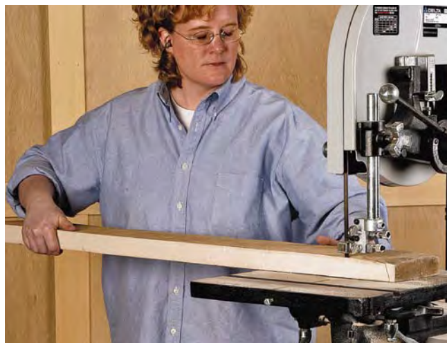
Resaw logs into lumber. The bandsaw can cut angles and curves, crosscut, rip, and resaw thick pieces of wood into thinner pieces.
