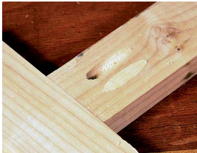
A pocket-hole screw joint is easy to make, self-squaring, and strong.
