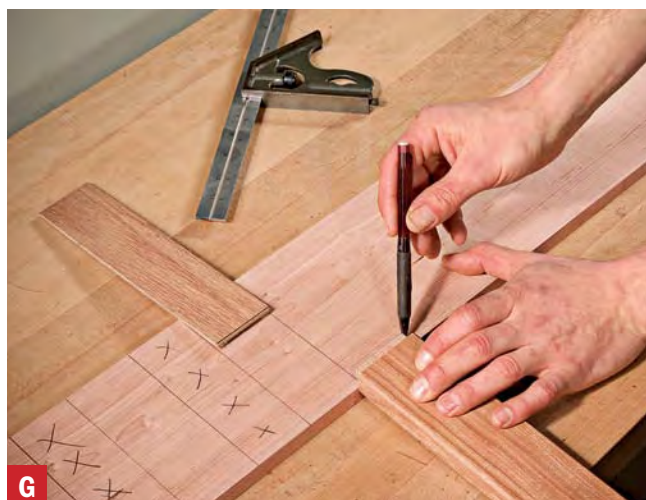
Numberless layout. Use a 2\frac{1}{2} " spacer strip and your test slat to lay out the location of the dados on your mortise strip. Use your square to extend the lines, not to measure.
