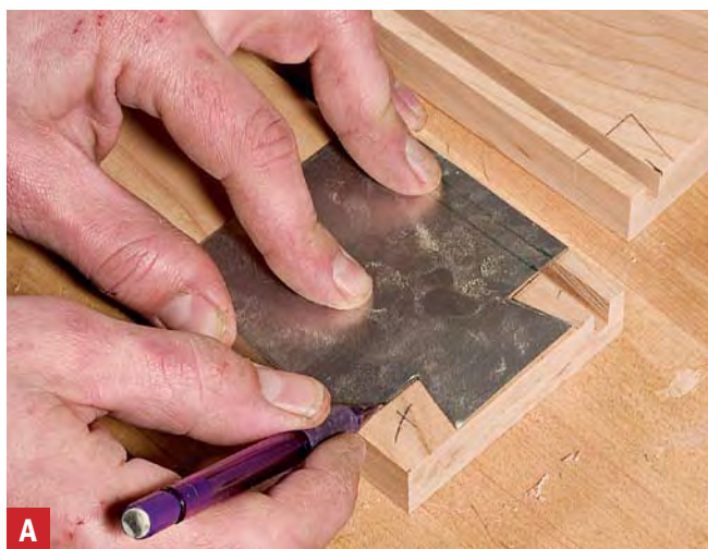
A tin tail template. Making a template from a scrap of flashing is faster than measuring out the tail on four separate ends. Note how the tail misses the groove for the bottom panel.
