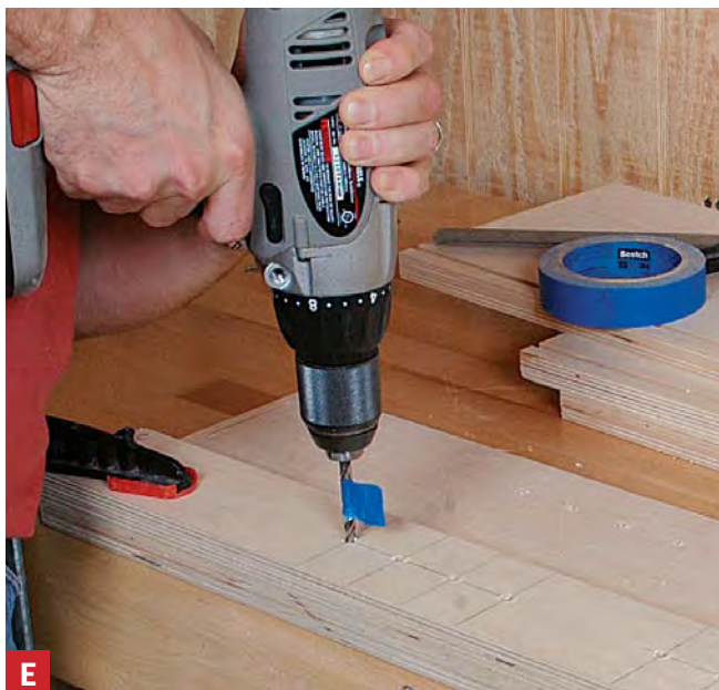
E Drill for the shelves. Clamp the guide in place against the edge of the case side. Take care not to drill all the way through the side of the cabinet.
