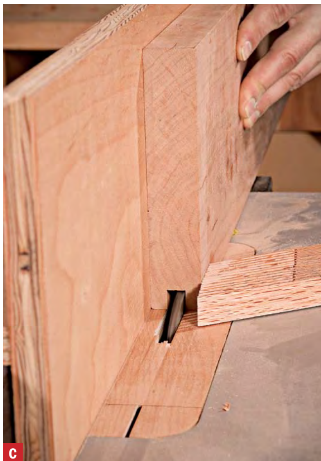
C Ready the rails for mortise strips. The mortise strips fit into a ½"-wide by ½"-deep groove. Use an auxiliary fence and featherboard at the tablesaw to prevent the rail from tipping in midcut.
