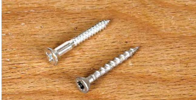
Two #8 × 1¼" wood screws: an old-fashioned screw (left) and a modern rolled-thread wood screw (right).
