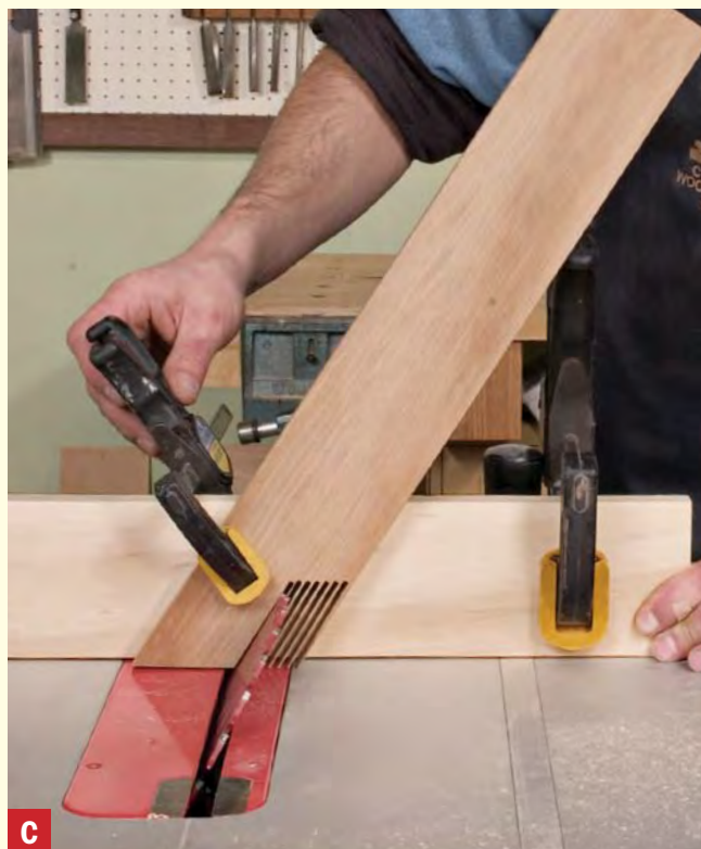
Clamps control the cut. Be sure that the clamp is safely out of the blade's path as you make the cuts.
