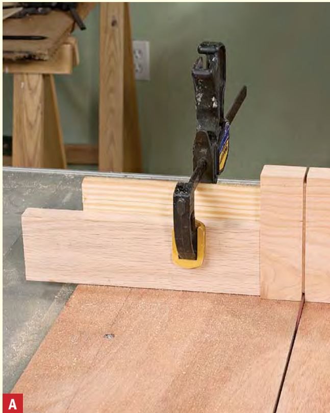
A Cutting the shoulders. A crosscut sled is good for much more than its name suggests. Adding a stop enables you to use it for cutting tenon shoulders.
