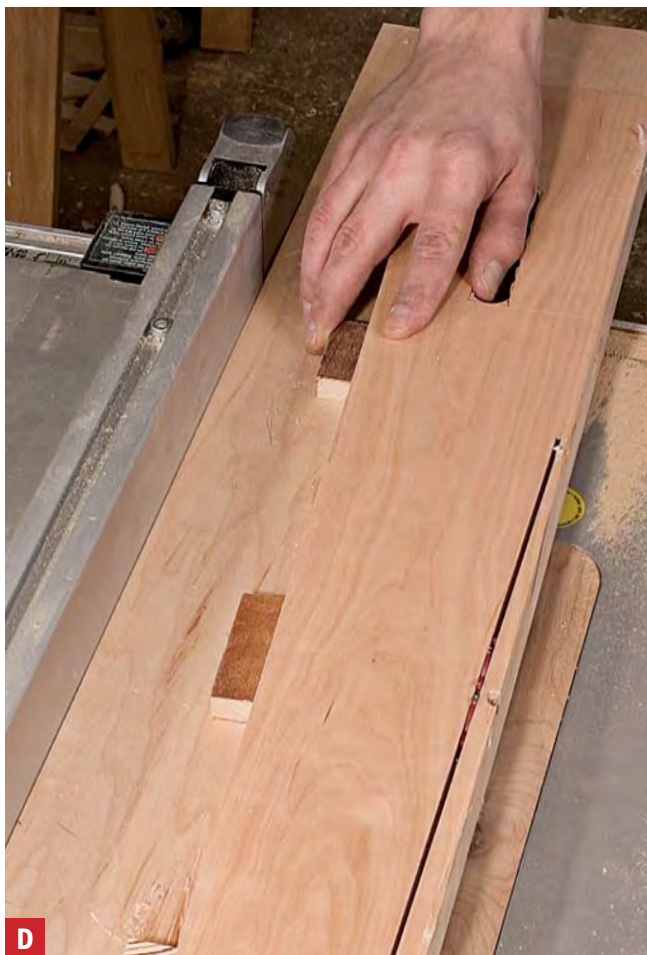
D Cutting tapers on a plywood sled. There are slicker tablesaw tapering jigs, but plywood works well enough for a few cuts.
