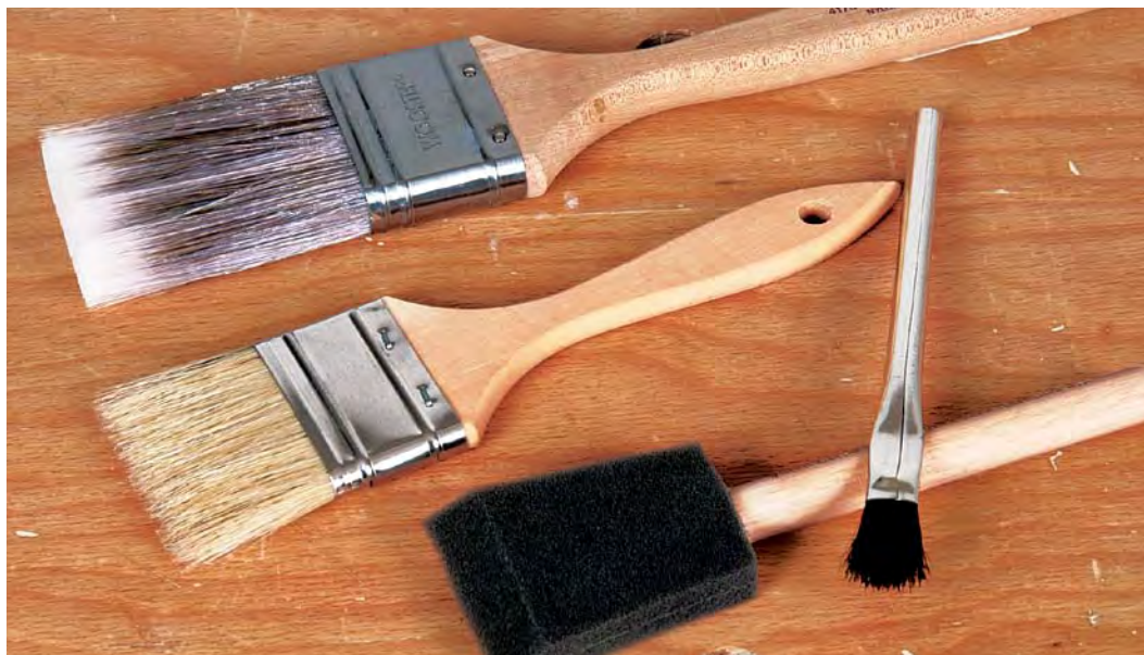
To start woodworking, you need only four types of brushes: (bottom to top) disposable acid brush, foam brush, cheap bristle brush, and moderate-quality nylon-bristle brush.
