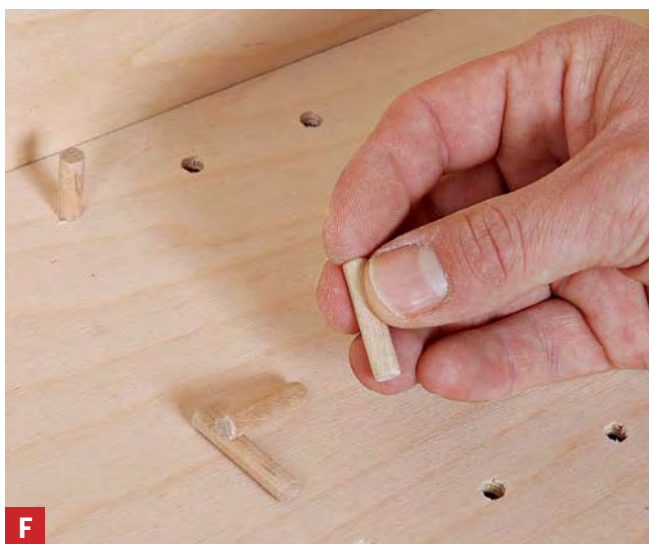
F Insert the shelf pins. Once the cabinet is assembled, insert shelf pins into the holes to anchor the shelves.
