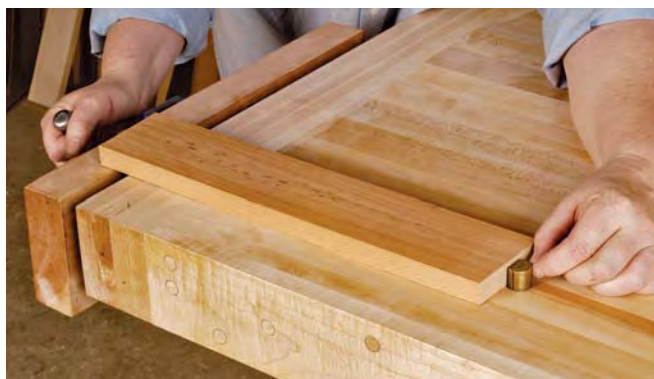
One dog acts as a stop; a second set in the cheek of a vise secures work.
