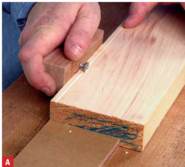
A A simple shopmade beading tool makes a decorative detail on the lower edge of the aprons.
