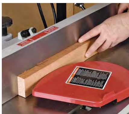
Removes bow and twist from the face edge and squares it to face side.
