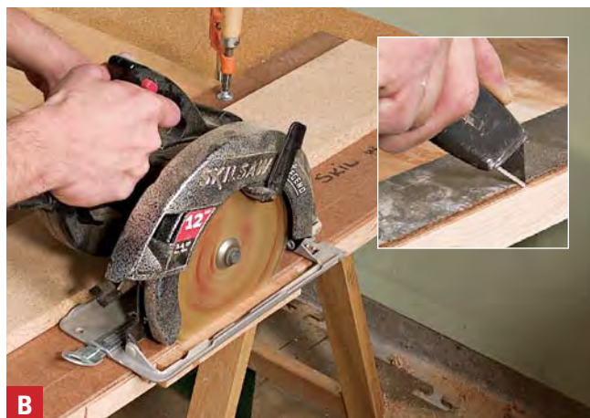
Scored then sawn. When a cut has to count, score the good face with a knife to prevent the blade from splintering the surface. Clamp both ends of the edge-cutting guide to ensure that neither it nor your work shifts in midcut.
