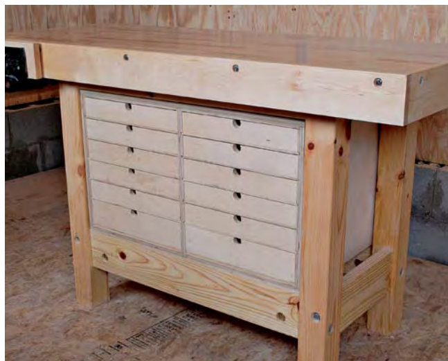
Small space, lots of storage. This drawer unit provides a dozen drawers and plenty of storage for small hand tools and supplies.
