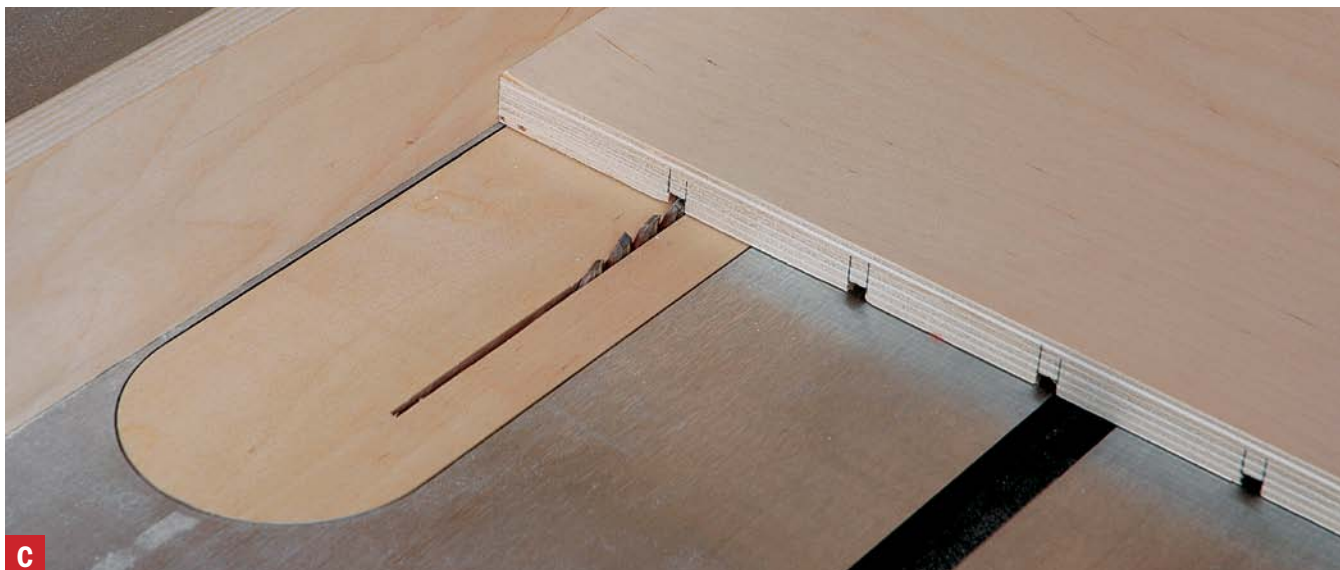
Dado using a single blade. Instead of using a dado set to make the \frac{1}{4} "-wide dado, you can simply make two passes with a single blade.
