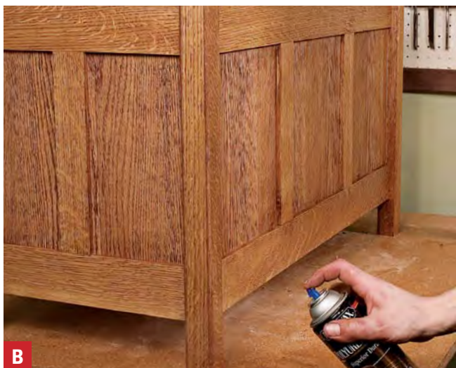
Quick spray finish. Perhaps it's not as thick as a brush-on finish, but spray polyurethane offers protection and extra color.
