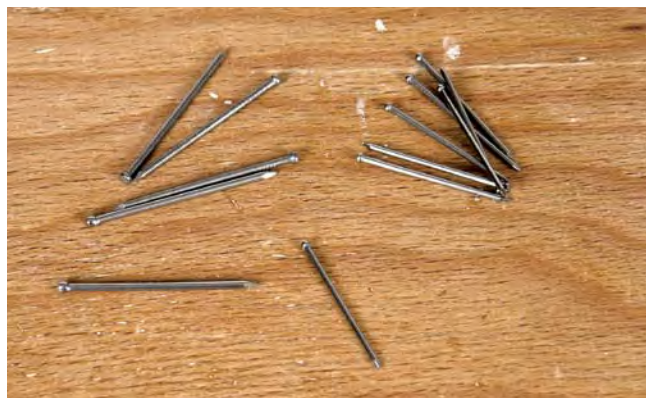
When woodworkers use nails , the nails are typically thin, small brads, or finishing nails such as these.
