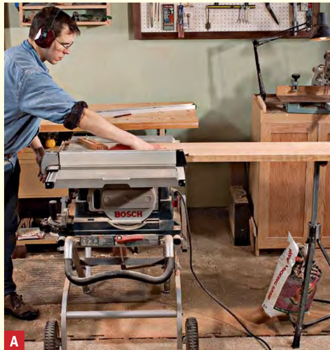
Better balanced board. Position the stand far enough away from the saw so that the board doesn't tip at the end of the cut. The sandbag ensures that the stand doesn't tip in midcut.
