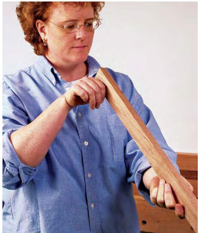
Sight down a board to check it for crook, bow, and twist.
