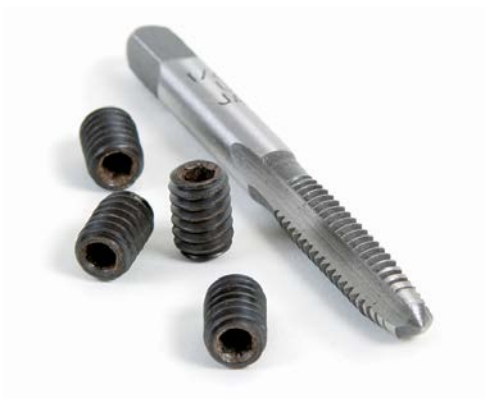
Level from above. Predrill the adjustment holes in the insert and then use a tap to make the \frac{1}{4} -20 threads in the plywood.
