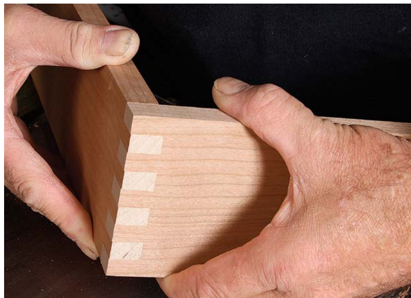
A perfect fit. When the jig is set up correctly, the cut is flawless and the joint is tight and free of gaps.
