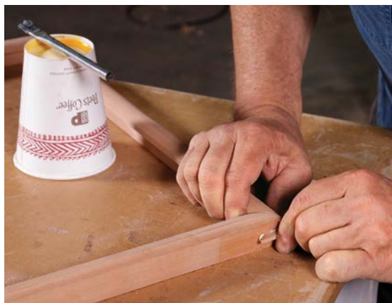
Slotting for the splines. Cullen cuts spline grooves with a slot-cutter at the router table. A piece of scrap stock cut at a 45° angle and drilled to accept clamps guides the frame through the cut.
