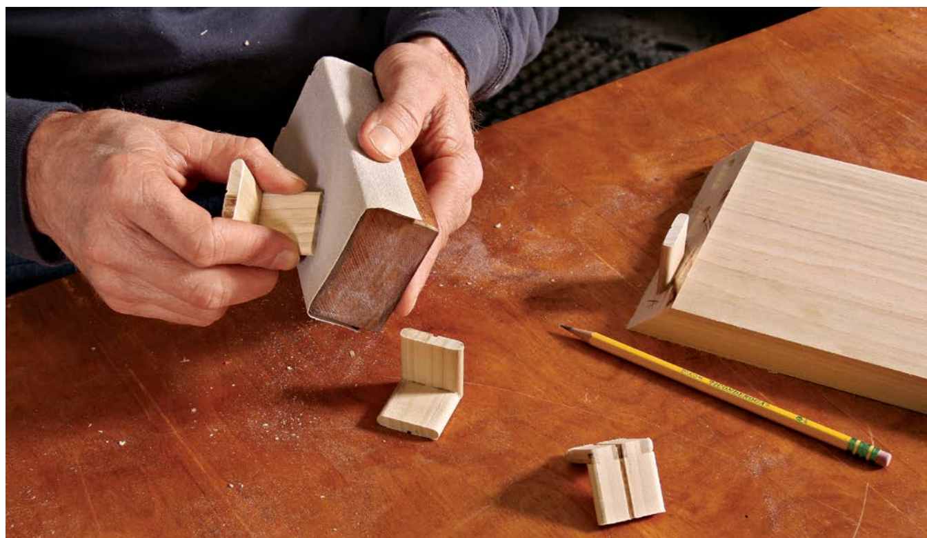
Quick chamfer. Break the edges with a few strokes of a sanding block.
