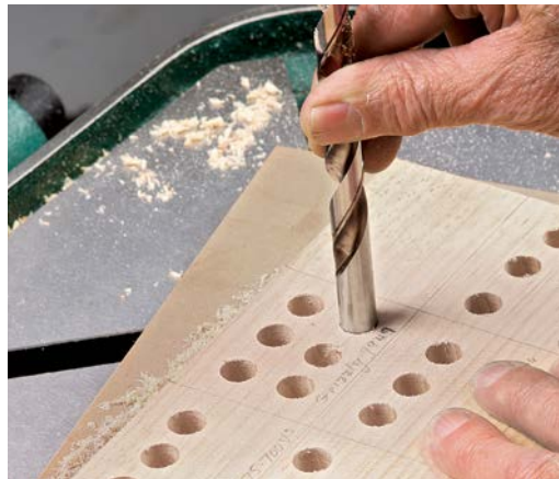
Timed test for power. Peck drilled through 2 in. of maple with a 2-in.-dia. Forstner bit. All the machines handled this tough test well, but elapsed time varied.
