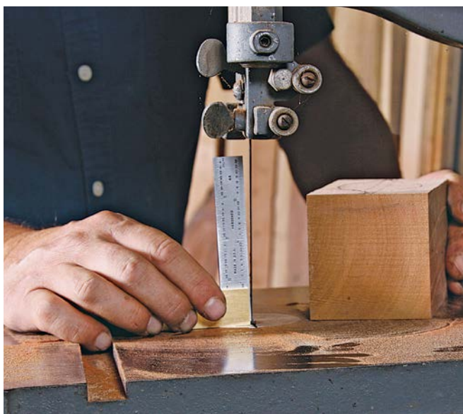
Initial sawing. After milling a block of wood, saw a slice off the top and set it aside—this will become the lid.
