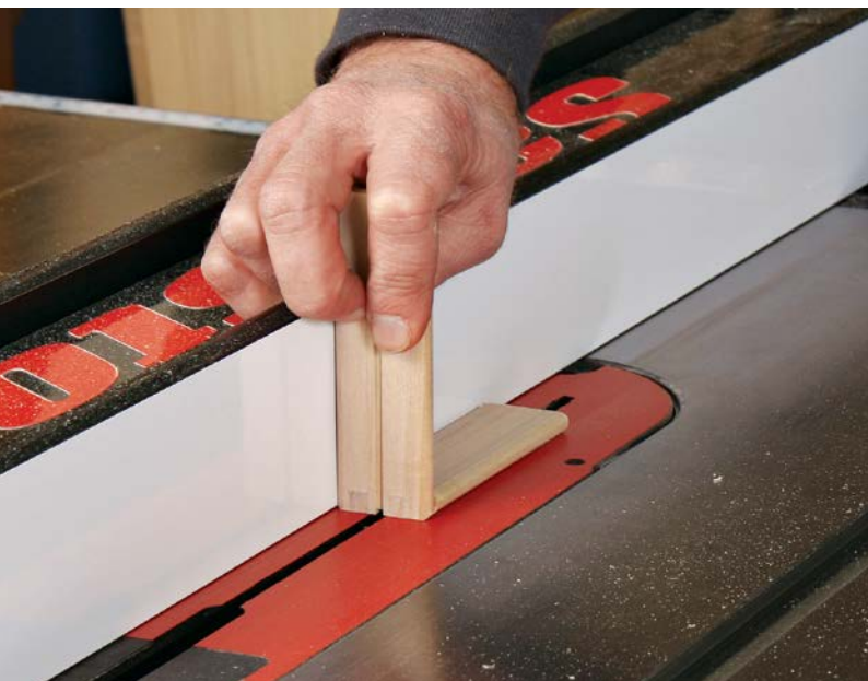
Glue slot. One careful pass over a tablesaw blade raised \frac{1}{16} in. produces an escape route for glue.
