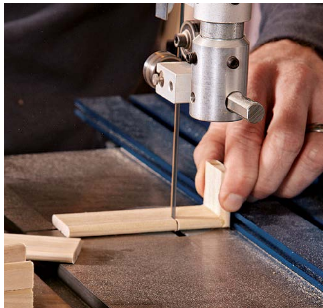
Off with the excess. A low fence at the bandsaw simplifies trimming the legs of the tenons to final length.
