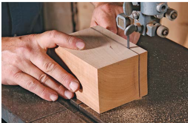
Initial sawing. After milling a block of wood, saw a slice off the top and set it aside—this will become the lid.
