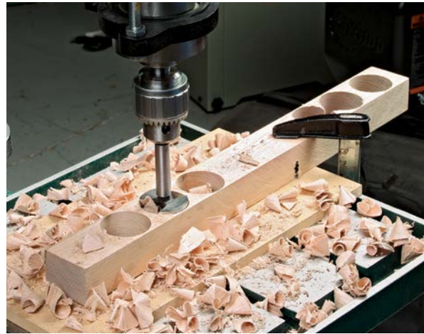
Timed test for power. Peck drilled through 2 in. of maple with a 2-in.-dia. Forstner bit. All the machines handled this tough test well, but elapsed time varied.
