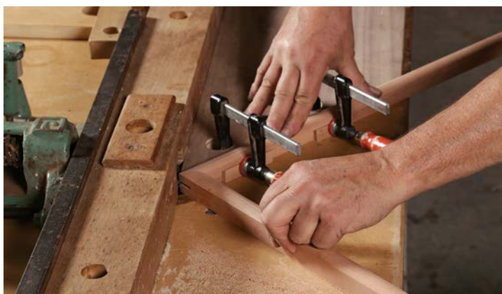
Slotting for the splines. Cullen cuts spline grooves with a slot-cutter at the router table. A piece of scrap stock cut at a 45° angle and drilled to accept clamps guides the frame through the cut.
