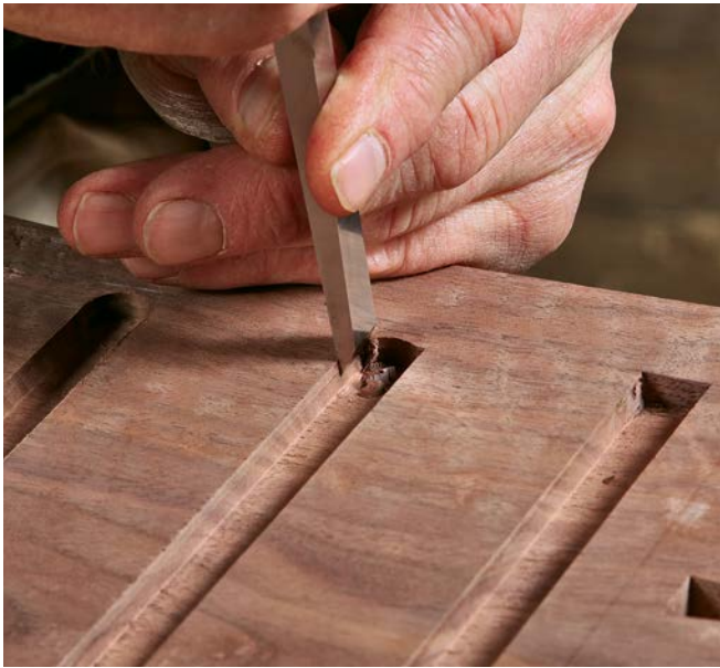
Square up. Scribe a line to mark the front end of each dado, then use a chisel to chop the routed ends square.
