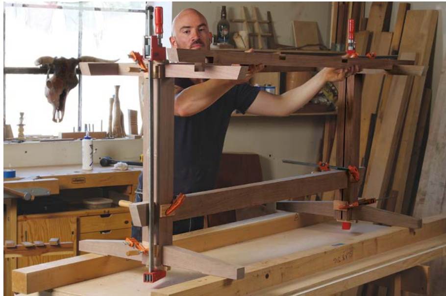
Add the top cross rails. Glue and tap the cross rails into place (left). Dry-fit the top stretchers (right) and the cross supports. These pieces help keep things aligned during glue-up, but are left dry so the table can be disassembled for transportation and maneuvering through tricky doorways or tight corners.
