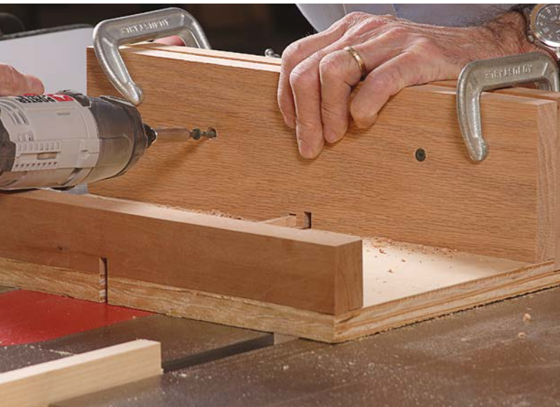
Screws set the fence. When you've established the perfect fit, screw the pin board in place. This jig will now work with any box you make using this blade.
