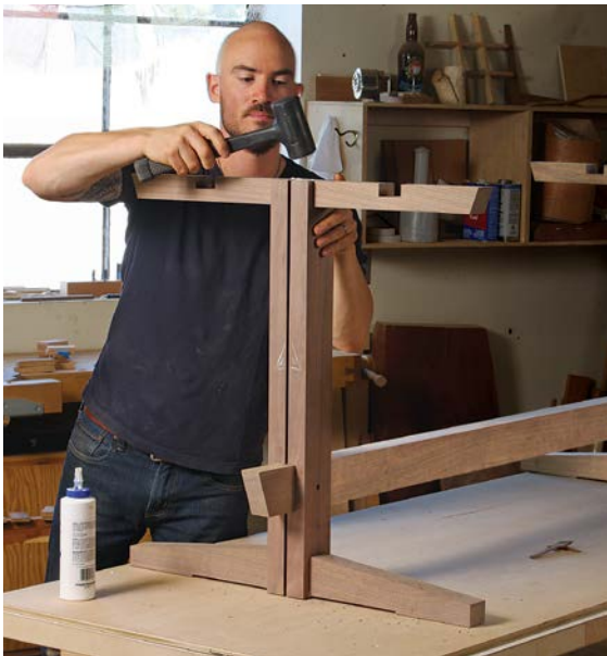
Add the top cross rails. Glue and tap the cross rails into place (left). Dry-fit the top stretchers (right) and the cross supports. These pieces help keep things aligned during glue-up, but are left dry so the table can be disassembled for transportation and maneuvering through tricky doorways or tight corners.
