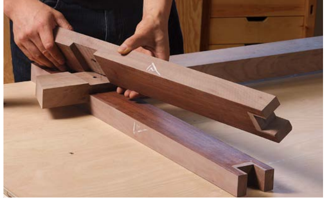
Prefinish the inside of the posts. Because the space between the posts is so narrow, you must finish the inside of the posts and the spacers between them before assembly.
