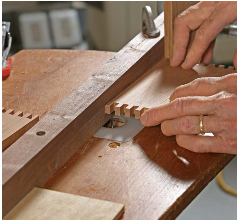
Groove for the bottom. To prepare for a bottom panel, Stowe routs \frac{1}{8} in. above the lower edge. Two parts get a stopped groove, two get a through-groove.
