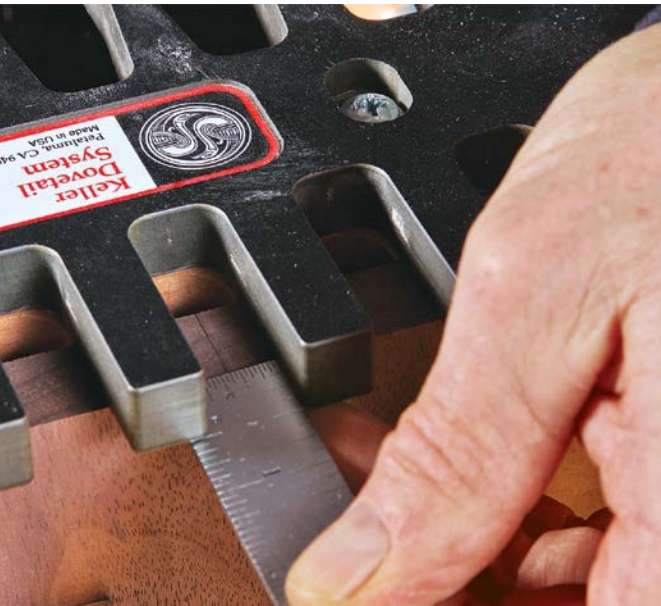
Set up and cut the tails first. After marking a centerline (top) and aligning the template (above left), clamp the jig in place and cut the tails (above right). The stop block clamped to the cleat helps locate the jig for the remaining cuts.
