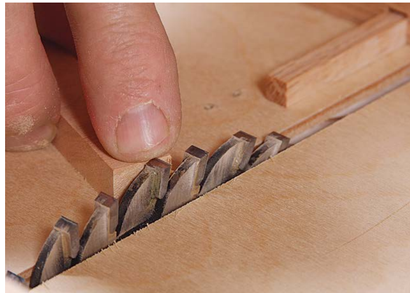
Offcut sets the blade height. Raise the blade about \frac{1}{64} in. above the stock to create a cleanup allowance. The fingers can be sanded flush to the box sides following assembly.
