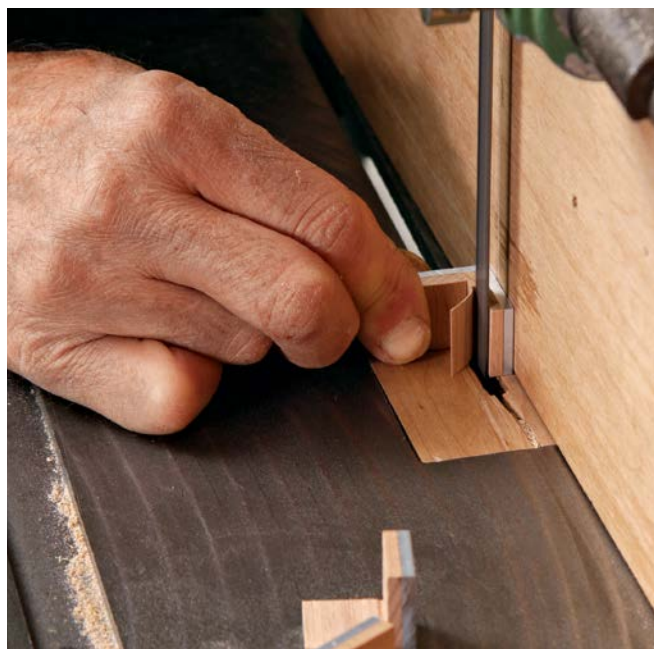
Tenon trimming. Coleman trims the tenon to exact thickness by shaving the wood face on the bandsaw.
