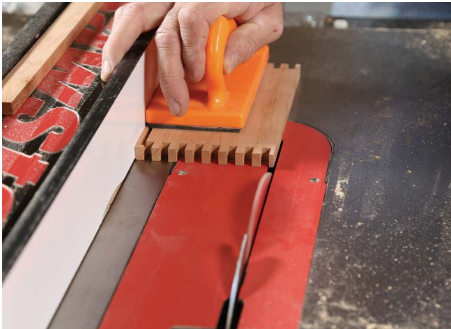
Trim the excess. Stowe cuts the fingers in stock that is a little wide and rips it to width later. This lets him clean up any cumulative error, like the thin finger on the right, that may have crept in.
