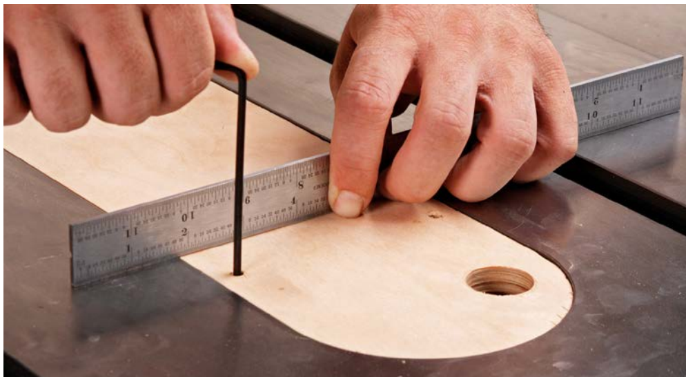
Get the inserts flush with the table. Using a straight rule and Allen key, bring the plate up until it's flush against the ruler and doesn't rock on the adjusters.
