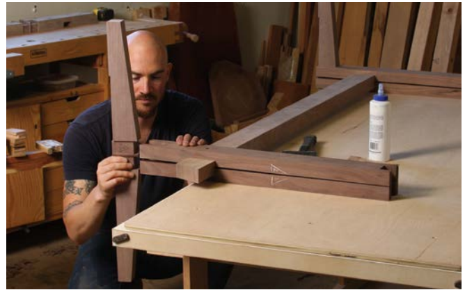
Stretcher, posts, and feet. The first step of the glue-up is to sandwich the stretcher in between the posts and add the two feet.
