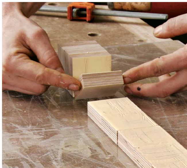
Glue up a stacked blank. When gluing up the stack of Baltic-birch squares, be sure the grain direction on the face alternates in adjacent blocks. Hansuld marks each block to show grain direction. He uses cauls along all four sides of the stack to maintain alignment during the glue-up.
