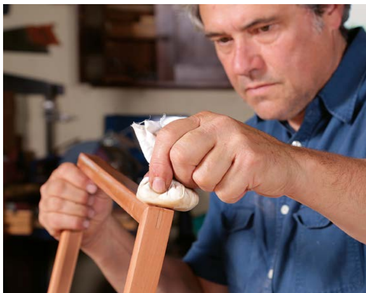
Finished frame. Cullen pads on shellac in thin coats, building to a low luster.
