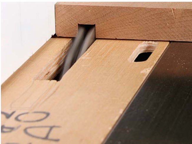
Easy grooves and dadoes. To cut grooves and dadoes, stack the blades and set the depth of cut.
