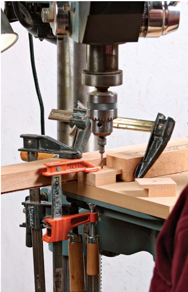
Clamp near the edge. Pivot the table to clamp small workpieces like these tabletop buttons.
