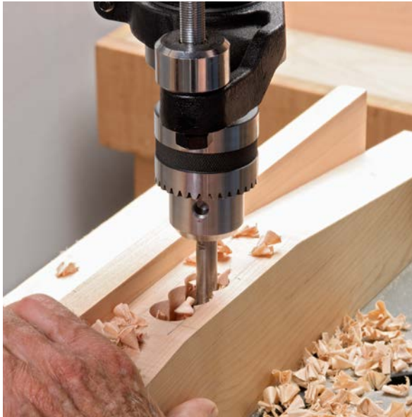
Extra quill travel. We looked for at least 4 in. of travel, for mortising this big trestle foot, for example.
