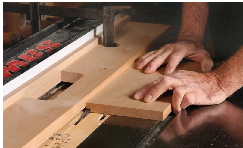
Rabbets, too. To cut rabbets, clamp a sacrificial fence to the rip fence and position it over the blade. Set the depth of cut and run the stock against the fence.
