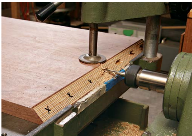
Cut the joint. Coleman cuts his miters first, then cuts the mortises with a horizontal mortiser. A router or Domino would work as well.
