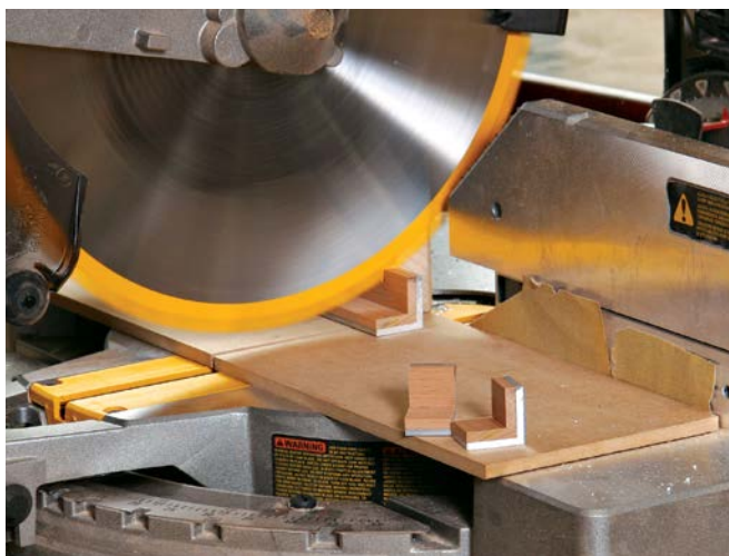
Chop chop. A regular woodworking blade in the chopsaw (or tablesaw) makes quick work of cutting the long blank into dozens of tenons.
