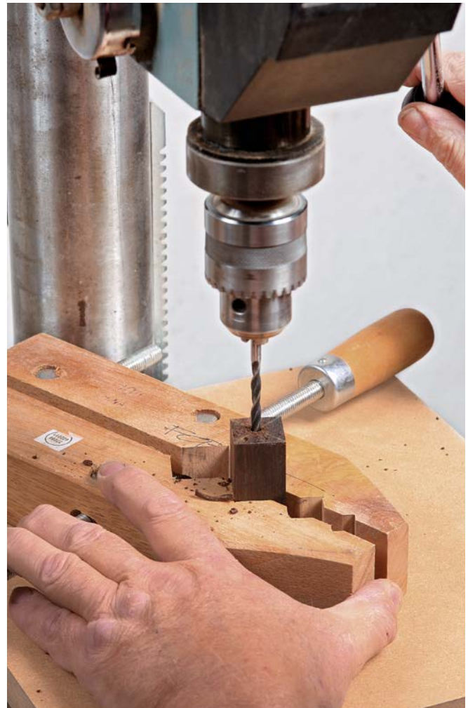
Doctor a hand screw. To hold short pieces upright, Fortune uses a notched wooden hand screw.
