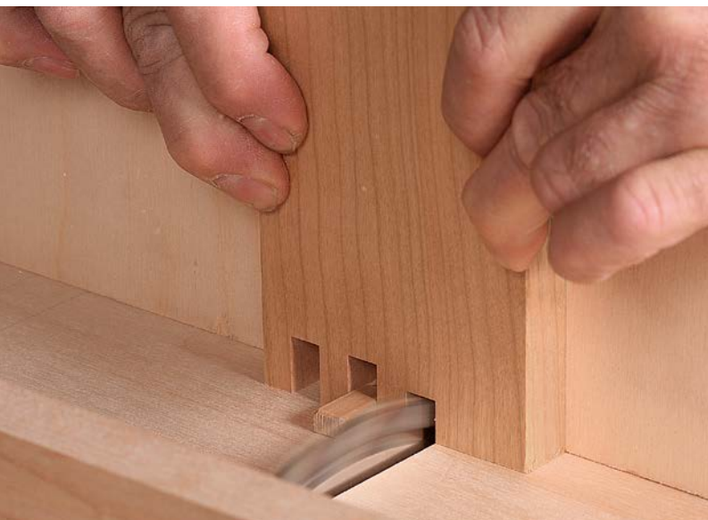
Box-joint basics. A jig holds the workpiece upright while an indexing pin sized to match the blade spaces out the joint precisely.
