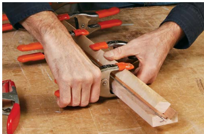
Clamp the sandwich. With the aluminum angle resting in a cradle and the wood strips glued, Coleman uses a square-section caul to distribute clamping pressure. The caul and the cradle are both waxed to resist glue.
