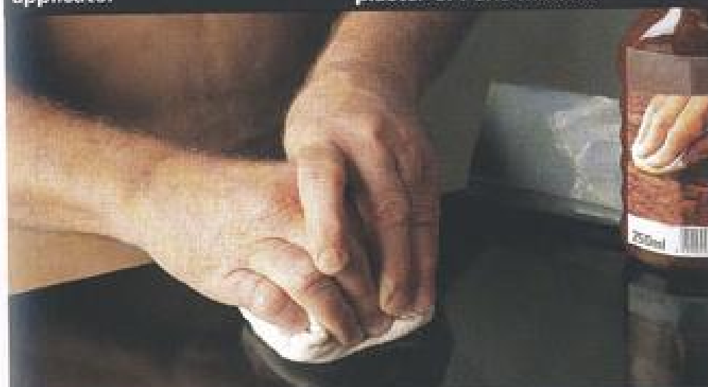
Applying French polish evenly across the surface
