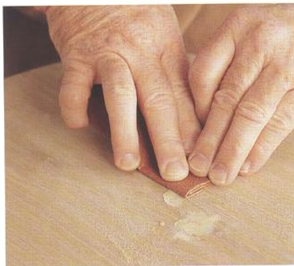
Gaps, holes or cracks in the surface should be filled with matching wood filler. Once dry, the filler should be sanded flush with the surface.
