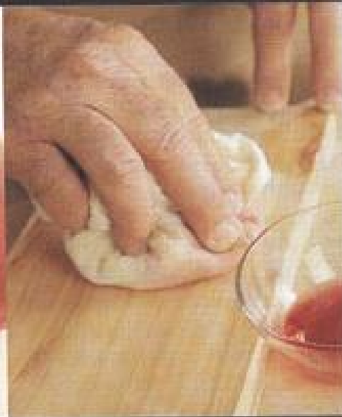
Stroking in an oil finish
