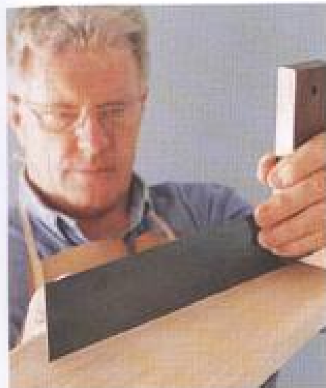
Use a try square blade to check that the face side is flat and true.
