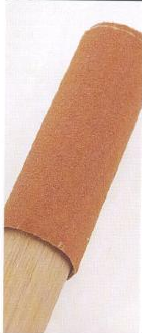
Abrasive paper wrapped around a dowel rod
