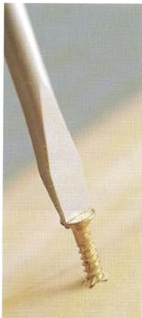
The screwdriver blade and screw head should be the same width.
