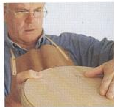
Catching the light at just the right angle will show up any problems or imperfections on the surface.
