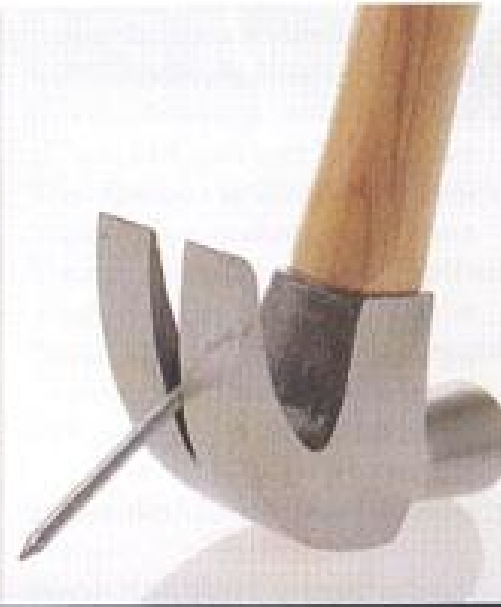
Claw hammer extracting nail
