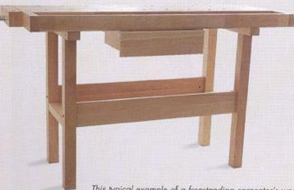
This typical example of a freestanding carpenter's workbench includes features such as a fitted bench vice with large and efficient jaws, and a drawer for tools or odds and ends.
