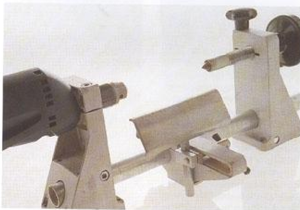
A bench-top lathe powered by a standard electric drill can be used to create small turned items, such as table lamps or small bowls.
