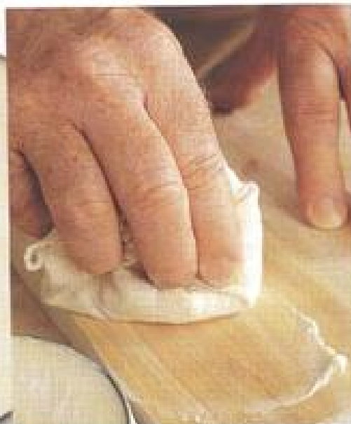
Rubbing in a wax finish
