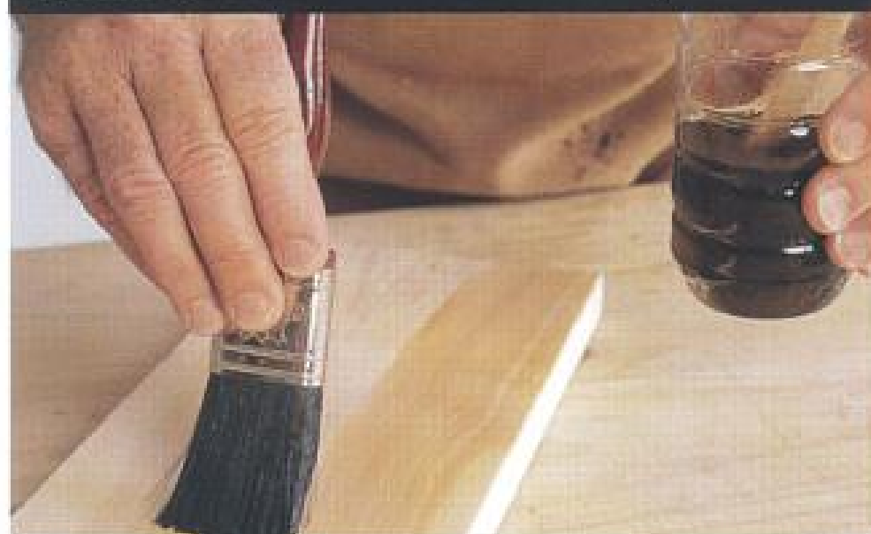
Applying the first coat of polyurethane
