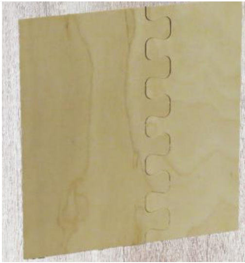
Board Extending with Jigsaw Keys
