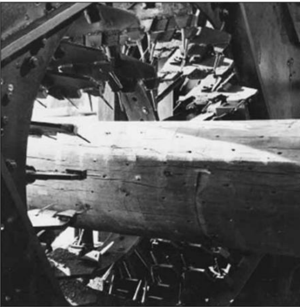
Figure 15-4. Deep incising permits better penetration of preservative.
