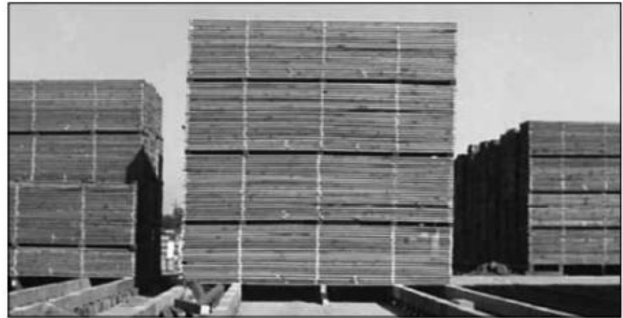
Figure 14–7. A sanitary, well-drained air-drying yard.
