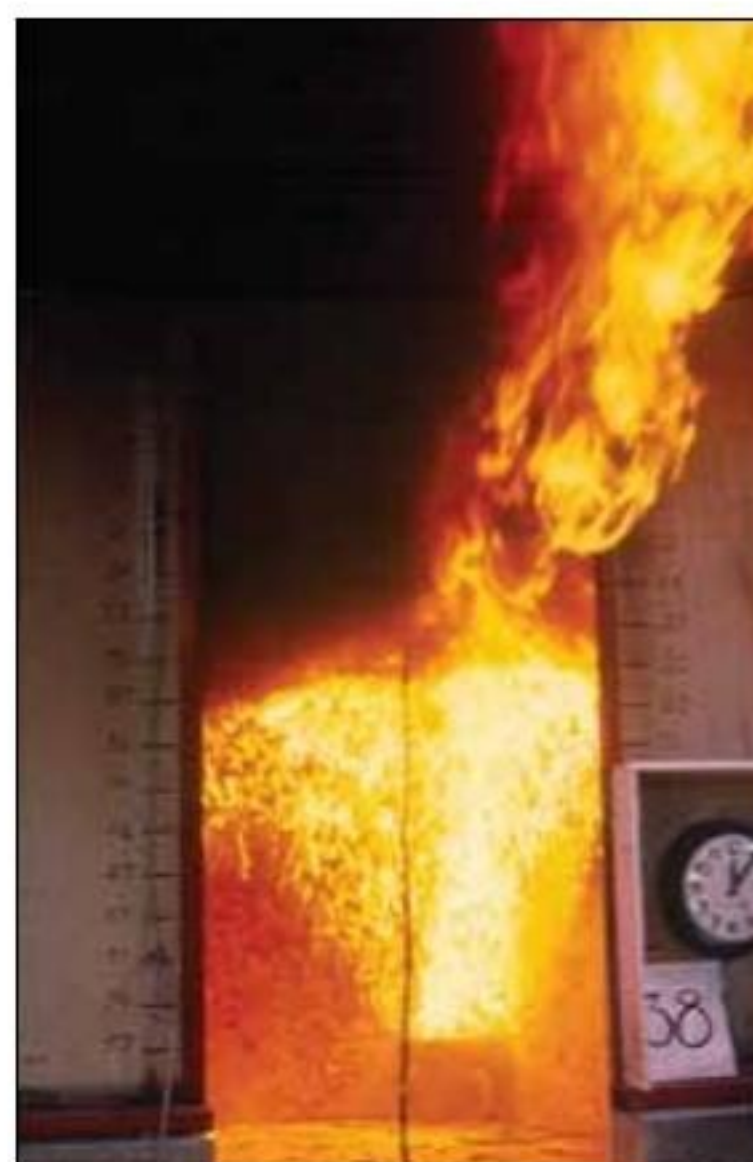
Figure 18–1. Flashover in standard room test.
