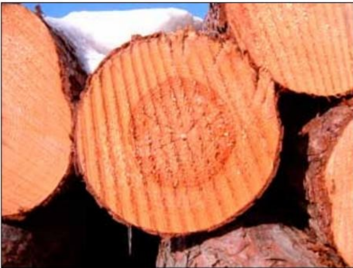
Figure 13–9. End checking in red pine logs.
