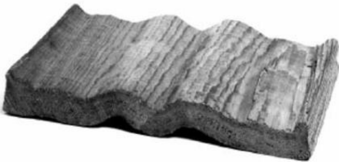
Figure 13–10. Severe collapse in western redcedar.
