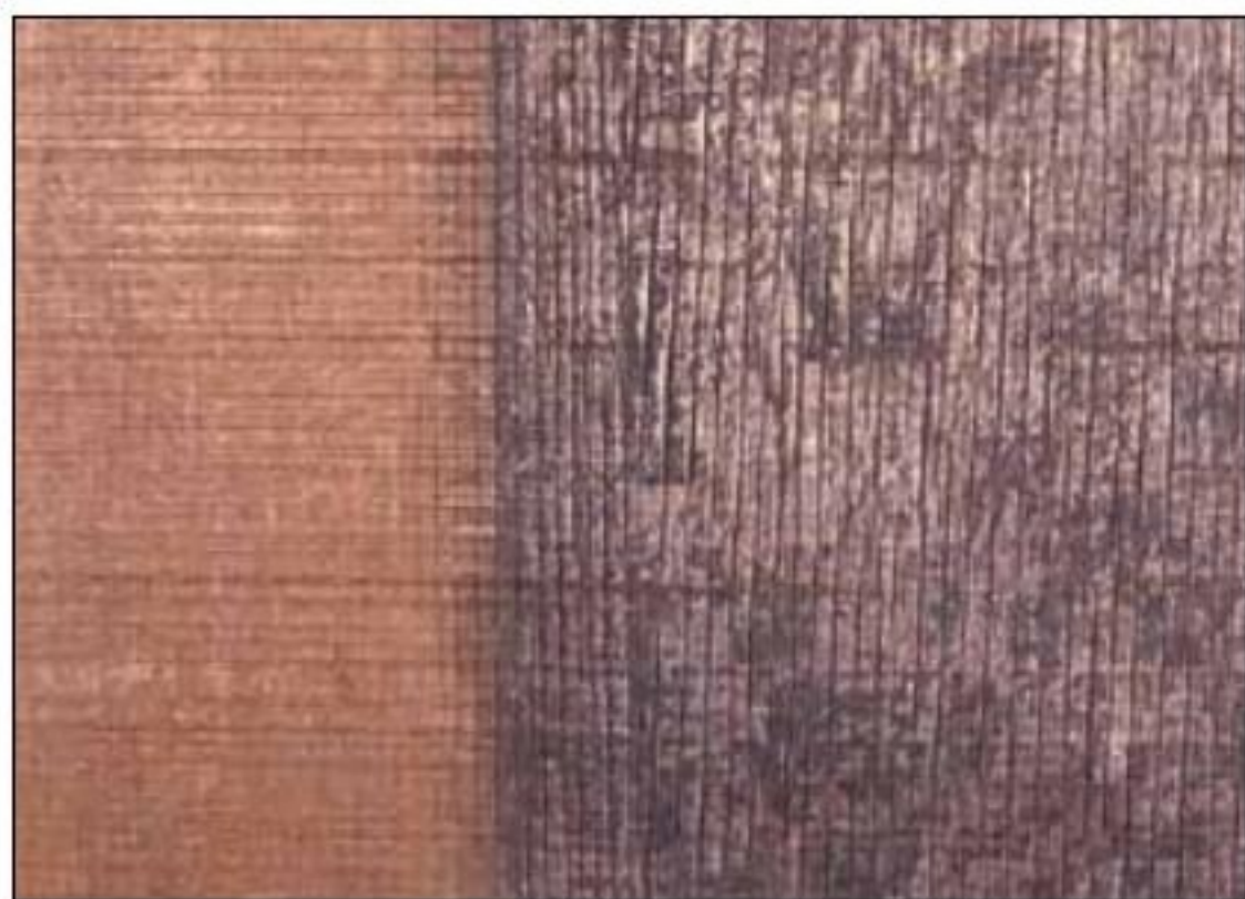
Figure 16–18. Front view of exterior grade of plywood siding after 10 years of exposure. The right-hand portion was exposed to the weather, whereas the left-hand side was covered with a board to give a board-and-batten appearance.
