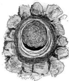
Fig. 5.67 Decayed knot: rot <1/3 in the cross-sectional area of a conifer, spruce ( Picea abies )
