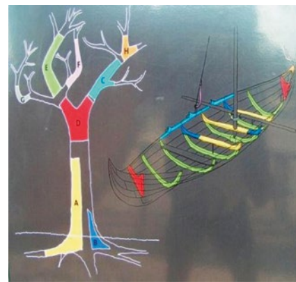
Fig. 5.25 Naturally shaped forks, root, stem, and branches used in shipbuilding (replica of Viking ship (Roskilde, Denmark))
