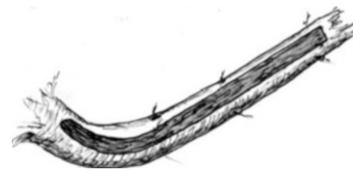
Fig. 5.19 Sled runner made from a crooked stem base (Lapland, Finland)
