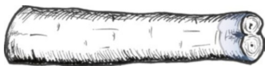
Fig. 5.31 Fork base left for protection on a veneer log
