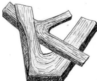
Fig. 5.32 Ship frame from a replica of a Viking ship, Roskilde, Denmark
