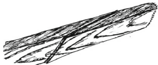
Fig. 7.18 Frost crack markings on a board from a spiral grain stem
