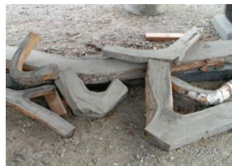
Fig. 2.5 In shipbuilding, care was given to use naturally shaped wood for the various parts of a vessel – i.e., branch forks (red markings), crooked branches, and curved stems. The photo to the right shows frames and stern posts made from an oak tree for the replica of a Viking ship (Roskilde, Denmark)
