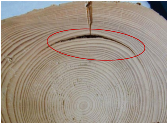
Fig. 5.101 Different wood densities in the narrow and wide tree rings of this spruce ( Picea abies ) lead to varying shrinkage behavior in the wood. The tension is neutralized by a ring and radial shakes
