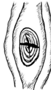
Fig. 5.79 Dry crack in a knot in a board
