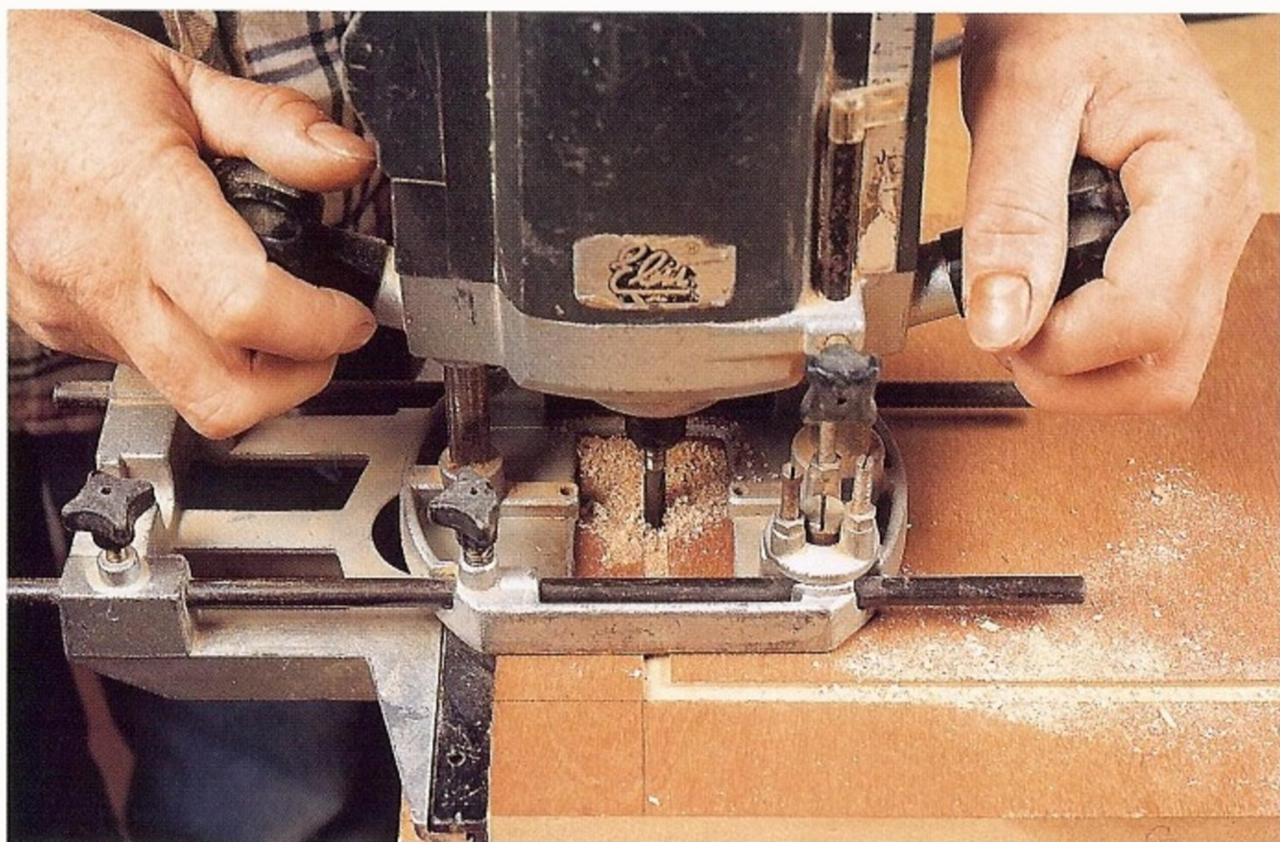
Fig 2.8 Specialized bits adapt the power router for particular jobs.
