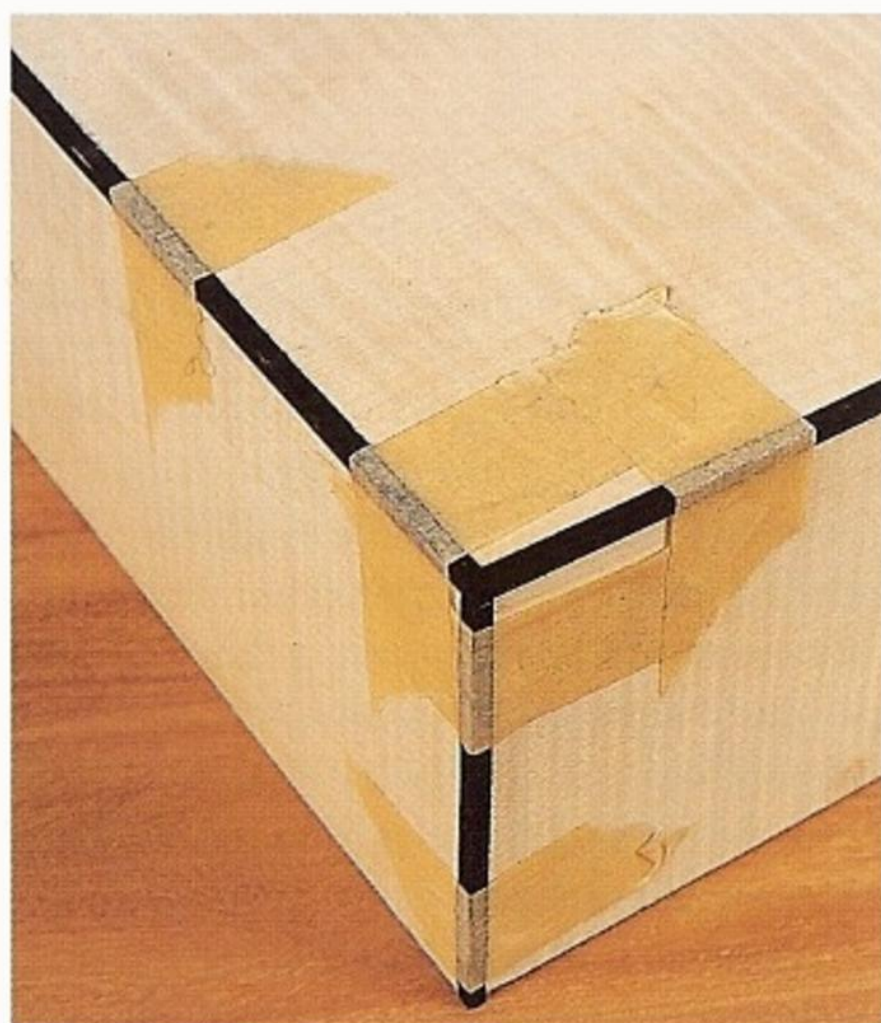
Fig 7.19 Holding a square string in its rebate while the glue dries.
