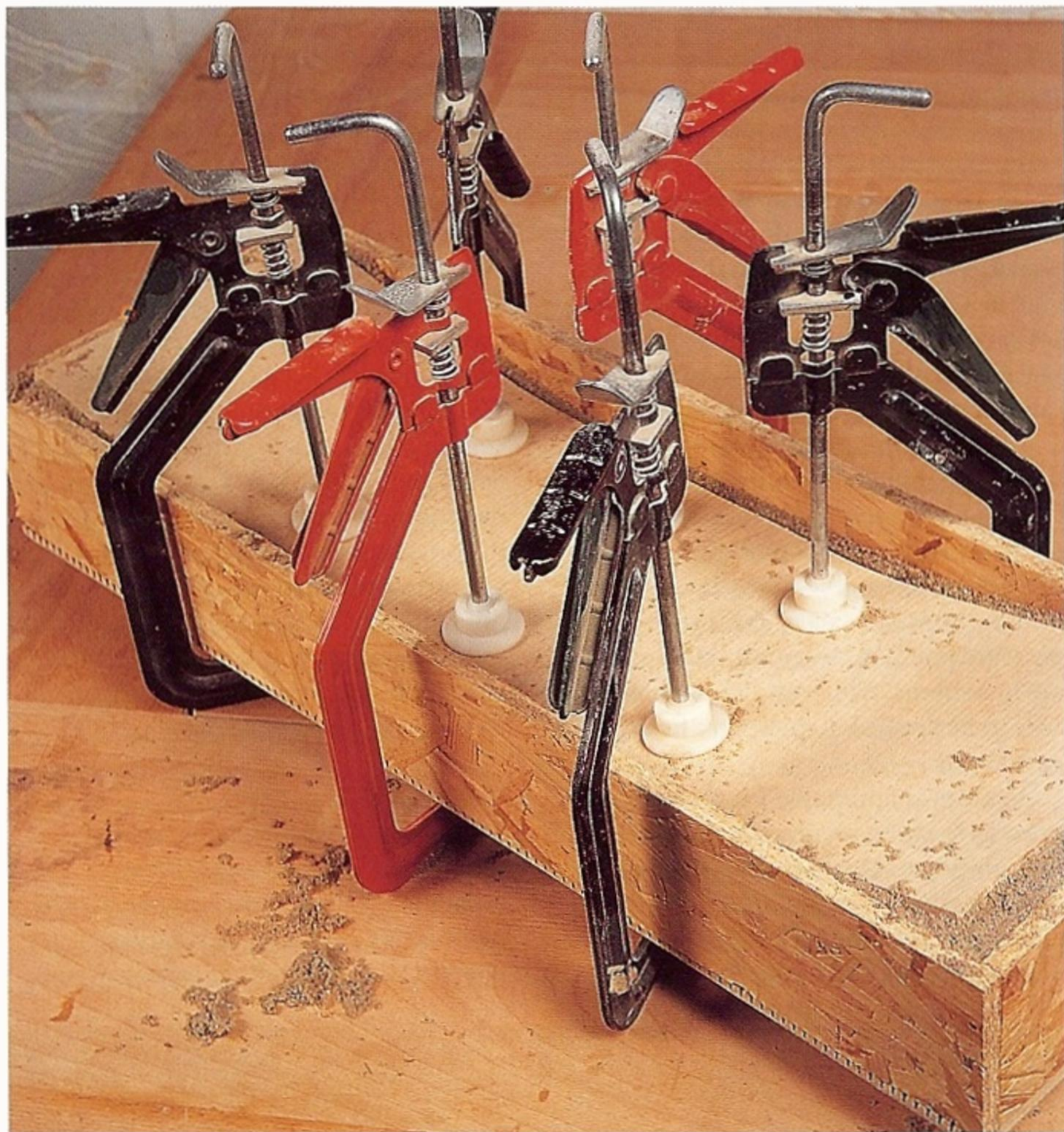
Fig 4.31 The groundwork is pressed into the sand, under the pressure of cramps, to create a reverse profile. In effect, the sand will act as a shaped caul.
