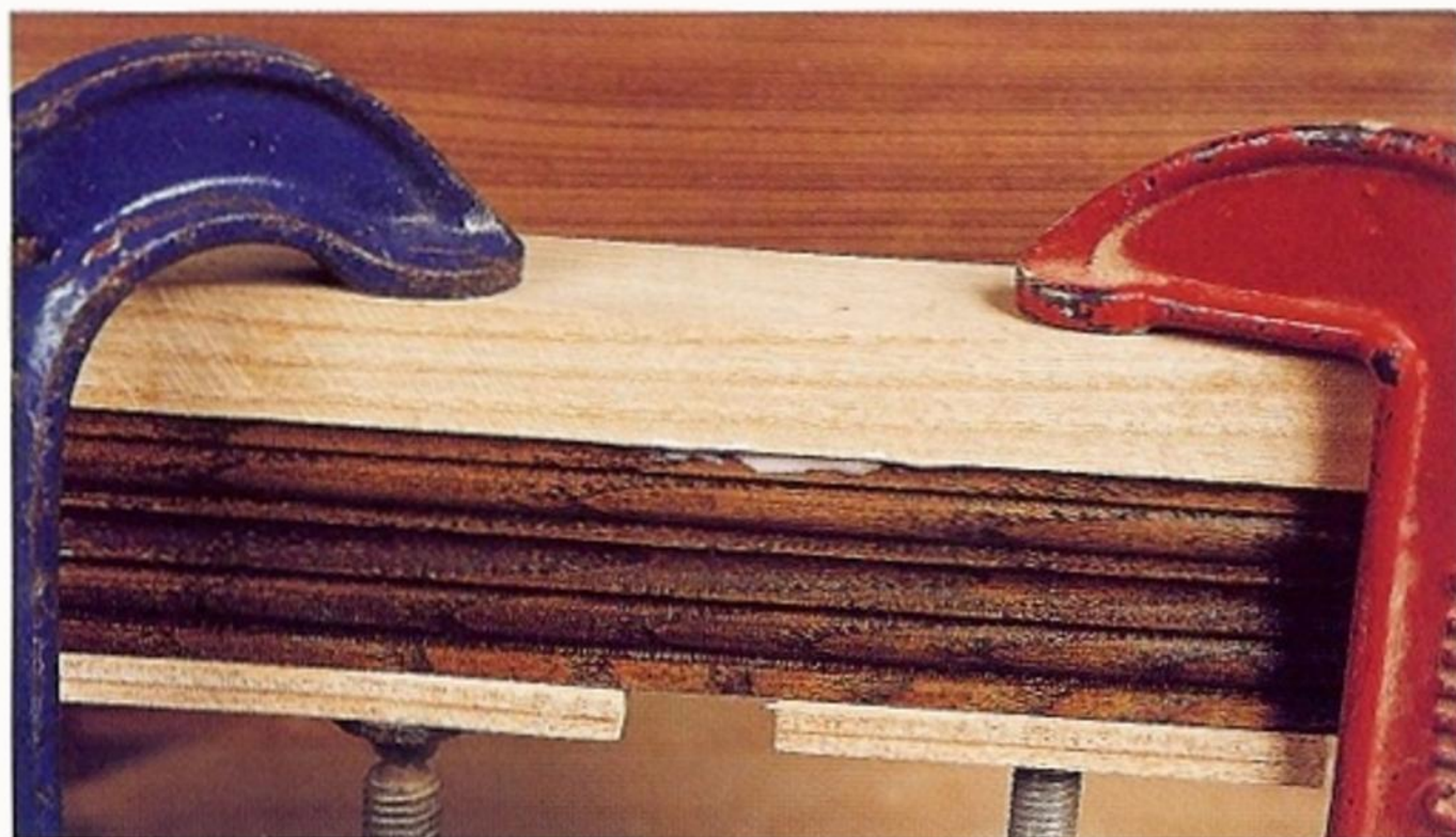
Fig 4.36 Cramping the edge after the glue has been slipped under it.
