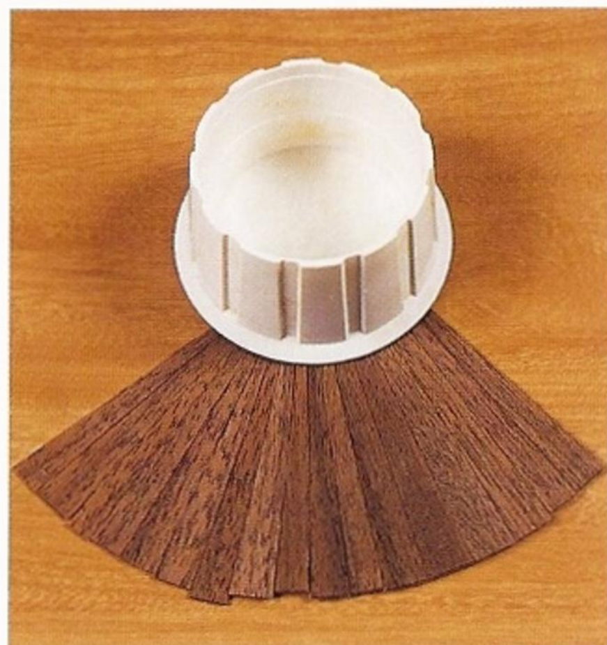
Fig 5.12 Use the template to make the inner curved edge to the corner cross-banding.
