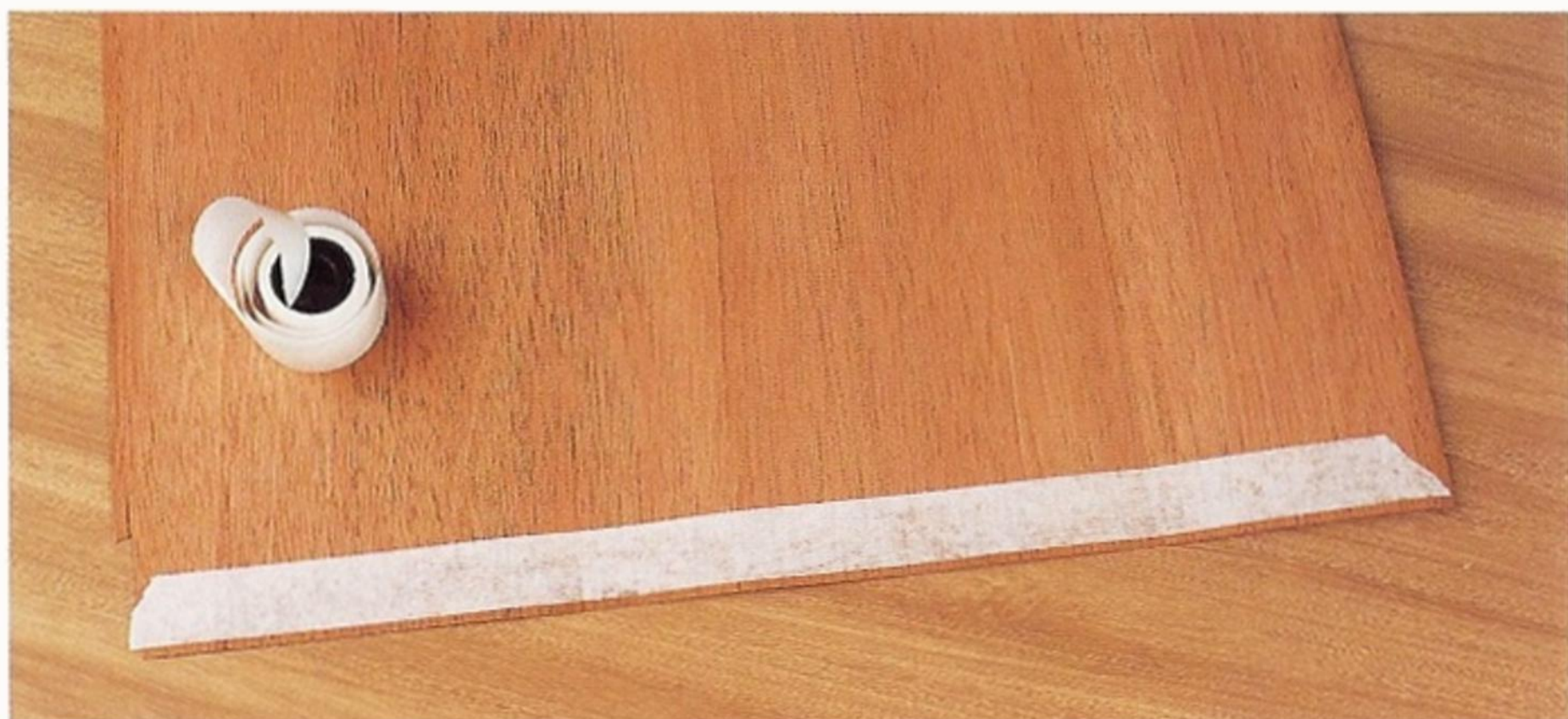
Fig 3.1 Taping the ends of a leaf of veneer will reduce the risk of splits appearing and worsening.
