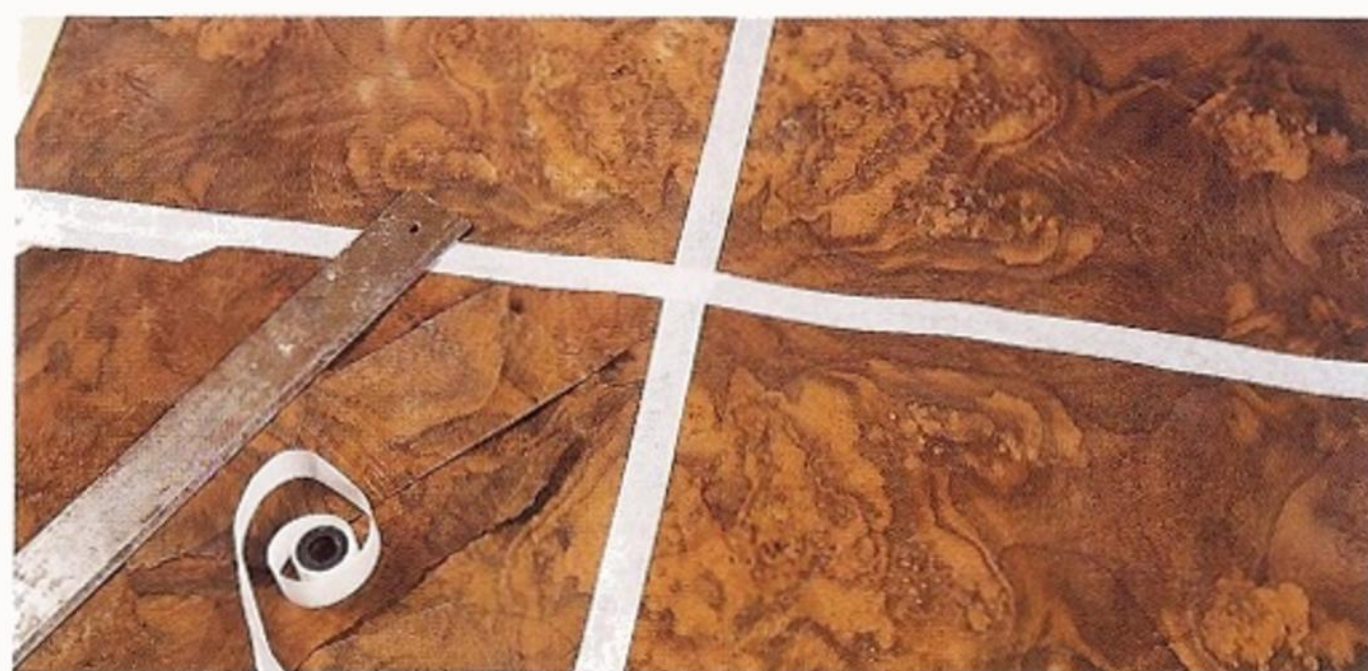
Fig 6.11 A quartered panel, with joints taped, is ready for laying.
