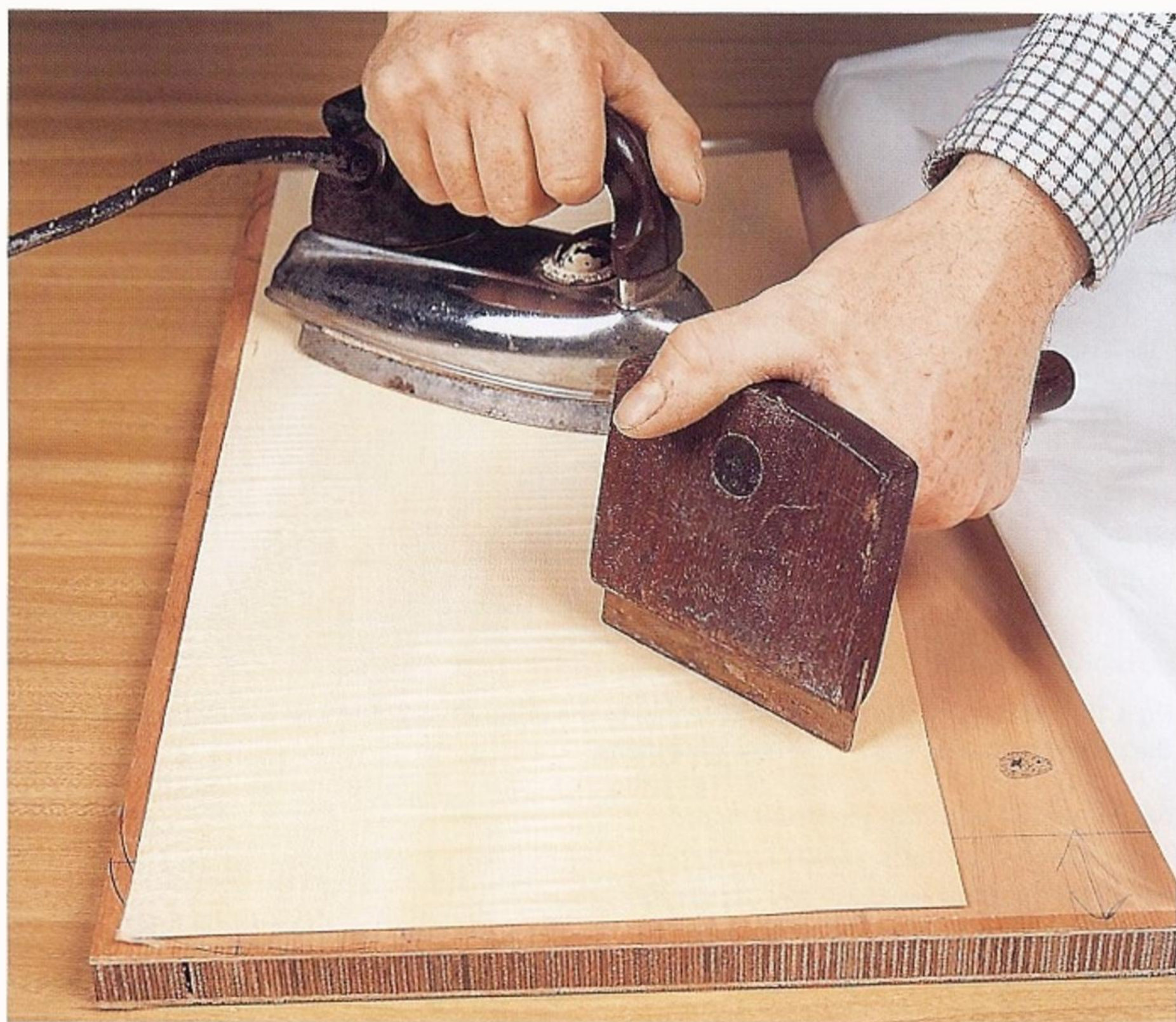
Fig 4.11 As the iron melts the glue, use a veneer hammer to press the veneer down, applying pressure from the centre out.
