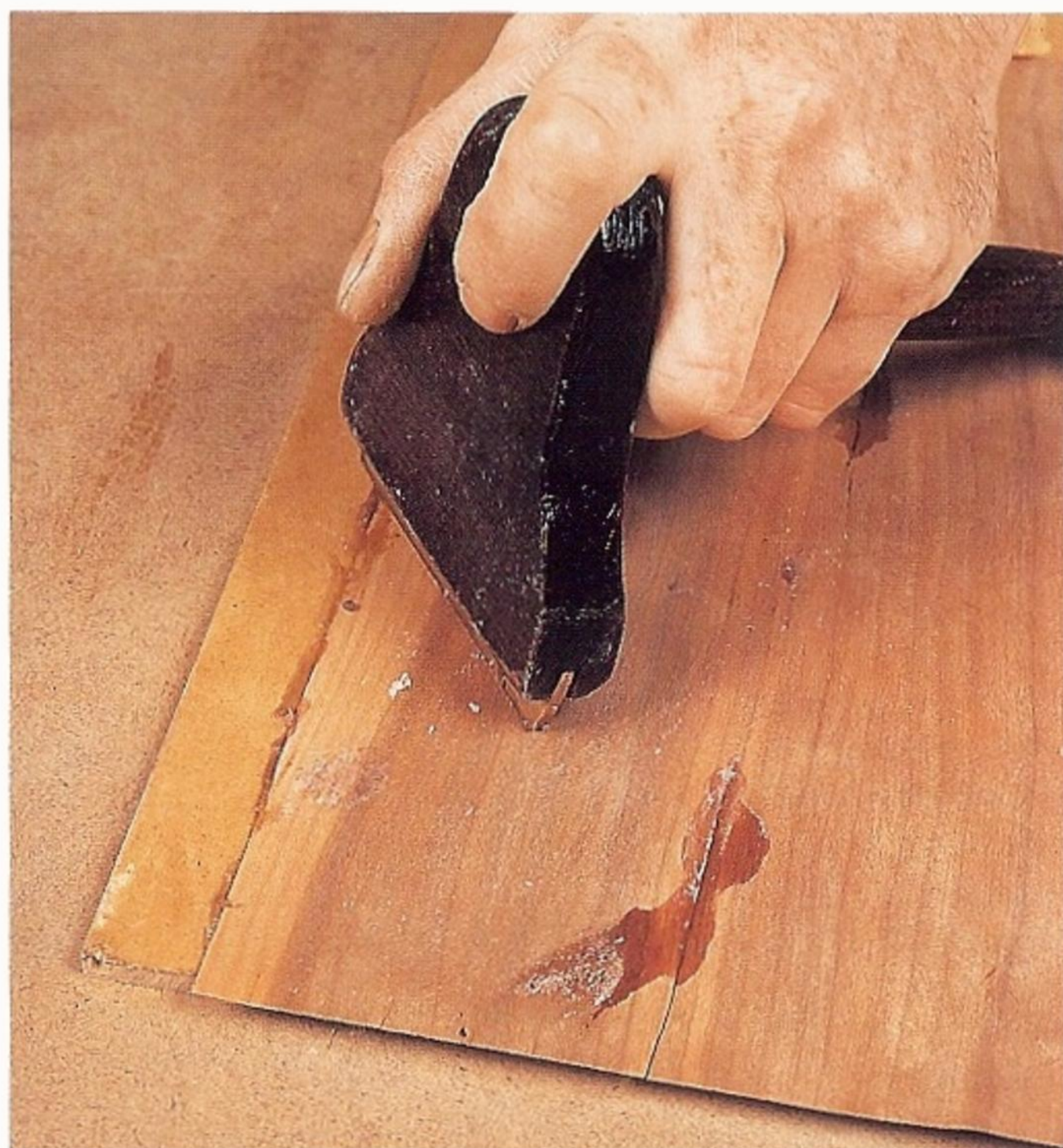
Fig 4.16 Use the veneer hammer to press the veneer down onto the groundwork.
