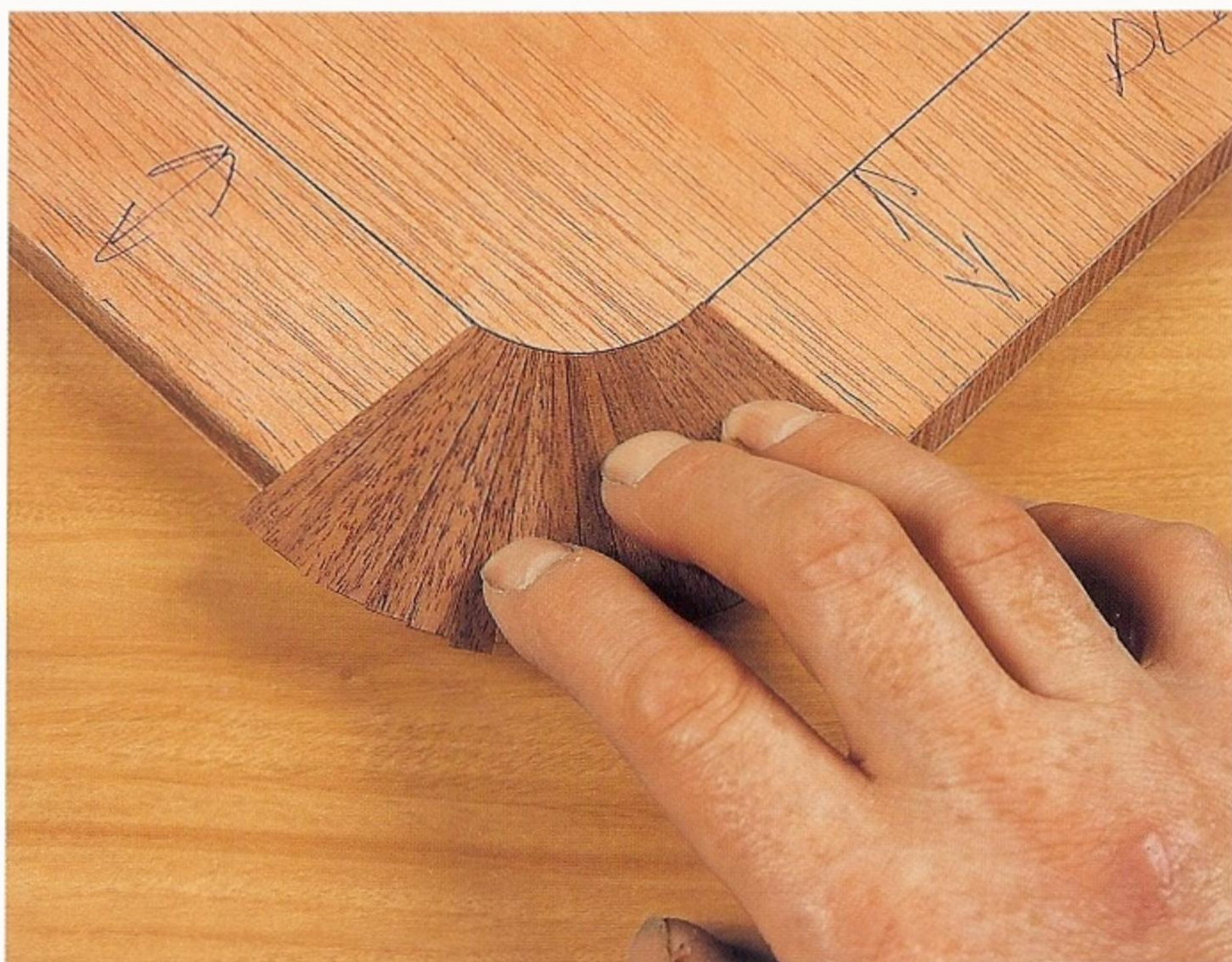
Fig 5.13 'Rubbing' the prefabricated corner into place. This is done by sliding the veneer into position. The natural 'grab' of pearl glue will hold it in place.
