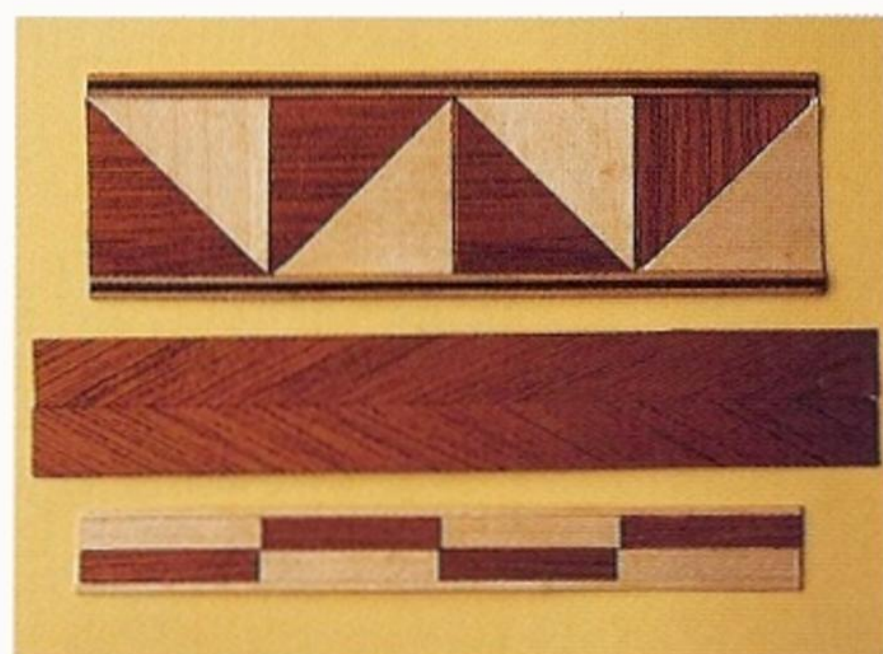
Fig 7.3 Bandings are made up of two or more species, though the feather banding in the middle row uses just one.
