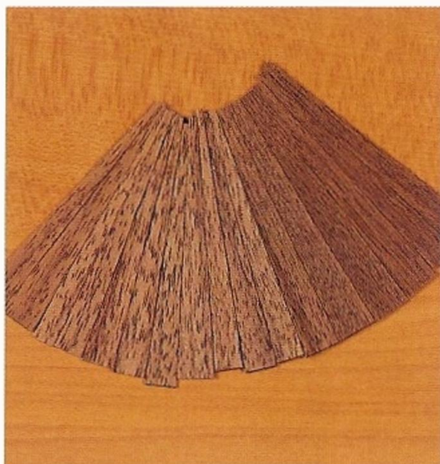
Fig 5.11 Prefabricate the veneer for the corner: it is a lot easier than trying to lay several small sections of veneer with accurate joints.
