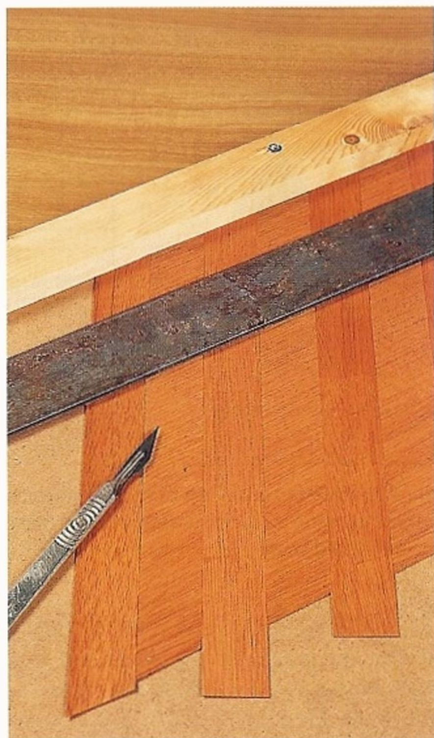
Fig 8.17 Cutting strips of diamonds.
