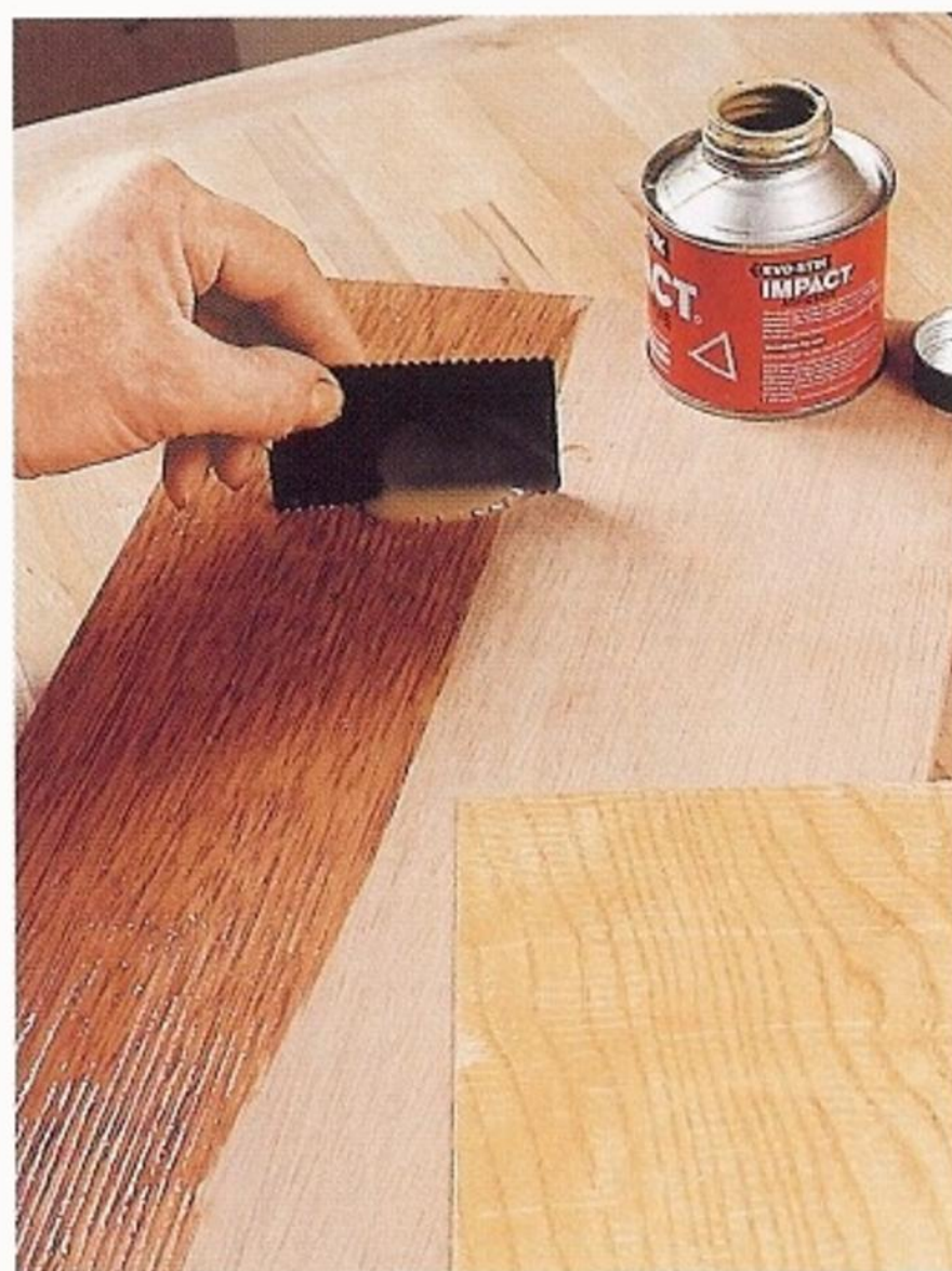
Fig 4.12 Spread a thin, even coat of contact adhesive over the veneer and the groundwork. A serrated spreader is provided with the adhesive.
