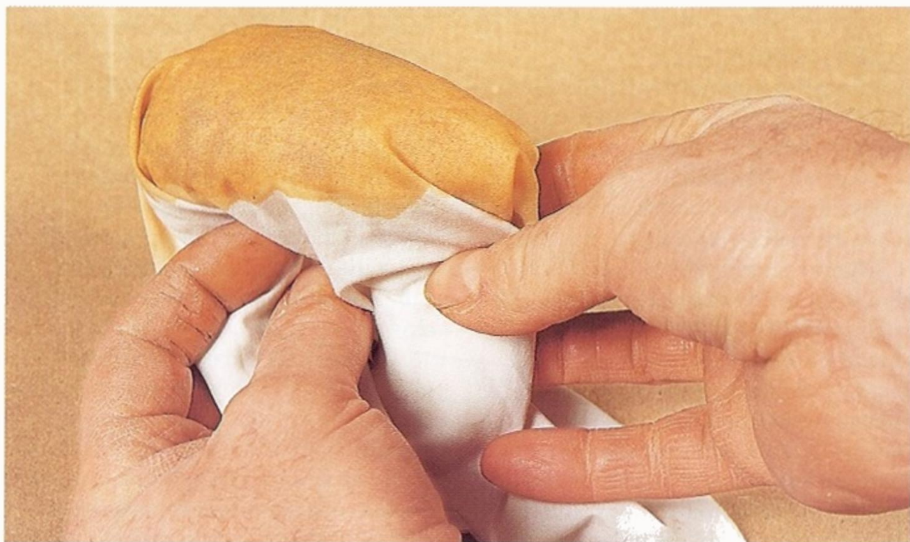
Fig 9.3 Making a french polish rubber.
