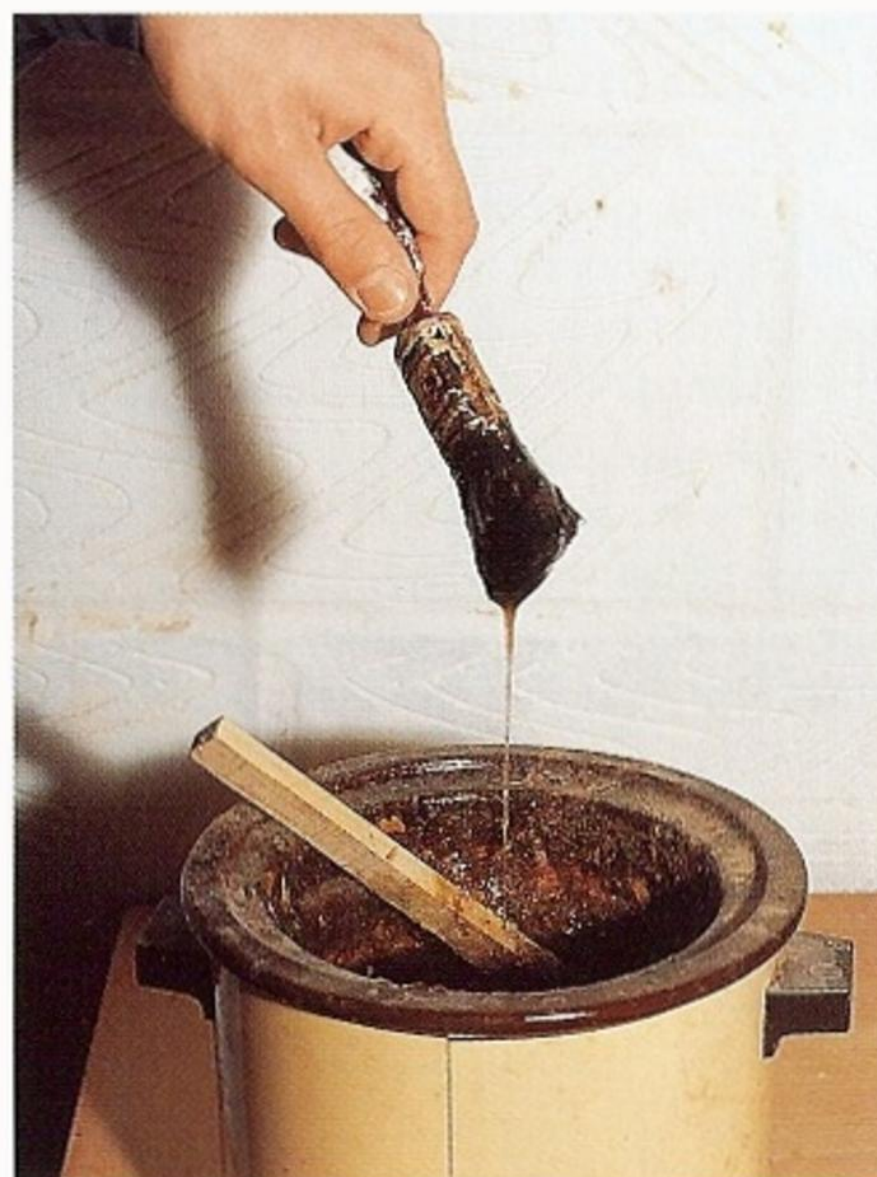
Fig 1.22 The perfect consistency for glue: it runs off the glue brush in a steady stream.
