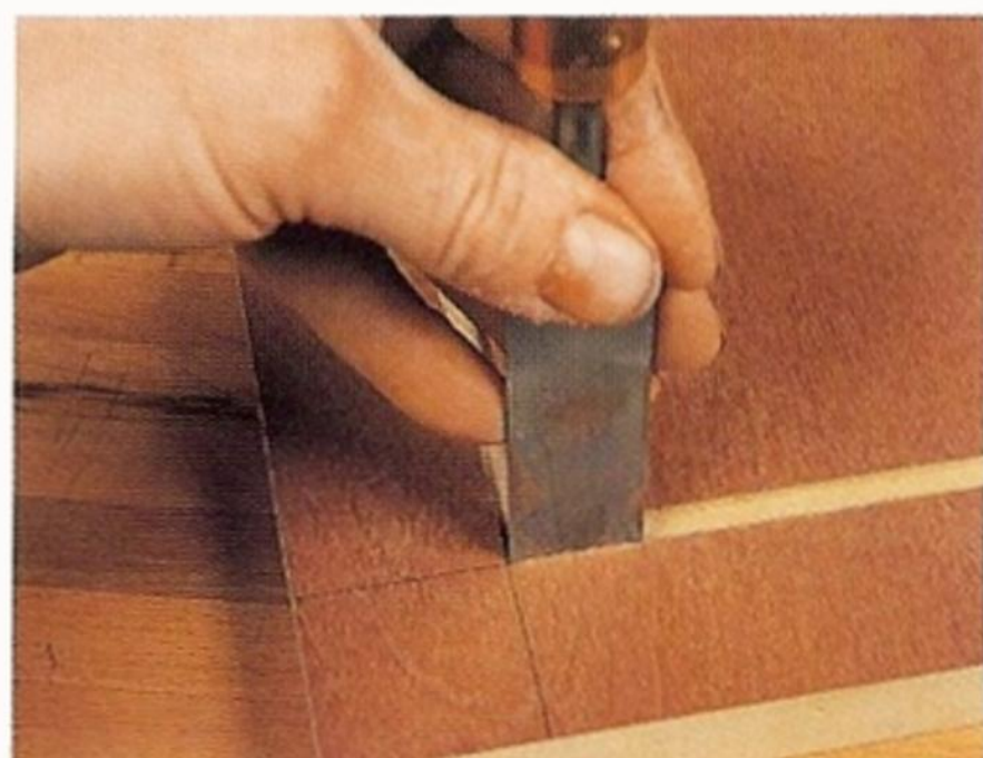
Fig 7.16 Use a veneer knife or chisel to square off the rounded corners.
