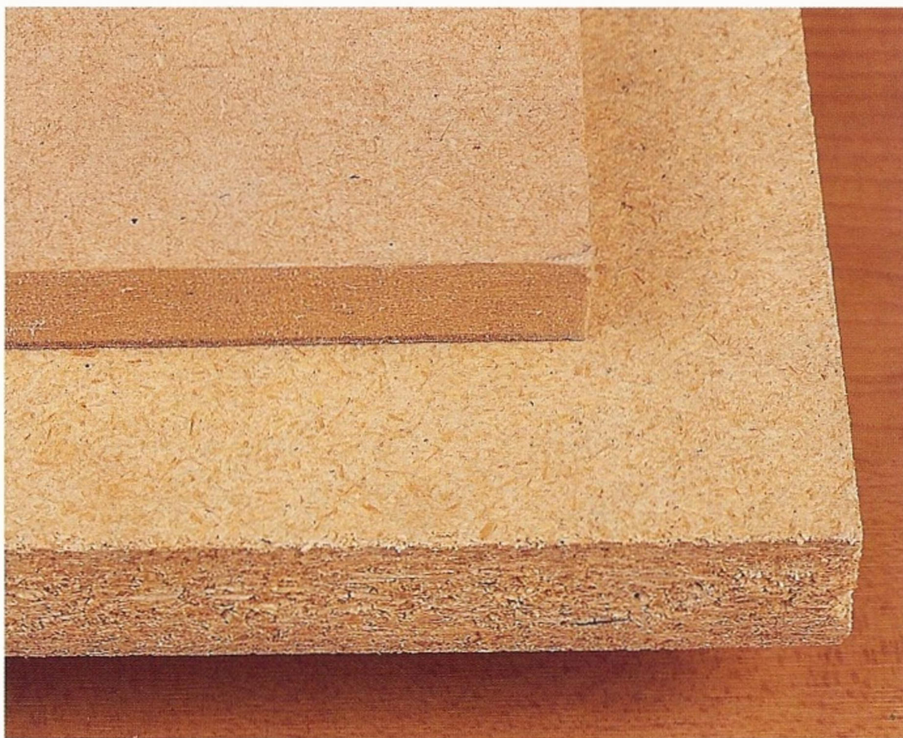
Fig 1.19 Top: medium density fibreboard (MDF). Bottom: chipboard.
