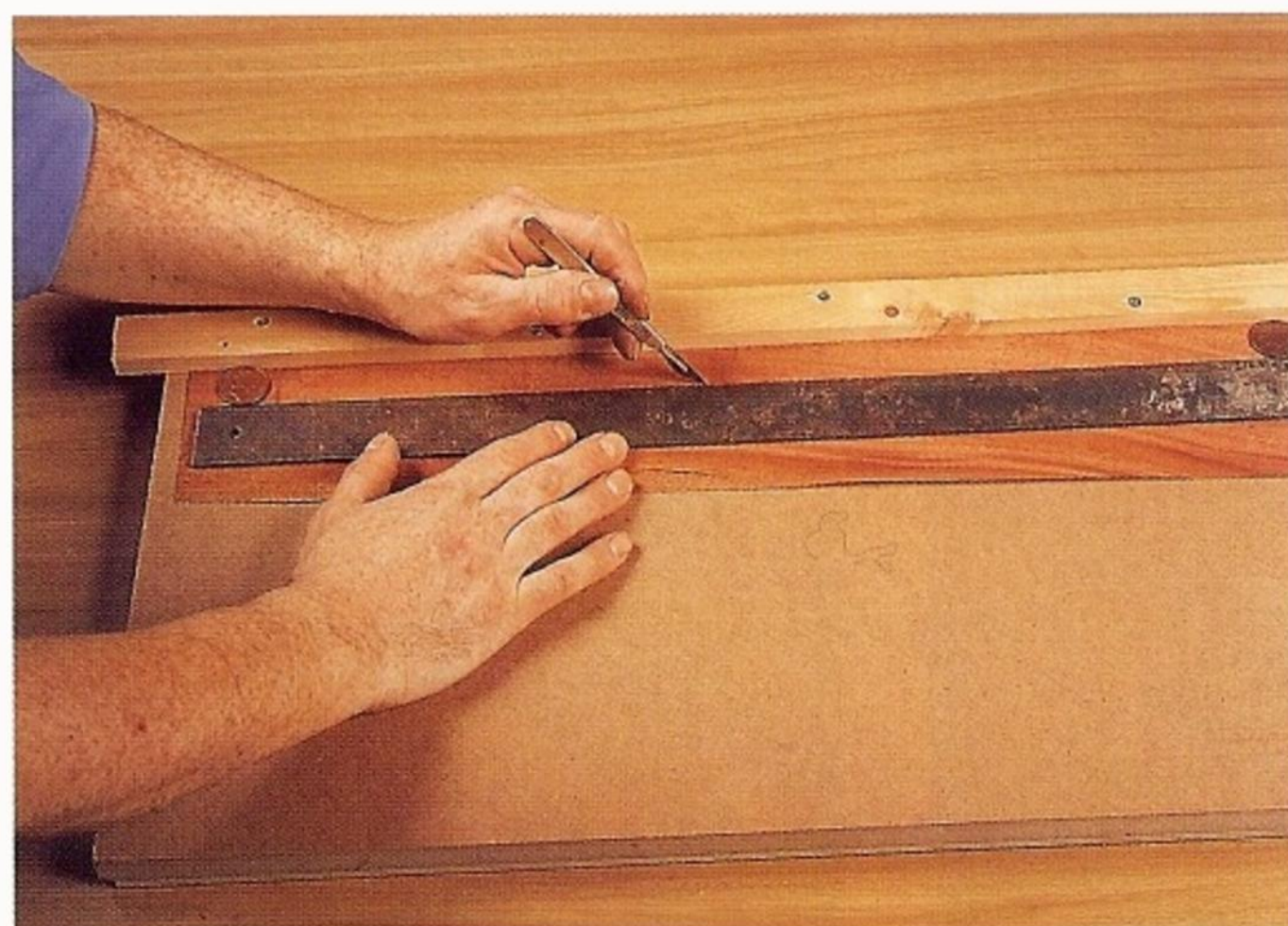
Fig 8.8 Cutting parallel strips of veneer using the jig.
