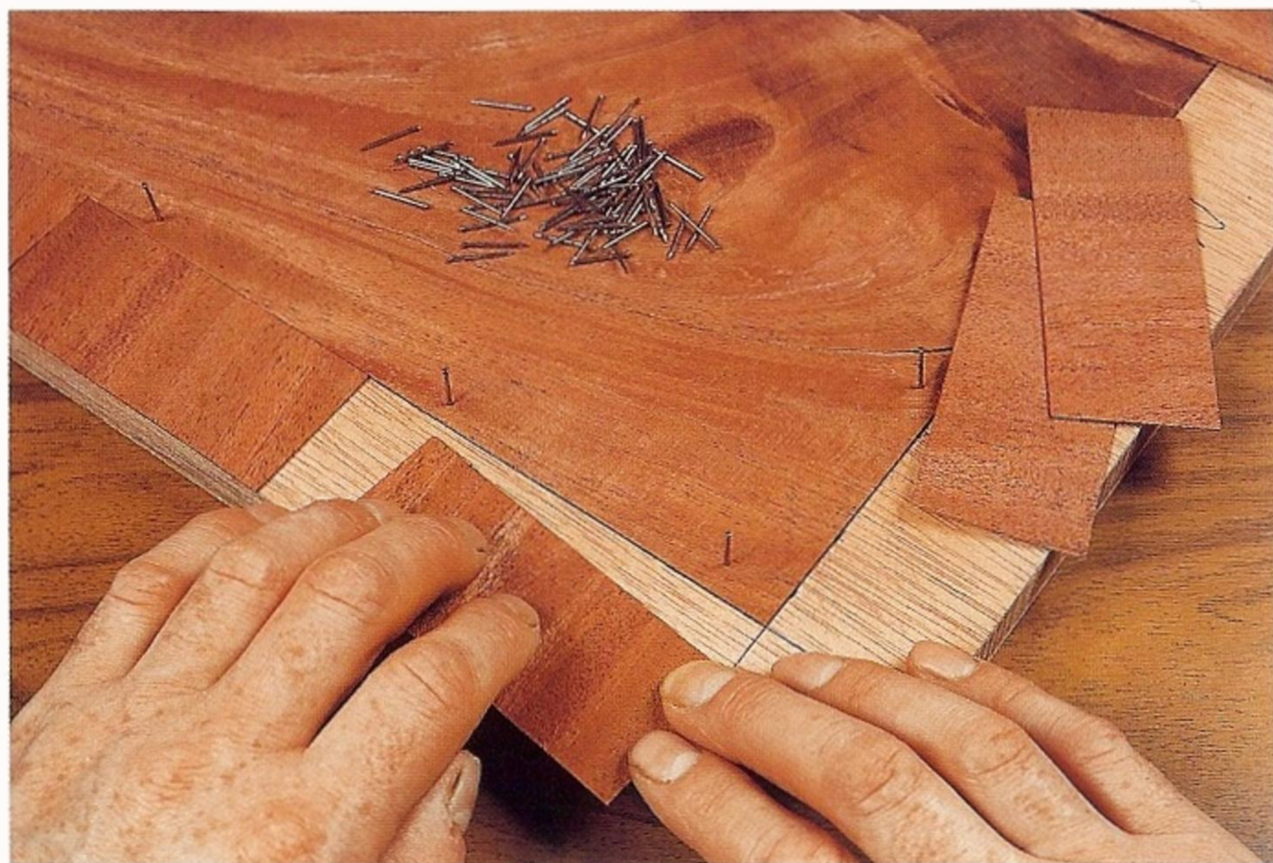
Fig 5.17 The central panel is held in place with veneer pins while fitting the cross-banding.
