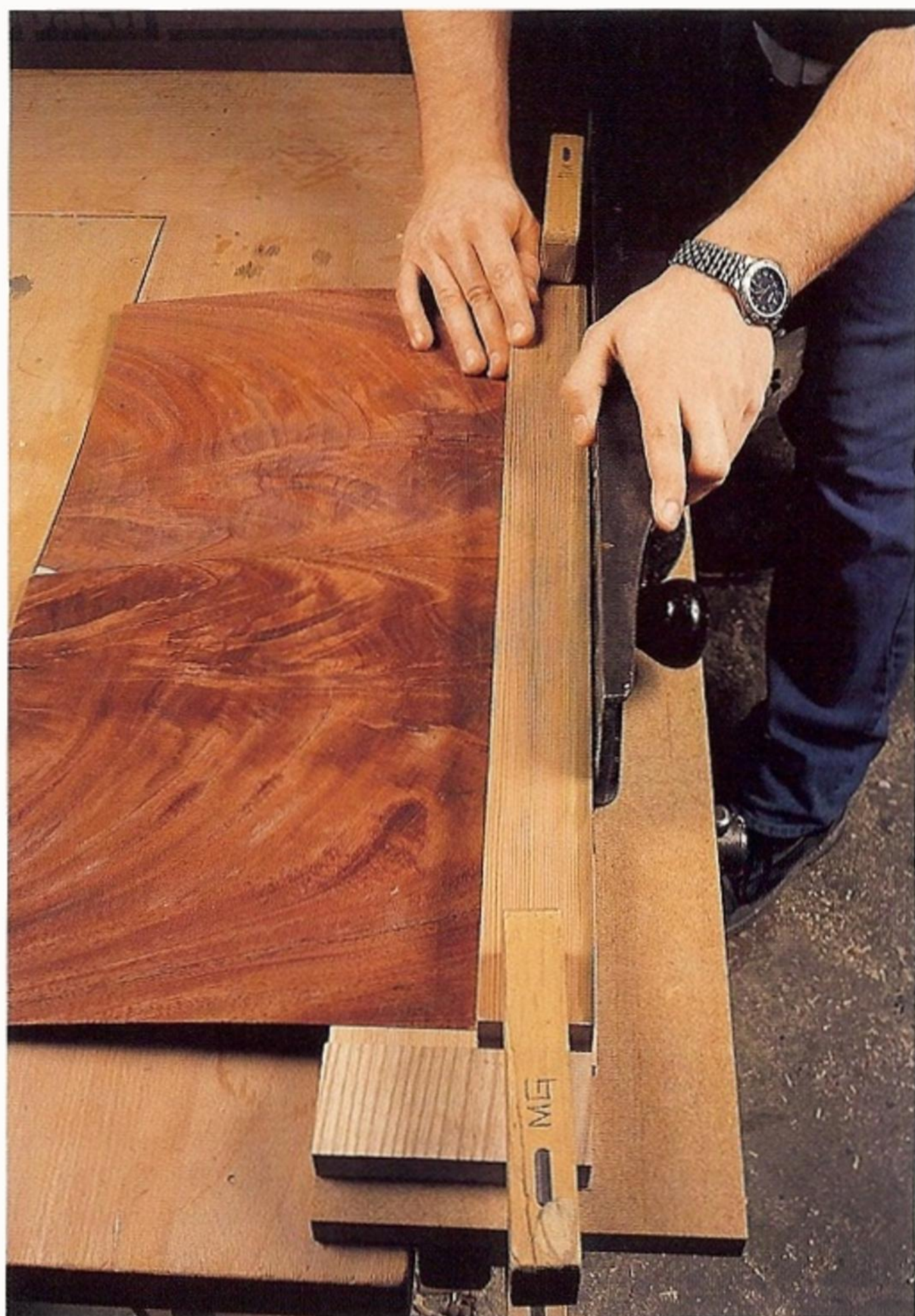
Fig 6.8 Trim the joining edges on the shooting board. Note the use of a batten to hold the edges flat and secure.
