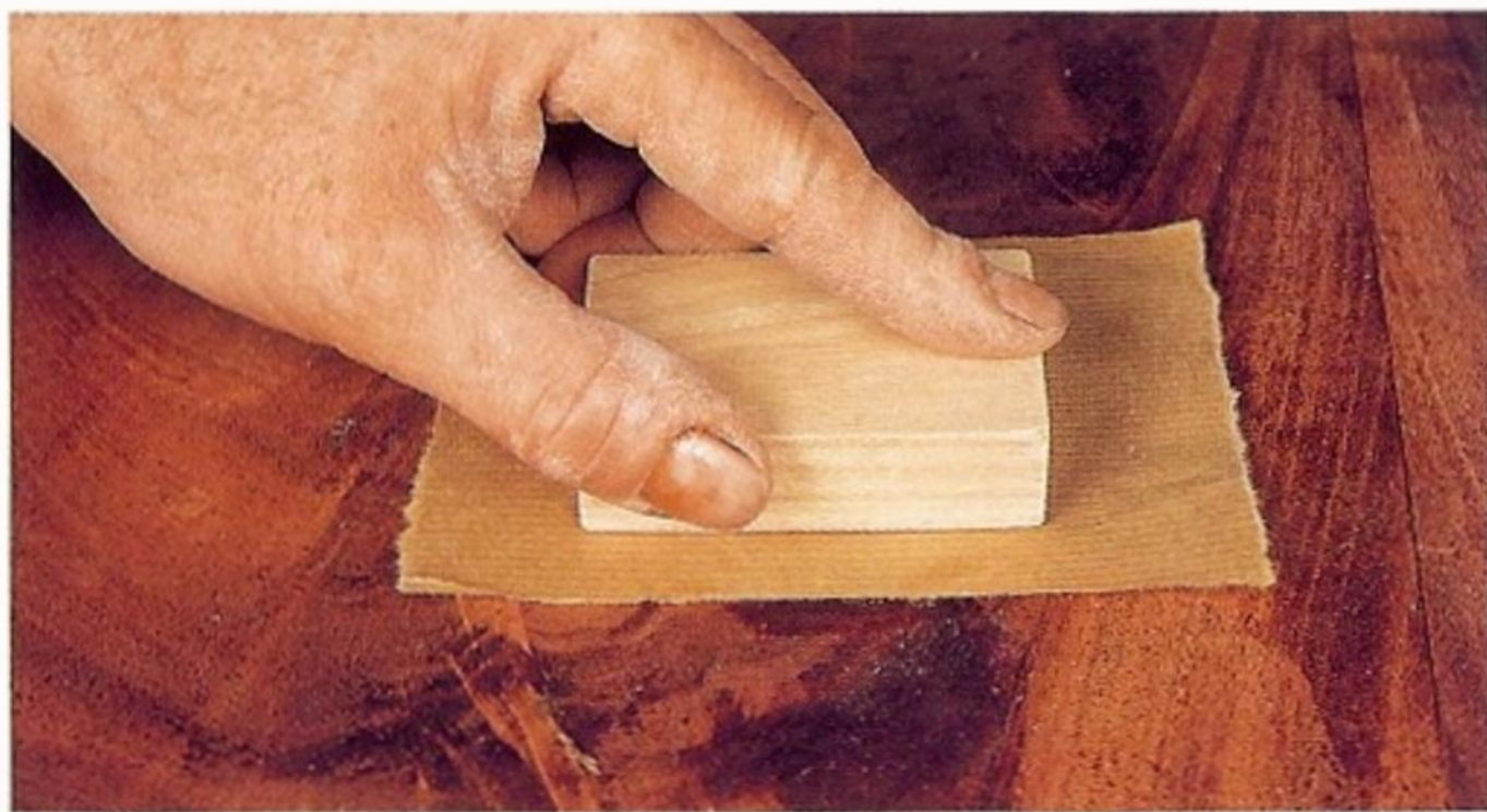
Fig 4.34 Pressing down blisters. Note the paper which prevents the wooden block sticking to the veneer.
