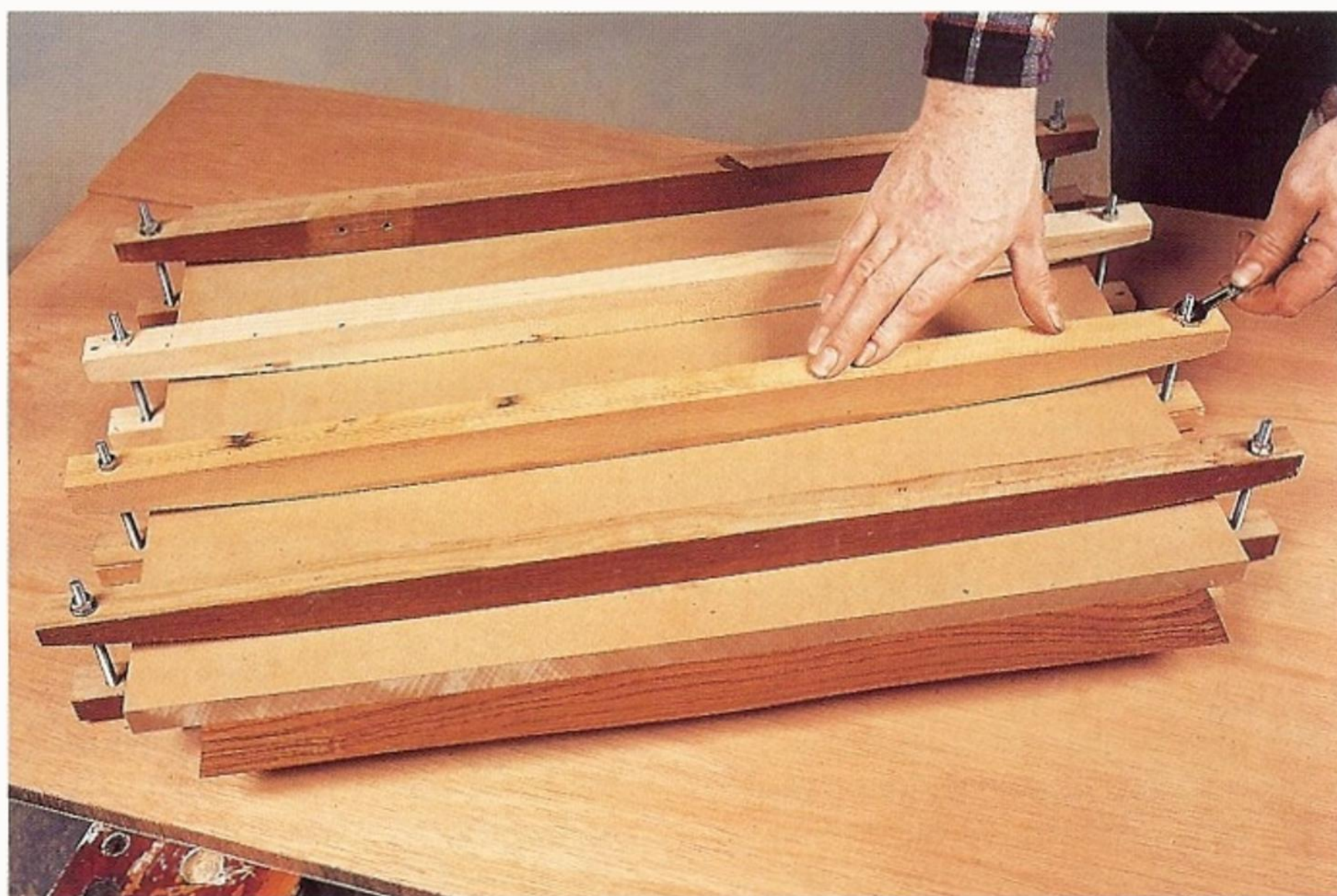
Fig 4.27 Tightening the bolts on the bearers to generate pressure.
