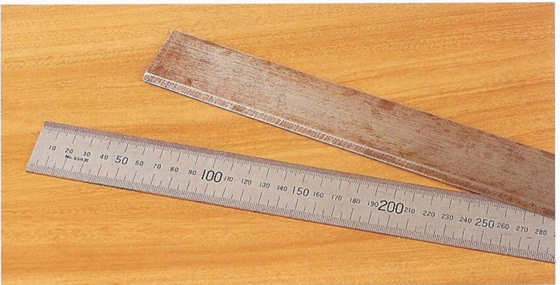
Fig 2.4 Top: Engineers' rule. Bottom: Straightedge.
