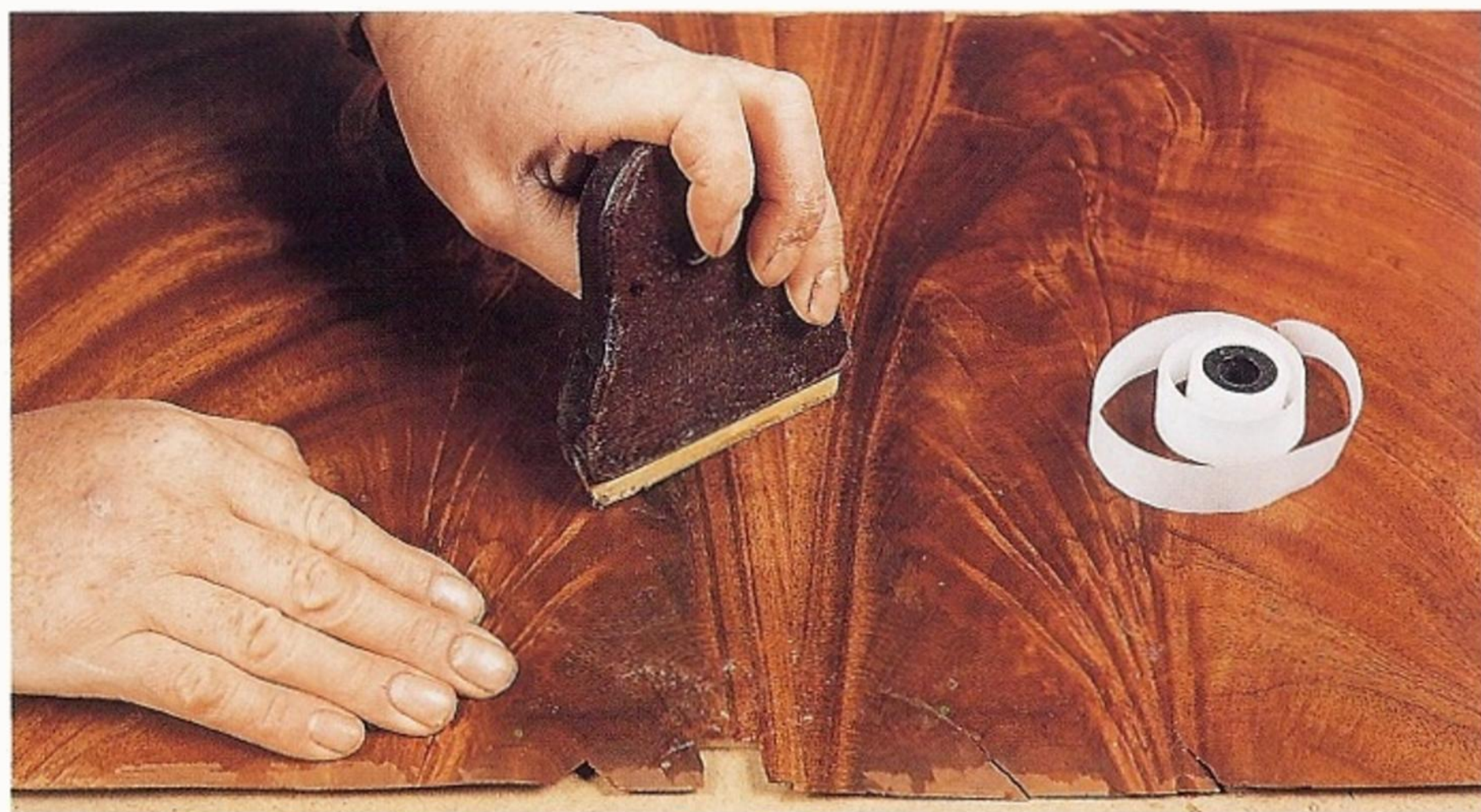
Fig 4.25 After removing the waste, iron the joint to re-heat the glue and hammer the edges down. Tape the joint to prevent it opening as the glue dries.
