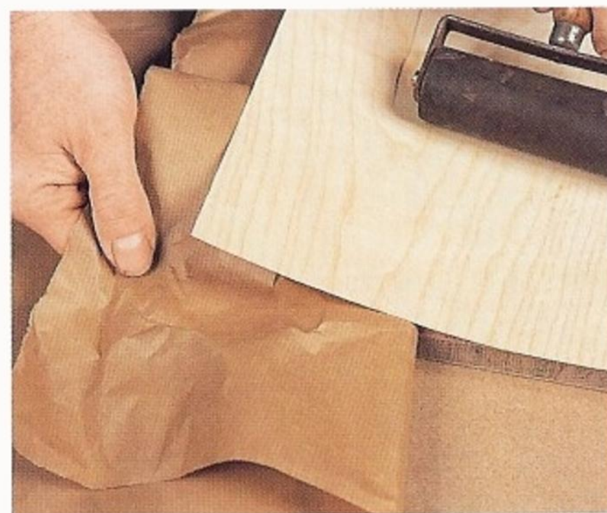
Fig 4.13 The slip method prevents premature bonding of the veneer to the ground, giving much more control over the process.
