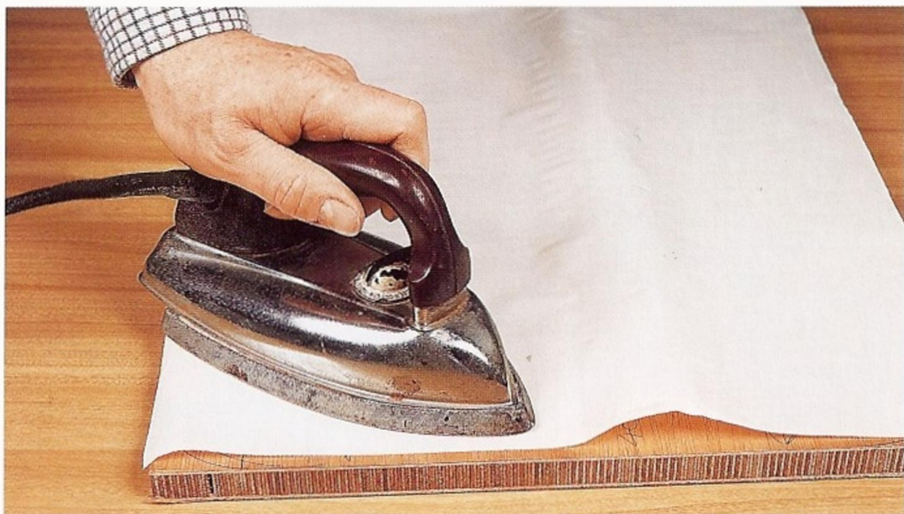
Fig 4.10 Transferring the glue from glue film to the groundwork. The iron is moved slowly over the paper backing to ensure that the glue melts.
