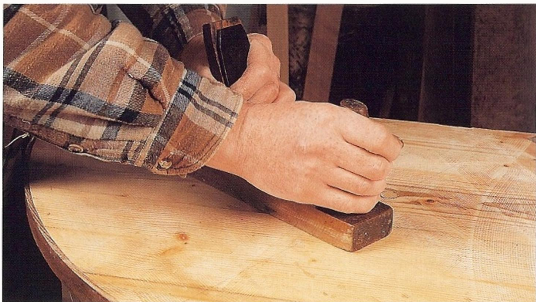
Fig 4.2 A tothing plane must be worked randomly over the entire groundwork to remove blemishes and possible high spots.
