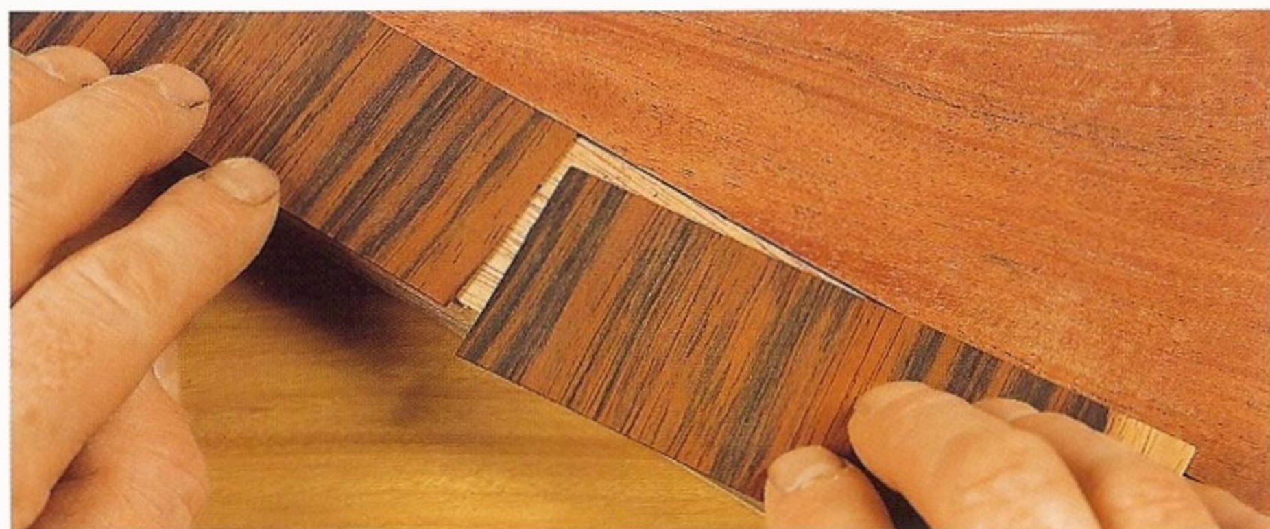
Fig 7.4 The cross-banding is offered up to the central panel.
