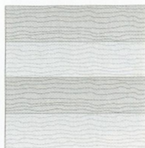
A Cut strips of light and dark veneers, the width of each being equal to the sides of the chessboard squares, then tape alternate strips together.
