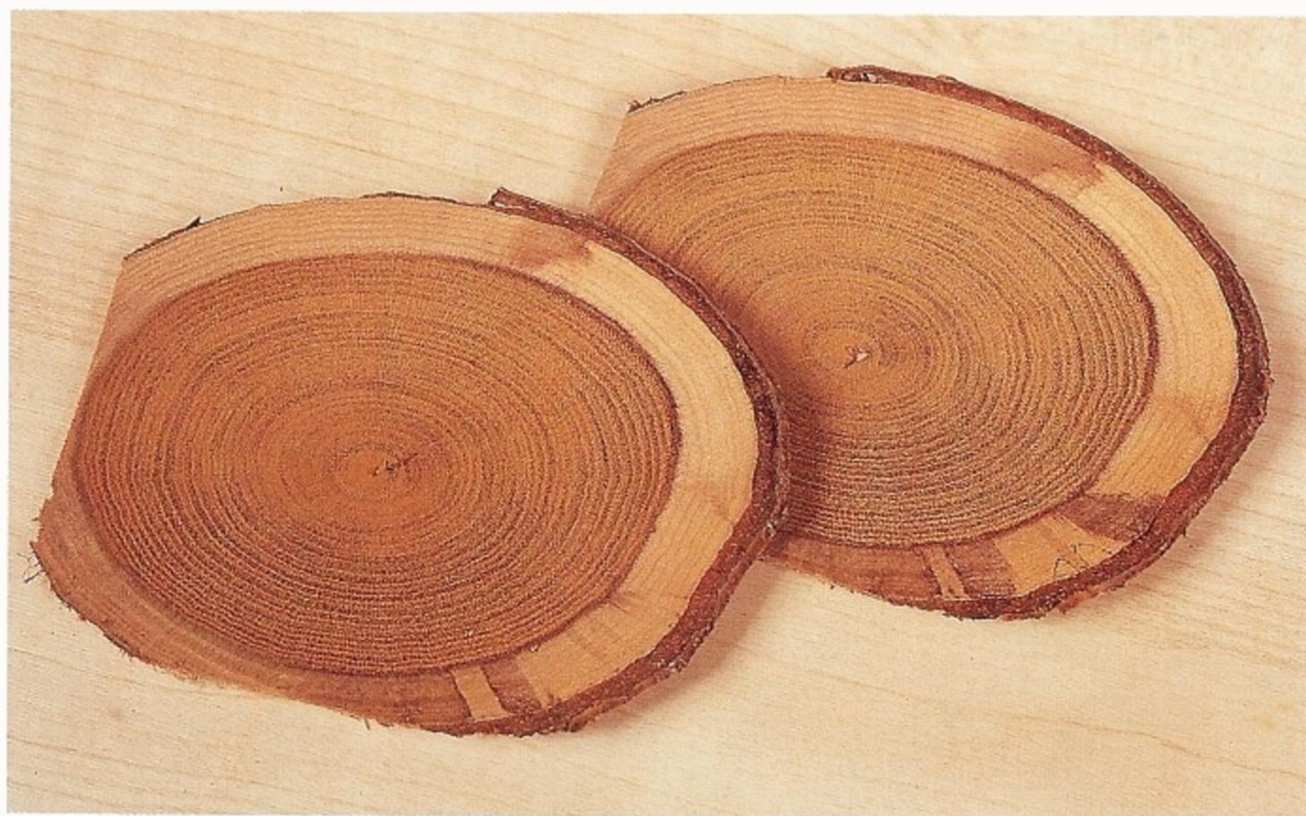
Fig 1.9 Oysters are produced by cutting across narrow diameter logs, either at right angles to the length of the log or obliquely across it. Laburnum and holly are traditional timbers for this, but any narrow log can be used to create oysters.
