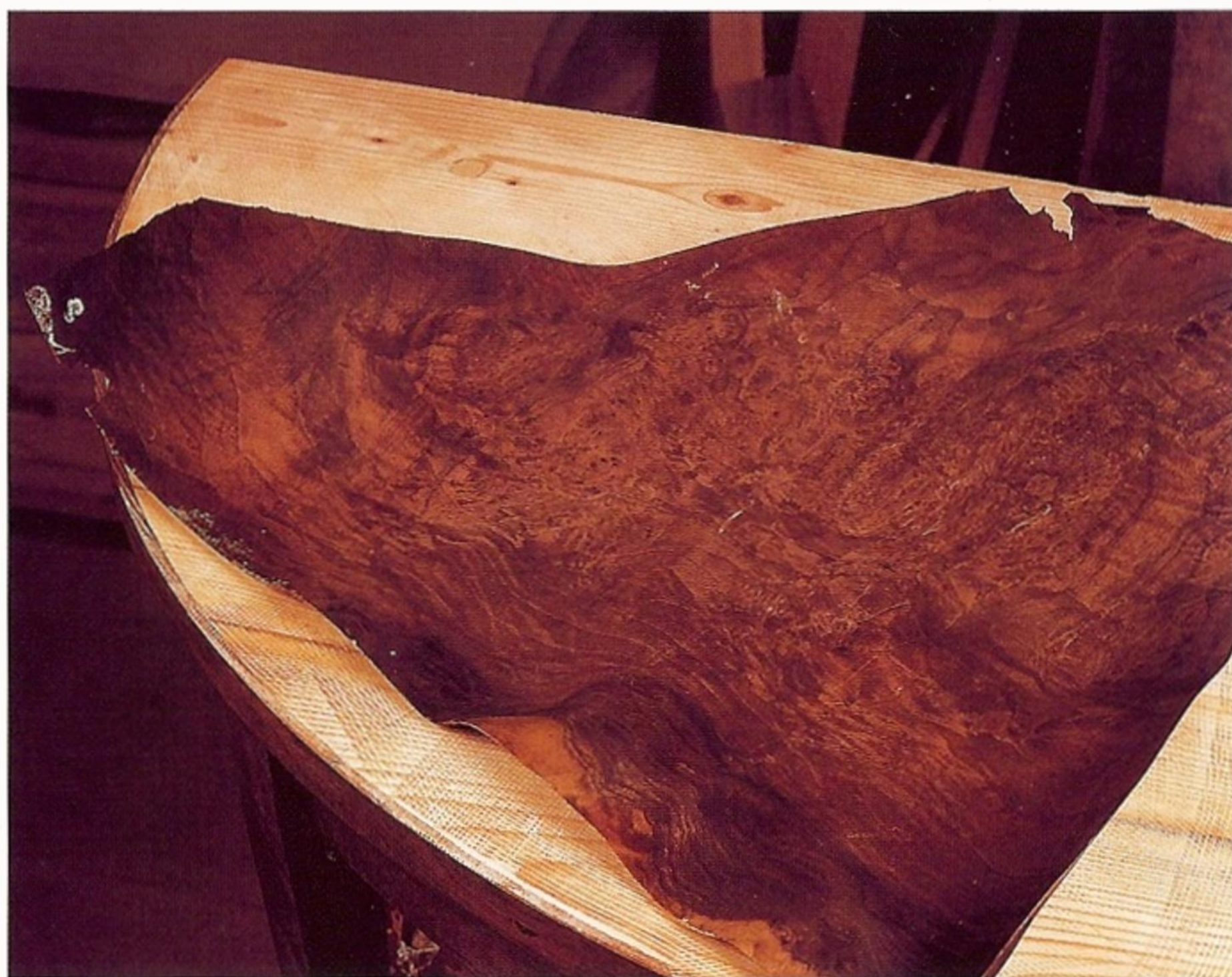
Fig 3.9 This buckled piece of burr walnut needs to be flattened before it can be laid.
