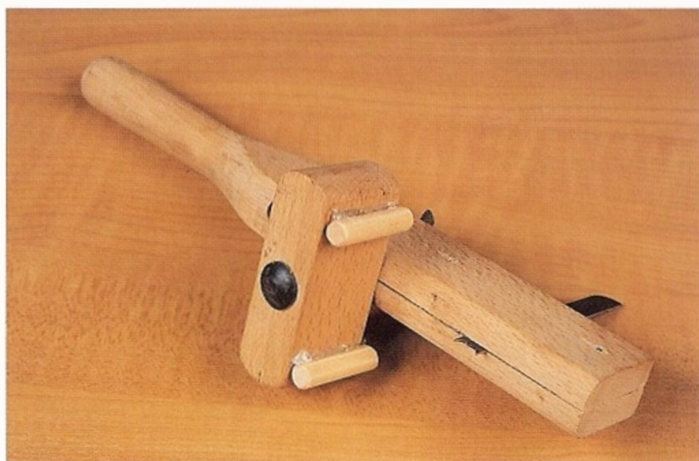
Fig 7.11 A specially made scratchstock for circular work.
