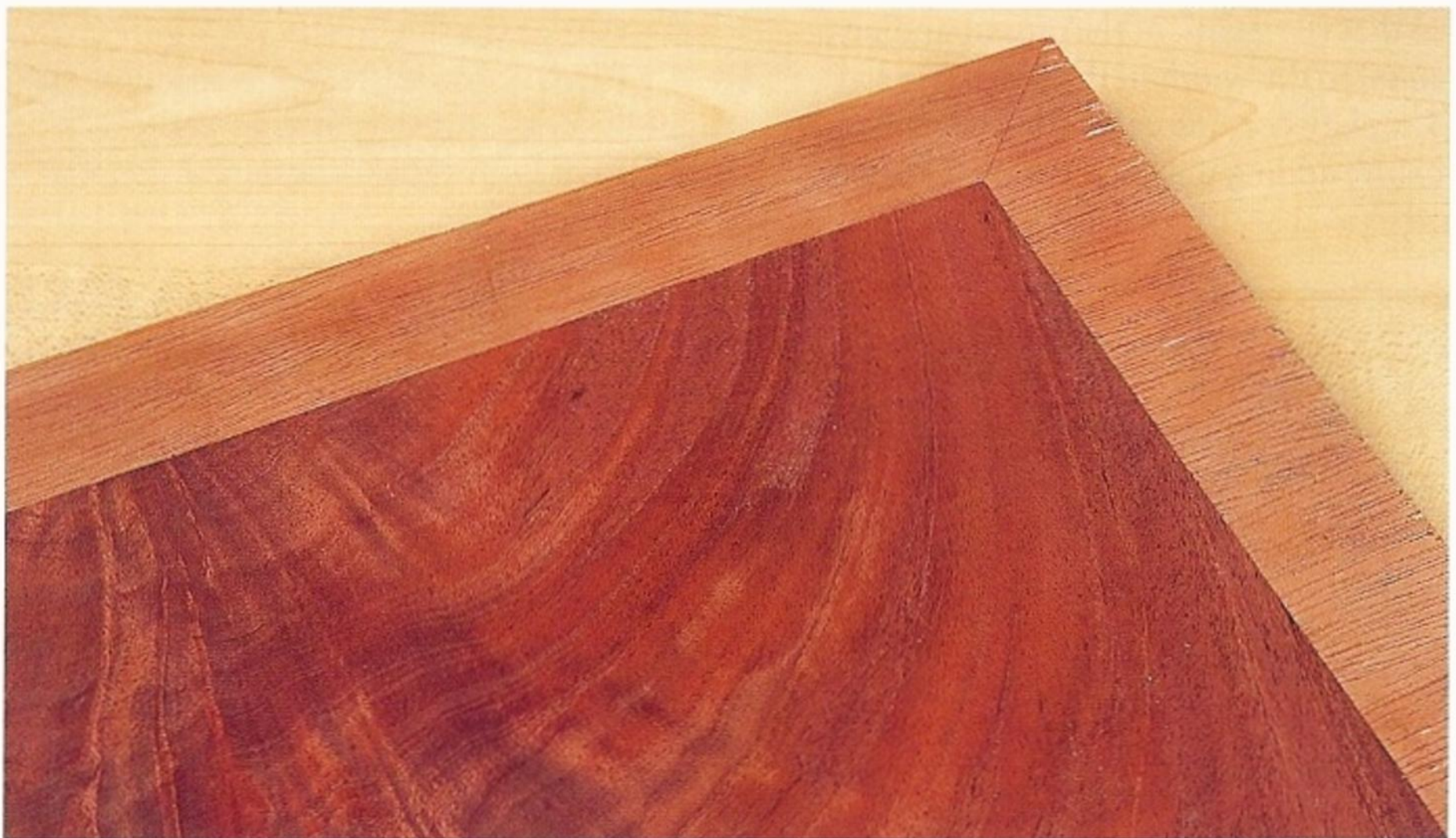
Fig 5.3 The central panel of veneer stands some way in from the edge.
