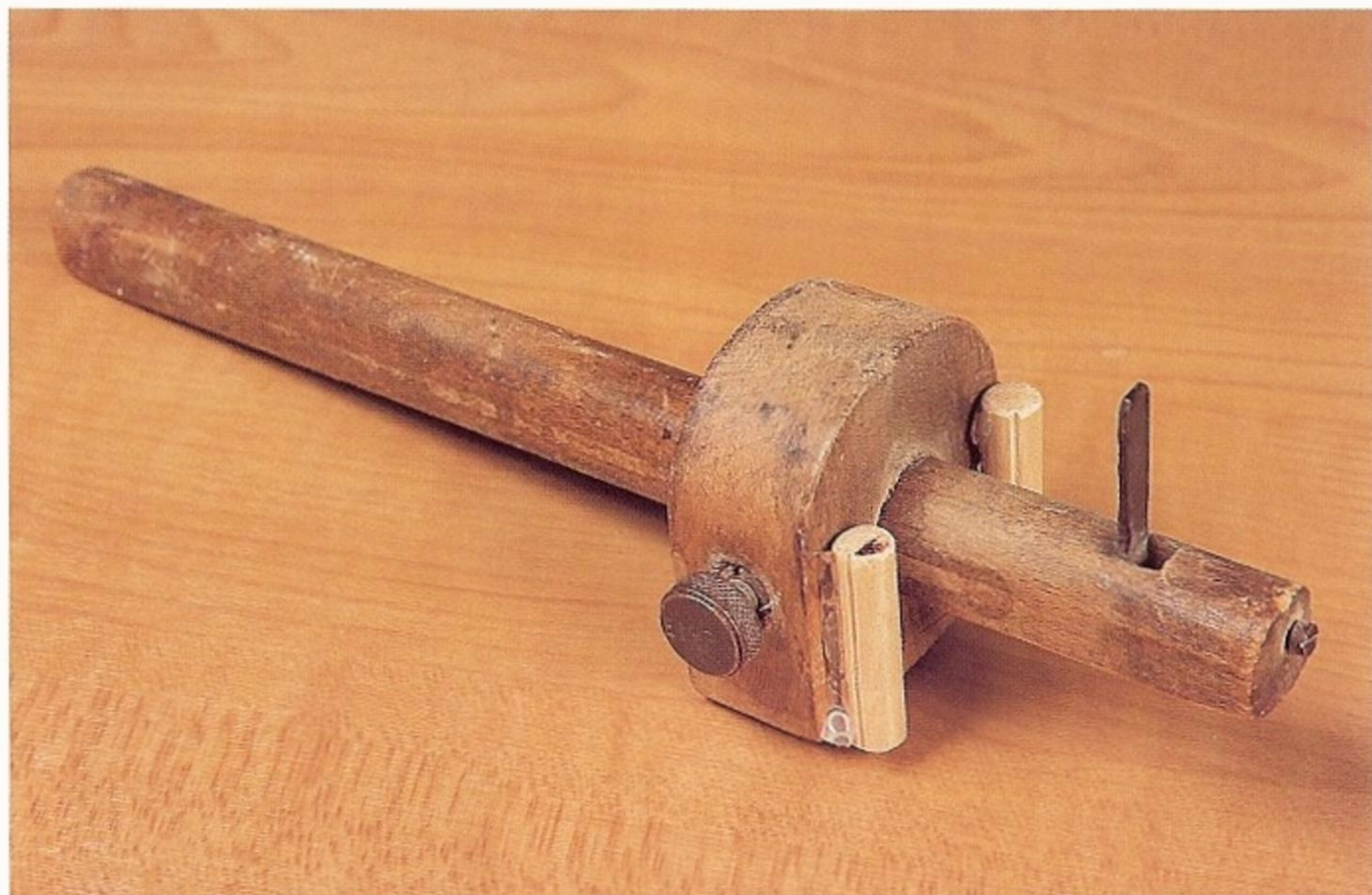
Fig 5.14 A modified cutting gauge for working with curved groundwork.
