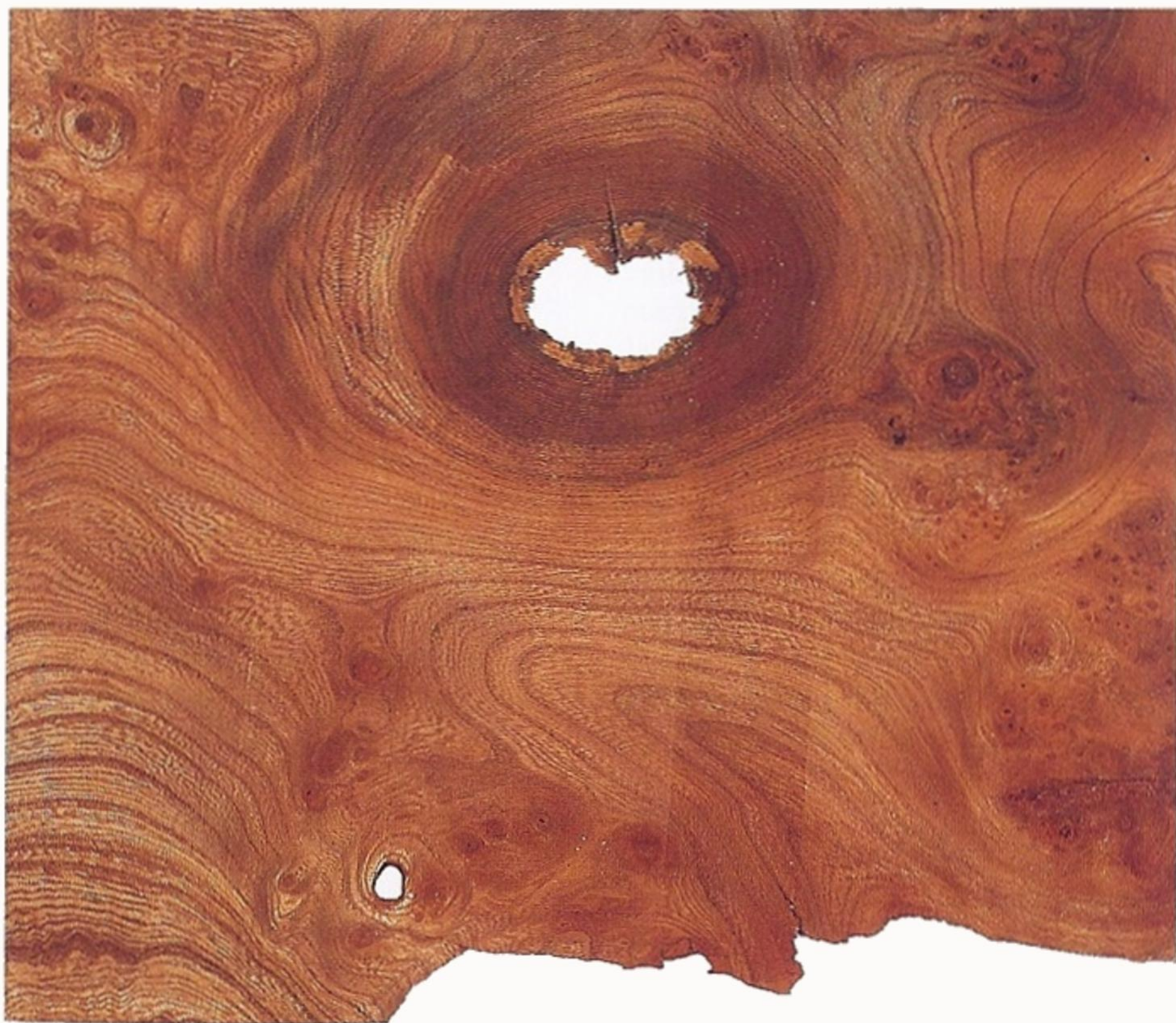
Fig 3.7 Burr veneers (elm in this case) are prone to naturally occurring holes.
