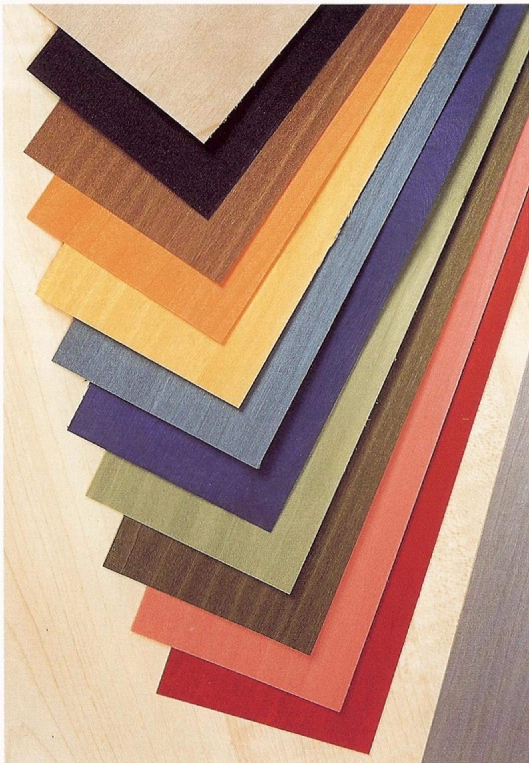
Fig 3.10 These brightly coloured veneers have been produced by soaking sycamore veneer in water-soluble aniline dye.
