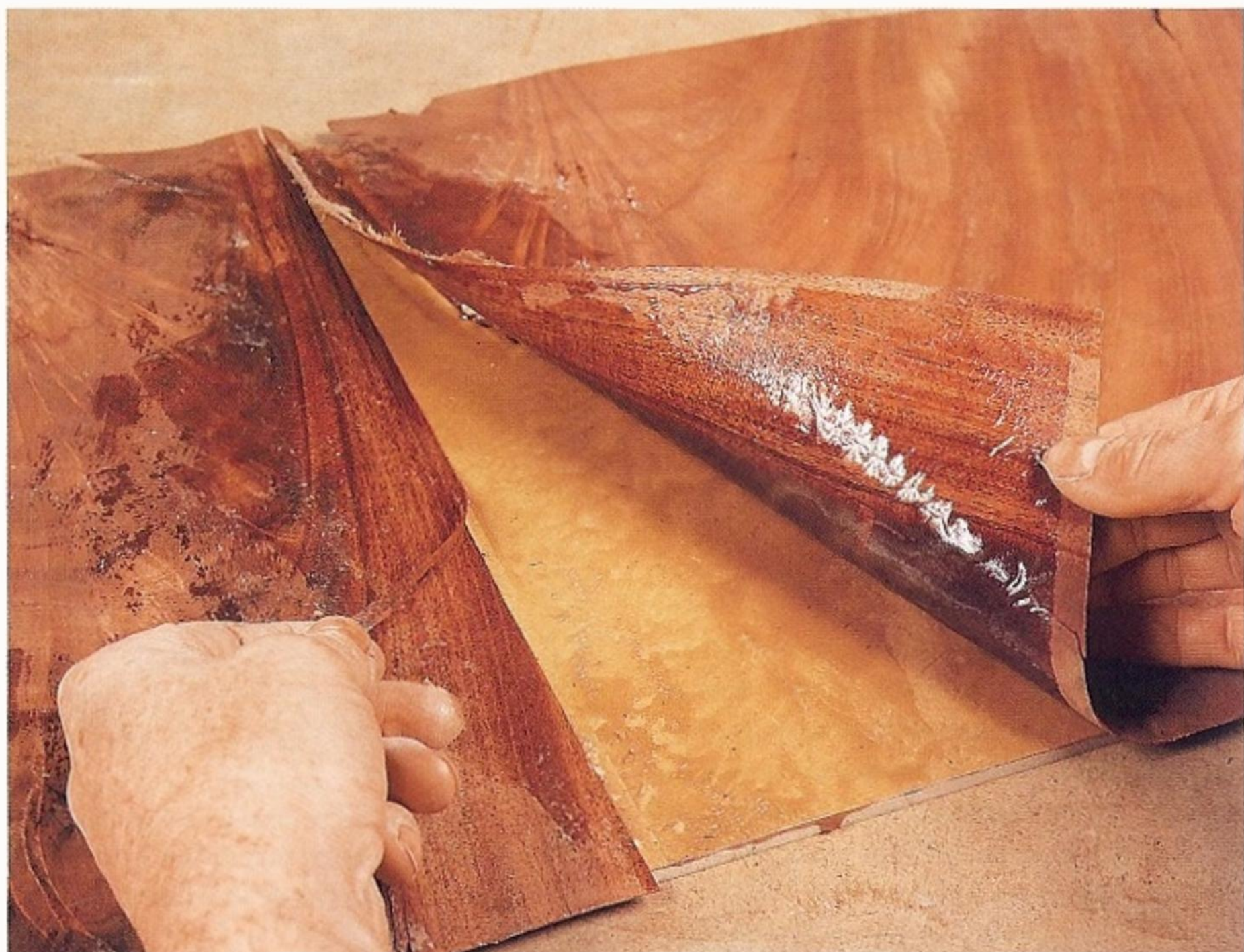
Fig 4.24 After removing the waste veneer from the top, lift the top veneer and remove the waste from underneath.
