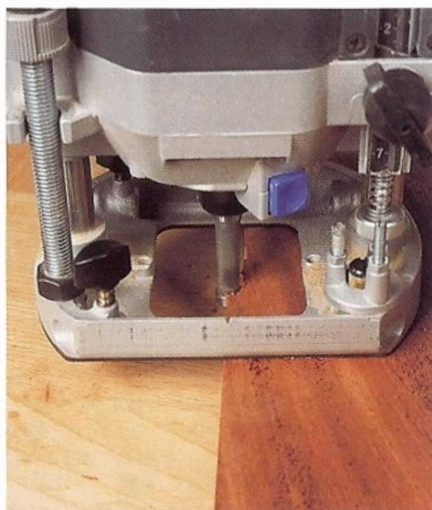
Fig 4.33 A self-guided laminate trimmer and router is ideal for quick and accurate removal of the excess veneer.
