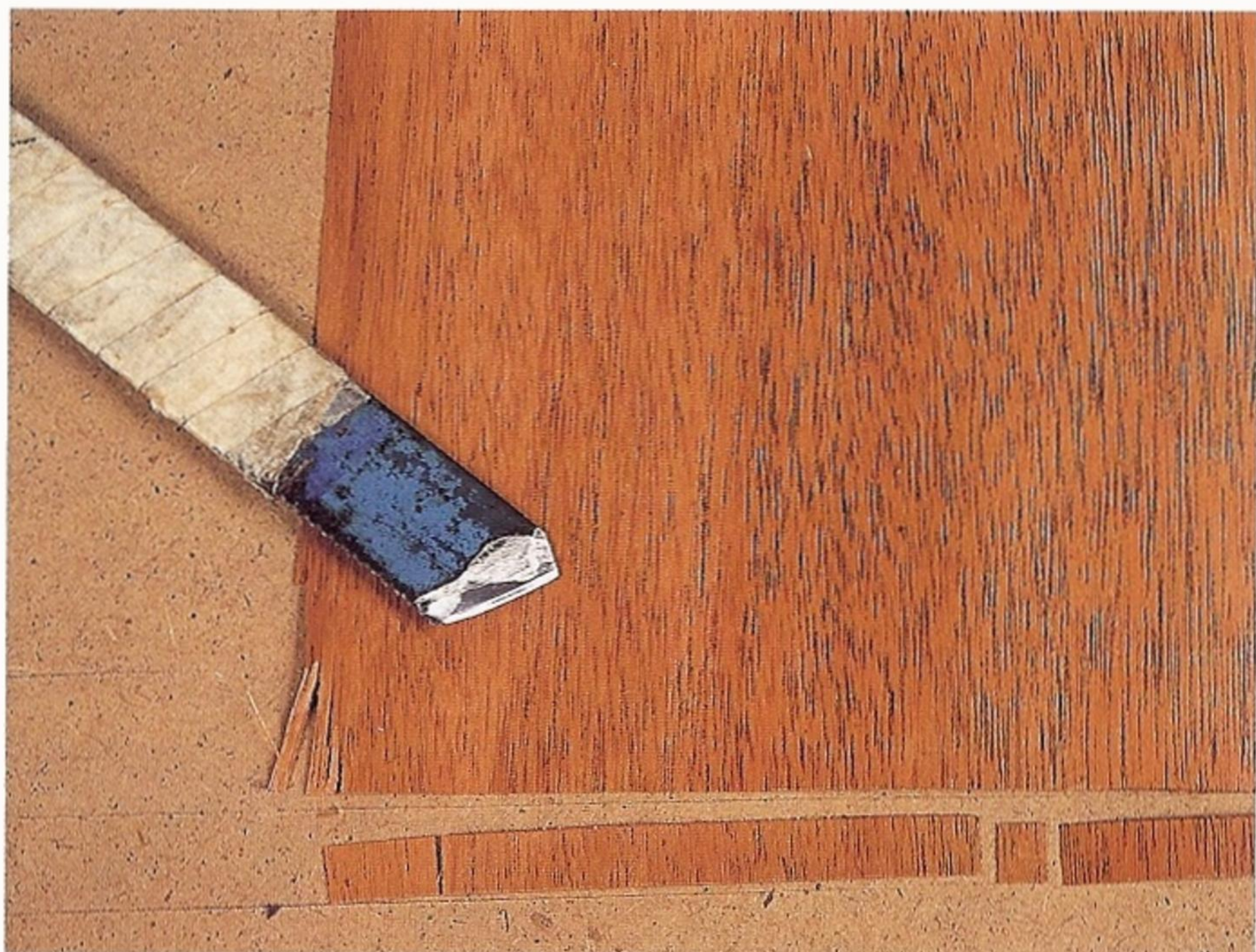
Fig 3.3 There is a high risk of the veneer splintering out at the edge when cutting across the grain.
