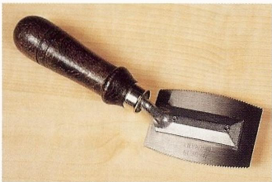
Fig 2.5 The curved blade of the veneer saw.
