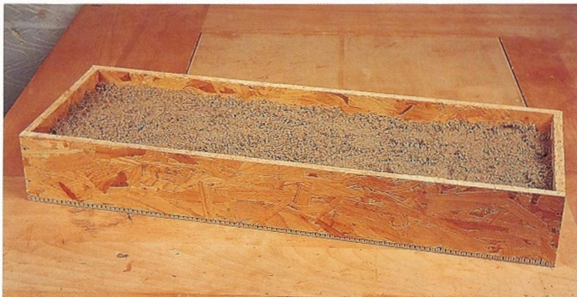
Fig 4.30 A sand box suitable for veneering the shaped groundwork.
