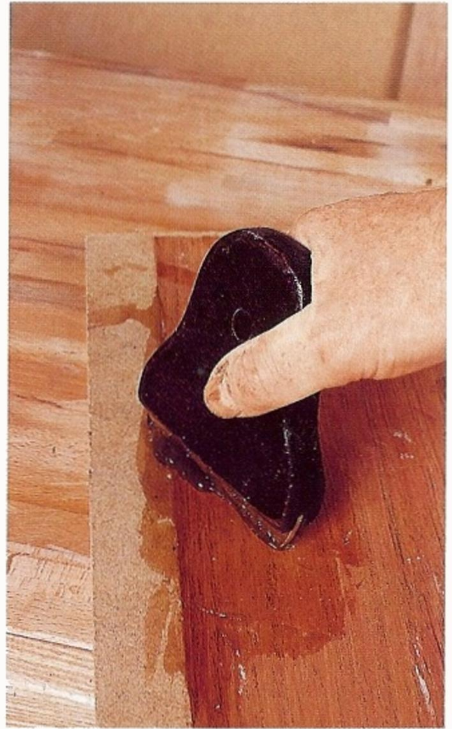
Fig 2.11 The brass strip in the veneer hammer creates the pressure to bind the glue and veneer.
