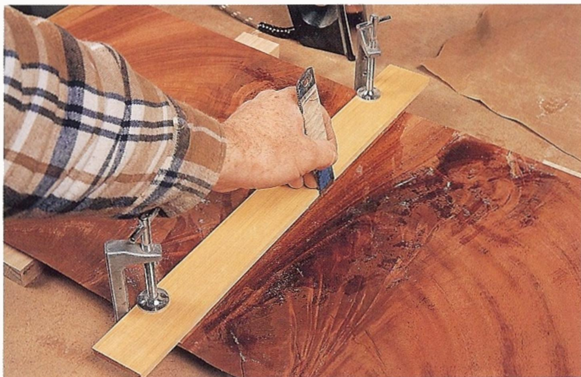
Fig 4.23 A veneer knife and clamped straight edge are used to cut through the overlapping veneers to make the joint.
