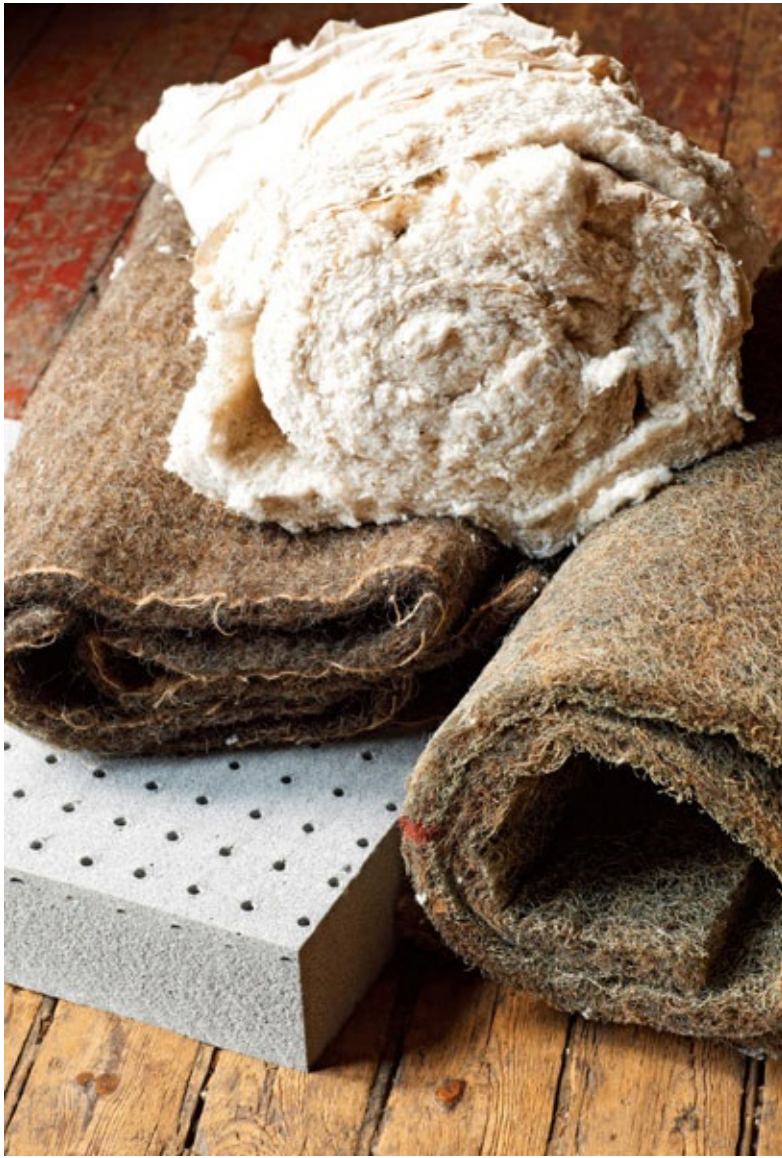
Latex rubber sheeting, rubberized hair, horsehair on hessian and white cotton felt.
