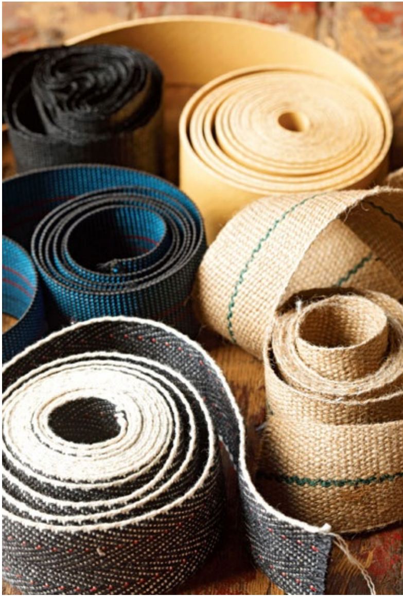
Traditional black-and-white webbing, jute webbing, elasticated webbing, rubber webbing and polypropylene webbing.
