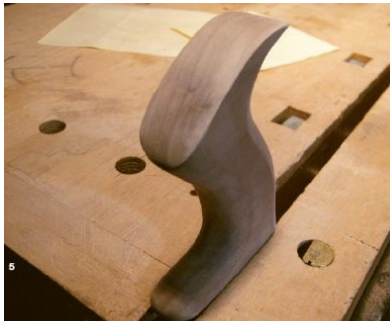
4. The tenon provides a grip for the vise while shaping the tote.
