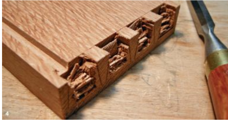
4. Chop out the waste in the drawer front after the tails have been carefully transferred over from the drawer sides.
