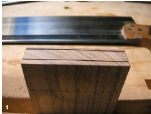
1. Saw the tenons in the apron stock. I use a 14-in. ripsaw for this size joinery.
