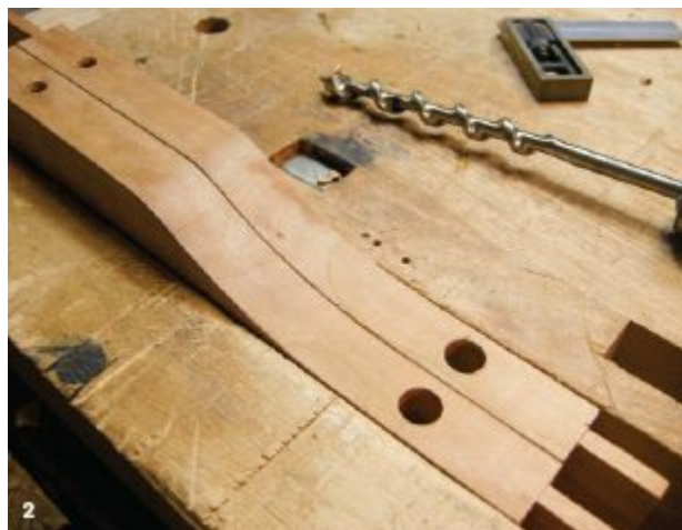
2. The \frac{5}{16} -in. holes for the support pins and the \frac{1}{2} -in. holes for the Roto hinges complete in the sides of the seat frame.
