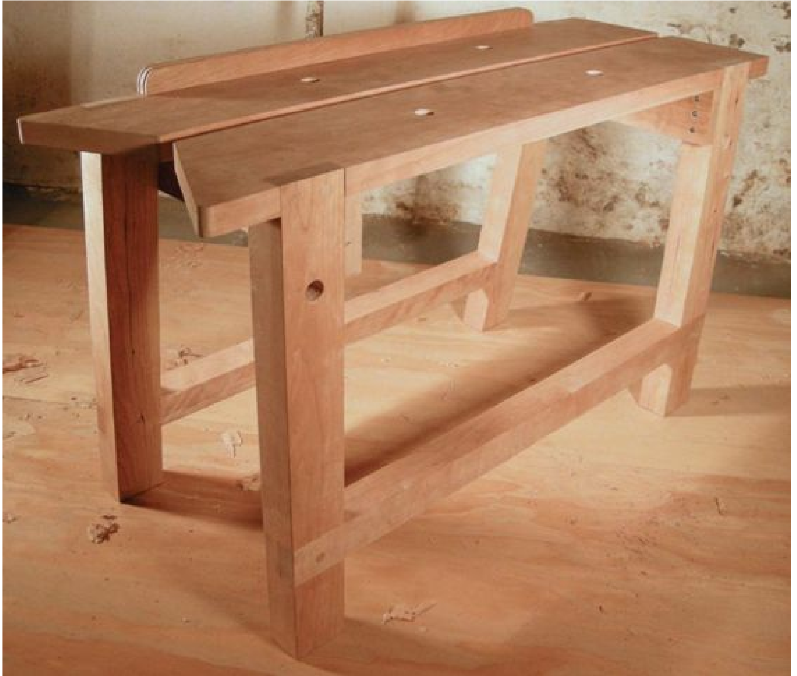
The finished saw bench in cherry.
