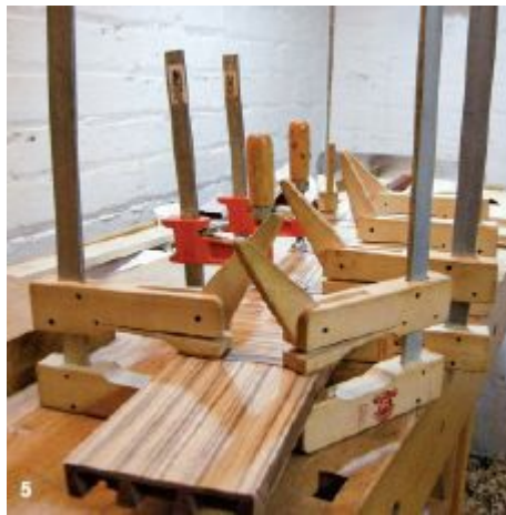
5. With its four false dividers, five alternating wood grain veneers, and large width, the lower drawer front is the hardest to make.
