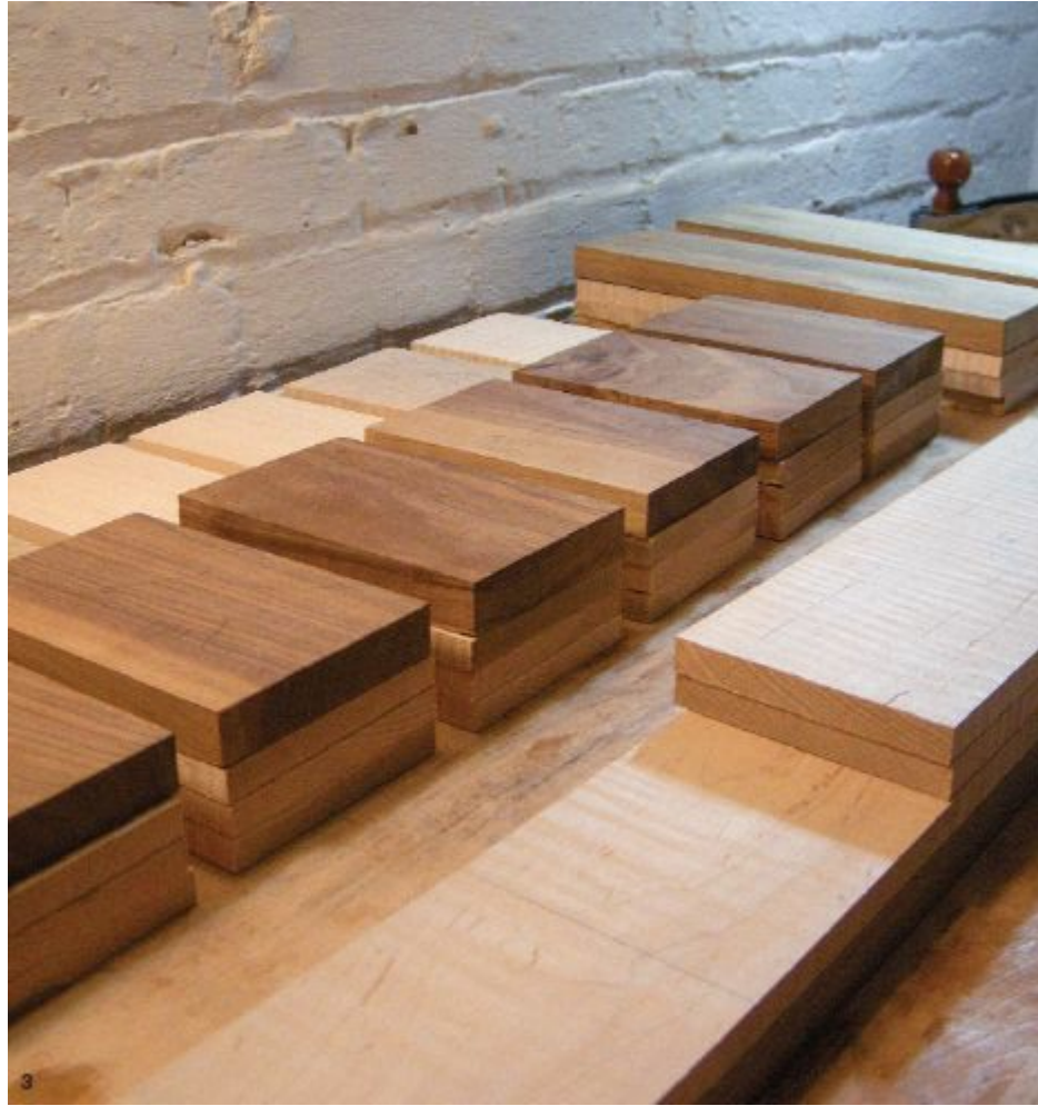
3. The drawer components are ready for dovetails after all of the parts have been carefully fit to the drawer openings.
