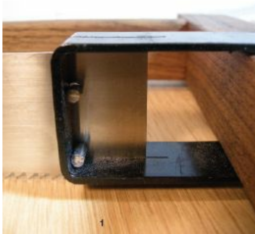
1. Properly seated, the \frac{3}{16} -in. retaining pins hold the saw plate tight against the bracket end wall.
