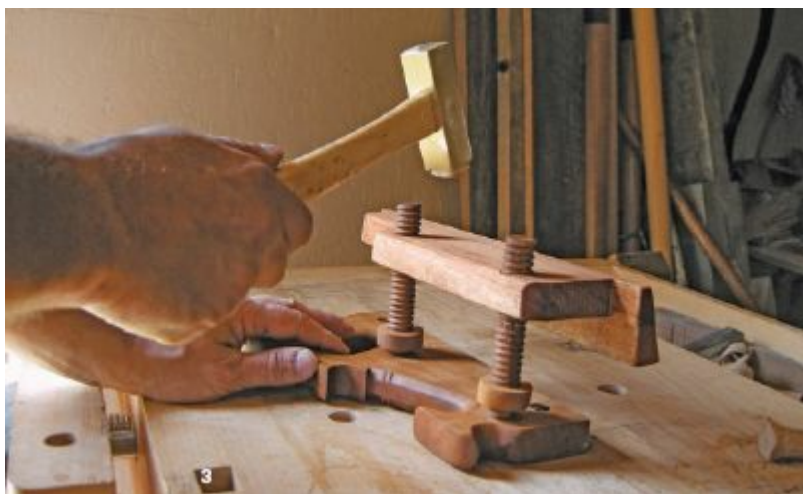
3. I use a small wood and brass hammer to tap the fence into position—similar to adjusting a wooden plane iron with a wedge. Set the bolts close and gently tap the fence to the final width of cut desired.
