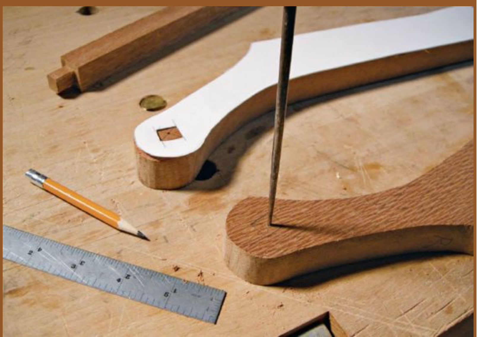
Paper templates assist in locating mortises in curved components (here, the top drawer-box supports).
