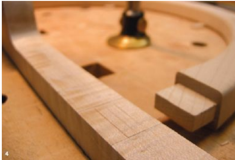
3. Before the final shaping, pin the bridle joints with wooden dowels.
