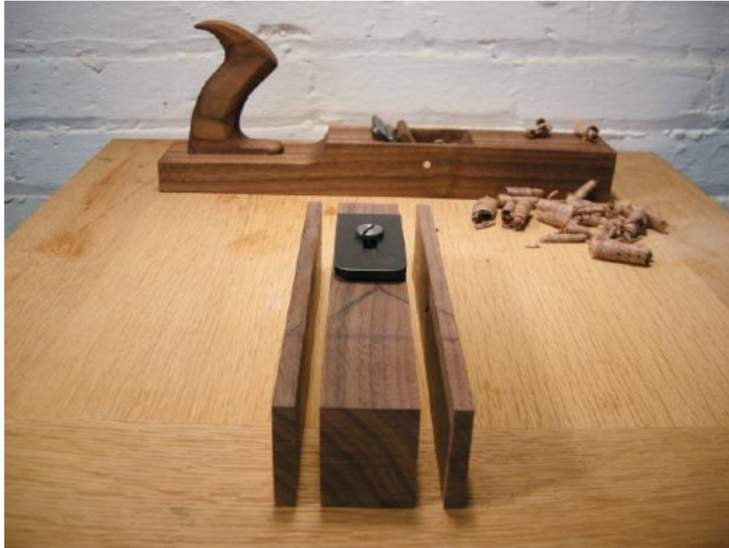
The raze plane (background) is ideal for flattening the parts of the high-angle smoother (foreground).
