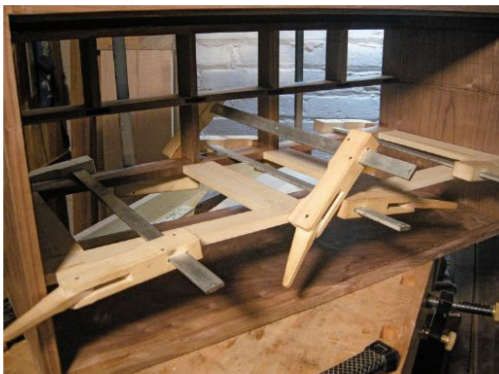
Gluing the lower assembly of runners and rear stretchers inside the carcass.
