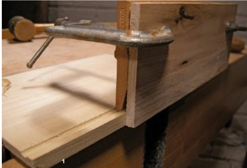
1. A makeshift fence guides the molding plane to begin the grooves.
