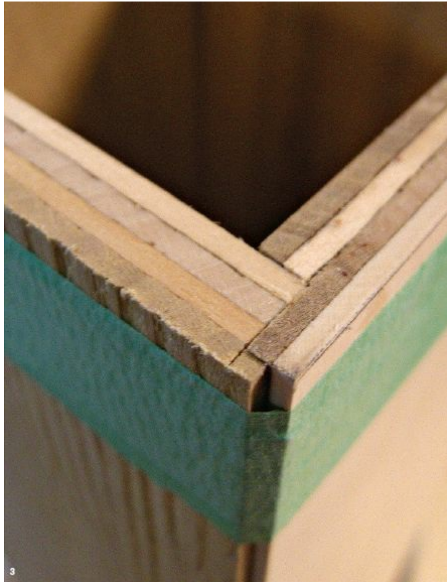
3. Detail of corner rabbet joint. The outside corner gap will be filled with \frac{1}{8} -in. banding after the boxes are glued.
