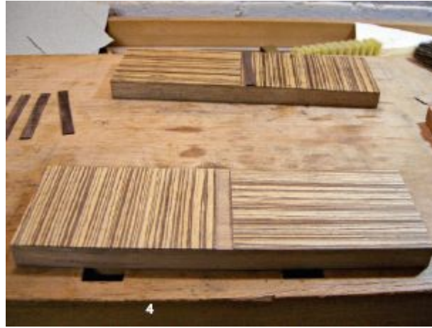
4. After the face veneer is applied to the drawer fronts, clean up the middle divider location before the false divider is glued in place.
