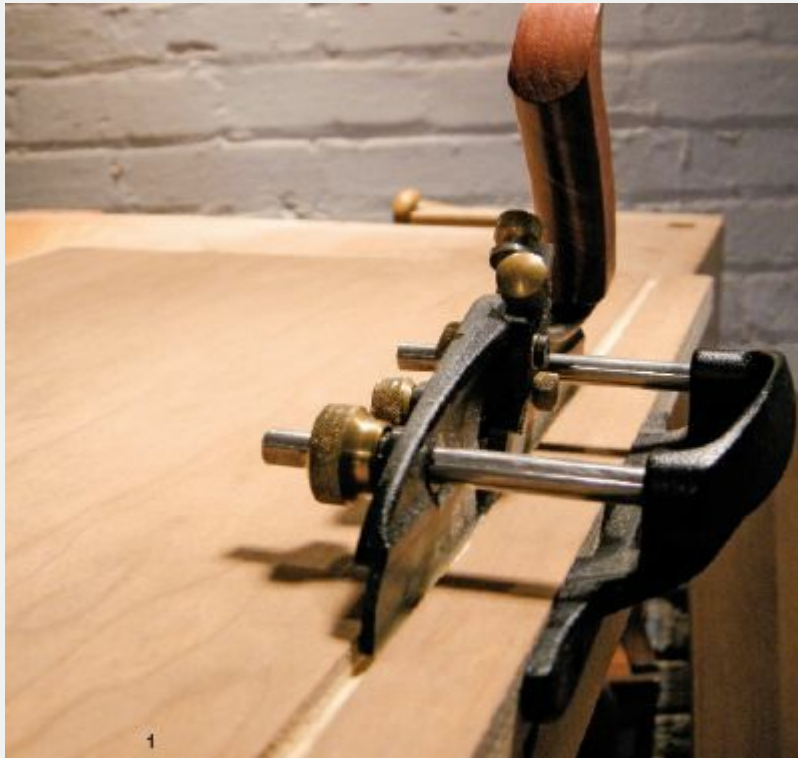
1. Cut a shallow groove into the plywood base using a plow plane.
