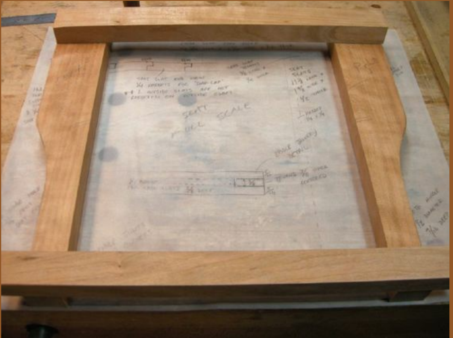
Chair frame parts ready for joinery.
