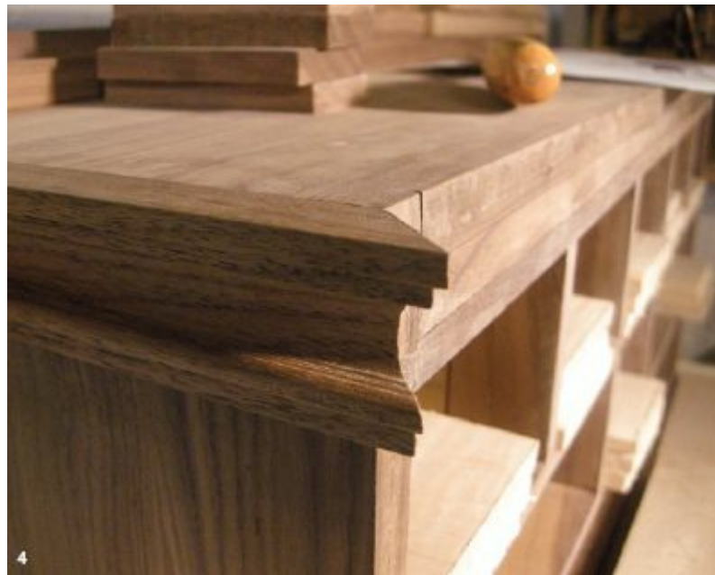
4. Dry-fit the sides of the molding and fine-tune the front for a perfect fit.
