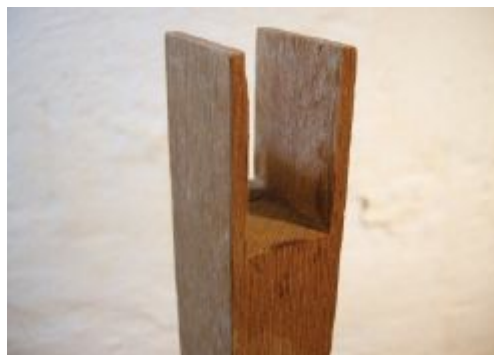
Rough out the top of the leg joint where the drawer-box supports are attached.
