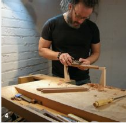
4. The dogs make the process of rounding furniture parts easy and enjoyable.
