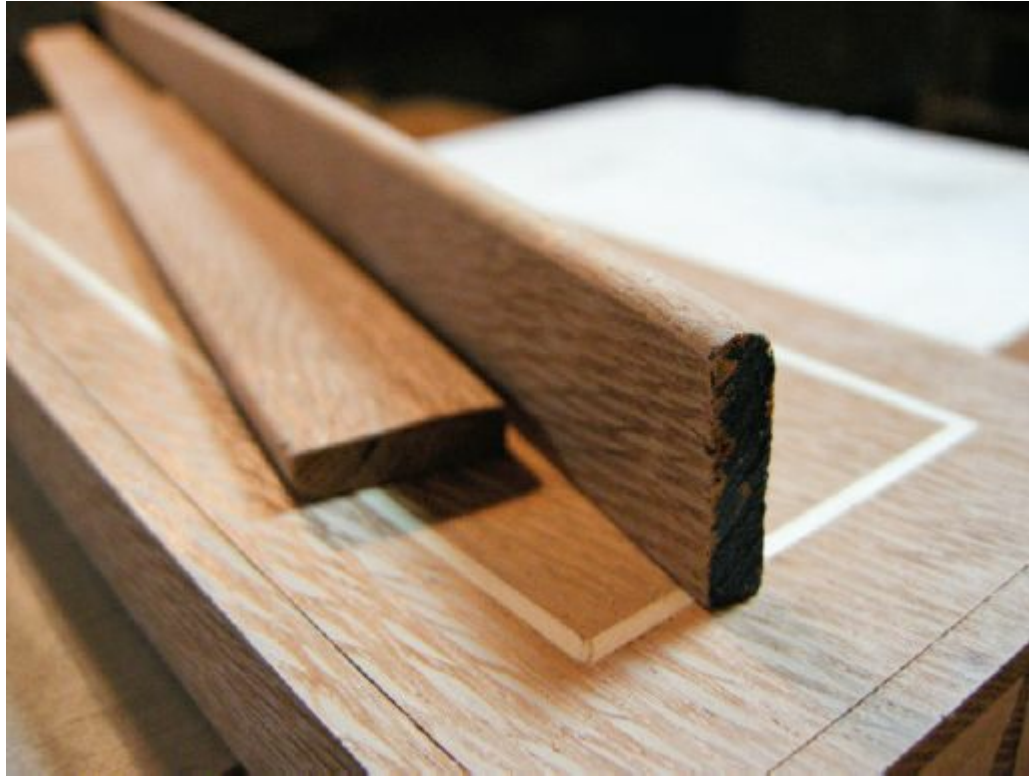
Prepare the beading stock and cut scribe lines around the drawer face.
