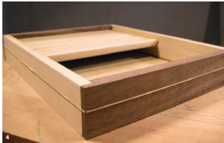
4. Once all the grooves are cut, dry-fit the drawer with the pencil tray.
