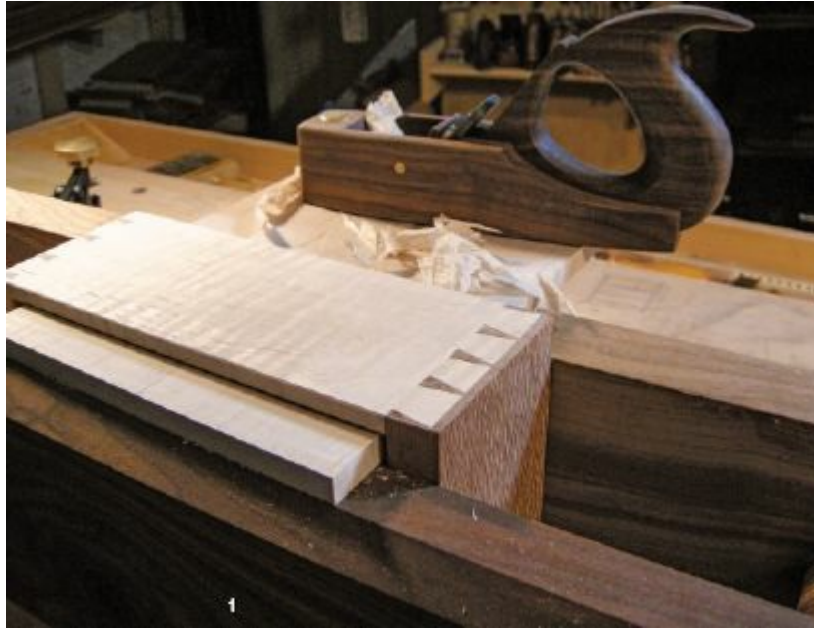
1. Plane the drawer sides flush with the front. The high-angle smoothing plane is perfect for dealing with these curly maple drawer parts, and the lying press and a hardwood support block make this process easier.
