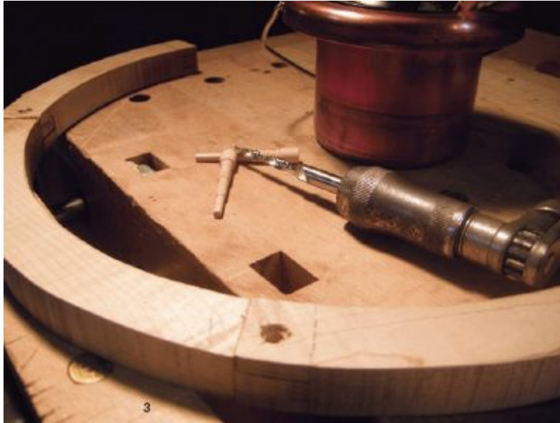
3. Before the final shaping, pin the bridle joints with wooden dowels.
