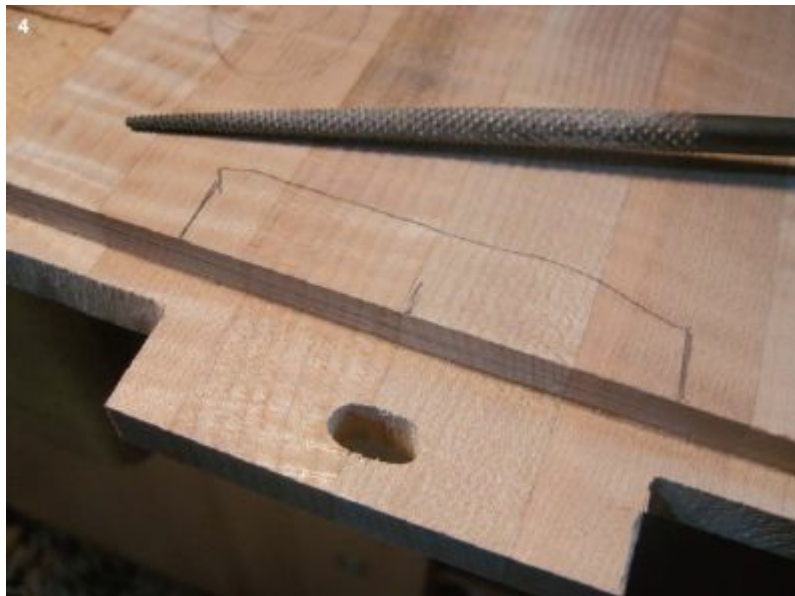
3. Detail showing breadboard end mortises and drilled tenons.
