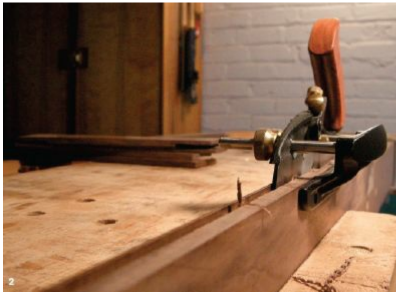
2. Plow a \frac{3}{16} -in.-deep groove for the back panel in the frame parts.
