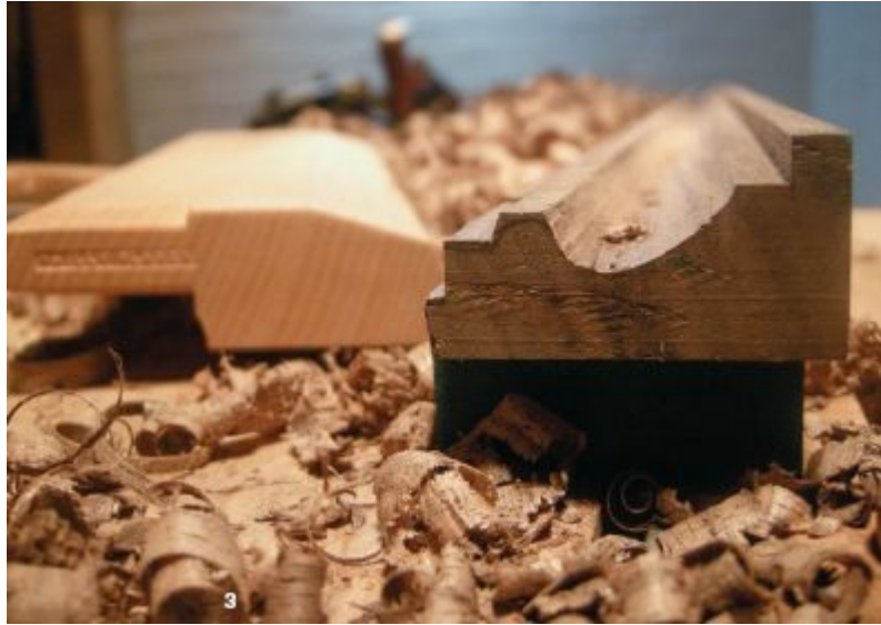
3. After the rabbets are made, molding planes are used for the inside round areas.
