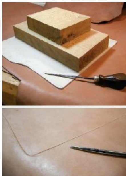
Weight the card stock pattern with oak blocks to make sure it will stay put while you scribe the shape with an awl.
