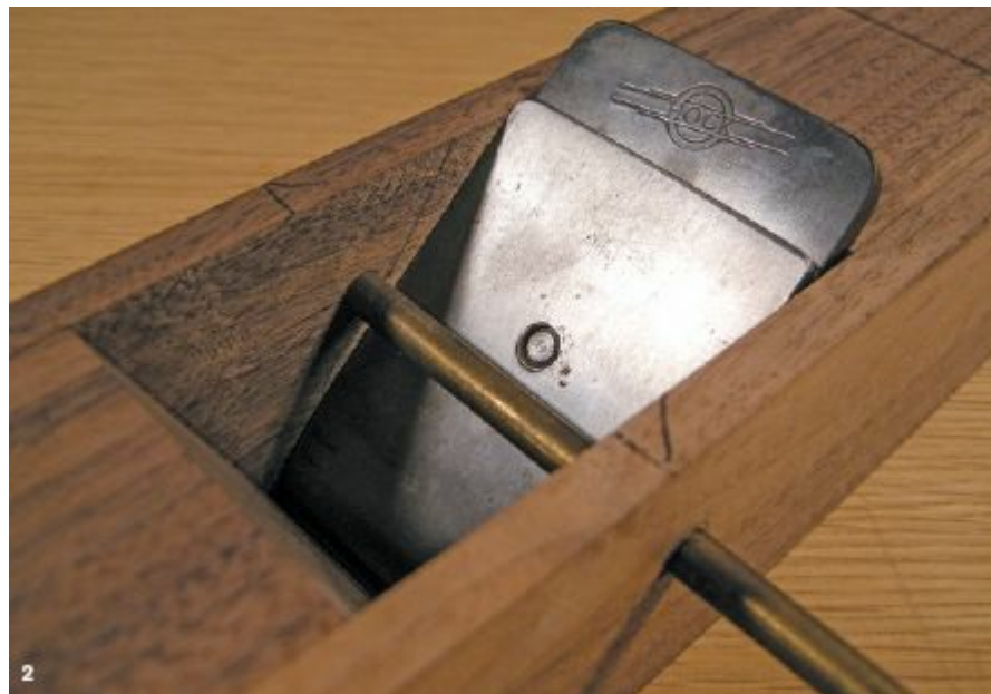
2. Drill the holes in the cheeks, insert the brass rod, and mark it for proper length.
