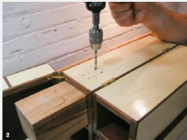
2. Drill the matching holes in the chest sides. The block inside the chest helps prevent any blowout on the inside of the chest sides while drilling.
