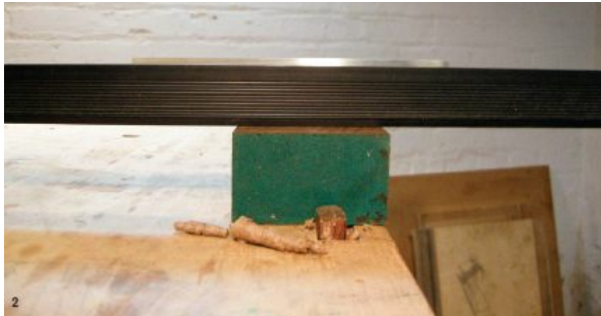
2. Plane diagonally between these areas and then the full face again until you see a flat face.
