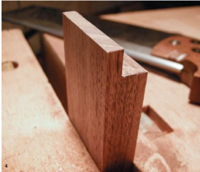
4. Rip-cut the cheek and, as always, fine-tune the joinery with a sharp chisel and check it for square.
