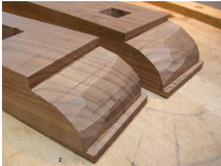
2. The profiles on the toes are roughed-out quickly with a bowsaw and then some quick paring cuts with a chisel. I like them like this.
