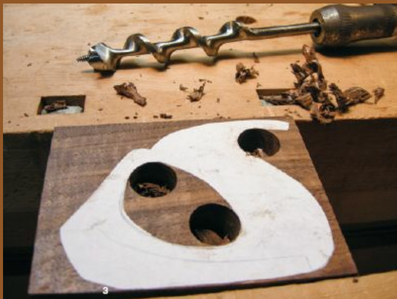
3. Glue the pattern directly to the walnut blank and establish the round sections of the tote with an auger bit.
