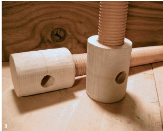
2. Boring the hub holes at a slight angle (about 2° off of 90°) keeps the handles away from the jaw while in use.
