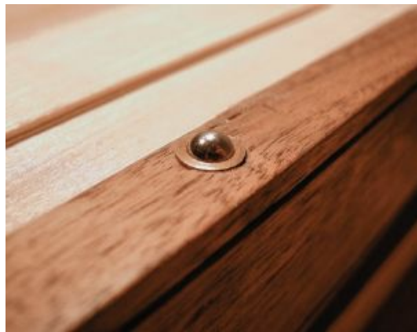
Install a bullet catch in the drawer front bottom to keep the drawer in place when transporting the box.
