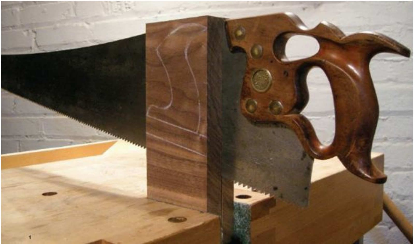
1. Resaw the blank stock for the rear tote. The second line underneath the tote marks the tenon that will be mortised into the rear of the plane body.
