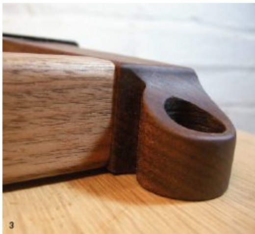
3. The side arms are rounded and shaped so the union between the two parts is protected but softened.
