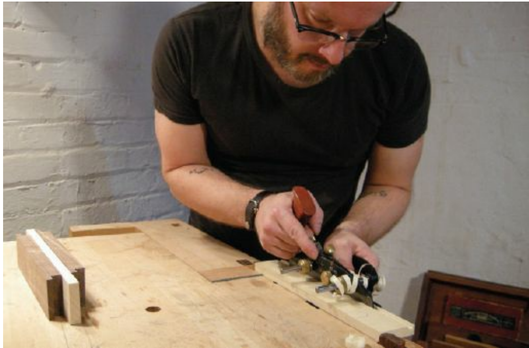
A plow plane makes quick work of the grooves for a drawer bottom. The fence and depth stop ensure accurate results.
