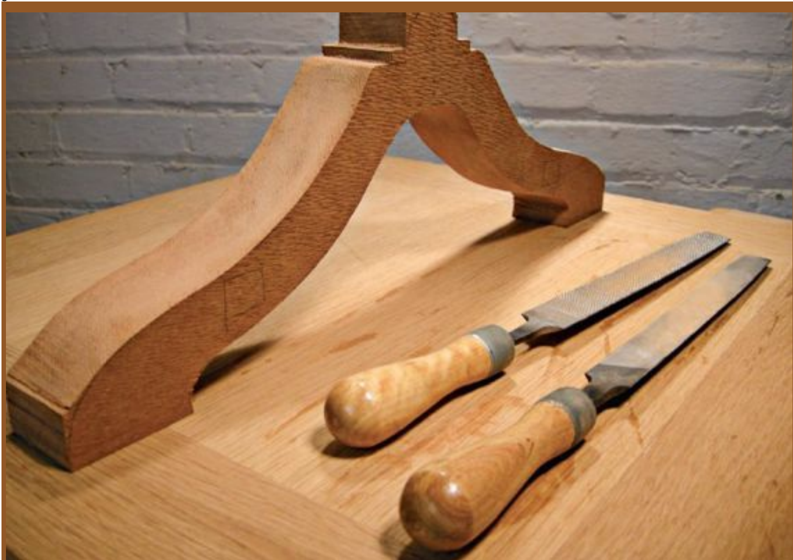
Use rasps to define the curves after rough sawing.
