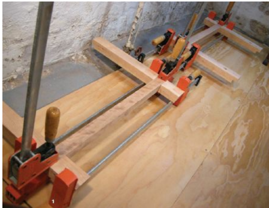
1. Assemble the legs and stretchers first; clamp and leave to cure overnight.
