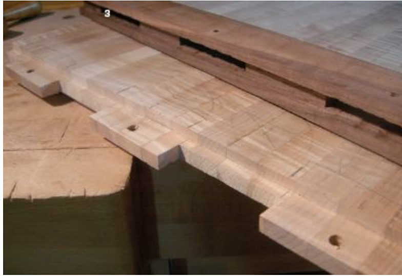
3. Detail showing breadboard end mortises and drilled tenons.
