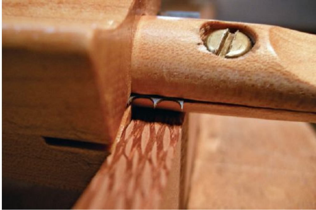
A special-purpose cutter in a beading tool is used to profile the moldings.
