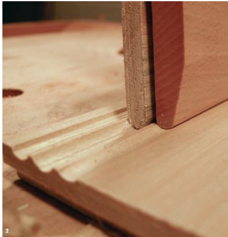
2. The fence rides in each groove as you work across the tray.
