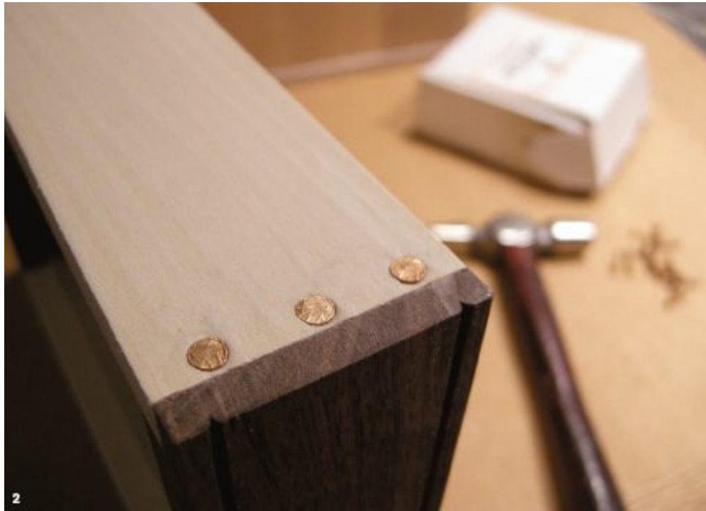
2. Silicon bronze ring nails will hold this drawer together for years.
