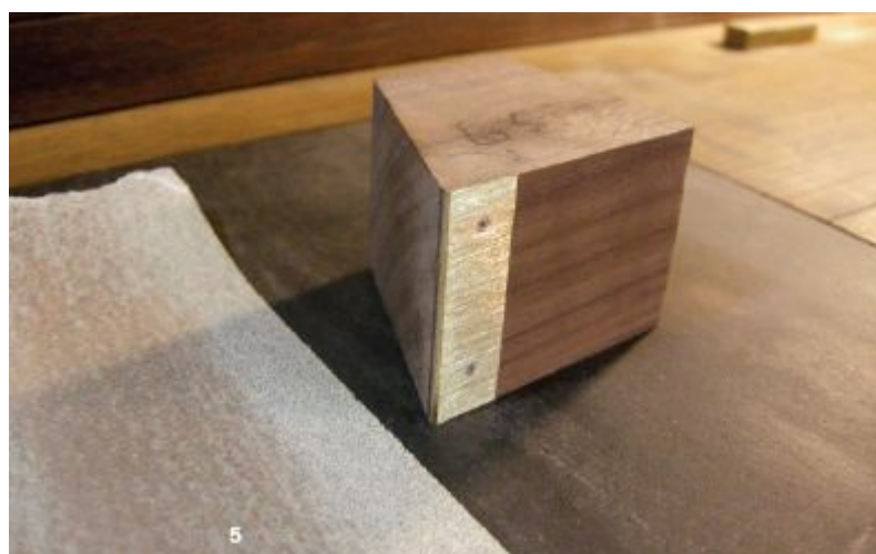
5. True the blank on sticky-backed sandpaper applied to granite slab.
