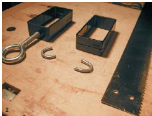
1. Bend the steel rod for the retaining pins using a metal bending jig. (This one is available from Lee Valley Tools.)
