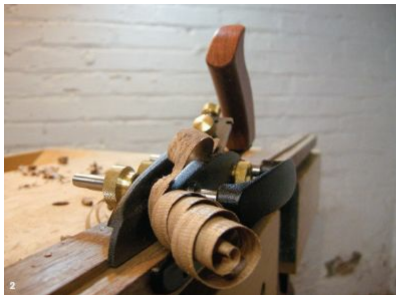
2. For the initial molding, a plow plane begins the excavation and establishes the first groove, or fillet, at the top of the molding profile. Follow with a rabbet or moving fillister plane to knock down the main face of the molding. From here, three more rabbets were made to define the bead along the bottom.
