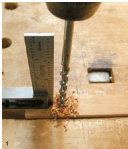
1. A small square set on the workpiece helps maintain square as you drill.
