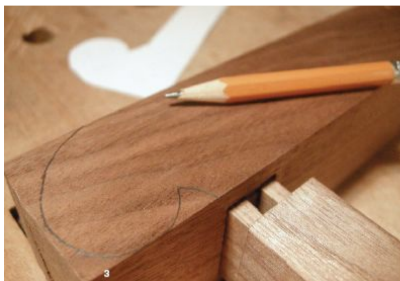
3. I used a French curve to design a basic corner shape for the front arm. Make a full-size paper template and transfer the round corner shapes onto the frame.
