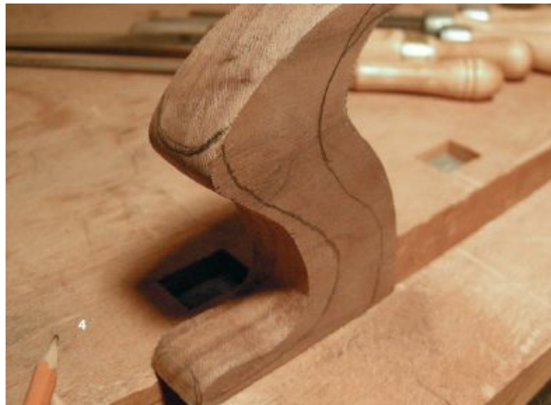
4. The tenon provides a grip for the vise while shaping the tote.
