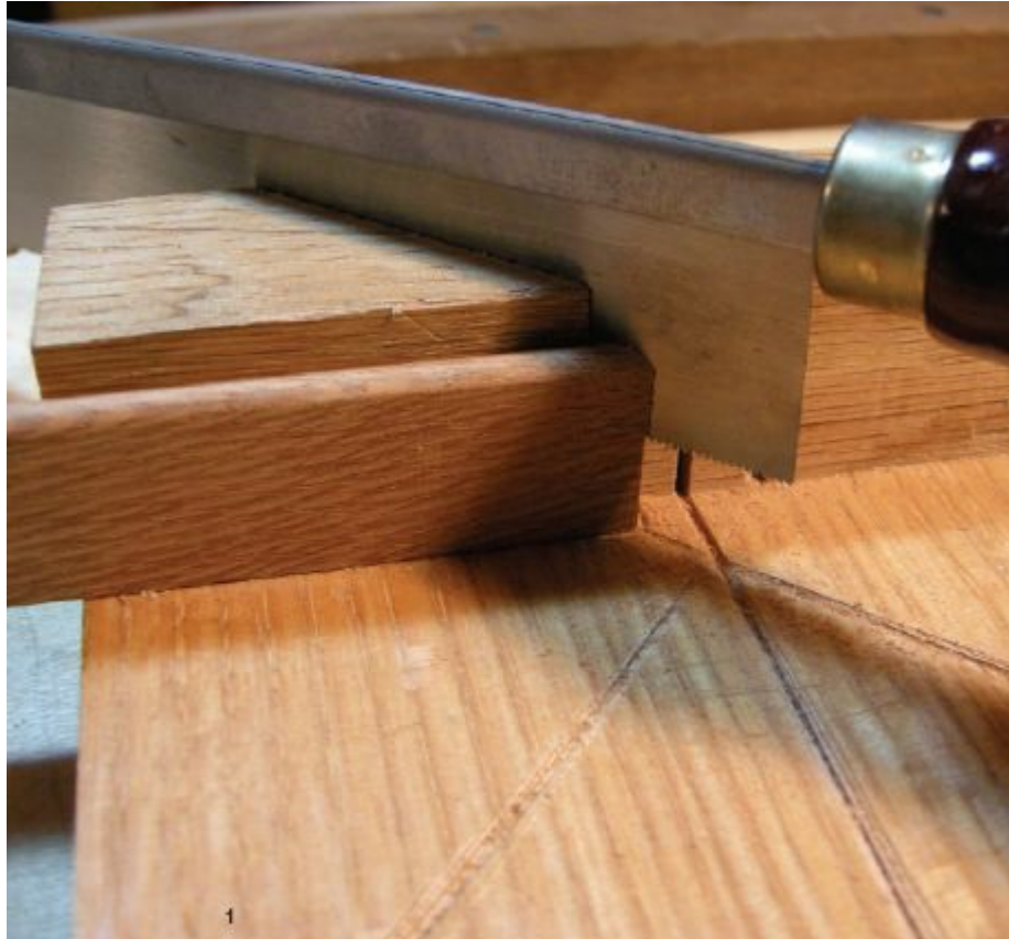
1. Saw stopped miters in the top and bottom moldings.
