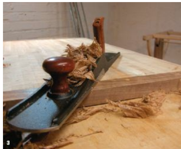
3. Plane the breadboards and dowels flush with the tabletop. Use a high-angle smoothing plane and a card scraper for the final smoothing.
