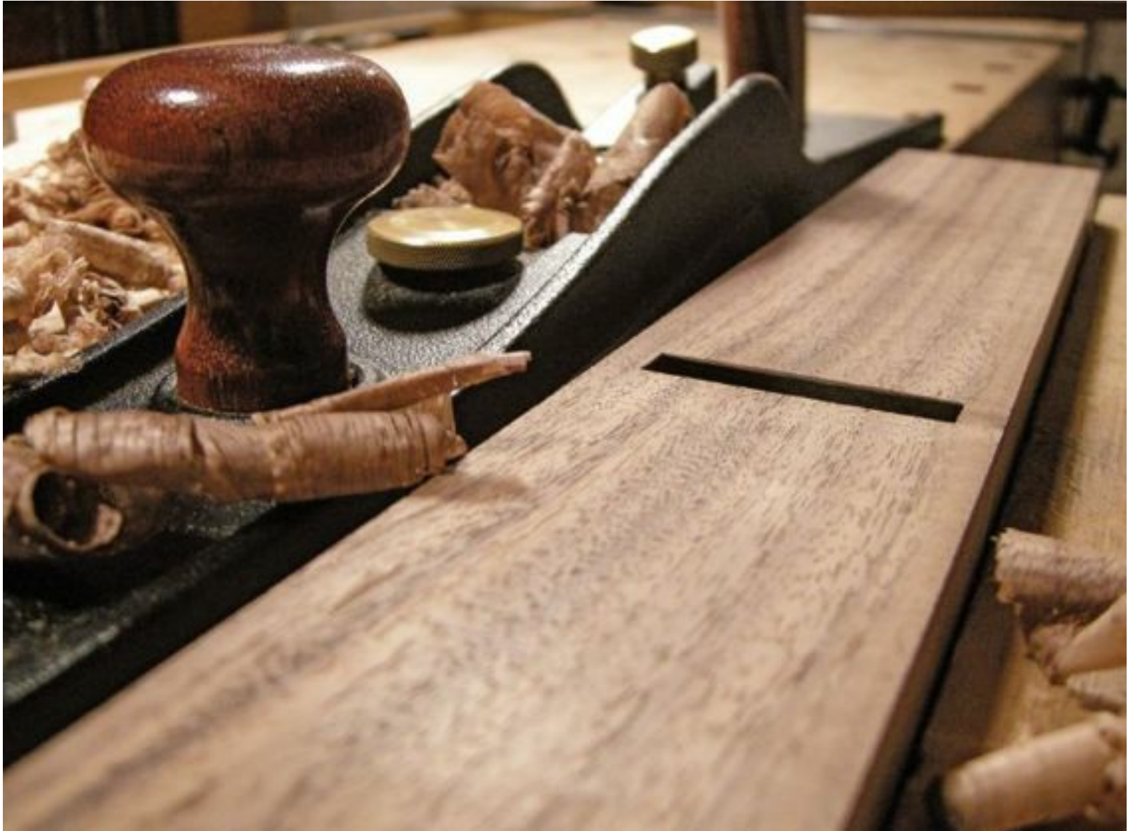
Flatten the sole with a finely tuned jointing plane.
