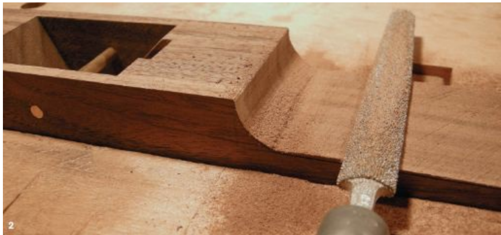
2. Refine the curve with a half-round rasp.
