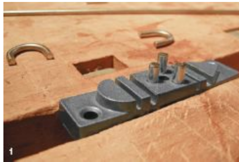
1. Bend the steel rod for the retaining pins using a metal bending jig. (This one is available from Lee Valley Tools.)
