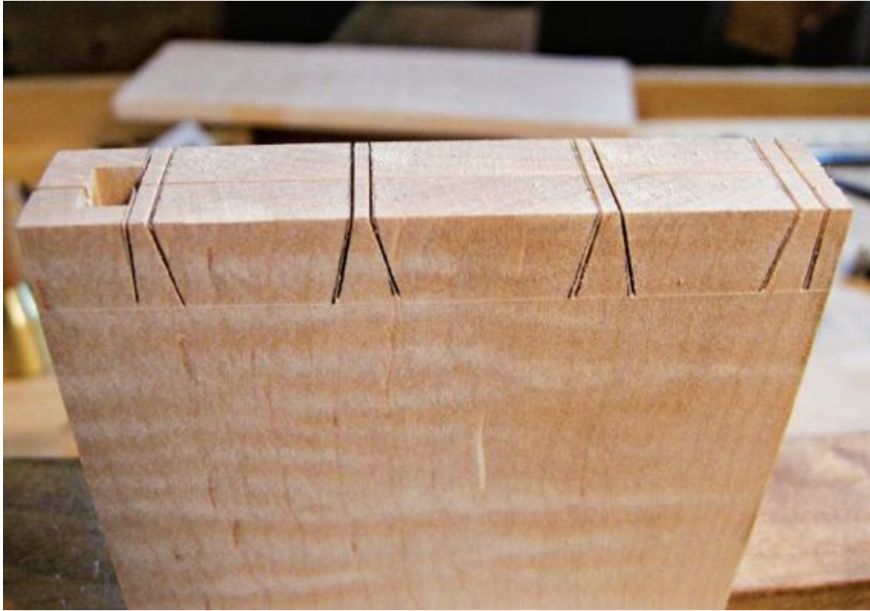
The through dovetails at the back of the drawer are laid out slightly differently from the front half-blinds. No outside shoulders here.
