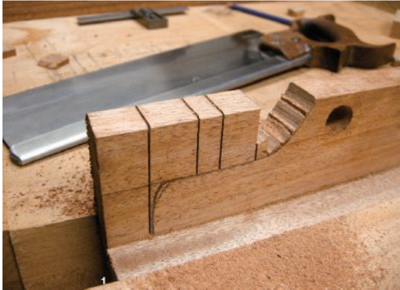
1. Crosscuts make removing the waste area of the fence easier.
