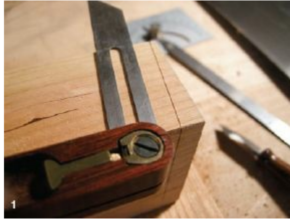
1. Set a sliding bevel gauge for the top and bottom of the splayed legs.
