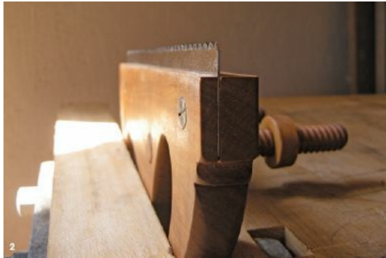
2. After the fence is complete, reinstall the saw plate and install the new fence.
