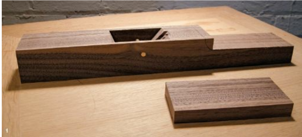
1. To create a razee-style plane, begin by removing the back section.
