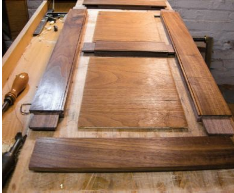
1. The back panel is straightforward, frame-and-panel construction. A quick coat of shellac at this point protects the part during the build.
