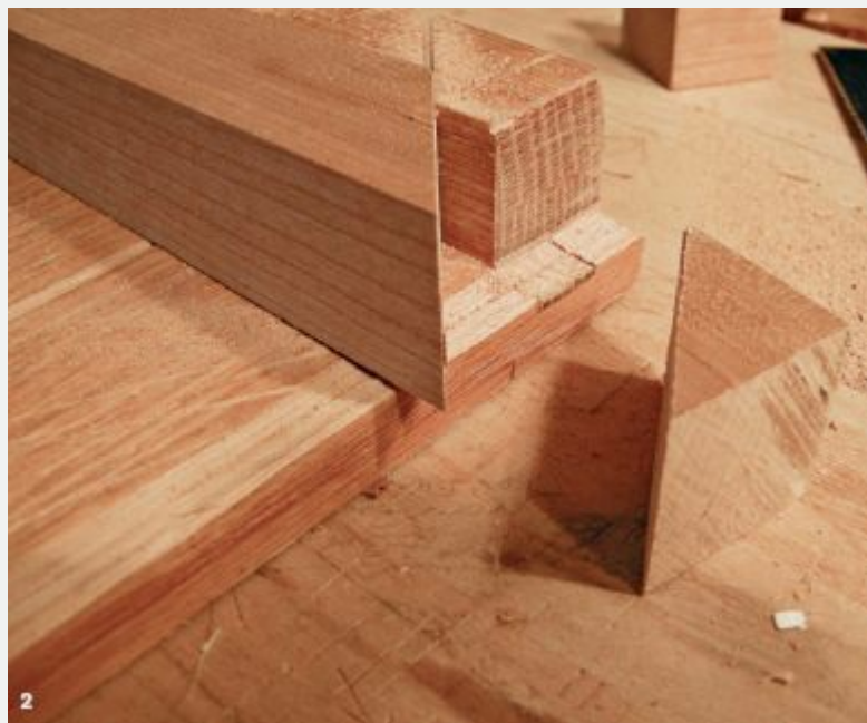
2. Cut the end stops at 45° and refine the slope with a low-angle block plane.
