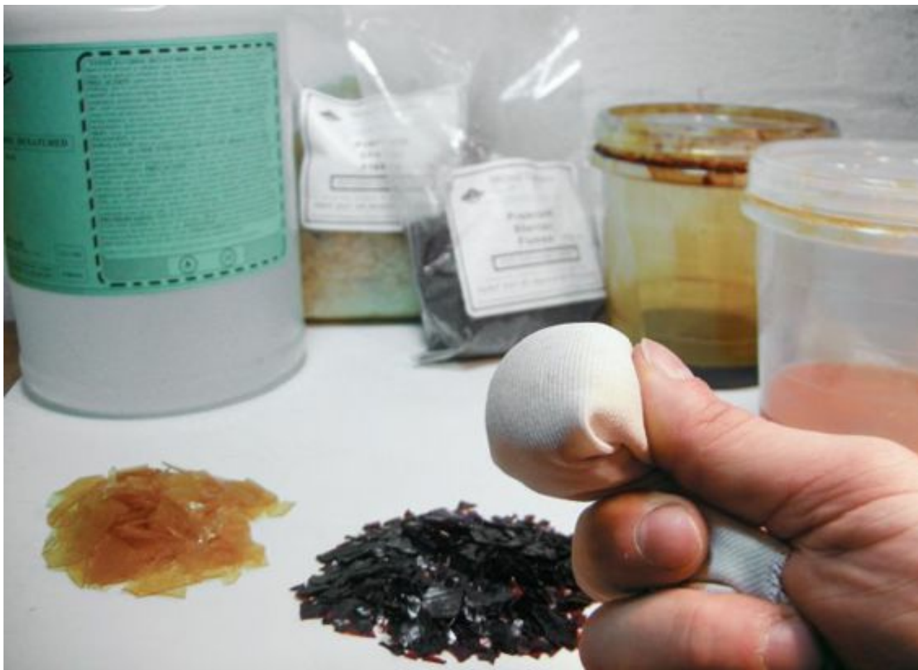
A small ball of cheesecloth wrapped in a tightly knit fabric makes a great shellac applicator.
