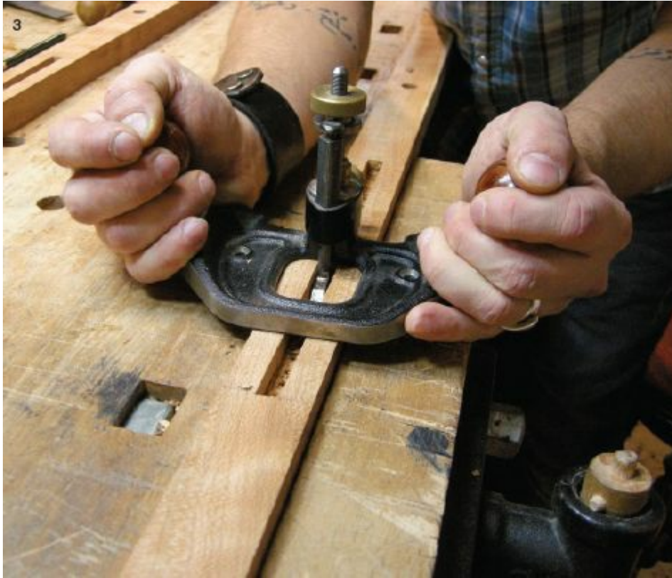
3. A large router plane is the ideal tool for refining the depth of the slot.
