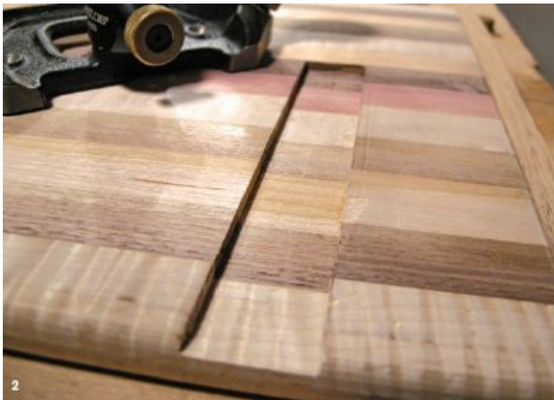
1. Chisel out two stopped dados to give the legs somewhere to go while the surface is not in use.
