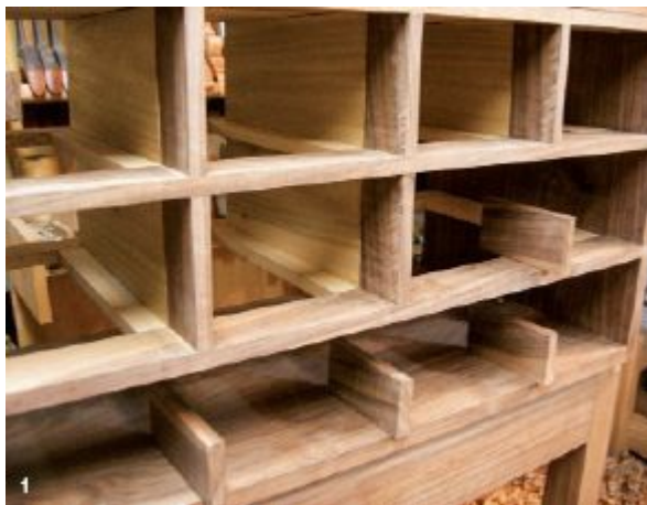
1. The false dividers are laid out in sequence to the “real” drawer dividers already in place. The grain flows through the parts thanks to the step you did earlier when roughing-out the stock from the same piece. Now after all that work, make sure to label everything and keep the parts in order.
