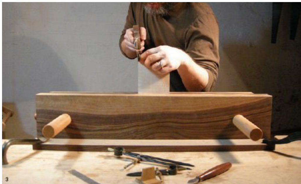
3. The lying press is the perfect jig for holding parts while making drawers.
