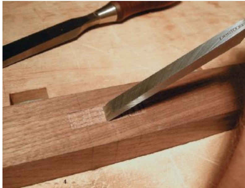
1. Small bites and light taps are all that's needed for the shallow mortise for the wear plate.
