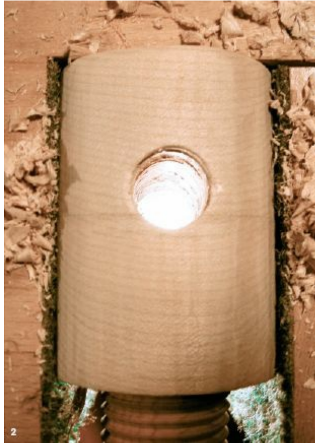
2. Boring the hub holes at a slight angle (about 2° off of 90°) keeps the handles away from the jaw while in use.
