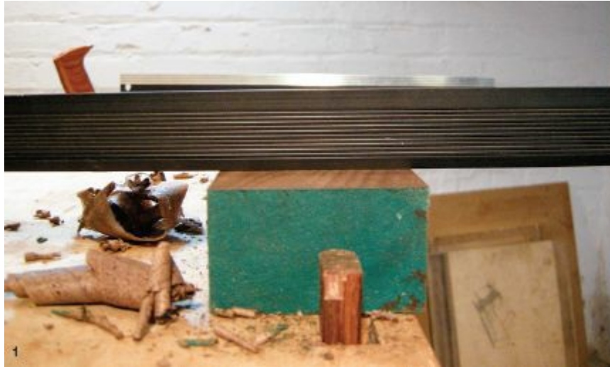
1. Winding sticks exaggerate any twist or wind in the stock. Here, the workpiece winds from the far left to the nearest right corner.
