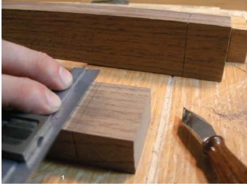
1. Scribe the depth of the shoulders for the double tenons on the ends of the arms.
