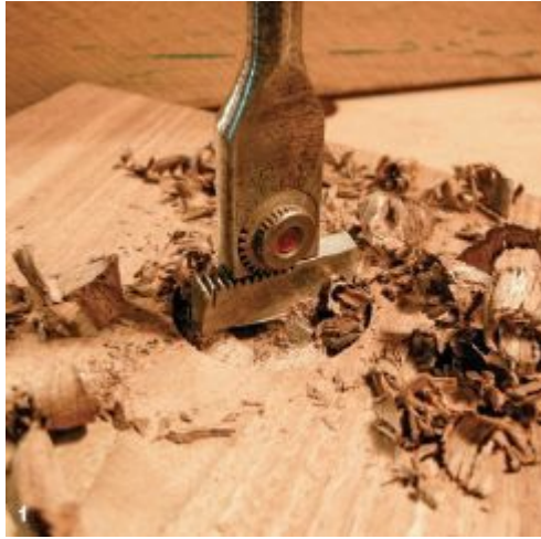
1. An expansion bit is the tool to use for boring the 1 1 / 2 -in. holes in the front jaw.
