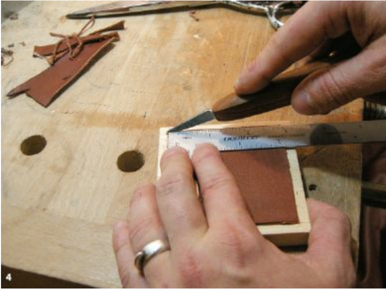
4. Trimming the fat off one of the bottom panels after the glue is dry.
