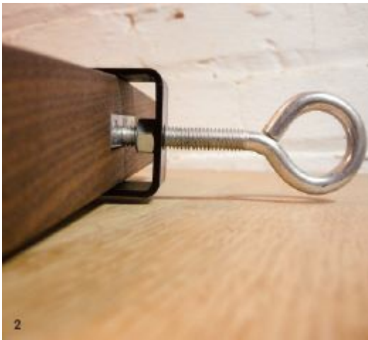
2. The front tensioning bolt is all lined up with wear plate. I left the bolt long for now, but if you like you can trim it down to about 1\frac{1}{2} in. of threads in length. The longer bolt just makes it a little easier to grip while tightening.
