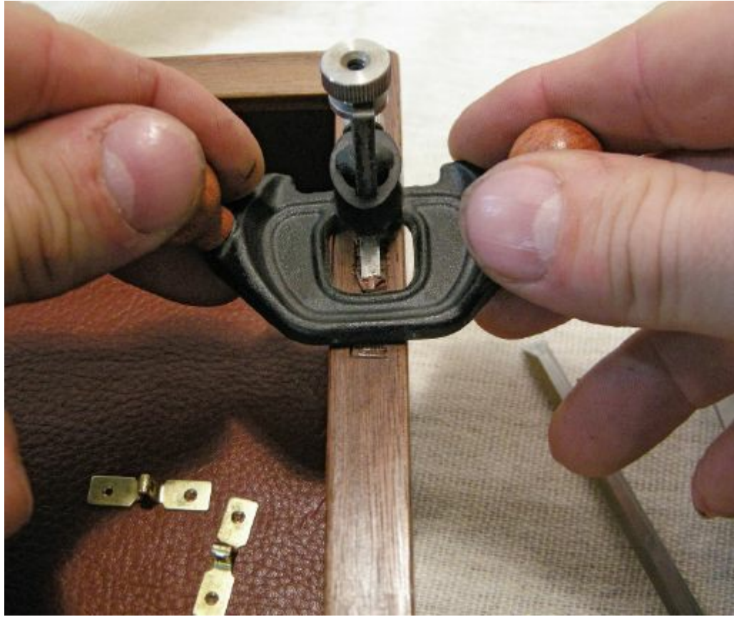
Land of the giants? This miniature router plane made by Veritas is a 3-in. replica of its full-size counterpart. The blade is only \frac{1}{8} in. wide, making it the perfect fit for removing the waste in this tiny mortise.
