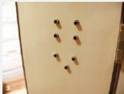
2. Drill the matching holes in the chest sides. The block inside the chest helps prevent any blowout on the inside of the chest sides while drilling.
