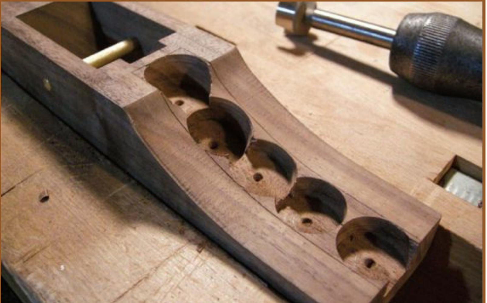
5. Remove the waste in the rear mortise.
