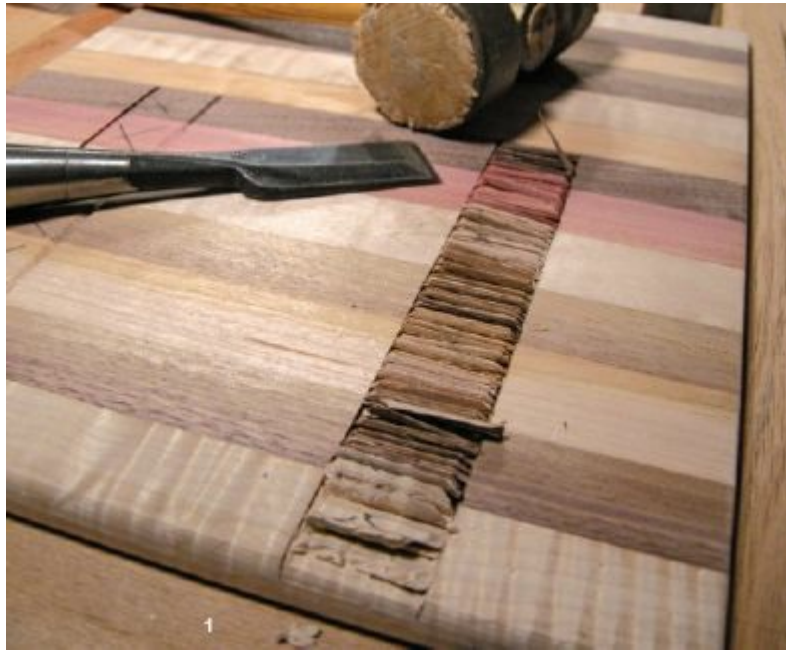
1. Chisel out two stopped dados to give the legs somewhere to go while the surface is not in use.
