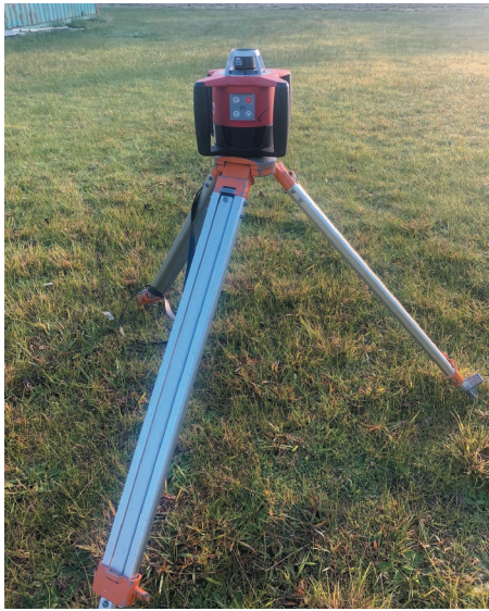
Fig. 14.4 A tripod set at a low height for a laser level to be used
