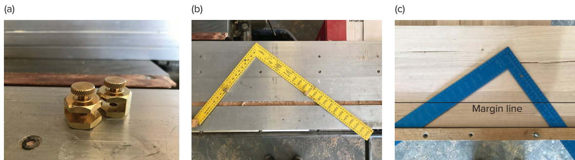
Fig. 33.24 (a) Angle gauges for builder's square; (b) builder's square with angle gauges; (c) marking gauge with timber cleat
