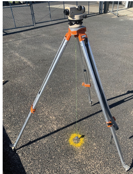
Fig. 14.6 The instrument set up with a plumb bob over a reference point
