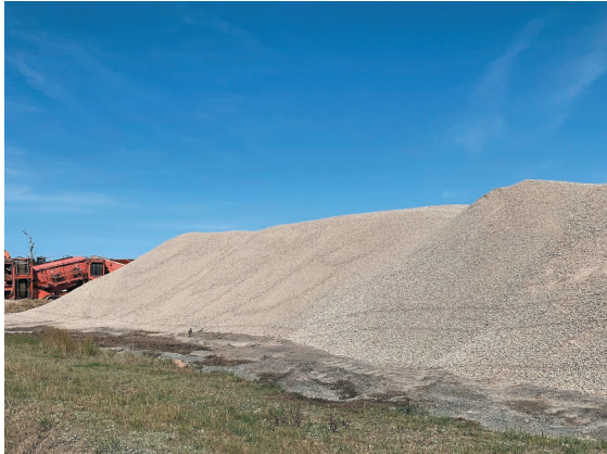
Fig. 31.42 Recycled concrete as road base
