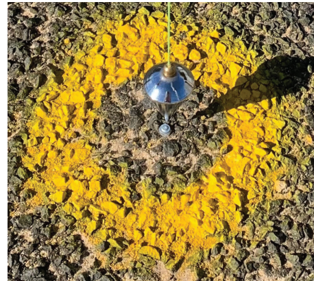
Fig. 14.10 Plumb bob set up over reference point
