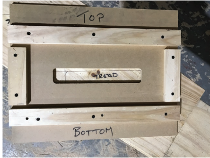
Fig. 33.36 Completed step jig ready for use
