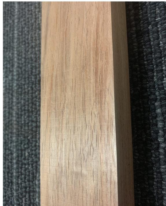
Fig. 11.60 In-feed roller marks
