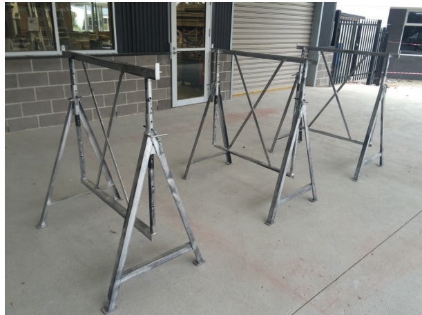
Fig. 26.10 Space trestles according to plank length
