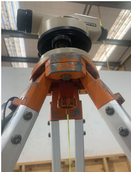
Fig. 14.5 The plumb bob attachment point on the underside of the stage
