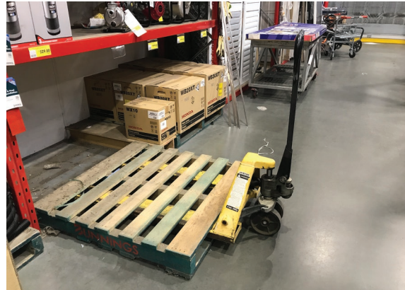
Fig. 12.6 Timber pallet and pallet jack
