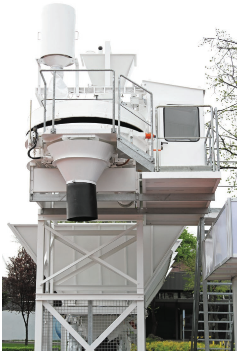
Fig. 31.22 Mobile site batching plant
