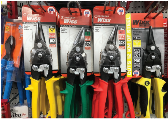
Fig. 12.8 A selection of tin snips for straight, left and right cutting
