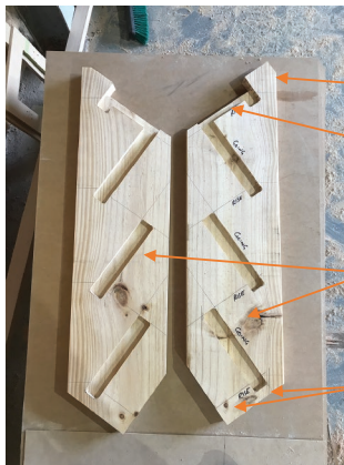
Fig. 33.38 Routed left- and right-hand stringers
