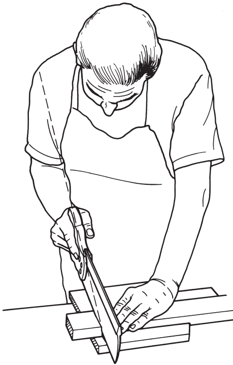
Fig. 7.25 Stance for using the tenon saw
