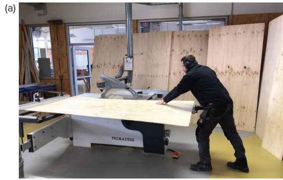
Fig. 11.38 (a) Straightening a board; (b) squaring a board
