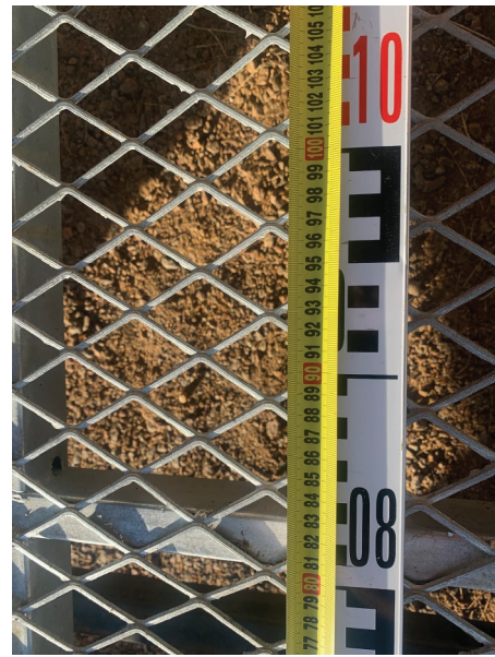
Fig. 14.3 A tape measure can be run over the staff to check readings
