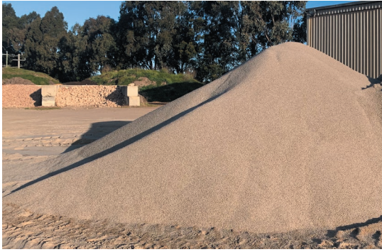
Fig. 15.3 Pile of sand resting at the angle of repose
