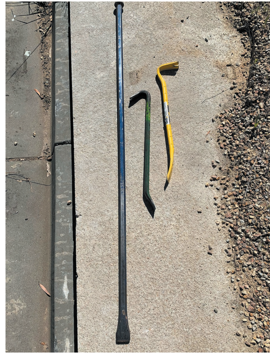
Fig. 34.9 Bars used for demolition work
