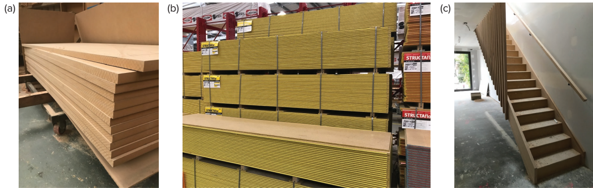
Fig. 12.24 (a) 32 mm MDF sheets; (b) 19 mm yellow tongue flooring; (c) MDF staircase treads and risers
