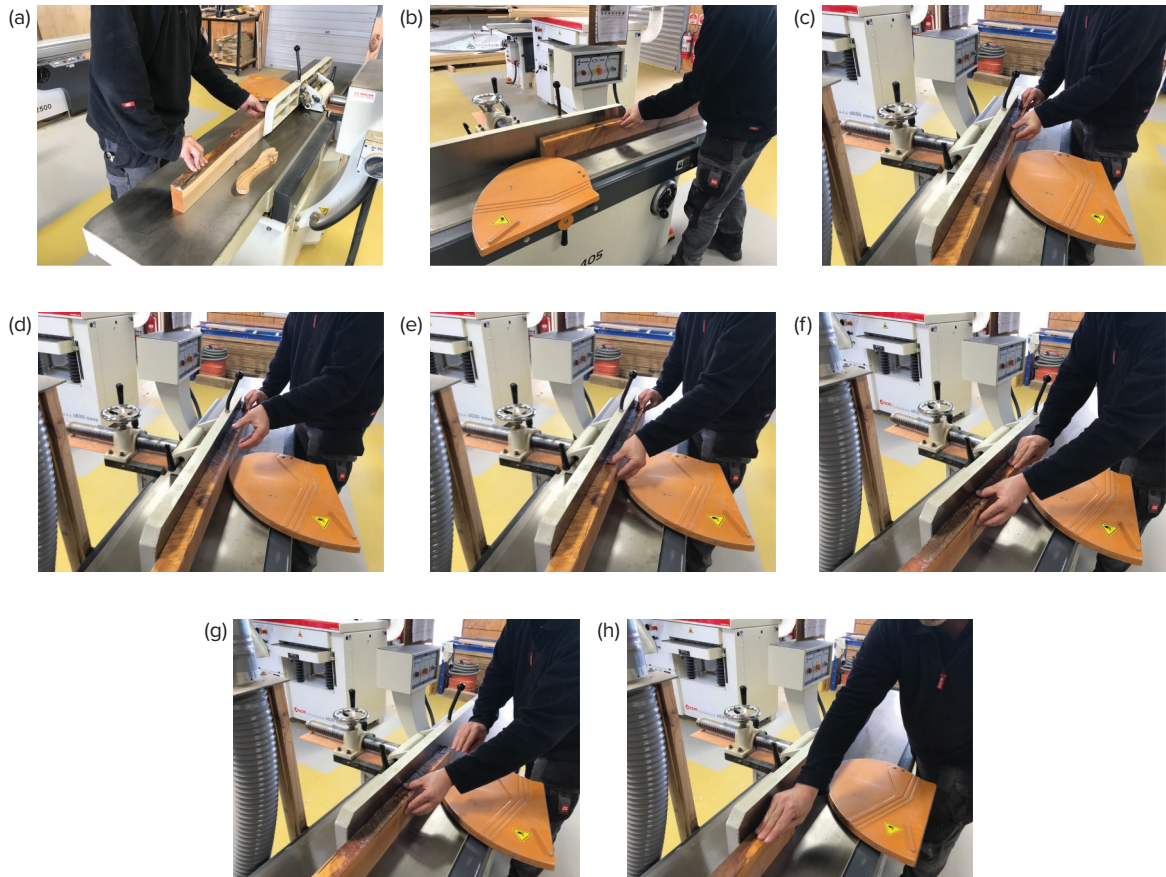
Fig. 11.26 Surface planing the edge of a piece of timber/squaring timber: (a) face of timber held firmly against squaring fence; (b) bow of timber facing up; (c) hands firmly supporting timber; (d) stepping hand over blades; (e) hand stepped over blade and supporting timber; (f) front hand in a position to support timber as back hand is ready to be stepped over blade; (g) back hand is stepped over blade; (h) back hand stepped over blade and pushing timber out over blades
