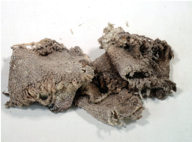
Fig. 1.19 Damaged bonded asbestos with asbestos fibres exposed
