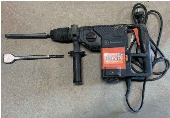
Fig. 34.12 Rotary hammer drill/jackhammer for ceramic tile removal or smaller concrete demolition work
