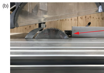
Fig. 11.41 (a) Panel saw rip fence set-up for solid timber; (b) rip fence set-up as a stop plate
