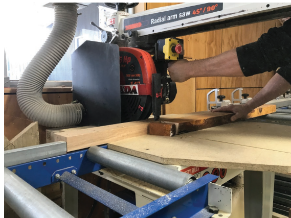
Fig. 11.17 Saw pushed back behind the fence
