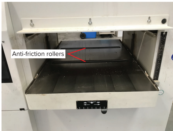
Fig. 11.58 Panel planer anti-friction rollers
