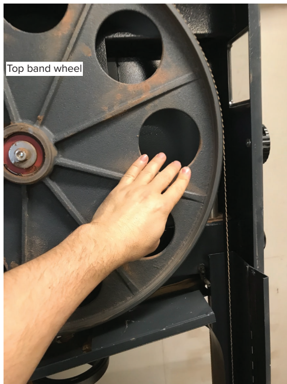
Fig. 11.45 Band saw blade set-up test
