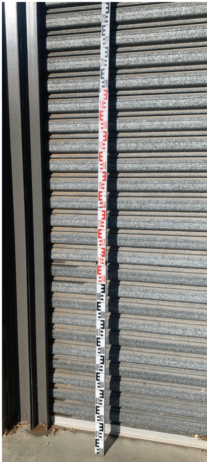
Fig. 14.1 A metric staff showing the change of colour from black to red every metre
