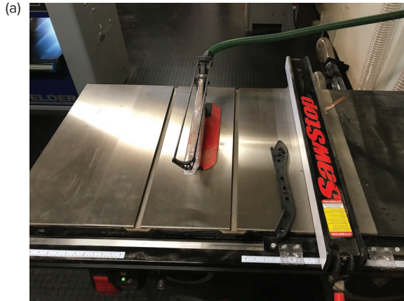
Fig. 11.11 (a) Plastic push stick; (b) timber push block
