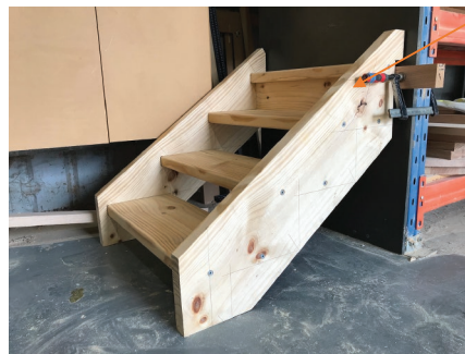
Fig. 33.41 Assembled and squared staircase unit
