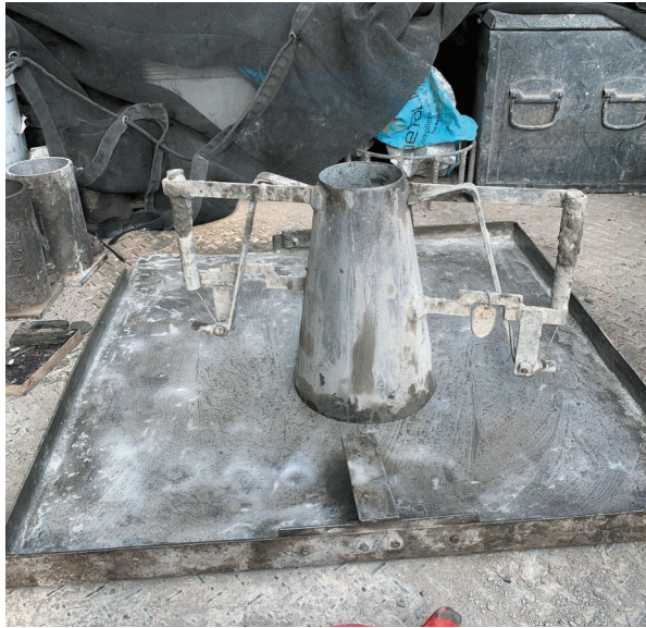
Fig. 31.46 A concrete slump test cone and tray ready to be used
