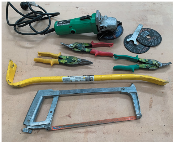
Fig. 34.10 Tools used for the demolition of steel-framed walls
