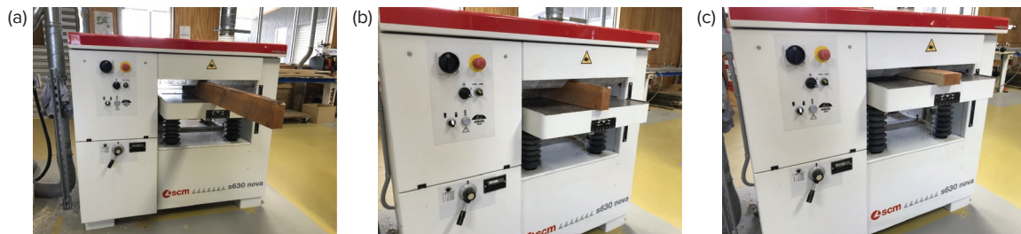
Fig. 11.59 Process of thicknessing material: (a) edge of timber first; (b) machining the edge; (c) machining the face of the timber
