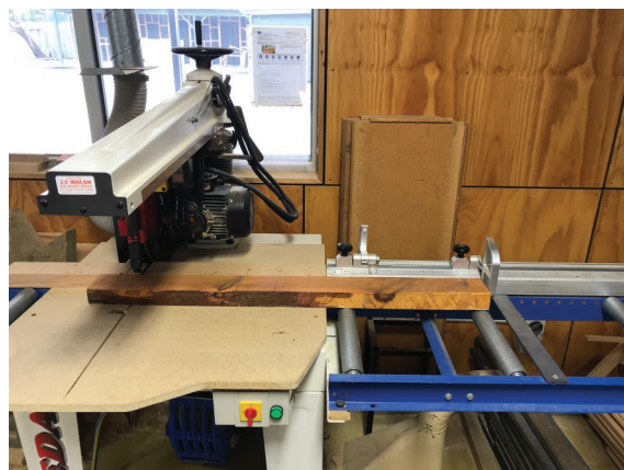
Fig. 11.18 Set-up of stop plate
