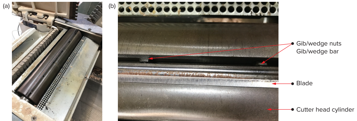
Fig. 11.63 Combination surface planer: (a) panel planer cutter block; (b) cutter block components
