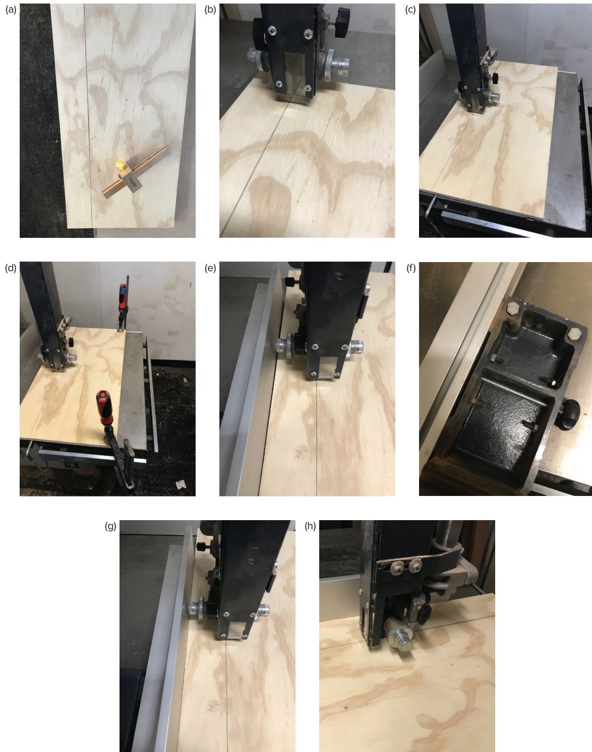
Fig. 11.51(a–h) Alternative method of squaring fence to blade
