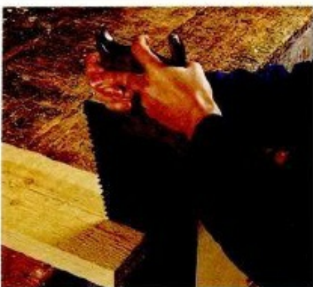
ABOVE: Overhand ripping on a bench
