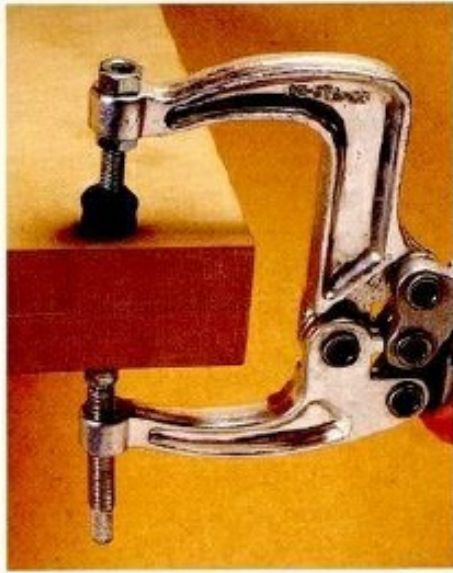
ABOVE: A set of aluminum scissor clamps with adjustable heads and rubber pads.
