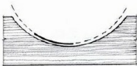
ABOVE: Adjust the sole to a smaller curve than the workpiece when working concave shapes.
