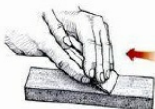
ABOVE: Honing the cutting edge.
