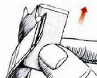
ABOVE: Using a slip stone on a lipped brad-point
