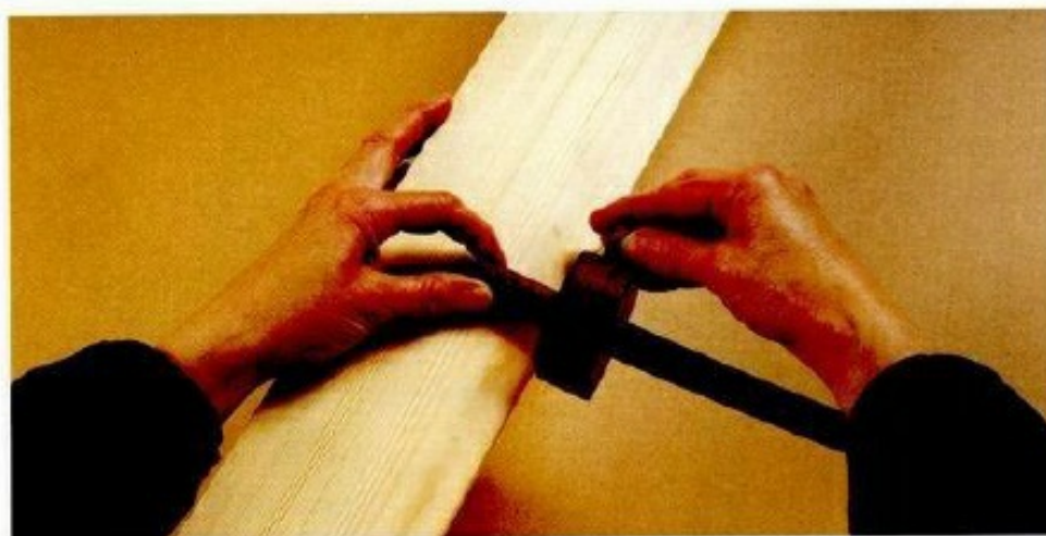
ABOVE: Spike the pin on the mark, slide the fence against the edge and tighten the screw.
