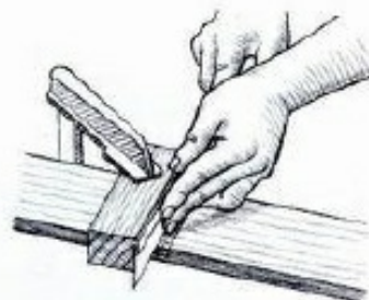
ABOVE: Some gent's saws are so delicate that they need to be used with two hands.
