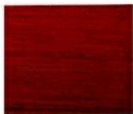
LEFT: Coarse-grained Honduras mahogany – not good for bending.
