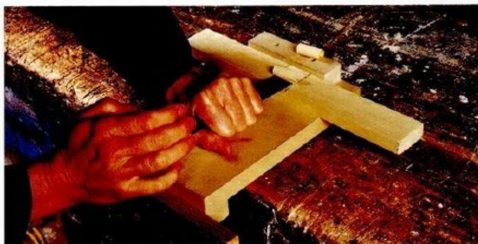
ABOVE: The bench hook stop prevents tool-exit damage.
