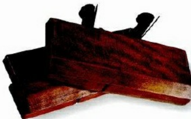
ABOVE: A matching pair of hollow and round molding planes.
