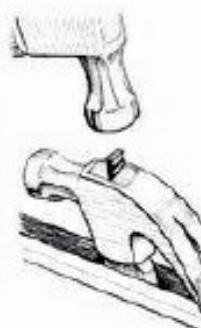
ABOVE: Securing a nail handle with a wedge
