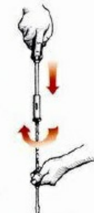
ABOVE: The Yankee-type screwdriver — with its chuck and selection of bits — is a great all-round tool.
