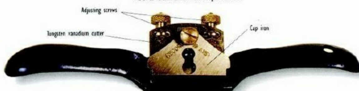
ABOVE: Flat-bottomed spokeshave for working concave surfaces
