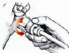
RIGHT: The cam ring action.
