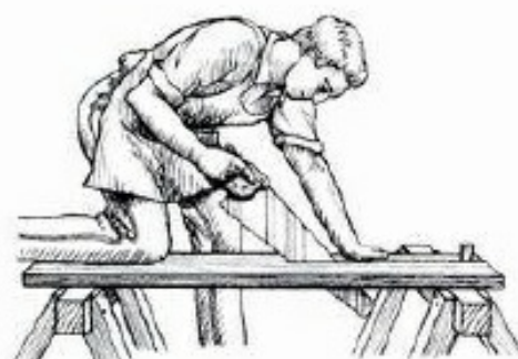
ABOVE: Using the rip saw – side view of correct stance.
