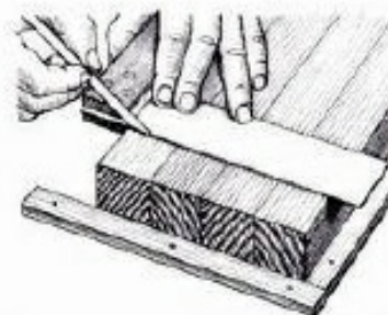
ABOVE: Hold the square so that the wooden handle – sometimes known as a "stock" – is hard up against the workpiece.
