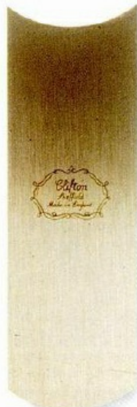
ABOVE: Scrapers are very useful for removing patches of rough grain in an otherwise smooth surface.
