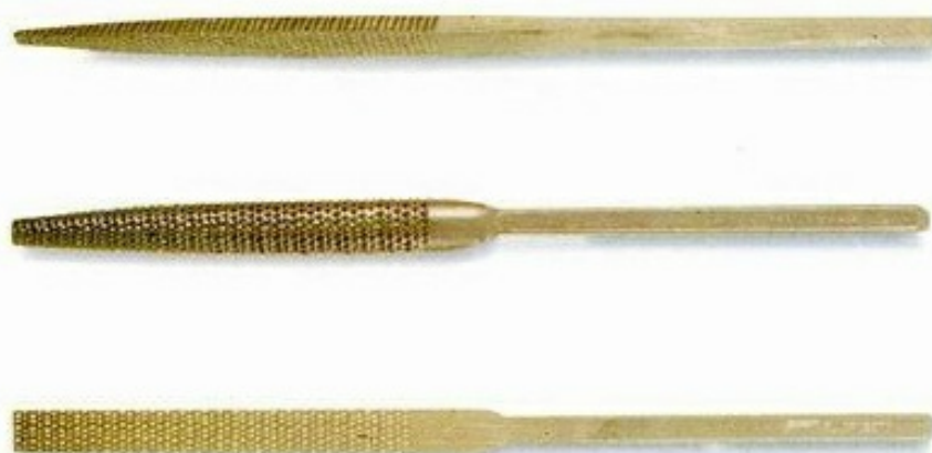
ABOVE: Three carver's rasps – each forged from one piece to create an integral handle.
