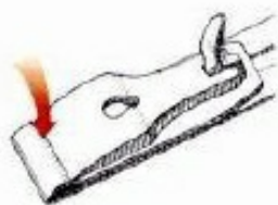
ABOVE: The lever cap must be a flush fit on the cap iron.
