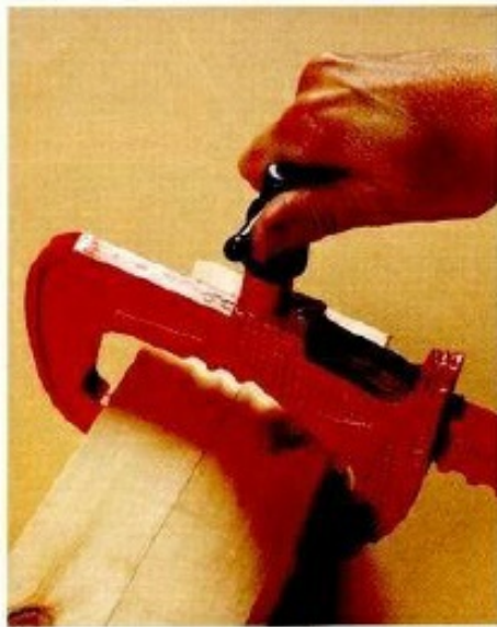
ABOVE: This particular clamp can be tightened up without any twist-damage action.
