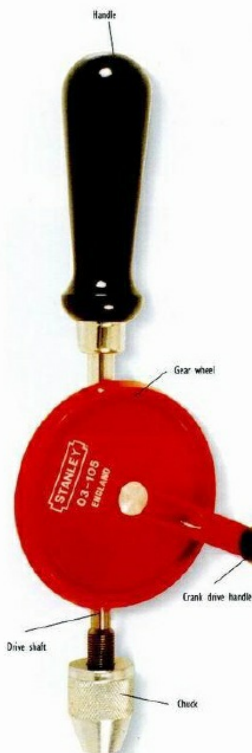
ABOVE: Single pinion hand drill with die-cast gear wheel.
