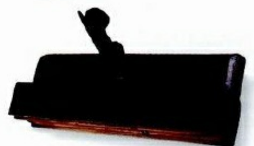
LEFT: Beading plane – designed to cut a bead profile on the edge of a board.
