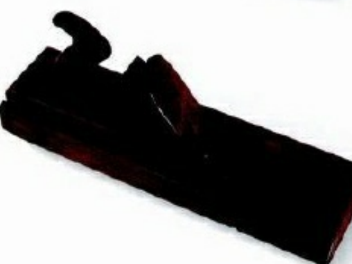
LEFT: Panel-raising plane – with a skewed blade and an adjustable fence.
