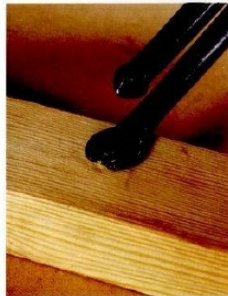
ABOVE: The split end of the handle is designed to be used as a tack extractor.
