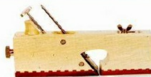
ABOVE: The bench rabbet plane – with the characteristic open cheeks.
