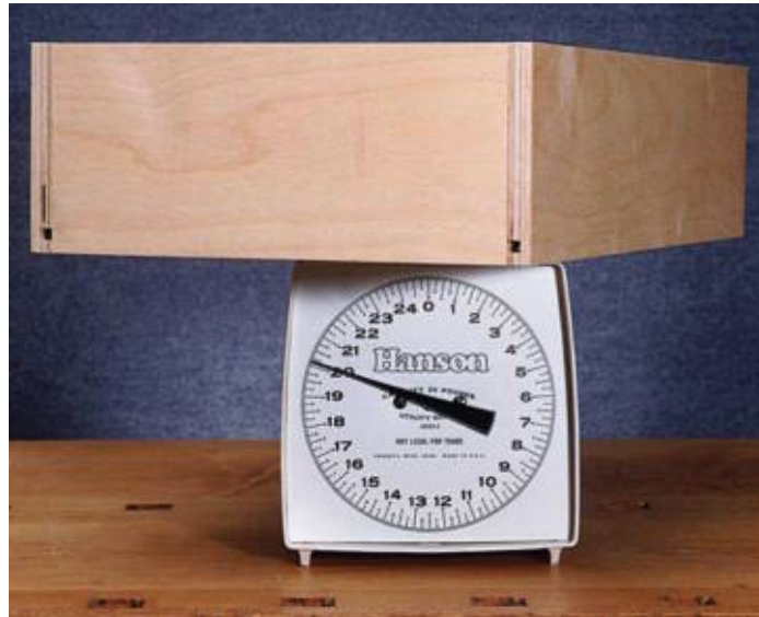
A kitchen scale will weigh small drawers and their contents, but you'll need the bathroom scale to figure load ratings for file drawers.
