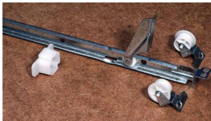
The single-track drawer slide utilizes a three-point suspension—two nylon rollers attach to the face frame, and the center roller rides the rail.
