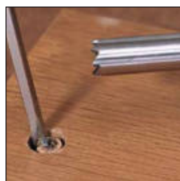
Removing a Damaged Screw
