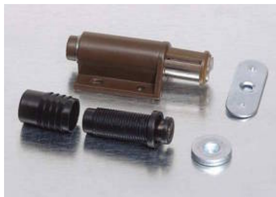
You'll find touch latches in many styles, shapes, and sizes. The one at top mounts on the surface, whereas the other requires you to drill a mounting hole for the press-in insert. You then screw the threaded latch body into the insert.
