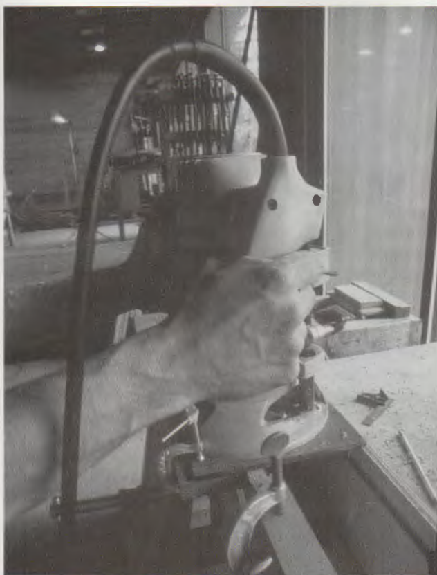
To cut mortises, Savage uses a plunge router and the shopmade jig shown above and in the drawing on p. 156. Stiles are clamped in the jig horizontally. Rails and muntins are held vertically. (Photo by Charles Miller.)
