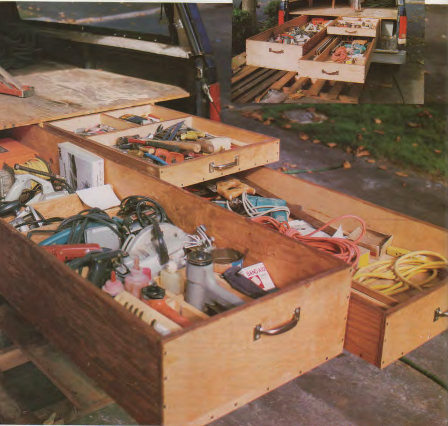
The trim carpenter's toolkit has to balance speed, accuracy and portability. Carrying tools in sliding bins like these protects them from damage and theft.
