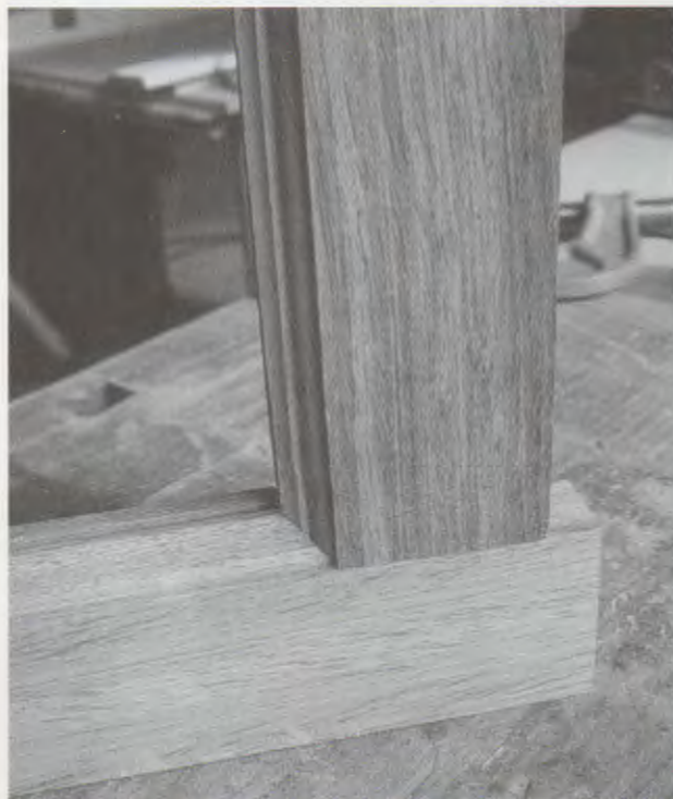
A completed rail-to-stile joint with its molded section mitered. Although more difficult to make, a coped molded section better hides the effects of wood movement. (Photo by Charles Miller.)
