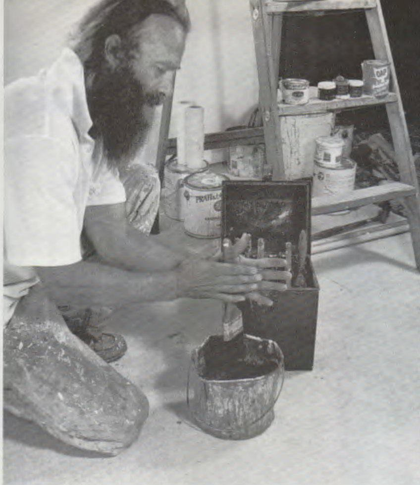
After cleaning a brush, twirl it as shown to remove excess thinner. Store clean brushes in a brush box or upright, wrapped in newspaper or foil to preserve their shape.
