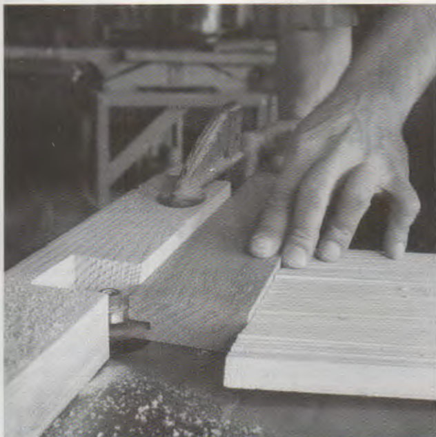
Before they're molded and joints are cut, rails and stiles should be grooved for panels. This can be done on a router table, as shown here, or on a table saw.
