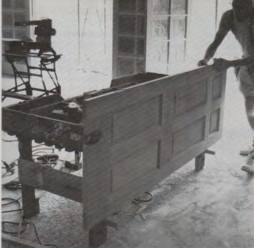
The door hanger's bench has clamps to hold the door for planing and holes in the legs for pegs to prop the work at a convenient height. Inside the bench's frame are trays for tools.
