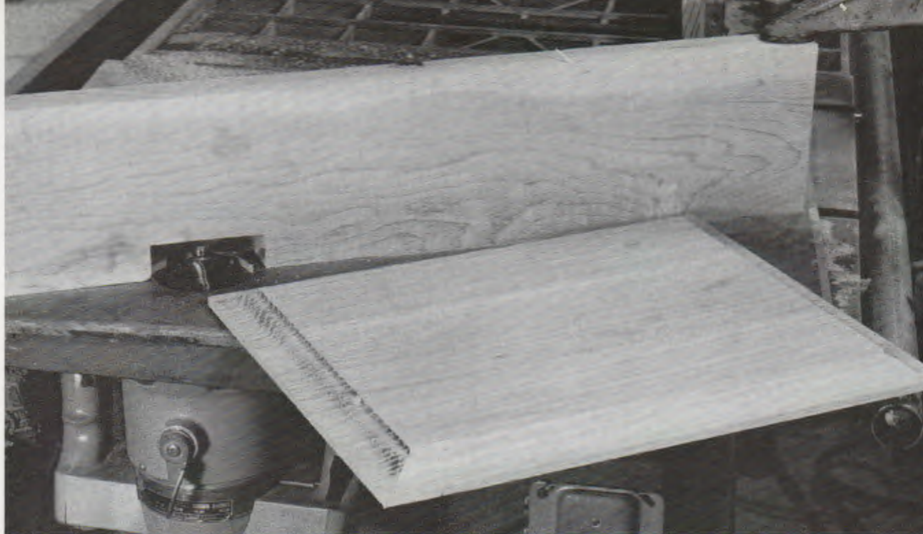
Panels for wainscot can be raised on the router table, as shown in these photos, or on a table saw. Although relatively expensive, panel-raising router bits make a clean cut that requires less sanding than tablesawn panels. Use a fence with either method and feed slowly and deliberately, with hands well away from the bit or blade.
