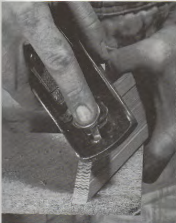
A block plane can also be used to trim miters. Support the molding on a bench or sawhorse and angle the plane across the cut.
