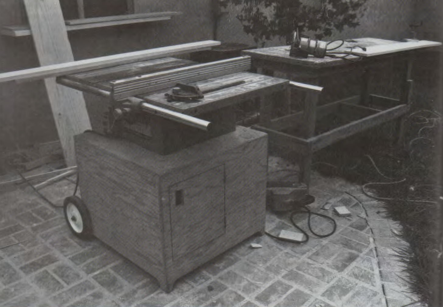
A table saw is more luxury than necessity for the trim carpenter, but it's useful for cutting miters and for making molding. This saw has been mounted on a stand with rollers so it's easy to move around the job site.
