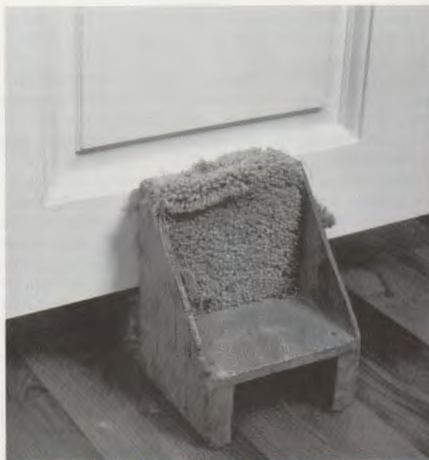
The door buck is one way of holding a door for planing. This door buck has been padded with carpet to keep it from marring the door.
