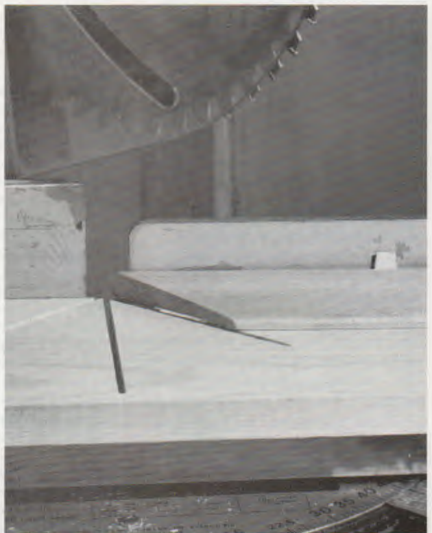
To adjust miter cuts, place wedges between the fence or sawtable and the molding to vary the cutting angle. This is faster than changing the saw's angle of cut.
