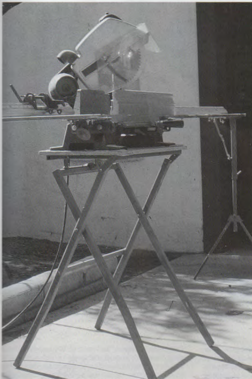
Power miter boxes, or chopsaws, are the trim carpenter's tool of choice for sawing miter and butt joints. Chopsaws should be equipped with extensions to support long stock during cutting.
