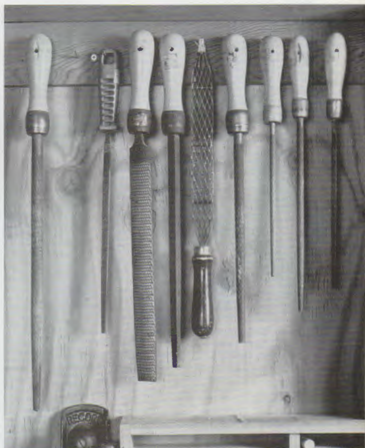
Files are indispensable for fine-fitting cope joints. Rasps, like the one shown fifth from the right, are useful for trimming overhanging drywall.
