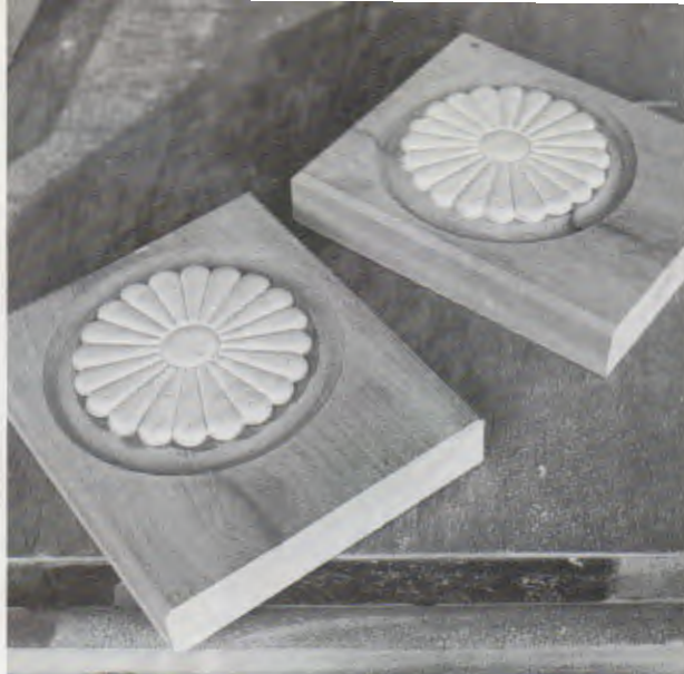
In butted trimwork, corner blocks are a nice detail. They can be bought commercially or made on site out of the same wood as the rest of the trim.
