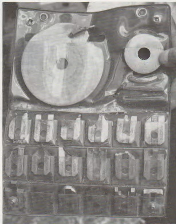
Several manufacturers make molding heads in single-knife, double-knife or three-knife models. This single-knife head has 18 knives whose profiles can be combined to make hundreds of moldings.
