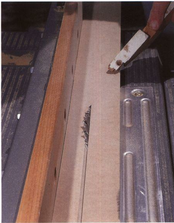
A museum rail is ripped from a single board with the table saw set at a 45-degree bevel.
