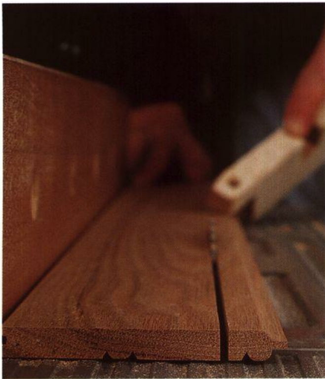
Rip the board to width, cutting off the tongue side.
