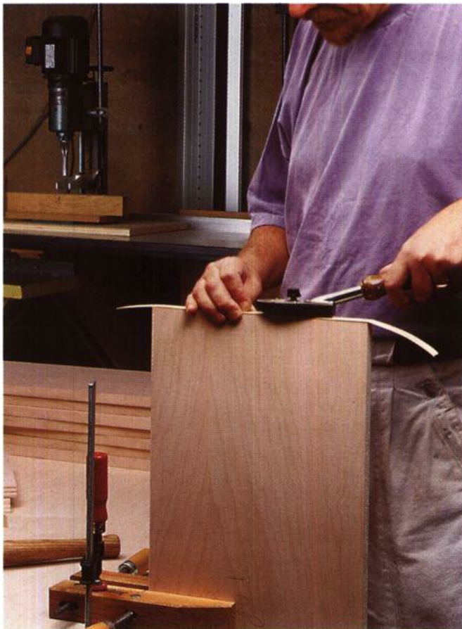
Apply veneer tape with a hot iron. After the adhesive cools, cut the ends of the tape flush to the corners with a utility knife and plane the edges flush to the faces.
