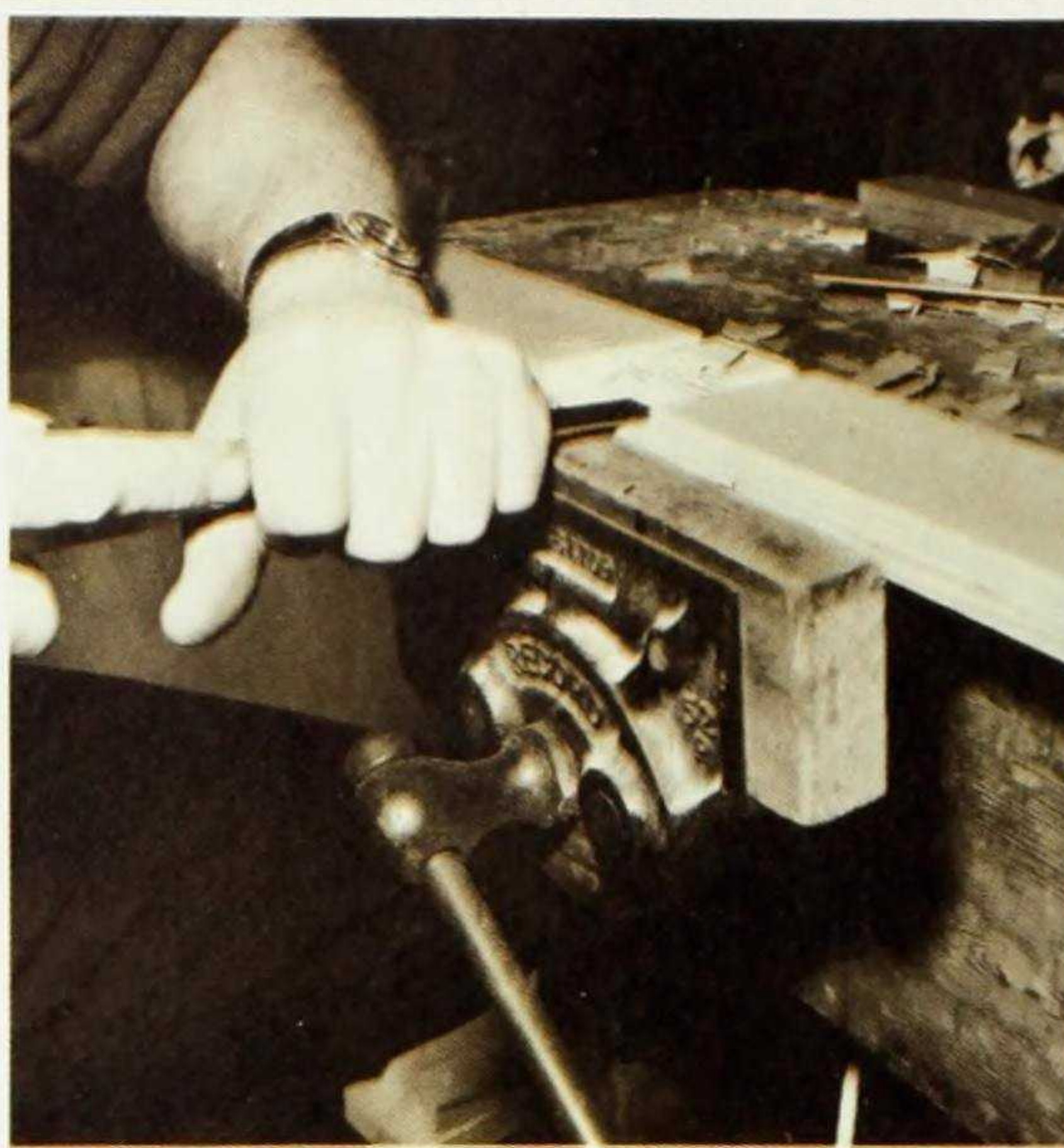
Fig. 4. Then the wood between the slanting cuts is removed with the chisel blade held bevel edge downward.
