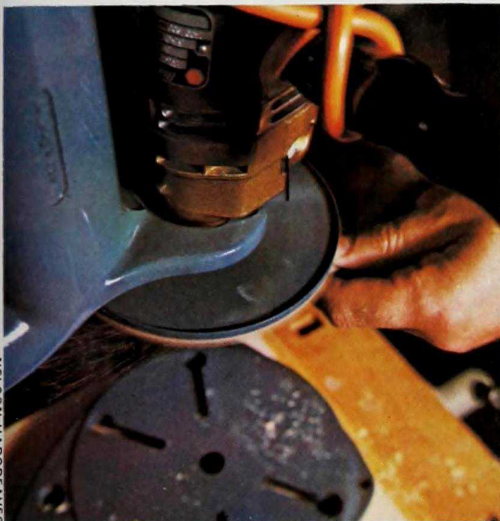
Fig. 11. The rapidly passing slots allow you to see, through the disc, whether you are holding the blade at the right angle.
