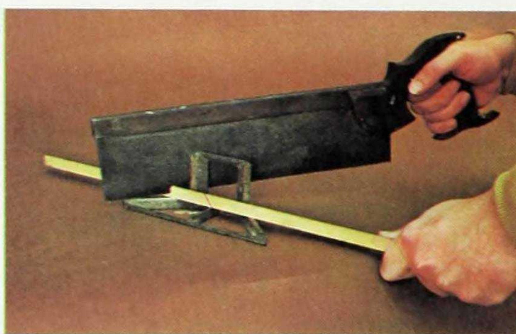
Fig. 2. Next, a back saw is used to trim the wood. Cut from the good side toward the back, so that any splintering is hidden.
