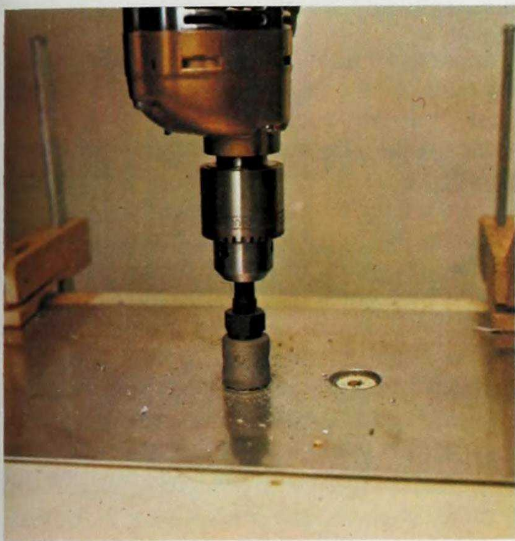
Fig. 7. A hole saw cutting large circles out of an aluminum sheet, which is firmly clamped to a wooden backing.
