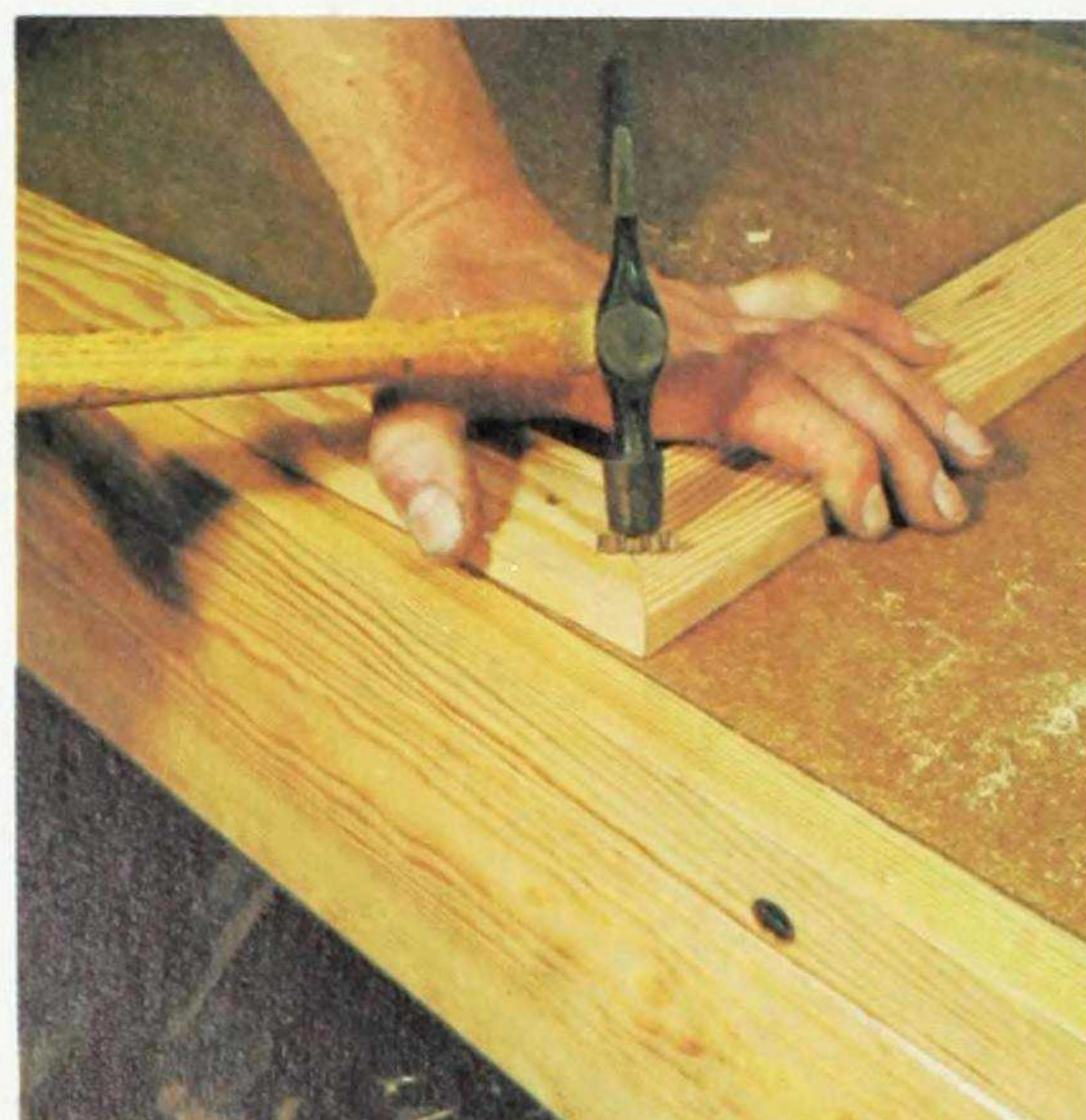
Fig. 4. An alternative method of holding mitered corners together—corrugated fasteners driven into the back.
