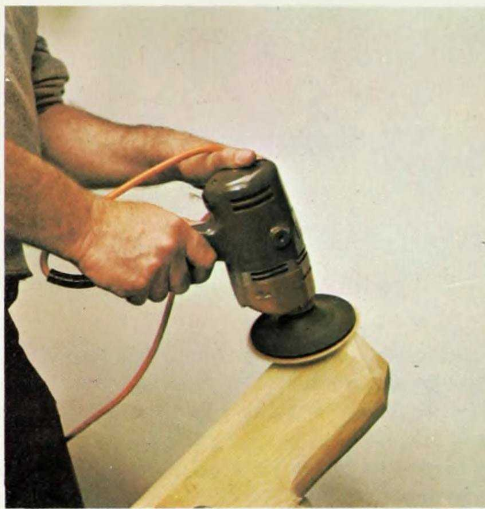
Fig. 5. The same disc can also be used, with practice, to sand rounded objects. Note how the cable is being held away from the disc.
