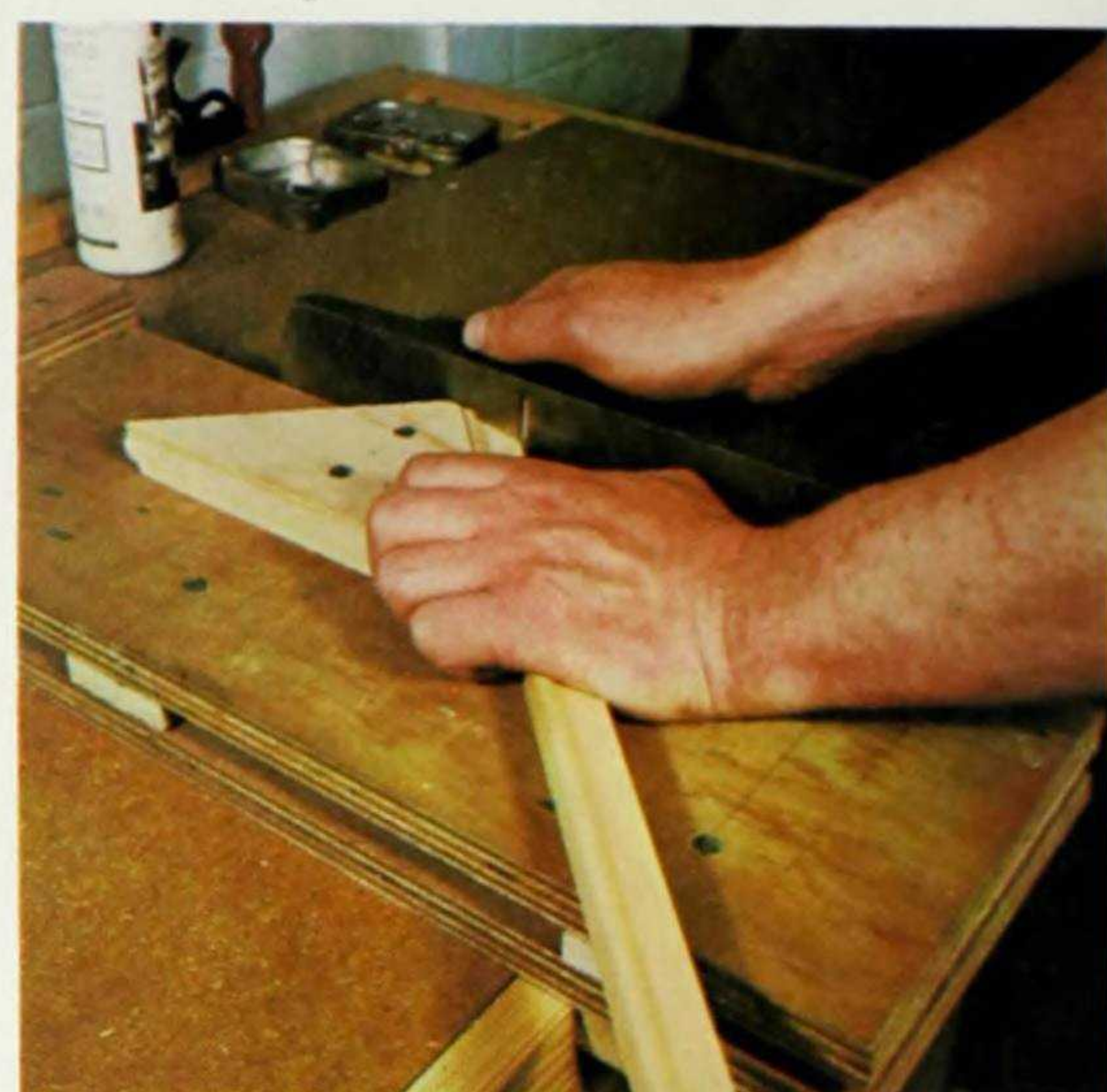
Fig. 3. The miter shooting board ensures 100 percent accuracy in cutting a miter at exactly the right angle.
