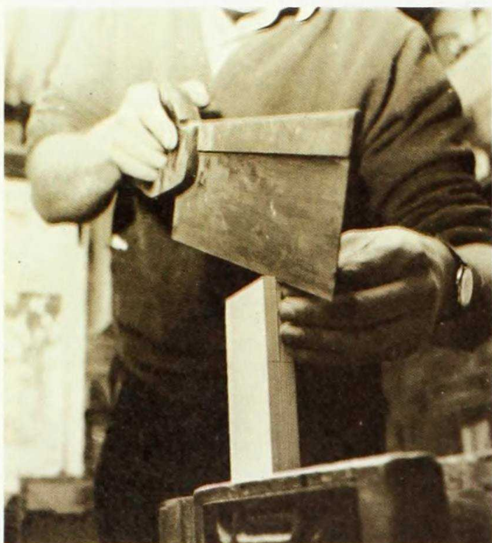
Fig. 5. Starting the "rip" (along the grain) cut for a lap joint. A small notch is made in the far edge of the wood.
