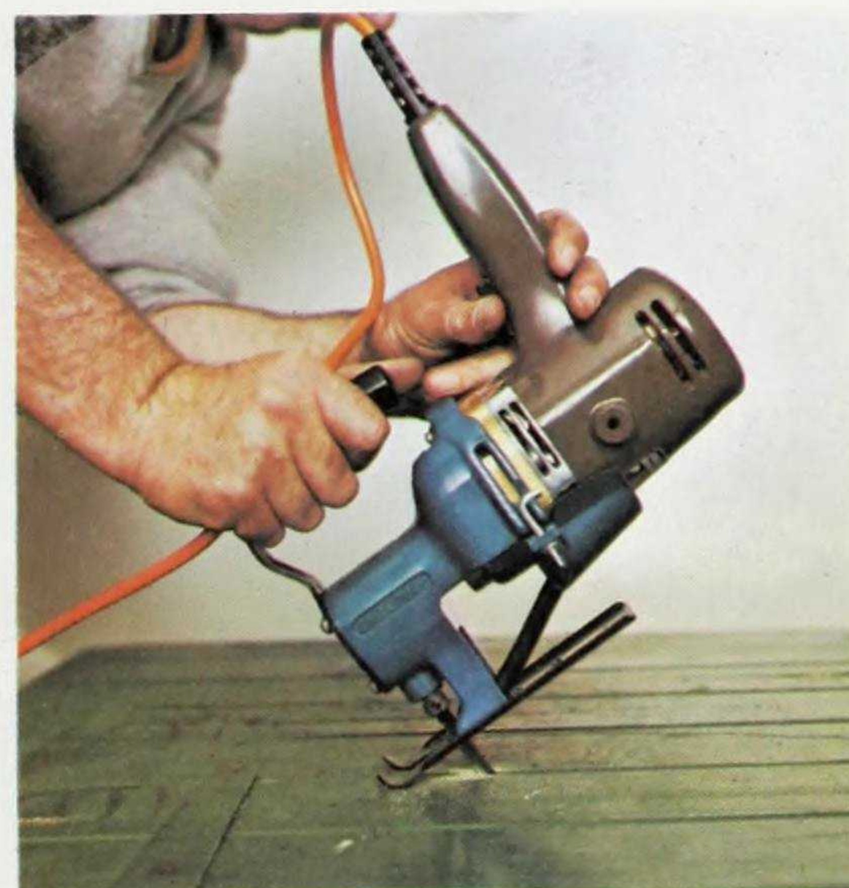
Fig. 2. A sabre saw attachment. Here, a cut is being started in the middle of this wooden door by tipping the saw on its nose and gradually lowering the blade into the wood.
