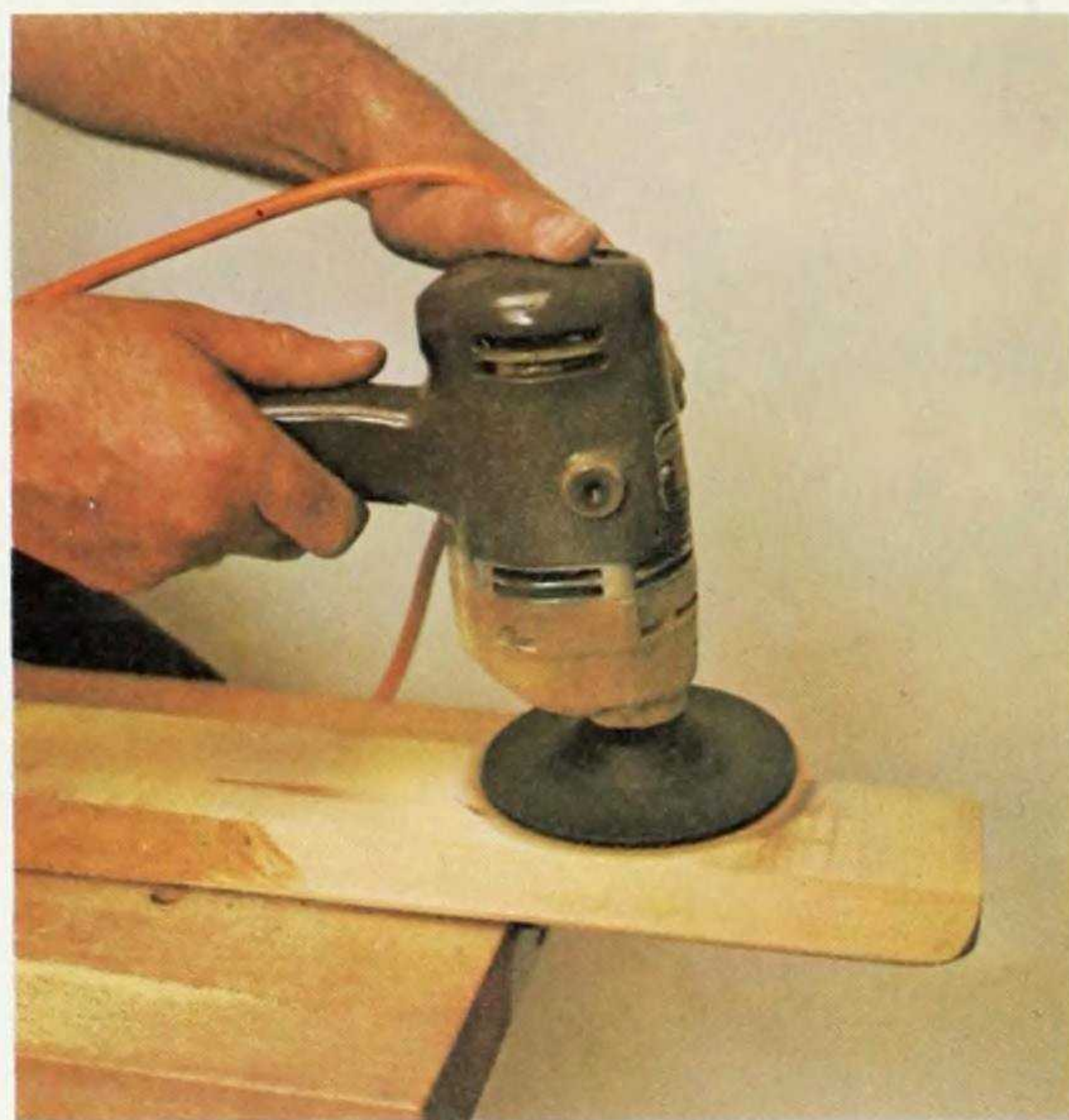
Fig. 4. When sanding a flat surface, you should hold the rubber disc at an angle to the wood to minimize swirl marks.
