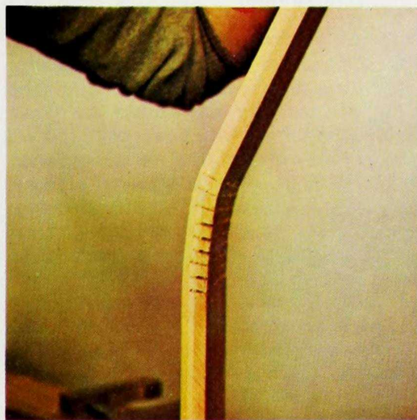
Fig. 5. A bench saw is particularly useful for kerfing —bending a piece of wood into a curve by making rows of deep cuts in it.
