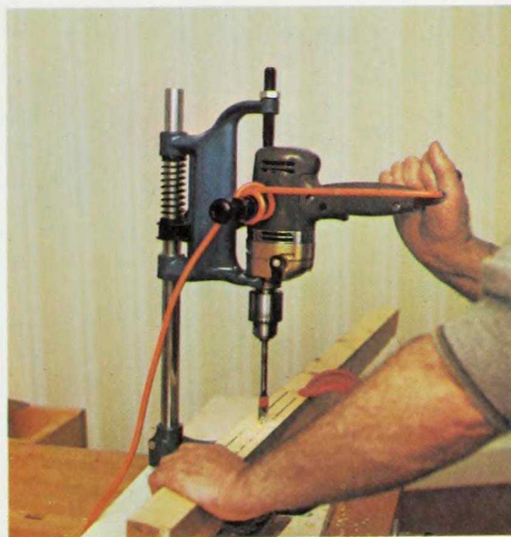
Fig. 1. A drill stand is one of the most useful accessories for your drill. It allows you to make perfectly accurate vertical holes in wood, metal or plastic.
