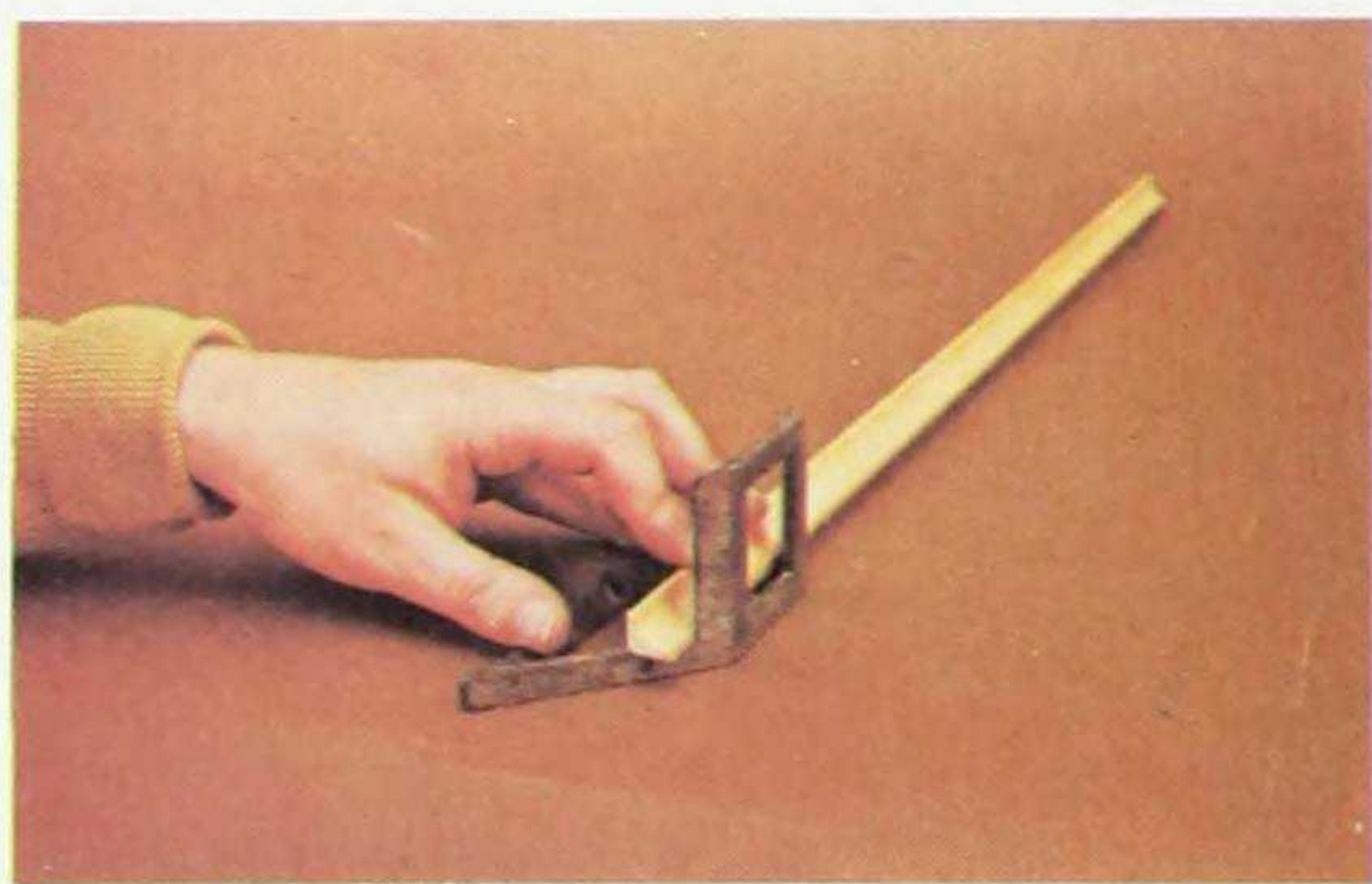
Fig. 1. Using a miter iron to cut cove molding. A try and miter square may be used for this.
