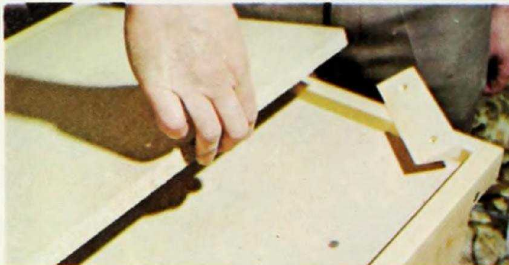
Fig. 11. Nailing on the tool rack at the rear of the bench. Tools and unfinished parts can also be stored in the well on the top.
