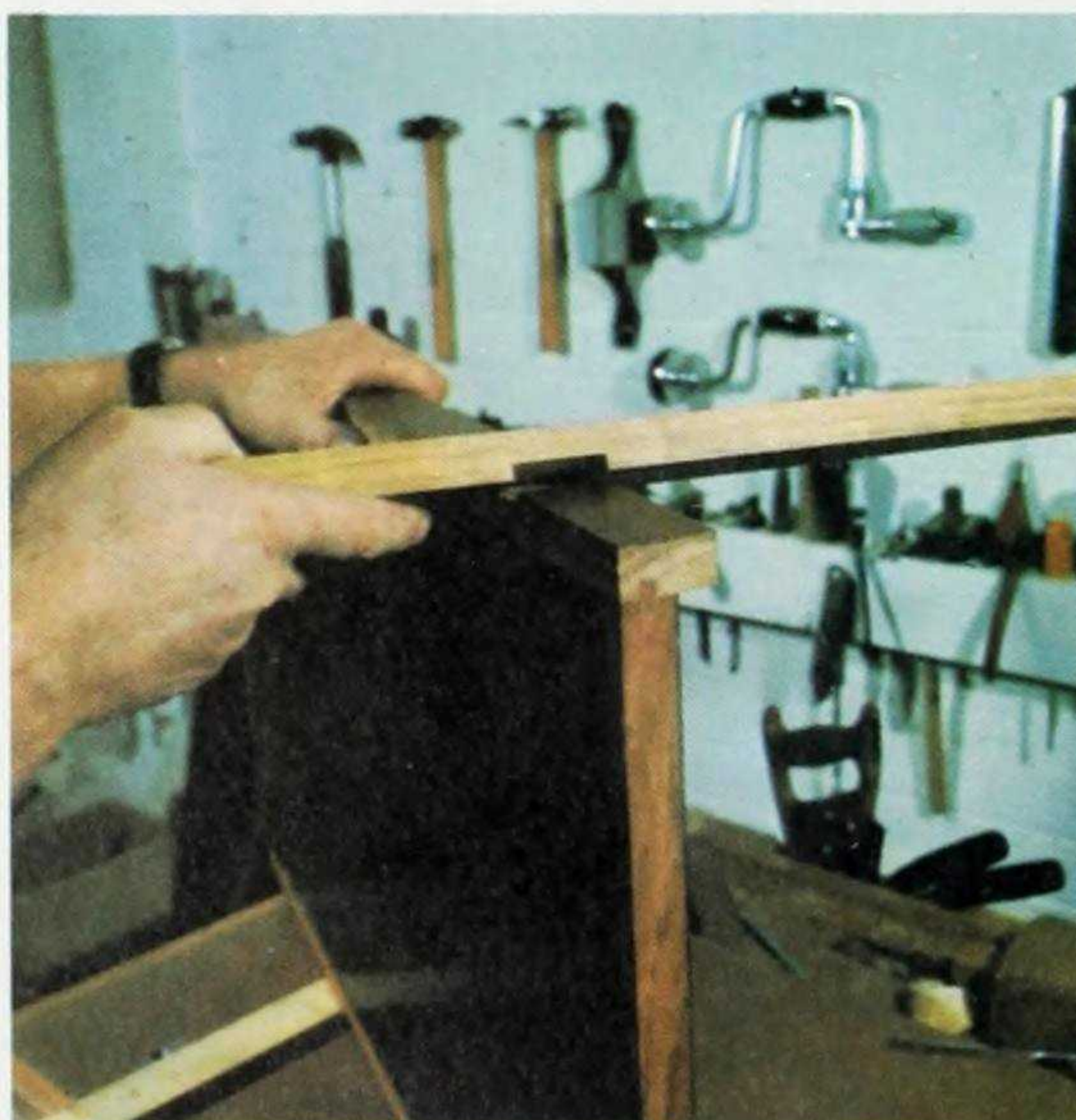
Fig. 1. Applying the laminate to the tray. Fig. 2. Trimming the edges of the laminate. Fig. 3. Cutting the groove in the tray side. Fig. 4. Fitting the side piece to the tray with a plywood fillet which is glued in place. Fig. 5. Fitting one of the back legs into the lap joint cut in the side piece. Fig. 6. The dimensions of the lap joint that is used to join the side pieces of the trays to the front legs. Fig. 7. The box joint between the trolley handle and the back legs. Fig. 8. The box joint is marked out with a marking gauge. The wood is divided into five more or less equal widths. Fig. 9. The dimensions of the groove cut in the trays and sides, and of the plywood fillet. Fig. 10. An exploded view of the tea trolley.
