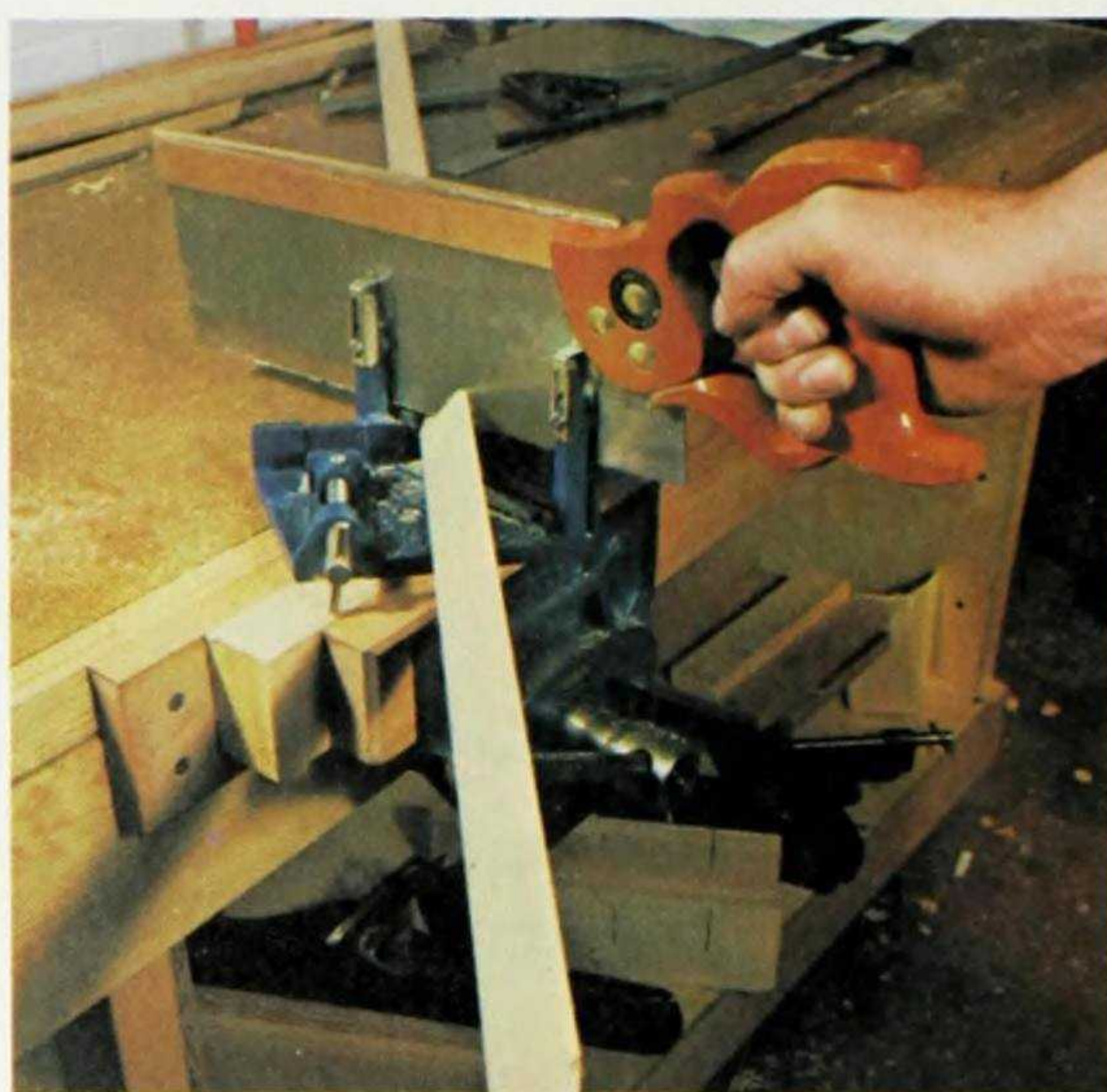
Fig. 2. A more expensive and accurate metal miter guide with built-in screw clamps to hold the wood steady.
