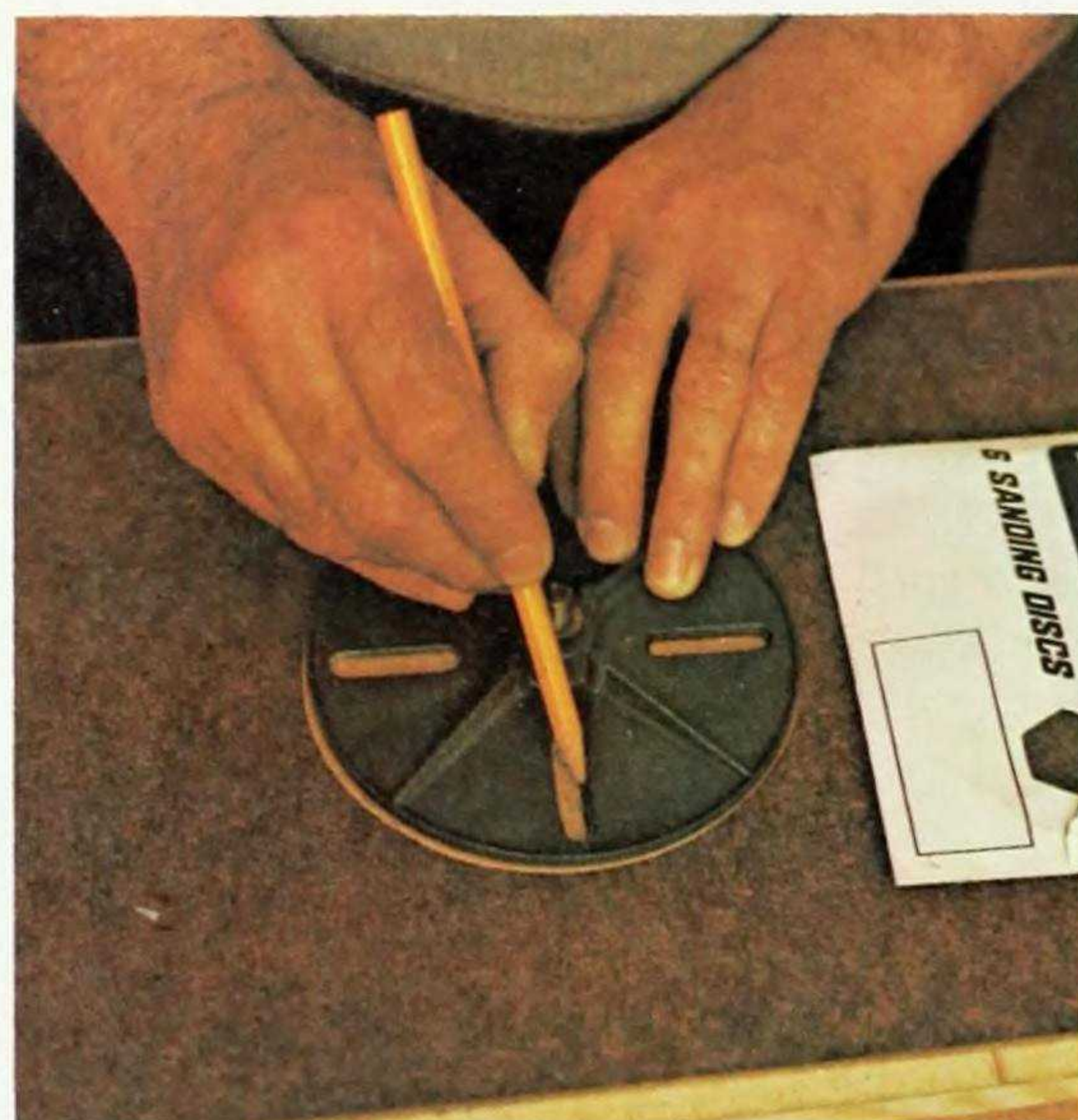
Fig. 8. An easy way of sharpening chisels without a grinder. First mark and cut slots in a fine-grade sanding disc . . .
