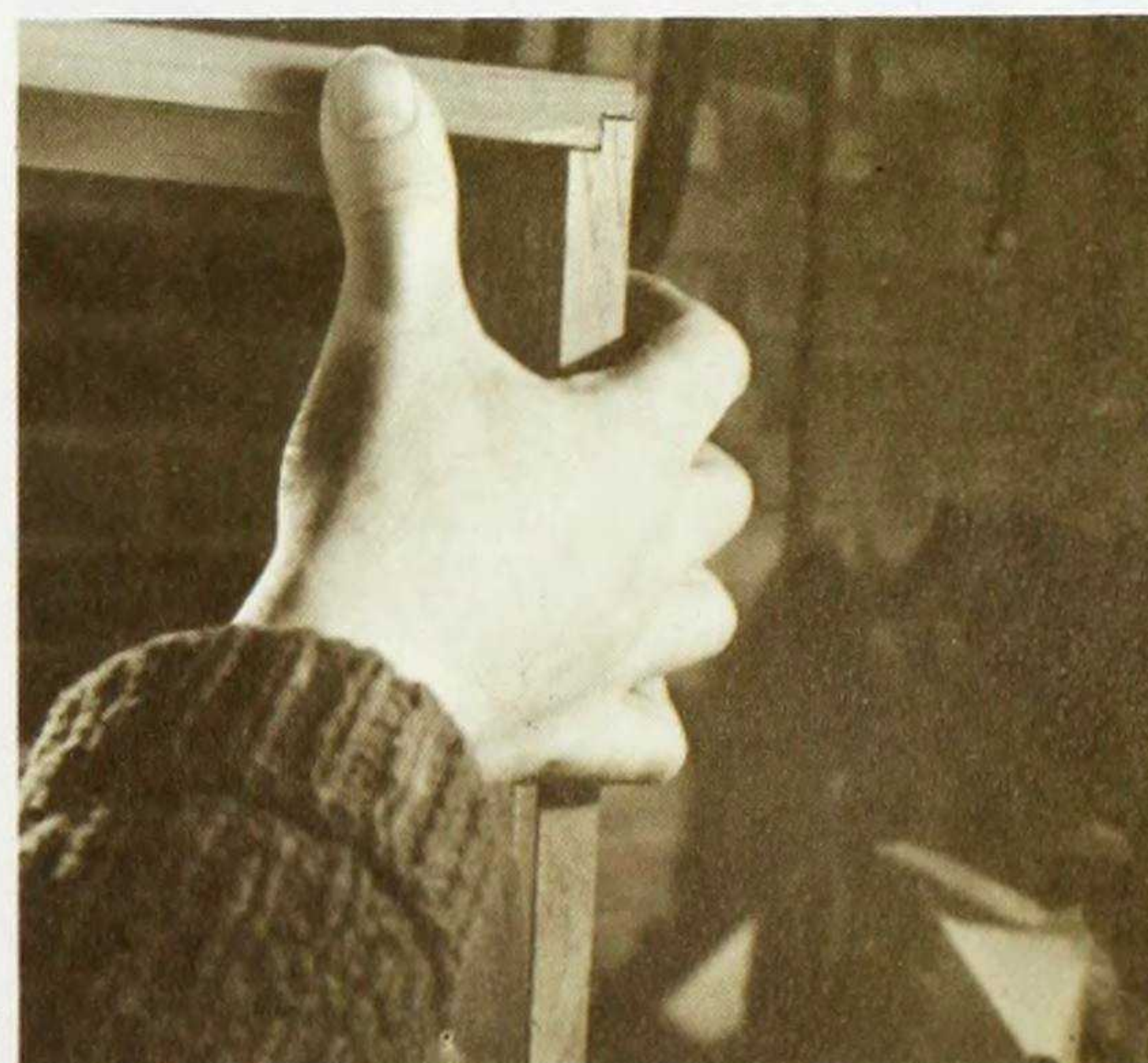
Fig. 7. When the two rabbet grooves have been cut, they are fitted to form the joints at the top of the bookcase.
