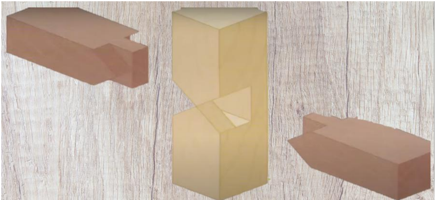
Sliding dovetail joint: Used in chair construction to connect legs to the rail.
