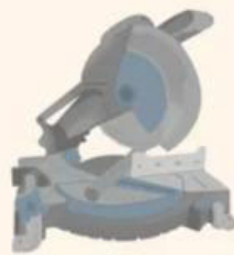
Compound Meter Saw
