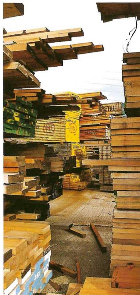
Above The country of origin of imported product is identified by distinctive shipping marks on the wood.
