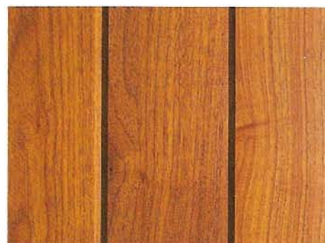
Above A fine example of black walnut, with a plain-sawn panel on the left, quarter-sawn on the right and rift-sawn in the centre. The changing angle of growth rings across the panel can be seen clearly.
