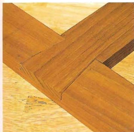
Above The finished lapped dovetail joint.
