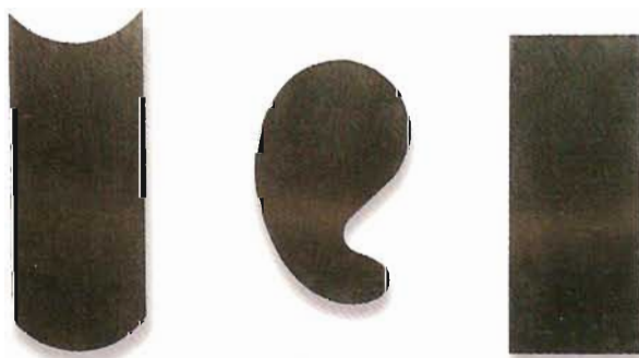
Concave, gooseneck and flat cabinet scrapers
