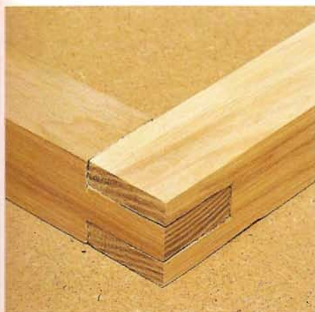
Above The completed corner bridle joint.
