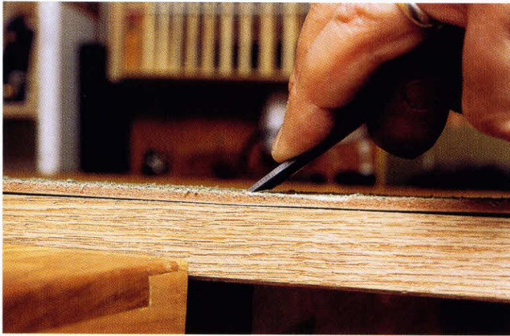
4-29. ♦ Stropping the microbevel. You can see in this photograph the very slight lifting of the edge so the strop will contact the microbevel.
