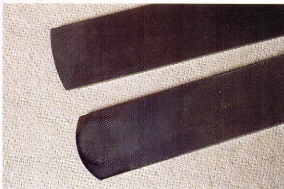
5-11. ♦ A Lie-Nielsen scrub-plane blade as it comes from the manufacturer (top) and ground to a 2\frac{1}{4} -inch radius (bottom). The blade with the more narrow radius will cut faster and with less effort.
