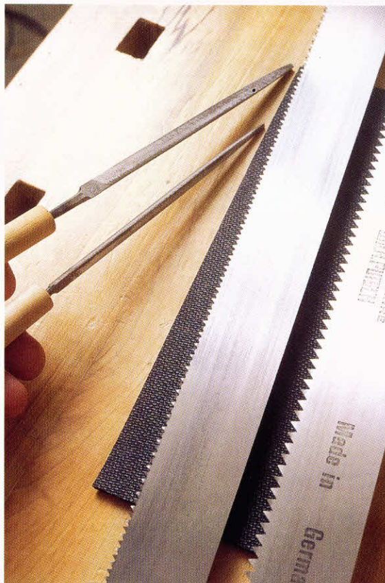
4-1. ♦ Left to right: slim file for 5-point blades; double extra-slim (XX) file for 9-point blades; 9-point bow-saw blade; and 5-point bow-saw blade.
