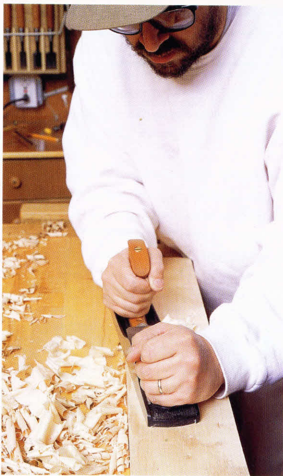
5-18. ♦ Finally, with the low-angle jack plane set for a very fine shaving, the board is planed with the grain.
