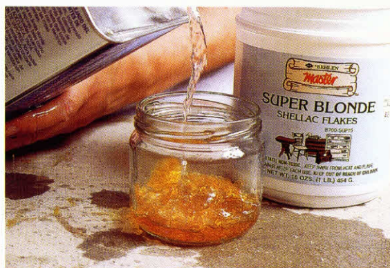
7-21. ♦ Adding denatured alcohol to super-blond shellac flakes. For a small amount like this, I cover the flakes about 1/2 inch with the alcohol.
