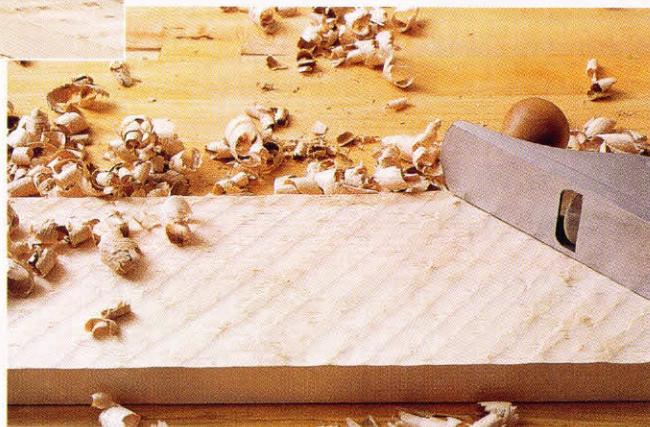
5-13. ♦ The rounded scrub-plane blade leaves ridges in the board. These will be removed with a jack plane.
