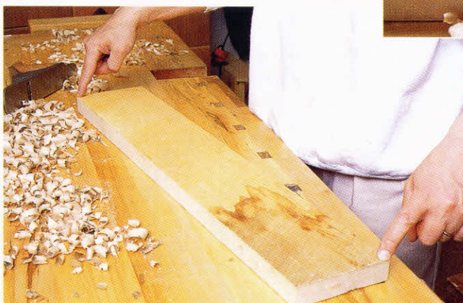
5-14. ♦ Rocking the board to check for flatness. Unless the board is very long, doing this on a flat workbench will tell you if it's flat or not.
