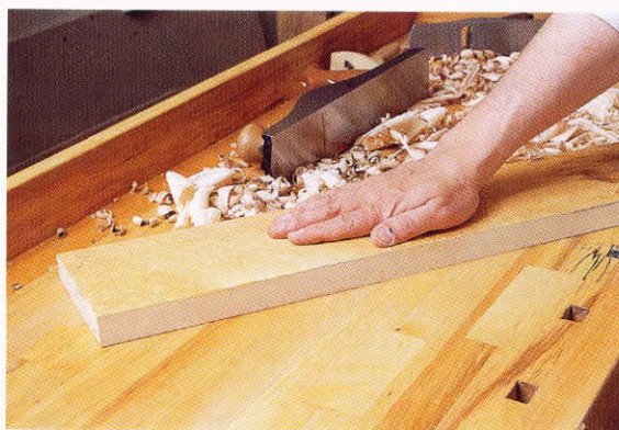
5-19. ♦ When finished, the board lies even with the benchtop. It's flat.
