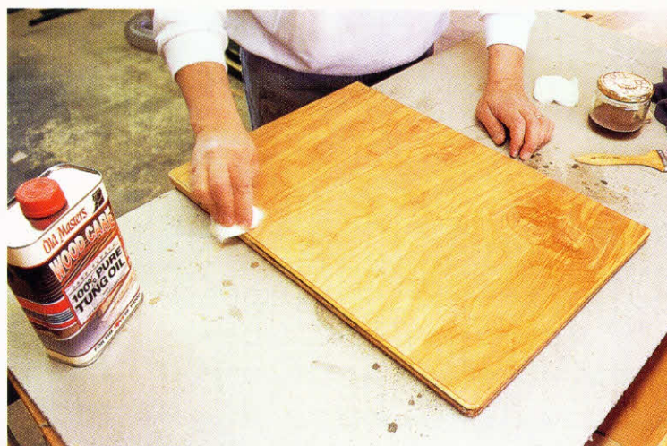
7-18. ♦ Removing tung oil with a rag. Once the surface has been flooded for about 30 minutes, excess oil can be wiped off.
