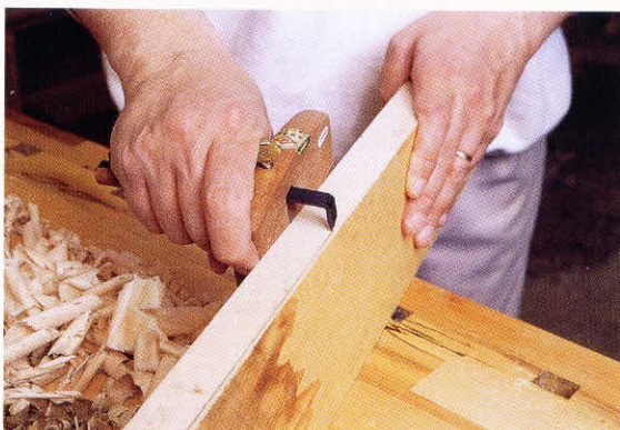
5-19. ♦ When finished, the board lies even with the benchtop. It's flat.
