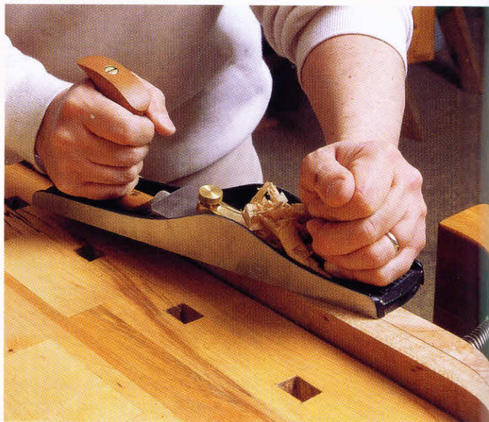
5-22. ♦ To edge-joint two boards, clamp them together and plane them both at the same time.
