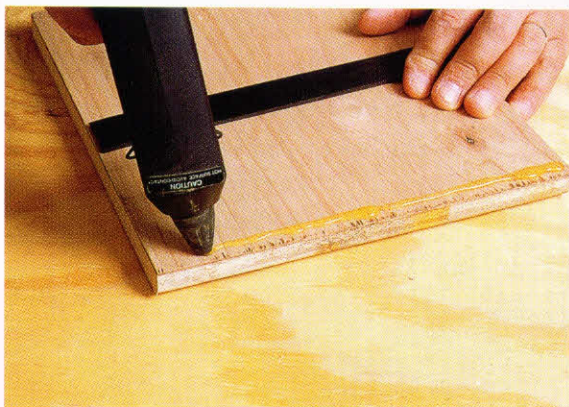
4-5. ♦ Spreading hot-melt glue to adhere the rubber jaws to the plywood. Cleaning the rubber pieces is a good idea. Work quickly!
