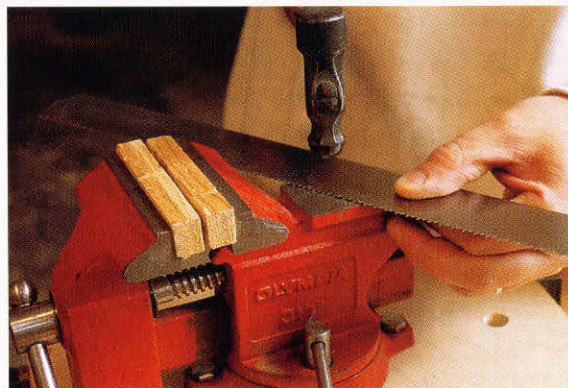
3-6. ♦ One tap per tooth from the small peen on a ball-peen hammer will remove excess set in a saw blade.
