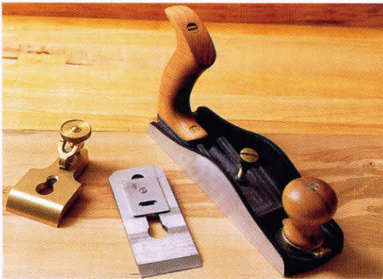
7-2 and 7-3. ♦ A low-angle smooth plane—like the jack plane—has few parts. It works especially well on difficult, knotty woods.
