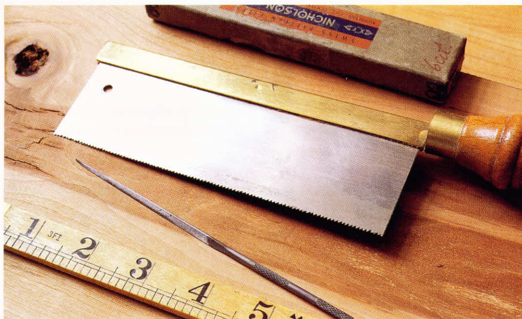
4-9. ♦ Needle file (chalked) shown above the wood rule. These tiny files are used to sharpen the very small gents-saw teeth. An easy, gentle touch is called for when filing these saw teeth.
