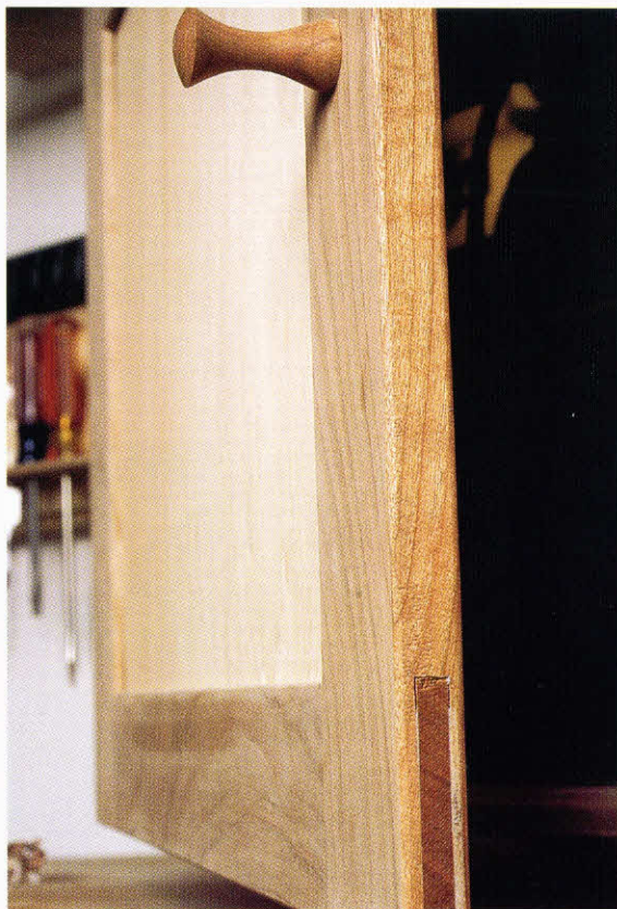
1–15. ♦ Bridle joint shown in a cabinet door. In this frame-and-panel door, the door stands alone and is hinged to the cabinet. The stronger bridle joint (or open mortise-and-tenon) is a better choice than the half lap.
