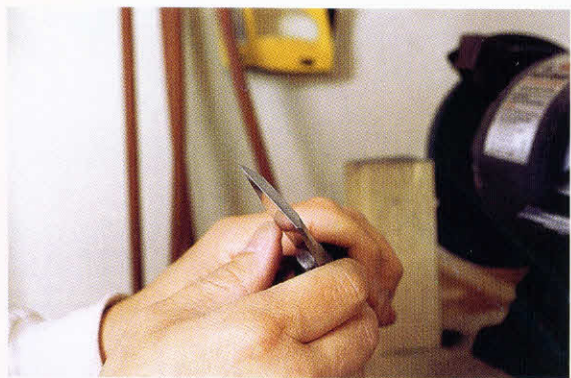
4-18. ♦ The light clearly glinting off the edge of the chisel blade after grinding to the line reveals that it's very dull. The next step is to grind the bevel until this line is about the width of a human hair—without burning the steel.
