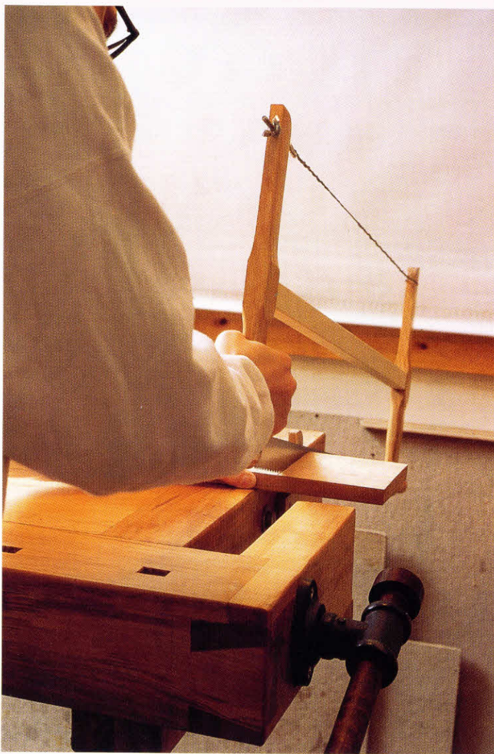
3-14. ♦ Crosscutting with a bow saw. If you grip the bow saw loosely and pay attention on the cutting line, the bow saw will seem to almost cut by itself.
