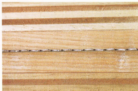
3-7. ♦ These 5-point bow-saw teeth have the proper amount of set. They look like they have no set at all.
