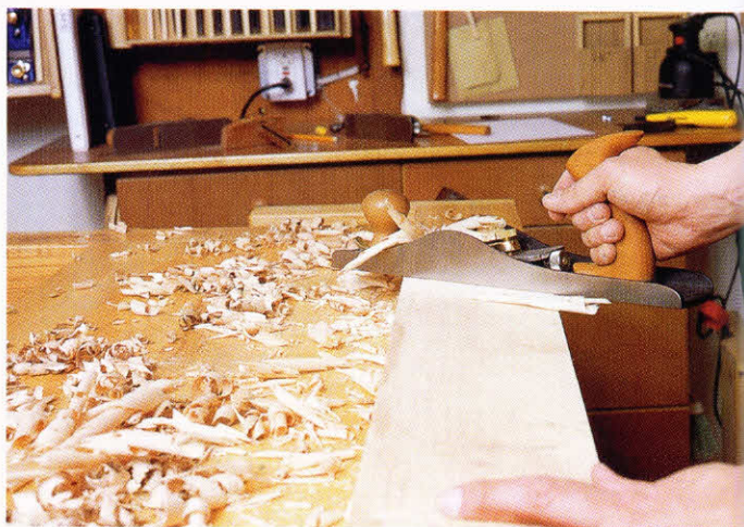
5–16. ♦ With the jack plane set for a slightly thick shaving, the diagonal planing motion is repeated to remove the scrub-plane ridges (but not to unflatten the board!).
