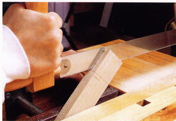
6-6. ♦ Sawing to the line with a 9-point bow saw (German). Clamping the piece at an angle helps to begin the joint-cutting.
