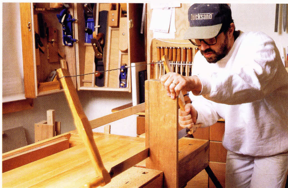
3-15. ♦ Rip-sawing with a bow saw. A bow-saw blade can be turned at an angle to the frame to clear the board for work like this. These saws cut so well you can do entire projects with them.
