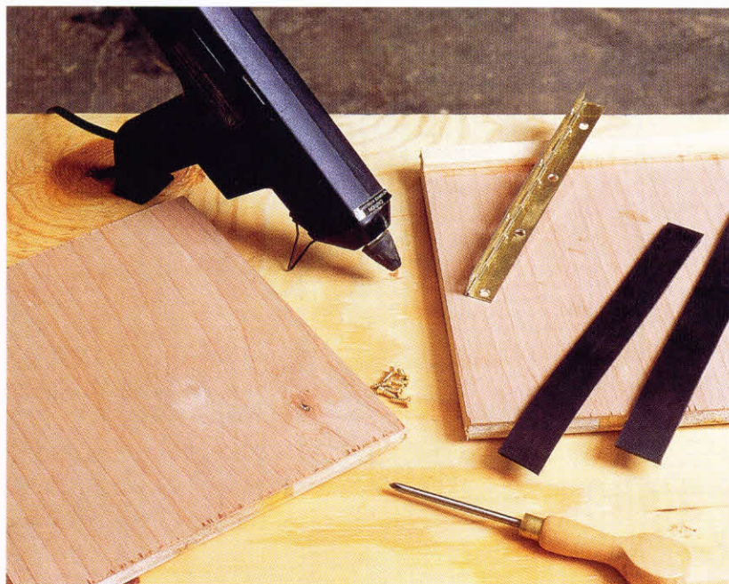
4-4. ♦ Materials necessary for making a sharpening vise: plywood pieces, rubber strips, hinges (a scrap of piano hinge is shown here), hot-melt glue gun, and screwdriver. Note that the spacer piece is already glued to one of the pieces of plywood.
