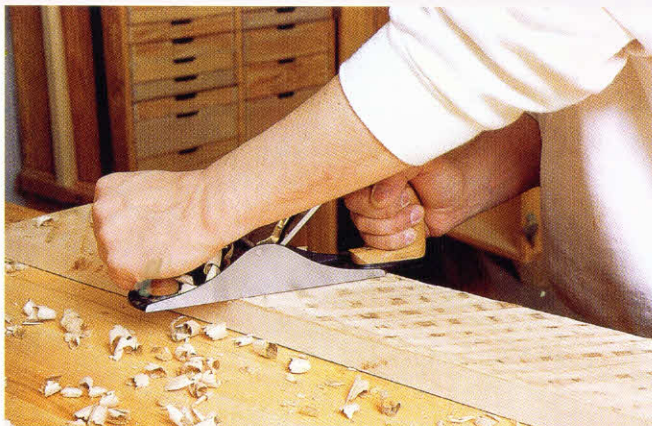
5-12. ♦ Scrub-planing. Go diagonally down the board in one direction, and then from the other.
