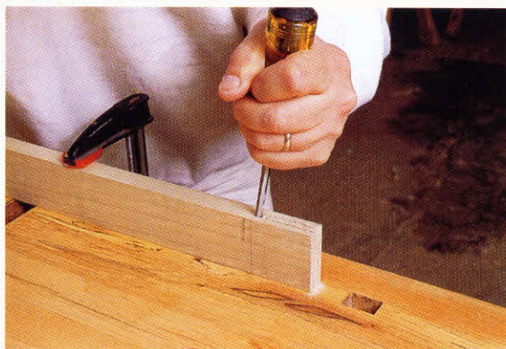
6-8. ♦ Chopping out the bridle-joint mortise. Here, I'm just beginning, and you can see the chisel angled slightly for the undercutting in the end grain.
