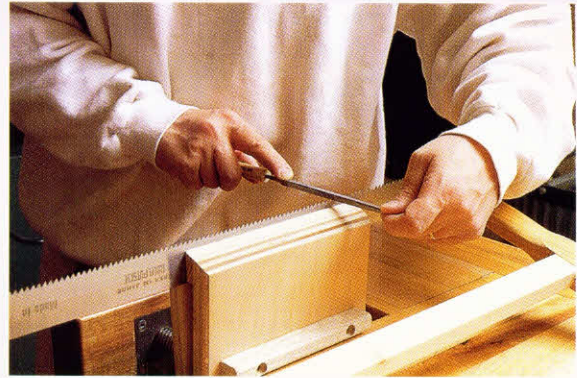
4-12. ♦ With the blade at a comfortable height, one or two strokes per tooth will get it nice and sharp. The file is perpendicular to the saw blade's horizontal and vertical axes.
