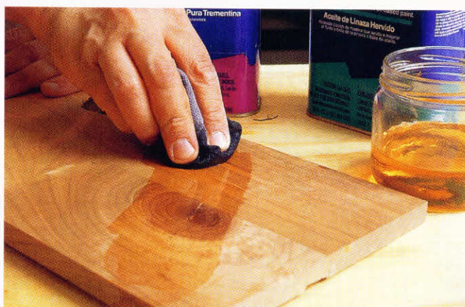
7-16. ♦ Applying linseed oil with a rag. Use generous amounts of oil—especially for the first coat. Linseed oil darkens the wood more than other oil finishes. Promptly dispose of the rags outside after use.
