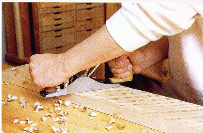
5-12. ♦ Scrub-planing. Go diagonally down the board in one direction, and then from the other.
