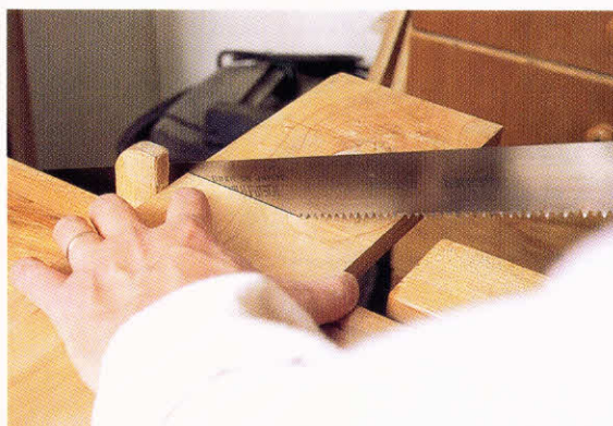
2-16. ♦ The saw blade rests in the V-cut and it's easy to saw cleanly and accurately.
