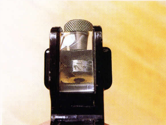
3-11. ♦ The saw set at the proper setting for 5-point bow-saw teeth.
