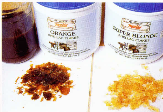
7-20. ♦ Orange and super-blond shellac. The flakes are mixed with denatured alcohol to make a working solution. Orange shellac is good for darker woods, super blonde for lighter woods.
