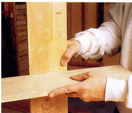
1-1. ◆ Good glue surface. An edge surface being bonded to a face surface.
