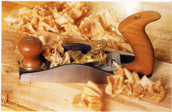
7-4. ♦ A low-angle smooth plane can be used for surface preparation. The low-angle design makes it possible to plane even a difficult surface. Note the thin shavings that can be produced with this plane.
