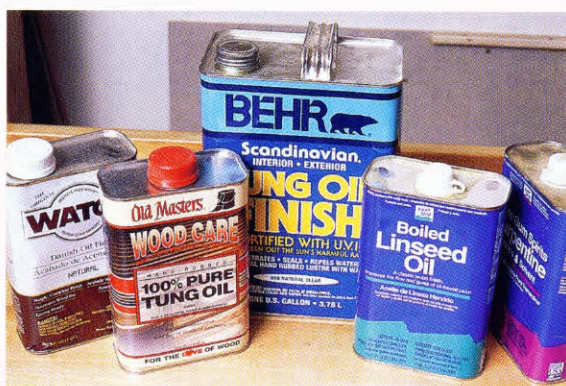
7-13. ♦ All of these penetrating oil finishes will do a fine job on furniture. An oil finish gives the wood a plain, natural look.
