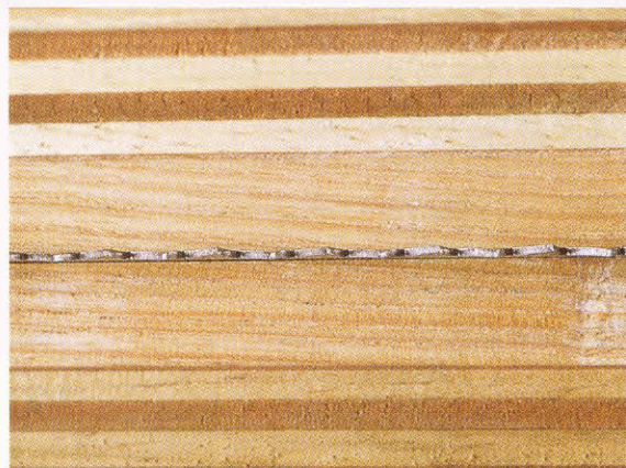
I-2. ♦ A close-up of the teeth on a bow saw showing the proper amount of set. Chapter Four discusses sharpening techniques for bow saws, plane irons, chisels, etc.
