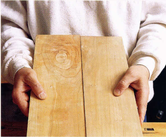
1-3. ♦ Good glue surface. An edge-to-edge bonding.
