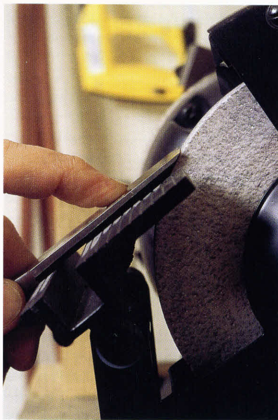
4-19. ♦ Setting the tool rest using the existing bevel on the chisel. The bevel angle doesn't have to be precise. It should be about 25 degrees; a few degrees either way is fine.
