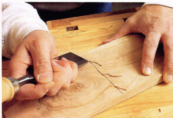
2-14. ♦ Using a chisel to make the V-cut.
