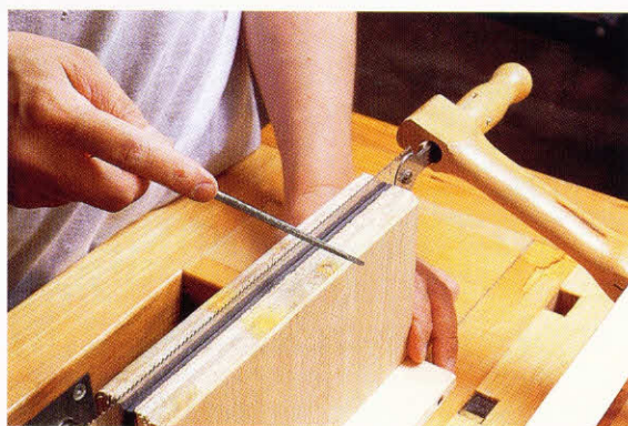
4-8. ♦ The vise about to be put to use. The rubber jaws lock the saw blade tightly in place. Note the lower cleat, which holds the vise up against the Scandinavian workbench. If you're using an English-style vise, you don't need it.
