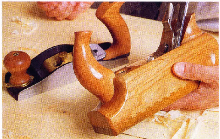
7-8. ♦ Wooden smooth plane. This is a good, general-purpose smooth plane.
