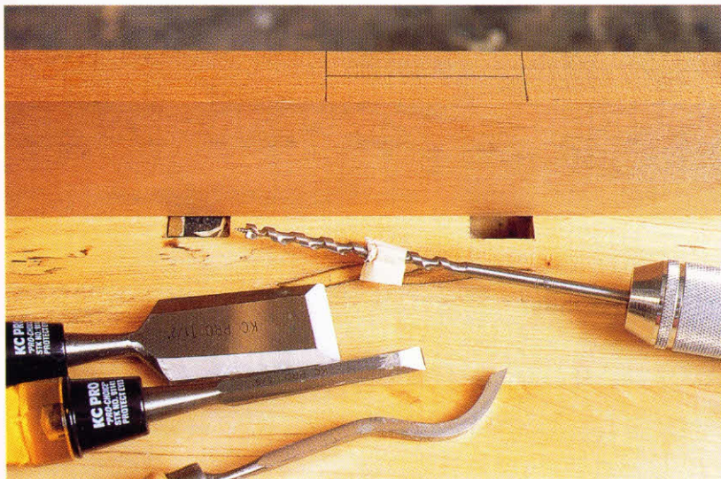
6-17. ♦ As shown in the background, the edges and the center of the mortise have been marked. Note the crank-neck chisel in the foreground; it is useful, but not essential, for cleaning out the bottoms of housed mortises.
