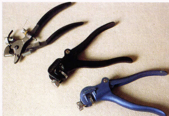
3-9. ♦ Saw sets. The middle and bottom saw sets are easy to use. The top one is a German model that's a bit more difficult to use.
