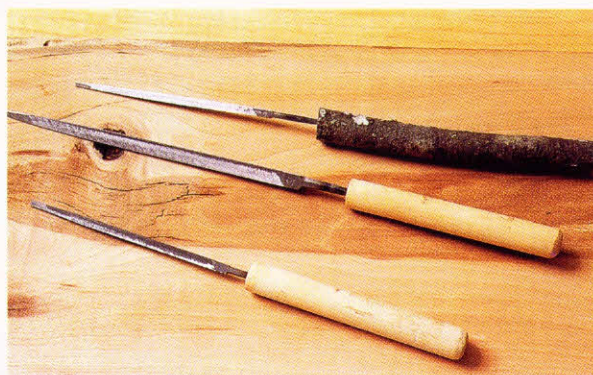
4-10. ♦ Files for sharpening handsaws. I use pieces of dowel for handles (old, discarded foam-brush handles work well). Round over the ends for comfort. Shown on top is a handle I made from a tree branch.
