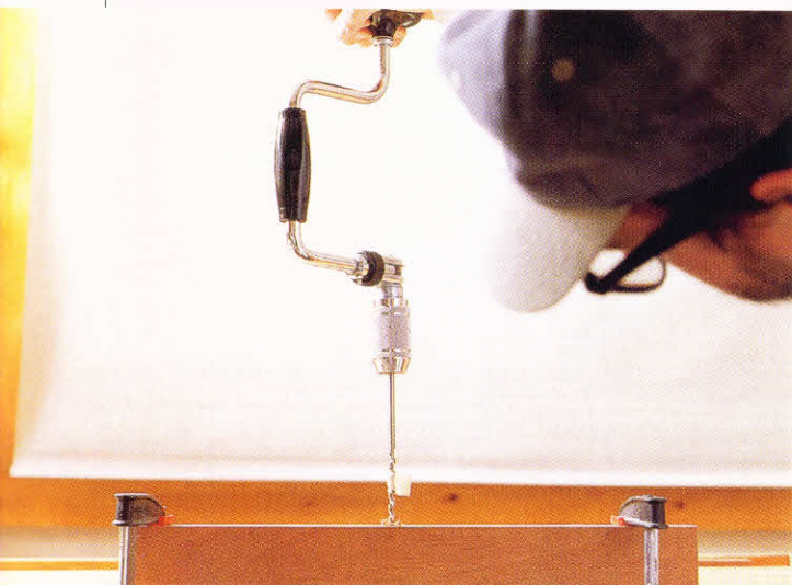
6-18. ♦ Aligning the brace and bit with the work. After a while, boring straight, square holes with this tool becomes a matter of "feel."
