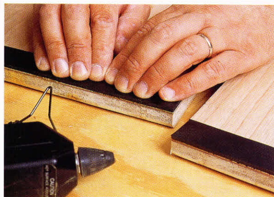
4-6. ♦ Pressing the rubber jaw into position on the inside top of the plywood piece.
