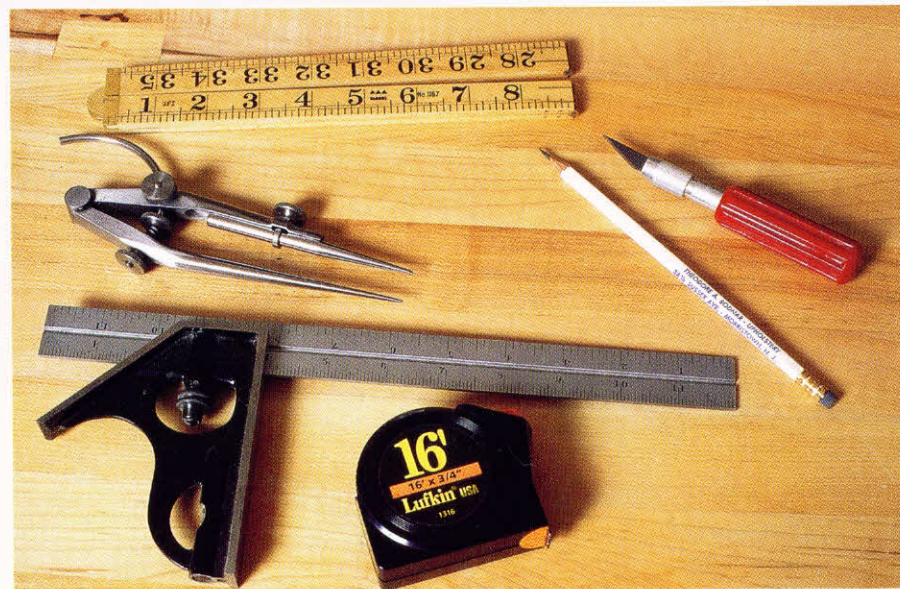
2-2. ♦ The tools needed for measuring and marking wood. Clockwise from the top: a folding rule, marking knife, pencil, tape measure, combination square, and dividers.
