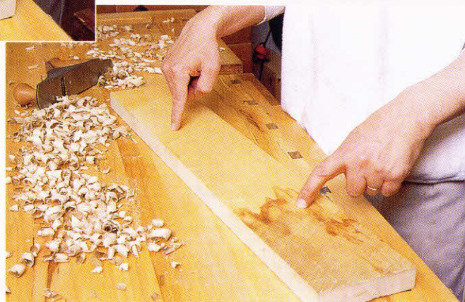
5-15. ♦ If the board still rocks after scrub planing, move your fingers in until it stops rocking. In between them is a high spot.
