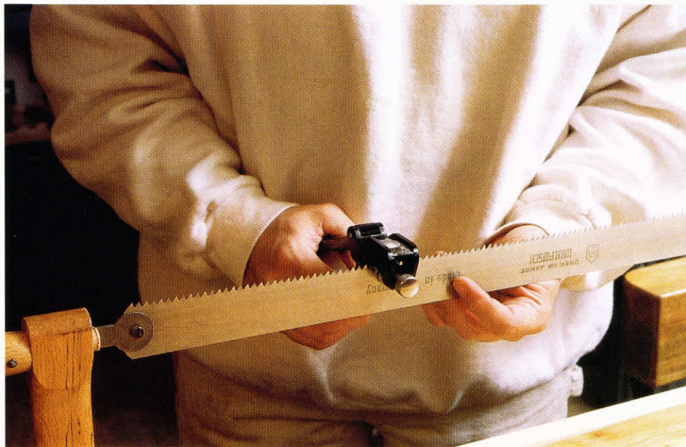
3-13. ♦ Setting saw teeth. Here I'm using the Stanley saw set on my 5-point bow saw. The saw set pushes the teeth away from you, so do one side, turn the saw around, and then do the other.
