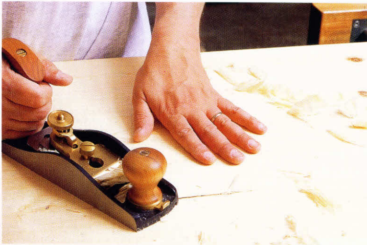
7-5. ♦ Using a low-angle smooth plane to prepare the surface for a finish.
