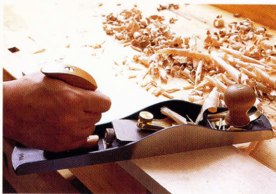
5-1. ♦ Removing scrub-plane marks with a jack plane. Most difficulties with hand-plane use stem from poorly manufactured tools and/or using the wrong plane for a given job.
