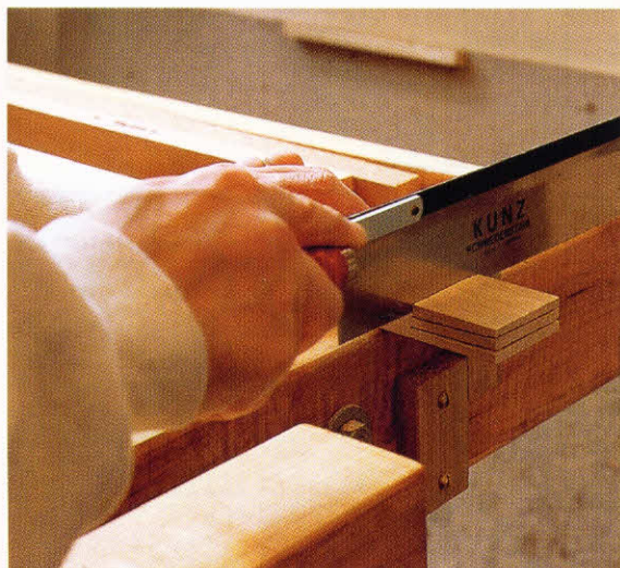
6-10. ♦ Cutting the tenon shoulders. Since the material I'm removing is about \frac{1}{4} inch thick, the small saw works well.
