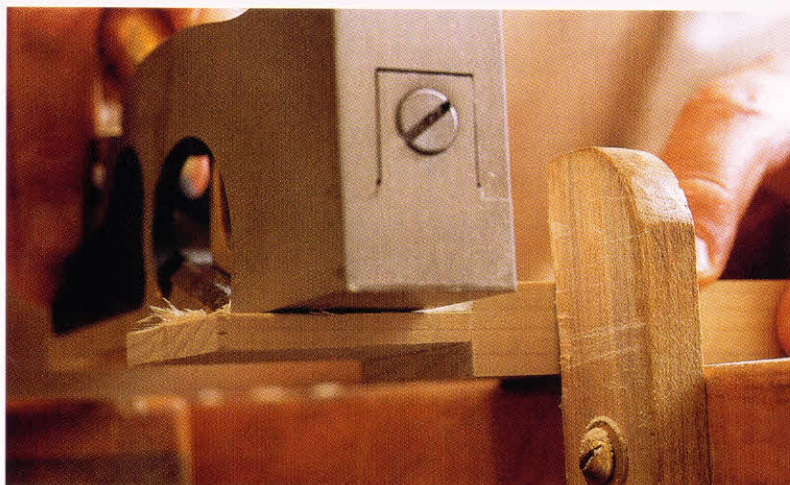
6-11. ♦ Using a shoulder plane to trim the tenon cheeks (the wide parts) for a good fit.
