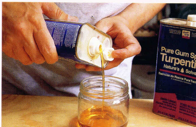
7-14. ♦ Preparing a first-coat linseed-oil finish. First, pour boiled linseed oil into a glass jar.
