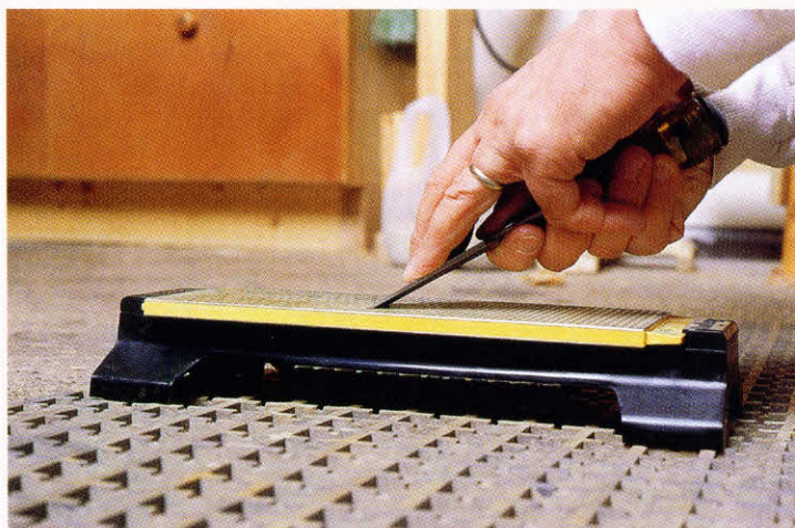
4-26. ♦ Honing the microbevel. The grip is firm, but relaxed. When the hairline of light no longer glints off the edge, this step is done.
