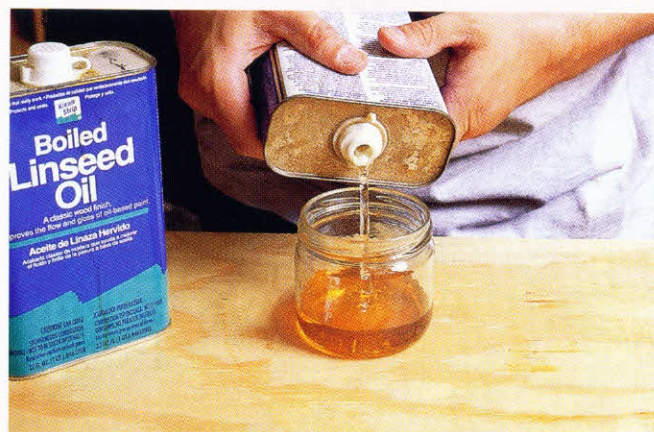
7-15. ♦ Adding turpentine to the linseed oil. About a 50-50 mix of turpentine and oil works well.
