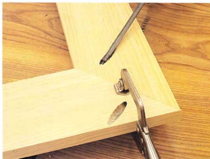
CORNER MITER JOINTS
