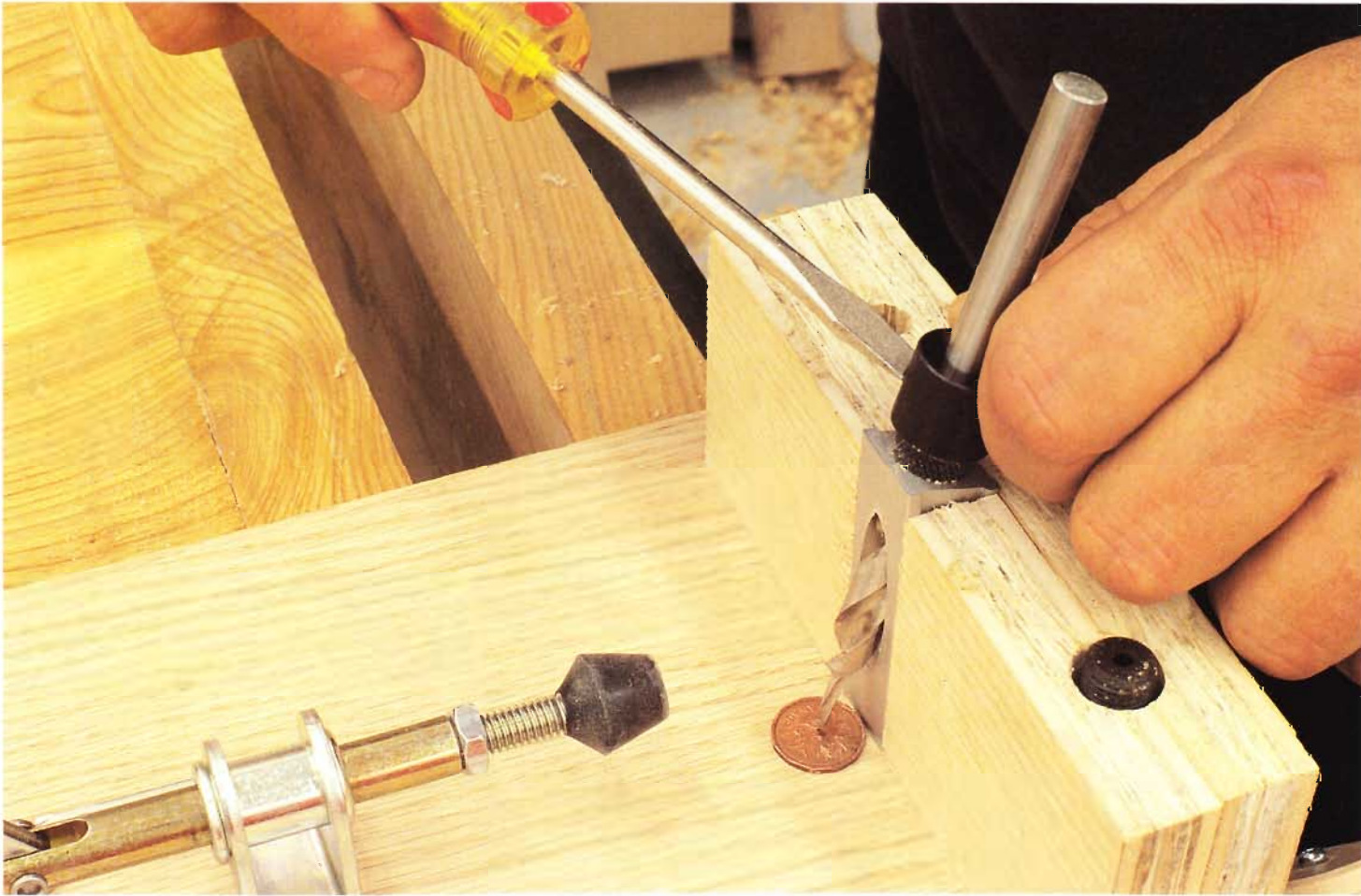
THIS IS A DRILL BIT STOP COLLAR SETTING.
