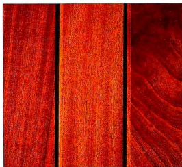
Above Sapele is an example of a hardwood with a difficult grain, the alternate formation of each band of cells producing a striped effect. The right-hand panel in this photograph not only shows unacceptable short grain, but also another defect known as reaction wood.
