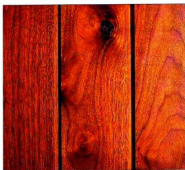
Above This panel of black walnut contains a good example of a dead knot. The small "pin" knot lower down creates an attractive pattern, but the large dead knot above it is a defect to be avoided.
