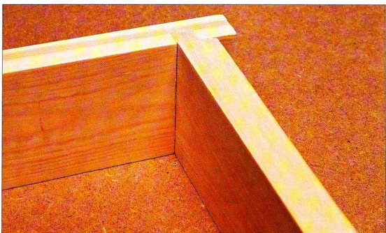
Above The finished bare-faced housing joint.
