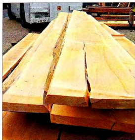
Above This shows how not to air dry timber. The boards have been piled in irregular fashion, unprotected from the heat of the sun. Rapid, uneven drying can split a board quite easily. Note the discolouration where the sticks were laid.
