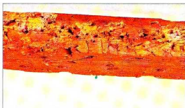
Left Woodworm damage
