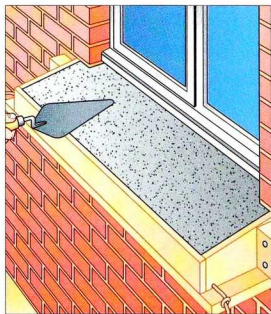
Above Fill the shuttering with concrete, making sure the surface is level.
