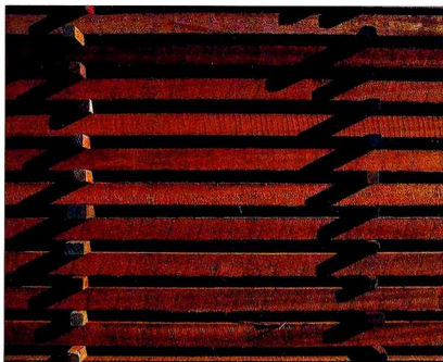
Below An air-dried timber (lumber) stack.
