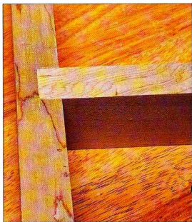
Above The completed full housing joint.
