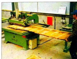
Above Resawing an oak board to remove the heart shake.
