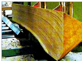
Above Quarter sawing oak on a bandmill.
