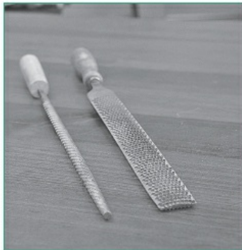
Round or rat-tail rasp (left) and combination flat and curved rasp (right)
