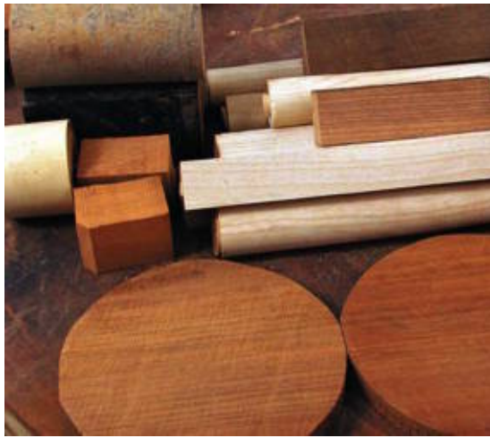
The grain in the face-work discs ( front ), tool handle blanks ( rear right ), and end-grain blanks ( rear left ) runs from left to right.
