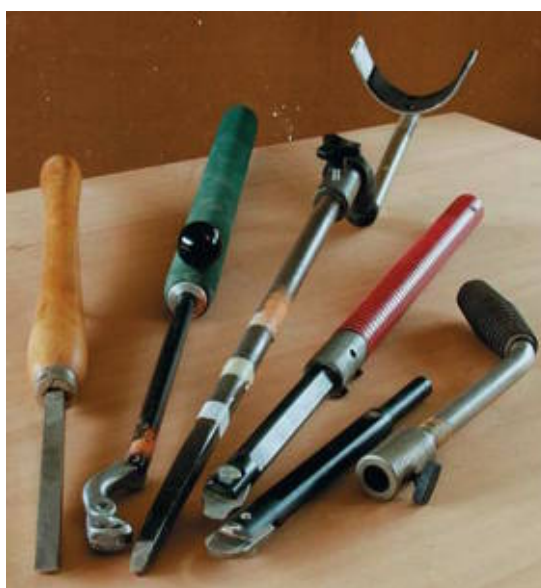
Deep-hollowing tools need to be long and strong or have a Stewart system arm-brace ( center ) or pistol-grip handle ( right ).
