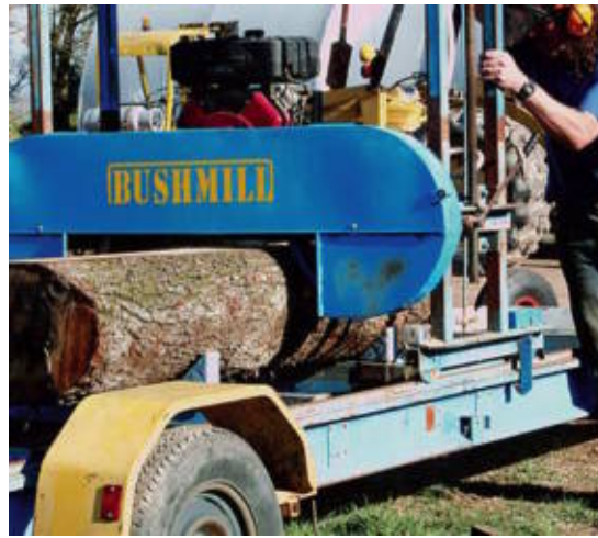
A portable bandsaw mill makes quick work of sawing logs into manageable sizes. The resulting slabs will be cut into a range of turning blanks.
