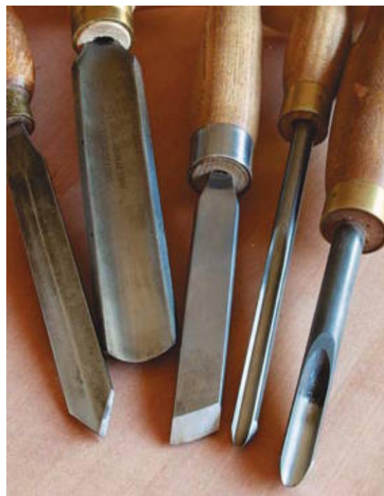
Center-work tools commonly include (from left) a parting tool, a roughing gouge, a skew chisel, and various spindle gouges.
