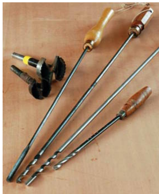
Forstner or multispur bits ( left ) will bore large-diameter holes in items such as pepper mills and hollow forms. Long drills and augers ( center ) are used for drilling out lamp bases. Many holes can be bored free-hand on the lathe using a depth drill ( right ).
