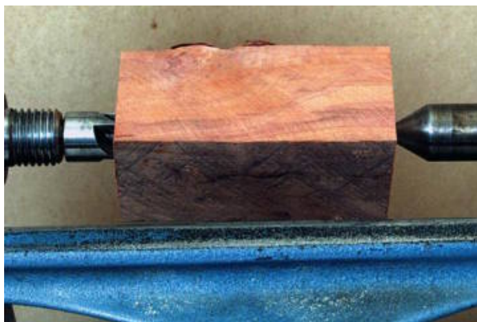
Center work, also called spindle work, is mounted between a spur drive center ( left ) and a tail center.
