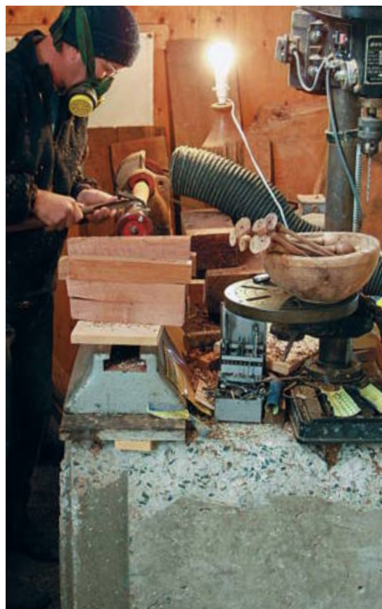
An ancient lathe bolted to a ton of concrete runs vibration free. The motor for this lathe is set to the rear of the headstock.
