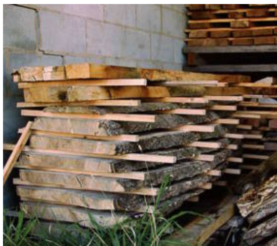
This slatted elm log is being naturally air dried. The wooden stickers separating the slabs allow air circulation.
