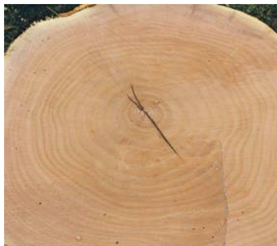
Most logs contain major splits across the pith at the center as well as shallow splits at the surface, called checks .
