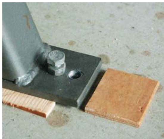
Use blocks or wedges to level and support the lathe before bolting it to the floor.
