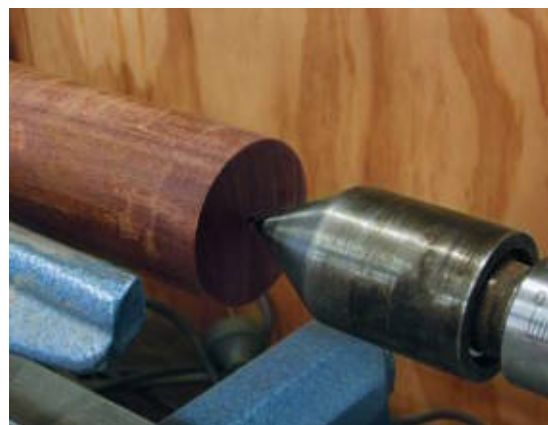
To check the alignment halfway down the bed, inspect the rotation of a chuck-mounted cylinder in relation to the tail-center point.
