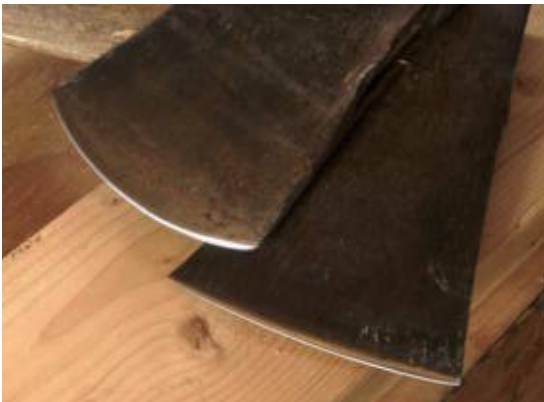
An ax with a curved edge (left) is better to use for green hardwood, whereas a straighter edge (right) works better in dry wood.
