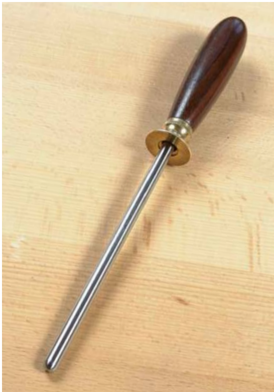
Burnishing tools, whether triangular, round, or oval in cross section, are made of polished, hardened steel.
