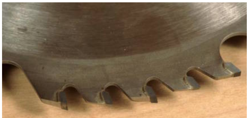
Carbide sawteeth have very high bevel angles because the material is very brittle as well as hard.
