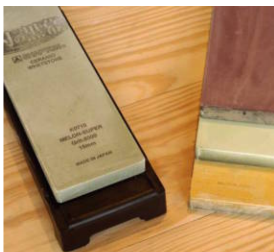
Shapton waterstones, in grits of 1,000, 2,000, 5,000, and 8,000, cut quickly and wear well.
