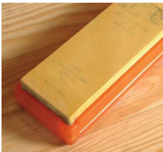
Shapton's storage box doubles as a stone holder for sharpening.
