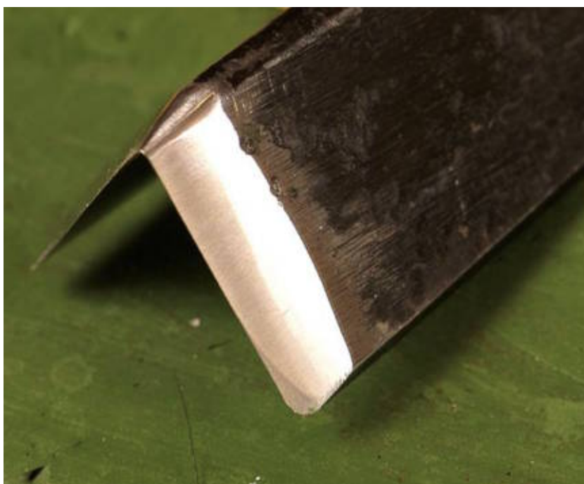
The part of a bevel that meets the shank of a carving tool is called the heel. It should be gently rounded and polished so it bur-nishes the cut.
