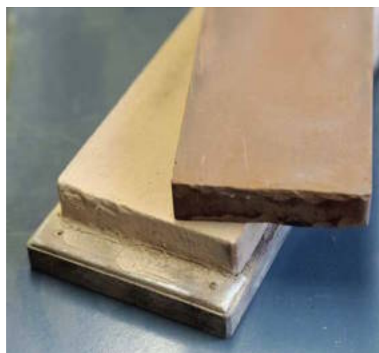
Man-made Japanese waterstones cut fast and are a good value, but they must be flattened regularly.
