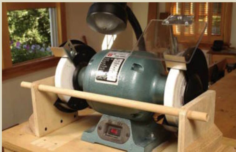
This jig can be used for both honing and grinding, making it more convenient than a single-purpose jig.
