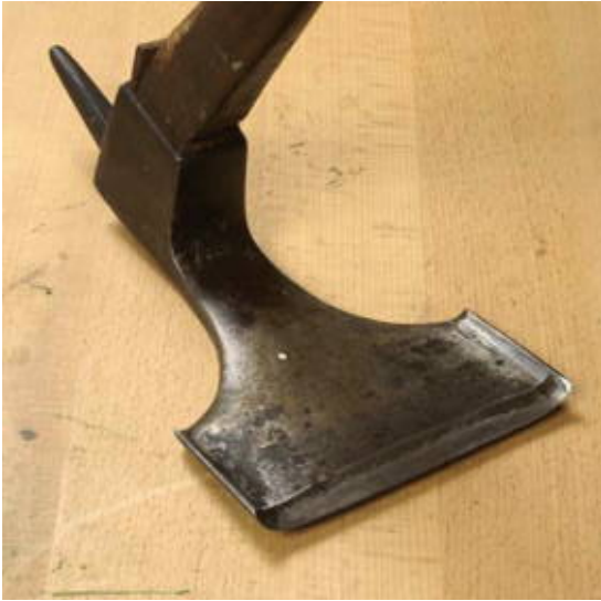
A shipwright's lipped adze is designed to cut cleanly across the grain.
