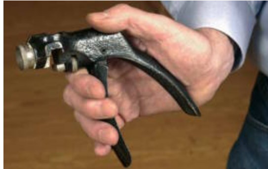
Pistol-gripped saw sets are the most comfortable style to use for extended periods of time.
