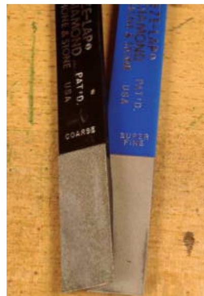
Diamond files are handy for honing hardened-steel tools, especially odd shapes.
