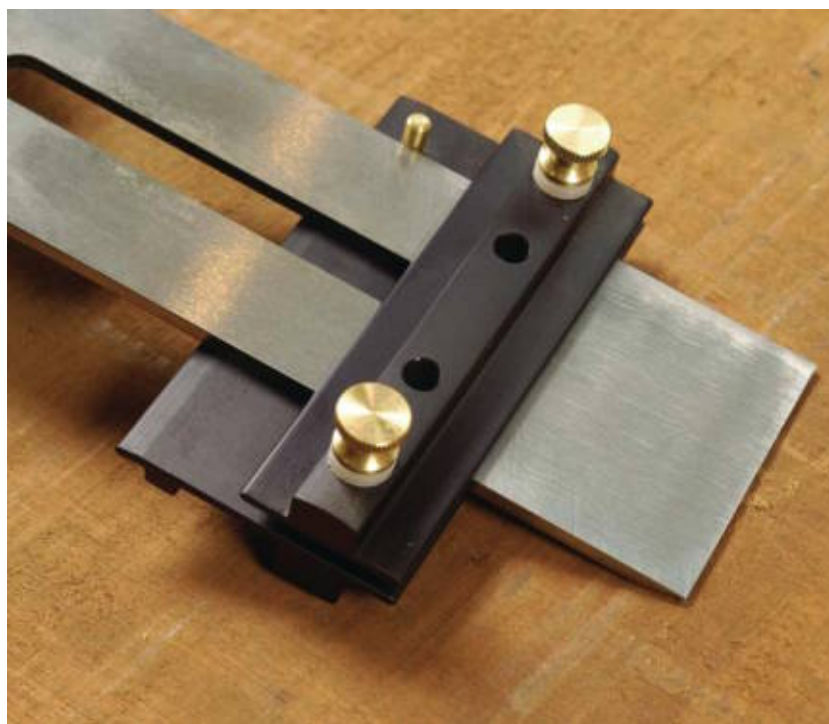
An alignment pin on the Veritas grinding jig helps keep blades square but also can be used with skew blades.
