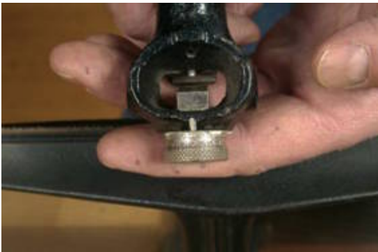
Numbers on the set's adjustment knob correspond to the number of teeth per inch on the saw.
