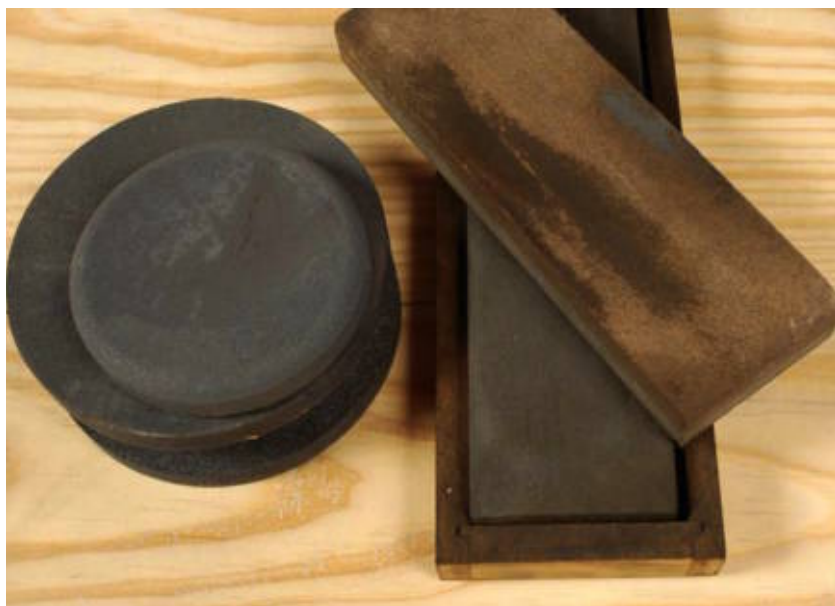
Crystolon ax stones and fine India oilstones are good for heavy stock removal.
