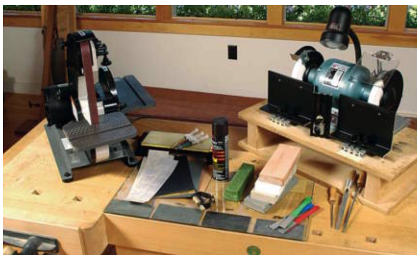
A top-of-the-line sharpening kit also includes a 1-in. belt sander and several grades of diamond paste.
