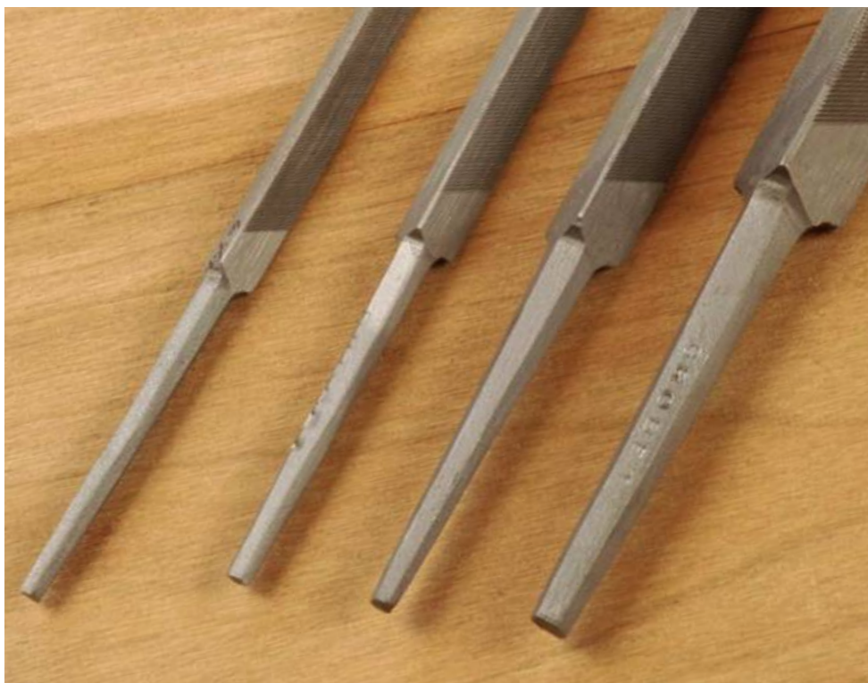
Six-inch triangular files come in several standard sizes, including regular taper, slim taper, extra slim, and double extra slim.
