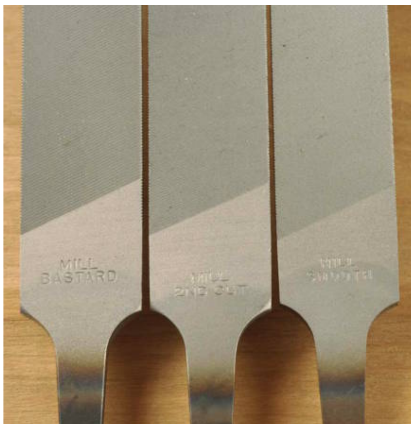
From coarse to fine: bastard, second-cut, and smooth files.
