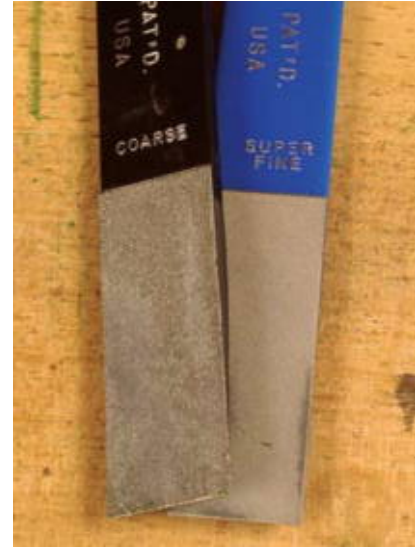
Diamond files are useful for shaping and cleanup. They cut quickly.
