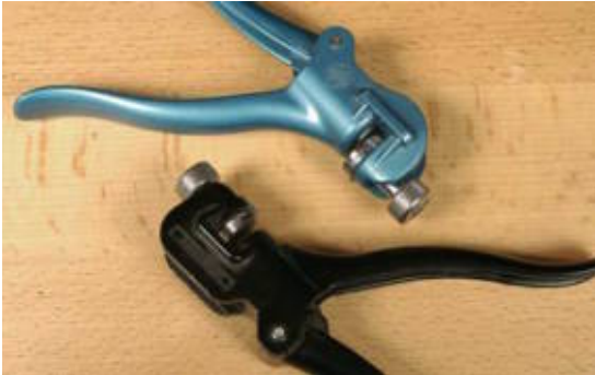
Saw sets are adjustable devices that bend teeth away from the sawblade.
