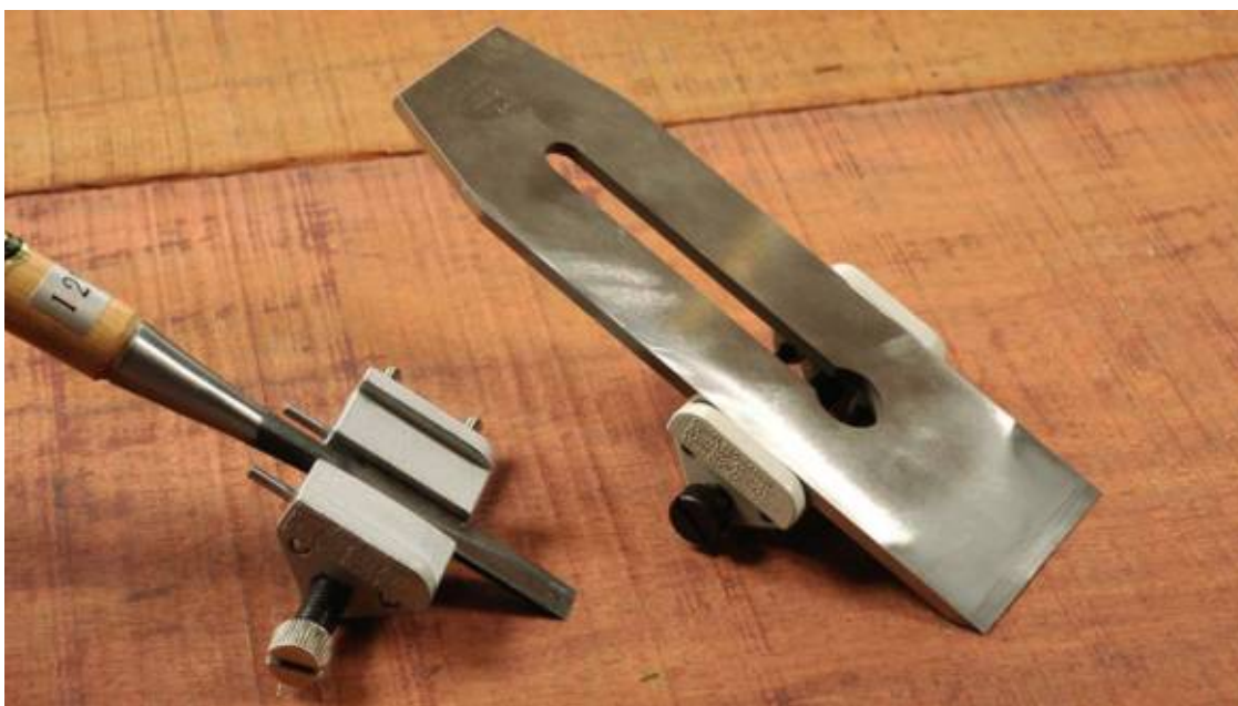
An Eclipse jig clamps blades from the side, making it easier to hone a square edge.
