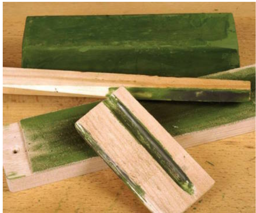
A leather strop with honing compound puts on a final edge. Simple wooden slips can be made to fit specific carving tools and be saved for future use.
