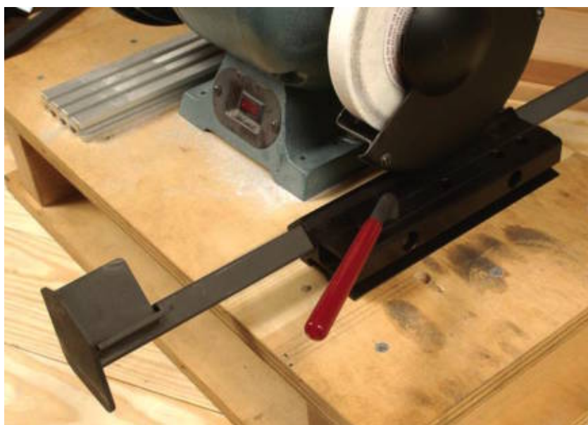
The adjustable Vee Arm attachment for the Wolverine system allows a gouge bevel to be ground accurately.
