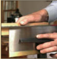
150 Jointing and Setting
