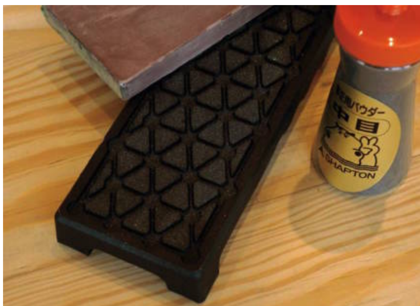
Shapton's lapping system for flattening waterstones includes a steel plate and abrasive powders.
