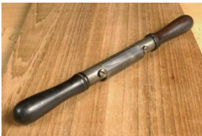
A cigar spokeshave has a semicircular blade whose bevel is honed on a stone. The inside of the curve is touched up with slipstones.
