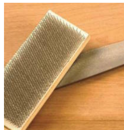
A file card is used to clean debris from the teeth of a file.
