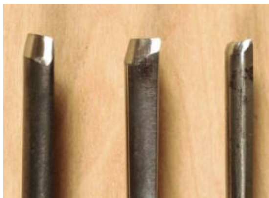
Gouges can be sharpened with a forward or backward sweep but are usually sharpened square.
