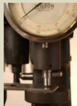
The Rockwell hardness tester is an industry standard for precisely measuring the hardness of tool steels. It presses a stylus into the steel's surface under controlled pressure.
