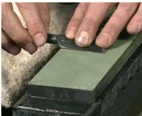
Japanese tools are traditionally sharpened on waterstones.
