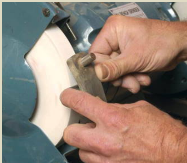
Before putting tool to stone, make sure the face of the grinding wheel is flat and square to the sides. A diamond dresser makes the process fast.
