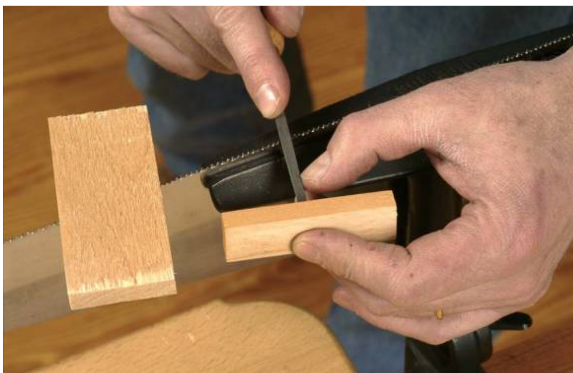
A small block of wood on the end of the file helps maintain the rake angle. A second block guides the file at the right fleam angle.
