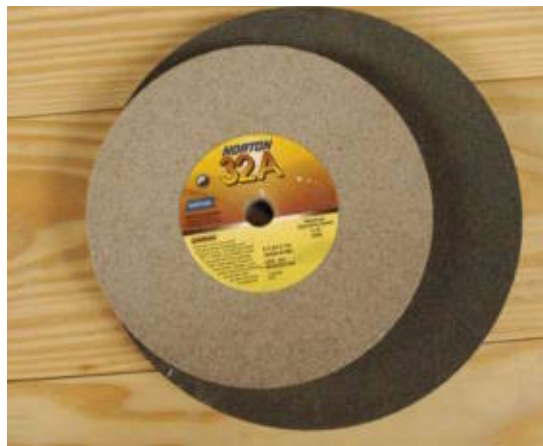
An 8-in. grinding wheel is a better choice for turning tools than a 6-in. wheel because the hollow grind it creates is less pronounced and, as a result, stronger.
