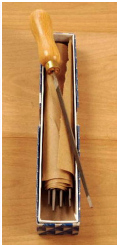
Six-inch triangular files come in several standard sizes, including regular taper, slim taper, extra slim, and double extra slim.
