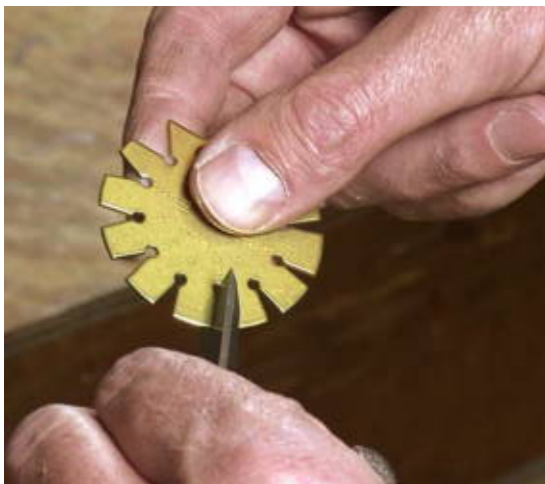
Carbide sawteeth have very high bevel angles because the material is very brittle as well as hard.
