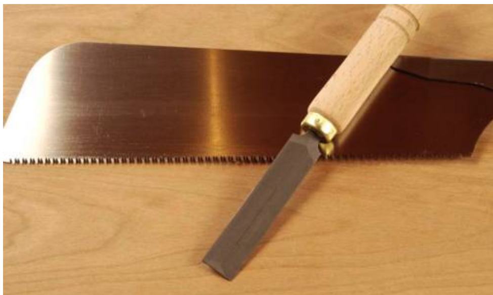
Feather files are used to sharpen Japanese saws.
