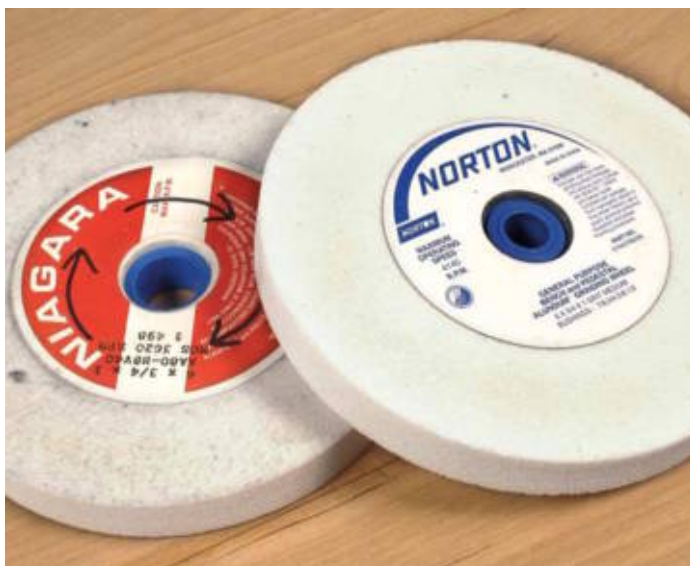
Friable aluminum-oxide grinding wheels wear a little more quickly than standard wheels but dissipate heat more efficiently.
