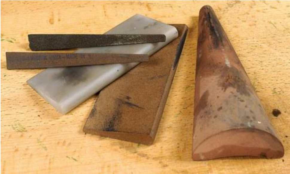
Triangular India slipstones, fine India and Arkansas slipstones, and India gouge slipstones are good for both gouges and parting tools.
