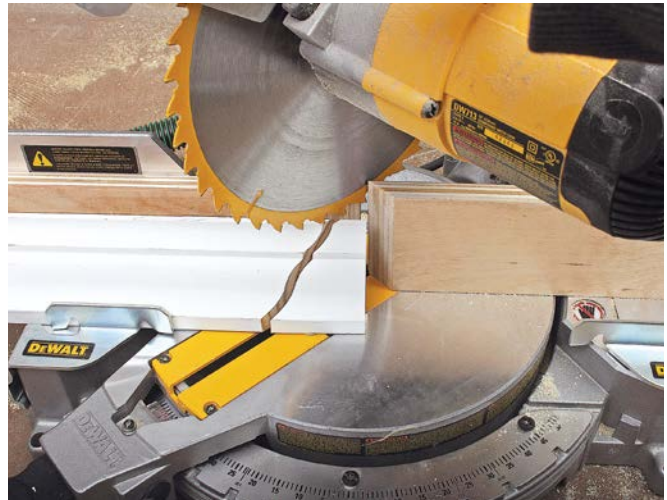
RIGHT INSIDE. To cut the right side of an inside corner (in preparation for making a cope cut), adjust the blade to a 45-degree angle to the left and place the board to the left.
