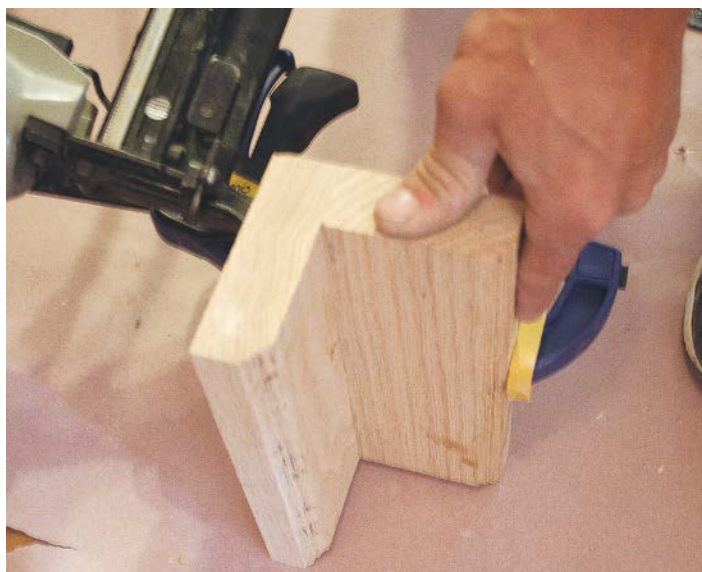
DOUBLE PLINTH BLOCK. At a corner, make a plinth block with two pieces fastened together. Rout the edges of only one side of each piece. (This doubled plinth is seen in the top left photo on p. 142).
