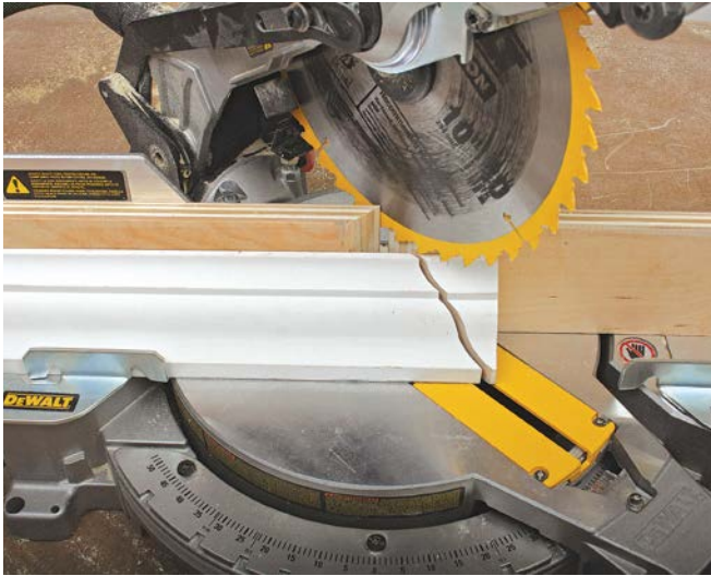
RIGHT OUTSIDE. To cut the right side of an outside miter, adjust the blade to a 45-degree angle to the right and place the board to the left.
