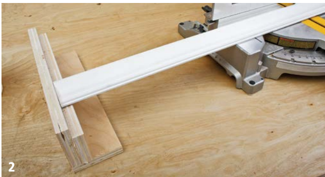
SUPPORT OR STOP. Use as a support for long boards (1) or as a stop guide (2).
