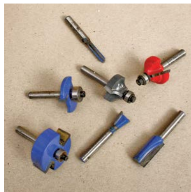
ROUTER BITS. An assortment of router bits can be used, perhaps in combination, to make a great many profiles.
