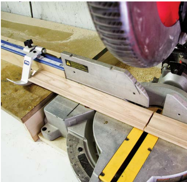
SHOP SETUP. Secure the miter saw to a workbench and set up a working surface on either side.
