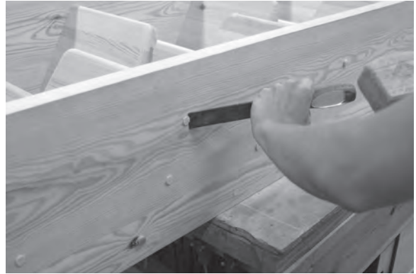
Figure 9.62 Carefully cut the protruding pellets flush with the surface of the string.
