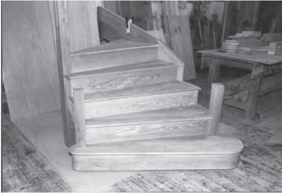
Figure 10.62 (above) and Figure 10.63 (below) The circular section of the newly built Ascot staircase – still in the workshop – with its open-to-closed right-hand string.
