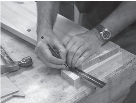
Figure 8.84 Mark the nosing return's 25mm rear projection.
