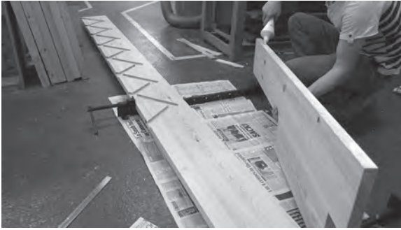
Figure 6.20 (above) and Figure 6.21 (below) With the routing of the straight step housings complete, the easements can now be glued to the wall and return strings.
