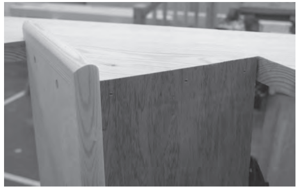
Figure 5.57 Accurately prepared mitres will result in neat-fitting risers
