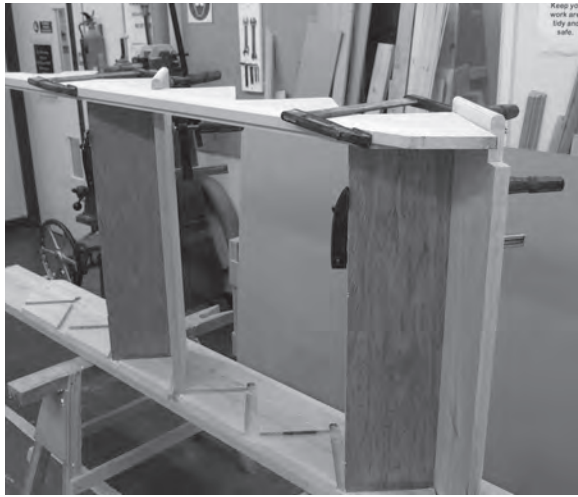
Figure 5.54 Use two further F-clamps to hold the outer string in place.
