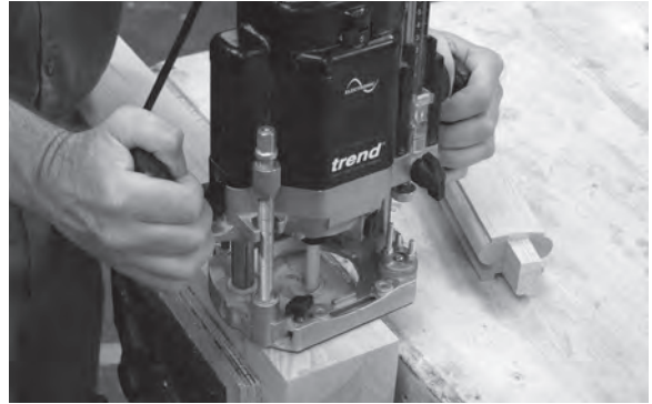
Figure 11.21 Rout out the majority of the waste to a depth of 6 mm, using the router freehand.
