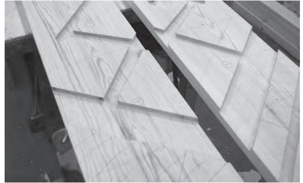
Figure 4.43 The string tenons, shown before the second shoulder is cut and prior to haunching.
