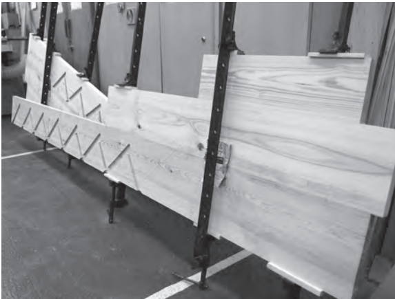
Figure 6.20 (above) and Figure 6.21 (below) With the routing of the straight step housings complete, the easements can now be glued to the wall and return strings.
