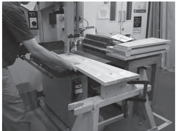
Figure 8.82 Marking the upper side of these left-handed treads means that their length – which should be supported – will extend away from the band saw's throat during cutting.
