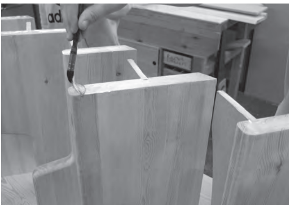
Figure 9.56 Apply PVA glue to the opposite ends of the treads and risers.
