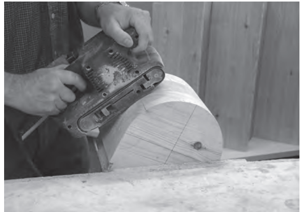
Figure 10.10 The block's semicircular surface is prepared for veneering with a belt sander.
