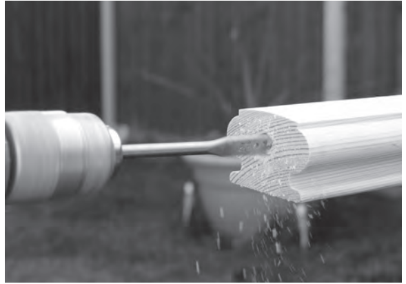
Figure 12.79 Holes, 13 mm in diameter, are drilled into the meeting ends of the handrail halves ready to receive the inserts.
