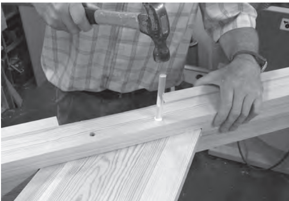
Figure 6.86 Draw-bore dowelling pulls the joint up tight.
