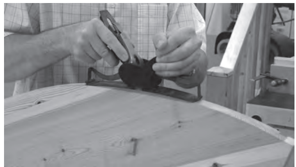
Figure 6.30 Smooth off the easing of the top edge of the return string using a compass plane.
