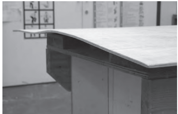
Figure 8.27 Plan to bend the flexi ply in the direction of its natural bow.
