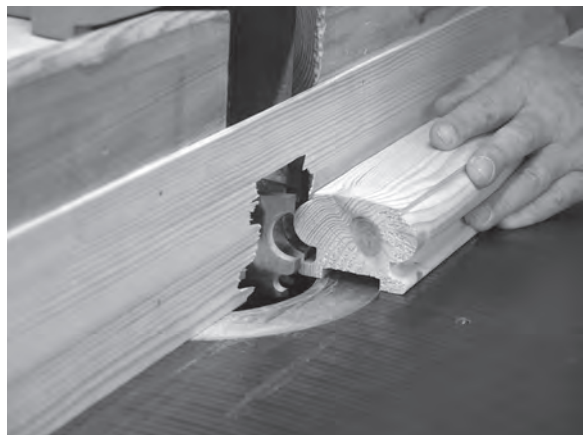
Figure 11.14 (above) and Figure 11.15 (below) The Whitehill cutters produce a classic handrail profile.
