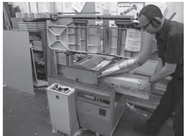
Figure 10.6 Once the glue has dried, the laminated block can be thickened to its finished height.
