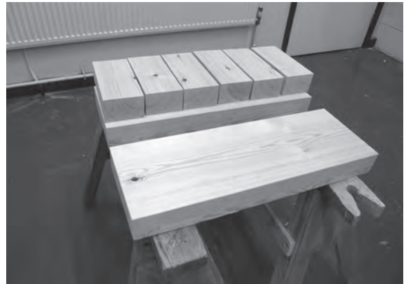
Figure 10.4 (above) and Figure 10.5 (below) A block for the step's round end is built up in alternating layers of European Redwood.
