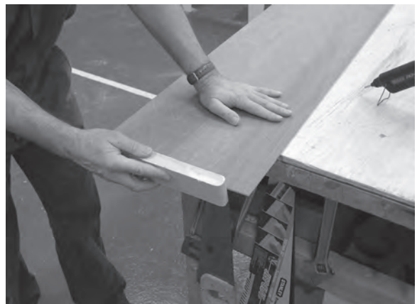
Figure 8.20 Use a sanding block to prepare the plywood for lengthening.
