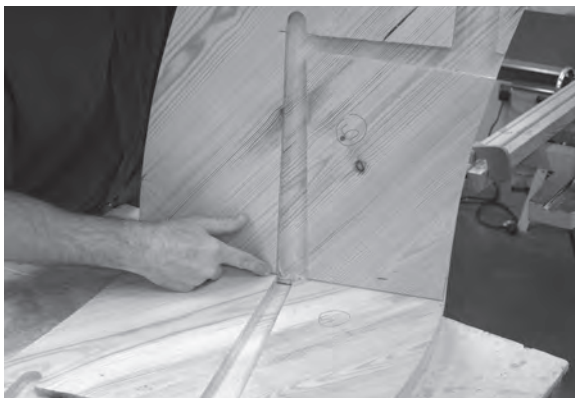
Figure 6.32 A flush fit where the housings for tread number 5 (the kite winder) meet indicates correct alignment of the two strings.
