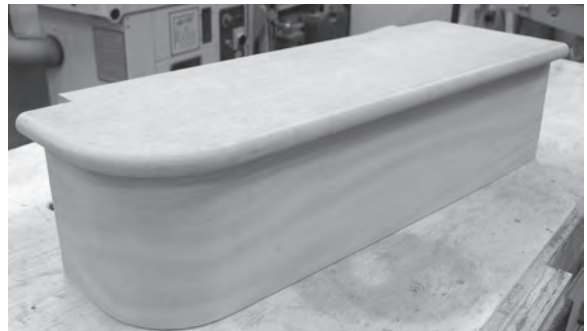
Figure 10.38 The finished bullnose starting step. Note the L-shaped notch at the left-hand rear of the tread, prepared so that the step can be housed into the bottom newel post.
