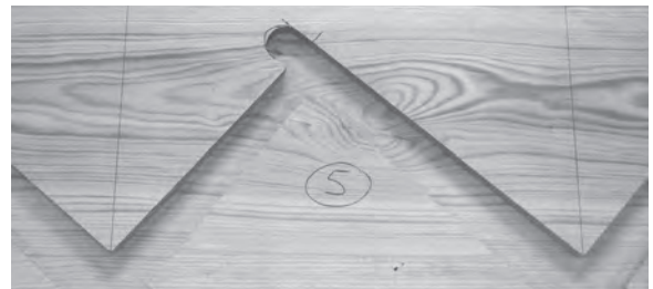
Figure 4.36 The clean, sharp corners, where the back of each tread meets the next riser, will be maintained, provided the steps are routed from left to right.
