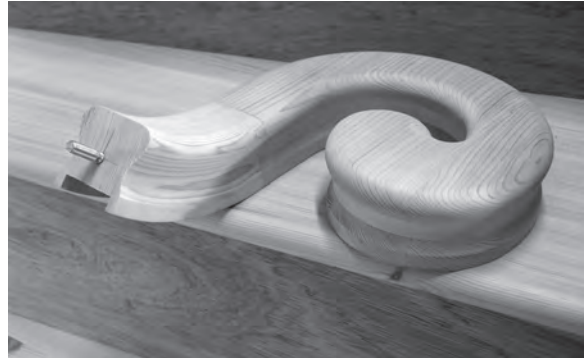
Figure 11.82 The rail bolt is screwed into the end grain of the upward easing, its position marked using a template provided with the volute.
