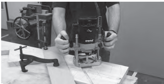
Figure 5.23 Rout the inside face of an outer cut string to produce 20 mm thick bare-faced tenons before trimming the waste to leave a tenon length equal to approximately two-thirds the newel post thickness
