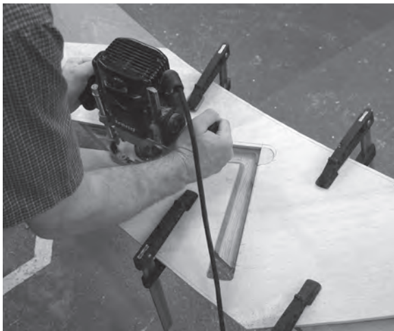
Figure 8.47 A router jig, made from an offcut of flexi ply, is firmly secured to the concave surface of the wall string.
