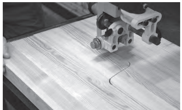
Figure 9.28 A narrow band saw is used to cut the alternating treads from the panels. Cut on the waste side of the line so that the sawn edge can be cleaned up later.
