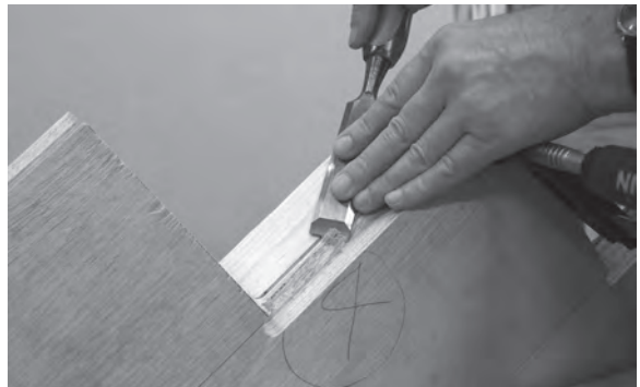
Figure 8.72 (above) and Figure 8.73 (below) Finish the mitres with a sharp chisel while protecting the face of the string with a short piece of bevelled timber.
