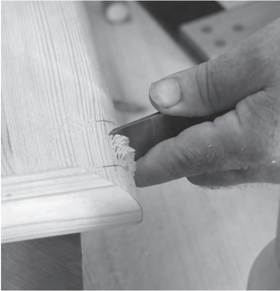
Figure 11.103 The rounded part of the tread's nosing is chopped out with a sharp chisel.
