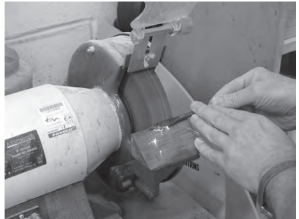
Figure 4.61 An inexpensive flat bit can, if necessary, be ground narrower to ensure a snug fit for the 12mm wooden dowel.
