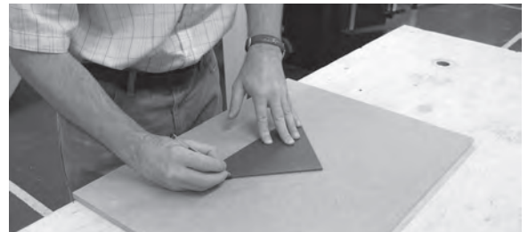
Figure 3.19 and Figure 3.20 Draw round the two shorter sides – the rise and the going – of the pitch board, after positioning centrally on the MDF.
