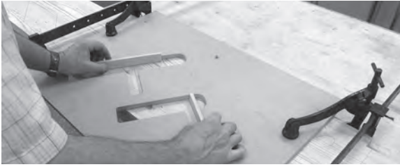
Figure 9.17 Use spacer blocks to ensure that the router jig is offset by the correct distance.
