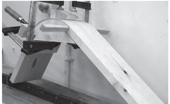
Figure 10.33 The wet riser is clamped to the laminated block, where its shape is held while it dries sufficiently for gluing.
