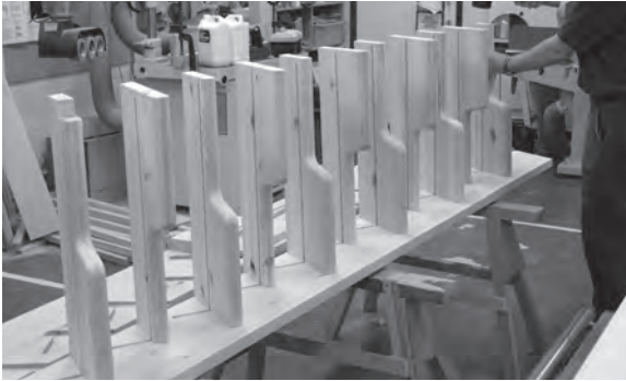
Figure 9.54 Tap the pre-numbered alternating treads into their housings.
