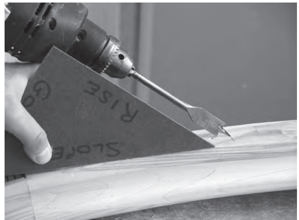
Figure 11.109 A pitch board can be used as a guide when drilling the inverted handrail on a work bench.
