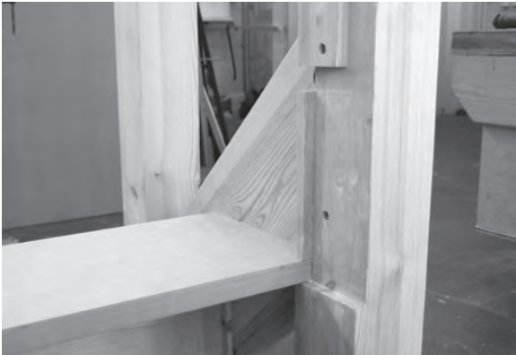
Figure 6.74 (above) and Figure 6.75 (below) The return flight is levelled and the intermediate newel post tested for fit.
