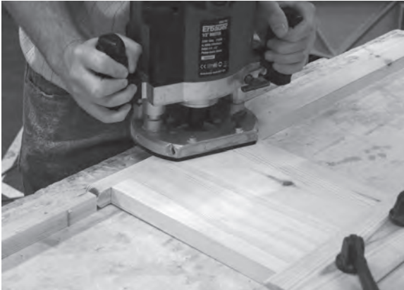
Figure 5.44 Nose the treads, taking care at the corners; here, timber offcuts butted at each end ensure a smooth and consistent cut with the router.
