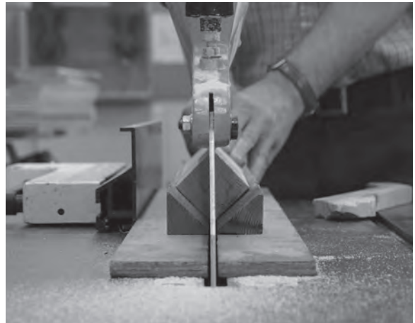
Figure 4.71 (top) and Figure 4.72 (above) Test the fit of the trial wedges before cutting the remaining wedges.
