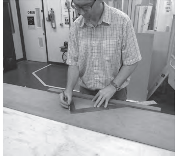
Figure 8.24 The relatively large surface area of a wooden fence, when compared to the stair gauges' points of contact, makes it more suitable for marking the thin facing plywood.
