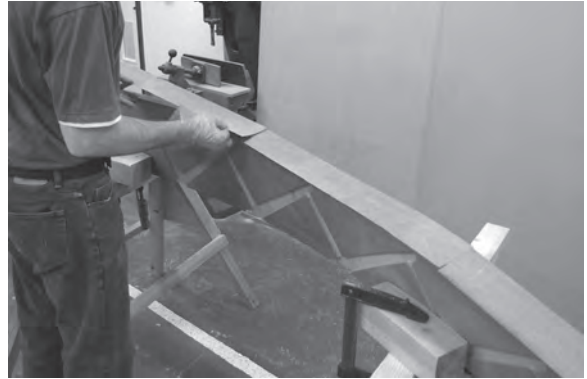
Figure 8.62 Carefully lay the over-width veneer strips onto the string's edge.
