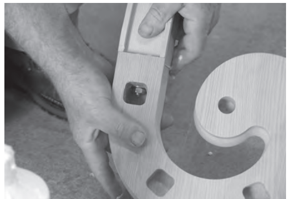
Figure 11.87 (above) and Figure 11.88 (below) The fixings are re-tightened causing glue to ooze out. The excess glue should be cleaned off with a damp cloth while still wet.
