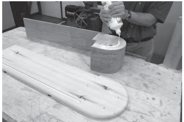
Figure 10.25 PVA adhesive is applied to the top of the laminated block and within the tread's riser housing.
