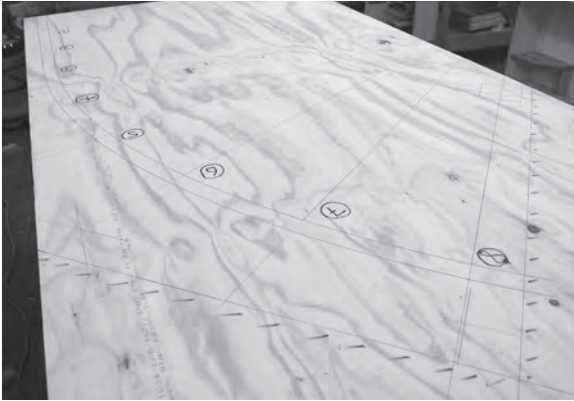
Figure 8.3 A full-size plan of the staircase can be set out on plywood, MDF, or chipboard.
