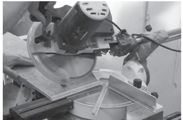
Figure 5.47 The risers are mitred at one end.
