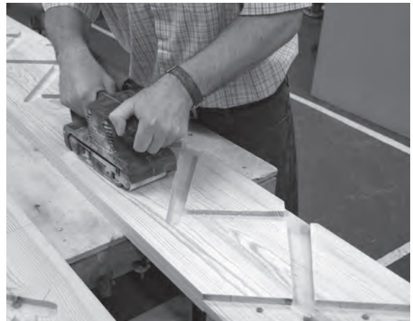
Figure 4.78 A belt sander can be used to clean up the components, although a drum sander is a far speedier option.
