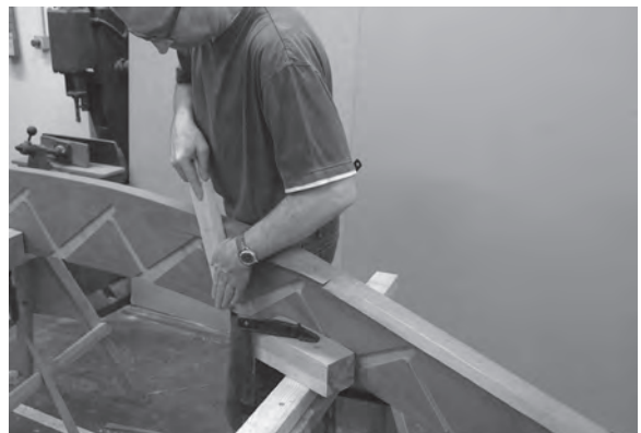
Figure 8.64 Use a sanding block to cut and remove the excess veneer.
