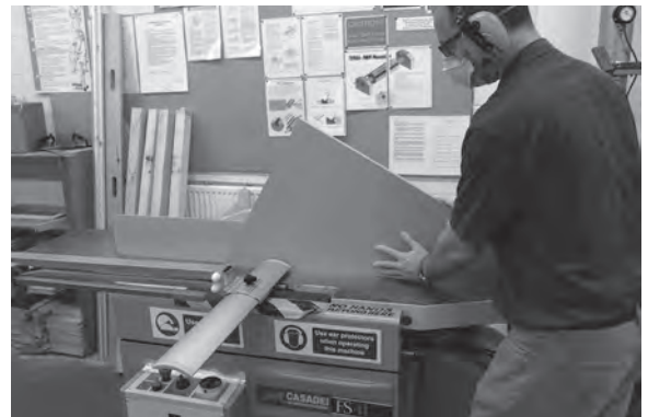
Figure 6.43 The rough sawn rear edges of the winders are skimmed over a surface planer.
