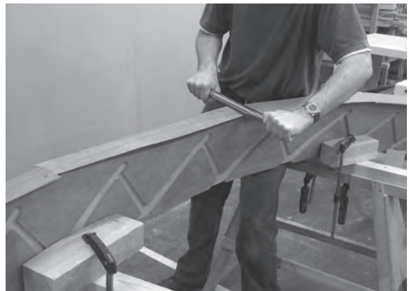
Figure 8.63 A short piece of bathroom towel rail, or similar, is ideal for applying pressure to the glued veneer.
