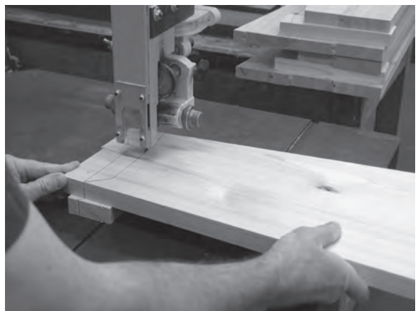
Figure 8.87 Third cut: the inside edge of the nosing return that will meet with the tread.
