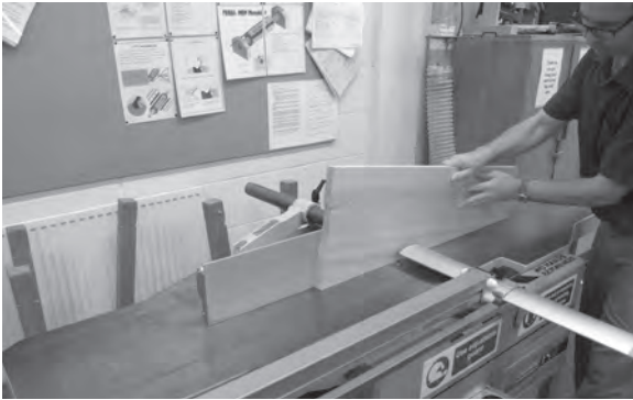
Figure 8.79 Plane smooth the treads' sawn back edges for a professional finish.
