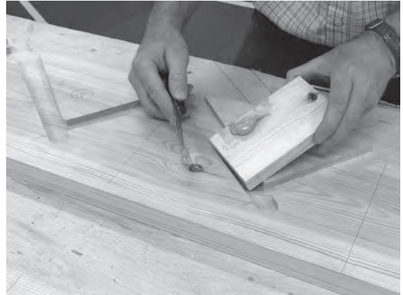
Figure 4.77 Fill any defects in the components prior to cleaning up.
