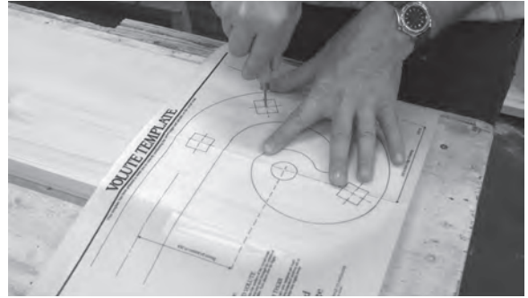
Figure 11.70 After aligning the template accurately with the balustrade centre line, the newel and baluster locations are marked with a bradawl.
