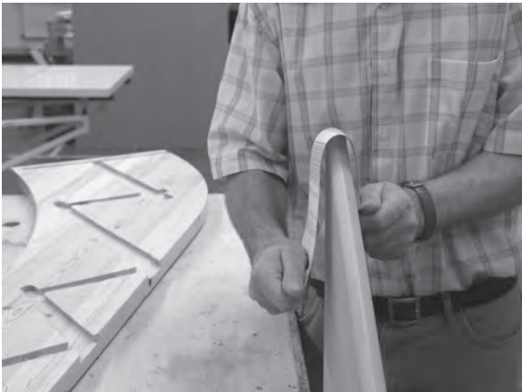
Figure 6.54 (above) and Figure 6.55 (below) Re-round the trimmed nosing so that it fits the string.
