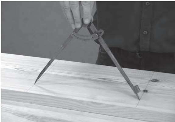
Figure 3.10 Dividers can be used to accurately space the markings for the steps on the strings.
