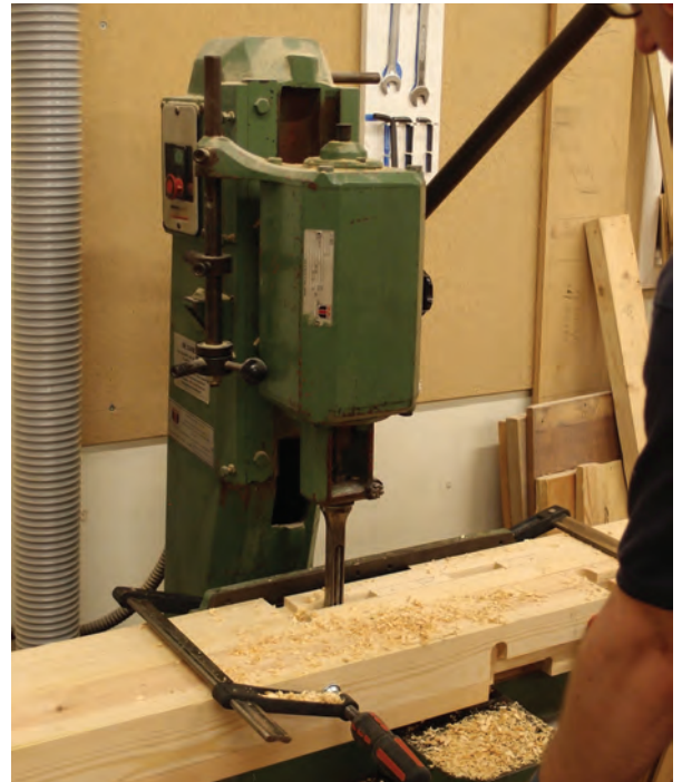
This wide intermediate newel post is being mortised ready to receive the tenons of two outer strings. The machine's clamp has been removed to accommodate the newel post which, instead, is held secure with a pair of F-clamps. See page 111.
