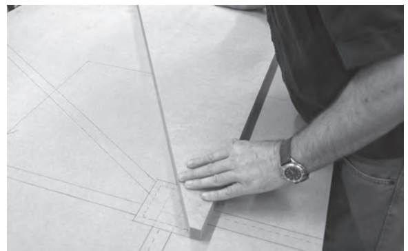
Figure 6.44 Test the angle and size of the winders on the MDF rod.
