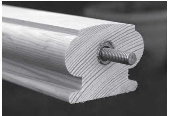
Figure 12.81 The two handrail halves are connected by a threaded bolt screwed into both inserts.
