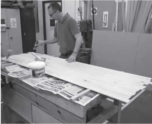
Figure 11.52 Cascamite adhesive is spread quickly and evenly on the timber strips ahead of bending and laminating
