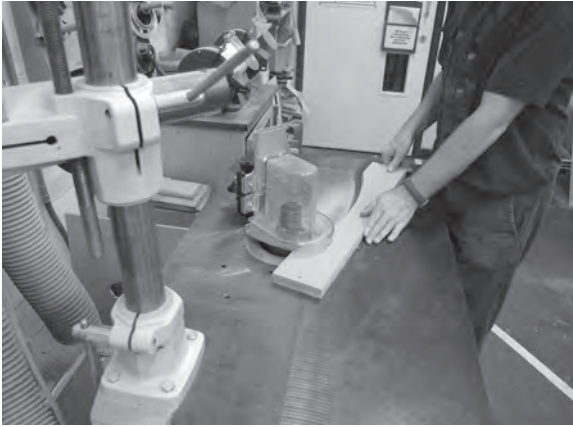
Figure 9.40 Using a spindle moulder with a ring fence, the arch of the pattern 'eyebrow' riser is reproduced time and again on the remaining 10 risers. Nailing near the ends of the jig to the over-length riser beneath will ensure that the resulting holes are lost when the risers are cut to their finished length.
