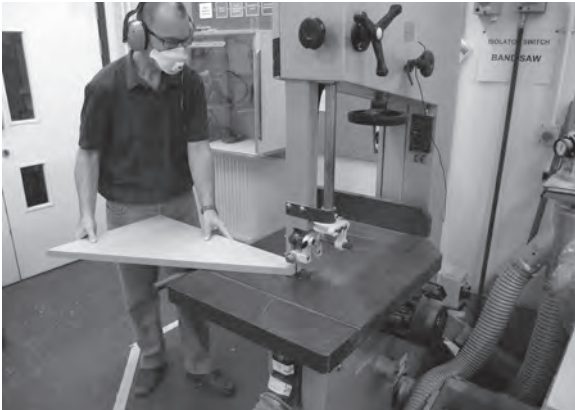
Figure 6.46 Cut the narrow end of the square winder that will be housed partly in the intermediate newel post and partly in the outer string of the return flight.
