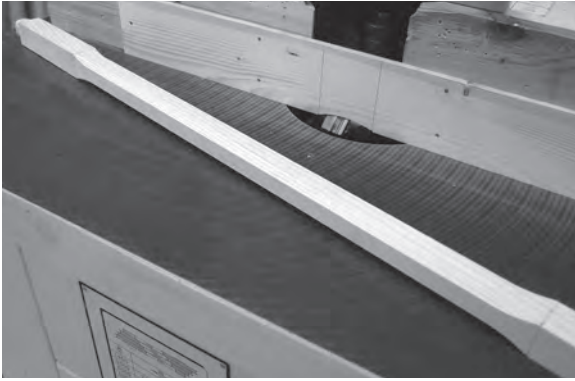
Figure 11.113 Stopped chamfers add an attractive finish to the balusters.
