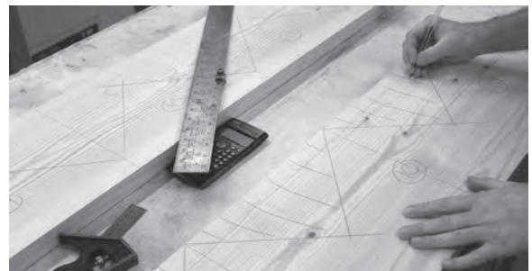
Figure 7.6 The triangular waste portions of the outer strings are shaded to indicate their removal.
