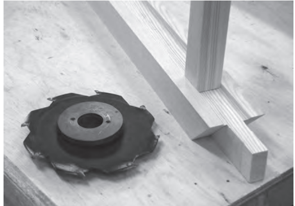
Figure 11.13 An adjustable grooving head can be used to plough a groove into the underside of the handrail, into which the balusters will be housed.
