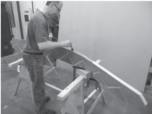
Figure 8.63 A short piece of bathroom towel rail, or similar, is ideal for applying pressure to the glued veneer.
