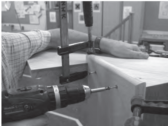
Figure 5.55 Screw through the treads into the outer string. Here a small clamp ensures good contact between the nosing return and string.
