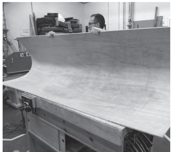
Figure 8.8 Long grain flexi ply will be used for the shorter, open string.
