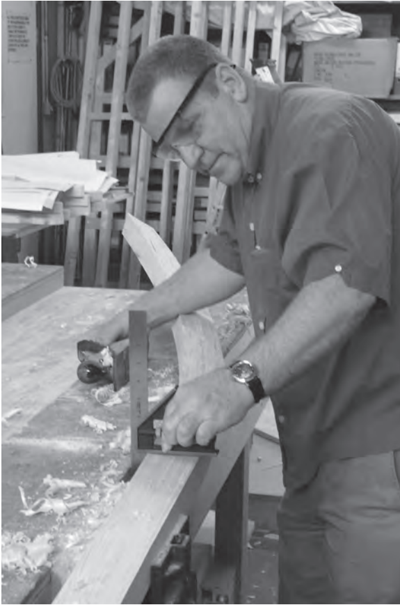
Figure 11.57 Steve pauses to check for squareness while cleaning up the handrail's glued surfaces.
