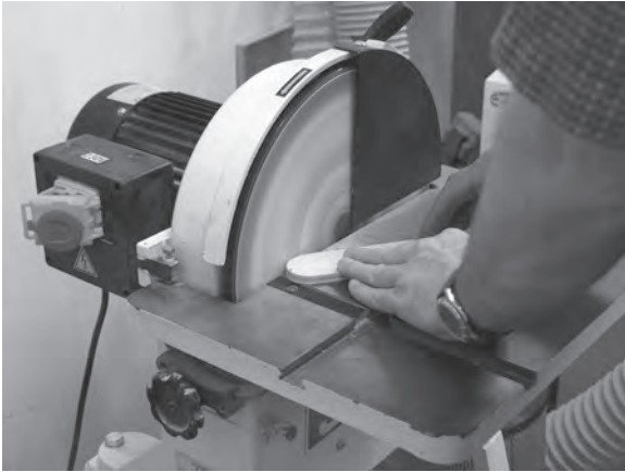
Figure 3.36c Neatly round the nosing, either by hand or mechanically.
