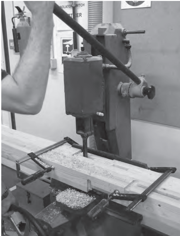
Figure 7.10 The wide intermediate newel post is held against the mortiser's fence with two F-clamps.
