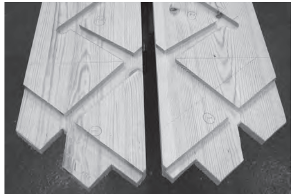
Figure 4.45 The string tenons, cut to form pairs and haunched.
