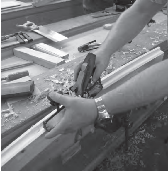
Figure 11.69 The handrail's sides are diminished to match those of the volute using a compass plane.
