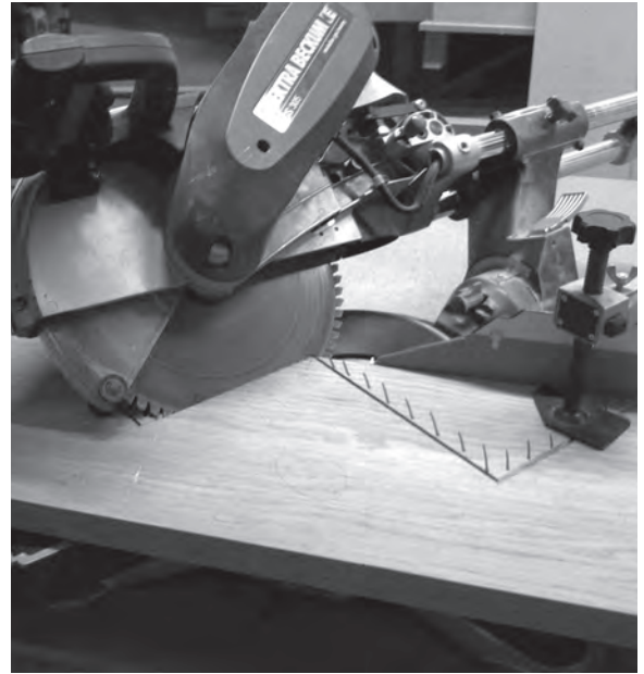
Figure 10.41 The mitred riser lines are cut using a chop saw. (Photo courtesy of Frank Turtle)
