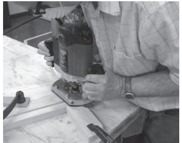
Figure 8.96 (above) and Figure 8.97 (below) When nosing the treads, prevent the 'dropping in' of the router cutter at the corners by abutting offcuts each side of the tread.
