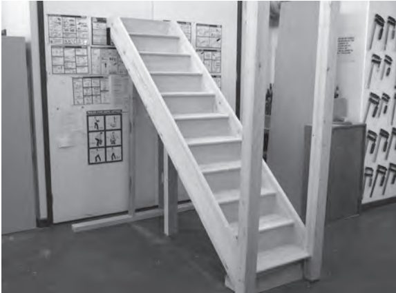
Figure 4.94 The finished staircase with newel posts test-fitted before delivery to the customer.
