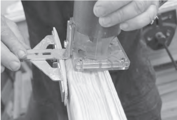
Figure 11.66 A small palm router with curved fence reaches parts that a larger router cannot.
