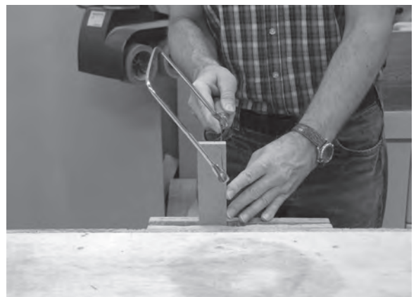
Figure 3.36b Use a coping saw to cut roughly to the shape of the nosing
