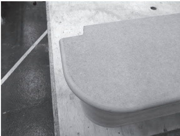
Figure 6.70 Ease the rear corner of the bullnose tread to permit entry into the newel post housing.
