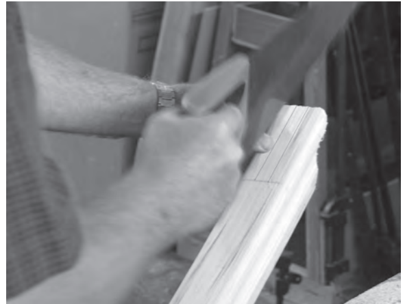
Figure 11.95 The tenon cheeks are cut with a handsaw.
