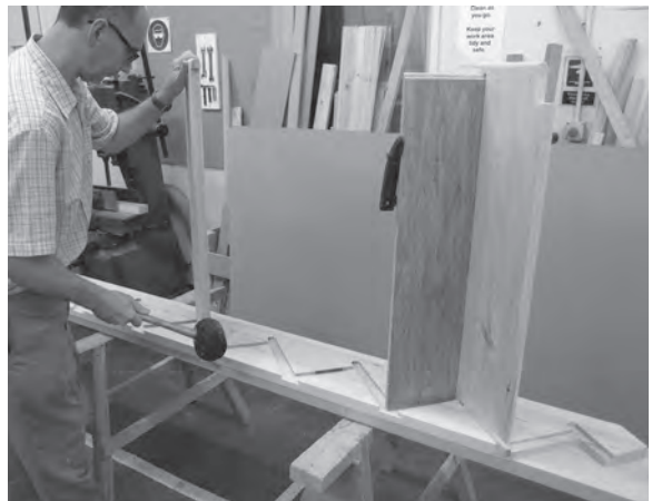
Figure 5.49 Commence assembly by locating two steps within their free-of-dust wall-string housings. The steps selected will be at opposite ends of the facing outer (cut and mitred) string.
