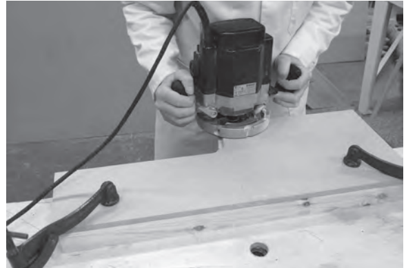
Figure 9.34 The treads' front edges are cleaned up with a 12 mm straight fluted cutter. Rout from left to right starting with the wide side of the tread.
