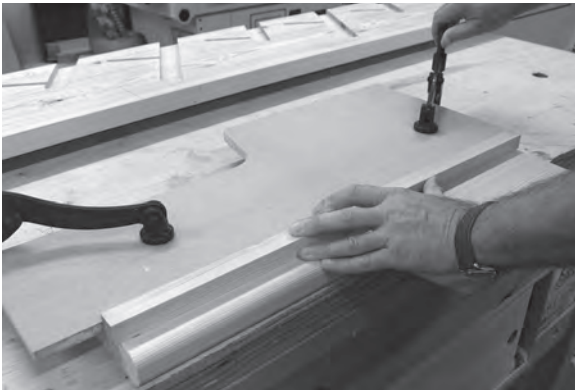
Figure 9.44 With a straight edge clamped to the underside of a tread, the routing of the riser housings can commence. Here a spacer block is used to accurately offset the straight edge by the correct distance.
