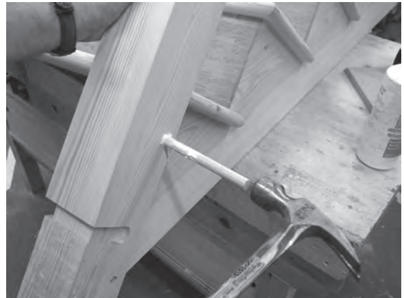
Figure 5.69 Glued dowels are used to pull the joint up nicely.
