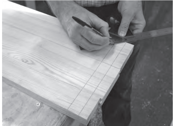
Figure 5.28 The shape of a nosing return is marked on the treads at the ends that meet with an outer (cut) string.
