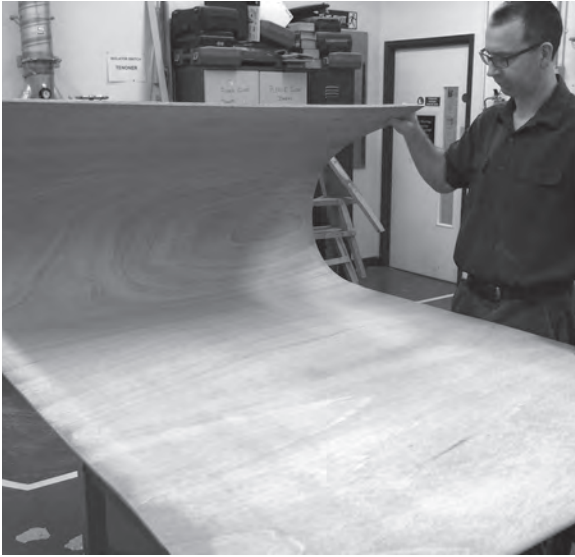
Figure 8.9 Cross grain flexi ply will be used for the longer, wall string.
