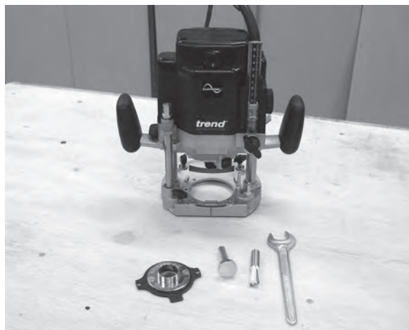
Figure 3.1 Electric router with accessories, from left to right: 30 mm guide bush with inner plate, guide bush line up pin, 16 mm stair housing dovetail cutter, and 22 mm spanner.
