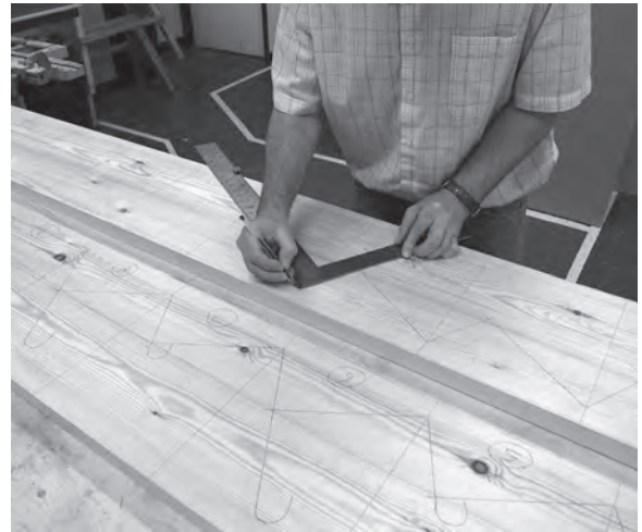
Figure 9.11 Marking the steps on the strings using a pair of stair gauges clamped to a steel roofing square.
