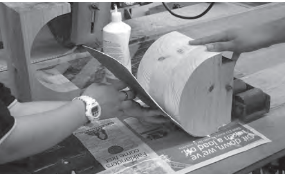
Figure 10.17 A D-step's smaller projection requires no straight return to the newel post.
