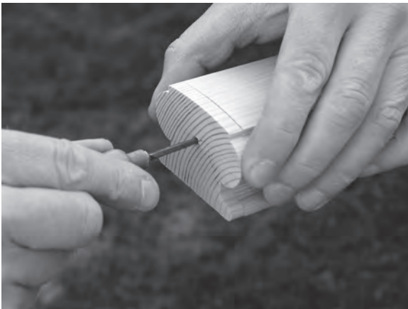
Figure 12.78 The template and a bradawl are used to mark the insert centres on the two handrail halves.
