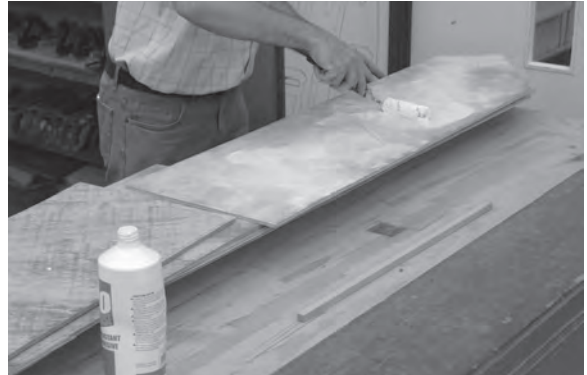
Figure 8.35 PVA glue dries quickly, especially in warm weather – so work quickly!
