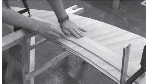
Figure 8.44 Use a straight-edge to mark the waste part of the string.
