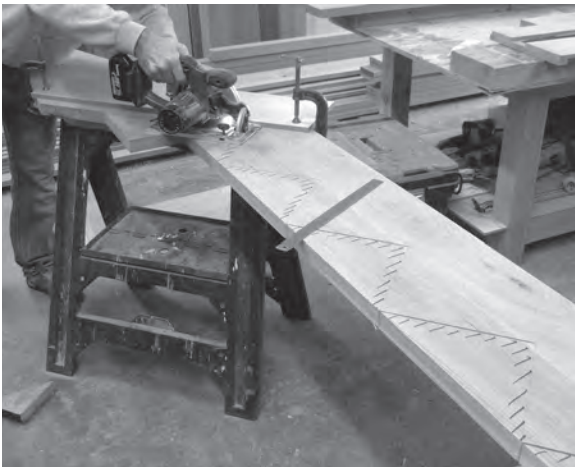
Figure 10.40 The tread lines are cut with a hand-held circular saw guided by a straight edge.
