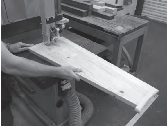
Figure 8.98 Use the template to mark the treads' length, and cut on the band saw.
