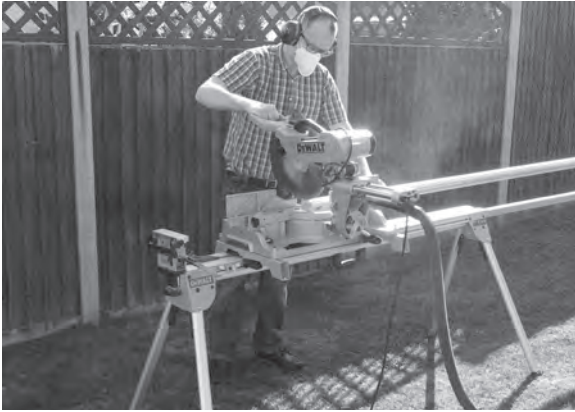
Figure 12.76 (above) and Figure 12.77 (below) Trim a thin handrail offcut for use as a template for marking the insert locations.
