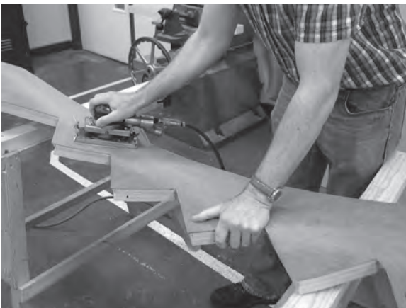
Figure 8.103 Clean up all components prior to assembly.
