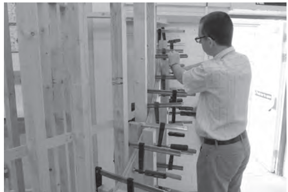
Figure 8.37 During clamping, ease the flexi ply round the form to maintain the string's sweeping curve.
