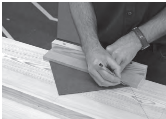
Figure 3.3 A pitch board and margin template in use.
