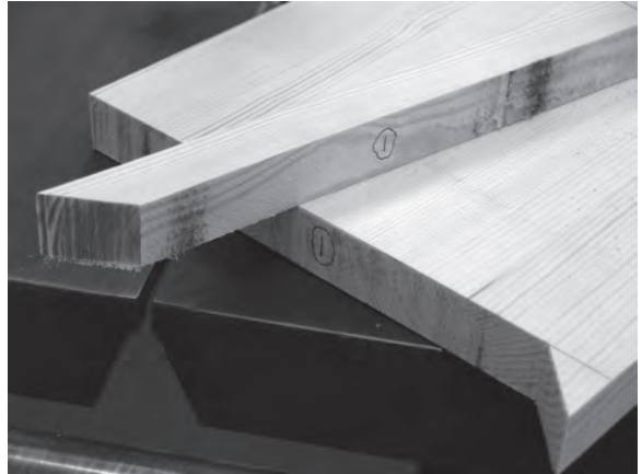
Figure 5.38 Number the treads and nosing returns for matching up later.
