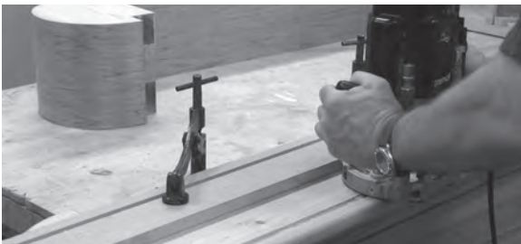
Figure 10.22 Running off a straight edge, the riser housing is routed into the underside of the tread; the round end is not grooved.
