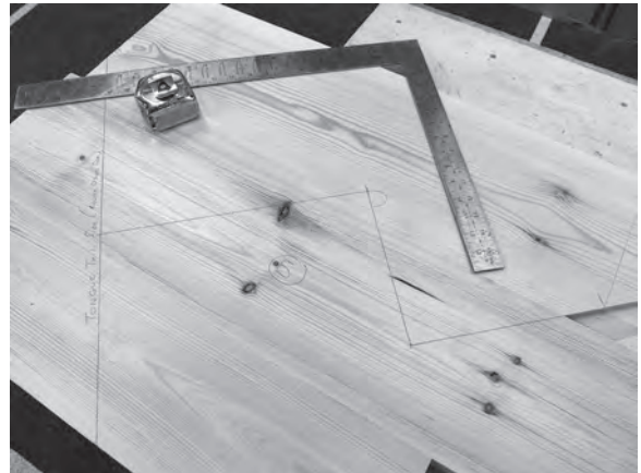
Figure 6.22 (above), Figure 6.23 (below), and Figure 6.24 (bottom) After cleaning off the dried glue, the marking of the wall and return strings is completed by using a steel roofing square to add the winding steps and the tongued housing joint that will connect the two strings.
