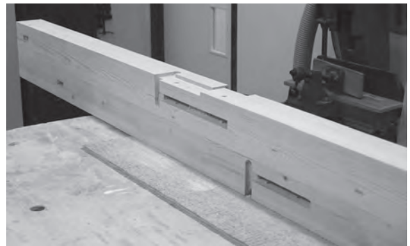
Figure 7.11, Figure 7.12, Figure 7.13, Figure 7.14 The four sides of the finished intermediate newel post.
