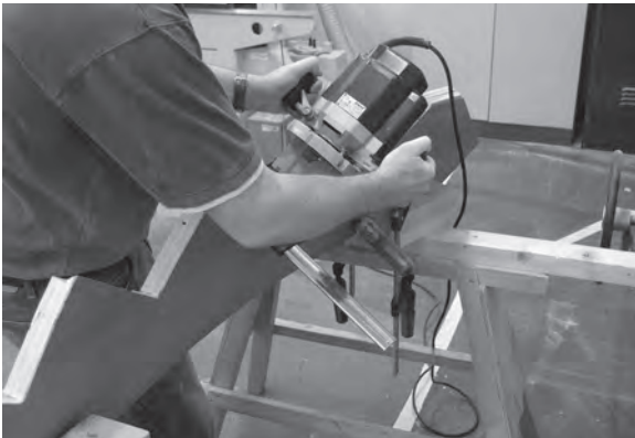
Figure 8.70 (above) and Figure 8.71 (below) A bearing-guided chamfer cutter can be used to rout the majority of the waste when mitring the open string.
