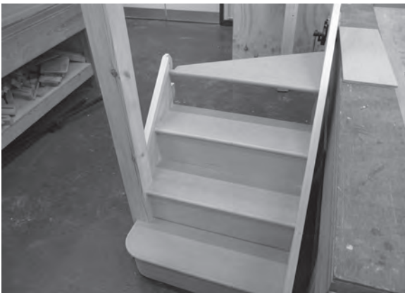
Figure 6.76 (above) and Figure 6.77 (top right) The intermediate newel post is temporarily removed to allow access for tread number 4 – the square winder.
