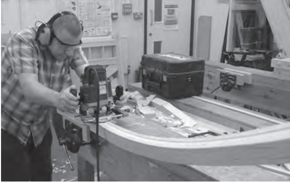
Figure 11.65 With the handrail secured, Steve begins the task of shaping the rail to match that of the Richard Burbidge volute.
