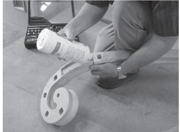
Figure 11.86 The nuts securing the assembly are loosened, and glue is squeezed into the joins.
