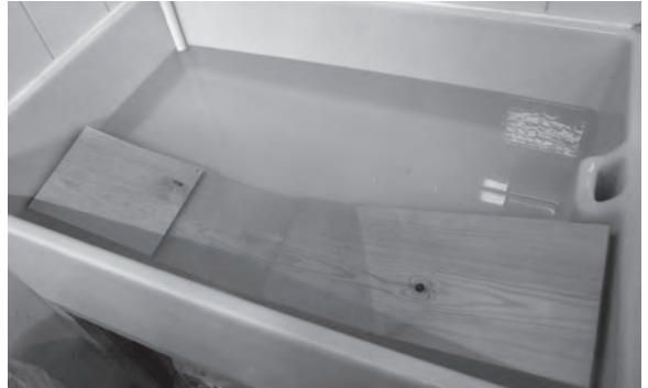
Figure 10.32 Submerging the European Redwood riser in water for 24 hours makes the diminished thickness section pliable enough to bend round the laminated block.
