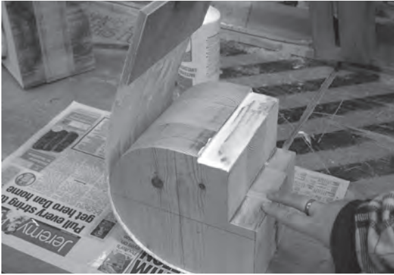
Figure 10.15 The diminished section of the plywood riser is wrapped around the semicircular block, leaving a short straight section which will return to the string.
