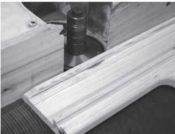
Figure 9.49 Converting the top tread into a landing nosing. Having trenched the underside of the tread with a rebate block in a spindle moulder, the remaining waste is removed using a thin saw blade. Here, the guard has been removed for clarity.
