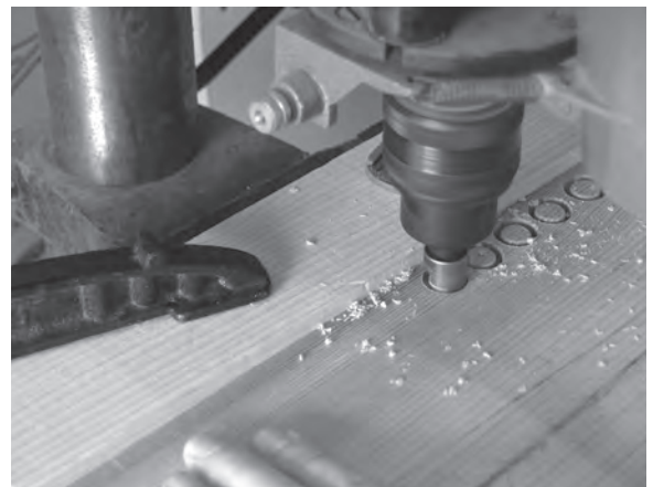
Figure 9.50 Cut pellets from a scrap piece of softwood.
