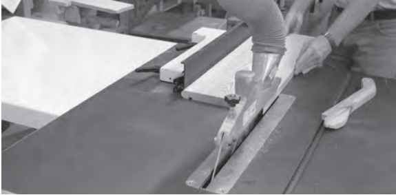
Figure 4.54 Cut the treads to width slightly proud of the mark.
