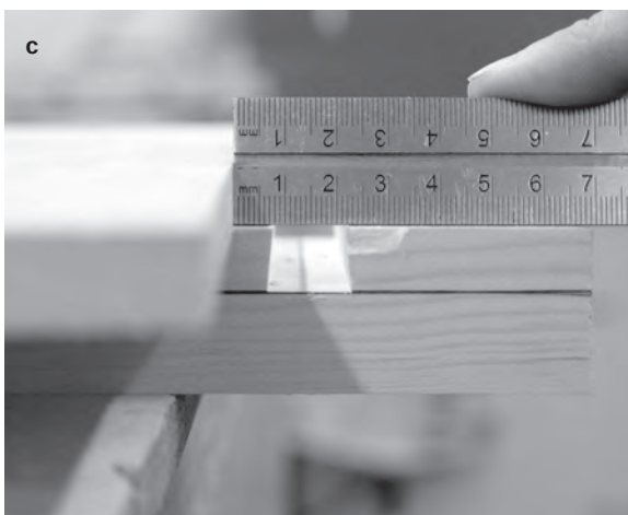
Figure 3.18a, b, c Cutting a groove using an electric router and straight edge in order to determine the 'cutter offset distance'.
