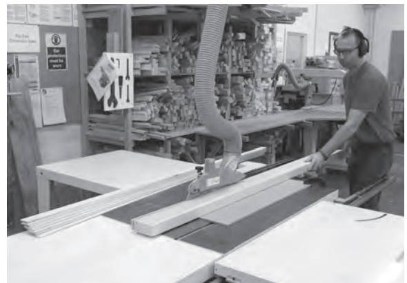
Figure 11.51 European Redwood, planed to the handrail's finished thickness, is ripped down into 5 mm thick strips.
