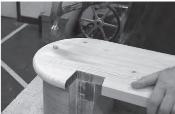
Figure 10.28 The D-step's screws are concealed beneath wooden pellets. Note the notches in both the tread and laminated block's rear where the step will be housed into the newel post.
