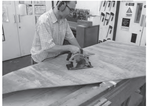
Figure 8.31 Use a hand-held circular saw to cut the flexi ply to width, taking care not to damage the work bench below.
