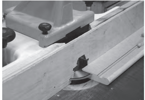
Figure 6.61 The marked portion of the landing nosing is removed using a thin saw blade in a spindle moulder. Here, the guard has been removed for clarity.
