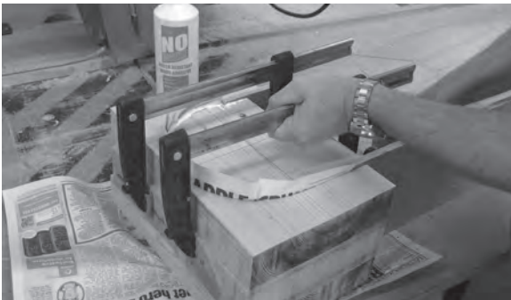
Figure 10.16 The offcut, preserved after band sawing earlier, is now used to distribute pressure from clamps. Newspaper will prevent the outside of the plywood veneer from sticking to the timber offcut.
