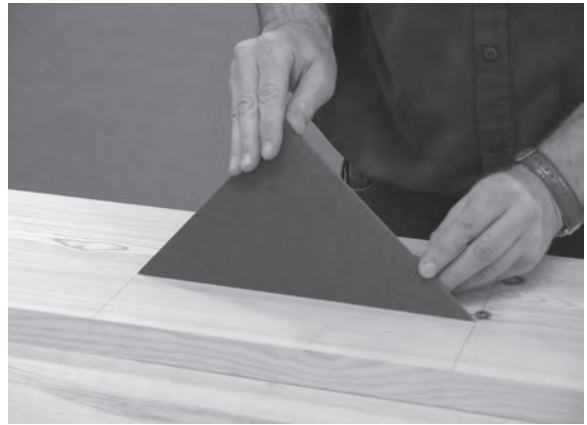
Figure 4.22 Your pitch board can be used to speedily check the marks for accuracy.
