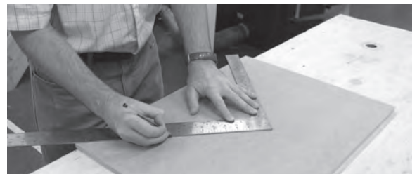
Figure 3.21 Use a steel roofing square to extend the tread and riser lines.
