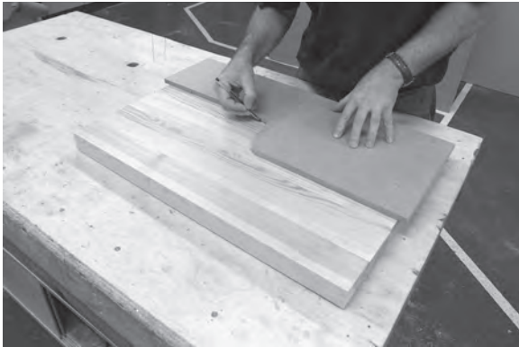
Figure 9.30 Use a template made from 12 mm MDF to mark the alternating treads.
