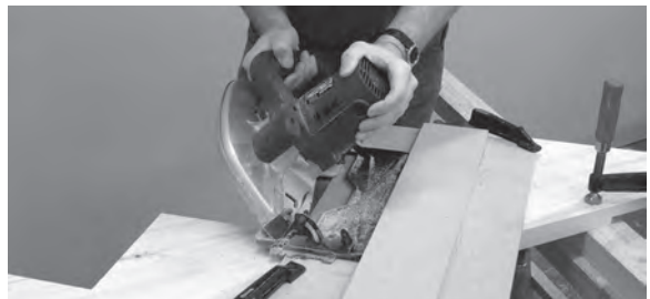
Figure 5.19 (above) and Figure 5.21 (below) The base of the hand-held circular saw is tilted to an angle of 45° and the mitres cut. Here I'm using an MDF fence for accuracy.
