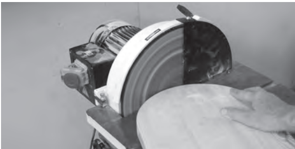
Figure 10.20 (above) and Figure 10.21 (below) The tread's rough-sawn round end is cleaned up using a disc sander before the nosing is applied.
