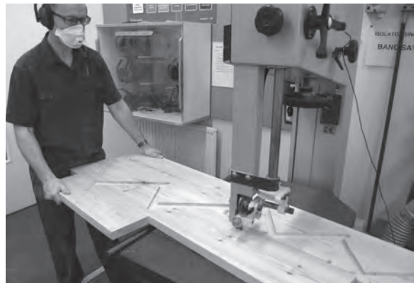
Figure 6.29 A band saw is used to cut the easings of the return string.
