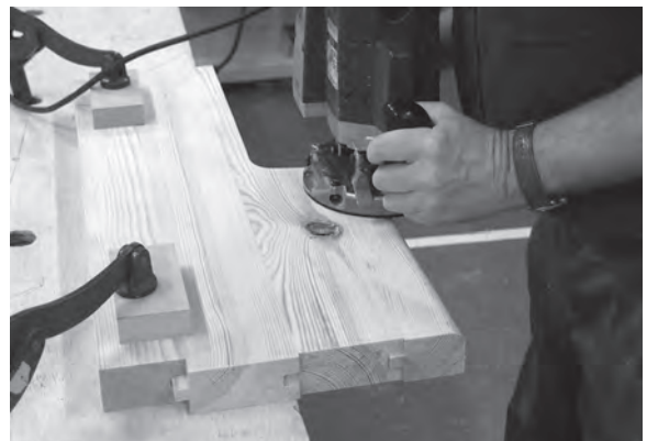
Figure 9.36 Cut the nosings with a bearing-guided round over cutter with a radius of 12.7 mm.
