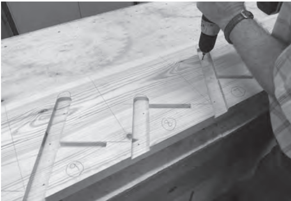
Figure 9.52 Drill through the tread housings to ensure that the screw holes are correctly located.
