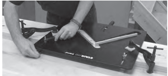
Figure 4.30 Trend's aluminium fence is secured by reversible barrel nuts, which permit quick switching of the jig from one string to the opposite string during use.
