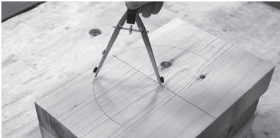
Figure 10.7 The round end is marked onto the laminated block with a compass.
