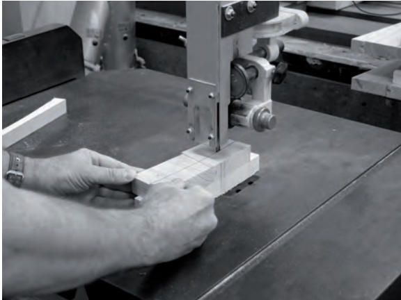
Figure 8.88 Fourth cut: the outside edge of the nosing return.
