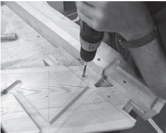
Figure 4.64 Drill holes through the tenons approximately 2–3mm closer to the shoulder.
