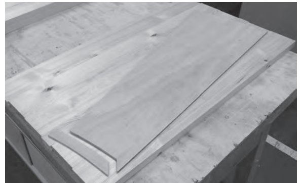
Figure 8.76 This thin plywood template is ideal for maintaining consistency when marking the treads; it comprises two parts: the main tread and the nosing return.
