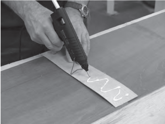
Figure 8.21 (above) and Figure 8.22 (below) The butt joint used to lengthen the facing plywood is supported by a thin, glued-on, plywood plate which is weighted while the glue dries.
