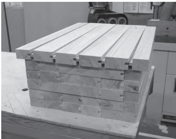
Figure 9.27 Twelve paddle-shaped treads will be cut from six tongued and grooved softwood panels.
