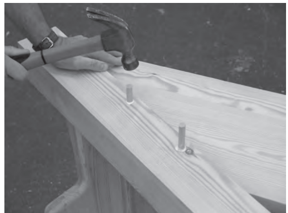
Figure 9.68 Drive glued wooden dowel through the offset holes to pull the tenon shoulder up tight.
