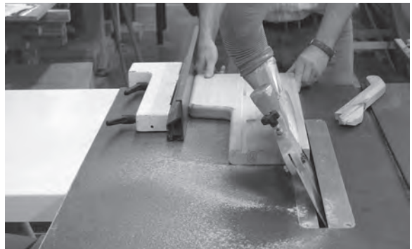
Figure 9.44 With a straight edge clamped to the underside of a tread, the routing of the riser housings can commence. Here a spacer block is used to accurately offset the straight edge by the correct distance.
