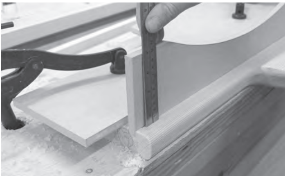
Figure 9.45 Check the fit of a riser in the first housing routed before proceeding further.
