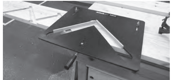
Figure 4.35 Trend's jig is secured during use by its built-in front clamp.
