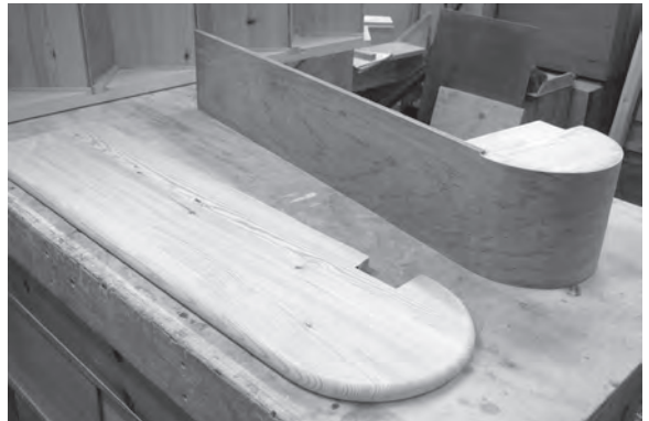
Figure 10.24 The D-step, with its notched rear for housing into the newel post, is ready for final assembly.
