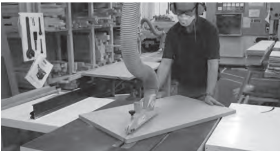
Figure 6.42 The MDF panel is cut diagonally to produce the square and skew winding treads.
