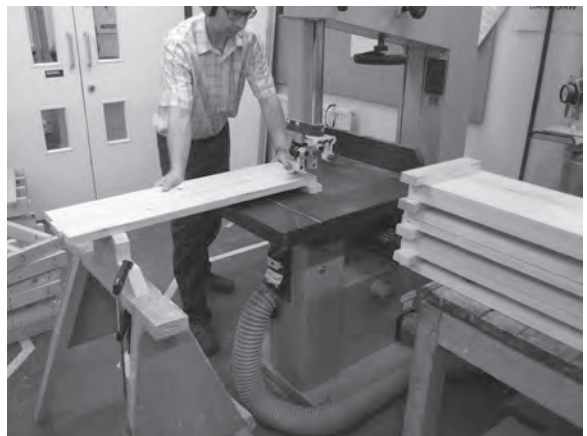
Figure 5.29 Arrange the marking and nailing of the nosing returns so that the treads extend away from the band saw's throat. Provide support to the treads during cutting.
