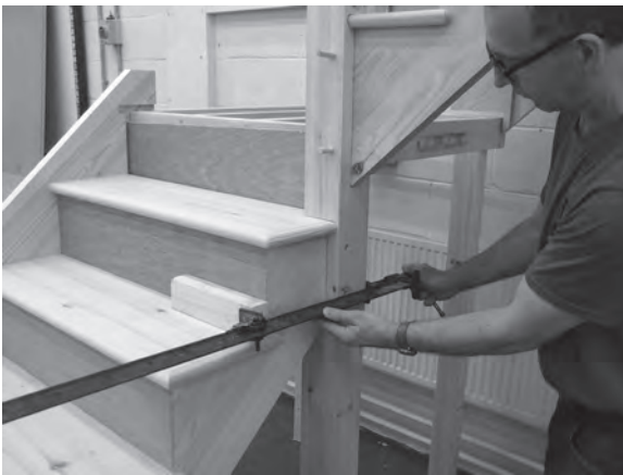
Figure 5.84 A cut string provides an opportunity for clamping not possible on closed strings.
