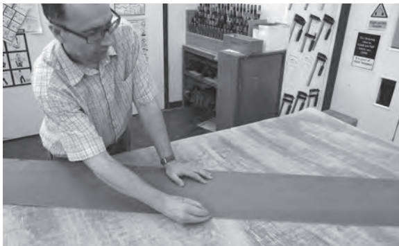
Figure 8.30 The flexi ply is best marked using the facing plywood to draw a diagonal line equal to the stairs' angle of pitch followed by repeated parallel lines.
