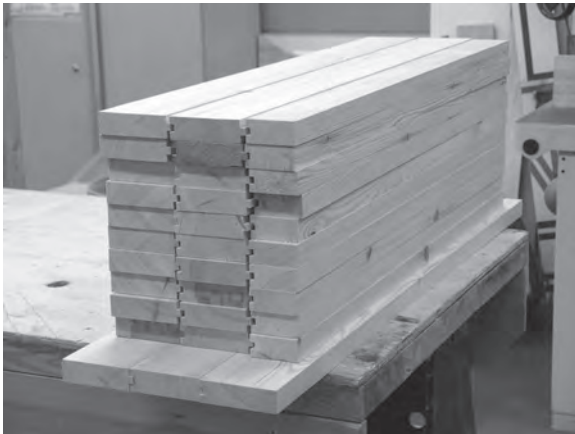
Figure 5.8 Making each tread from three relatively narrow pieces will help to avoid cupping.
