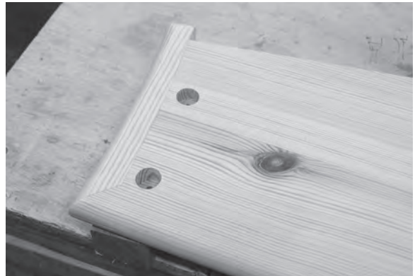
Figure 8.100 (above) and Figure 8.101 (below) The 18 mm diameter holes drilled to a depth of 18 mm will house future baluster dowels, and 6 mm diameter holes drilled through the remainder of the treads' thickness are screw clearance holes.
