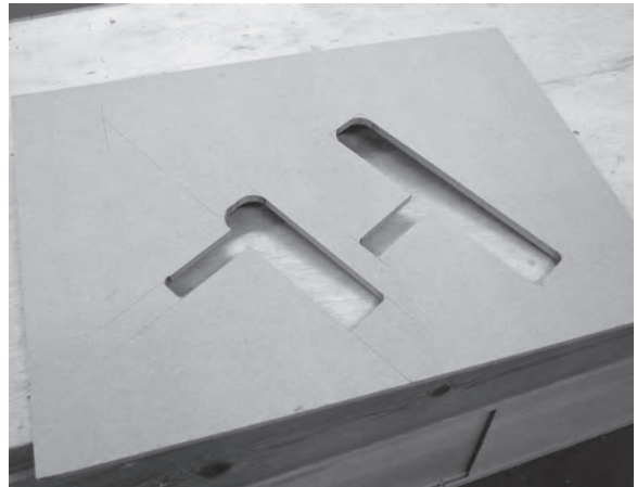
Figure 9.9 A carefully prepared router jig will permit the routing of both the wide and narrow sides of the alternate treads.
