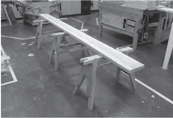
Figure 4.79 The first of a pair of 50mm thick protective boards is laid on top of three evenly spaced trestles.
