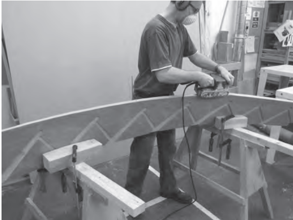
Figure 8.59 Prepare the string edges to be veneered with a belt sander.
