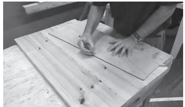
Figure 8.77 Use the main part of the template to mark the treads' angle of taper on each of the panels.
