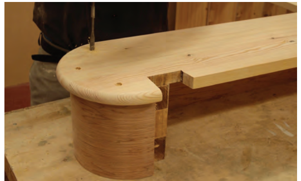
Above: In preparation for concealing the screws that will fix this round-end tread to the solid block below, holes for pellets are drilled with a 12 mm flat bit. The rear of the assembly has been notched for housing into the bottom newel post. See page 178.
