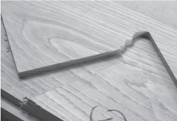
Figure 10.50 (above) and Figure 10.51 (below) Tread and riser housings routed into the wall strings include an allowance for the scotia mouldings.
