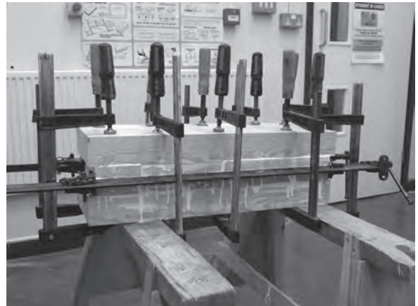
Figure 10.4 (above) and Figure 10.5 (below) A block for the step's round end is built up in alternating layers of European Redwood.
