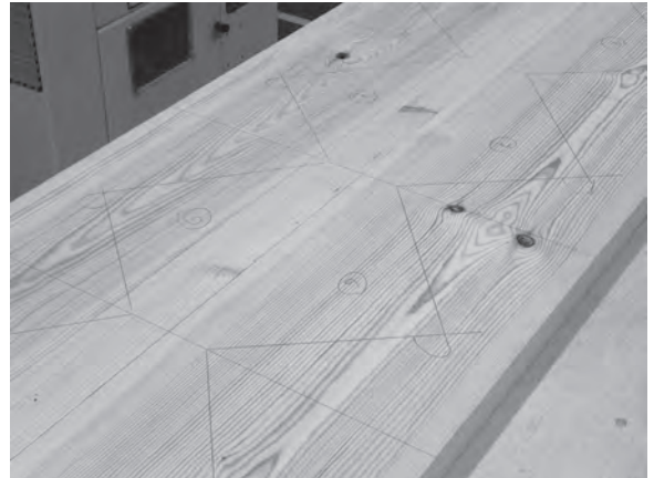
Figure 4.26 The steps are numbered and the nosing positions indicated.
