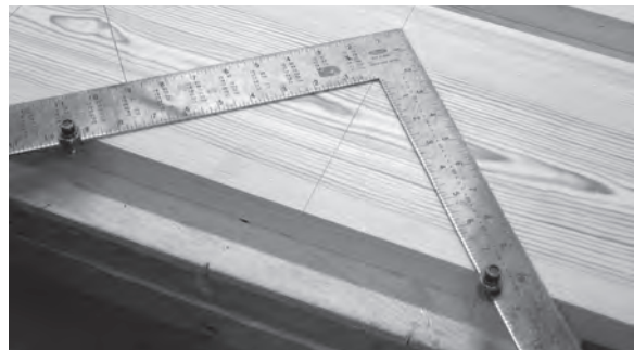
Figure 3.8 A pair of brass stair gauges clamped to a steel roofing square makes a good alternative to a pitch board and margin template.
