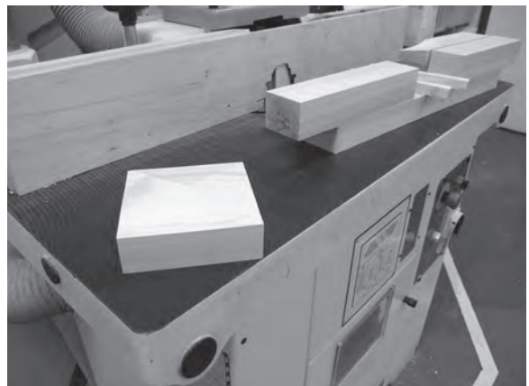
Figure 10.70 The completion of the pyramid is the end of the first spindle operation.
