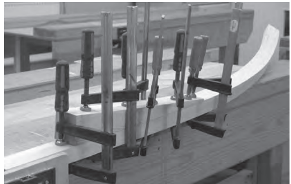
Figure 11.60 The change in going between the straight and tapered treads requires a kinked handrail, achieved by gluing a solid block to the rail's upper surface. The clamp at the front prevents the wedge-shaped block from sliding forwards on the wet glue.
