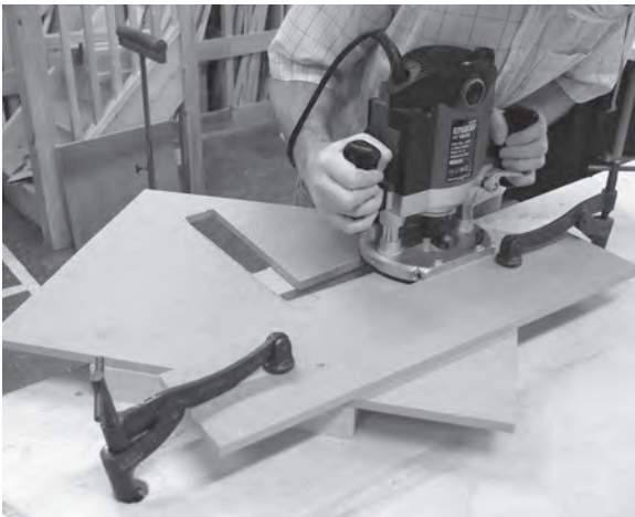
Figure 3.31 With a straight edge for guidance, rout neatly to your marked lines.
