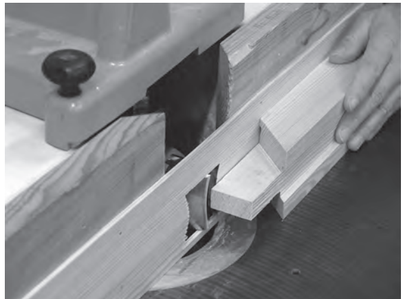
Figure 11.14 (above) and Figure 11.15 (below) The Whitehill cutters produce a classic handrail profile.
