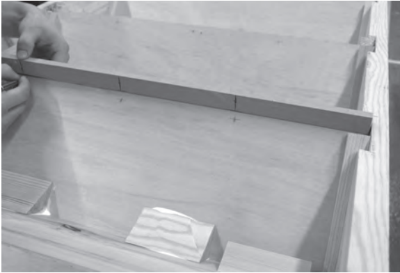
Figure 4.89 Screw positions are marked using a template for a uniform appearance.
