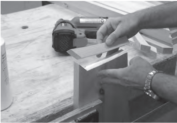
Figure 8.94 Line up the corresponding nosing return and bring the two components together.
