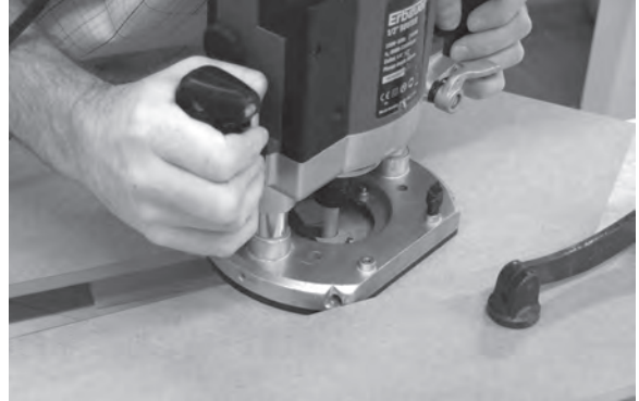
Figure 3.32 Freehand routing of the nosing. Gradually skim the MDF as you work towards the marked line in a gentle circular motion. Tip: Leave the straight edge in place, it will ensure that your nosing finishes flush with the line of the tread.
