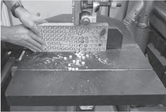
Figure 9.51 A band saw enables rapid removal of pellets from the scrap piece of softwood.
