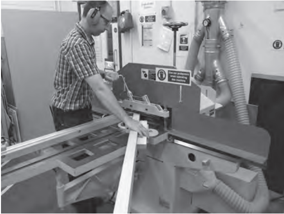
Figure 11.11 (above) and Figure 11.12 (below) Tenons can be cut either by hand or, as seen here, on a tenoning machine.
