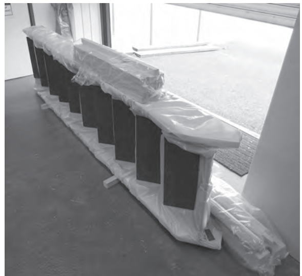
Figure 4.97 The staircase and loose components are protected and ready for delivery.
