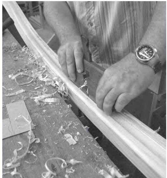
Figure 11.68 A curved-based wooden moulding plane with rounded fluting cutter is used to smooth out the handrail's outer, or concave side.
