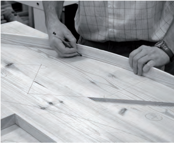
Figure 6.25 (above), Figure 6.26 (below), and Figure 6.27 (bottom) Use your preferred method for marking the string easings.
