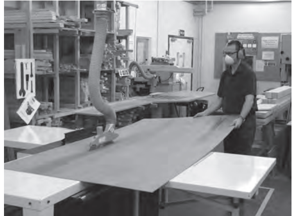
Figure 8.19 Plywood, which will form the faces of the strings, is ripped to width.
