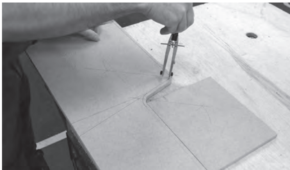
Figure 9.33 Geometry is used to mark the template prior to trimming the front edge so that it can be used as a jig.
