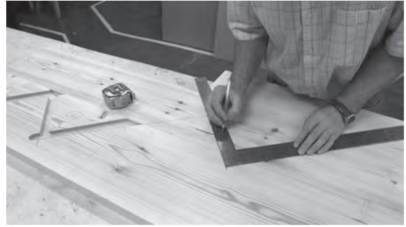
Figure 6.22 (above), Figure 6.23 (below), and Figure 6.24 (bottom) After cleaning off the dried glue, the marking of the wall and return strings is completed by using a steel roofing square to add the winding steps and the tongued housing joint that will connect the two strings.
