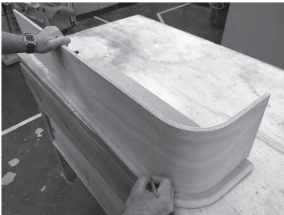
Figure 10.35 The underside of the bullnose tread is marked to house only the straight section of the riser.
