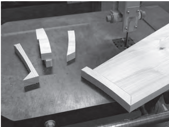
Figure 8.91 Ahead of fixing the nosing returns, form the riser housings by grooving the underside of the treads.
