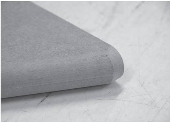
Figure 6.54 (above) and Figure 6.55 (below) Re-round the trimmed nosing so that it fits the string.
