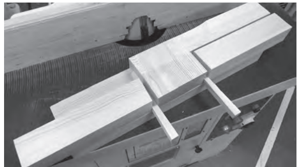
Figure 10.69 After cutting across the grain, two of the four passes required to form the pyramid are complete.
