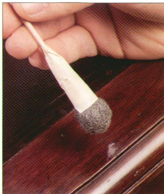
A wad of fine steel wool wrapped around the end of a dowel rubs a stain out of a tabletop. Using the dowel concentrates the abrasive action on the blemish, minimizing damage to the surrounding finish.
