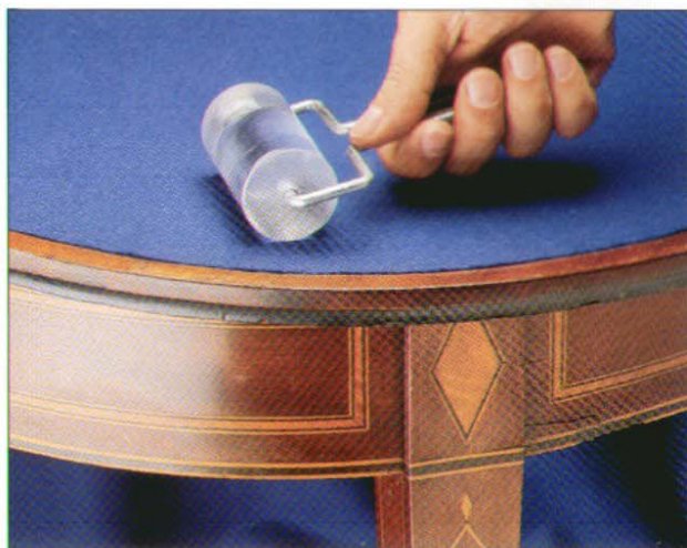
A covering of wool/rayon felt is pressed onto the playing surface of the gateleg card table shown above, rejuvenating the worn tabletop. Once a layer of fabric glue is spread on the surface, the felt is set in position and smoothed into place with a veneer roller.
