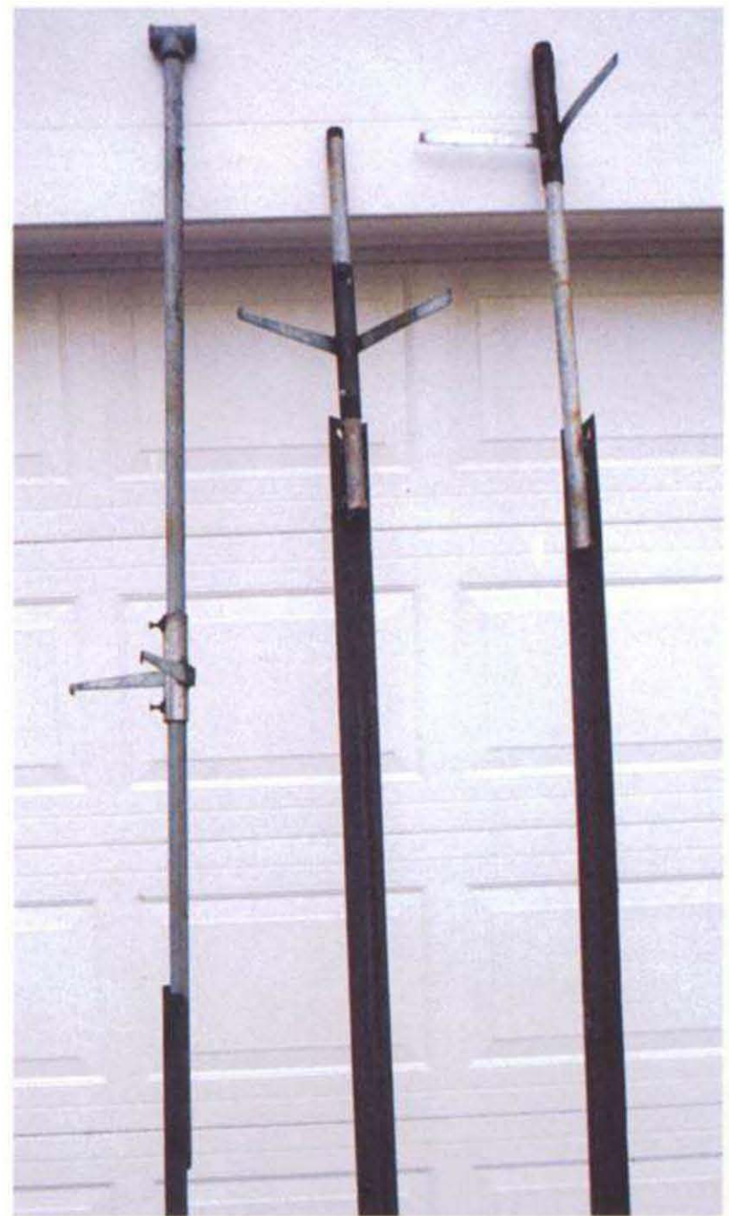
A simple tool for holding layout strings at foundation corners can be made from common steel stock.
