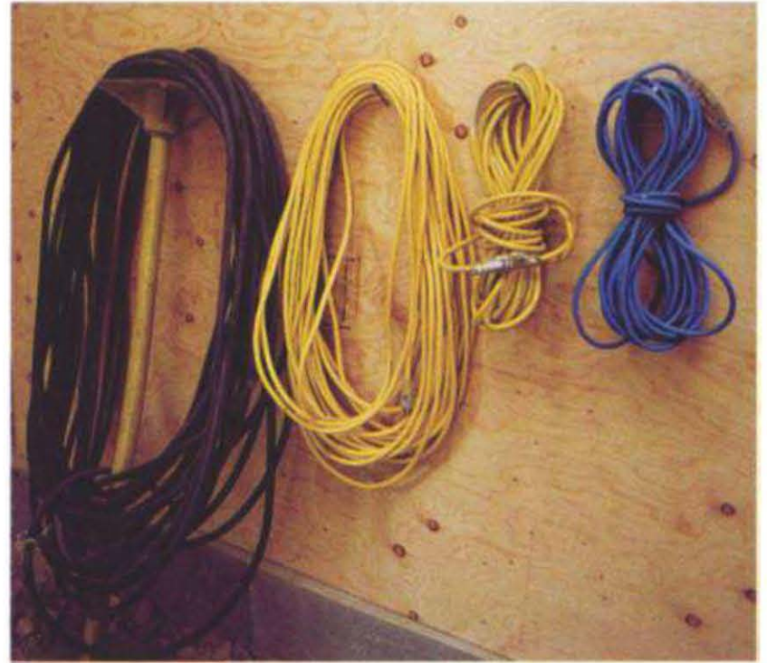
Extension cords. Heavy-duty, large-gauge cords—the lower the wire number the higher the gauge—and splitters are important. Skinny cords and bad connections quickly take their toll on your power tools by robbing them of needed amperage.
