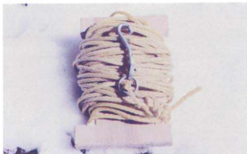
A metal clip fastened to the end of a long rope allows the crew member on the staging to easily release this tag line from a truss as it swings into place.
