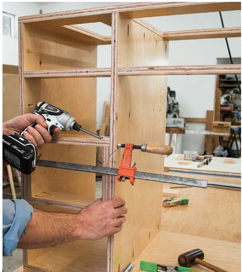
Install the middle drawer partition on the left-hand side last, again using plywood scraps to locate and install the partition.
