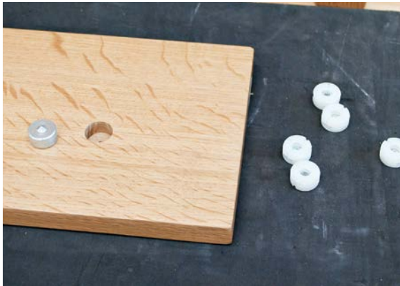
A dowel pin transfers the center of the locater hole to the drawer box.
