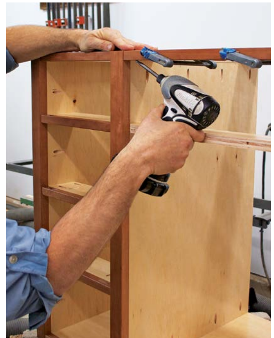
Clamp the top horizontal sink divider to the plywood web, and drive the pocket screws.
