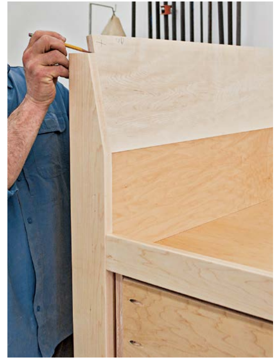
When the lower bevel on the solid maple inside panel is tight, mark the location of the top bevel.
