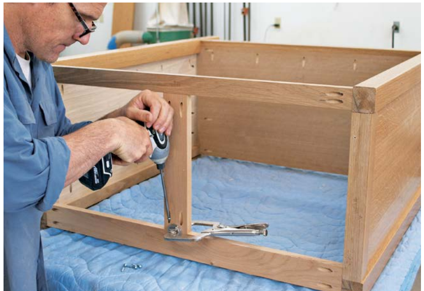
Hold the top frame short connector with a face clamp when driving the pocket screws.
