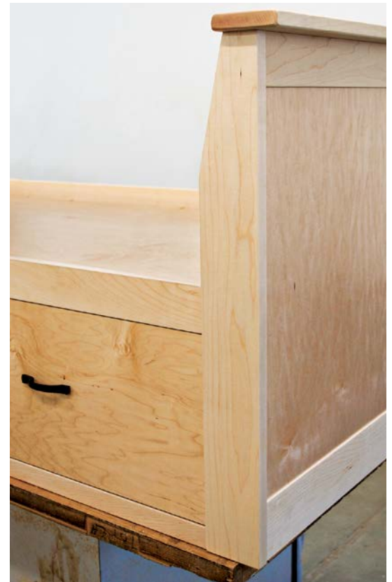
With pocket hole joinery, you can create strong joints without a single screw or screw hole visible. This is a detail of the daybed project (see p. 77).
