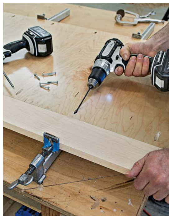
In the middle of the field, which is beyond the reach of the face clamp, use an extra-long predrill bit to get the hole started and to minimize shift.
