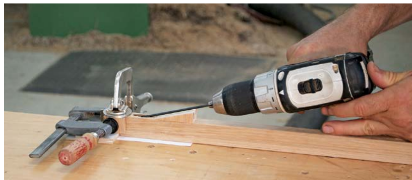
Pre-drill the end blocks of the handle using a 15-degree gauge, shimming up the handle bar with card stock so that it is flush with the end block. Clamp across the end block and hold in place with the face clamp.
