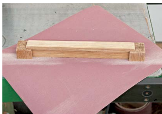
Pre-drill the end blocks of the handle using a 15-degree gauge, shimming up the handle bar with card stock so that it is flush with the end block. Clamp across the end block and hold in place with the face clamp.
