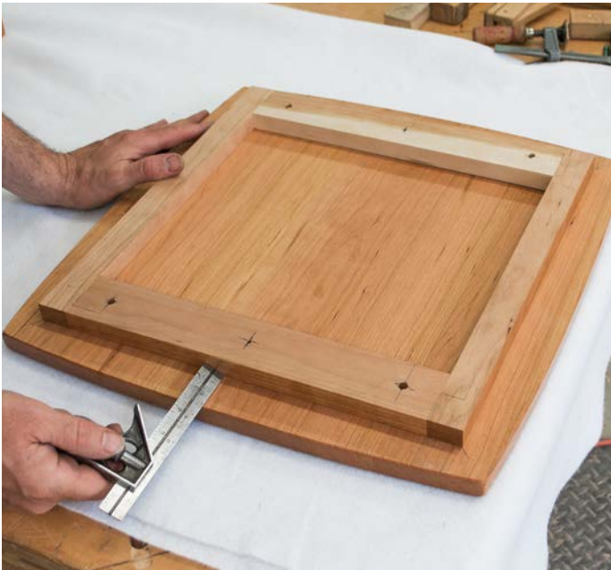
Mark the diagonals on the underside of the top to help locate the spacer frame, then use the diagonal marks and a square to center the frame on the top.
