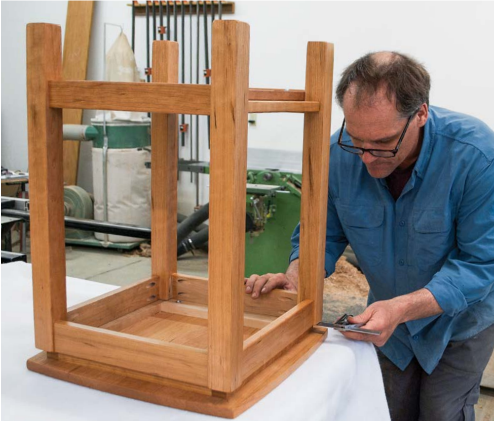
Mark the diagonals on the underside of the top to help locate the spacer frame, then use the diagonal marks and a square to center the frame on the top.
