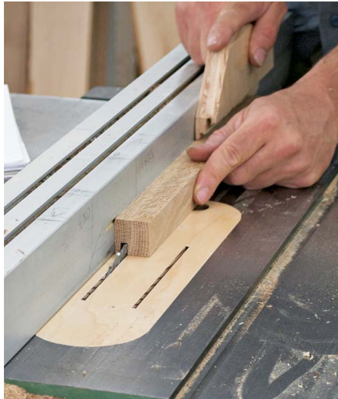
Cut the slot in the end blocks by making multiple passes over the tablesaw blade.
