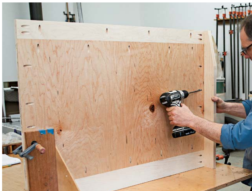
Biscuits keep the joint from shifting so it's not necessary to use clamps in addition.
