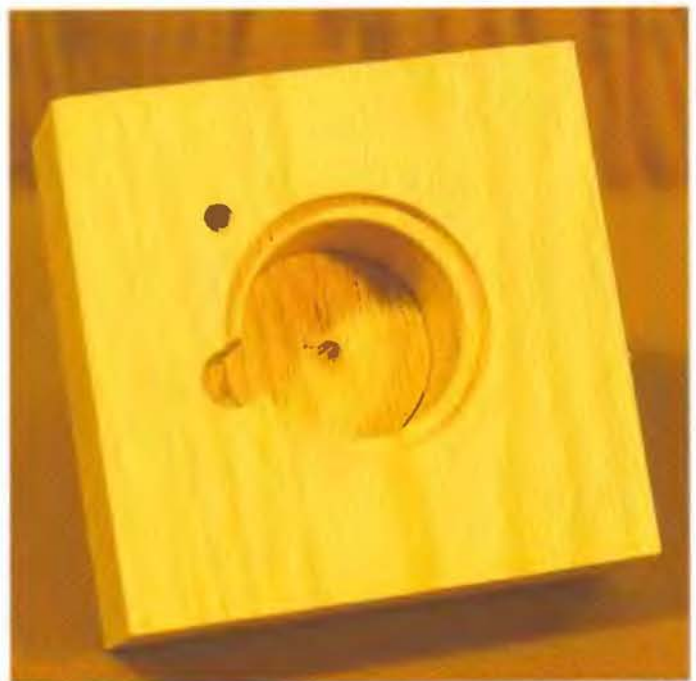
Recess for dial anchor plate.
