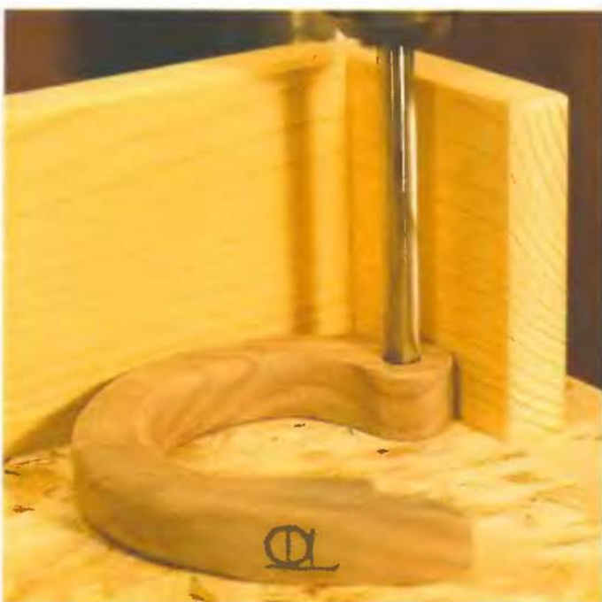
Drilling retainer pinhole in the shackle.
