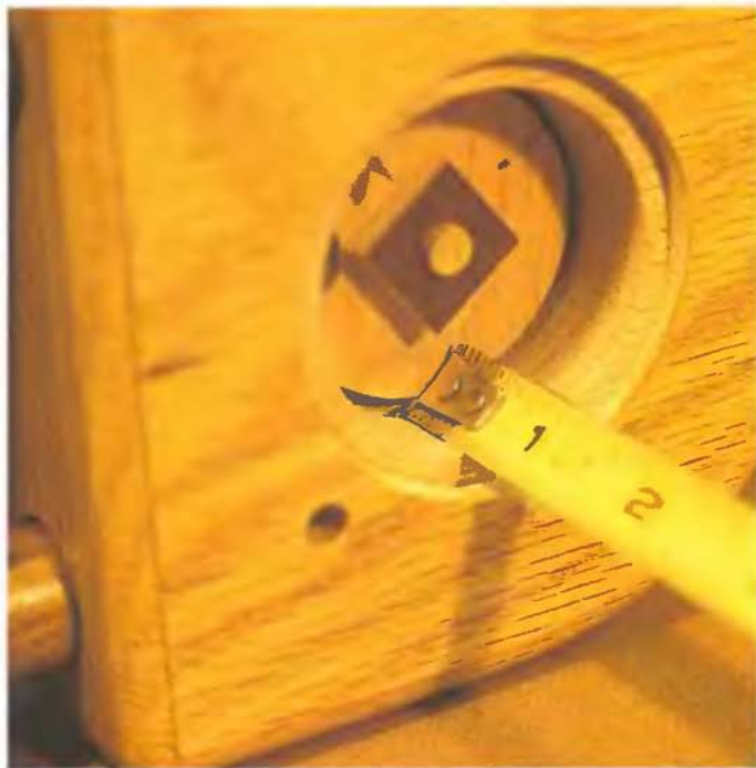
Measuring length of drive pin from face of lock.
