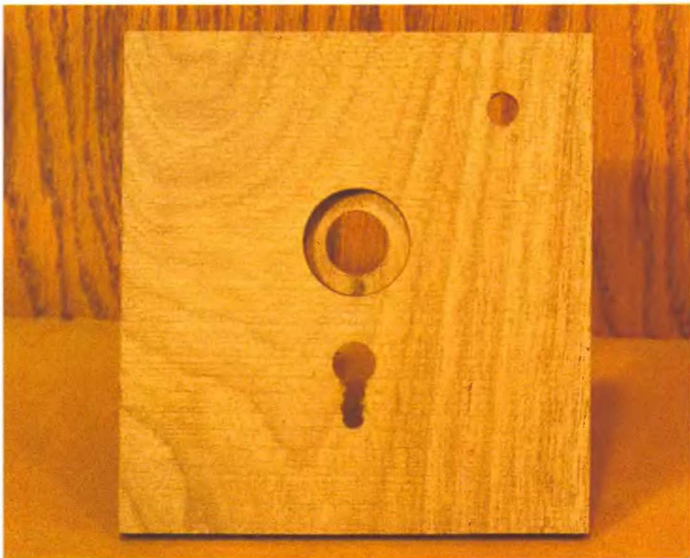
Lock face with holes bored.
