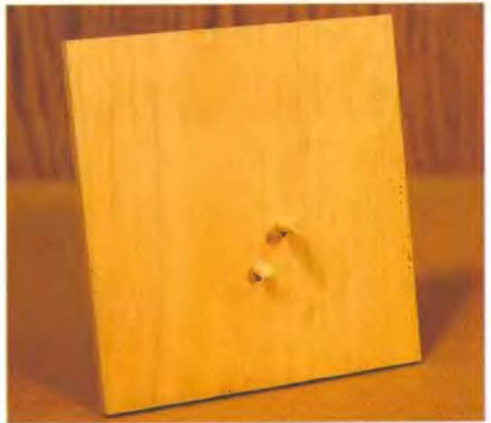
Back lamination with pivot dowels.
