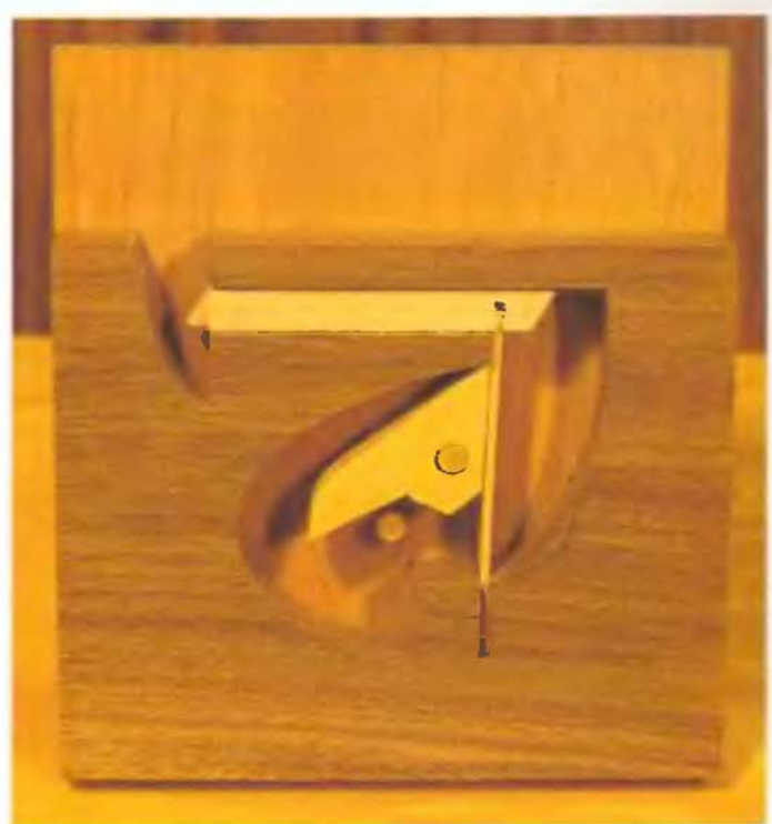
Back and center laminations with all interior parts.
