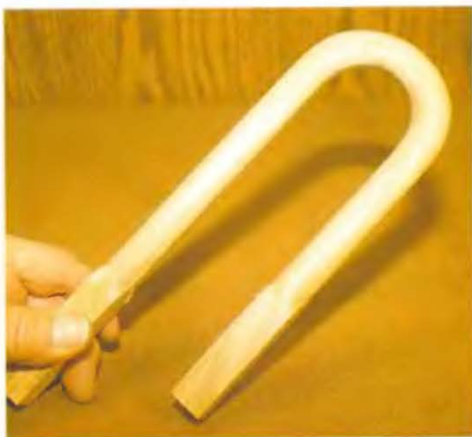
Shackle rounded over, not cut to length.
