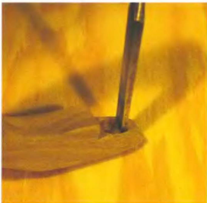
Using chisel to enlarge locking notch.
