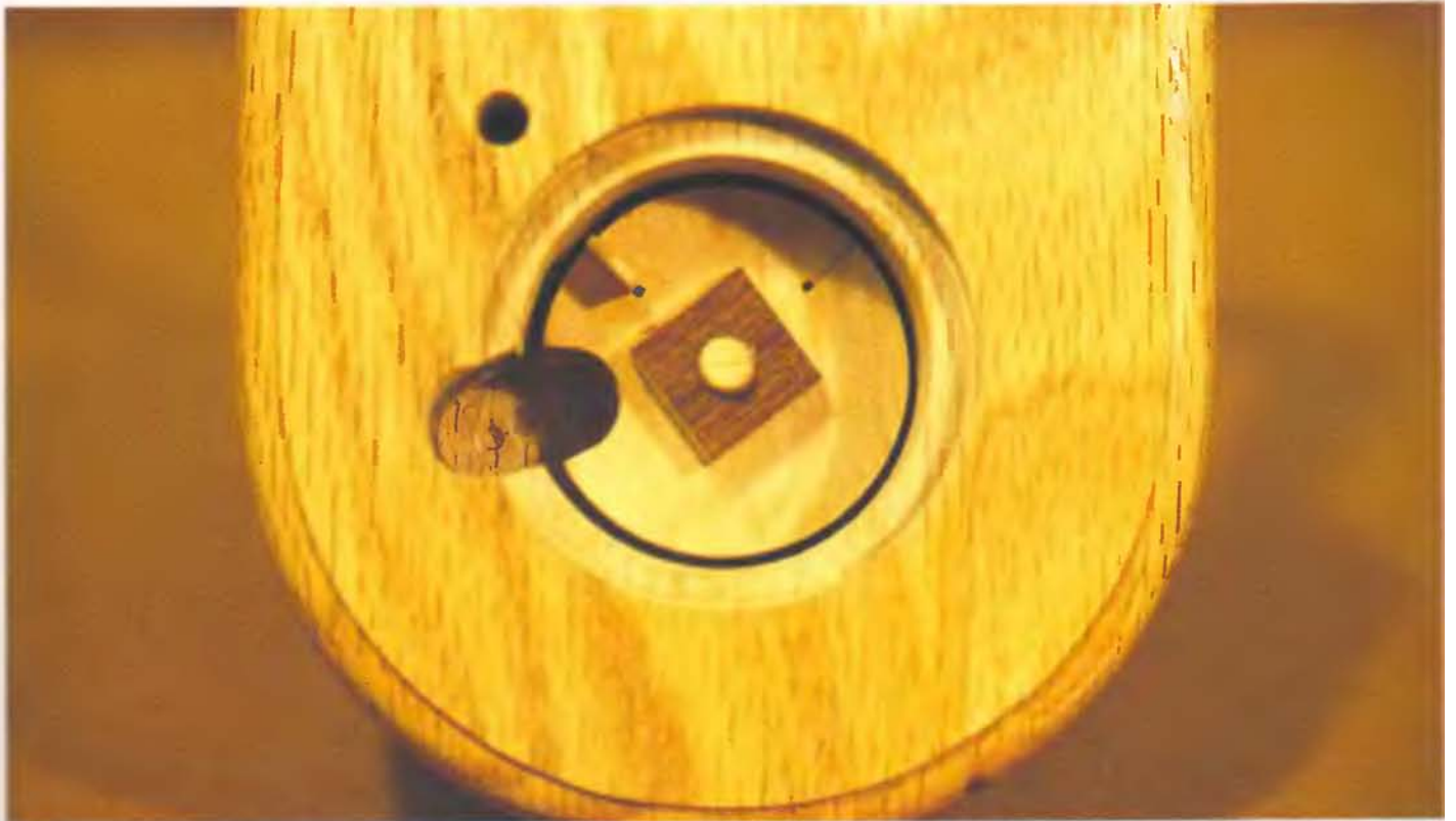
Photo 22. Tumblers lined up at locking notch.
