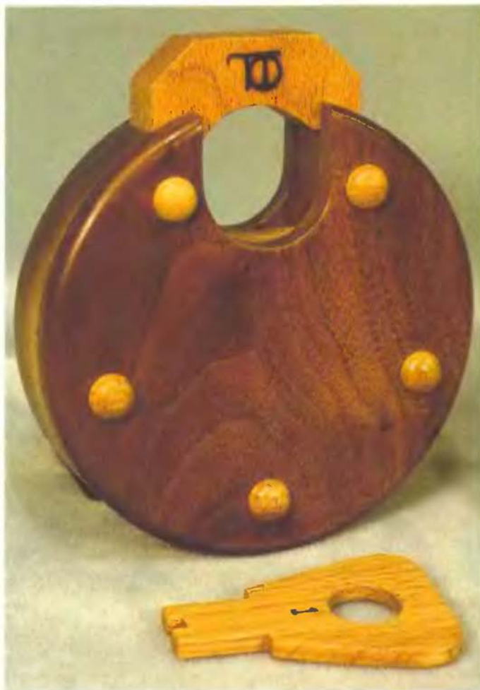
Finished push key lever lock.
