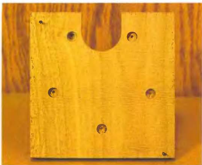
Front and back laminations with notch cutout.
