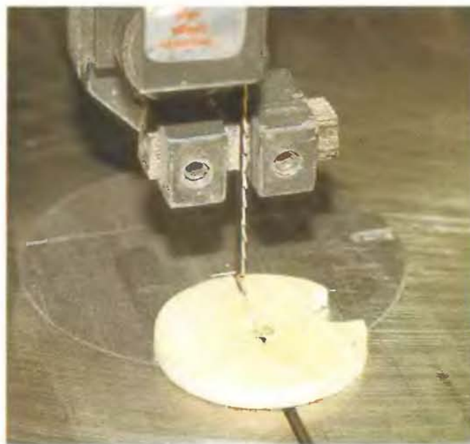
Cutting drive pin notches.
