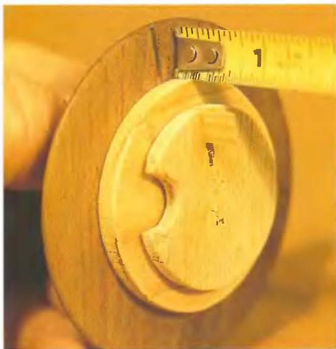
Measuring length of drive pin from dial back.
