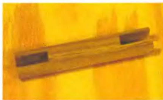
Key shaft with cutouts in each end.
