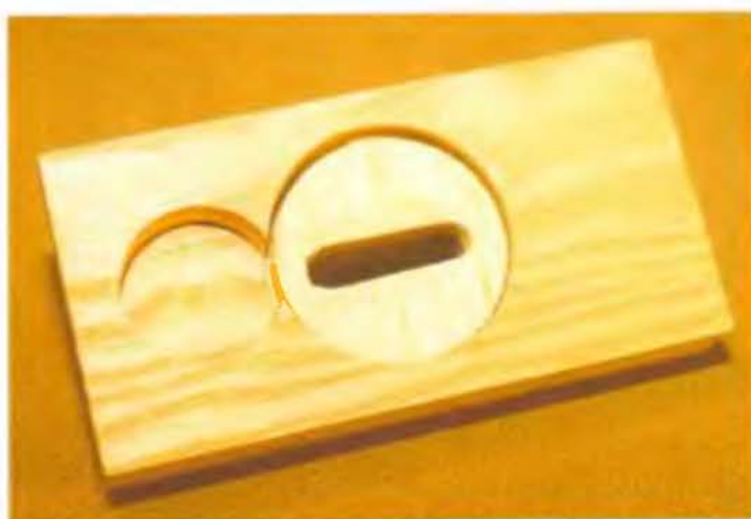
Lamination #5 with key insert in place.
