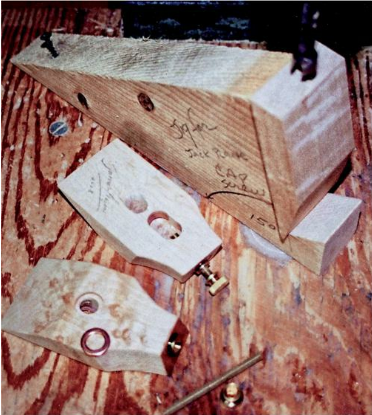
TWO-SCREW MECHANISM: Drilling top screw at 15^\circ will hold inverted thumb nut that threads the hole. Back of cap has space for rest button and \frac{3}{8} " lead screw hole. Front of cap has wear washer and adjustment rod.
