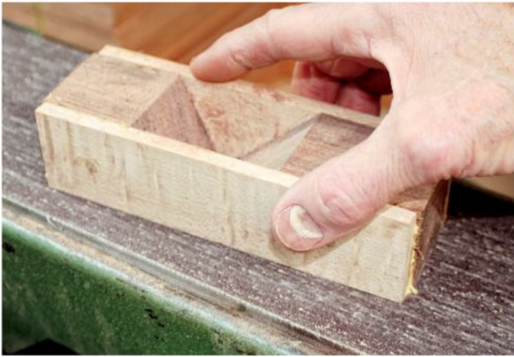
SHAPING BODY SEQUENCE I – all sides, top and sole flat and square.
