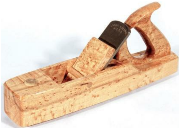
JACK PLANE WITH WEDGE AND RETAINER DOWEL PIN. This is a simple, yet effective, jack plane mechanism. Note also the wood strike button in the fore block.
