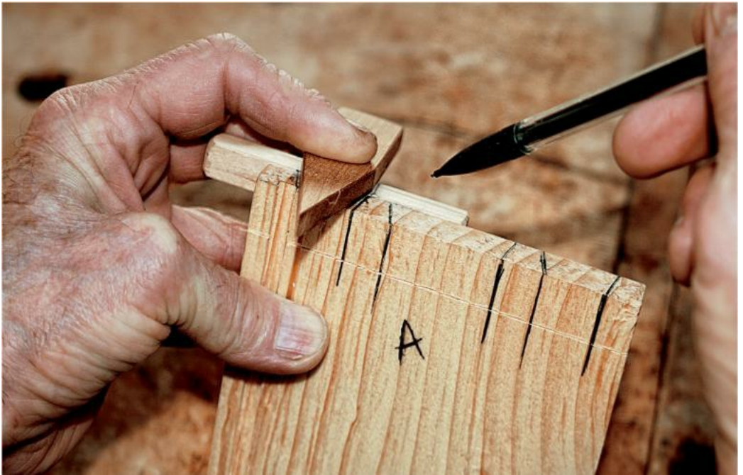
SCRIBE LINE the width ( \frac{9}{16} " ) of the other boards' thickness. Layout of pins uses both the 1:5 pitch and the square. Half pins (only one side beveled) start and end the pattern.
