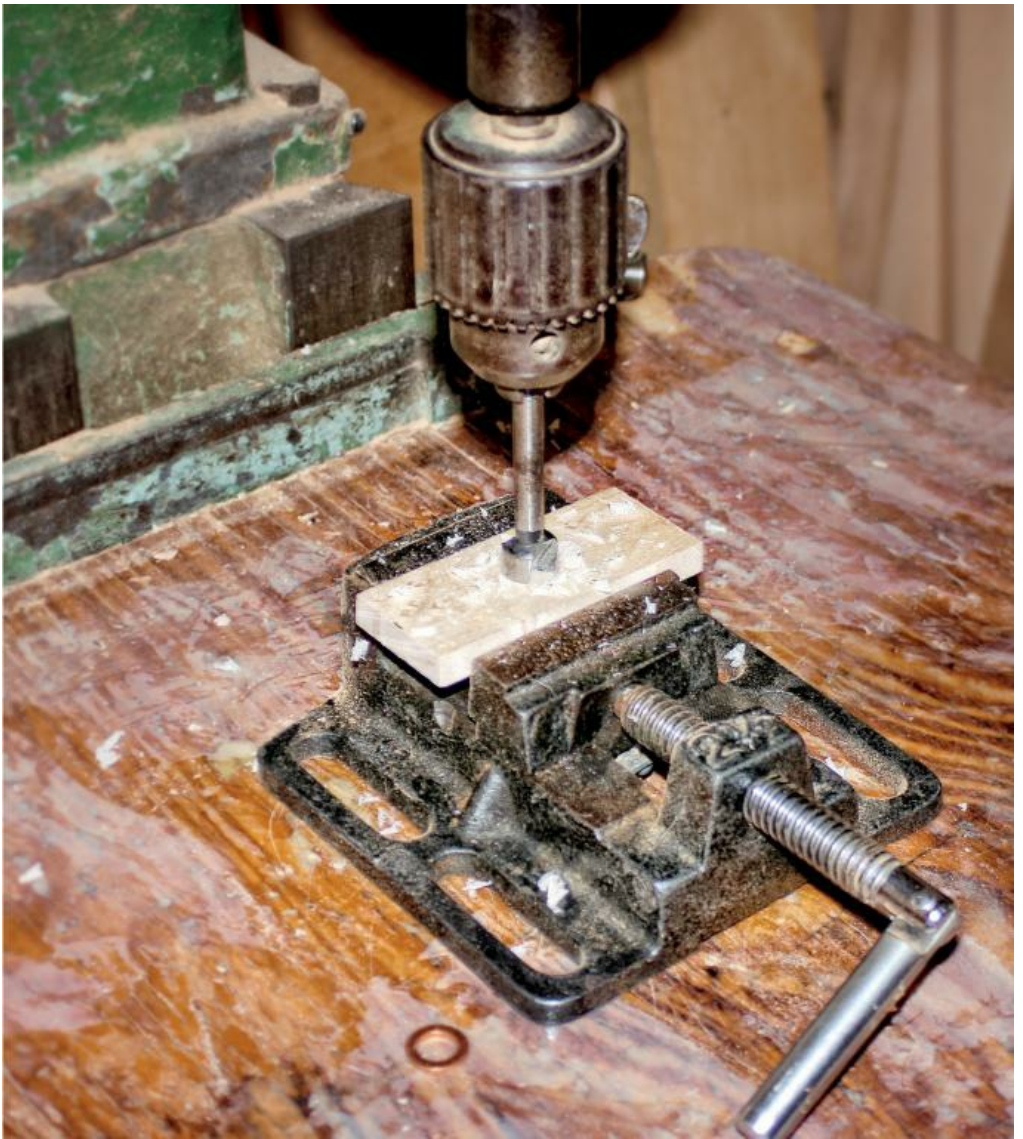
THE CAP is \frac{1}{2}'' \times 1\frac{1}{2}'' \times 3\frac{1}{4}'' with a \frac{3}{8}'' hole for the post. A nice touch is the copper ware washer shown here being drilled with a \frac{3}{8}'' Forstner bit. The washer is in the foreground.
