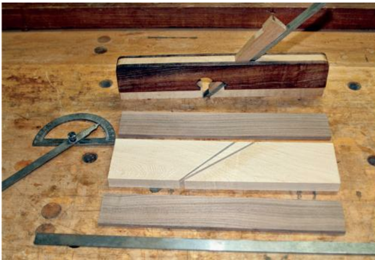
CORE BLOCK FOR SHOULDER PLANE has bedding angle of 37^\circ and fore angle 45^\circ , giving an 8^\circ wedge.
