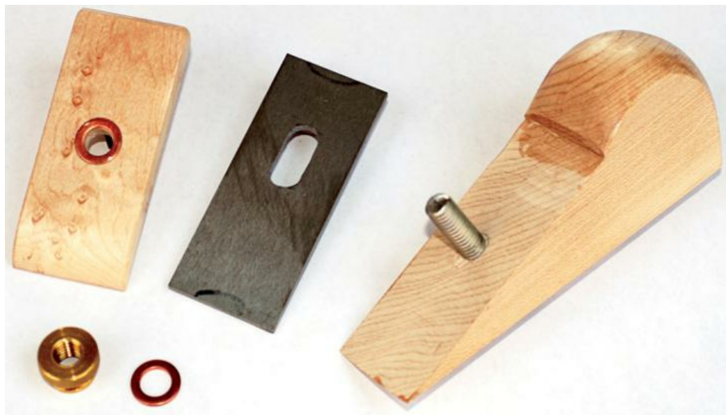
PARTS OF THE CHISEL PLANE. Cut the body from a maple blank 1\frac{1}{2} " \times 2" \times 5\frac{1}{2} ".
