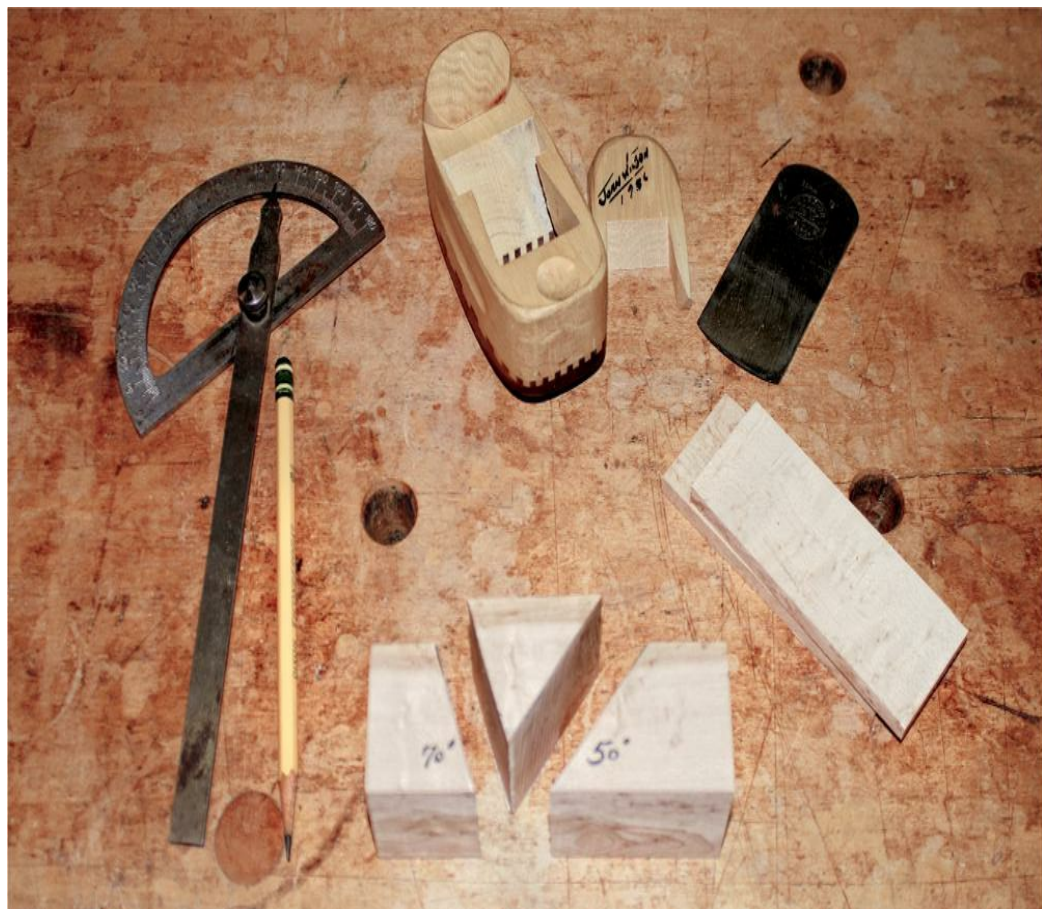
TWO COMPASS PLANES , one adapted from the German ECE block plane in the background, and parts for making one from scratch. The angles of 70° and 50° are drawn on the core block, which has been cut.
