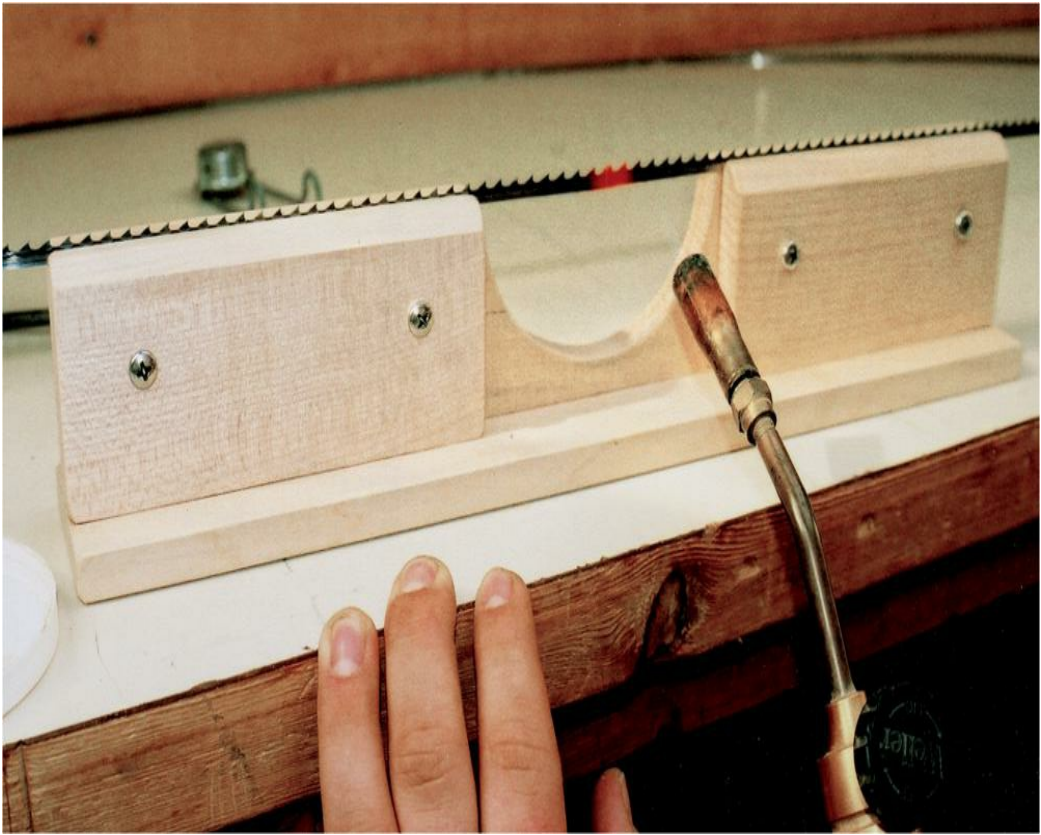
PROPANE TORCH heats joint to cherry red.
