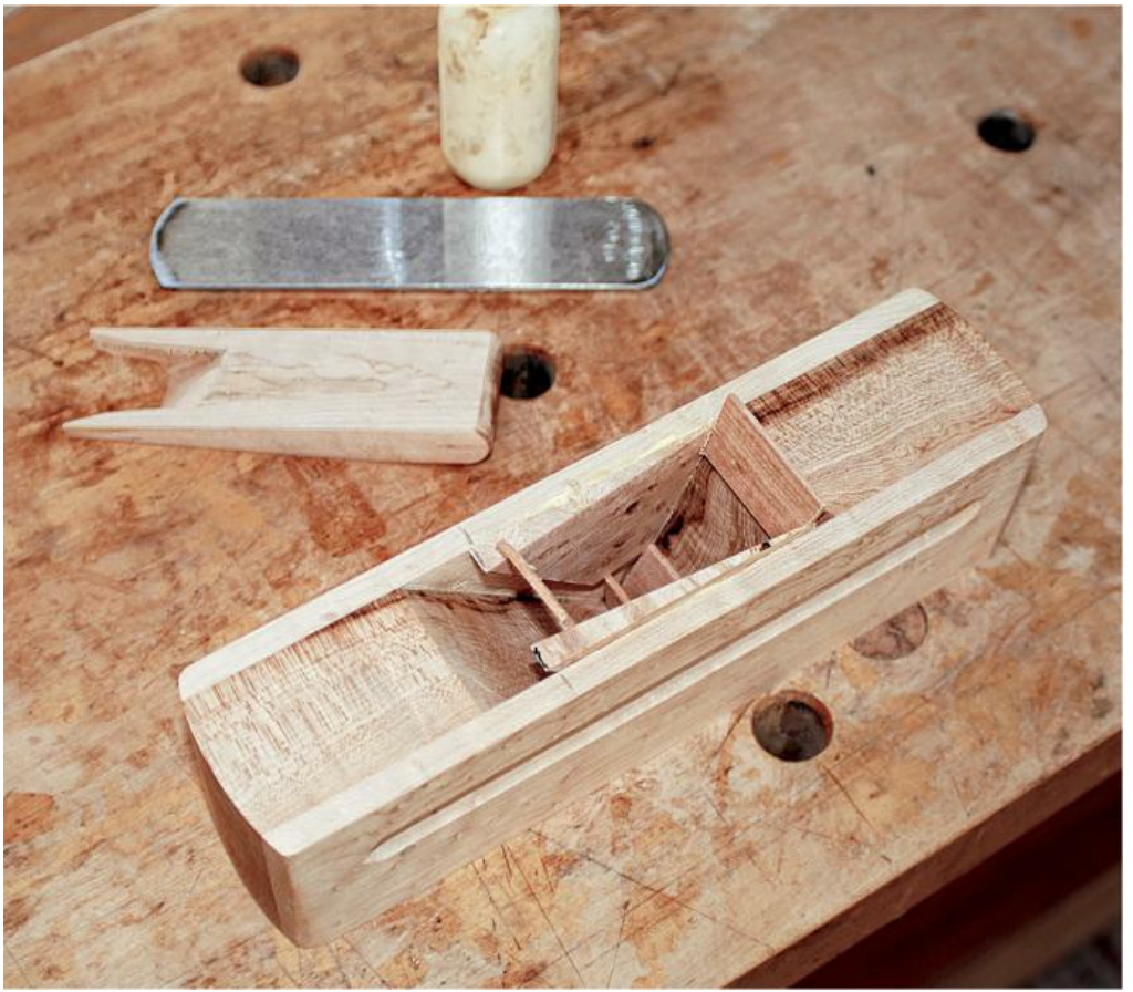
REMOVE THE WEDGE before glue sets. Final holding is made by several thin scraps of wood wedged into place.
