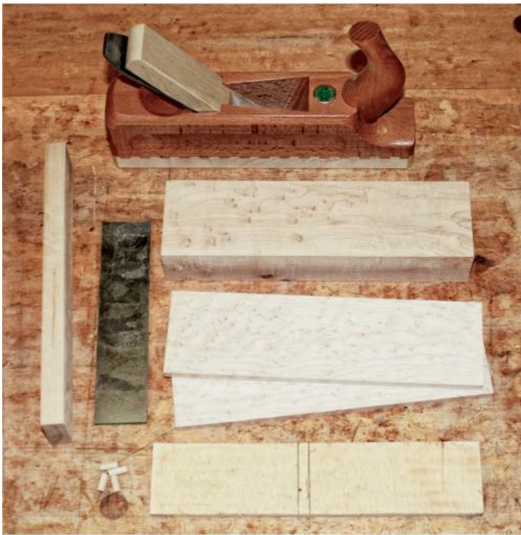
PARTS OF A SCRUB PLANE , with ECE Primus plane used as model in background.
