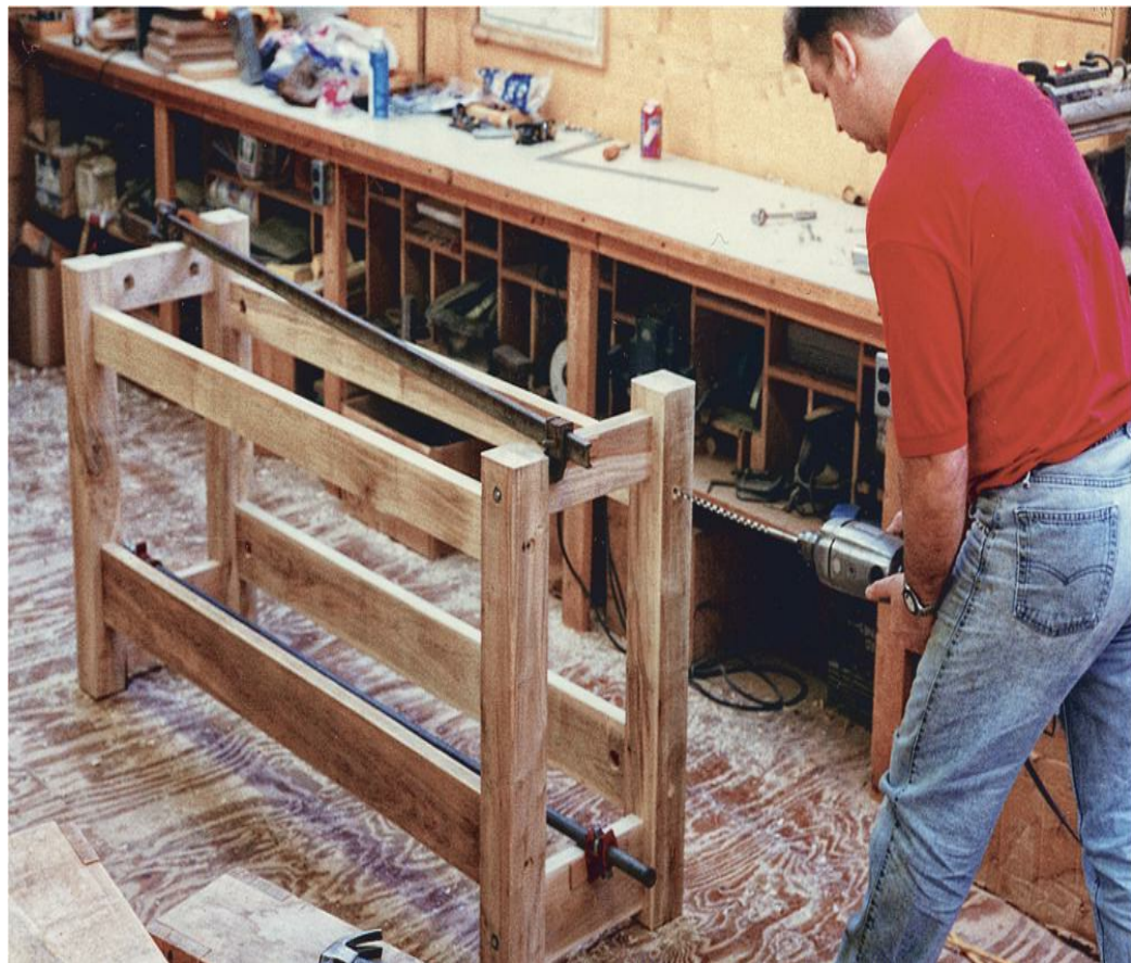
LONG CLAMPS hold the bench together, with one laid diagonally to adjust as needed to square the base. Once in place, the long \frac{3}{8} " drill completes the hole for the 6" bolts. My oldest son David is doing the work.
