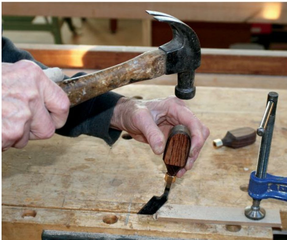
HELD IN THE VISE with the lower end resting on the bed ways, the handle is tapped in place.
