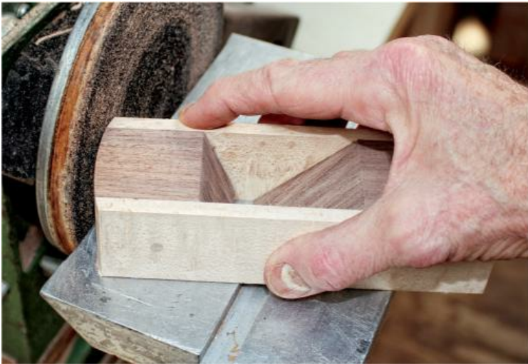
SHAPING BODY SEQUENCE II – finish both ends. Give slight arc to end on disc sander.
