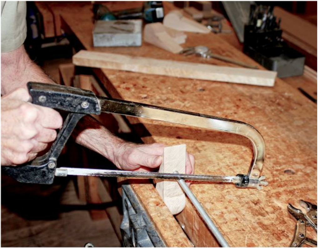
THE THREADED ROD is cut 1" long and end filed smooth.
