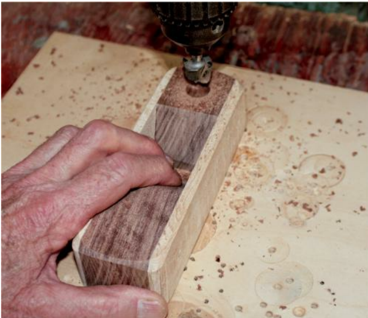
DIMPLE FORE BLOCK FOR FINGER HOLD using a router core bit chucked into the drill press. Note edge
