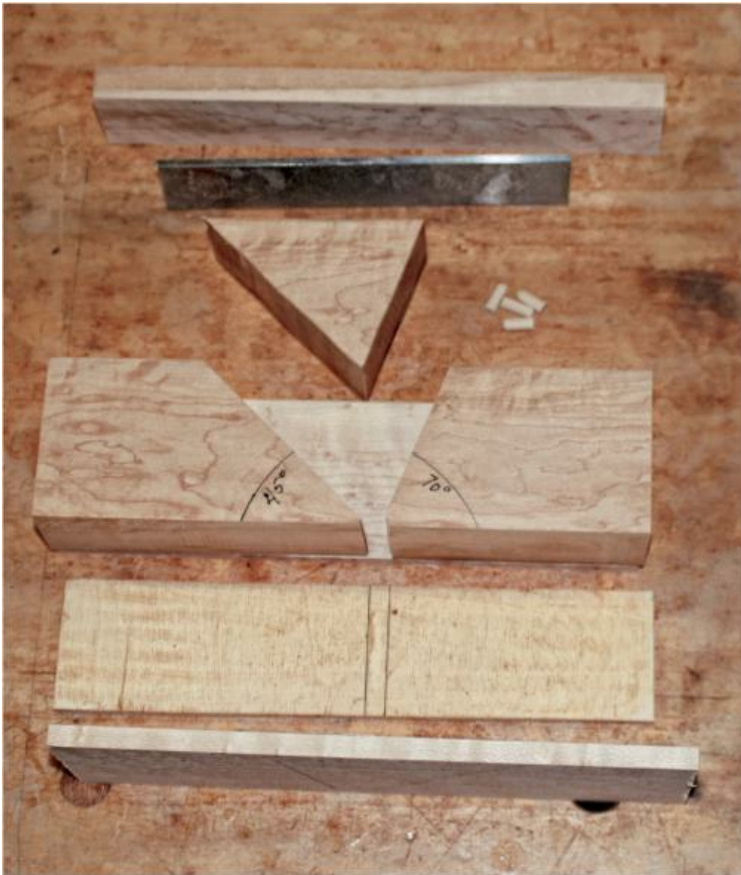
SCRUB PLANE PARTS with core block divided into fore (70°) and bedding (45°) blocks. The scrap piece will be used later for the hand block. Note the lines \frac{5}{16} " apart on the alignment board to ensure the proper throat opening.
