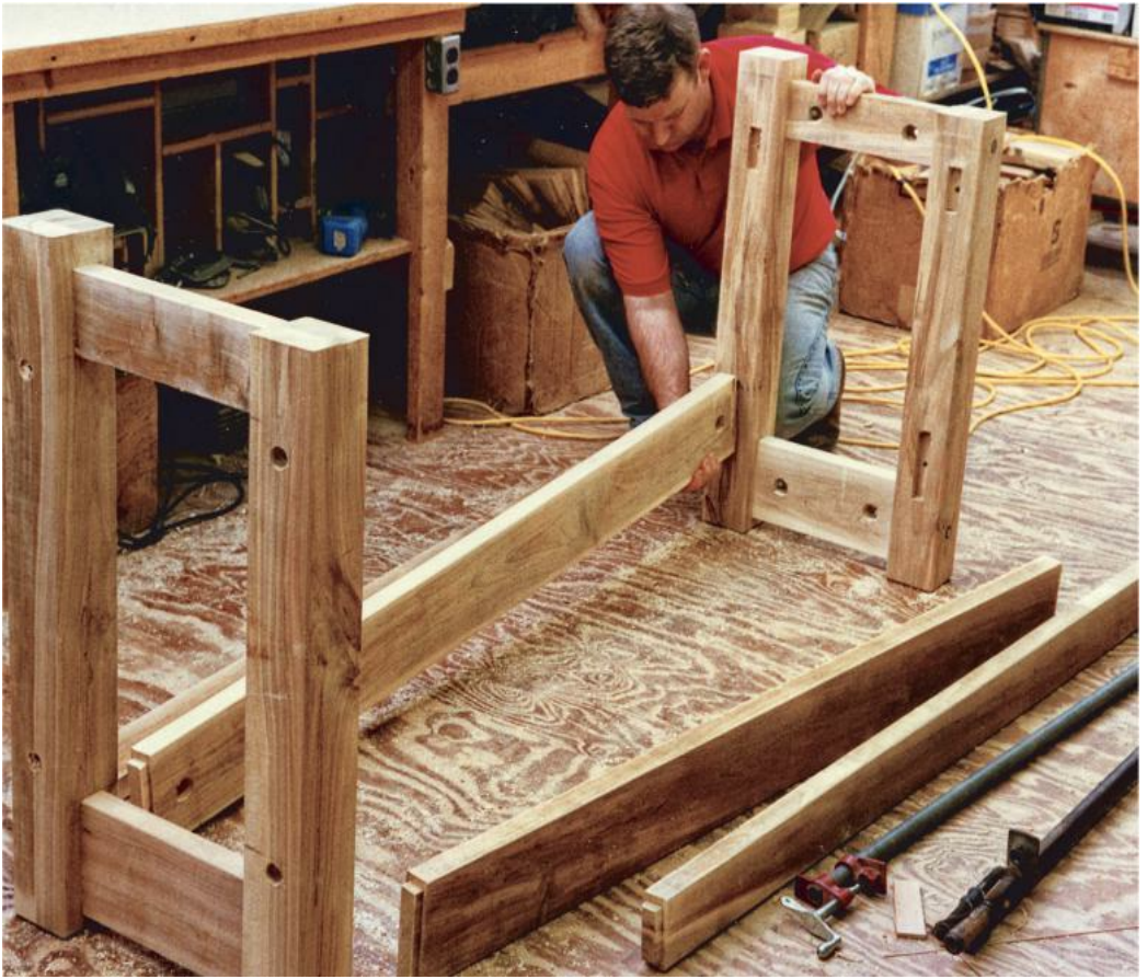
ASSEMBLY BEGINS with end sections bolted together. Here they are connected to the four long rails.
