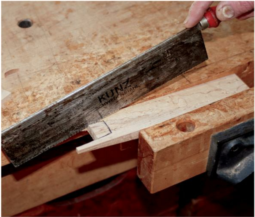
DEFINING THE SLOPE OPENING in the wedge.
