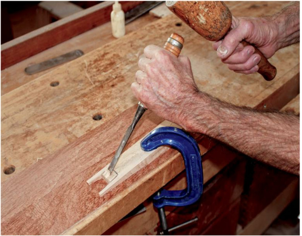
FINISHING THE CHIP CLEARANCE OPENING. The wedge is clamped to the bench using the scrap cut from the wedge and plywood under it to protect the bench. Save the scrap for gluing the abutments later.
