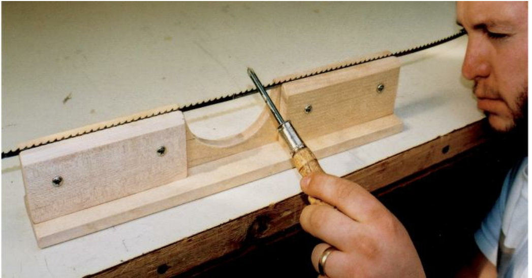
ALIGN SAW BLADE. Sighting allows accurate alignment using screwdriver to tap ends into position.
