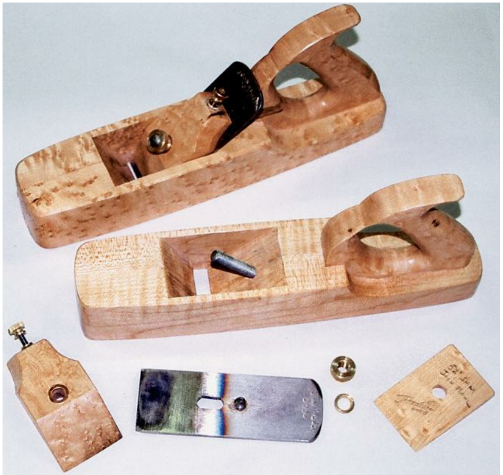
THE ELEMENTS OF A JACK PLANE WITH DOUBLE SCREW ADJUSTMENT: Razee plane body, cap with holding and adjustment screws, blade with rest button, and 52° wedge for optional smoothing plane pitch.
