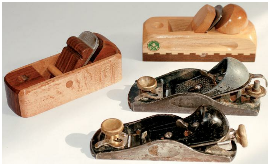
FOUR BLOCK PLANES. Stanley Model No. 9½ (middle) with standard blade angle and No. 60½ (bottom) low angle version. The wood-bodied E. C. Emmerich Co. (top right) and the shop-made model (top left) both have standard 45° angle of blade with the blade bevel down rather than up as the metal-bodied block planes do.
