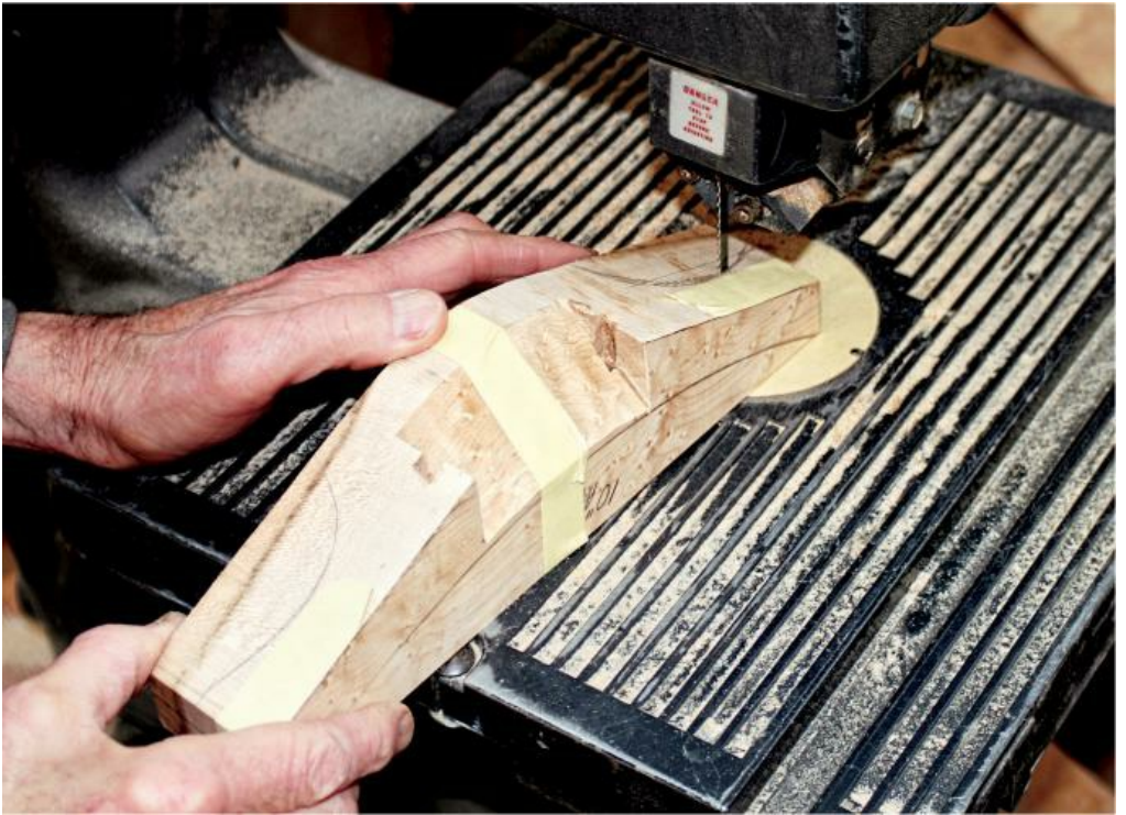
THE FINAL CUT creates the handles. The scrap block is taped to the underside to give a level base to the work.
