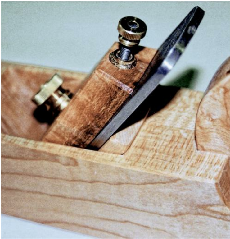
SMOOTHING PLANE OPTION: Cap assembly with added 52° wedge to allow standard 45° pitch to be changed to smoothing plane.
