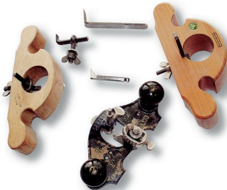
SHOWN HERE are three router planes: my shop-made version (left), an E. C. Emmerich plane (top right) and a Record No. 71, each with their cutter.
