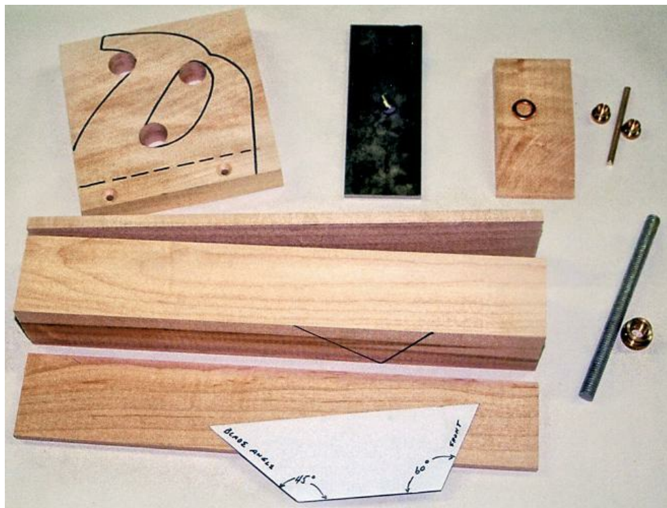
PARTS OF THE JACK PLANE: Handle with \frac{3}{4} " holes prior to cutting, blade, cap parts, core block and sides, angle pattern, lead screw and thumb nut.
