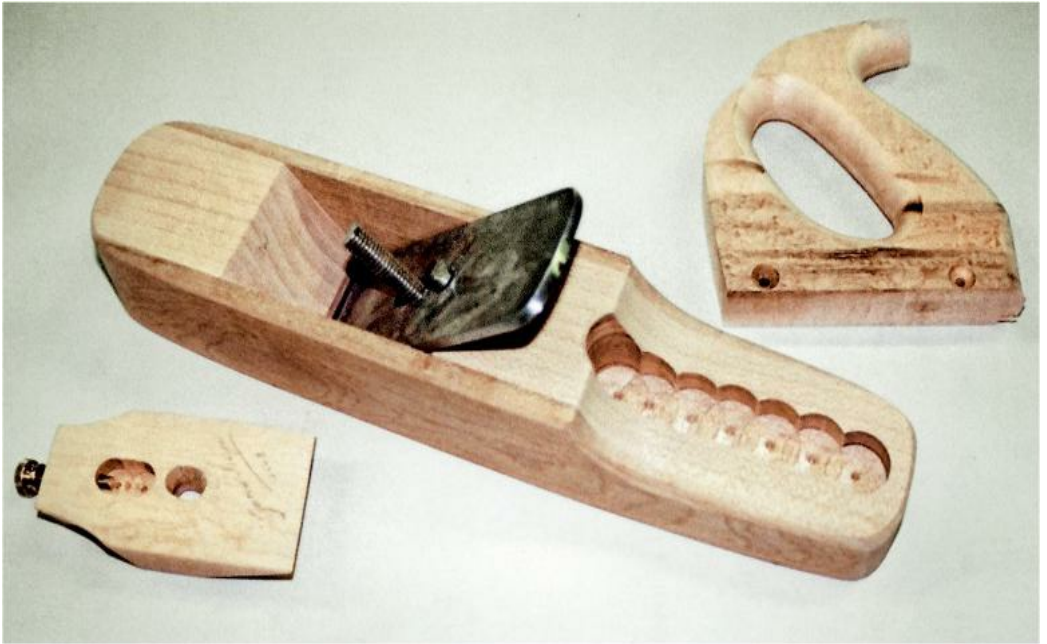
ONE STEP TO GO in fitting the handle. The body is glued and shaped. The threaded post and finished blade and rest
