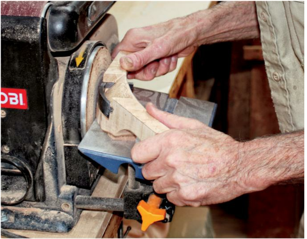
THE FINAL SHAPING is the 5° approach to the blade sanded on the sole.
