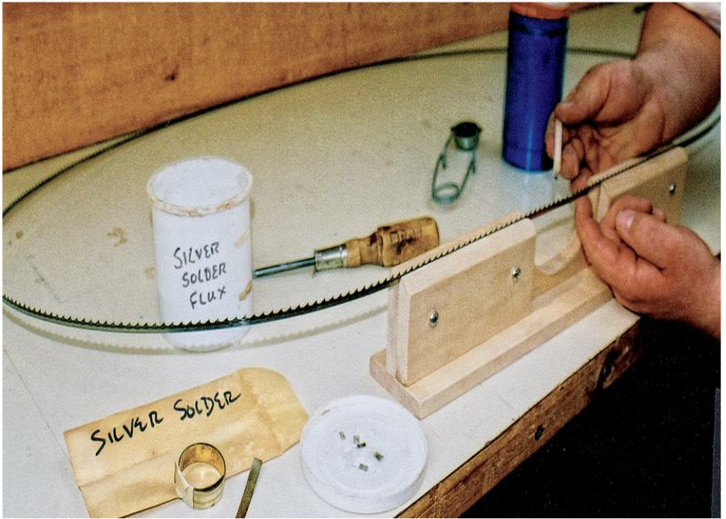
RIBBON SILVER SOLDER with nickel alloy is cut into small pieces (see container top). Silver solder flux and one measured piece of solder is put into the joint.
