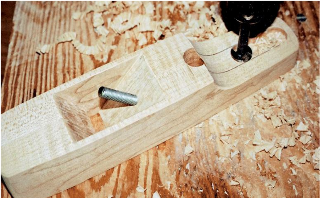
DRILL RECESS with Forstner bit for bedding the handle with Forstner bit.
