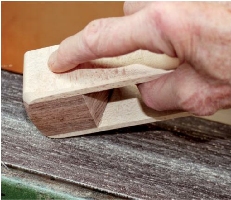
SHAPING BODY SEQUENCE III – round over where sides meet ends, then chamfer edges as seen in this and other photos.
