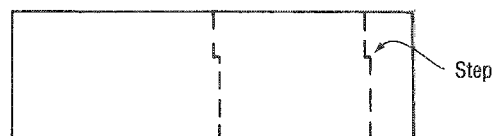
Fig. 4.30 Step caused by poor marking out or careless cutting.
