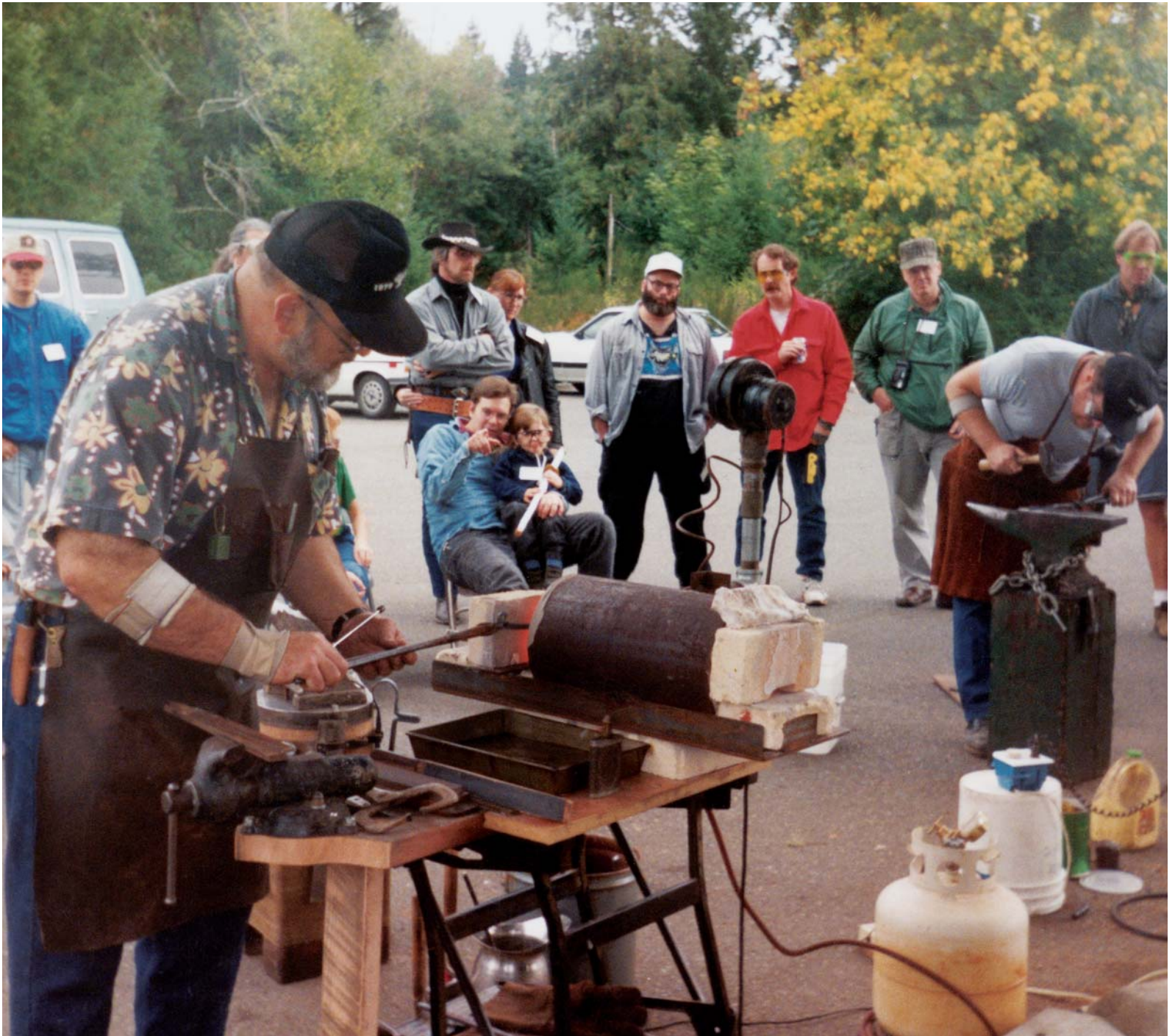
This photo shows the tabletop forge from the back side, note how the vise is set up. I'm holding the blade between a fire brick and the fire chamber to heat for the quench. Tempering was carefully done the same way. Gene Chapman is at the right trying to catch up with me.
