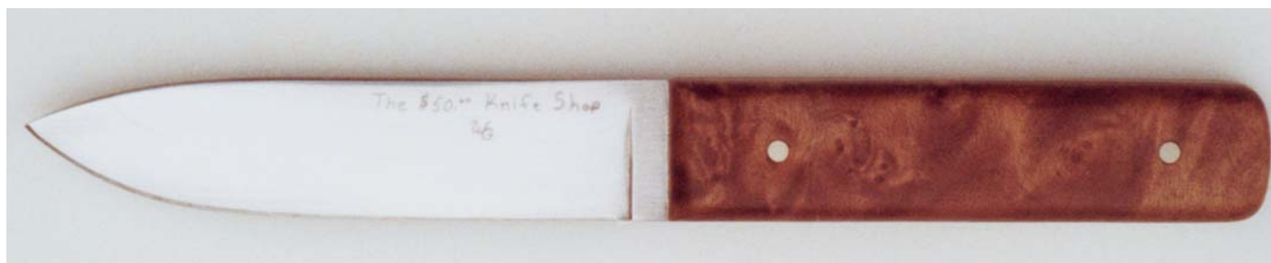
The finished stock-removal knife made from the lawnmower blade.
