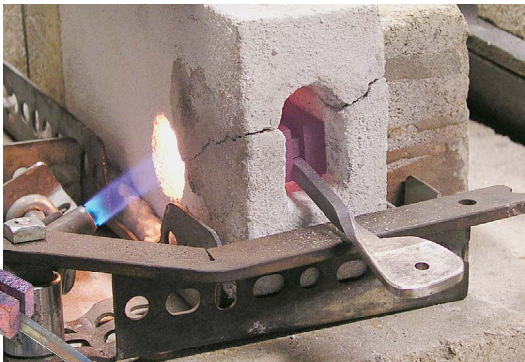
The tempering gizmo being heated.
