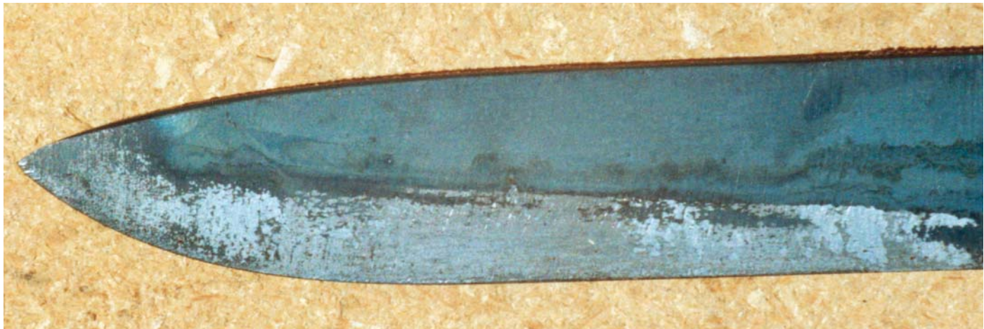
The appearance of a blade after an edge quench.
