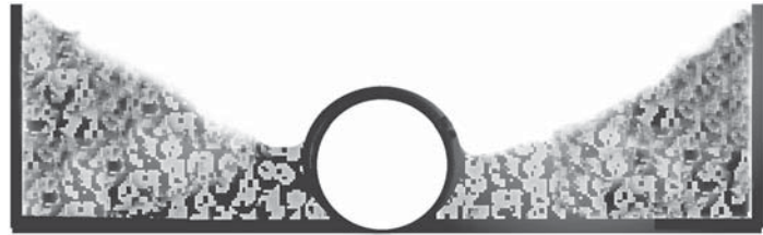
This is what the cross section of a pipe tuyere forge looks like.
