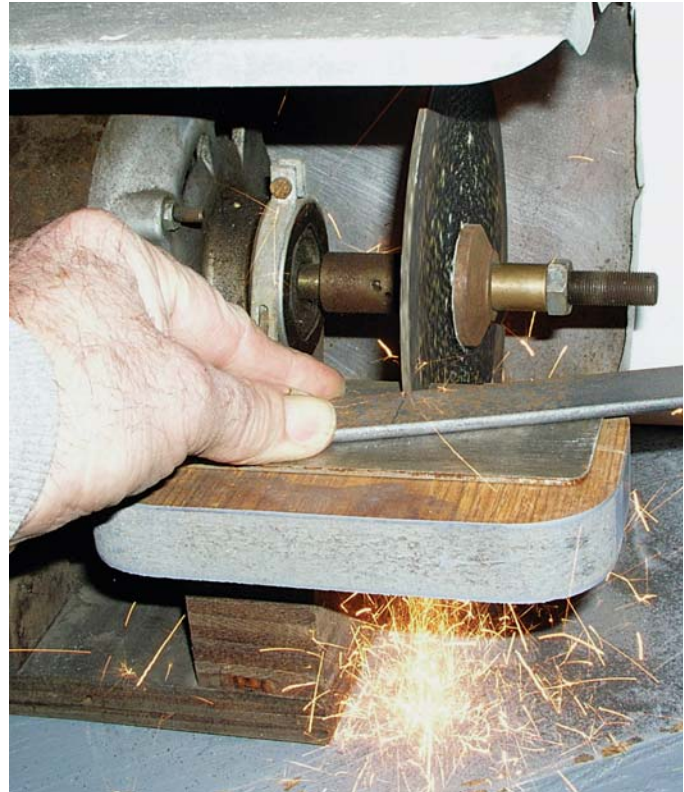
The Good News Grinder as an abrasive cut-off machine.
