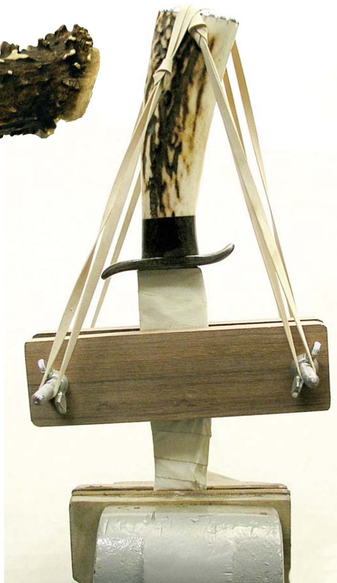
"The knife in the jig has a pommel cap that is screwed on, it wouldn't need the jig for the glue-up. (It was the only knife I had on hand to put in the jig for the photo.)"
