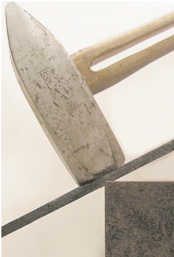
This is called the mush blow, it uses the edge of the anvil as a bottom tool. It's not the best way to hot-cut bar stock but I've been places where there was no other way. The sharper the edge of the anvil, the better it works.
