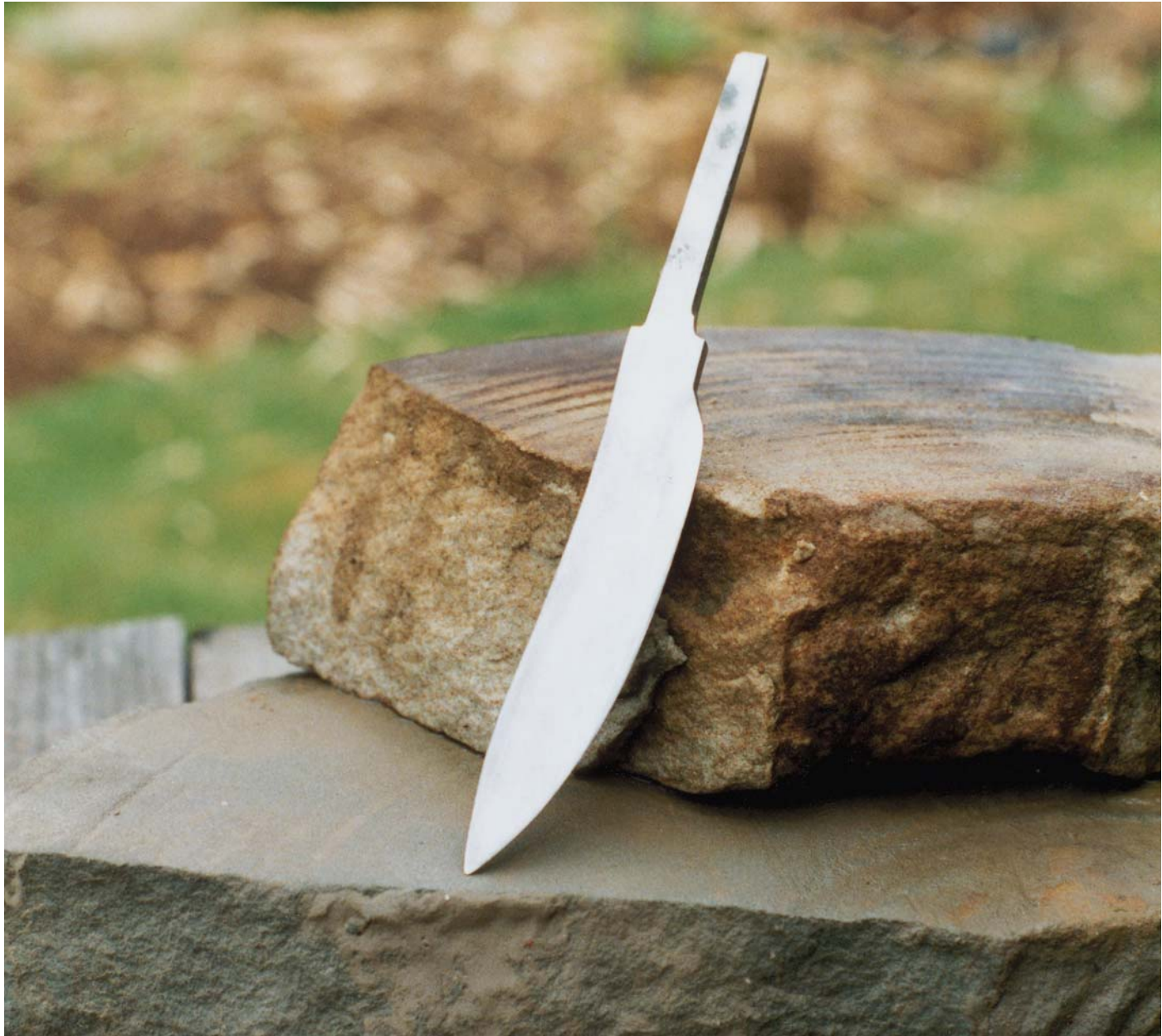
The two sandstone rubbing stones, one has a medium-grit size, the other fine. The forged project blade is ready for heat-treating
