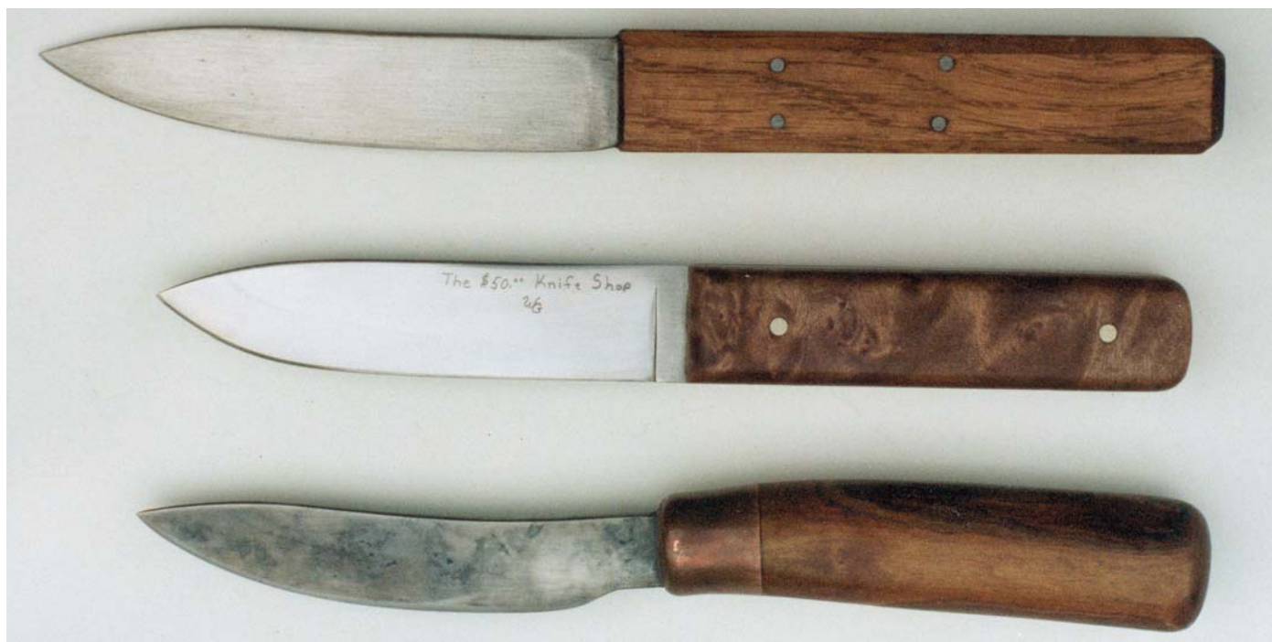
Top, the project knife from the 1988 article, “How to Make a Buckskinner Knife”. At center is the stock removal knife made from the worn out lawn mower blade. Bottom, the forged knife from The $50 Knife Shop series.
