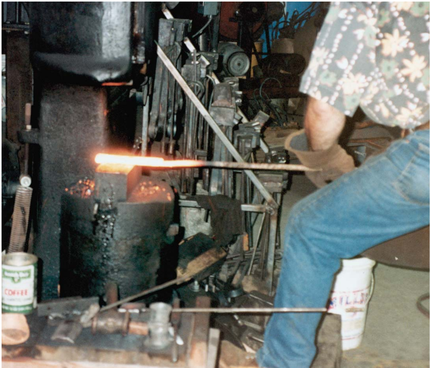
The author shown welding a billet of motorcycle chain under a Beaudry power hammer. This hammer is in the shop of Joe Elliot in Redmond, Oregon. The event was a workshop sponsored by The North West Blacksmith Association.
