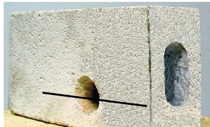
This photo shows the location of the fire hole in relation to the heat hole.
