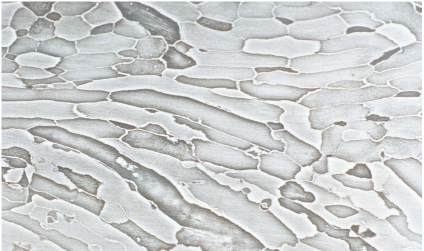
Close-up view of a wire damascus blade that is made from wire rope that has wires of three different alloy content.
