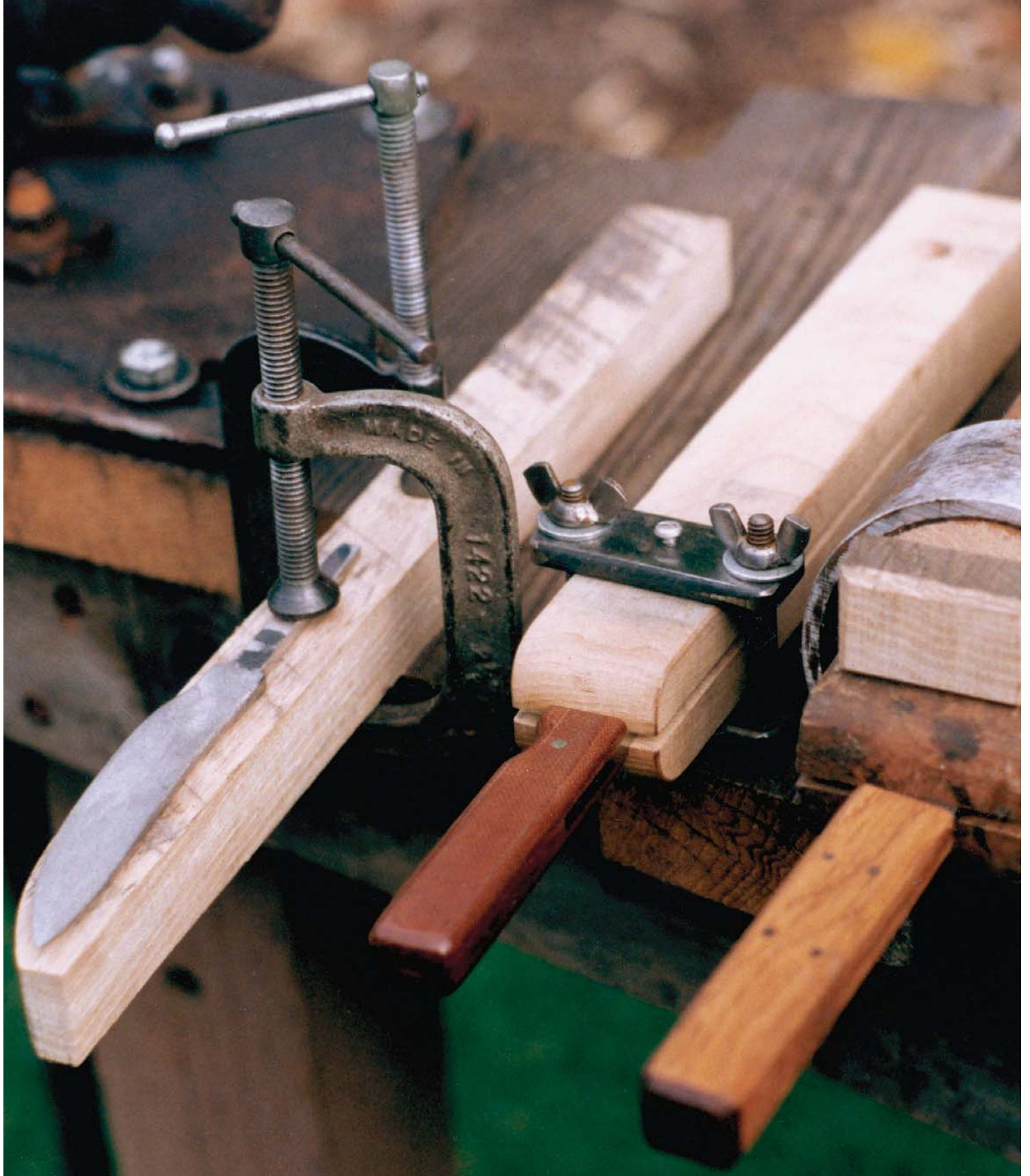
Left to right: A simple knife board with a blade in the working position. In the center an “improved” model knife vise made of wood. At the right a heavy-duty knife vise uses wedge power to hold a knife by the blade.
