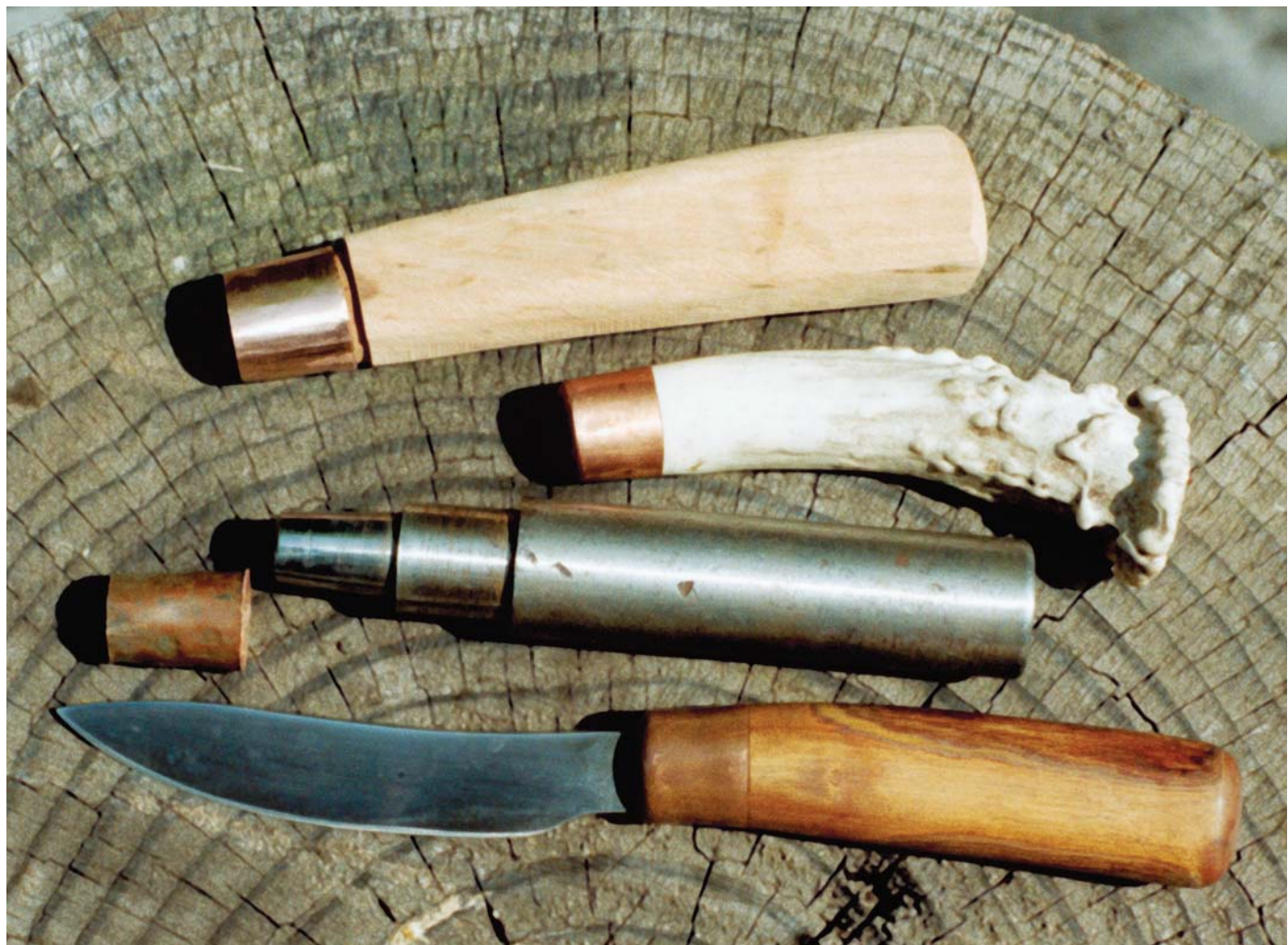
Top, a rough handle of chinquapin from a firewood pile that has been fitted for a copper ferrule. Chinquapin, genus Castanopsis is an evergreen tree found in the Pacific Northwest. It is light tan colored, about the hardness of maple or walnut. Second from top is a deer antler that has been fitted with a copper cap. This type of ferrule requires a bit more work to make the hole for the tang but gives a smooth and attractive transition where the blade comes out of the handle. The tapered punch used to form the ferrule is next to a piece of scrap copper tubing. At the bottom is the forged blade from The $50 Knife Shop Series. The handle had been stained and the knife seen some use by the time this picture was taken.
