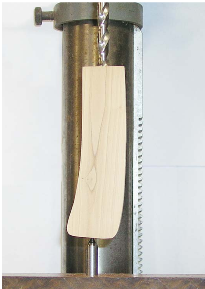
The handle material in alignment for through drilling.
