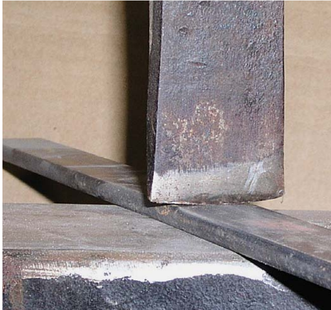
Using the hot cutter to cut bar stock.
