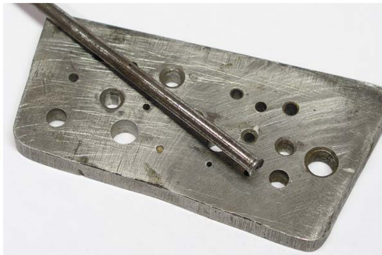
The swage block showing the head formed by driving it into the block.
