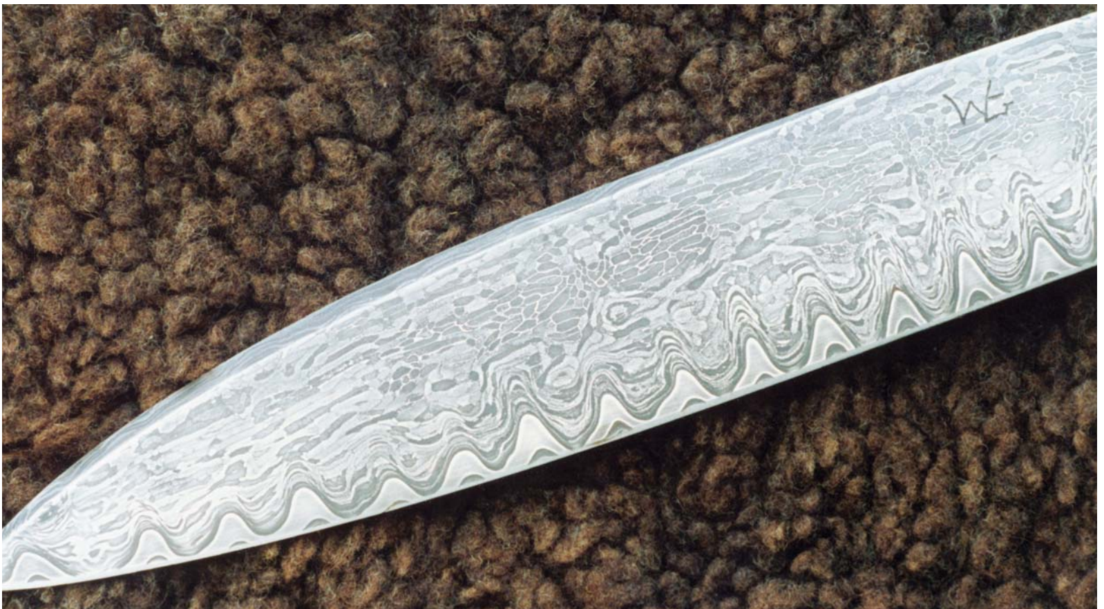
San Mai blade by the author. Wire damascus forms the outer skin, the core is bandsaw steel. Note how the hard core alternates with the wire damascus material at the edge.
