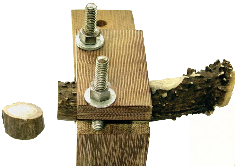
End view of the "V" block sawing jig.
