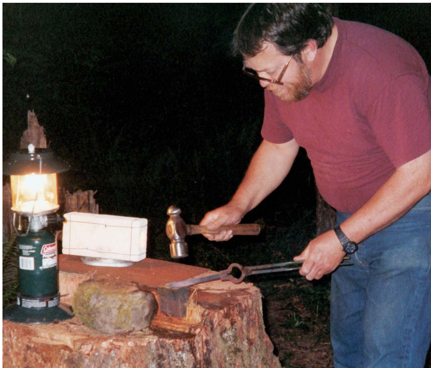
Dave Rider is up in the woods with his stump anvil and a one-brick forge. He forged a small blade from the tine of an old-time hay rake.
