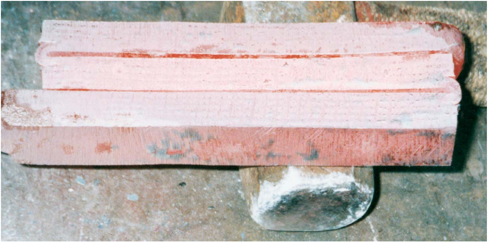
This pattern-welded billet has been tripled prior to the second welding heat.
