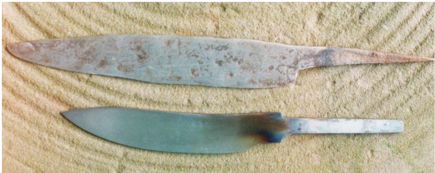
The tribal knife blade showing the tang detail. The blade at the bottom was the forged project for The $50 Knife Shop project. It qualifies as tribal because no electricity or power tools were used to make it. The heat color is the result of hot fitting the tang in to the handle.
