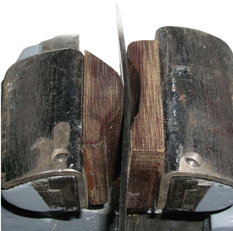
A three-point blade straightening setup made of Micarta and angle iron.
