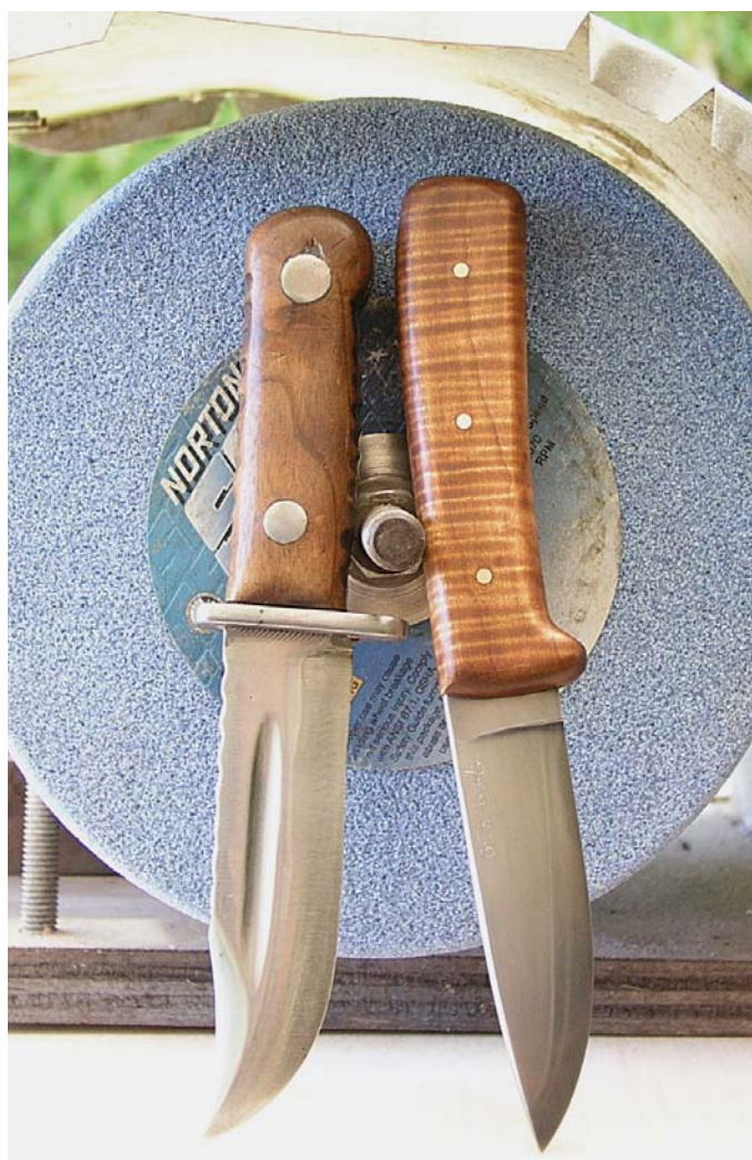
The two knives span the 42 years of Goddard knives. The knife on the left is the one that got me started on my life's work back in 1963. The one on the right is from 2005 and was ground and disc-sanded smooth using the Good News Grinder. It was my working knife project for the Krause book, BLADE's Guide to Making Knives .
