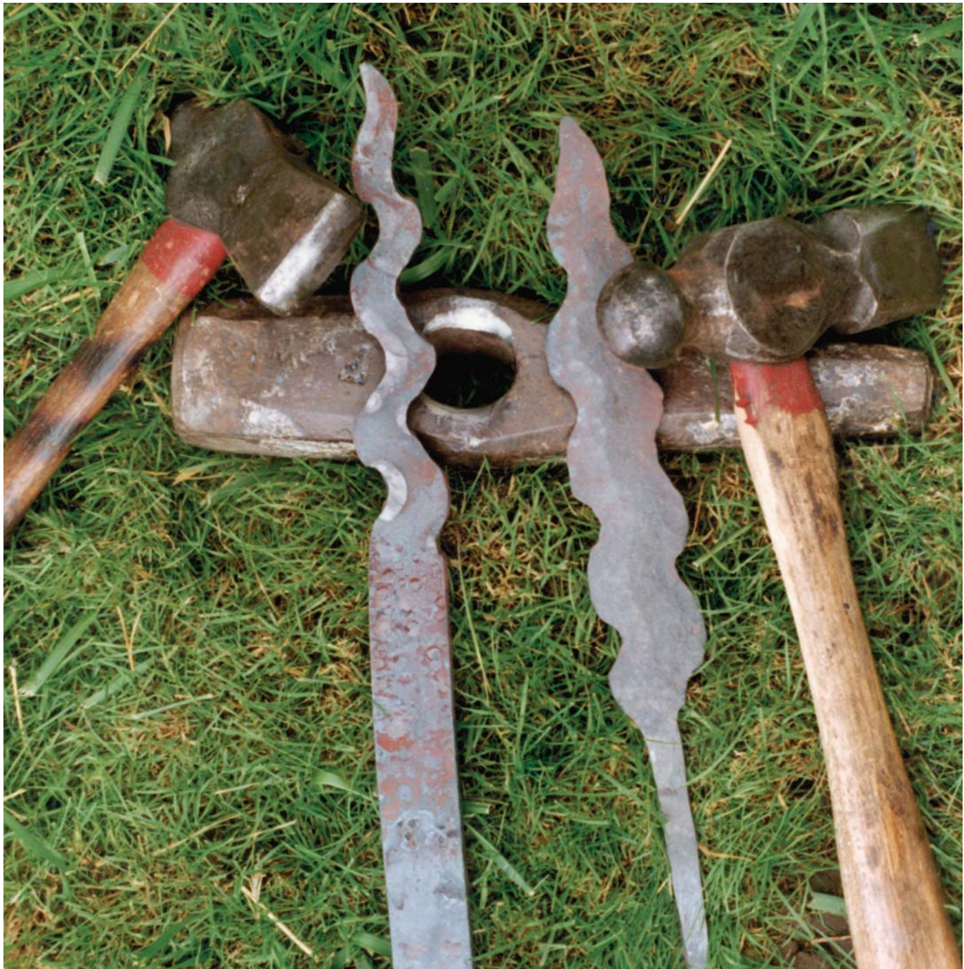
The pre-form is having waves formed with a top and bottom tool. Note the thickening at the bottom of the waves, it is important to keep this material pushed back into the pre-form as work progresses. The top tool is a reworked ball peen hammer, the bottom tool is a ship's maul that has the edges of the eye well rounded.
