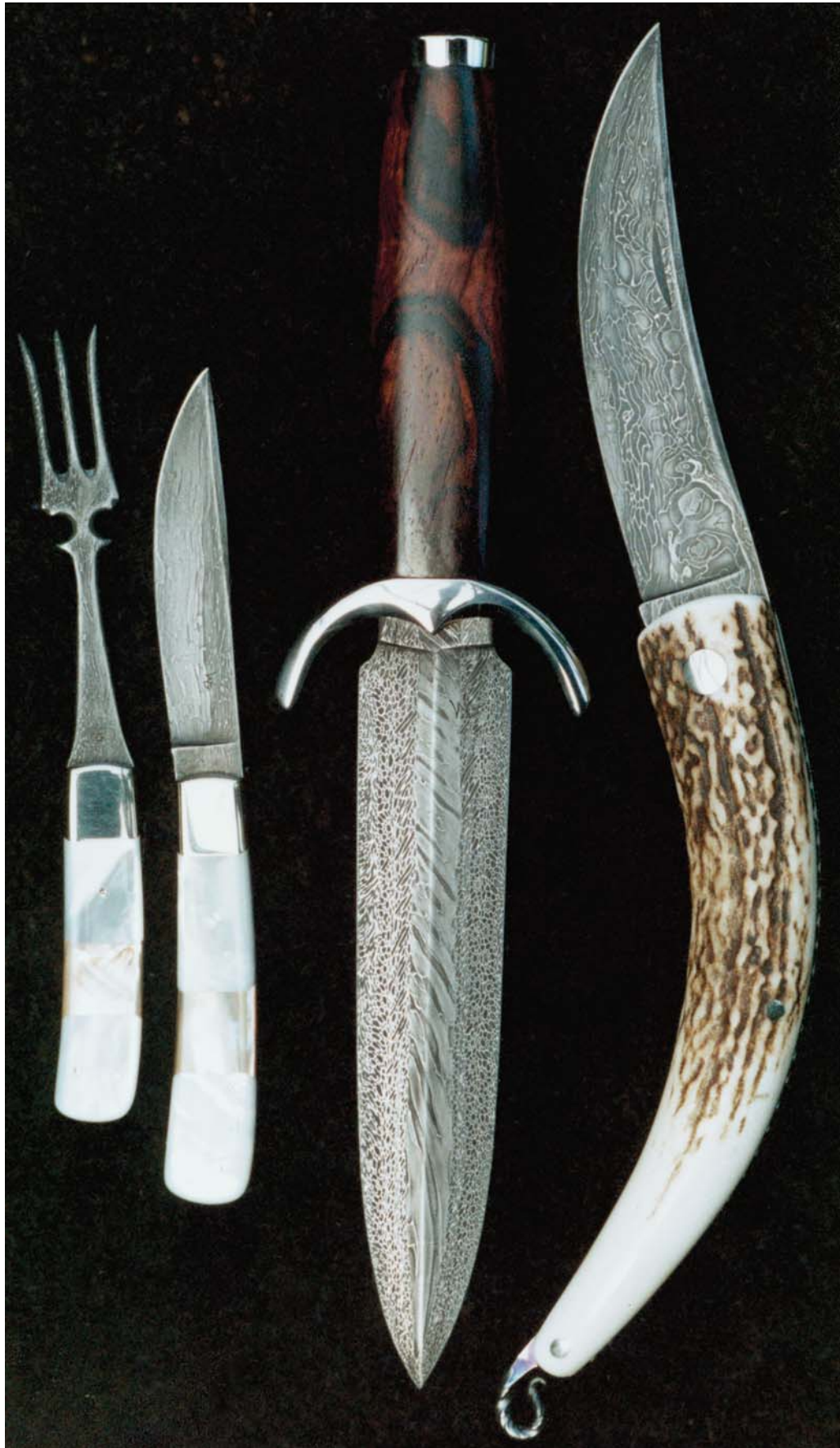
The finished dagger has three friends. The large folder has an elk brow tine for a handle, wire damascus blade. The knife and fork have wire damascus blades, pearl handles and nickel silver bolsters.
