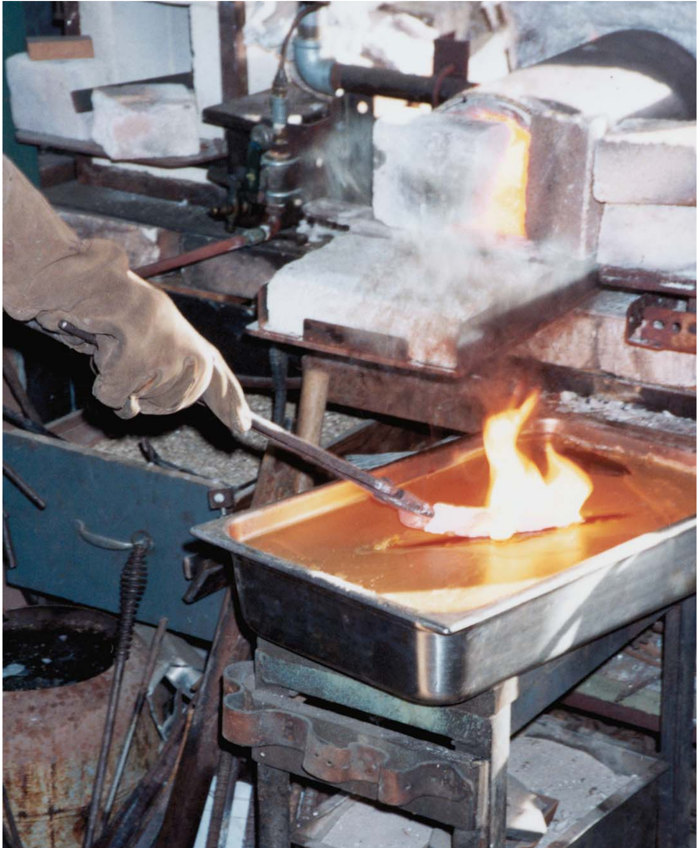
The heat treat area of the Goddard Smithy. The 10-inch blade is being quenched in the large goop pan. Note the small homemade gas forge above the goop. It's used for forging and heat-treating only. At the left of the goop is the annealing box that contains vermiculite. Under the goop is a pan full of wood ashes that are used for annealing high alloy steel types. The ashes, when preheated, will give a slower cool than the vermiculite.
