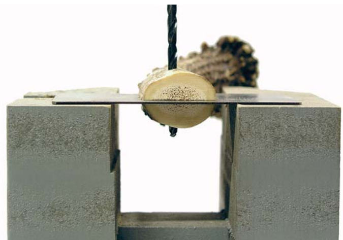
The setup for drilling the pivot hole in a slotted crown handle.
