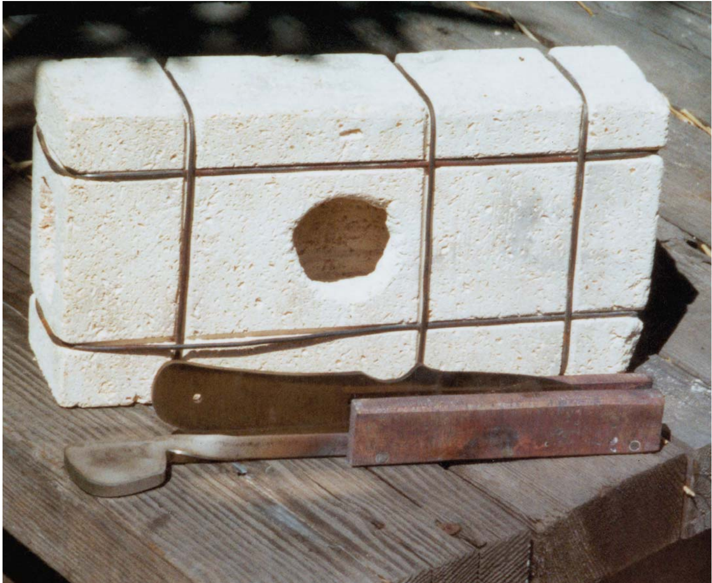
The tempering gizmo with a blade in it.
