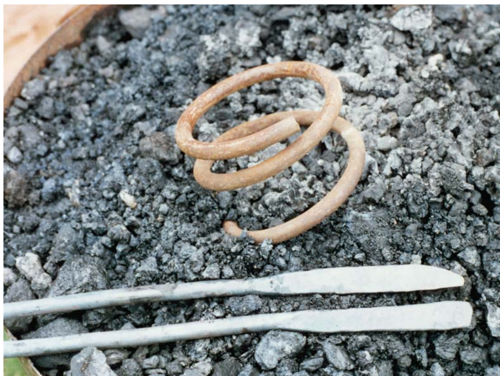
The coal forge made from a rusted out barbecue. A piece of Honda automobile spring, a flattened section on one piece, a pre-form on the other.
