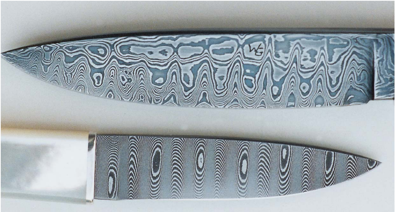
Two blades by the author. The top blade is random pattern welded at the back, incised at the edge. The bottom blade is stainless damascus made by Devin Thomas. It comes with the ladder pattern built in.
