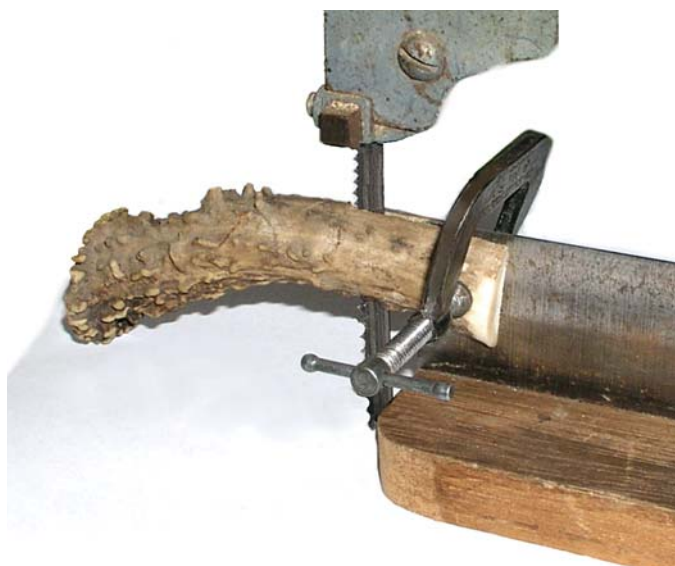
A crown handle piece clamped in the bandsaw jig and partially sawn.
