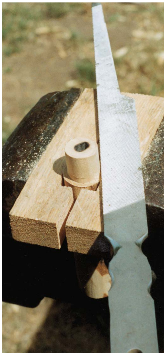
Shoulder filing jig for fitting the ferrule to the handle.
