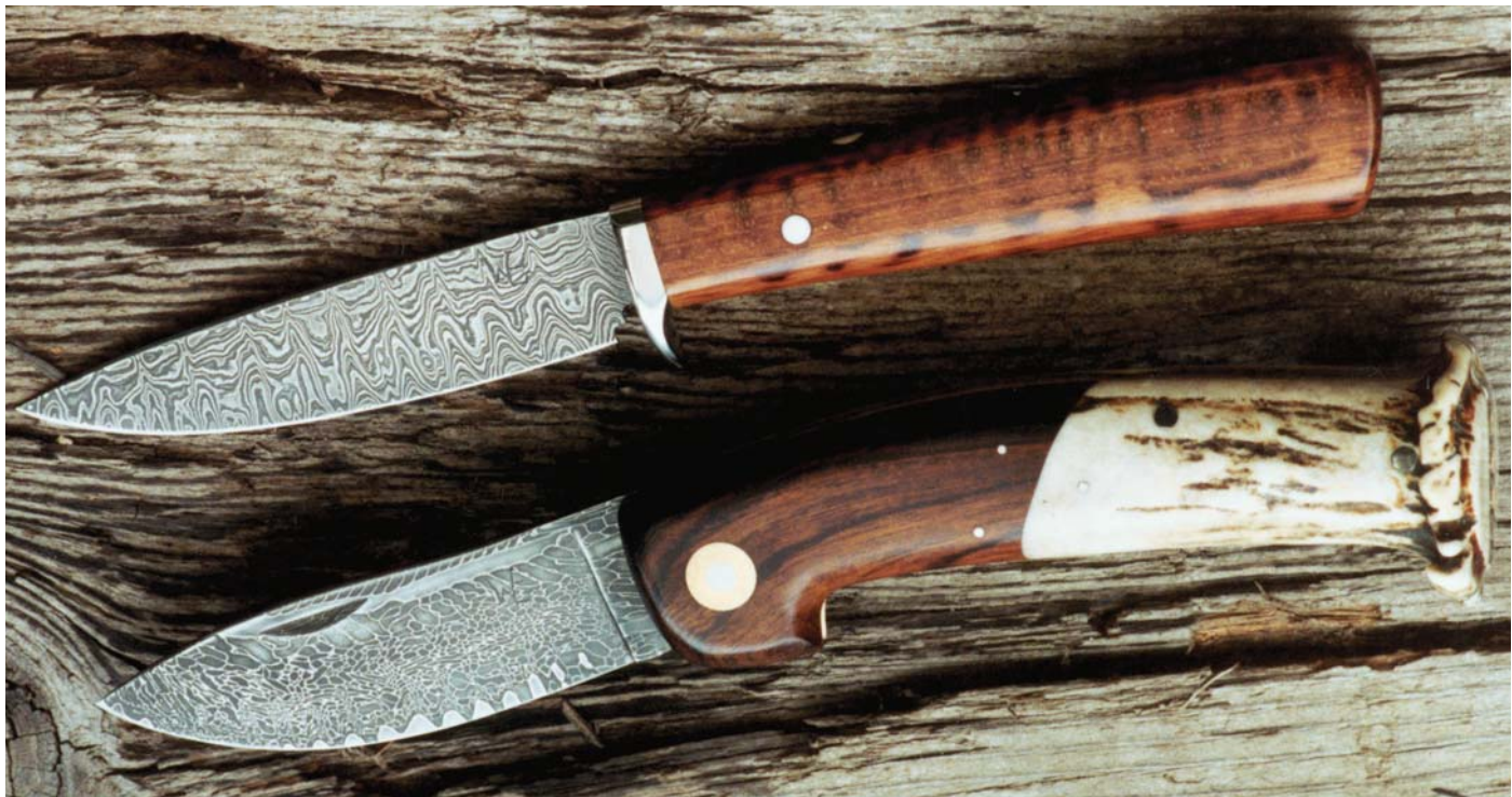
At the top a pattern-welded fixed blade exhibits a ladder pattern at the edge with a random pattern at the back. It has a snakewood handle and nickel silver guard. The folder at the bottom has a San Mai wire damascus blade, ironwood bolsters and a deer crown for a handle.
