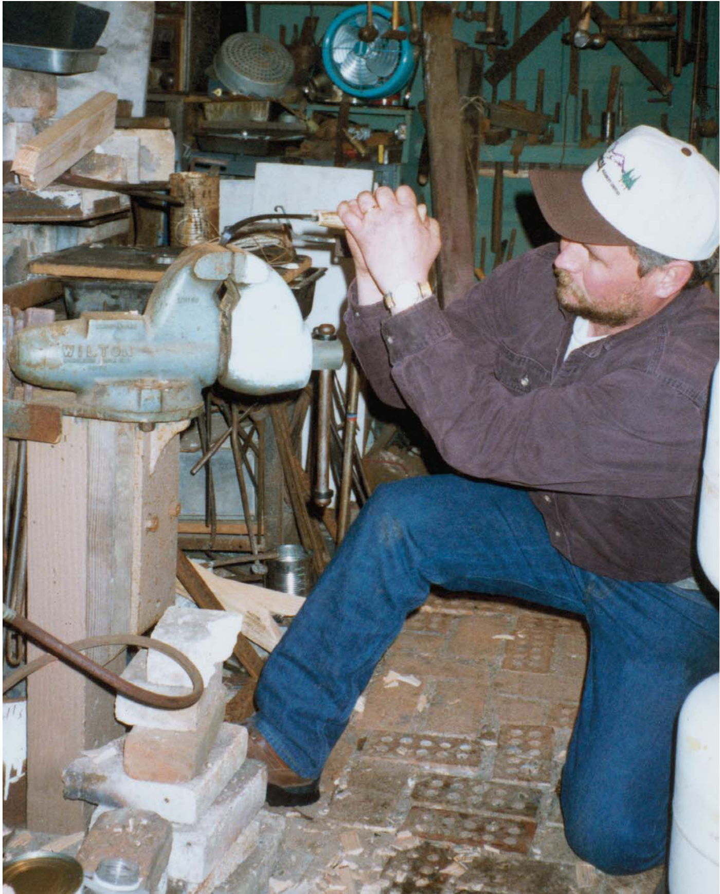
Mike Draper has passed the 90-degree flex test as part of the Journeyman Smith requirements for the American Bladesmith Society. Eye protection is always worn for the flex test; this picture was posed after the test was completed. (The Master Smith can't control the test and look through a camera lens at the same time.)
