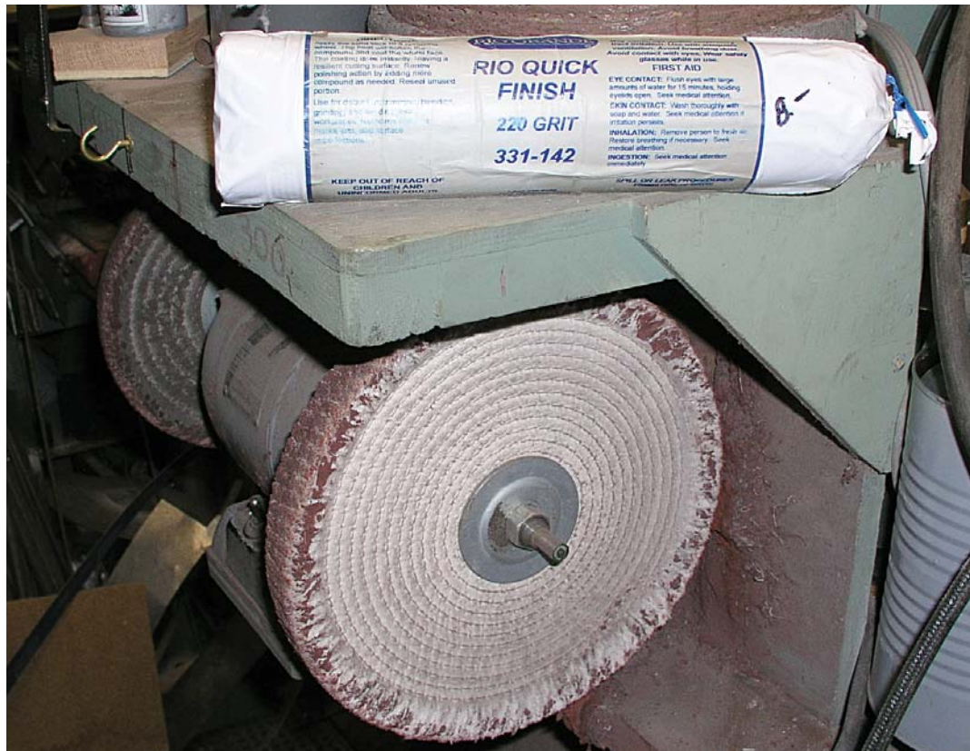
The satin finishing buffer with compound.
