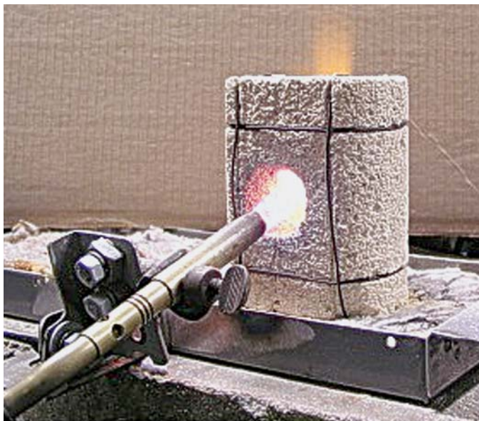
The even smaller one brick forge set upright and being used to heat small parts hung on a wire.
