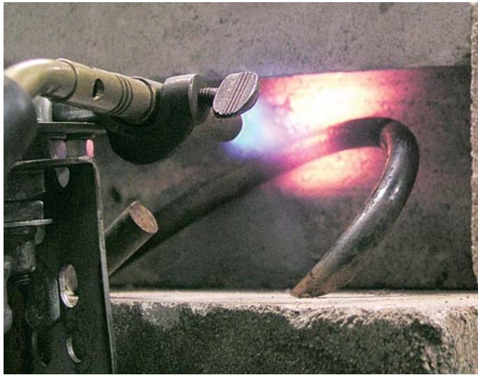
Using the side of a carved out brick to heat a section of coil spring for straightening. This is used for work that is too large to fit in the one-brick forge.
