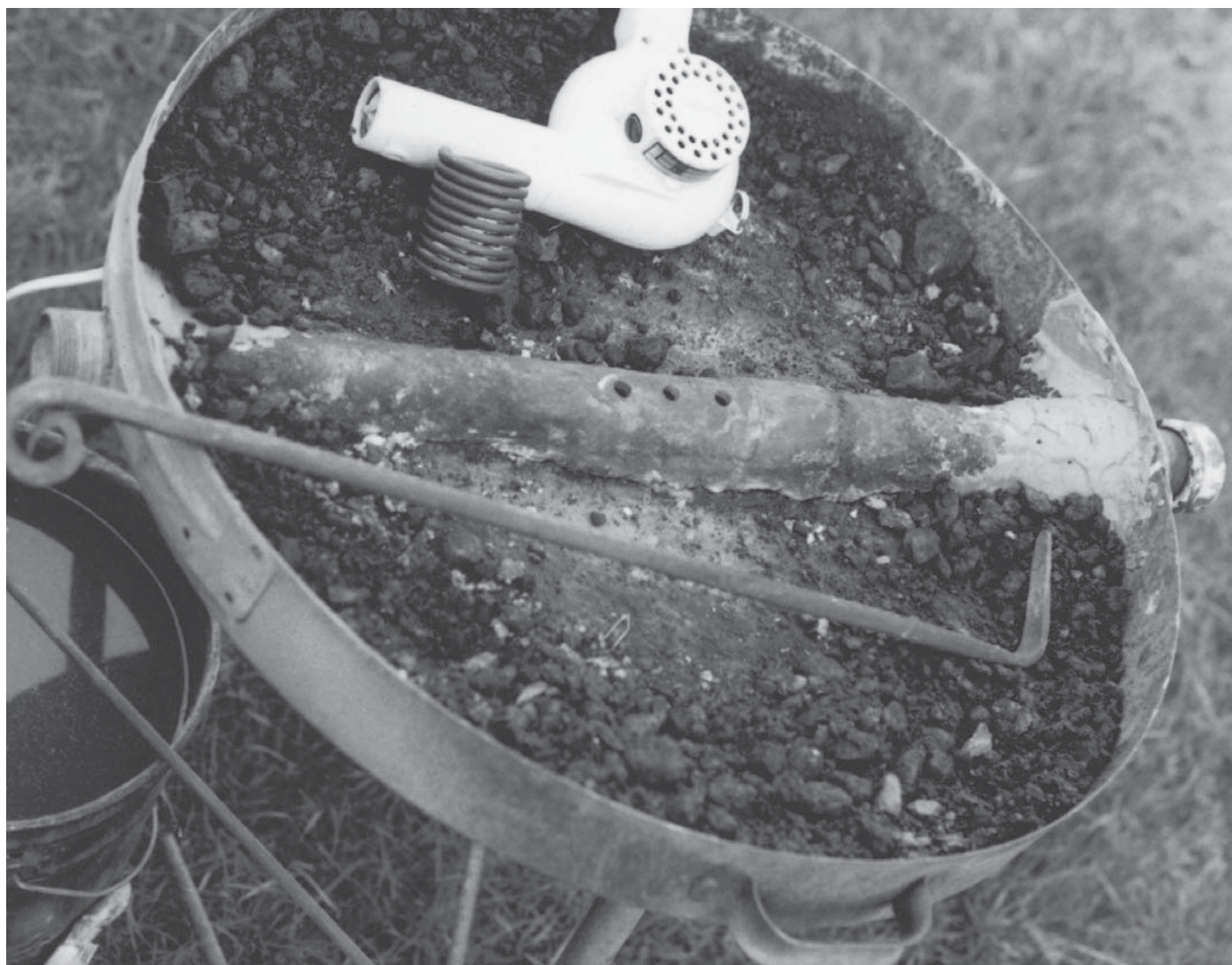
The pipe tuyère is shown as installed in the barbecue. This picture was taken before I drilled more holes in the tuyère. The “L” shaped tool is a rake for managing the coal.
