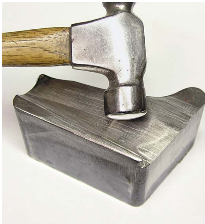
The specially shaped riveting hammer is resting on the anvil which is used to support the pin in the groove on a stag slab while the top side is being riveted. This little anvil was made out of a discarded punch-press punch.
