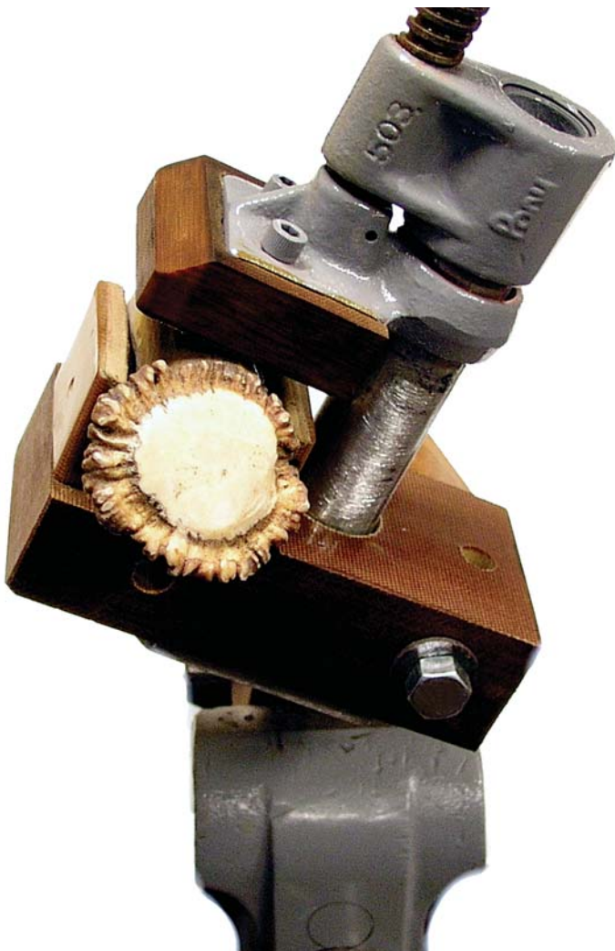
The third hand with the "V" block holding an antler crown for detailing.
