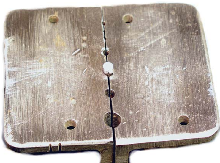
The pin stock is locked in place and ready for heading.
