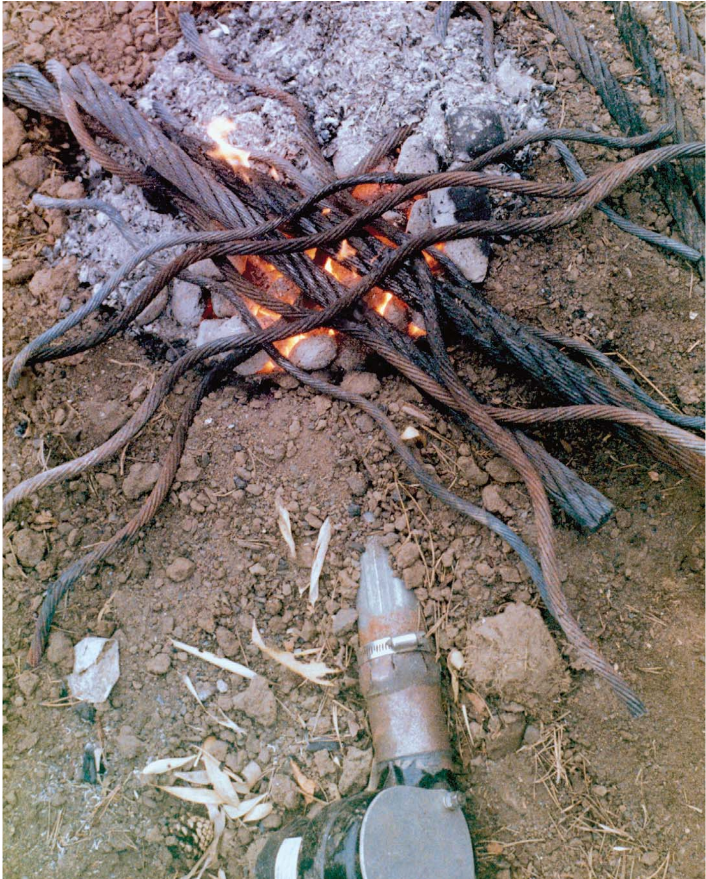
The Dirt Forge is shown using charcoal for fuel to burn the grease out of wire rope prior to forge-welding it to make wire damascus. After this picture was taken I stacked fire bricks over the top of the fire chamber and forged a blade using a hay rake tooth for material.
