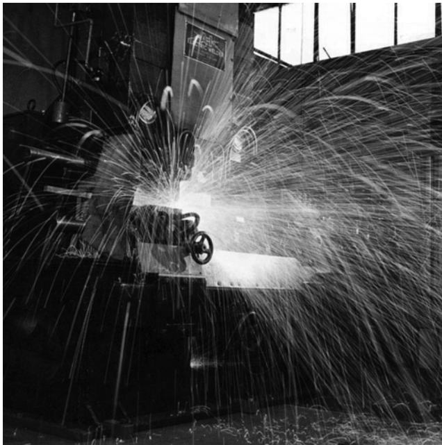
Fig. 3.11 Massive arcing and expulsion during flash welding
