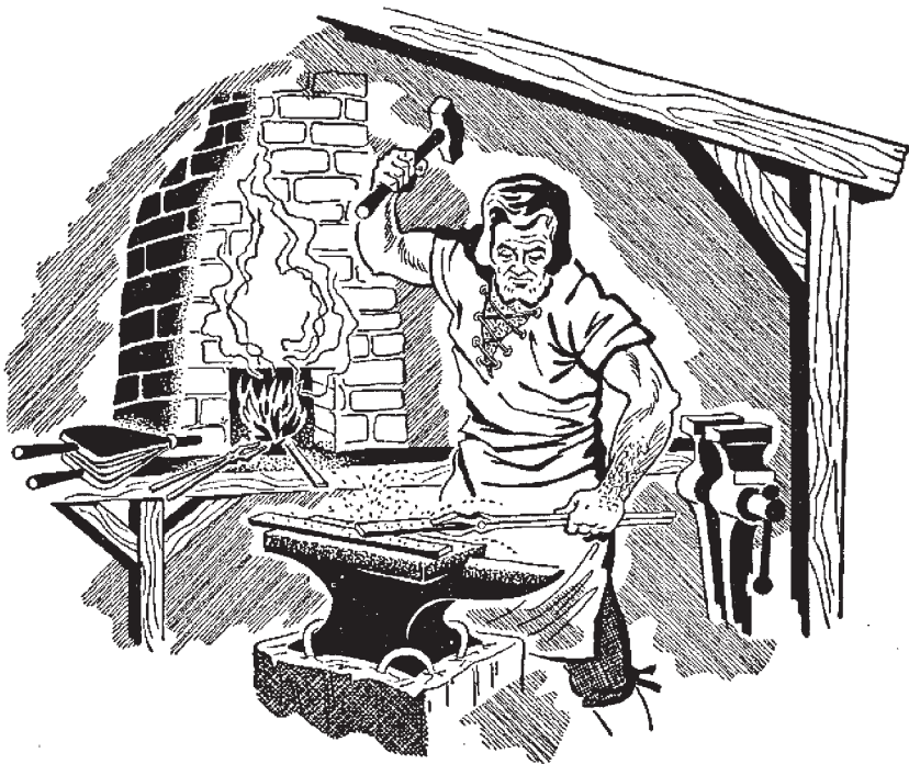
Fig. 6.5 Forging is one of the oldest crafts. From this shaping of metal by heat and hammering came the idea of forcing metal together by forge welding. Source: Ref 6.3, p 2
