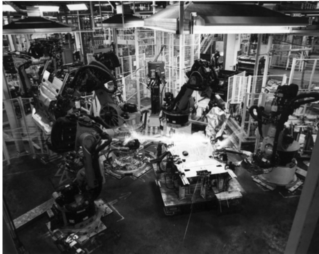
Fig. 3.1 Robot welding machines are operating in a work cell as part of an automated production line for automobiles. Multiple robots are often used to speed assembly, with each performing a different set of specific welds. Source: Ref 3.1, p 287
