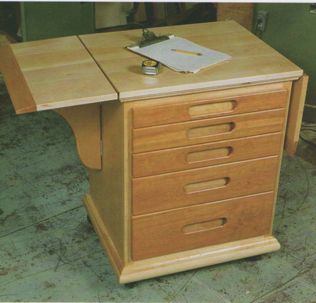
Jim Tolpin's small tool cart rolls on full swivel casters. Photo by Craig Wester.
