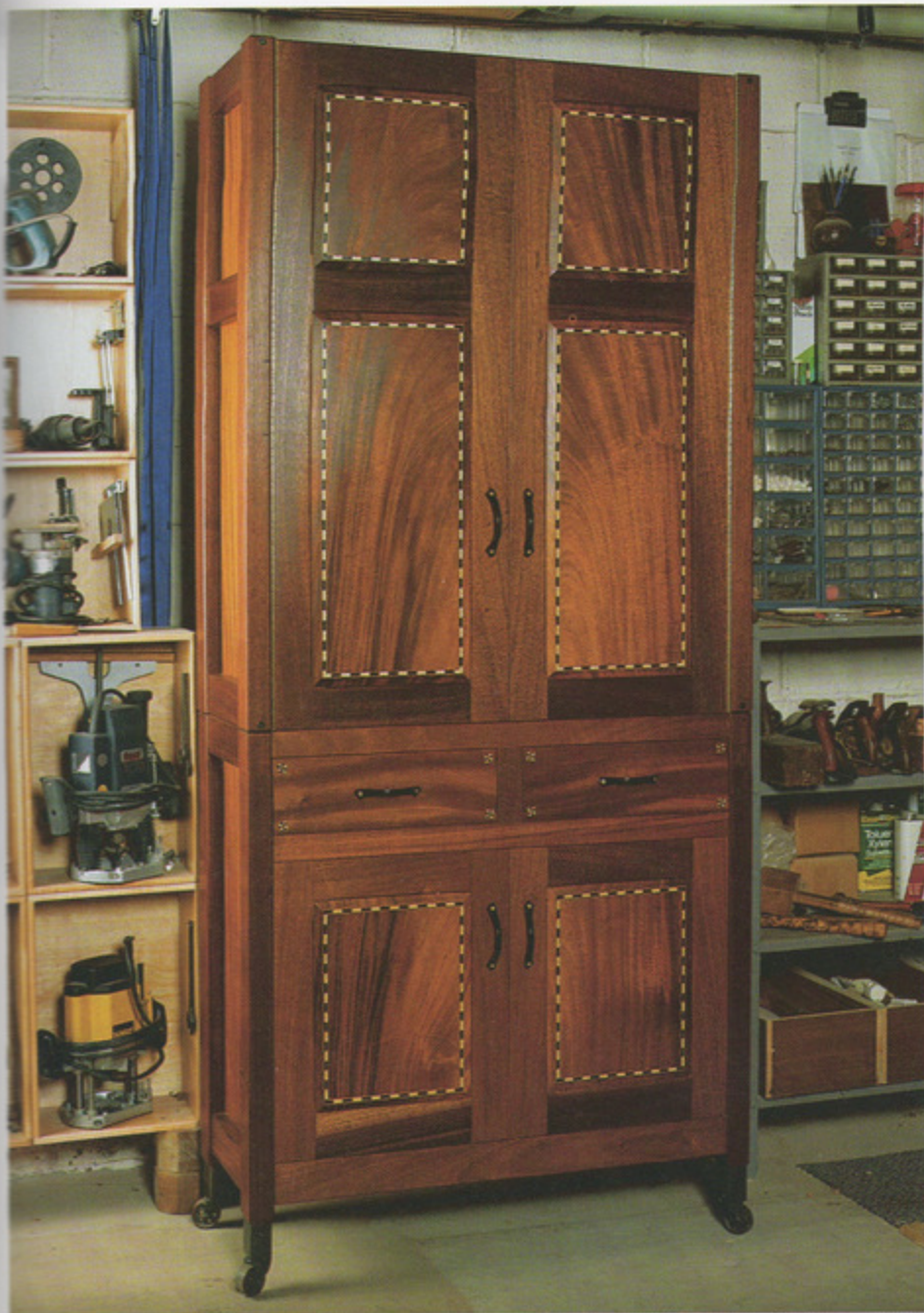
Rae's cabinet features holly and ebony inlay and ebony handles (left). The Honduras mahogany veneer on the doors is thick enough to create raised panels; the coved drawer face (above) mimics waist molding in traditional furniture designs. Photo by John Hamel.
