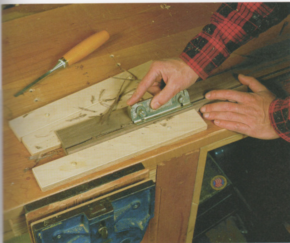
A Stanley side rabbet plane (No. 79) works a dado into a sliding dovetail groove. Konovaloff eyeballs the angle—a less experienced woodworker could make the cut with the tool held to a guide board. Photo by Craig Wester.
