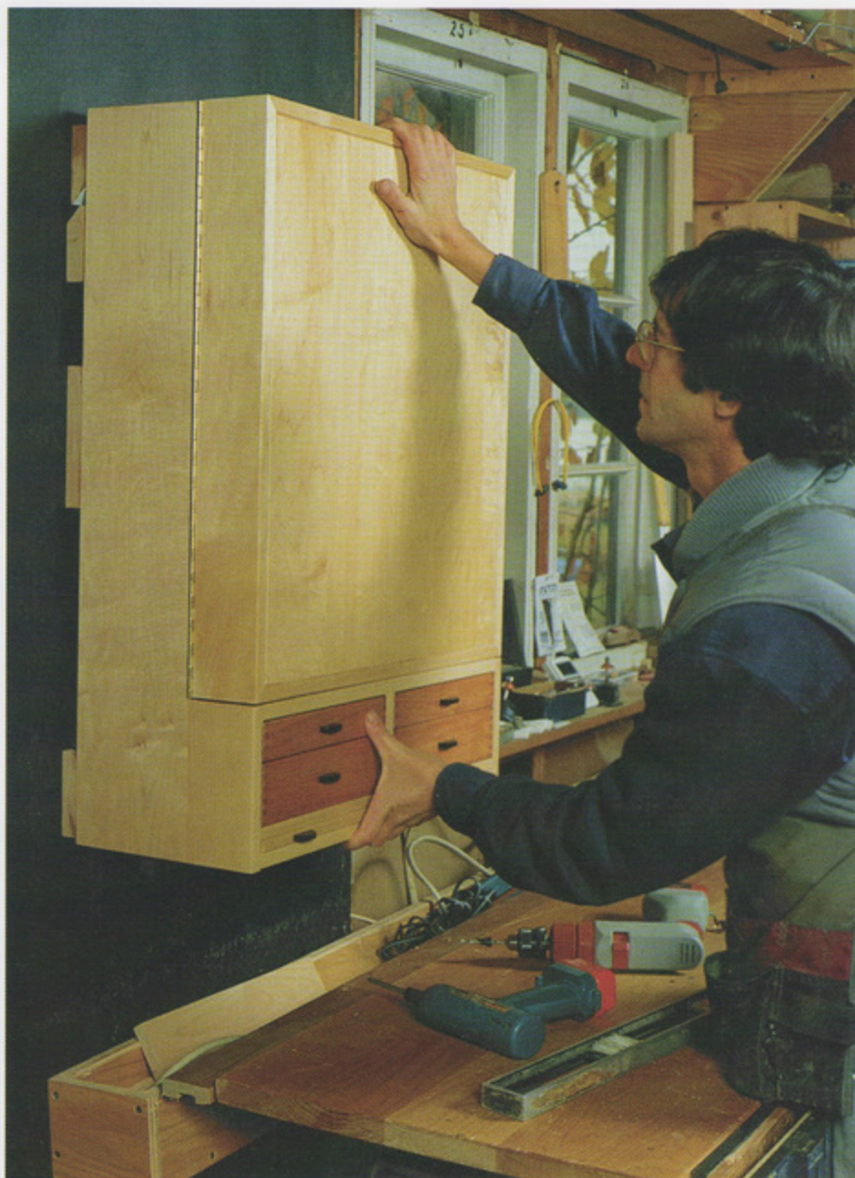
Because this cabinet hangs on angled cleats, it can easily be taken down and moved to another area of the shop. Photo by Craig Wester.
