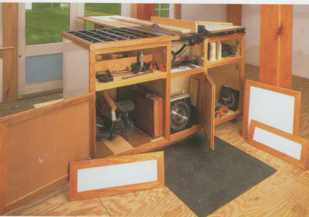
Cabinetmaker Charles Platt built this storage station around his 10-in. table saw, entirely replacing its metal stand. Making the most out of floor space that is typically wasted, he was able to create separate areas to store table-saw related tools, sawblades, power hand tools and a removable dust bin. Photo by Dick Fellows Photography.
