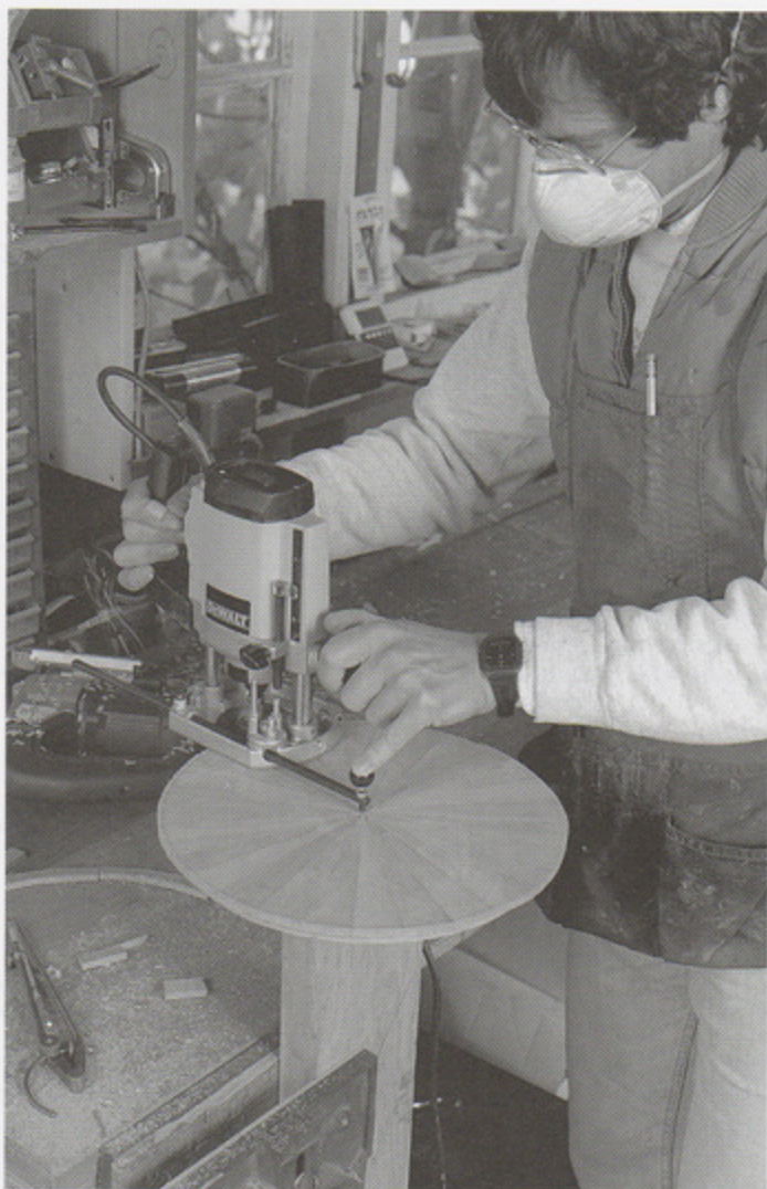
A final trim with a tram-mel-mounted router completes the fan-veneered end panel. Photo by Craig Wester.
