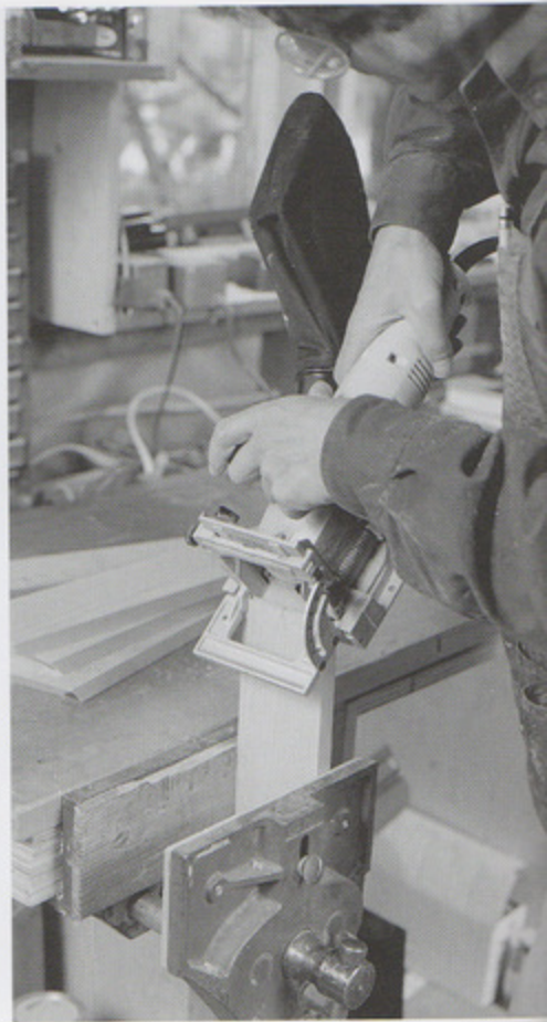
The mitered ends of the door banding are slotted with a biscuit joiner. Photo by Craig Wester.
