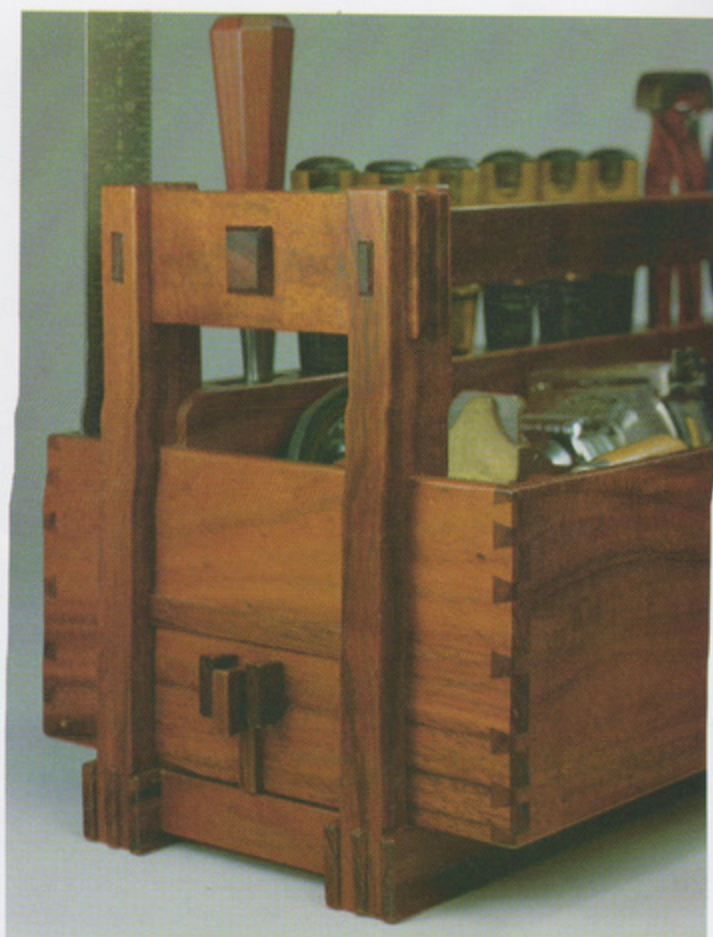
The drawer is opened and closed by means of pulls. Lifting the central sliding pull releases a retainer screw, as detailed in the drawing below. Photo by Dancing Man Imagery.
