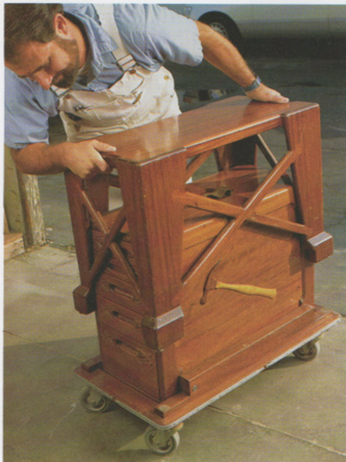
This combination toolbox/workbench by Michael Hayes rolls on a dolly. Note relief carving of hammer on box side, let-in support braces on bench. Photo by Alec Waters.
