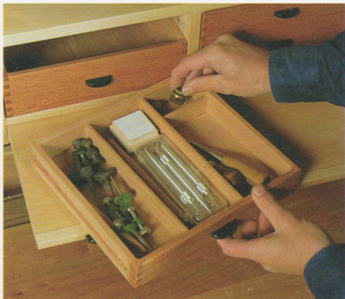
Jim Tolpin's wall-hung tool cabinet features removable drawers and a slide-out support tray. Photo by Craig Wester.
