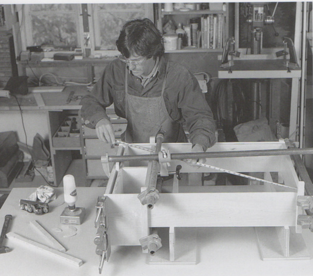
The case is glued up with the aid of leveling supports. A check of diagonal measurements ensures that the box is clamped square. Photo by Craig Wester.
