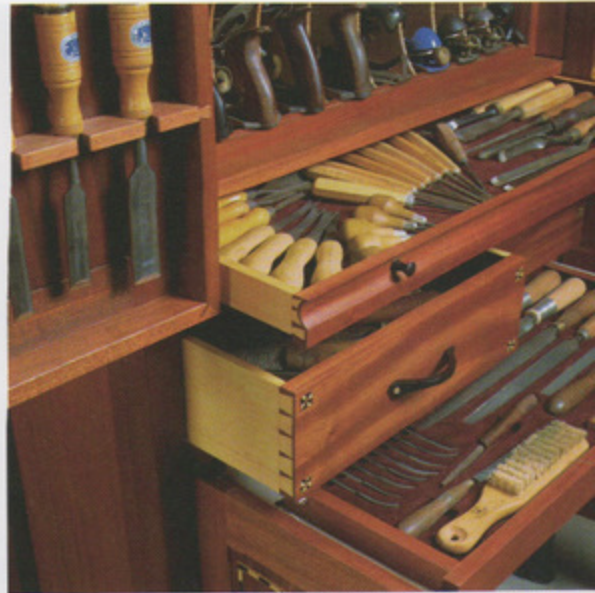
Rae's cabinet features holly and ebony inlay and ebony handles (left). The Honduras mahogany veneer on the doors is thick enough to create raised panels; the coved drawer face (above) mimics waist molding in traditional furniture designs. Photo by John Hamel.
