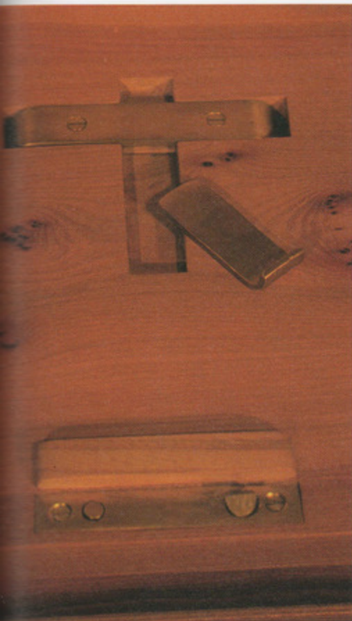
The bar-stock handle on the lower module protrudes through the floor of the upper module. A brass bar "key" slides into the recess in the floor of the upper module, locking the two modules together. Photo by Reinhold Faeth.
