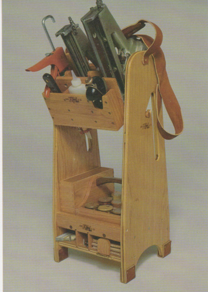
The trim-tool tote carries tools and supplies needed to install casings. It is shown here in the working position, with the compartment holding the nailers extended upwards. When the tote is stored in the van, the compartment slides down to the bottom of the slots.
