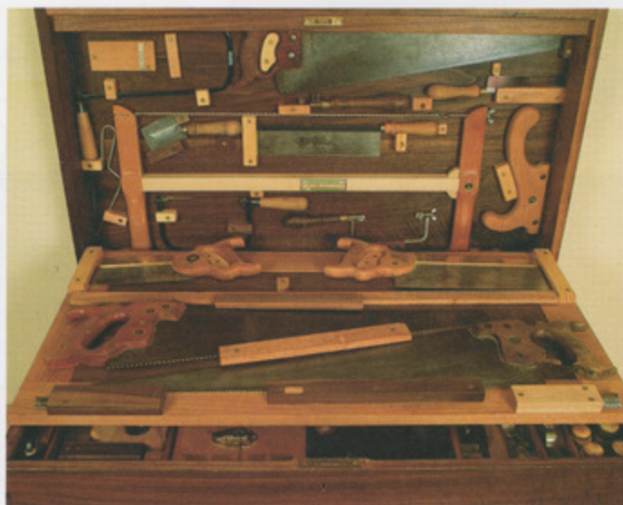
Lift-out boxes (above) hold a variety of small hand tools; note the French-fitted tray at left. The hollow lid (right) stores 15 saws. Photos by Vincent Laurence.
