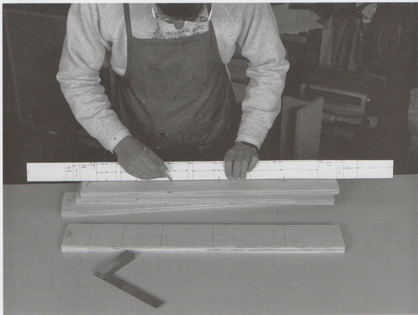
Using a story stick, mark the position of the drawer hardware along the case blocking. Photo by Craig Wester.
