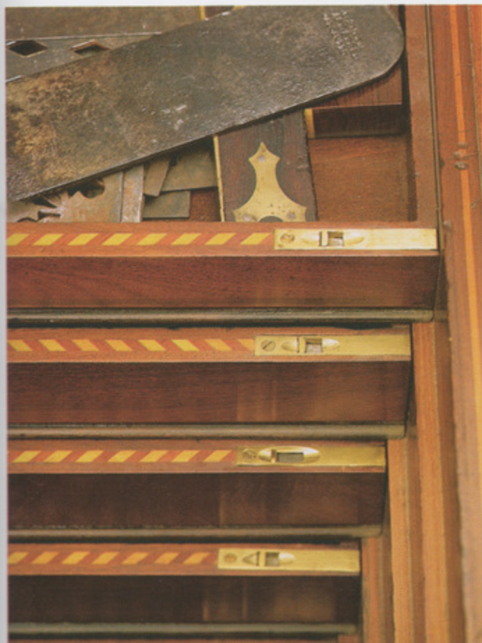
On this tool chest, sliding bolts keep the trays from opening when the chest is being transported. Toolbox courtesy of Donald Wing; photo by Vincent Laurence.
