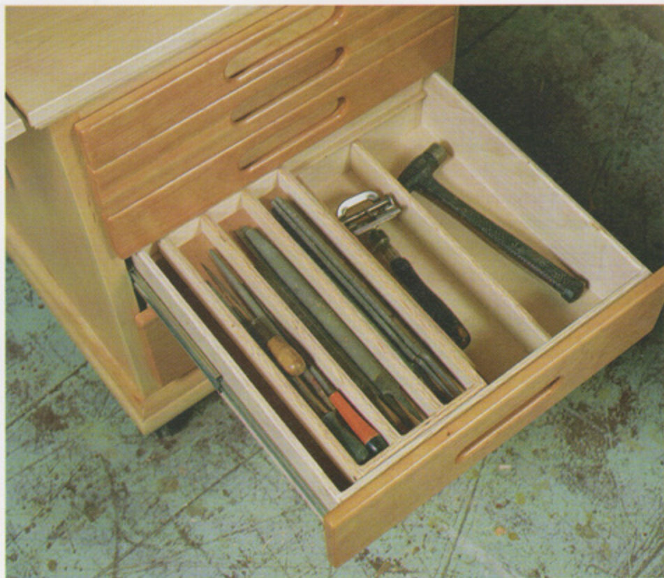
This divided drawer in Jim Tolpin's rolling tool cart has a sliding tray. Photo by Craig Wester.
