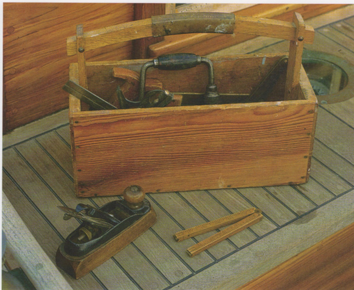
Boatbuilder and physician Bertram Levy, of Port Townsend, Wash., built this diminutive open shoulder tote to carry a task-specific selection of hand tools to his boat. The curved handle, which is wrapped in leather, helps to center the grip on the box and allows easy access to the tools. Photo by Craig Wester.
