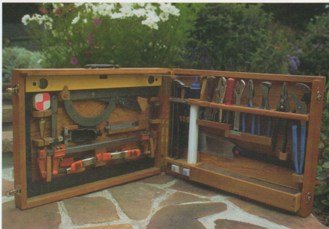
Carpenter Jeff Olson of Montara, Calif., wanted his toolbox to contain both a framing square and a 24-in. level, so he designed a briefcase-style tote. When the tote is open, all the tools within the case are easy to see and to get at. When closed, the narrow case is easily carried and stowed. Photo by Jeff Olson.
