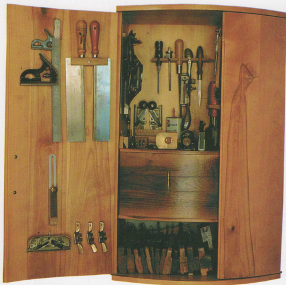
This bow-front wall-hung tool cabinet, designed and built by Garrett Hack, of Thetford Center, Vt., makes excellent use of space. Small items are in drawers at the middle of the cabinet; molding planes fill the lowermost bin, where their profiles are clearly in view; and handled tools are near the top of the cabinet on pegs or ledges. Photo by Vincent Laurence.
