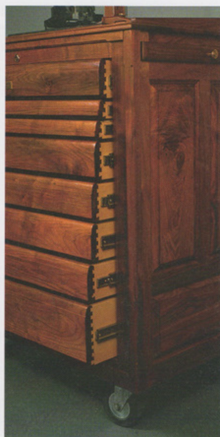
Steve Johnson's mobile cart, shown at far left with a small machinist's chest (also by Johnson), features full-extension drawers. When they are extended, the light-colored maple drawer sides stand out against the darker walnut (left), warning that the drawers should be shut before the cart is moved. Photo by Jon Binzen.
