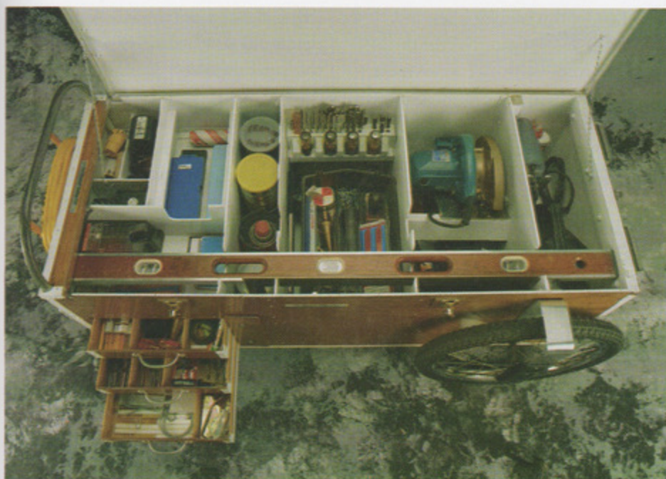
Interior partitions as high as the top of the cart keep the contents of the bins from shifting and also strengthen the case. Photo by Photomedia.
