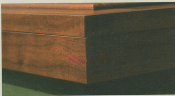
Mock-dovetail miter joints at skirt-board corners add a decorative touch when contrasting woods are used. Here, the mahogany dovetail contrasts nicely with the walnut skirting. Photo by Ray Fischer.
