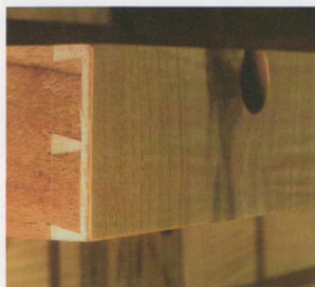
Dovetailed drawers have cut-out finger pulls. Photo by Greg Radley.
