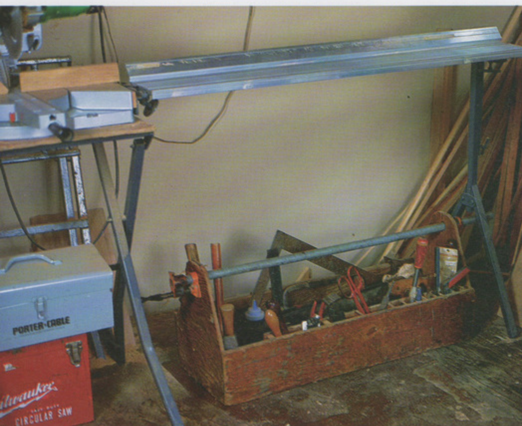
Jim Tolpin's toolbox for timber-framing tools. The side compartments contain chisels and other small carpentry tools; a slotted partition holds panel saws. A canvas cover provides a measure of protection from the elements. The original closet-pole handle has been replaced with a pipe clamp. Photo by Craig Wester.
