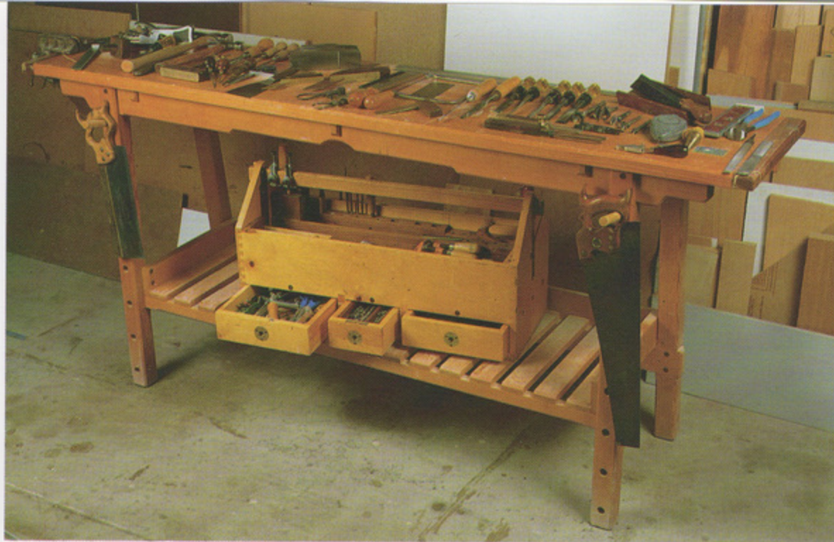
Stephen Freund built this open shoulder tote from pine, using router-made dovetail joints in the corners. Sized to fit behind the seat of his pickup truck, the box holds an impressive number of hand tools and accessories. Photo by Alec Waters.
