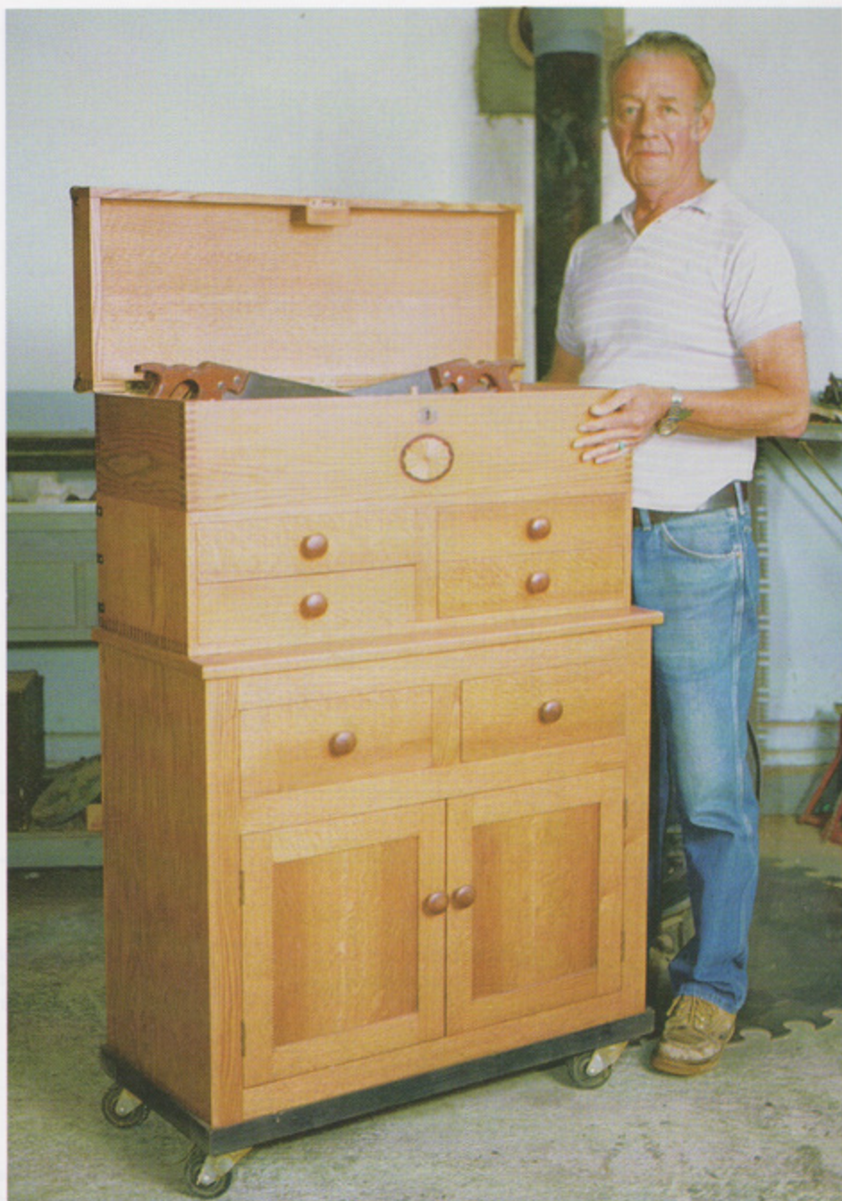
Craftsman George Snyder, of West Creek, N. J., built this rolling cart to carry his tools to work areas throughout his shop. Constructed largely of quartersawn red oak, it has solved the problem of scattered and misplaced tools. Photo by New Image Photography.
