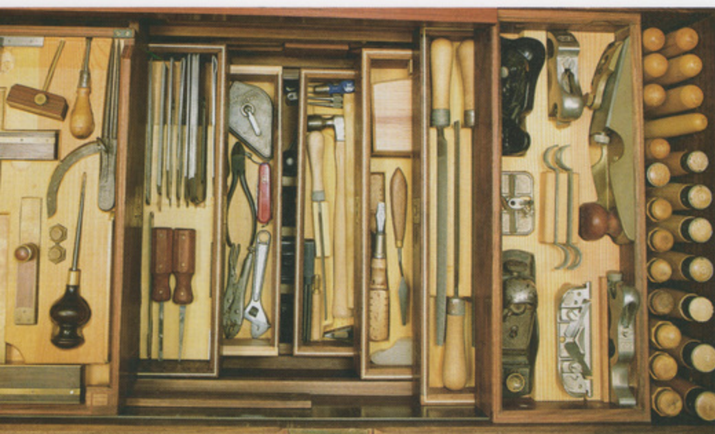
Lift-out boxes (above) hold a variety of small hand tools; note the French-fitted tray at left. The hollow lid (right) stores 15 saws. Photos by Vincent Laurence.
