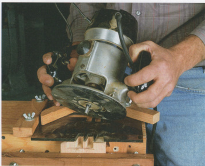
Using a shop-made jig, Winter routs dovetails on the drawer backs. Photos by Sandor Nagyszalanczy.
