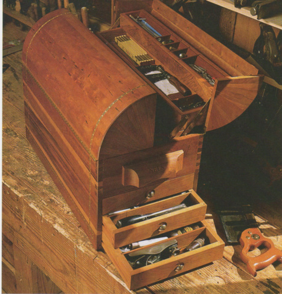
This tool tote by Mark Nels features fan veneer on its ends, swing-out trays and drawers for small tools and a well underneath for large tools. A coopered top discourages use of the box as a job-site seat. Photo by Alec Waters.
