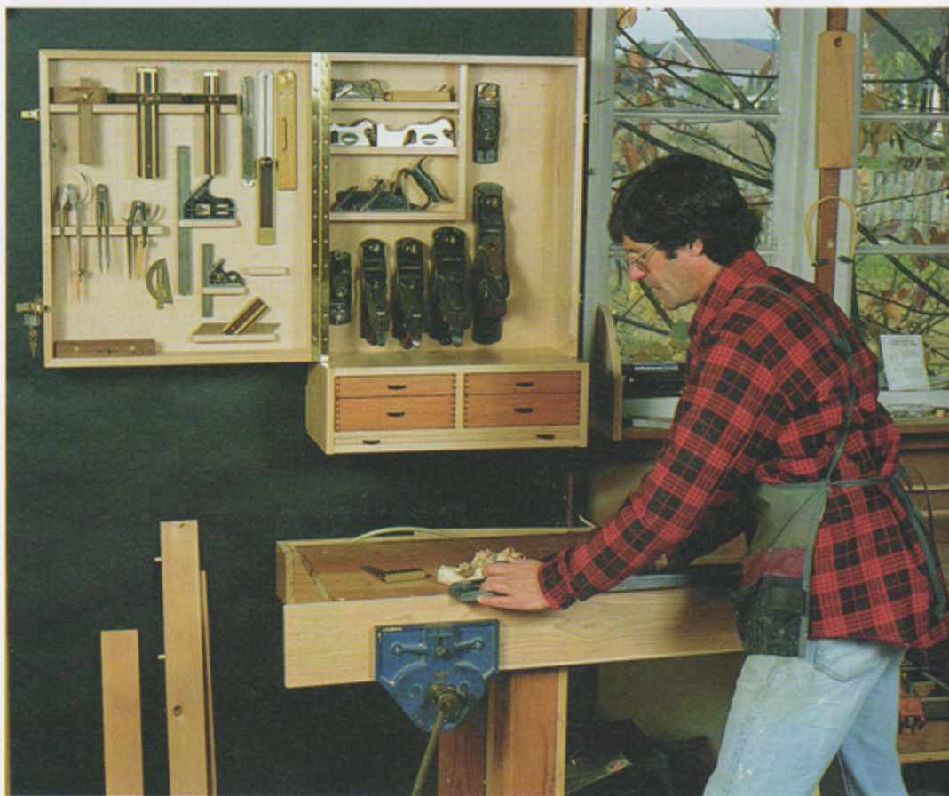
Tolpin's wall-hung tool cabinet houses tools for layout and joinery. In its location close to the vise end of the workbench, the cabinet blocks no floor space yet is only a step away from where the tools are used. Photo by Craig Wester.
