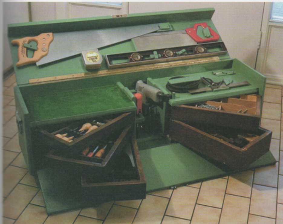
This lidded tote by furniture maker David Bevan of Gloucester, Ontario, Canada, features two movable lids—a top lid containing a pair of saws, a tape and a level, and a drop-front lid that opens to reveal a small open tool well and banks of pivoting drawers. Photo by David Bevan.
