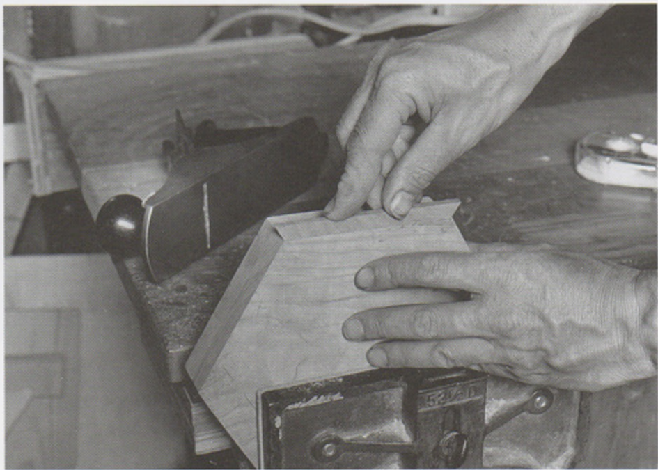
With the end patterns temporarily taped together, plane the facets (left), checking frequently against a test block (below). Photo by Craig Wester.
