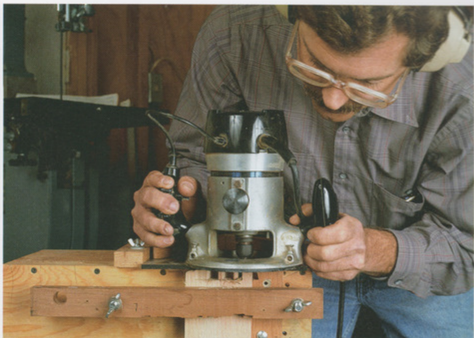
Using a shop-made jig, Winter routs dovetails on the drawer backs. Photos by Sandor Nagyszalanczy.
