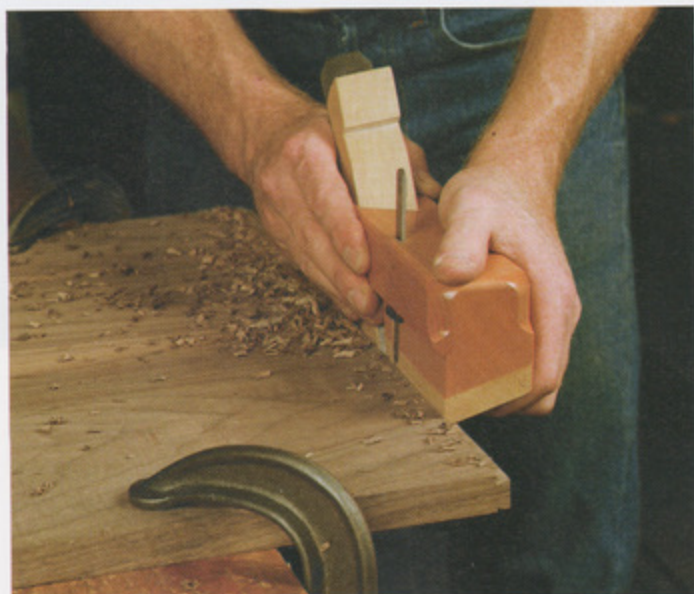
An Ulmia dovetail plane cuts the sliding dovetail on the end of the lid board. Sliding dovetails allow the plank of the lid to shrink and expand without splitting. Photo by Gary Weisenburger.
