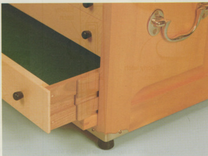
All-wood slides allow the drawers to extend fully for full access. Photo by Charley Robinson.
