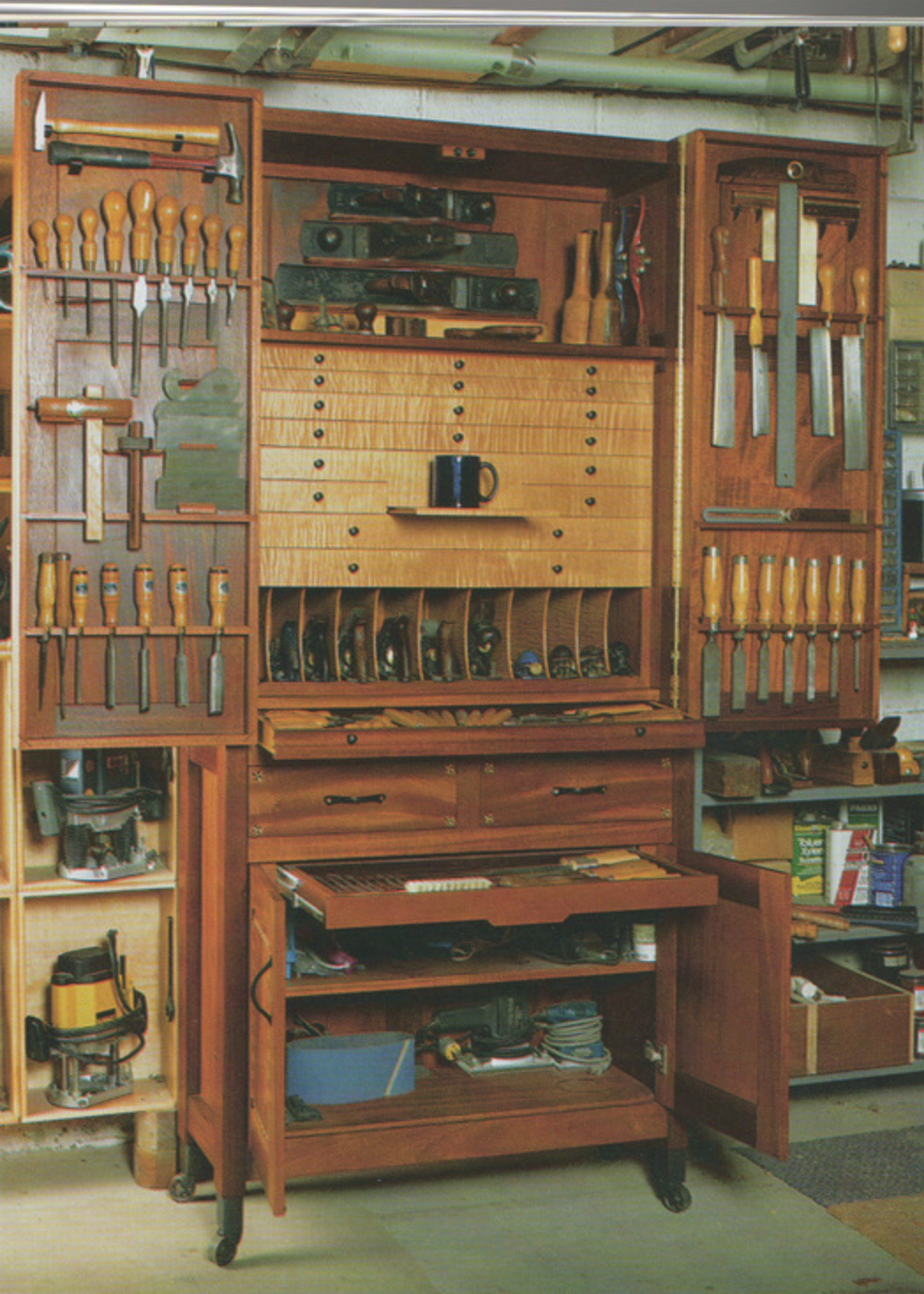
Andy Rae's tool cabinet is 7 ft. tall, 6 ft. wide (with doors opened) and 1½ ft. deep. It is built of Honduras mahogany, tiger maple and birch plywood. Photo by John Hamel.
