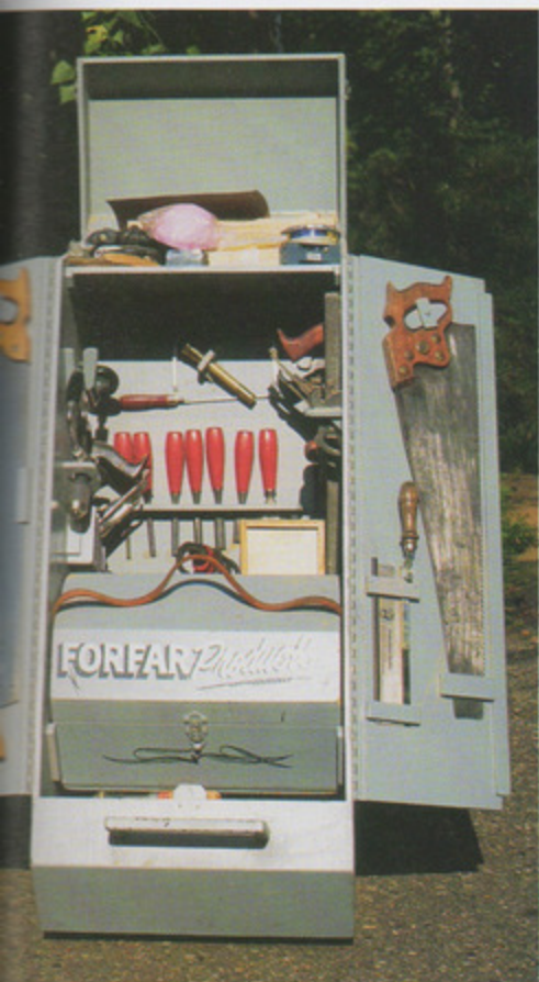
This rolling toolbox by Louis Plourd tilts on end to open. Plywood panels wrap around an interior frame of steel tubing, forming a strong, weatherproof skin. Photos by Forfar Products.
