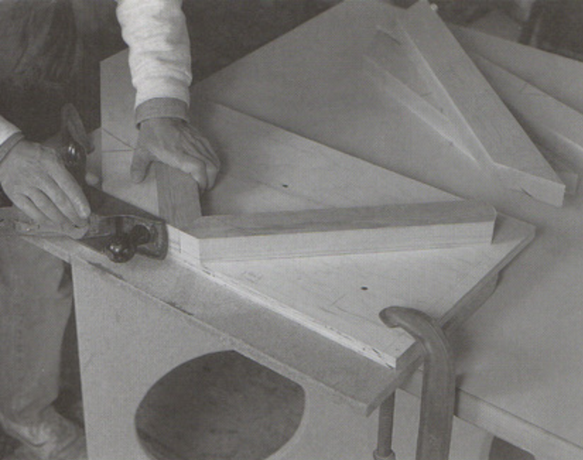
Plane the miter joint to fit by trimming its face on a shooting board. Photo by Craig Wester.
