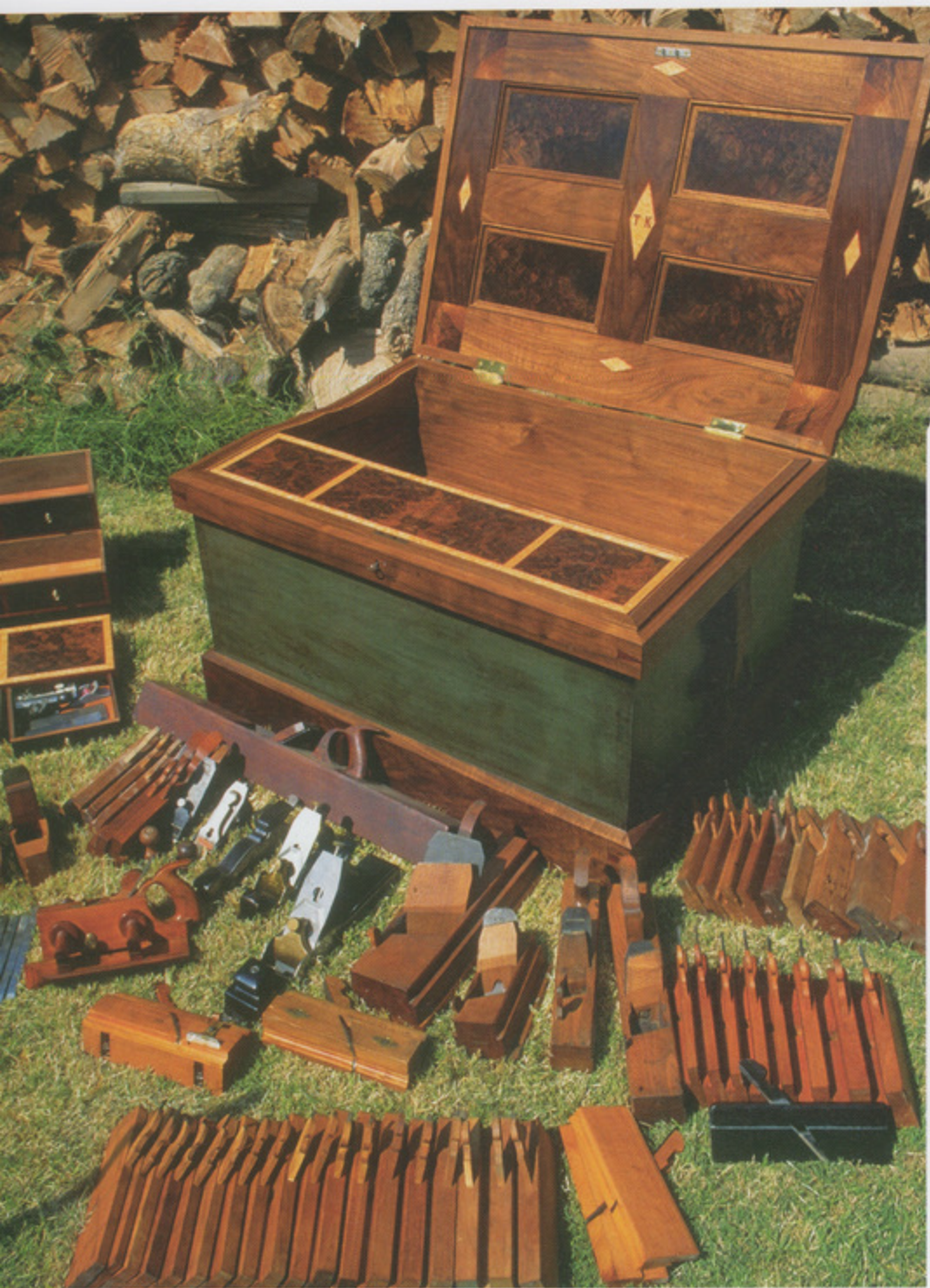
Tim Kimack's tool chest features extensive inlays, crotch walnut veneer and a sliding drawer till. Photo by Ray Fischer.
