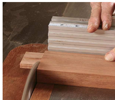
Remove the tenon altogether. Cut off the tenon at the shoulder.
