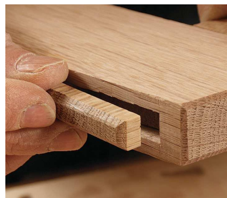
Top it off. Trim back the damaged tenon, then glue in the cap over the tenon for a seamless repair.
