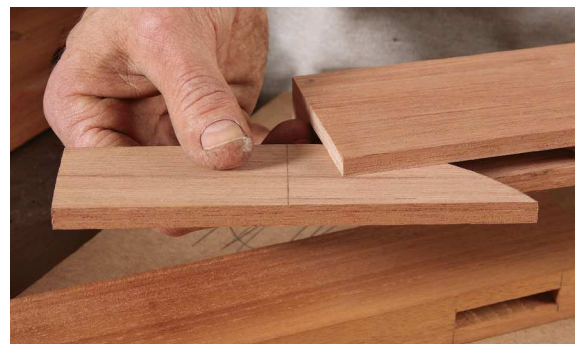
Curved piece fits right in. Mill a slip tenon for a snug fit in the groove, with one end curved to match the arc of the blade. You can use the blade to trace the arc.
