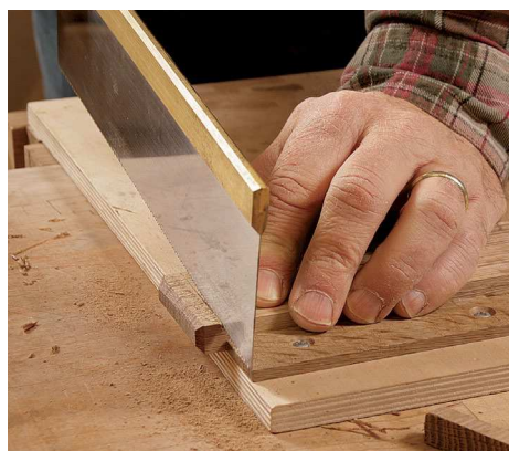
Make a cap. Mill a slip tenon for a snug fit in the outside of the mortise. Then cut off a piece long enough to meet the end of the real tenon.
