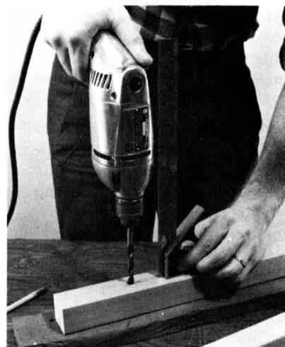
Combination square helps line up the drill when holes must be straight.
