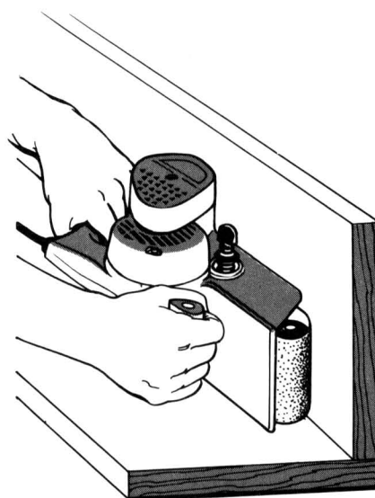
Belt sander provides the fastest sanding. It must be used in line with grain.
