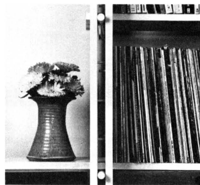
Small pegs fitted between vertical 1 by 4s support \frac{3}{4} " dowels; the dowels in turn support the 1 by 10 shelves.
