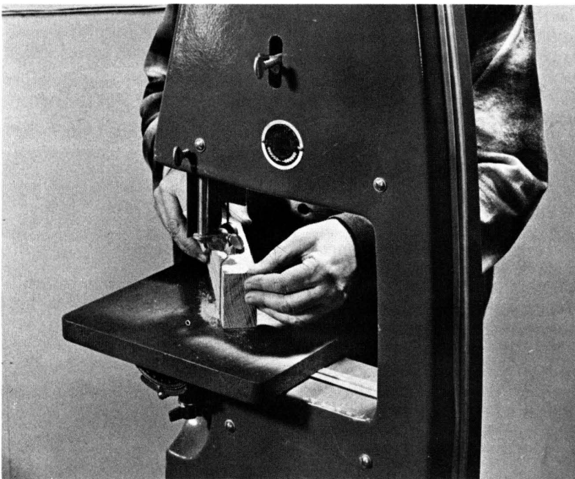
Bandsaw is a powerful, freestanding curve cutter. You push wood into blade.
