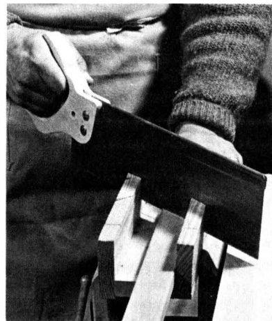
Backsaw in inexpensive miter box makes easy and accurate 45° and 90° cuts across small-dimension lumber.
