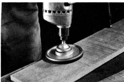
Disc sander smooths wood quickly. The disc attaches to shaft with a ball joint, allowing disc to lie flat.
