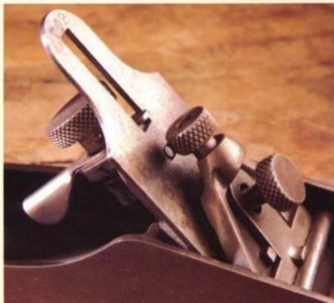
Sargent's VBM (Very Best Made) "auto-set" adjuster has a knurled nut that adjusts the depth of the cut and a large lever for lateral alignment.
