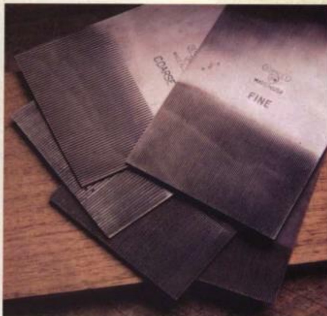
Toothing blades, finely serrated like saw teeth, have traditionally been used in scrapers for roughing the surfaces of the veneer and ground for a better glue bond, but they are also useful for leveling highly figured and ornery woods.
