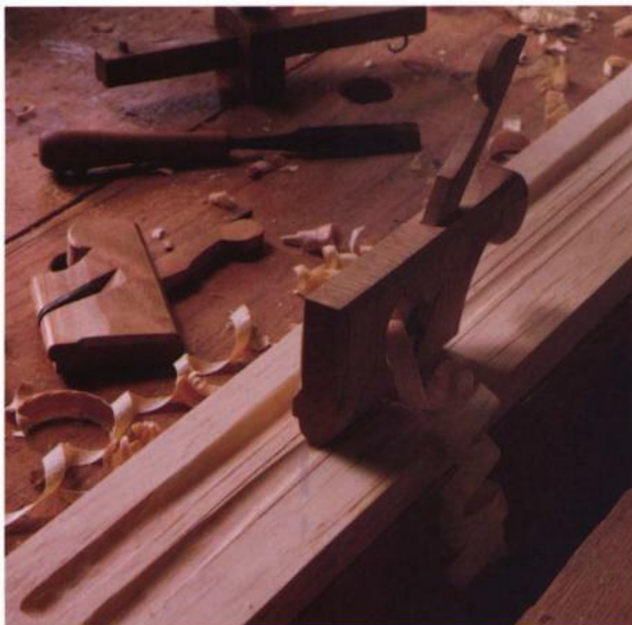
To cut a decorative flute, the curved stopped end is first cut out with a gouge and then the flute is cut along pencil layout lines. The fluting plane cuts straighter as it cuts deeper and stops when the depth stop cut into the sole contacts the surface.
