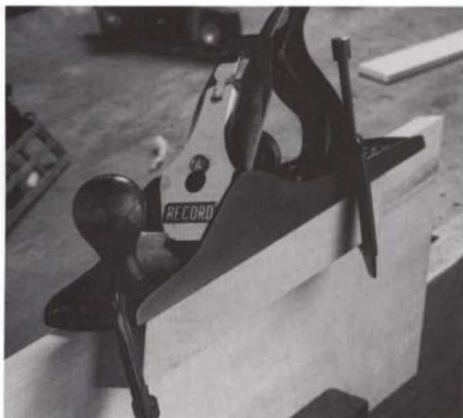
A beveled block of wood clamped to a bench plane serves as a simple jointer gauge.
