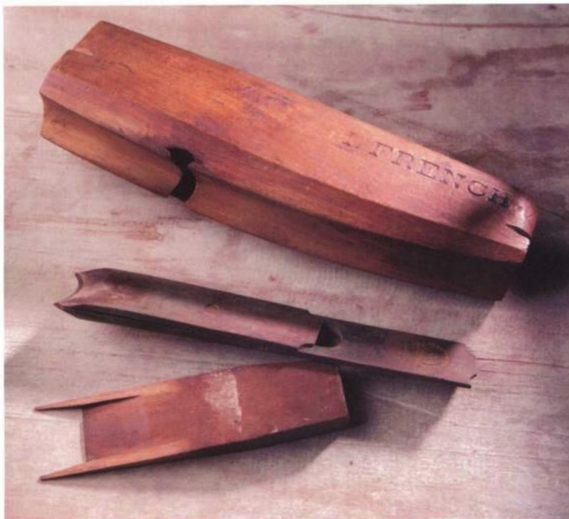
The introduction of the double iron, as on this unusual molding plane for heavy work, was a major development in the history of plane design.
