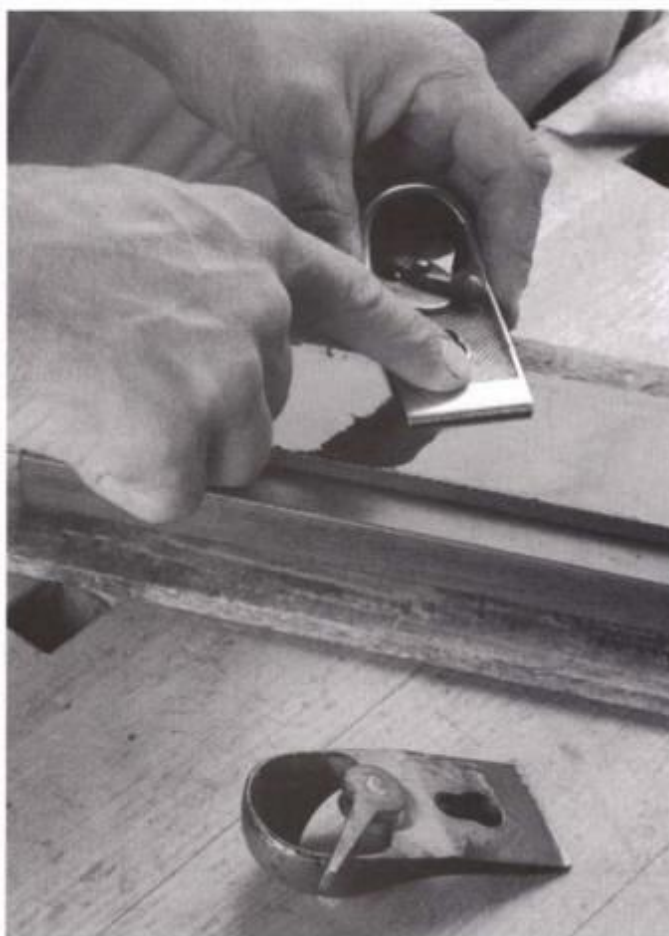
Tune a block-plane lever cap by flattening the underside of the leading edge on a coarse stone. The top edge should be polished smooth.
