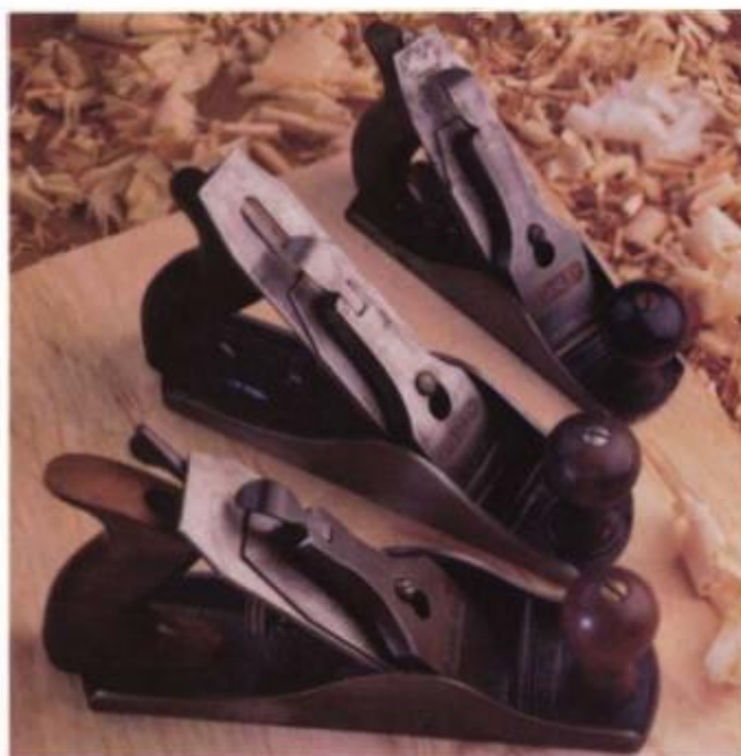
Common bench planes such as the #2, #3, and #4 shown here (from rear) have identical adjusters, rear handles, lever caps, and body shaping.
