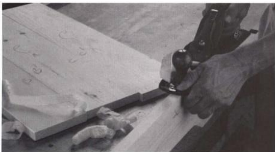
To joint boards for edge gluing, lay them out in order, mark the joints, and then joint each edge.
