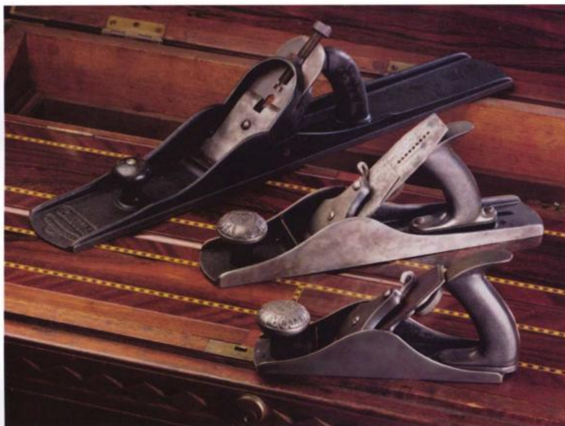
The Stanley #1 (atop the box) is the smallest and most rare of the bench planes. Competitors such as the Union Manufacturing Co., of New Britain, Connecticut, made a similar-sized plane, a #0 (foreground). The Stanley #4 1/2 in the background gives a sense of their tiny size.
