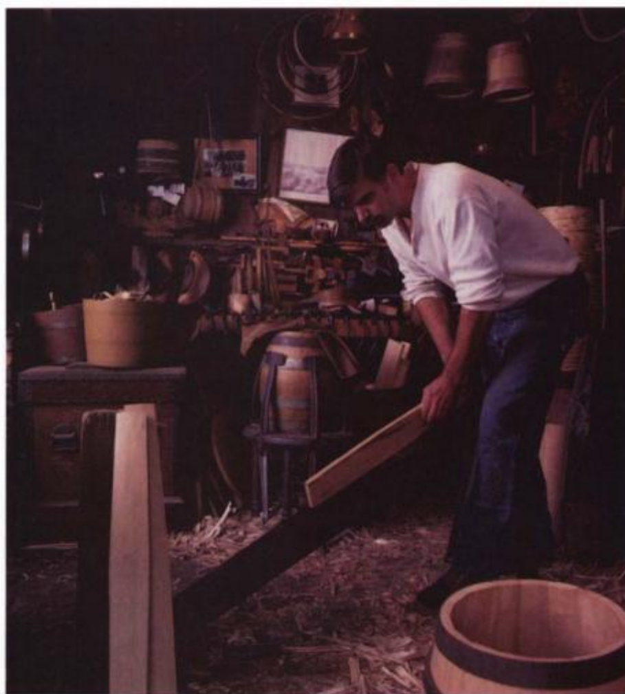
Ron Raisells, the cooper at Strawberry Banke Museum in Portsmouth, New Hampshire, shapes white-oak barrel staves on a long and heavy cast-iron jointer plane. This is the way coopers have always done it, trusting their hand and eye to get the taper and bevel right.
