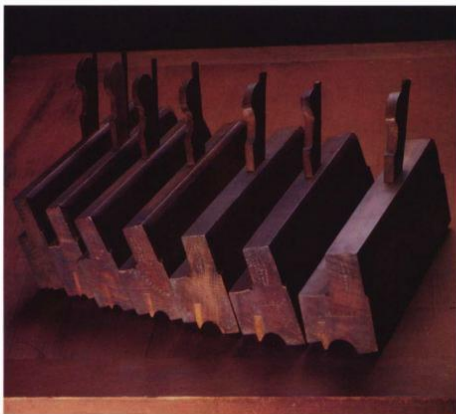
A complete set of high-quality side bead planes such as this one by E. Preston cuts beads from \frac{1}{8} in. to 1 in. wide or larger. The light-colored wood set into the narrow part of the sole that rides in the quirk is tough boxwood capable of holding up to the wear.
