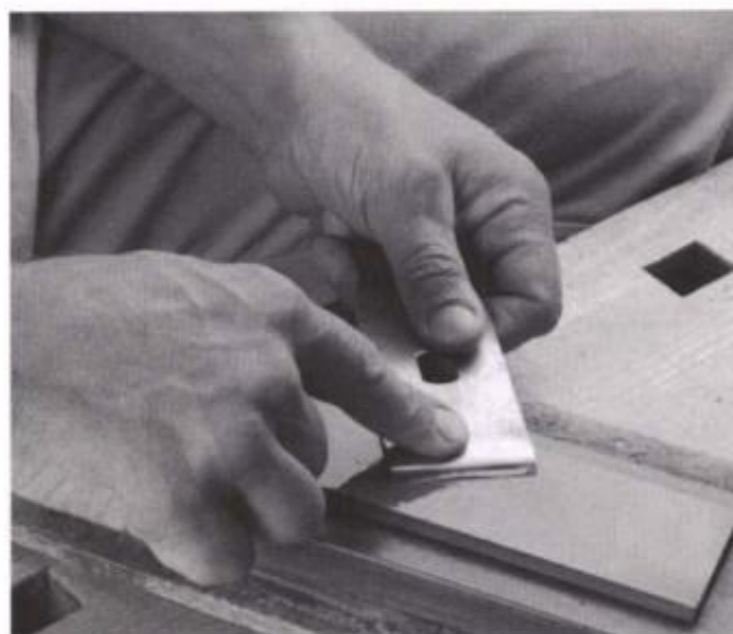
Hone the underside of the leading edge of a cap iron on a medium-grit stone, keeping the other end of the iron slightly lower than the surface of the stone.
