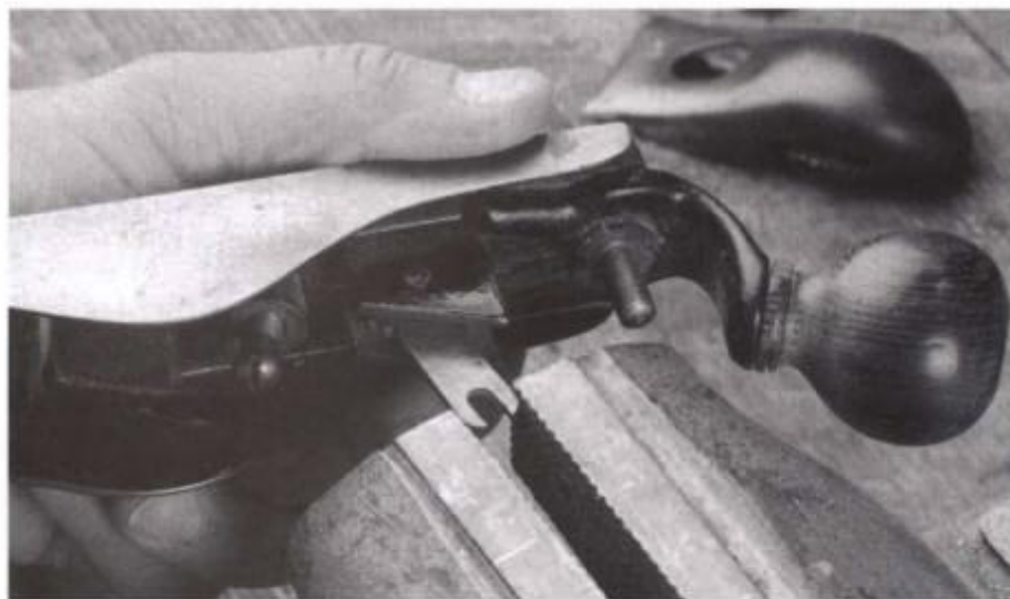
To take out any backlash or slop in the depth adjuster on a block plane, pinch the adjuster lever with a vise or pliers until it just fits the adjuster wheel.
