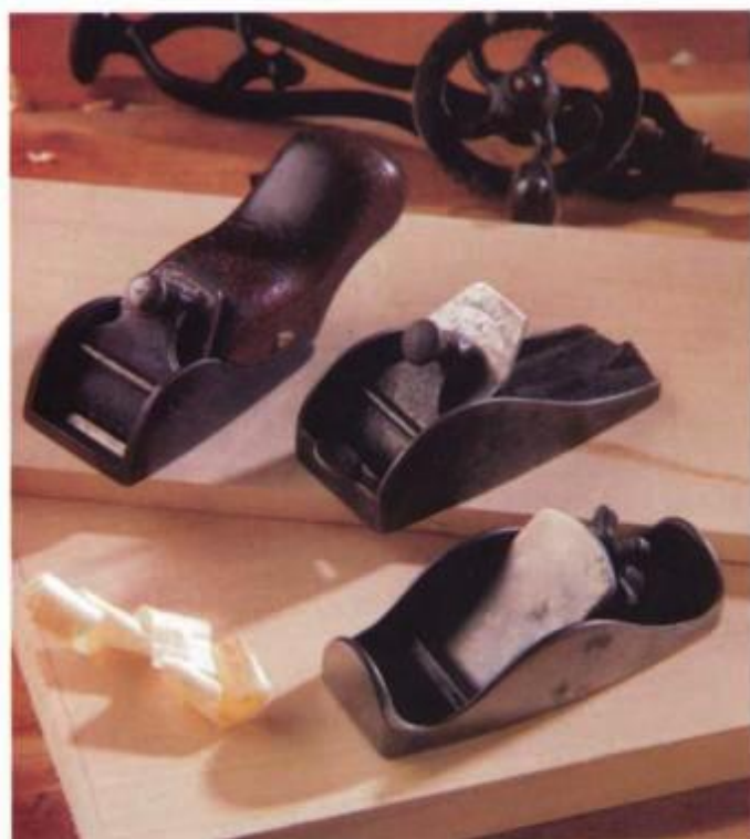
The simplest "handle" is a comfortably shaped plane body. The Little Victor (foreground) and the Stanley #101 1/2 (center) are held by two or three fingers alone. The owner-made handle added to the Stanley #101 bullnose plane (rear) provides a place to rest the palm for added control.
