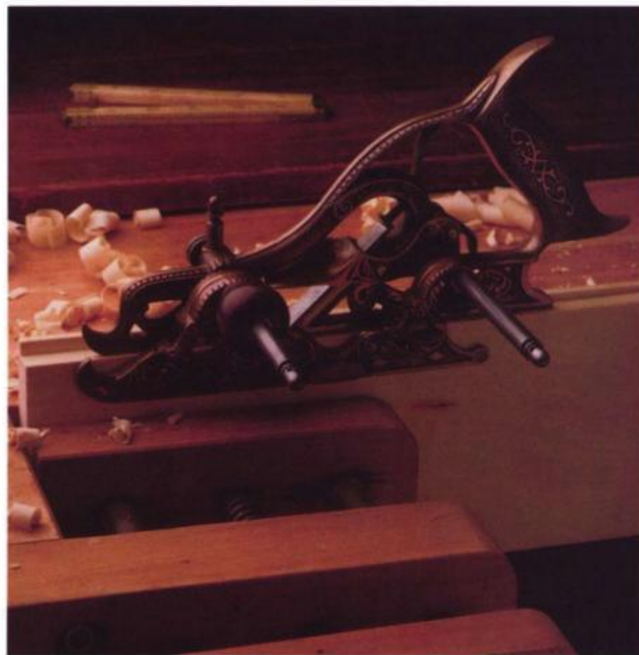
This Miller's Improved Joiner's plow plane by Stanley Rule and Level, 1872, is an extremely rare early combination plane. The castings were adorned with beautiful floral decoration to increase the appeal.
