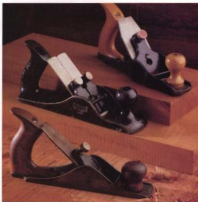
Scrub planes are the hardest-working bench planes. Shown here (from rear) are a Stanley #340 furring plane with minimal sole for "cleaning" rough boards; a Sargent #162 with two irons and cast-iron handles for a sure grip; and Ohio Tool's #040, which is nearly identical to a Stanley #40.
