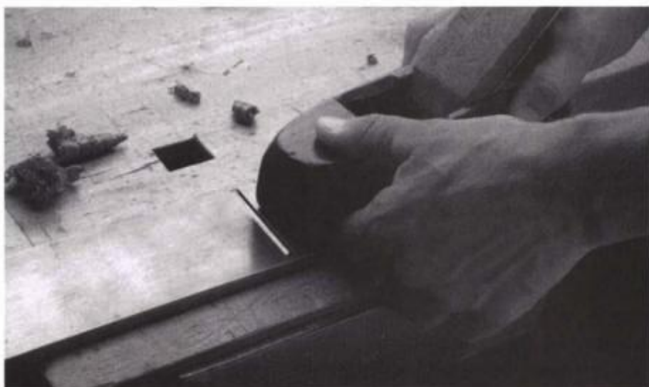
Flatten the sole of a wooden plane against a long jointer held upside-down in a vise.
