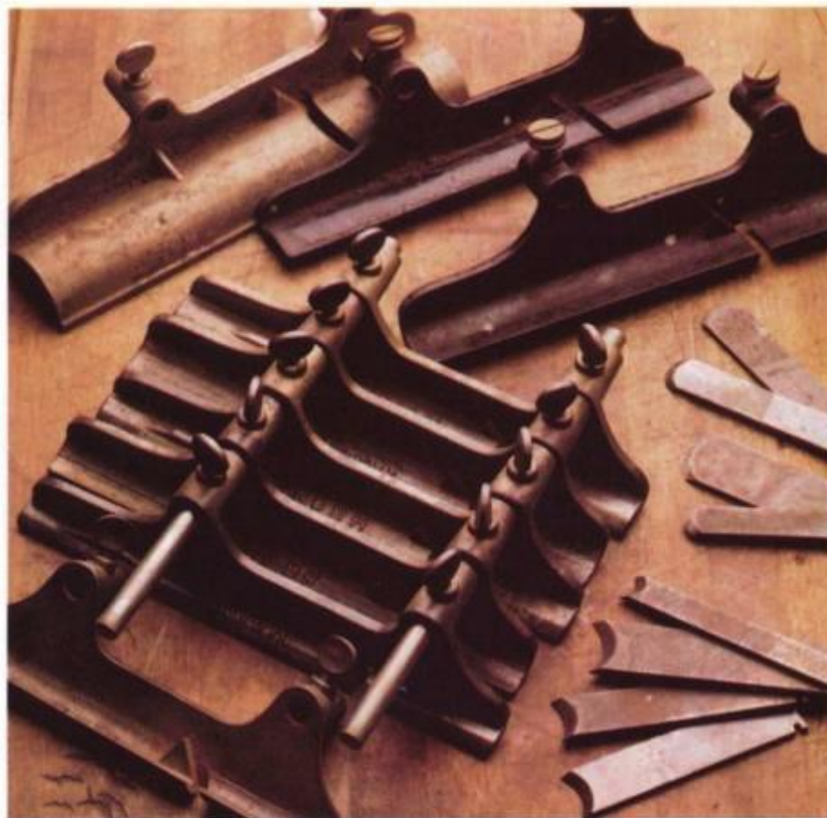
With a combination plane, one tool could do the work of many. To work as a hollow, round, or nosing tool (for the front edges of stairs and window sills), the Stanley #45 needed special bottoms, which were sold separately.
