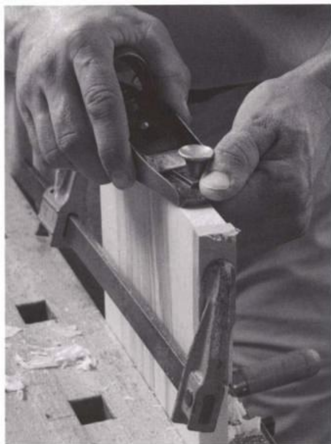
Clamp a scrap block to the workpiece to prevent the end-grain fibers from splitting out.
