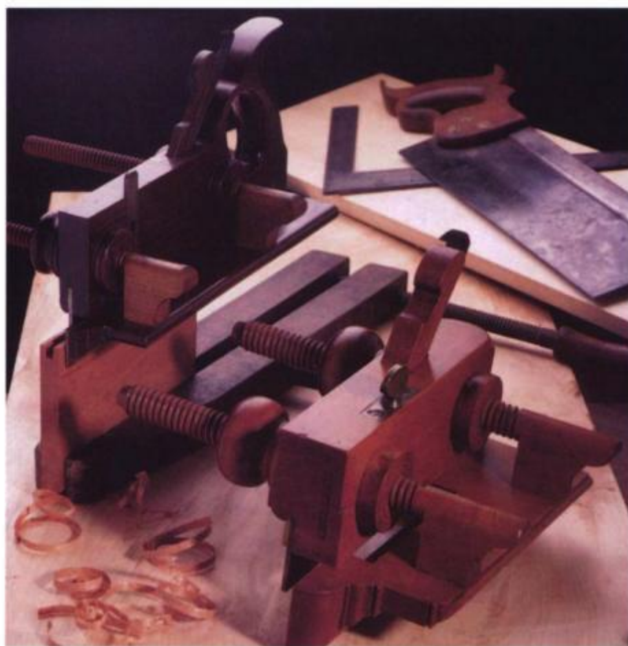
Screw-arm plows adjust slowly but positively. A nut on either side of the plane body locks the boxwood threads.
