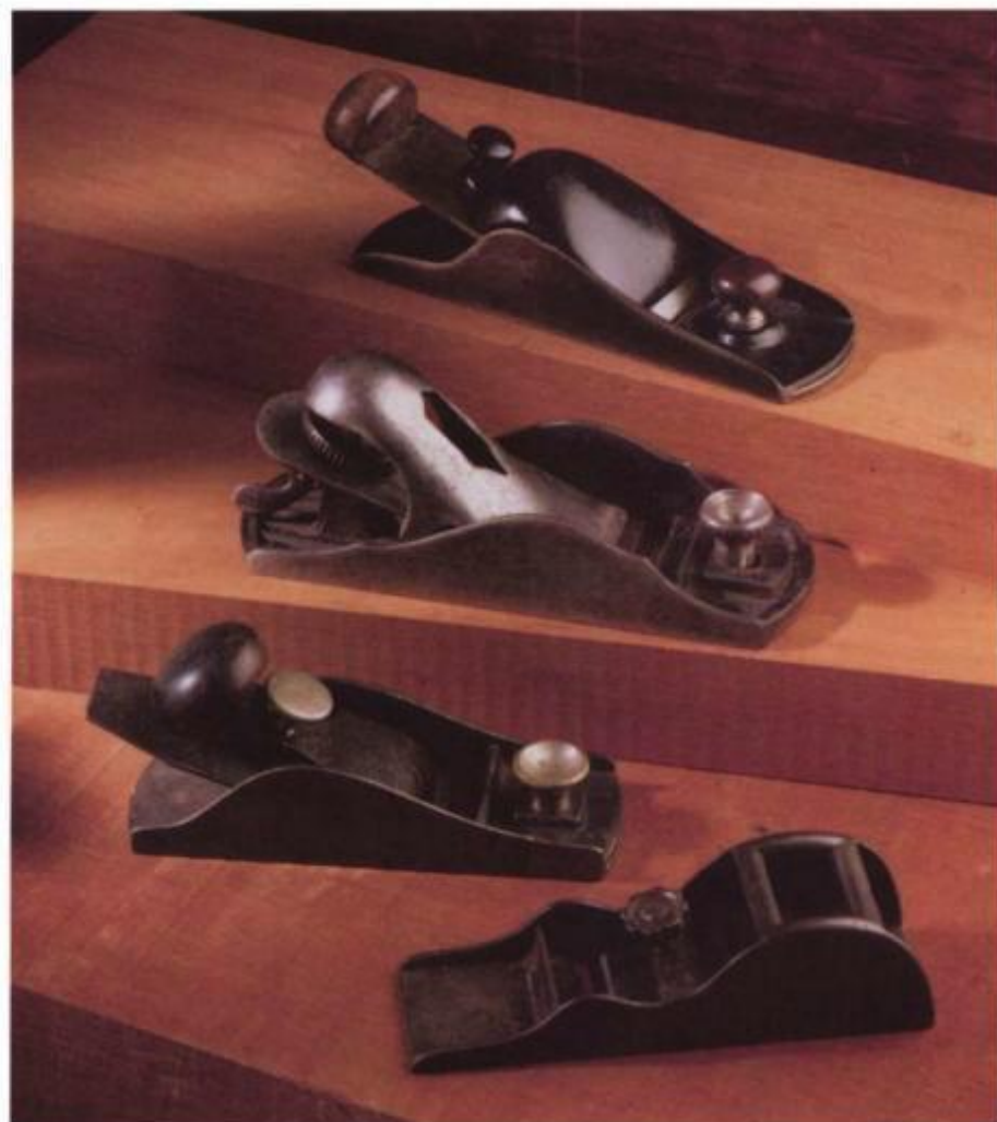
Block planes once came in a variety of qualities and sizes from many manufacturers. Shown here (from top) are planes from Metallic Plane Co. of Auburn, New York, c. 1873; O. R. Chaplin (with a corrugated sole and adjustable throat), 1888; Foss (patent #3 with adjustable throat), c. 1878; and Davis Level Co. of Springfield, Massachusetts, 1892.
