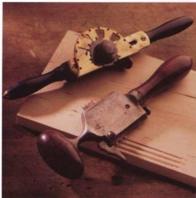
Two types of Windsor bead tools. The one at rear has a cutter wheel with different cutter profiles filed into the circumference; the one in the front takes individual cutters. Both have adjustable fences.
