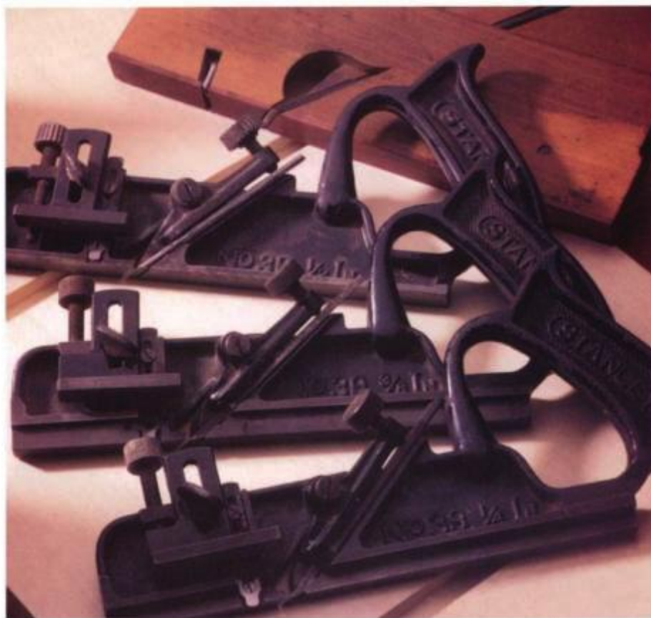
Stanley made a series of dado planes, with skewed irons, depth stops, adjustable nickers, and sole widths from \frac{1}{4} in. to 1 in. (#39 \frac{1}{4} , #39 \frac{3}{4} , and so on). The simple wooden rabbet plane in the background has a nicker iron wedged ahead of the main iron.
