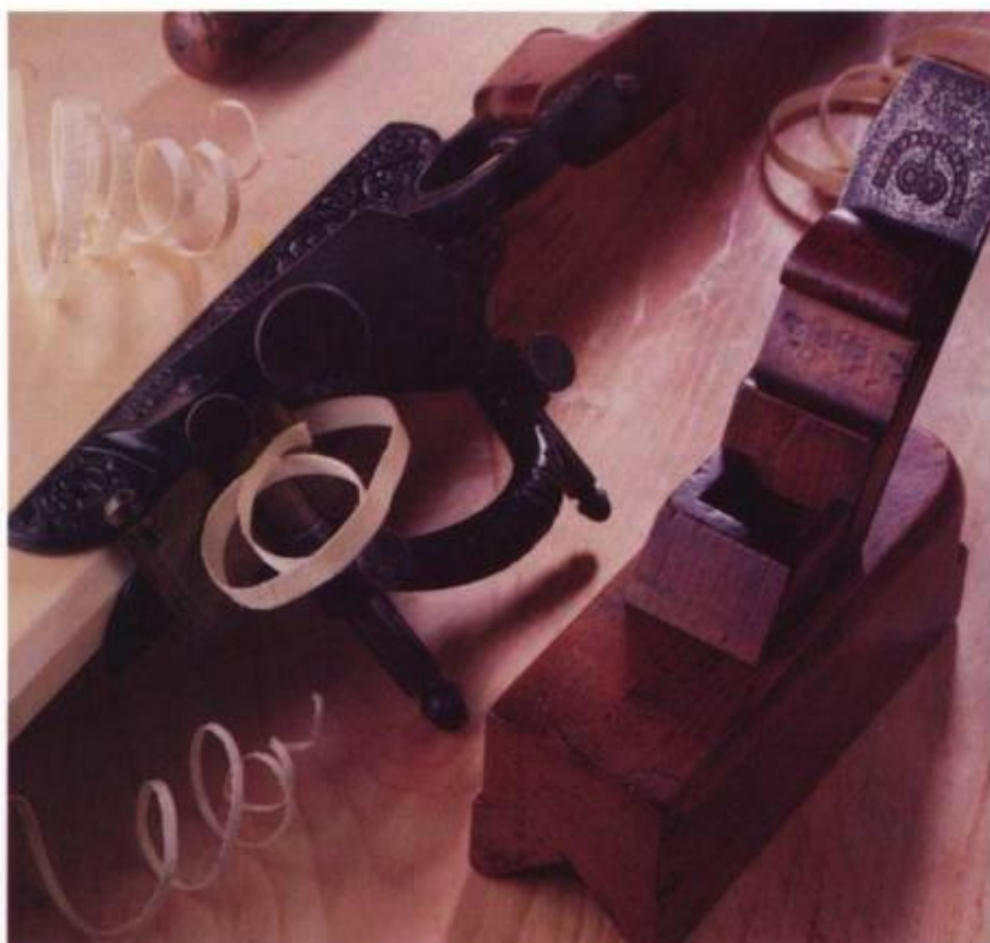
In the stop chamfer plane by Joseph Lee (1883) at left, half the sole slides open or closes to adjust the width of the chamfer. In the E. Preston chamfer plane at right, the whole center section of sole, iron, wedge, and throat moves to cut wide or narrow chamfers.
