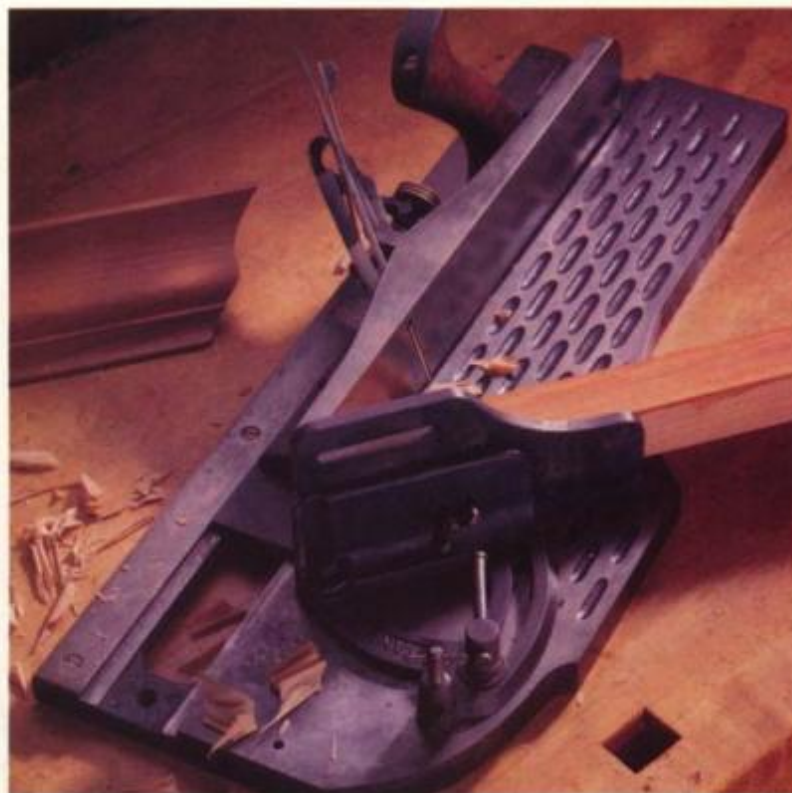
A Stanley shoot board and plane is a very accurate tool for cutting miters. The heavily skewed iron gives a clean shearing cut on work held against a stop that adjusts over a wide range of angles.
