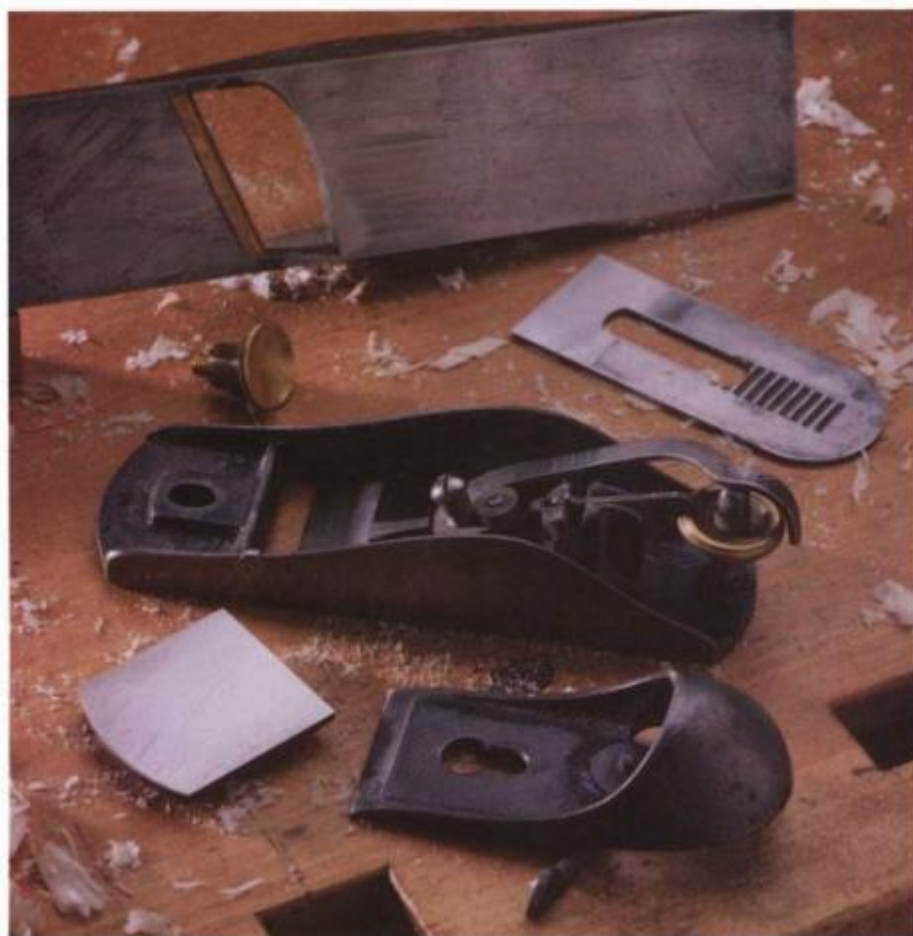
A block plane disassembled shows its single iron, adjuster, cam-locking lever cap, adjustable toe piece and the knob that secures it, and low bed angle. Too low a bed angle is fragile, as shown by the skewed block plane in the background whose bed has cracked away.
