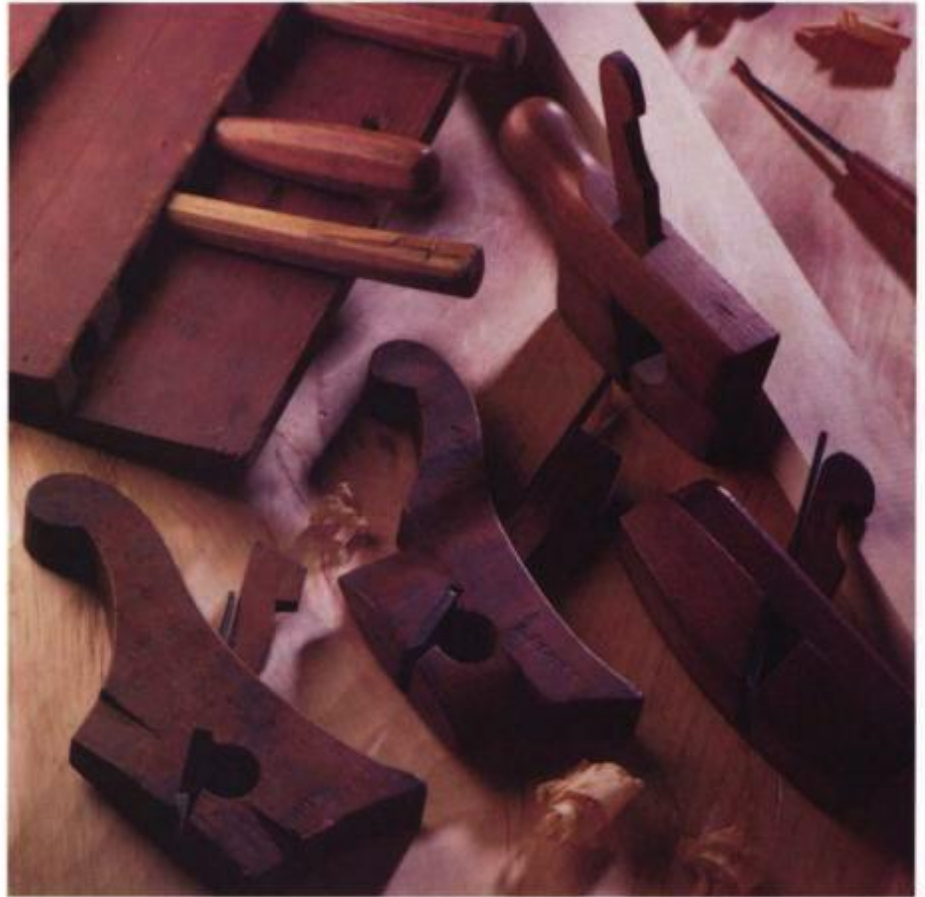
A coachmaker needed short-soled planes to work curved parts. The shape of the plane body evolved to an elegant and functional pistol grip, allowing one-handed control.
