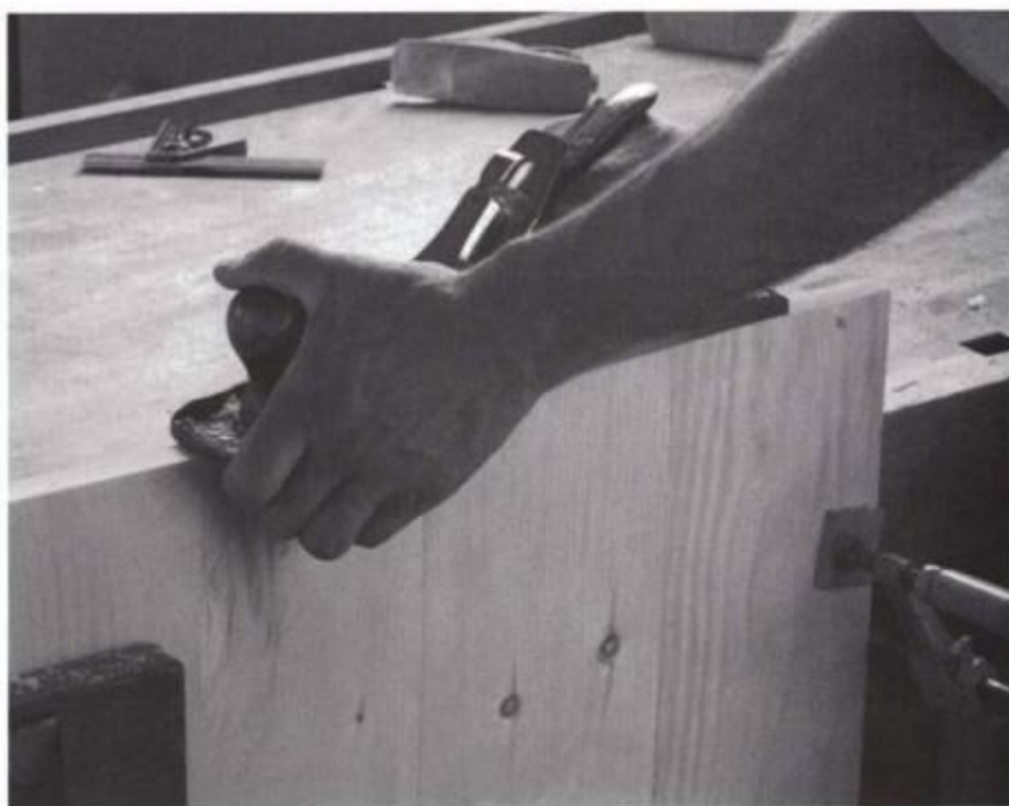
Shooting a long end-grain edge with a #5 or longer bench plane works well. A #5 cuts a true edge and is easier to hold and use than a smaller block plane.
