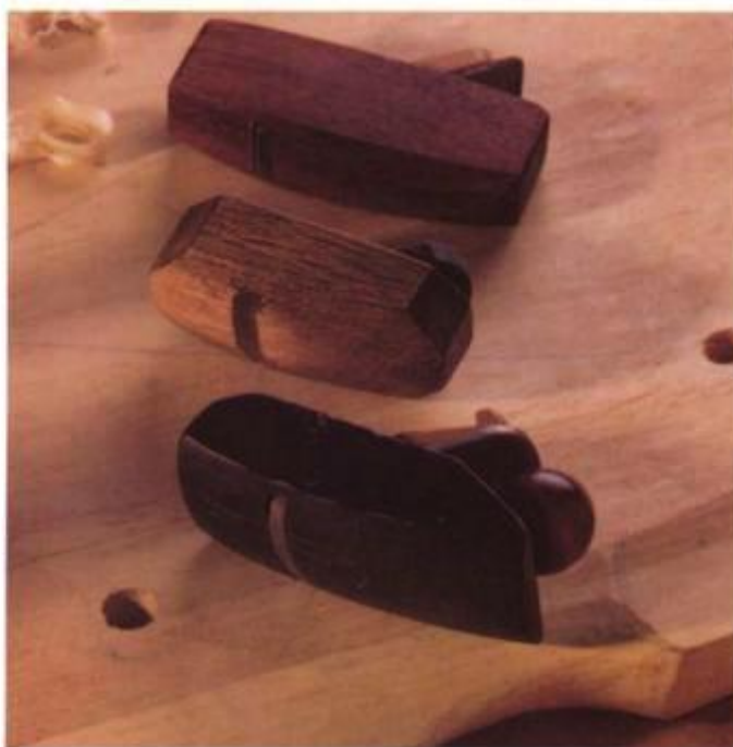
Small planes for shaping chair seats (here, resting on a pine seat for a Windsor chair) have doubly compassed soles to work into the hollow.
