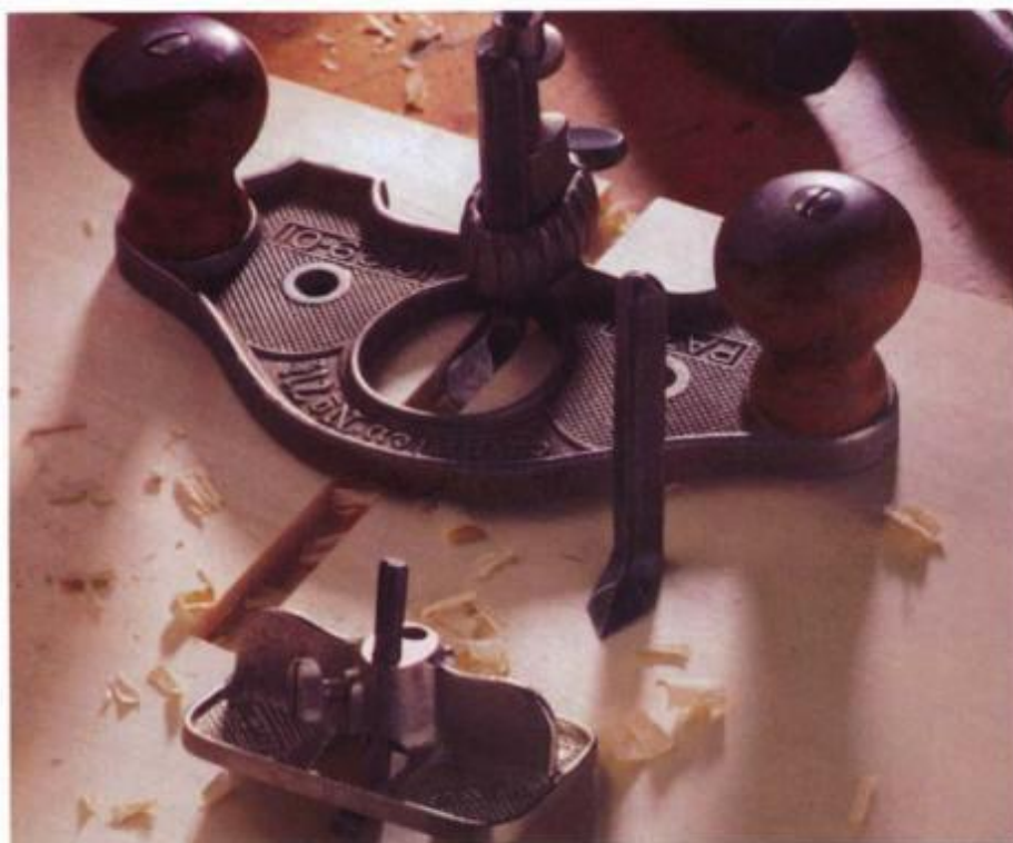
A Stanley router #71 1/2 came with two different irons, an adjuster to set their depth, and large maple handles for a good grip. The smaller router, a Stanley #271, is an extremely useful tool in tight places.
