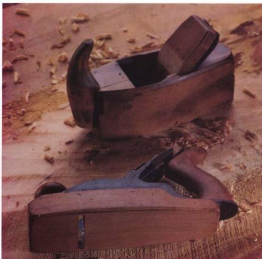
Old and worn wooden or transitional planes can be tuned as scrub planes by widening the throat and cambering the iron.
