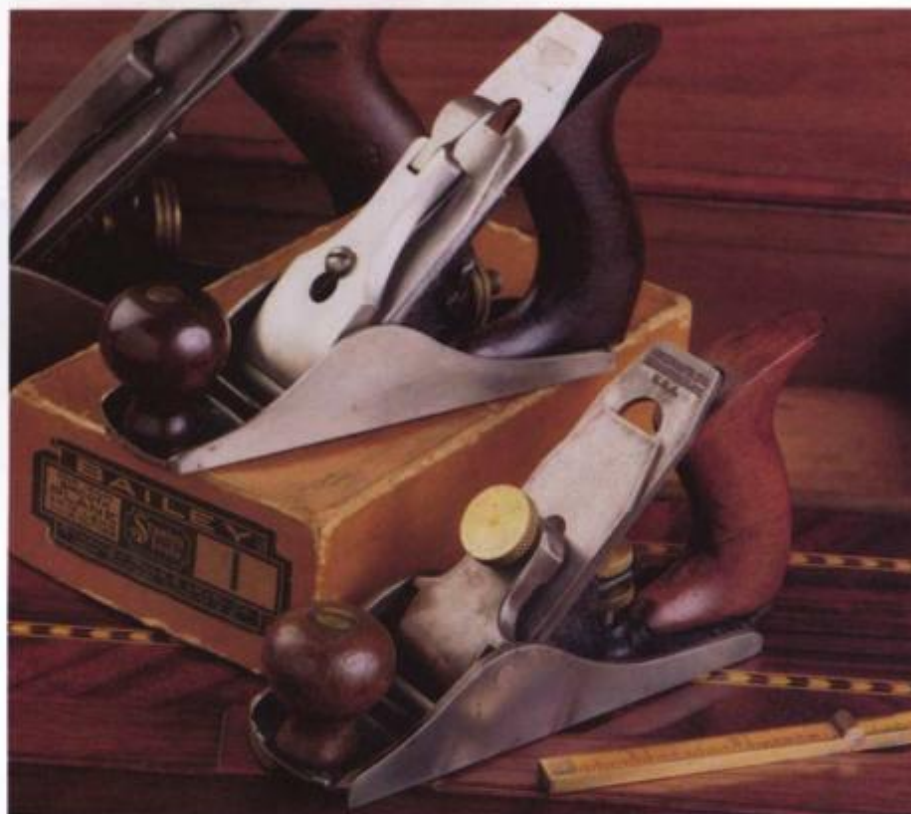
The Stanley #1 (atop the box) is the smallest and most rare of the bench planes. Competitors such as the Union Manufacturing Co., of New Britain, Connecticut, made a similar-sized plane, a #0 (foreground). The Stanley #4 1/2 in the background gives a sense of their tiny size.
