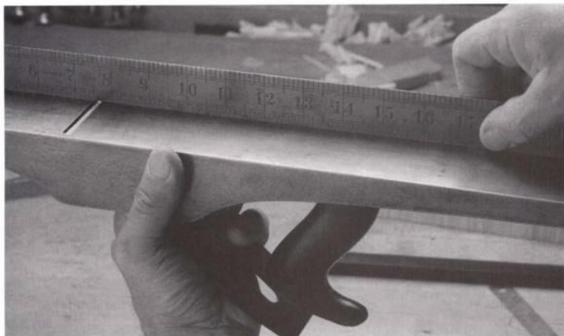
Check the flatness of the sole with a straightedge.
