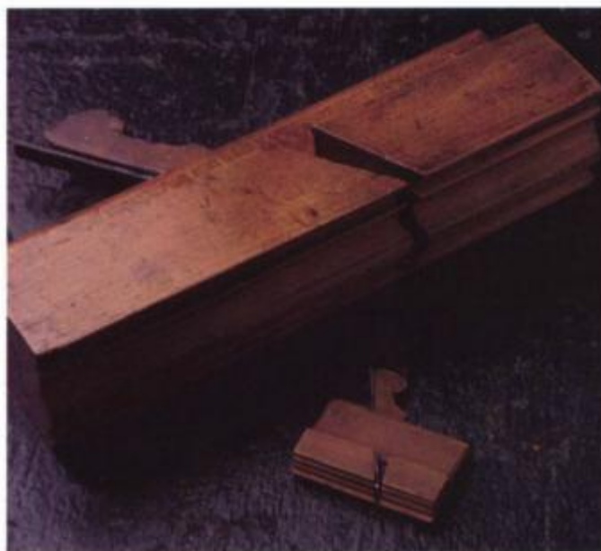
Most molding planes have a single iron, a simple wooden wedge, a rectangular body, and a side escape-ment throat. Both the planes shown here cut the same complex shape (a Grecian ogee).
