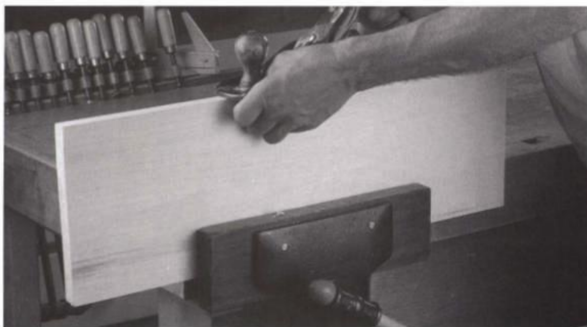
Short boards up to about 4 ft. long can be clamped in a side vise. The stronger the vise and the larger the jaws, the longer the board it can hold securely.
