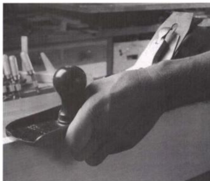
While jointing an edge, use your front hand to steady the plane, with your thumb against the front knob and your fingers wrapped around the sole against the board face.
