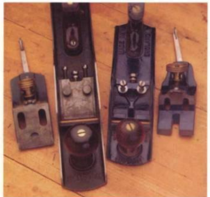
The Bed Rock frog (left) was an improvement on the Bailey pattern frog (right). It has a large, accurately milled bearing surface, a groove to locate the frog, and two large pins to secure it.
