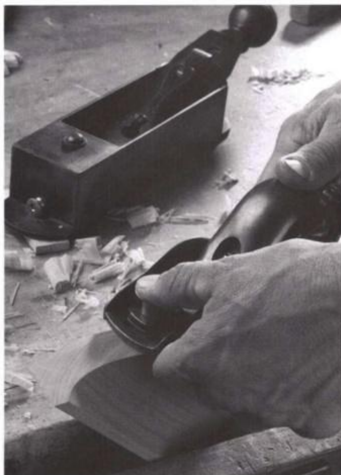
Frame miters can be planed quickly by clamping the piece in a vise and planing toward the point with a low-angle block plane.
