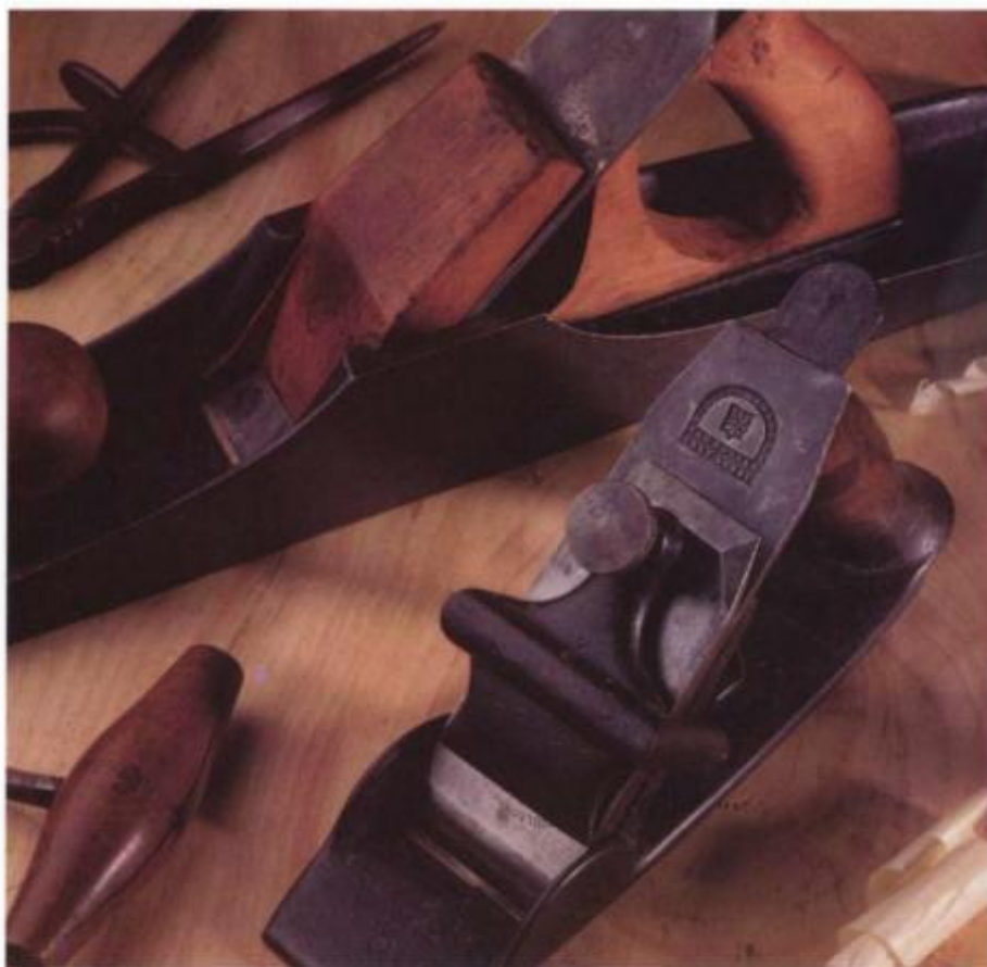
The first patented cast-iron plane, Hazard Knowles' plane of 1827 (at rear), had a frog cast integrally with the body. Another early cast-iron plane, a Birdsell Holly smoothing plane of 1852 (foreground), had a frog added to the plane and connected with the sole for better support.
