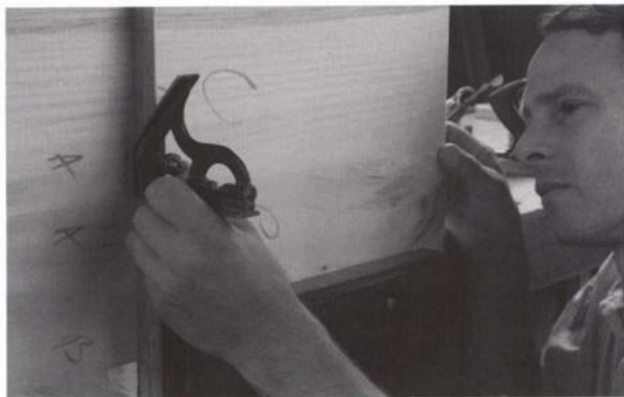
When edge-jointing two boards, check the dry joint with a straightedge and look for gaps between them.
