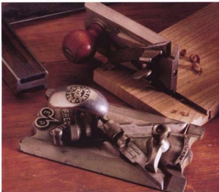
Side rabbet planes cut along the shoulder of rabbets and dados to widen them to fit other parts. These two planes with crisscrossed iron patterns are by Stanley competitors: The upright plane in the background (#81) is by Sargent of New Haven, Connecticut; the other fancier version with adjustable irons is by E. Preston of Birmingham, England.
