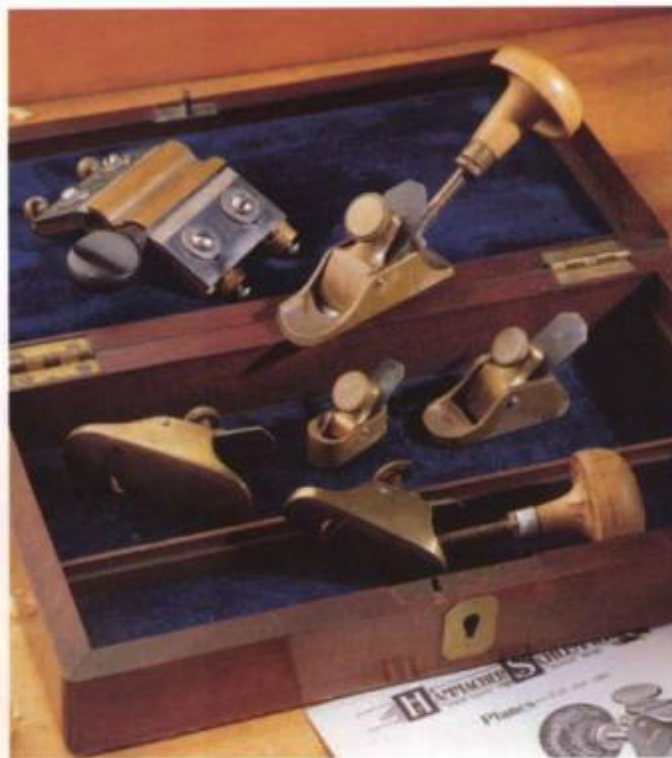
Hammacher Schlemmer violinmaker's planes, shown here in a fitted case, have detachable tail handles that screw into the frog. The tool in the background is a peg shaper, which works like a tapered pencil sharpener or spoke pointer.
