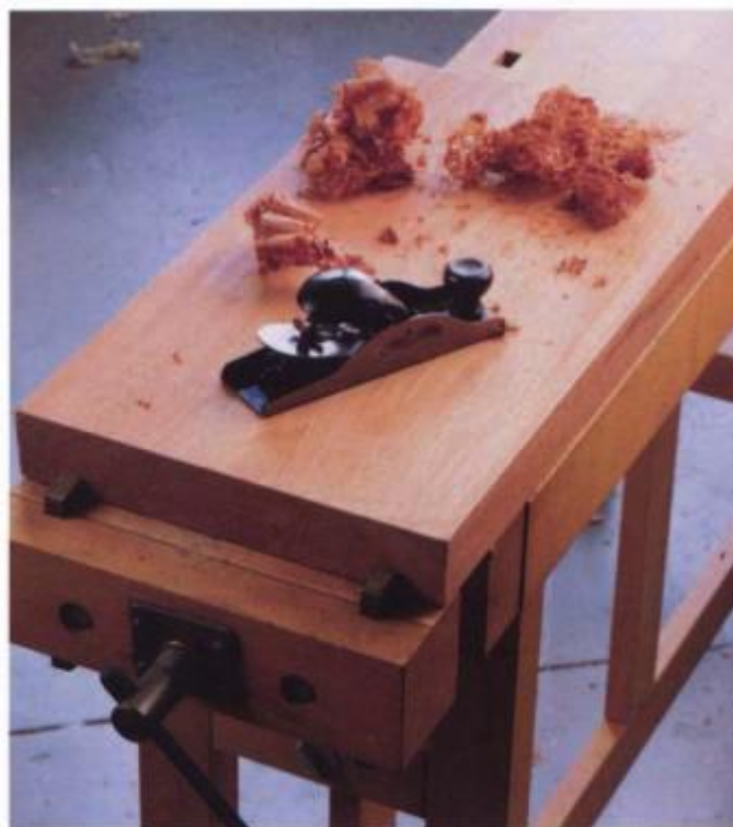
A large end vise with two bench dogs and a double row of holes down the bench can clamp large or oddly shaped parts securely. The plane on the bench is an experimental Stanley block plane.
