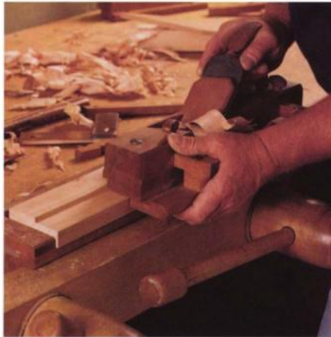
After dimensioning and squaring the stock, Ted cuts the handhold with a fillister plane.
