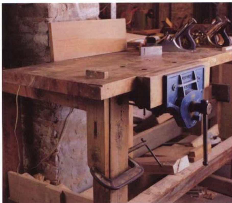
Benches don't have to be elaborate to work well. This basic bench has everything you need to hold the work: a large, quick-acting side vise, a flat top surface, and an adjustable stop projecting through the top to plane against.
