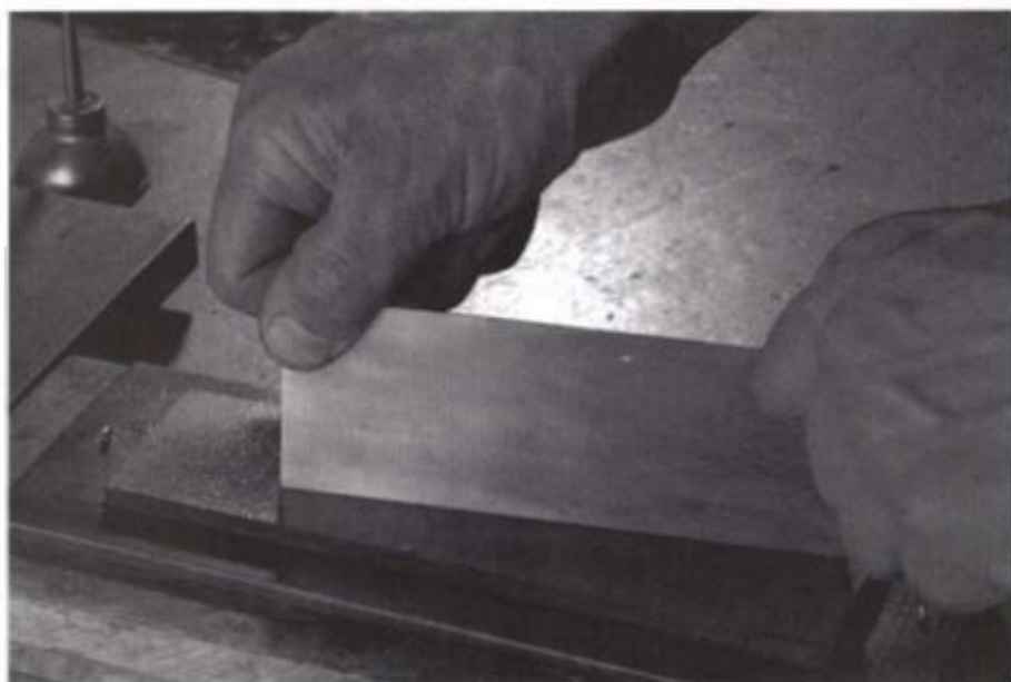
To hone the edge of a scraper, hold it upright and "saw" on the face of the stone, working back and forth and slowly side to side to avoid scoring the stone.
