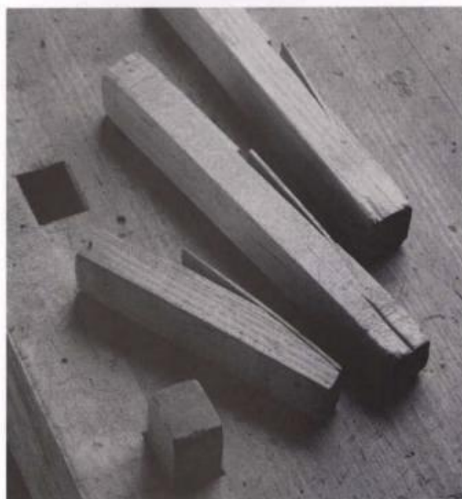
Wooden bench dogs are simple to make and replace and are less likely to damage a plane iron than ones of steel or brass. An ash strip set into a saw kerf or screwed on creates a spring to hold the dog in position.
