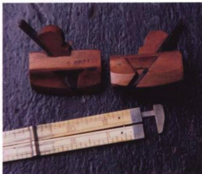
Miniature molding planes such as this pair were craftsman-made for some special work, perhaps for molding the fine mullions of a fanlight window. The planes are mirror images of each other, or "handed," to work with the grain in any direction.
