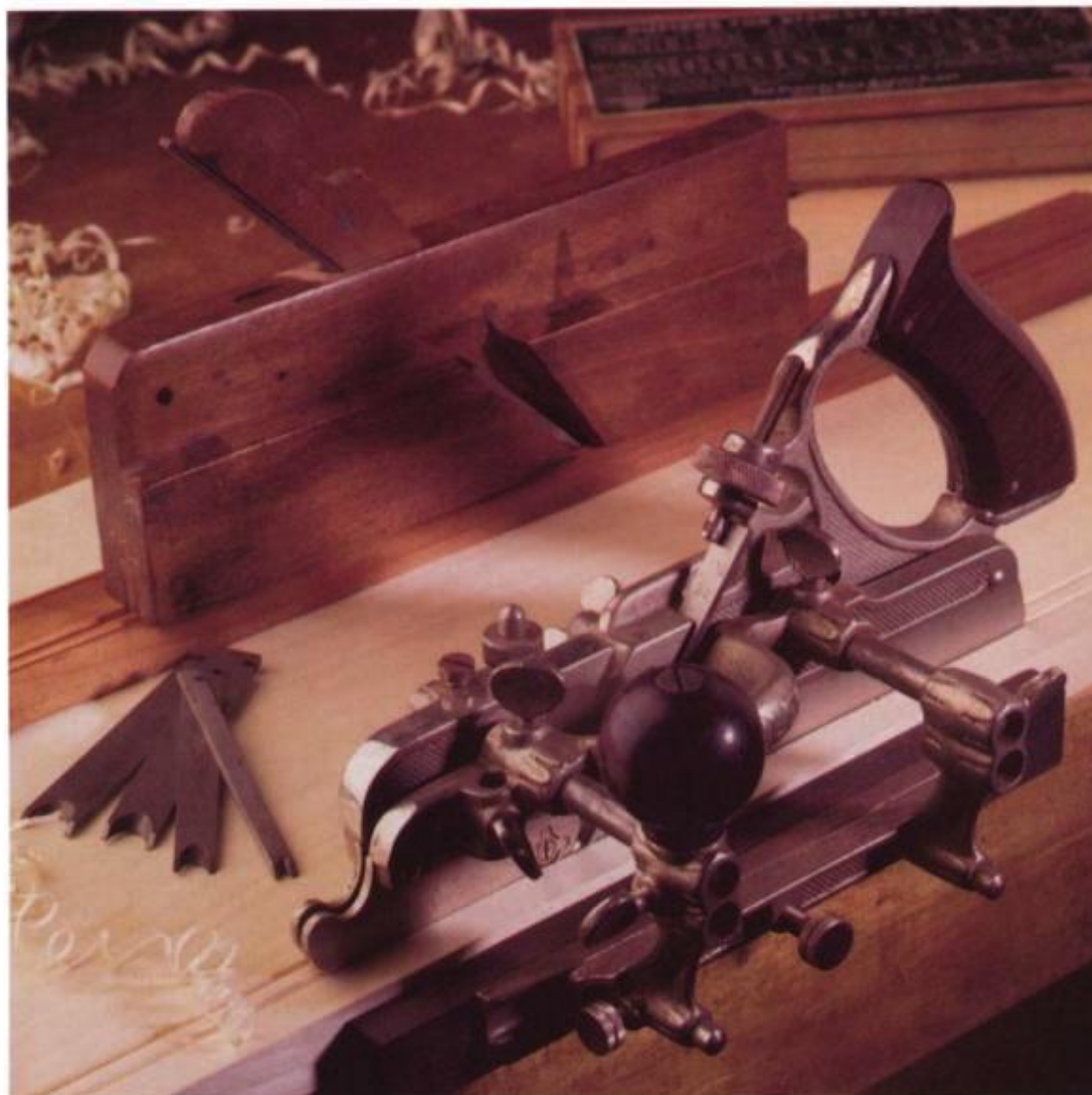
With an adjustable fence, a Stanley #45 combination plane easily cuts a center bead (or, with multiple passes, reeds). The wooden center bead plane in the background requires setting a guiding fence for each bead or reed.
