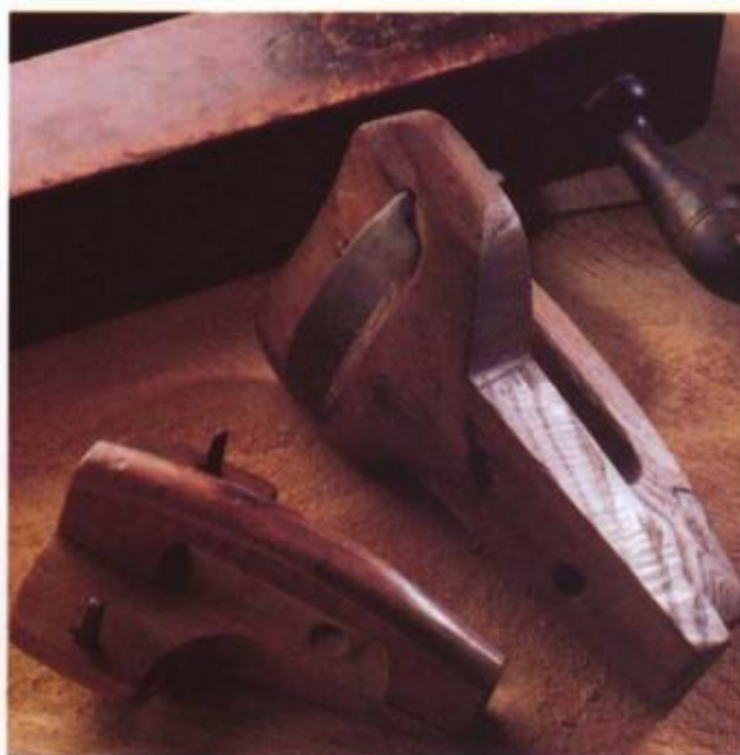
These two unusual shaves could be used to hollow a plank seat or just as easily to shape a shovel or scoop.
