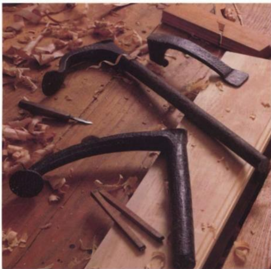
Holdfasts work as their name implies, with a long reach, secure hold, and quick release. All they require is a hole through the benchtop.
