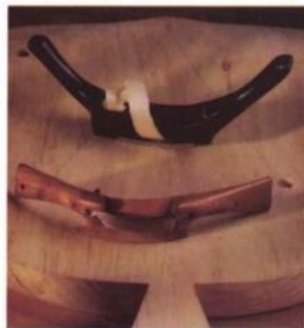
Travishers are shaves used to hollow and shape a seat. They have upward-sweeping handles to keep the chairmaker's knuckles well out of the way.
