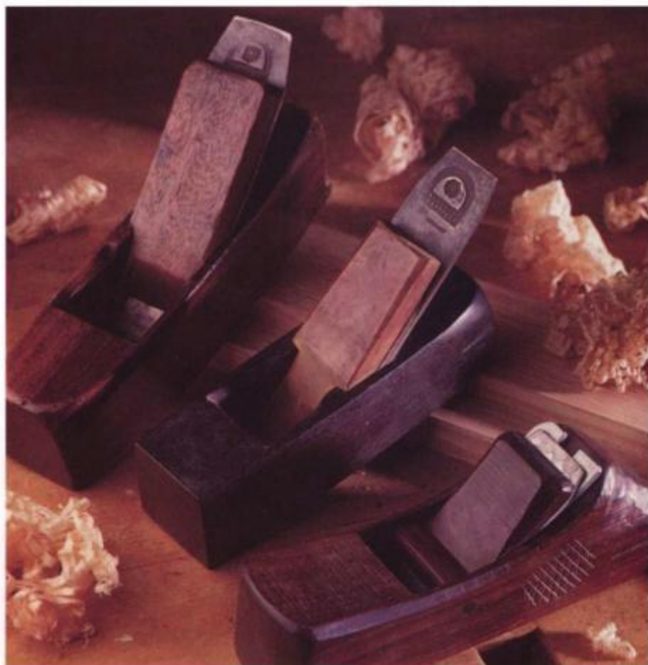
Traditional wood-bodied smoothers feel wonderful in your hands, are easy to tune, and can work exceptionally well. From rear are a lignum-vitae, coffin-shaped smoother; a small but heavy ebony smoother; and a distinctive cocobolo plane by James Krenov.
