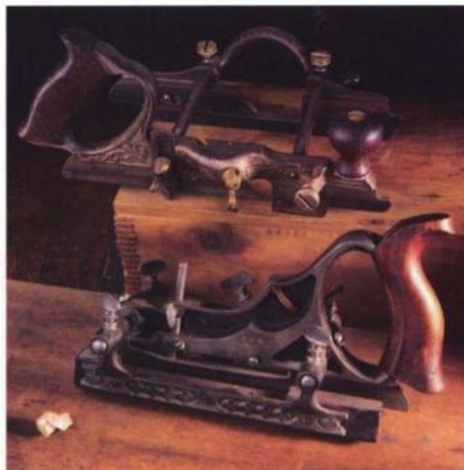
Combination planes evolved from plow planes to perform a variety of tasks, including cutting dadoes, rabbets, grooves, and tongues. These two early designs are a Stanley #46 with skewed cutters (at rear) and a Siegley combination plane.
