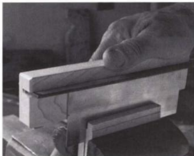
A simple jointing tool can be made by cutting a slot in a block of hardwood to hold a file snugly.
