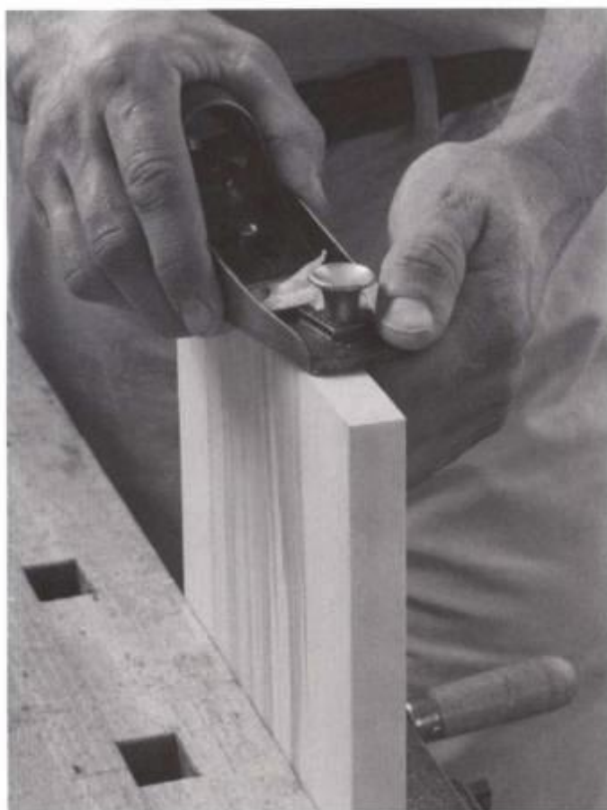
One way to plane end grain is with the workpiece securely clamped in a vise, your rear palm around the plane supplying the force and the control, and your fingers in front stabilizing the cut.
