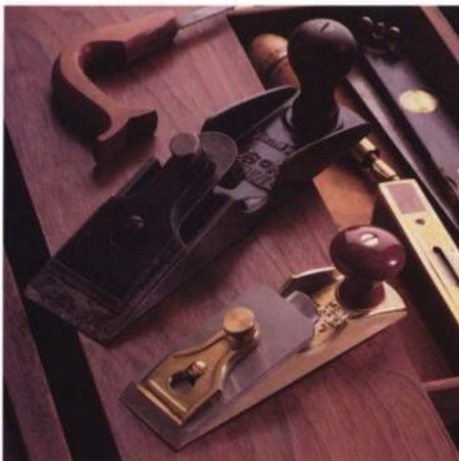
Stanley made a single-size chisel plane, a #97, for "Piano Makers and all Cabinet Workers" (center). Today, Lie-Nielsen makes a smaller version in cast bronze (foreground).
