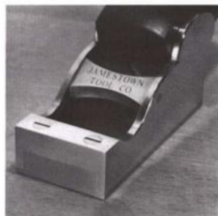
The careful alignment of the slots in the screws that secure the adjustable throat in this chariot plane is typical of Jamestown Tool Company's attention to every detail. (Photo courtesy of Jamestown Tool Company.)
