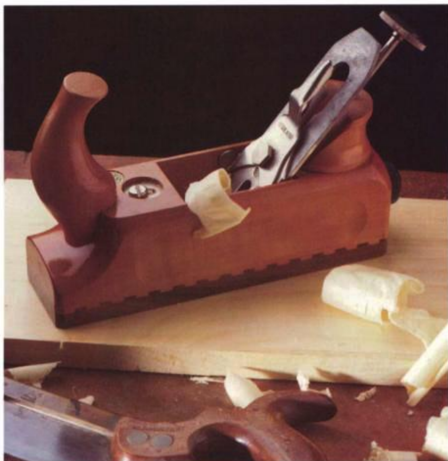
Whereas few wooden planes are still made in America, Continental European plane makers continue to produce them, such as this Primus plane made of pear with a lignum-vitae sole and unique adjusters.
