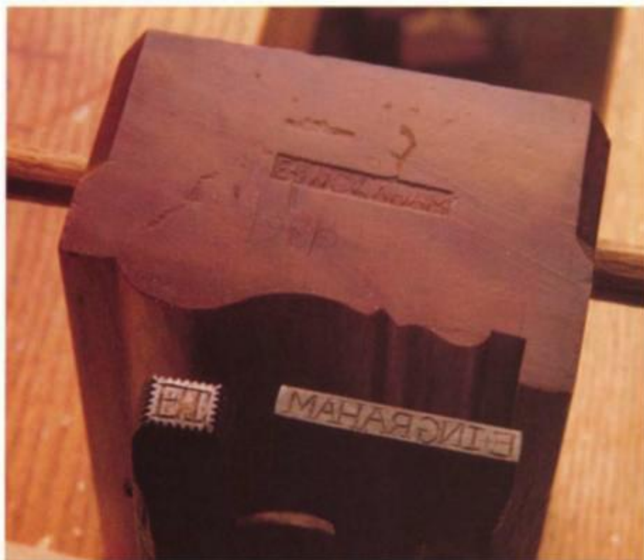
In the tradition of past plane makers, Ted Ingraham stamps the toe of his wooden molding planes with a stamp he cut and filed. This plane cuts a large cornice or crown molding.
