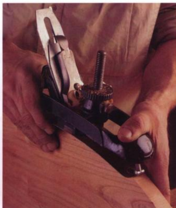
The Stanley #20 works well for fairing the outside curve of a tabletop as long as it's the arc of a circle. Varying curves are better shaped with spokeshaves.
