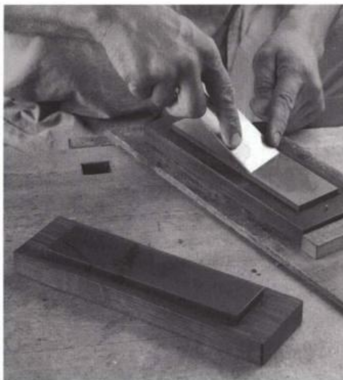
Using light pressure and with your arms locked to maintain a consistent bevel angle, stroke the iron up and down the stone in narrow figure eights. Use the entire surface of the stone.
