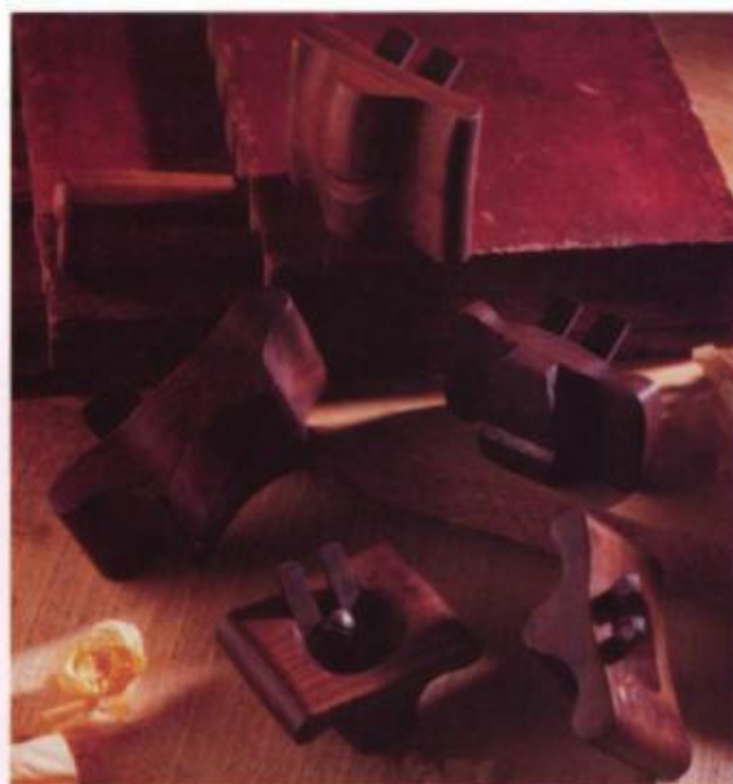
Short-soled molding planes shape the curved sections of the handrail. No matter how many shapes stairmakers owned, for some stairs they had to make special planes.
