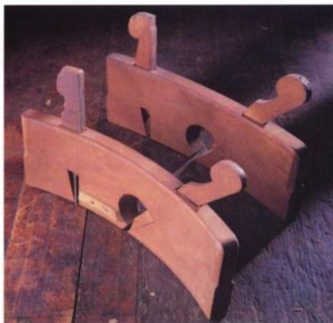
These unusual curved wooden dado planes were made for cutting dados of a specific radius for architectural work.
