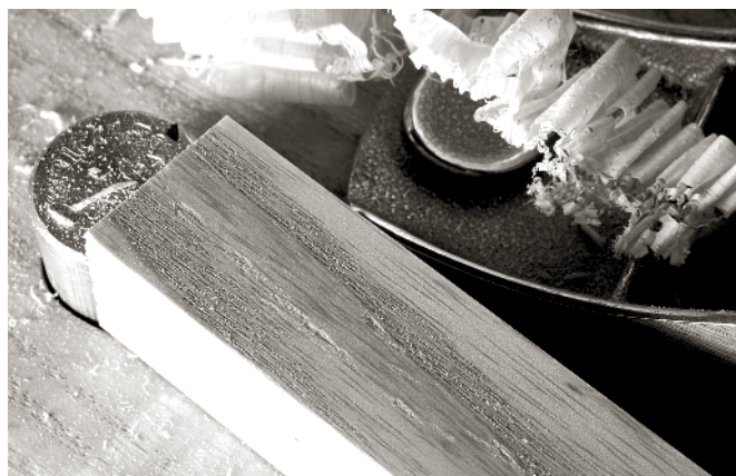
PLANING AT A 20^\circ SKEW (both skewing left and skewing right) created a little tear-out.
