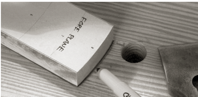
PLACE THE TEMPLATE ON YOUR iron and trace its edge on your iron. A thin, consistent line is best.
