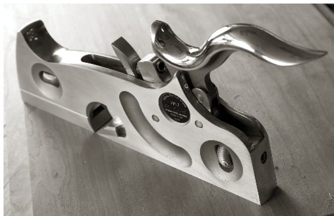
THE HP-7 IS SURPRISING AT every turn. The lever cap engages and releases by lowering and raising the grip. It's intuitive and simple in use (though mechanically complex inside).
