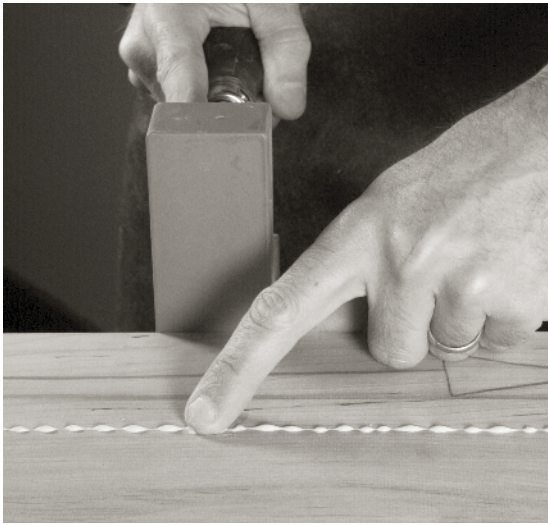
BEGIN CLAMPING IN THE MIDDLE of the panel. Apply pressure and check each seam with your finger. Adjust the boards until they line up.
