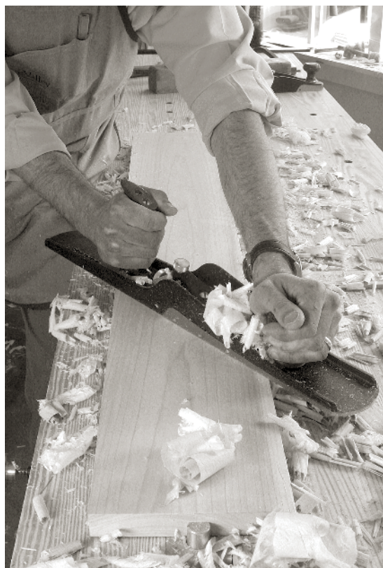
WORK NARROWER STOCK AT AN angle using the jointer, Moxon writes, to ensure flatness.
