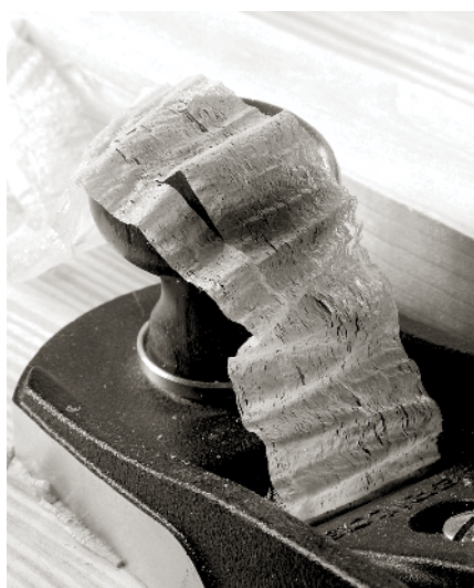
THIS SHAVING IS ABOUT HALF the thickness of the thick one. Use this size shaving if you start to see tearing on the surface of your project.
