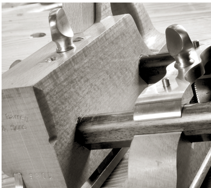
THE BRIDLE MECHANISM IS FLAWLESS in workmanship and in function. The fence locks parallel to the skate every time, which saves an immense amount of fussing.
