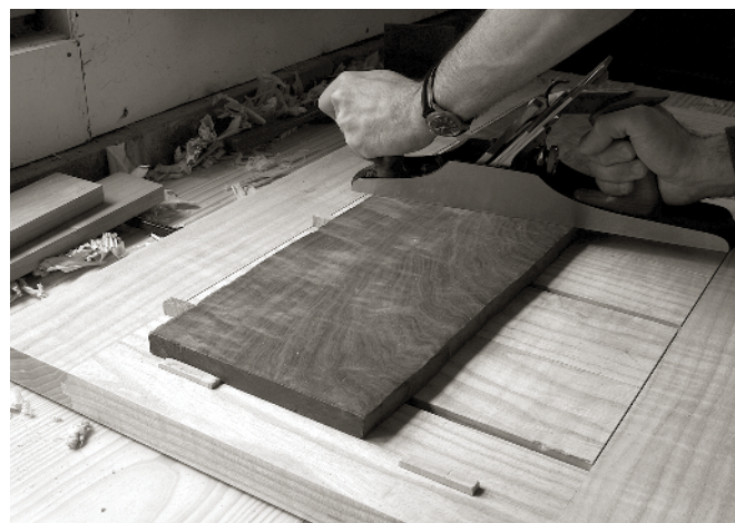
THE STOPS CAN BE USED when planing stock with the grain or across the grain.
