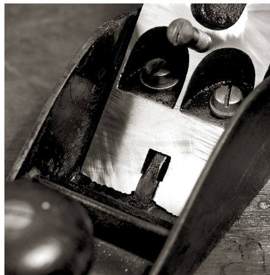
HERE YOU CAN SEE THE rib between the two legs of the frog. If this protrudes past the face of the frog, your iron isn't going to seat properly. File it down or adjust your frog forward.
