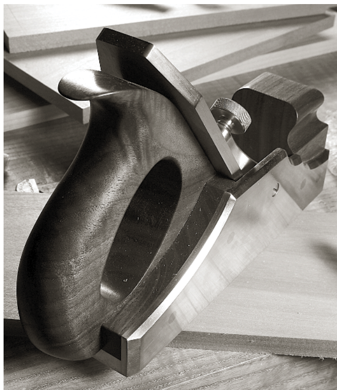
THE CHAMFERED SIDEWALLS OF HIS planes are just one more clue as to the care and attention that Brese lavishes on his smoothing planes.
