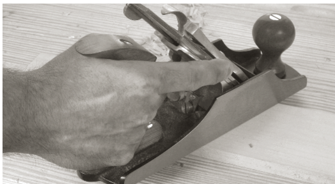
HERE'S THE CLASSIC THREE-FINGERED GRIP on a bevel-down tool. This is more comfortable to me than a four-fingered grip.
