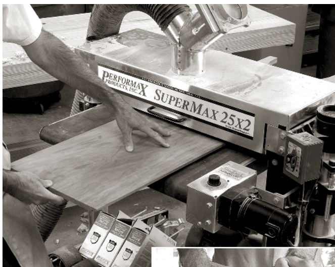
A DRUM SANDER (ABOVE) CAN level and true a panel much like a jointer plane. A random-orbit sander (right) is ideal for removing machining marks in a power-tool workshop.
