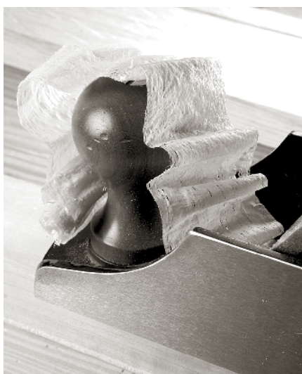
A SUBSTANTIAL SHAVING SUCH AS this one reduces the number of passes you take, but it can increase your chances of getting tear-out.
