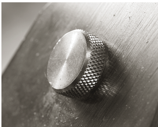
THE SMALL BRASS BUTTON PREVENTS the iron from sliding to the floor when the lever cap is released. I also used it as a sneck to retract the iron a tad when setting it.
