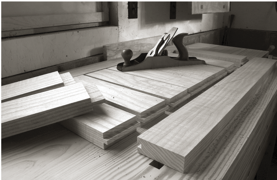
HERE YOU CAN SEE THE joinery of the planing board before it is assembled. It's like a door with loose slats instead of a fixed panel.
