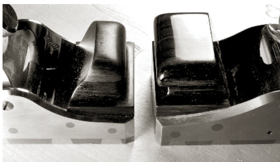
HERE YOU CAN SEE THE differences between the front buns of the two A13s – Holtey's is on the left; Hutchin-son's is on the right.
