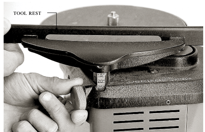
SET THE BEVEL ANGLE you want to sharpen with the Veritas system by adjusting the tool rest up and down.
