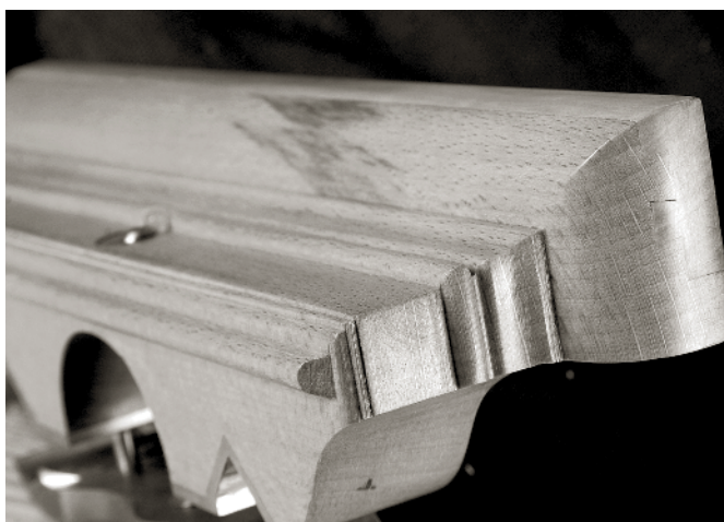
THE MOULDING ON THE FENCE is remarkably crisp, even as it returns across the front. Here you also can see (if you look closely) the boxwood lining and the two sliding dovetails that attach it.
