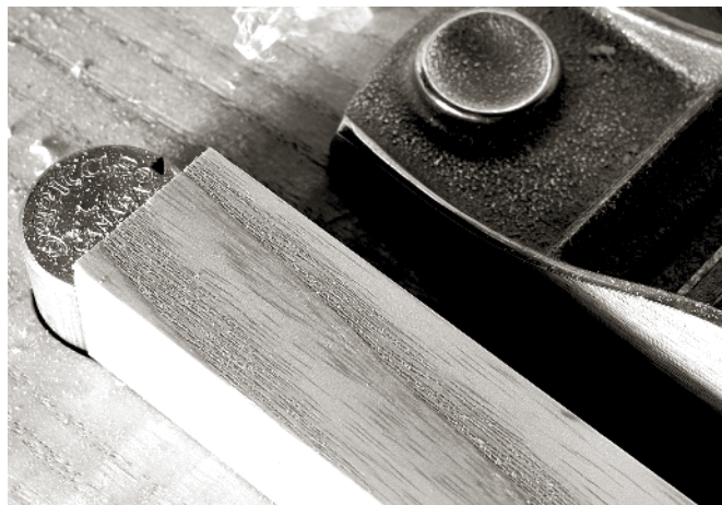
PLANING WITH NO SKEW RESULTED in no tear-out on this ash board.
