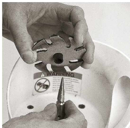
THE 3M TRIZACT SANDPAPER is attached to plastic discs (called Ninja Disc Backpads) that screw onto the machine's spindle. Swapping discs is fast and easy.
