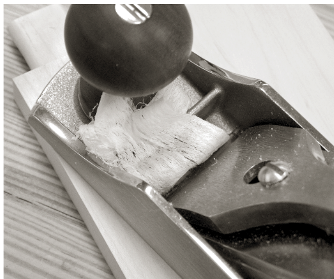
SEE HOW THE SHAVING EMERGES only in the middle of the mouth? That's how you know your iron is sharpened and set correctly.
