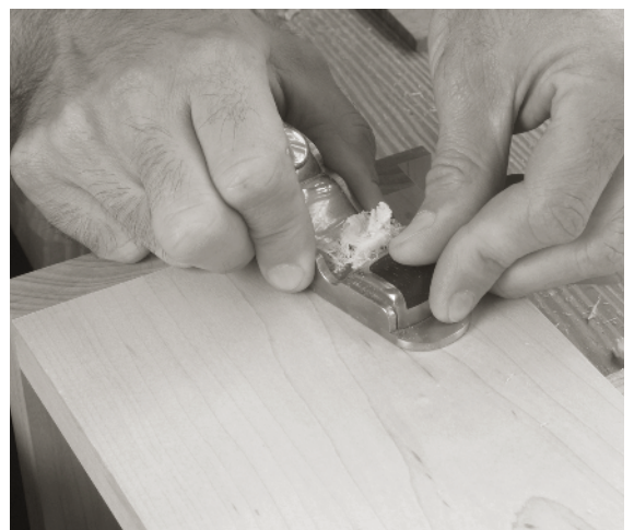
REMOVE THE HIGH SPOTS USING a plane that has a short sole. Then go back to rubbing.
