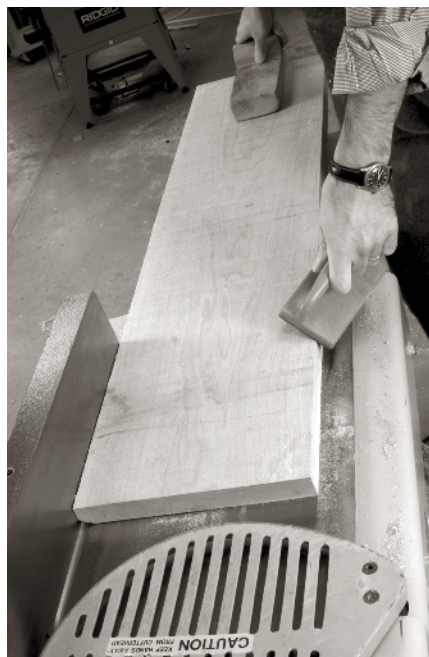
HERE YOU CAN SEE THE cathedrals, even in the rough. When jointing one face and the bark side is on the table, the cathedrals usually should point to the cutterhead.
