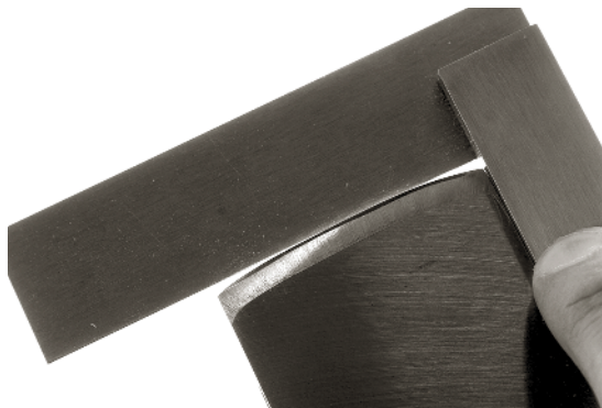
A SILHOUETTE OF THE SHAPE of my fore plane's cambered iron. It's an 8" radius, which allows me to take an almost \frac{1}{16} "-thick shaving in softwood.
