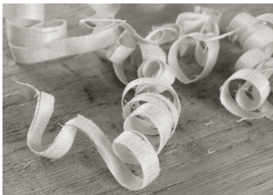
THE SHAVINGS SHOULD BE FAIRLY thick – you don't want to do this all day. These shavings are .015" thick. I could probably go a little thicker in pine.
