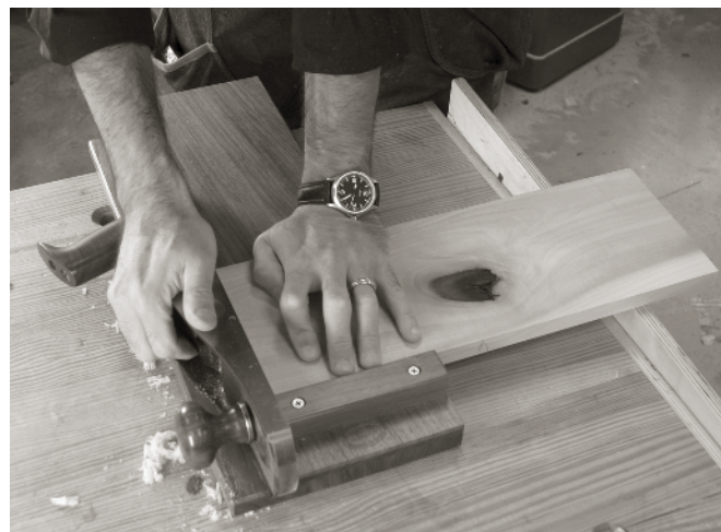
HERE'S THE SHOOTING BOARD in use . You don't want your work to slide left or right during the cut, so put your back into it.
