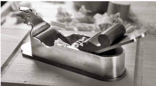
EARLY METAL PLANES LOOK LIKE what we could call a “miter plane.” However, they likely weren’t for shooting miters. Many examples had the sole proud of the sidewalls, such as in this modern interpretation of an early plane by Wayne Anderson.
