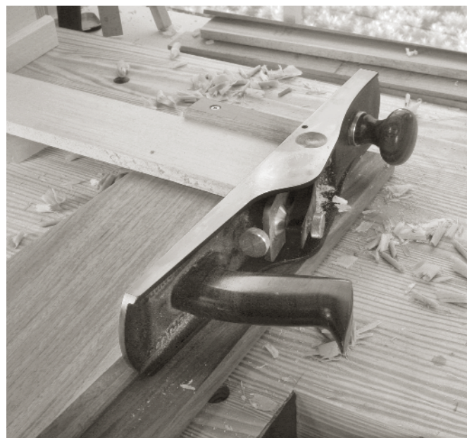
HERE'S A VERITAS BEVEL-UP JACK plane on a shooting board. The tool is ideal for shooting edges and ends, though you can set it up to do almost any task.
