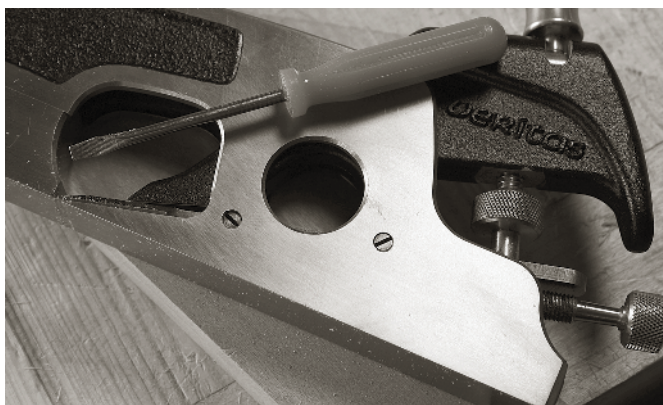
THE SCREWS IN THE SIDEWALLS create a precise channel for the iron to rest in. The actual blade adjuster is a Norris-style adjuster.
