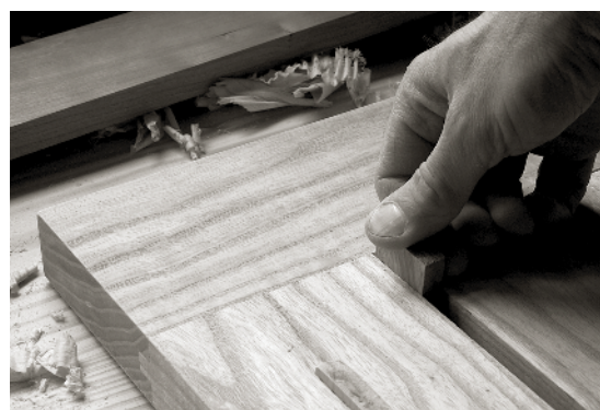
PLACE WEDGES BETWEEN THE SLATS to create stops for your work.
