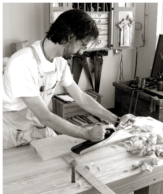
ON NARROWER CABINET COMPONENTS, THE jointer plane works along the grain. Skewing the tool slightly during the cut makes it easier to push and does assist in flattening. One wider panels – say 14" and wider – I'll begin with a few diagonal passes before switching to long-grain ones.
