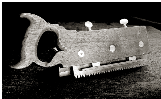
AN ENGLISH STAIRSAW, USED FOR cutting dados in stringers. Note the ingenious depth stop by the blade.
