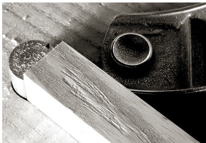
PLANING WITH A 30^\circ SKEW (both skewing left and skewing right) created this ugly patch of torn grain.
