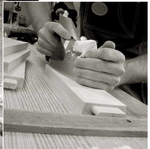
A SHOP-MADE PLANING STOP IS a simple and effective way to hold your work for smoothing (left). The force you use to push your plane also holds your work down and against the stop (below).
