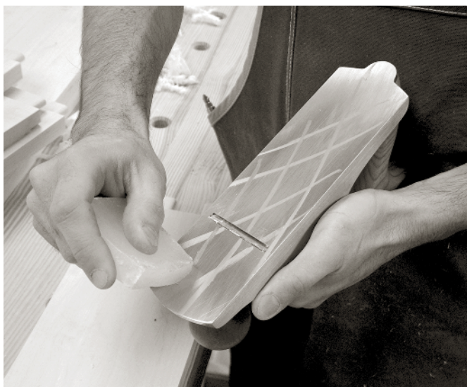
A LITTLE CANNING WAX ON your sole makes the work easier and your cuts lighter. Some craftsmen prefer a little mineral oil.
