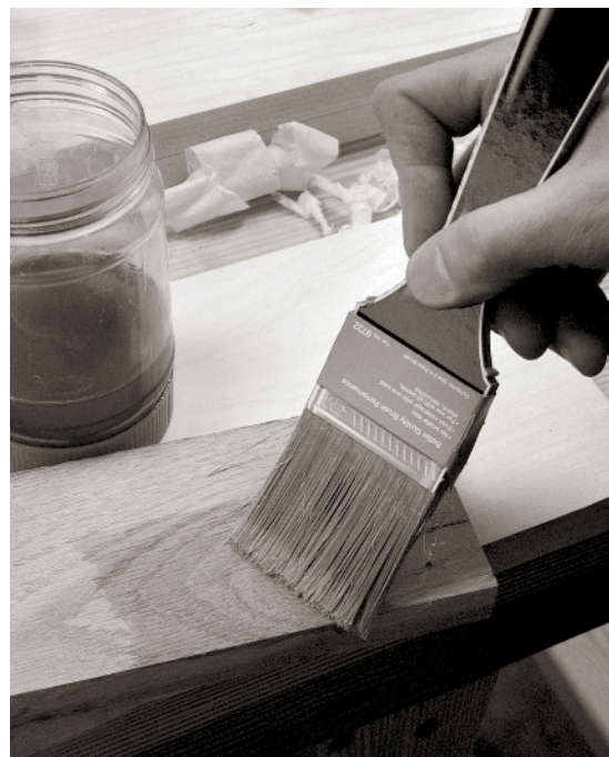
A LITTLE SHELLAC ON A problem tear-out will stiffen the wood fibers and allow them to be sheared cleanly – sometimes.
