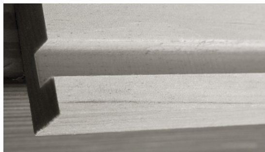
WHEN CUTTING IN SOFTWOODS OR with the grain of a board the groove should be neat like this. When you work against the grain , it can be a little ugly. You can score the extents of the groove with a cutting gauge before plowing when working against the grain. That will keep the top edge clean.
