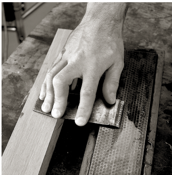
YOU CAN STONE THE EDGE of your cap iron freehand, but a scrap piece of wood will make the operation foolproof and quick. Stone this edge until it seats tightly against the iron.
