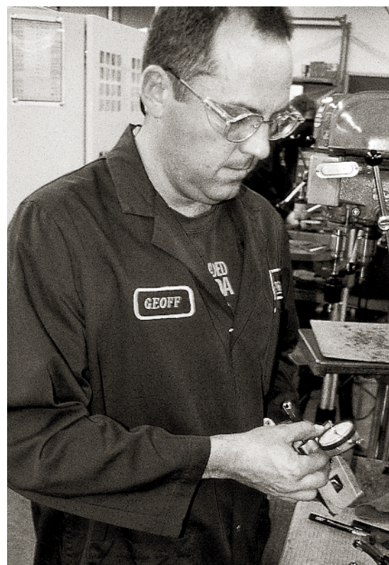
A VERITAS EMPLOYEE CHECKS THE machining on a plane's frog. Most home woodworkers don't have the correct instruments to measure tolerances or the skills to correct them. If you think your premium plane isn't right, contact the manufacturer before fixing it yourself. You could make it worse.
