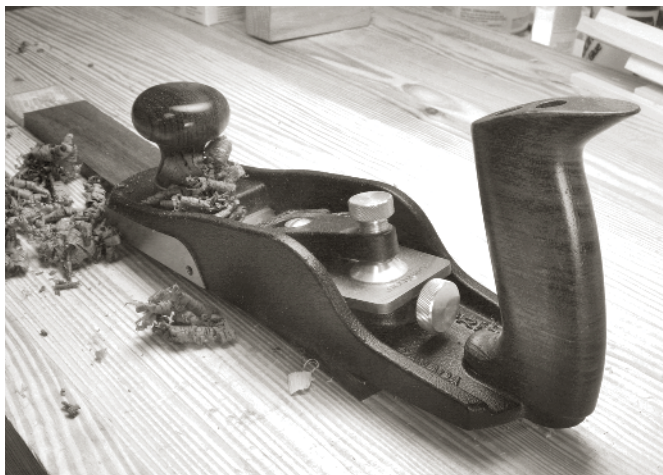
HERE'S A VERITAS BEVEL-UP SMOOTHING plane. These are easy for beginners to set up and excel at removing tear-out when sharpened with a high angle.
