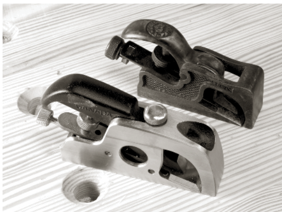
THE VERITAS BULLNOSE PLANE SHOWN with a vintage Preston version of the same tool. The Veritas plane has features and a shape that favors ergonomics and function over the classical form.
