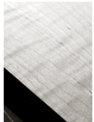
HERE IS THAT SAME SECTION of curly maple after planing it with a tool pitched at 62°.
