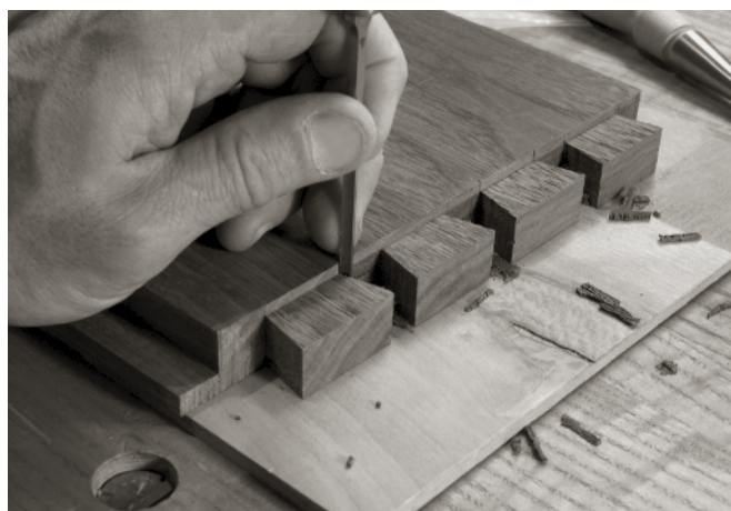
THE RABBIT ON THE INSIDE of the tail board also helps me when chiseling out the waste between the tails. It prevents me from overcutting past the baseline.
