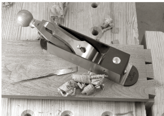
LIE-NIELSEN IRON MITER PLANE. A remake of the Stanley No. 9 cabinetmaker's block plane of the last century.
