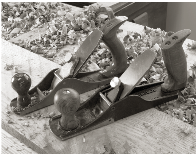
THE TWO MAJOR MANUFACTURERS OF premium planes now make scrub planes. Both are more refined than the original Stanley versions and are useful for rough work.
