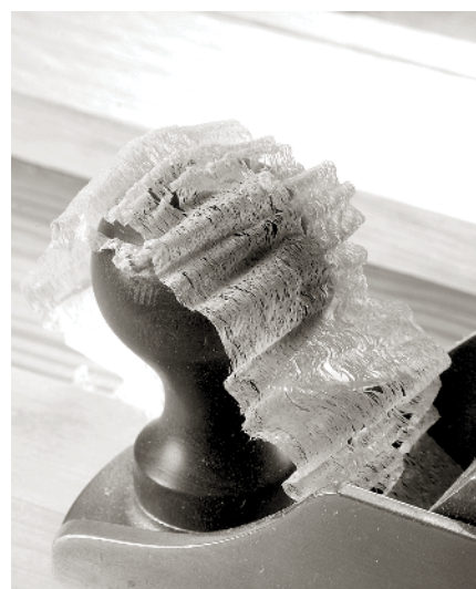
BEFORE I BREAK OUT THE sander I try cutting a shaving such as this one . It takes more passes than I like, but it is less likely to tear the grain.
