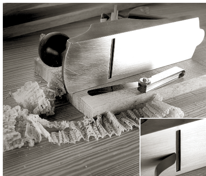
TIGHTENING UP THE MOUTH APERTURE of your plane can help in some cases, but you are likely to increase the chance of clogging up the works.
