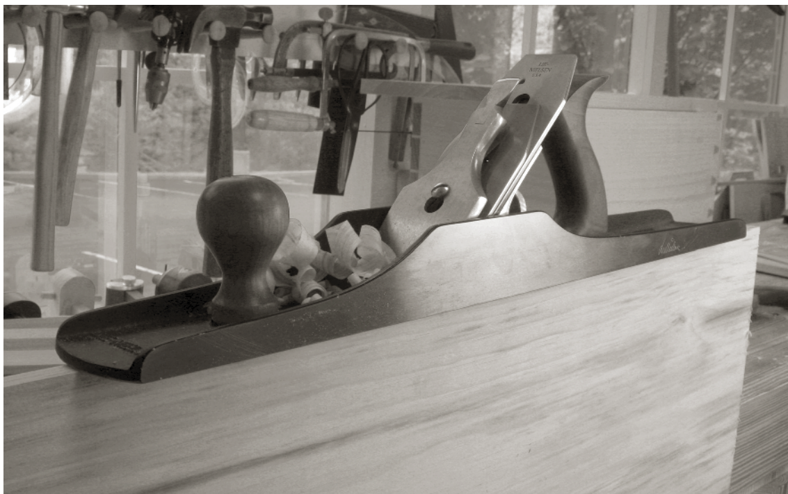
THE NO. 7 IS THE most common size of jointer . However, some people like the additional mass and length of the No. 8 and are willing to pay for it.
