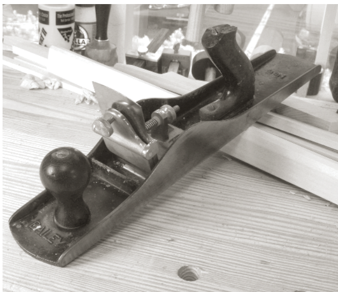
A STANLEY NO. 6 FORE plane with a scraping insert installed. This particular scraping insert is no longer available, though Veritas of Canada makes a similar insert.
