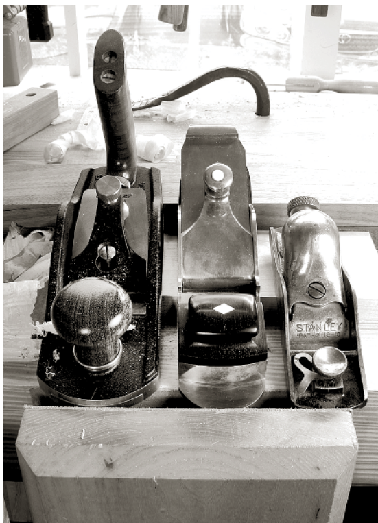
ALL THREE OF THESE TOOLS have their bevels facing up. This fact makes them easy to configure to a high angle of attack. It just takes a little sharpening.
