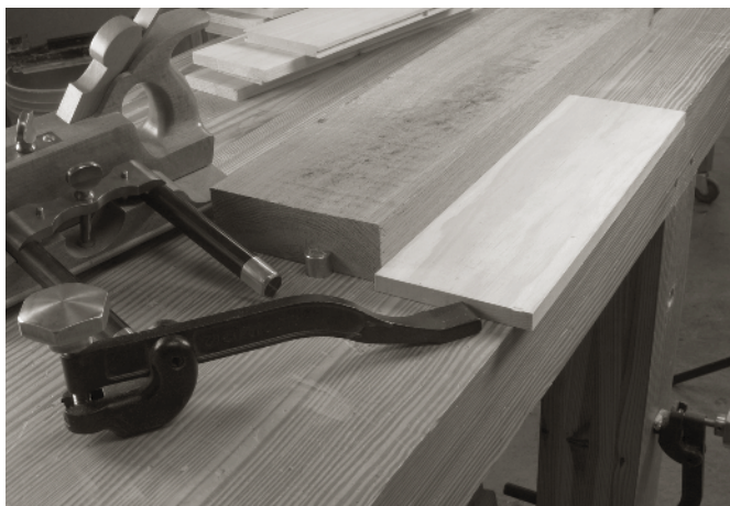
WHEN GROOVING A DRAWER SIDE, this is the setup I prefer. The hold-down acts as a stop. The thick board keeps the board from sliding to the side.
