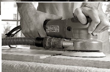
A DRUM SANDER (ABOVE) CAN level and true a panel much like a jointer plane. A random-orbit sander (right) is ideal for removing machining marks in a power-tool workshop.
