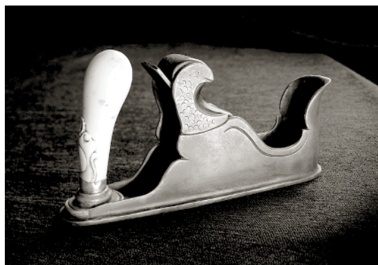
AN UNUSUAL EUROPEAN IVORY-HANDLED PLANE. The plane shows signs of use (lots of hammer taps on the wedge), and its construction suggests it is a scraping plane.
