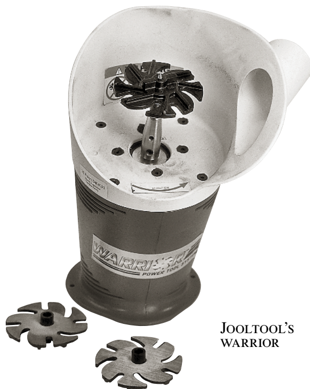
THE 3M TRIZACT SANDPAPER is attached to plastic discs (called Ninja Disc Backpads) that screw onto the machine's spindle. Swapping discs is fast and easy.
