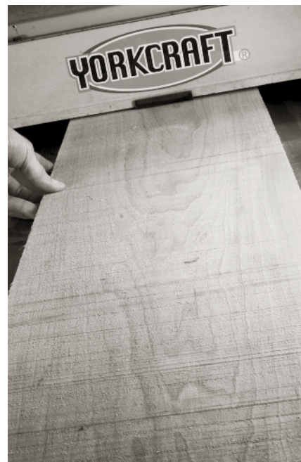
WHEN PLANING THE BOARD, THE heart-side cathedrals should point away from the cutterhead.
