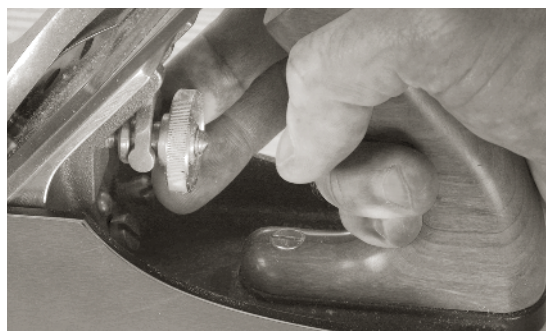
THE BAILEY-STYLE ADJUSTMENT MECHANISM IS (in my opinion) the best. It is robust and located right where you need it.
