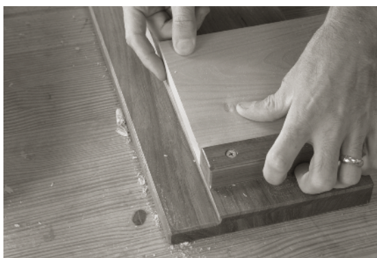
I USE MY FINGERS TO flush up the board on the shooting board with the waste area hanging out over the ramp .
