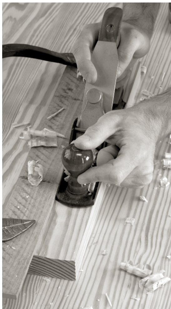
TO MAKE A SANDING STICK, first cut a trench in some softwood with the plane guided by a temporary fence. Then rip a section of the curved shape from the board.
