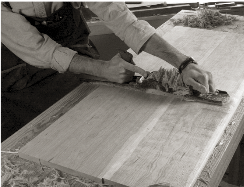
BEFORE YOU TRAVERSE ANY BOARD , be sure to plane a small chamfer on the out-feed edge. Otherwise, the edge will splinter (this is called “spelching”).
