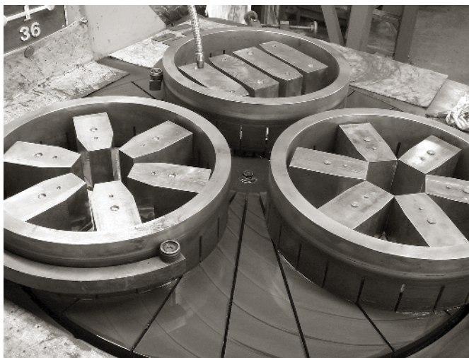
HERE YOU CAN SEE Lee Valley's lapping machine loaded with plane irons. The three rings rotate, as does the giant plate below. An abrasive slurry dresses the irons dead flat.
