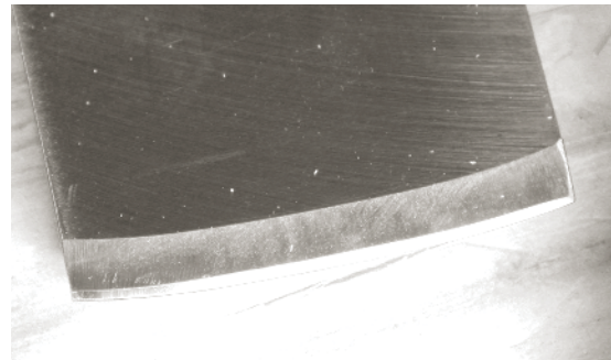
WHEN YOU ARE DONE SHARPENING you should have a nice even secondary bevel.
