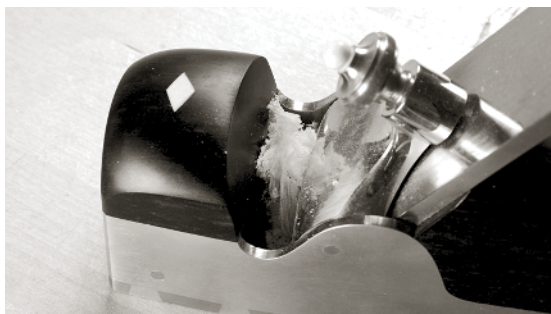
WITH NO CHIPBREAKER, SHAVINGS TEND to collect in the mouth. However, the tool doesn't clog, it just doesn't eject shavings as quickly.
