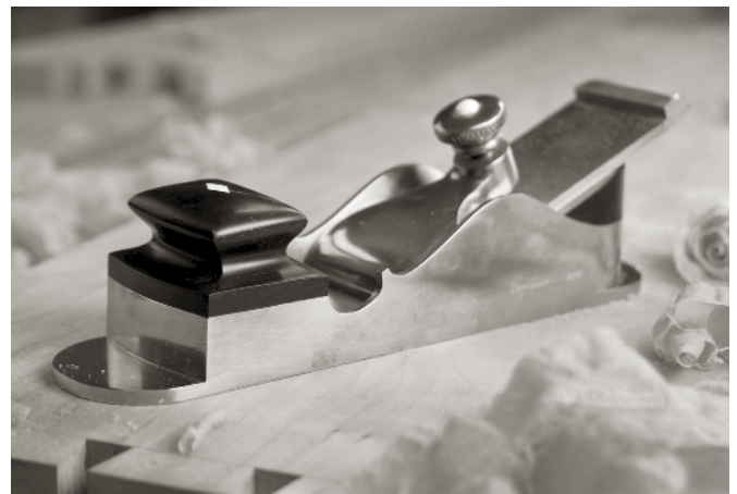
THIS IMPROVED MITER PLANE MADE by Wayne Anderson has been set up like a smoothing plane and performs astonishingly well.
