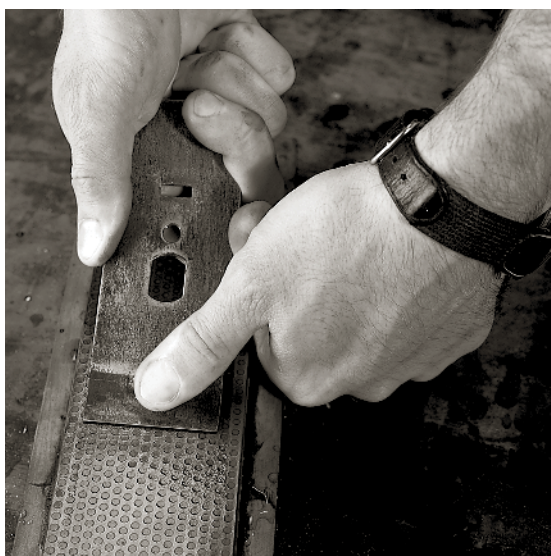
TAKE A FEW MINUTES TO polish the top hump of the cap iron . Anytime you can reduce friction you'll improve planing performance.
