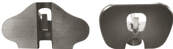
HERE YOU CAN SEE THE two throats of the router planes. The Lie-Nielsen (left) has an open throat. The Veritas has a closed throat.
