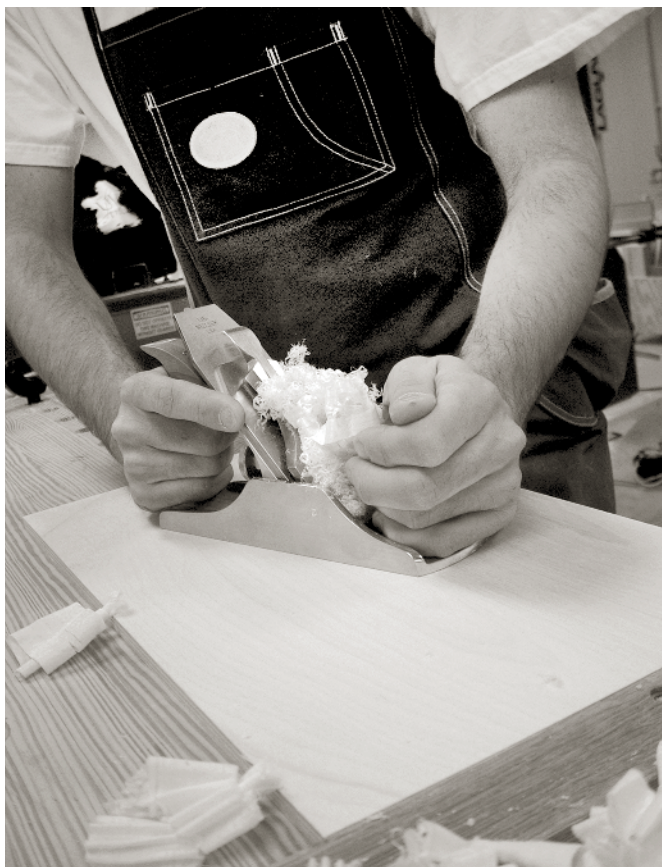
SKEWING THE PLANE BODY DURING the cut can help in tricky grain situations.
