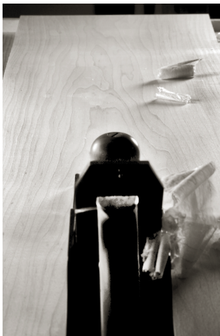
HERE I'M PLANING THE HEART side of this board. The plane is following the cathedrals and the wood is behaving nicely.
