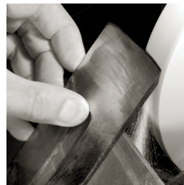
CAMBERING THE IRON ON a fore plane is a task best handled on a bench grinder.
