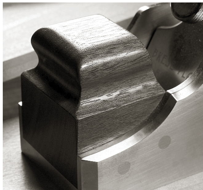
THE WALNUT INFILL ON THIS smoother shows remarkable attention to all aspects of the craft, and it's remarkably comfortable to grasp.
