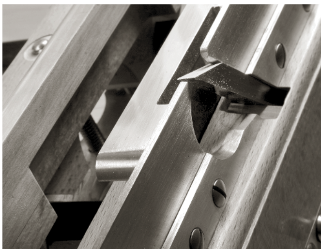
THE SKATE IRON AND DEPTH STOP all come together seamlessly. The tapered A2 irons all seat firmly against the skate and are held securely by the wedge. The set of eight well-made irons is just one of the selling points of this tool.
