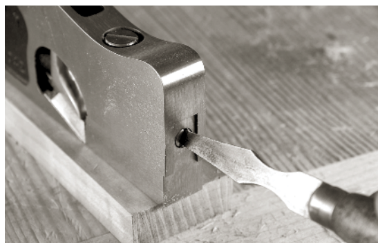
MOST TRADITIONAL SHOULDER PLANES with an adjustable mouth work like the Veritas. Loosen the screw on top of the tool then adjust the mouth with the screw in the toe. Then tighten the screw on top again.
