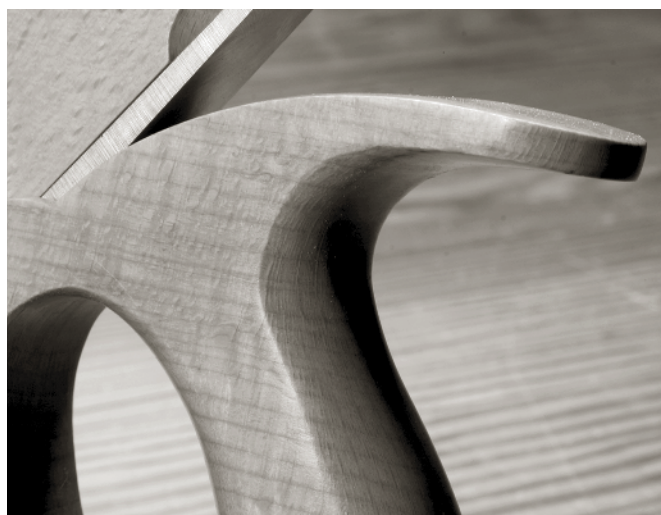
THE BEECH TOTE IS HAND-SHAPED and has no hard lines to nip at your fingers.
