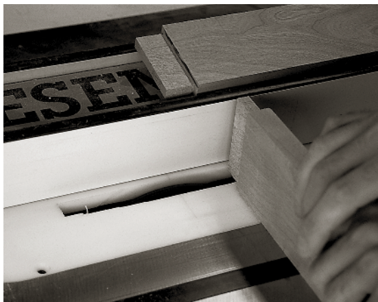
A DADO STACK MAKES QUICK work of tenons for the door. The table saw’s miter gauge guides the rails over the dado blades to cut the face and edge cheeks.
