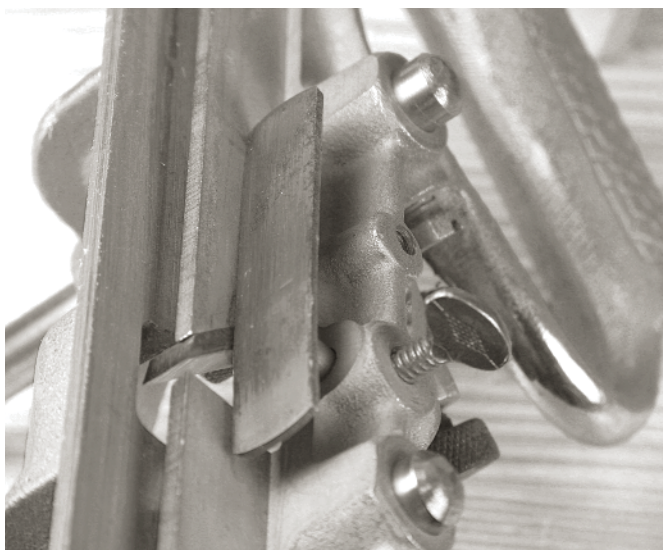
HERE'S THE DEPTH STOP ON the metal plow. It's on the side of the tool that's opposite the fence.
