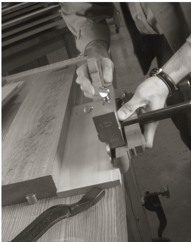
THE FIRST CUT WITH THE plow begins at the end of the board nearest the camera. This helps prevent accidents you cannot recover from.
