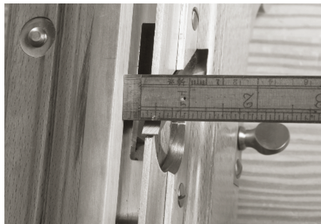
I THINK THE FENCE SHOULD be parallel to the skate of the tool. I'll check it at the toe, the iron and the heel.
