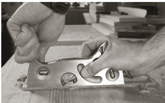
THE RHINO HORN AT THE toe of the tool makes it comfortable to push. The rear grip is intuitive – more so than on most other shoulder planes.
