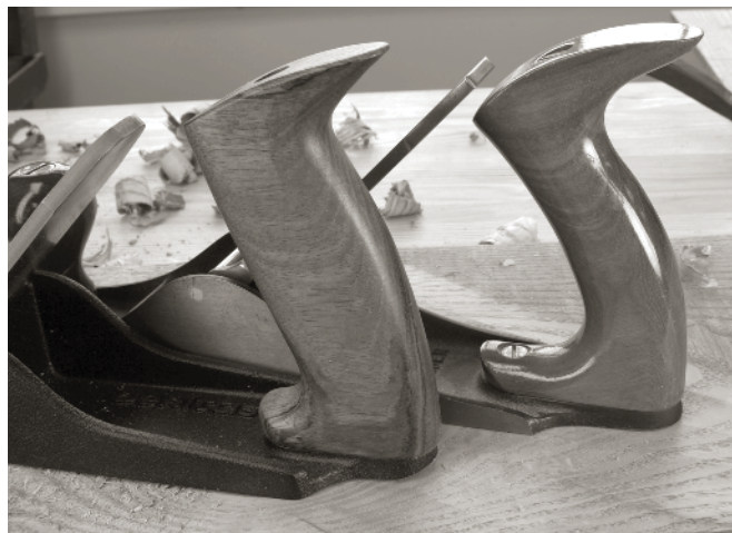
ONE OF THE SIGNIFICANT DIFFERENCES between the two premium scrub planes is in the tates. The Veritas's (left) is wider. Also worth noting is that the Veritas's tote is secured to the plane's body with two screws. The Lie-Nielsen's is secured with one.
