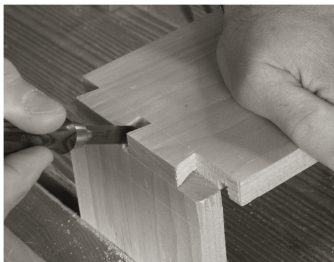
HERE I'M PUSHING THE RABBIT against my pin board. This makes transferring the shape of the tails a can't miss affair.
