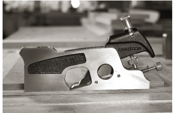
THE VERITAS MEDIUM SHOULDER PLANE shares a lot of the advanced features of the other Veritas planes. It has a modern rear end, but the toe resembles that of old infill shoulder planes.
