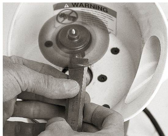
THE PLASTIC DISCS' SHAPE allow you to see the tool's edge as you grind and hone it. Shaping unusual tools is remarkably easy.
