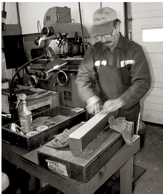
A SURPRISING AMOUNT OF HAND work is involved in building handplanes. Here a Lie-Nielsen employee flattens the unbeveled side of a plane iron using sandpaper.
