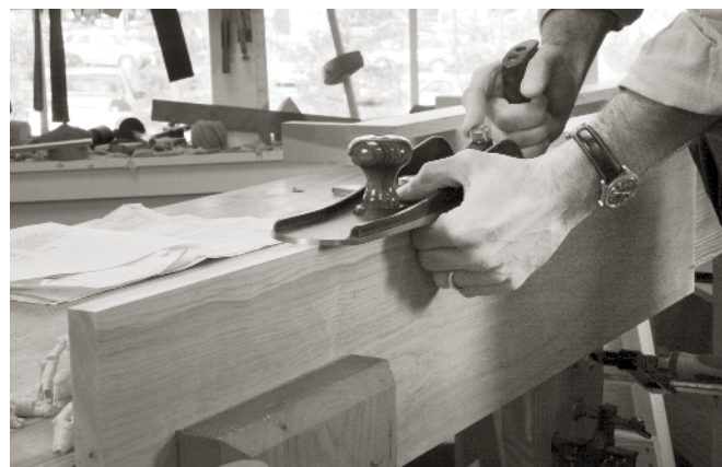
WITH SMALL PANELS (THIS ONE IS 42" LONG) you can join the edges using glue and clamps alone. For longer panels, consider a spline joint or a tongue-and-groove.
