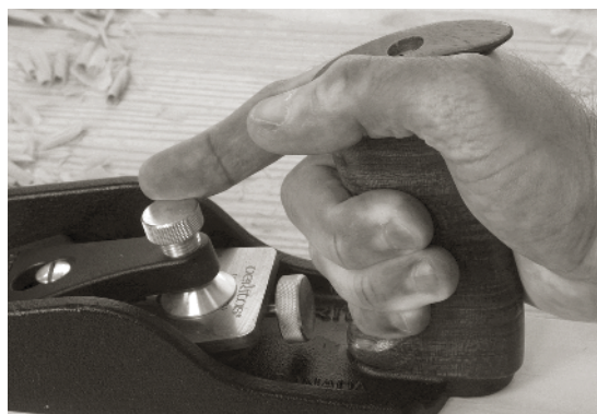
YOU CAN USE A THREE-FINGER grip with some Veritas bevel-up planes, such as this smoothing plane. But most tools encourage a four-finger grip.
