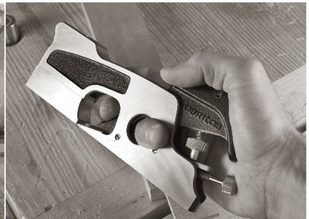
THE VERITAS SHOULDER PLANE PLACES your palm at the rear of the tool instead of above the escapement. This requires a slightly different method of pushing the tool – you'll notice this difference only if you own two different kinds of shoulder planes.
