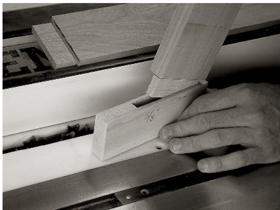
TEST THE FIT OF YOUR tenon in a test mortise. When you’re satisfied with the fit, cut the tenons on all the rails this way, being sure to check the fit after cutting each one.
