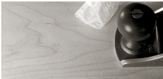
HERE I'M PLANING THE BARK side of a board. Note that I'm planing into the peaks of the cathedrals. Can you hear the barking sound?
