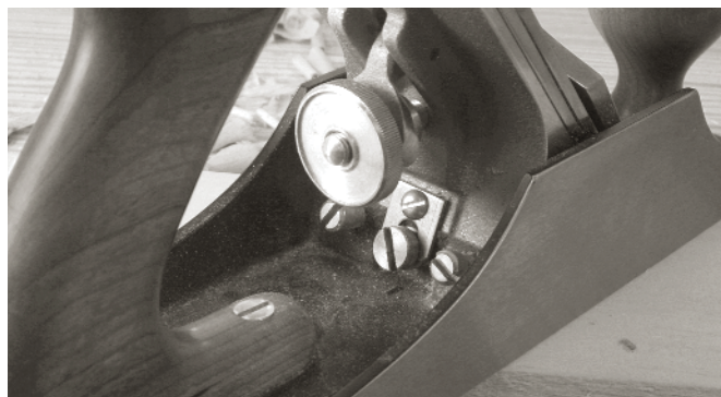
THE BEVEL-DOWN PLANES ARE a pain in the tuckus when it comes to adjusting the mouth aperture. Shown is the nicest system for adjusting the mouth, and it's still complex.
