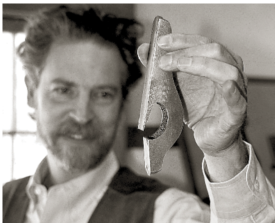
BOTH LIE-NIELSEN AND LEE VALLEY use ductile iron for their plane bodies. This material is nearly unbreakable and stable. Here Lie-Nielsen shows off one of the castings that has been brutalized to show how it won't crack.
