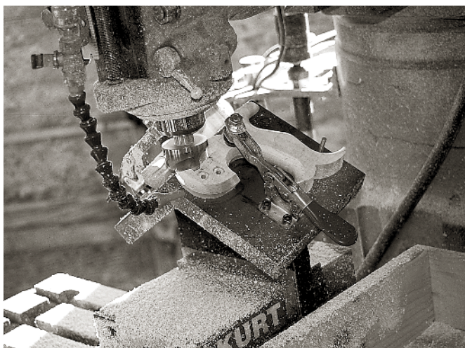
ONE OF THE BIG CHALLENGES for Lie-Nielsen and Lee Valley is to produce handles that are comfortable but that can be made with a minimum of hand work. Here, a Lie-Nielsen saw handle is machined to shape.
