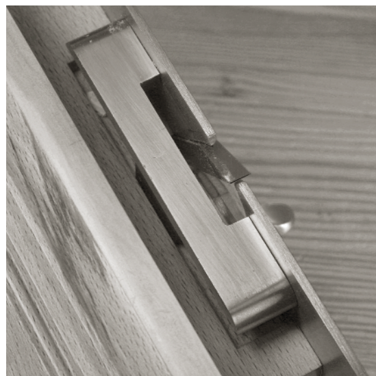
THE DEPTH STOP ON A wooden plow is traditionally between the fence and skate.
