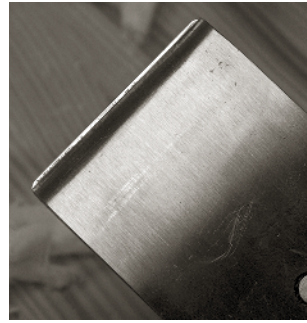
FOR SMOOTHING WORK, POSITION YOUR chipbreaker between \frac{1}{32} " to \frac{3}{32} " from the cutting edge.
