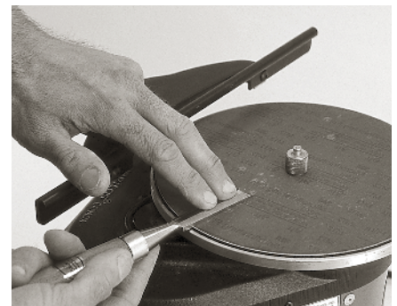
THE Mk. II ALSO ALLOWS you to flatten and polish the backside of your tools and remove the burr on the tool's backside while sharpening.
