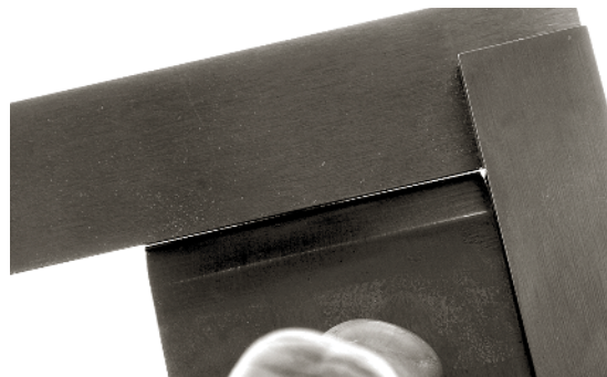
A SILHOUETTE OF A SMOOTHING plane iron. The camber is slight: .002" or maybe a little more.
