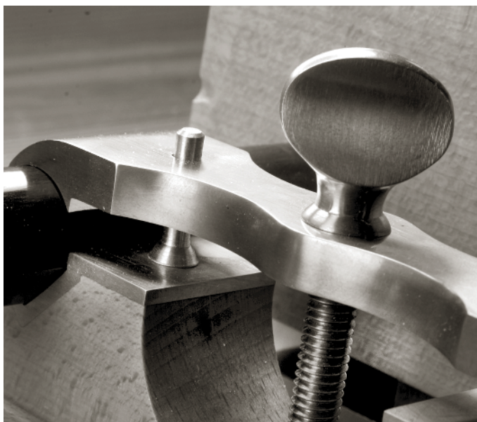
THE BRIDLE MECHANISM IS FLAWLESS in workmanship and in function. The fence locks parallel to the skate every time, which saves an immense amount of fussing.
