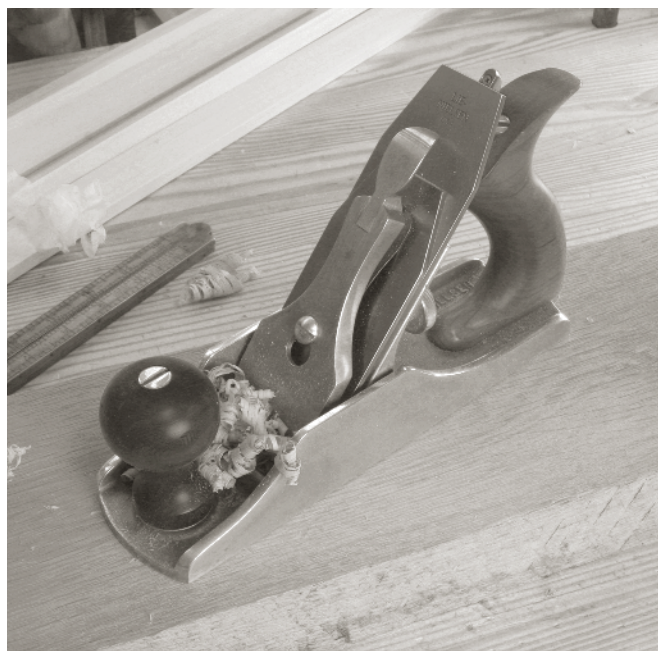
A No. 4 SMOOTHING PLANE is the most common smoothing plane. Why's that? I think it's the most useful all-around size.
