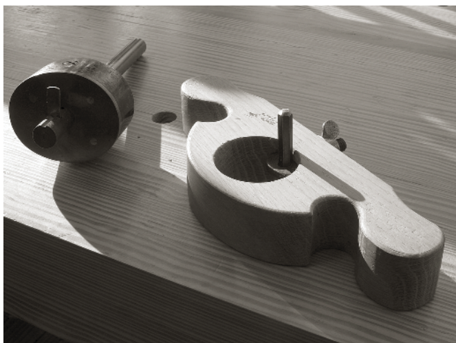
THIS SHOP-MADE D-HANDLE ROUTER ISN'T sophisticated , but it works quite well and can be built to suit any custom application. This model was built using an Allen wrench as a cutter – which is just the right hardness for the task.
