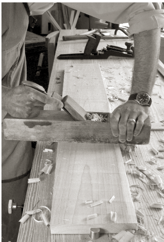
PLANING ACROSS THE GRAIN IS easy to do . Work the high spots until they're the same as the low spots on one face of the board.
