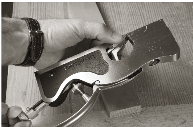
WITHOUT A LATERAL ADJUST LEVER, you must rely upon your ability to test the iron's position with your fingers or sliver of wood.
