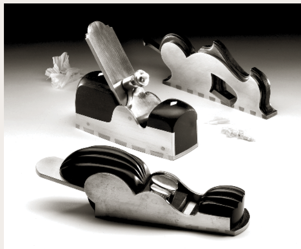
THREE WAYNE ANDERSON PLANES: A rhino-horn shoulder plane (rear), a coffin smoothing plane and chariot plane.
