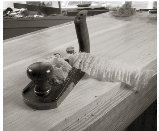
A WELL-PREPARED PANEL SHOULDN'T REQUIRE more than a few minutes with the smoothing plane to dress. As a bonus, you won't have to sharpen or adjust your smoothing plane as much.
