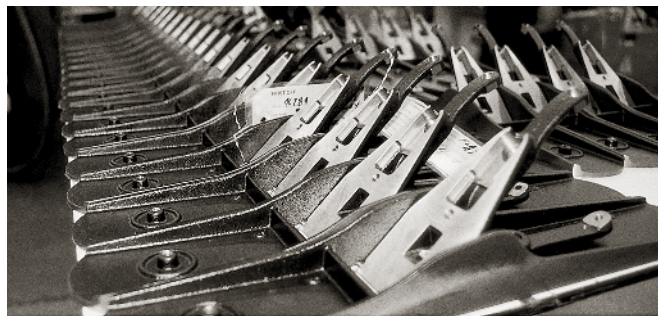
VERITAS NO. 6 FORE PLANES after the frogs have been machined. Unlike a traditional No. 6, the Veritas has its mouth located further back than the Stanley versions.
