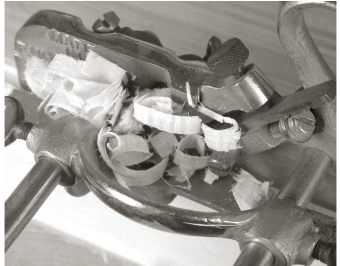
THE SHAVINGS IN A METAL plow tend to bunch up between the fence and the tool's body.
