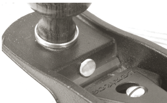
WITH BEVEL-UP PLANES, YOU TWIST the front knob of the tool, move the throat plate and twist again to lock it. The small brass wheel is a stop for the mouth to prevent you from striking the blade with the mouth.
