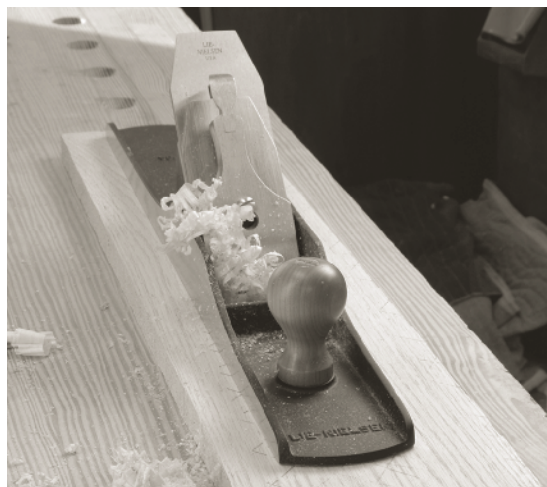
THE JOINTER PLANE EXCELS AT truing stock , both the long edges and faces of boards. The pencil marks on the wood in the photo are low spots found by the plane after two passes over the board – which was fresh from the planer.
