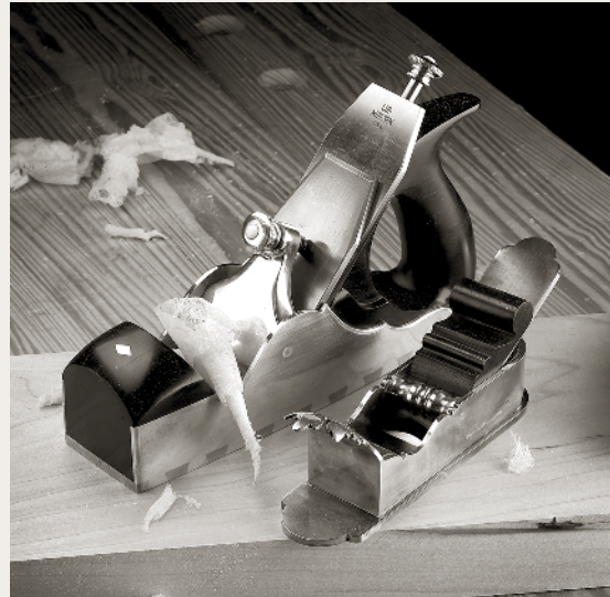
TWO PLANES FROM WAYNE ANDERSON: A full-size smoothing plane with ebony infill (top) and a small plane inspired by some of the earliest metal-bodied planes from Europe.
