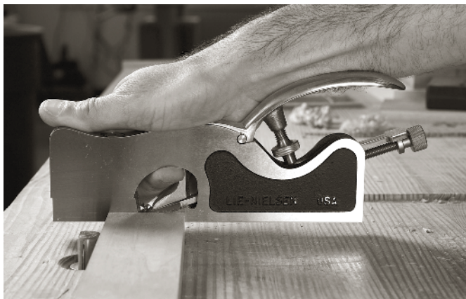
A ONE-HANDED GRIP MAKES MY right hand look a bit claw-like. But this does focus the force of your hand right over the cutting edge, a major advantage when working the tool.
