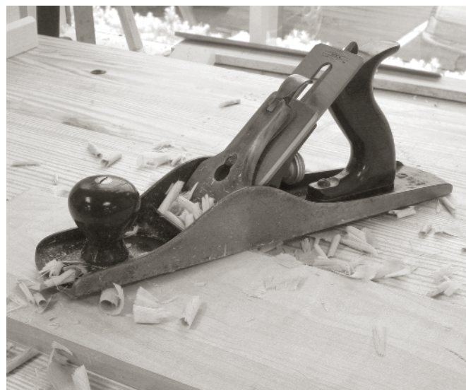
A STANLEY NO. 5 JACK plane. This tool was the most popular size sold. Why? Because it can be used for almost anything.
