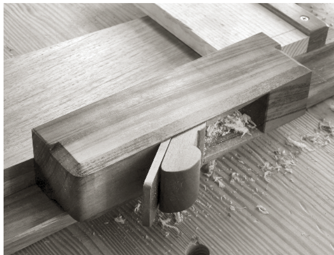
THE PHILLY PLANES MITER PLANE excels on a shooting board, as shown here.
