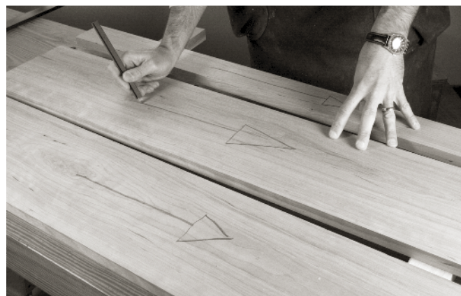
I USE LARGE ARROWS TO indicate the grain direction on the faces of all the boards. Bold marks help ensure you won't make a mistake at assembly.
