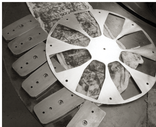
THESE INSERTS HOLD THE PLANE irons inside the rings of the lapping machine. The weights press the work against the abrasive.
