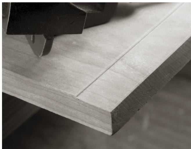
HERE'S THE COMPLETED RABBIT. It's less than \frac{1}{32} " and a bit more than \frac{1}{64} ". It's all you need.
