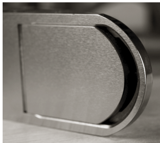
WITH MOST BLOCK PLANES THE sole plate is visible from the front of the tool. The Veritas designers went all out and captured the plate in the plane's body.
