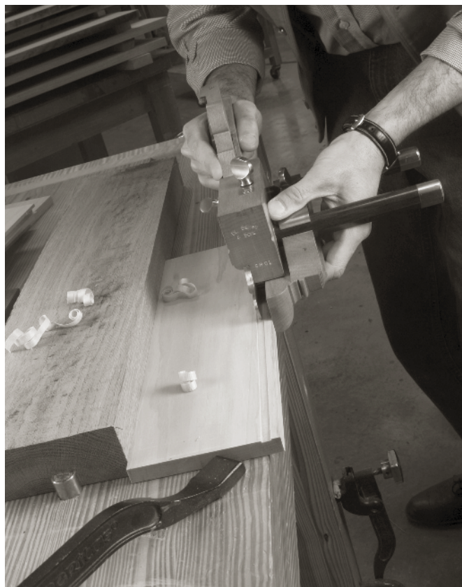
EACH STROKE IS A LITTLE longer until you are plowing the entire board. Keep the skate in the groove – it's faster.
