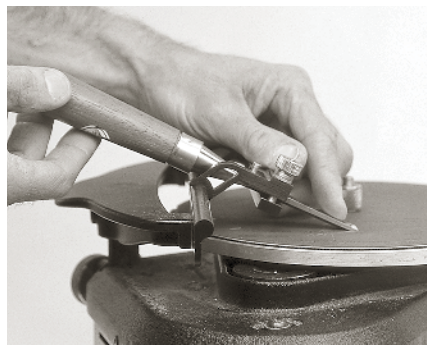
LIGHT FINGER PRESSURE IS ALL it takes to hone a polished edge quickly and easily on the Veritas machine.
