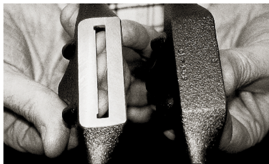
MODERN PLANES HAVE FAR MORE machining than vintage tools. On this Veritas spokeshave, the mouth and sole are milled out on precision equipment. This extra work means less blade chatter for woodworkers.
