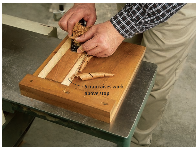
Bench hooks can be used almost anywhere (such as on the bed of this jointer) and can do some surprising tasks. Here it is being used as a small planing board. The light-colored scrap below the work raises the work above the bench hook's stop.
