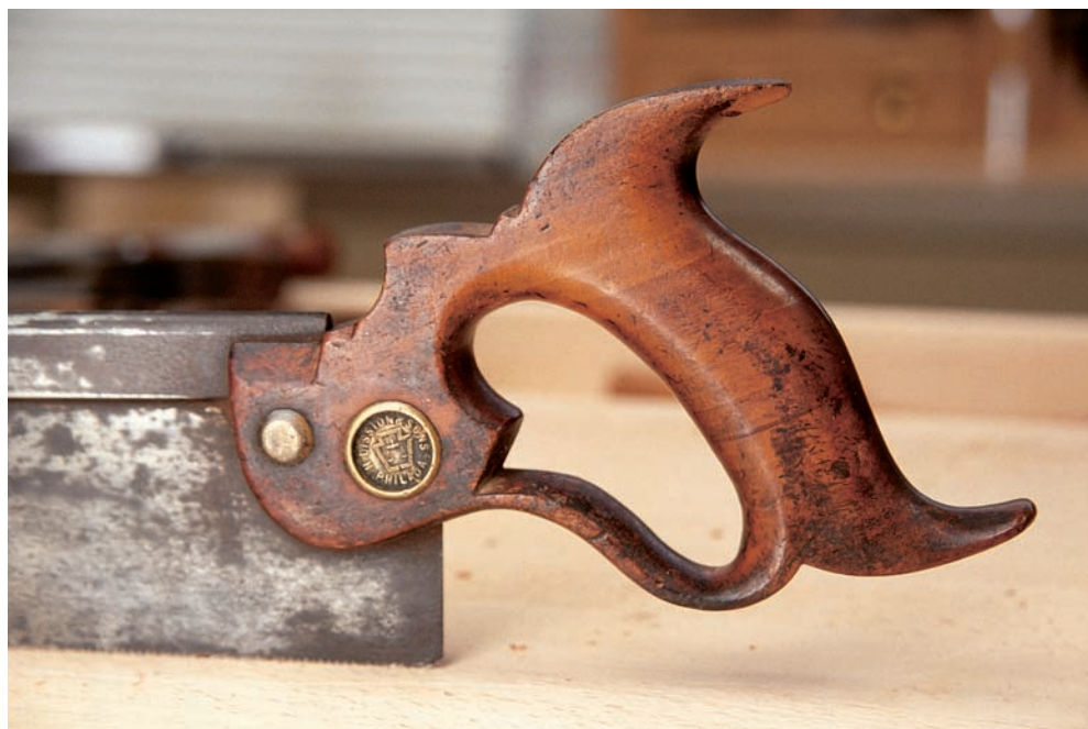
This $18 Disston No. 4 backsaw cuts incredibly well now that it has been properly sharpened. The handle on vintage Western saws will fit your hand like a glove. Later handles are uncomfortable to use and look crude by comparison.
