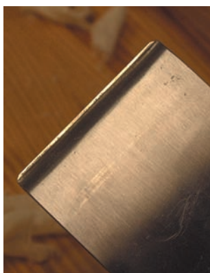
For smoothing work, position your chipbreaker between \frac{1}{32} " to \frac{3}{32} " from the cutting edge.
