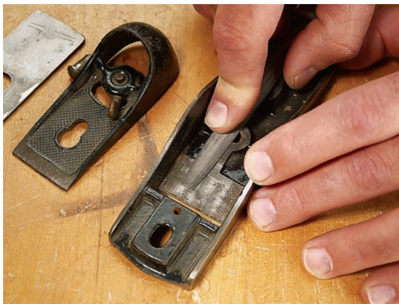
A small mill file can rescue the bed of an inexpensive plane by ridding it of any defects. However, a light touch is key. You can easily overdo it.
