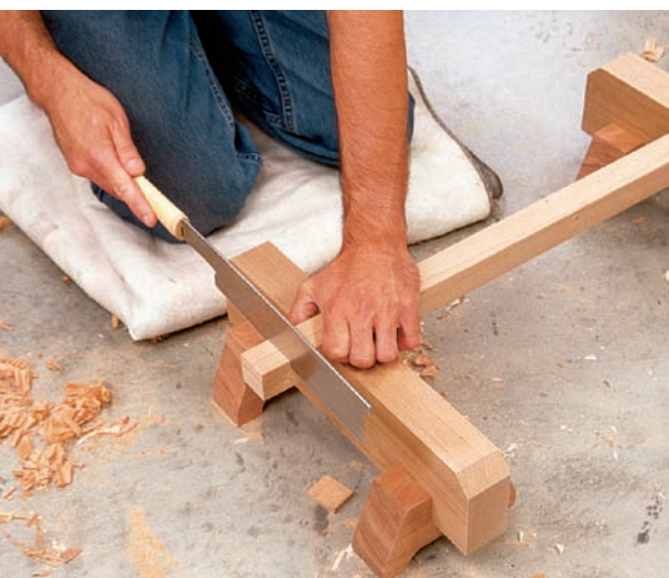
For crosscutting in joinery, the Japanese will use a dozuki saw (which means “shoulder of a tenon”). There are various ways to grip the saw.
