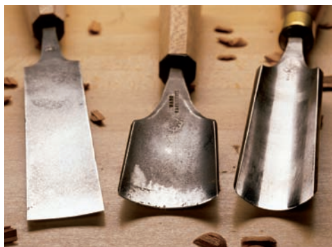
Bench gouges are available in three sweeps: (from left) flat, middle and regular. The regular sweep is the most useful for general work.
