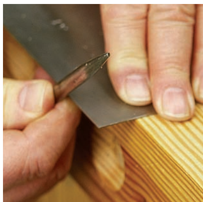
Next, hold the burnisher square – perpendicular to the face – and rub the edge.
