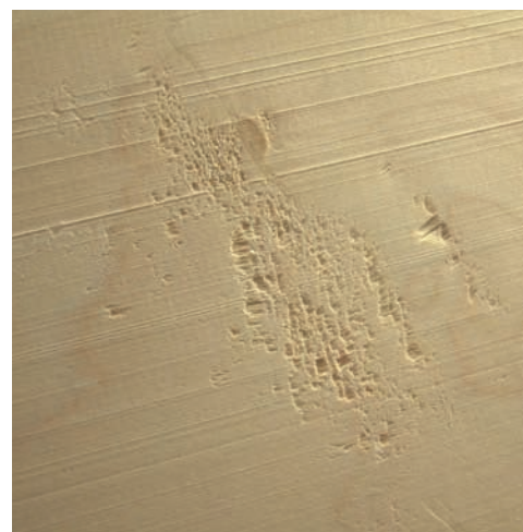
This is what tear-out looks like. Avoid it. When a finish is applied, it looks terrible.
