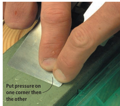
To sharpen an iron for smoothing, work the corners on your sharpening stones. This will give your cutting edge a bit of a camber – which is perfect for smoothing.
