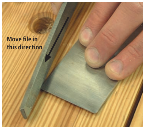
To avoid “plane tracks,” clip the corners of your iron by filing a tight radius on the corners of your cutting edge.
