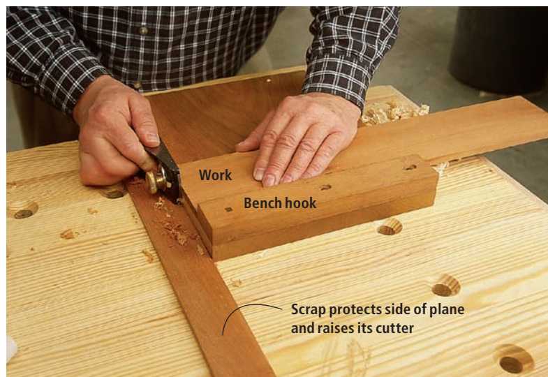
The bench hook makes an effective shooting board for truing the ends of small pieces. The piece of scrap below the plane protects the side of the tool and centers the tool's cutter on the work.
