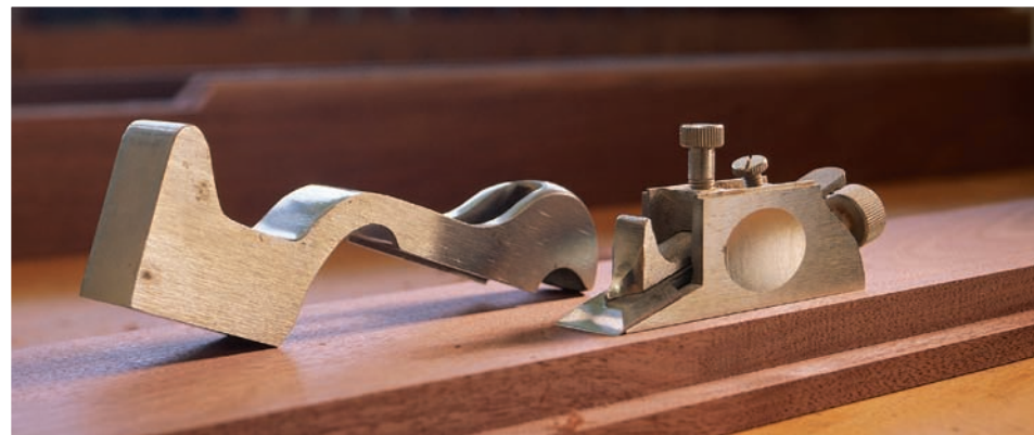
Some shoulder planes, such as the Stanley No. 92 shown here, feature a removable front piece, which transforms the tool into a useful chisel plane.
