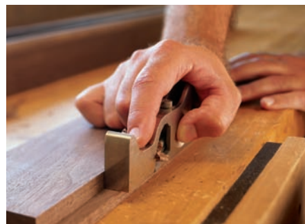
Because the sides of a shoulder plane are open, it's easy to trim into corners of rabbets.
