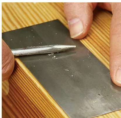
The first step in burnishing is to consolidate the edge by running the burnisher flat on the face.
