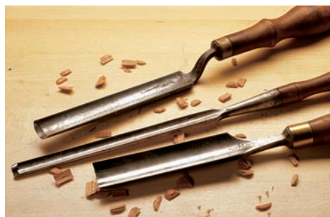
The three types of gouges for cabinetmaking are, from top to bottom, the cranked gouge, the paring gouge and the firmer gouge. The paring gouge is in socket form, while the other two are in tang forms.
