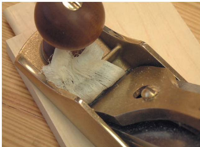
See how the shaving emerges only in the middle of the iron? That's how you know your iron is sharpened and set correctly.
