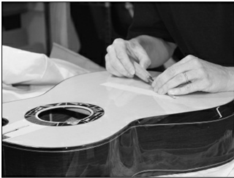
FIGURE 3.4.7. Once we've completed the scribe line, we chisel away the finish to the scribe line.
