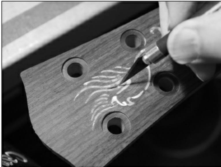
FIGURE 1.4.103. After sanding the inlay flush to the headstock surface, you will typically find some gaps that weren't filled with glue. These gaps (some large and some very small) will often be filled with white powder from the inlay dust after sanding. Clean the gaps with an X-ACTO knife, blow the area clean with compressed air, reapply the brown Sharpie ink, and put more superglue into each gap.
