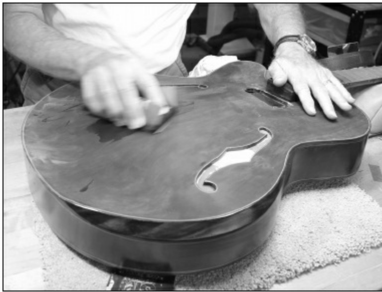
FIGURE 2.2.30. This photo shows the guitar being sanded after spraying. Due to the curved surfaces, we will usually sand an archtop by hand. However, the sanding schedule is the same as it was with the steel string. We'll start with 600- or 800-grit paper (wet sanding), depending on how smooth the surface is, and proceed to about 1200 before we start buffing.
