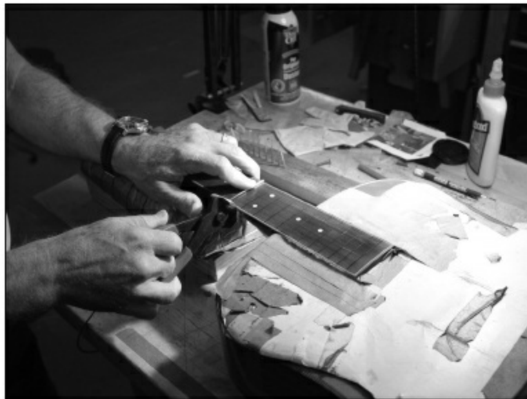
FIGURE 1.7.41. As each of the frets is cut, they are placed in a board as shown with numbered holes responding to each fret. This helps us keep each length of fretwire assigned to the proper fret.
