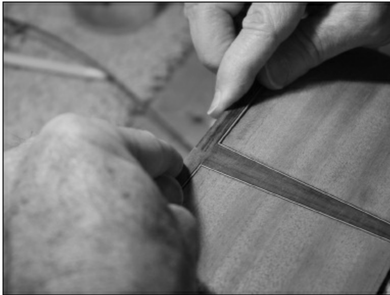
FIGURE 1.3.79. After a little fitting between the edges of the purfling angles and the ends of the bindings and after sanding on the disc sander, we make all the edges line up.
