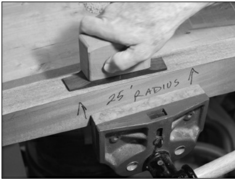
FIGURE 1.5.32. Here is the bridge, held in place with the handle above, getting a 25' radius sanded onto its underside. The 25' radius jig is simply a mahogany board about 2' long, with a 25' radius sanded onto one edge, covered with sticky back sandpaper. This step will reduce the thickness of the bridge by about \frac{1}{32} ". At this point the bridge is done, with the exception of some final shaping and rounding of the sharp edges that we will cover in chapter 1.7.
