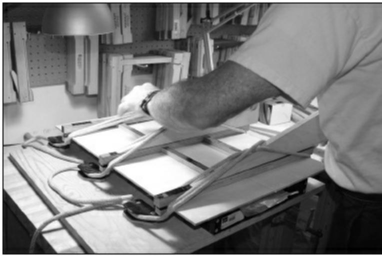
FIGURE 1.1.7. Finally, we put wedges between the ropes and the frame. This will do two things. It will pull the two sides together and push the halves of the top down, making sure neither side climbs up during the gluing process. After you put the wedges in, tap them with a rubber mallet to be sure they are seated as well as possible.
