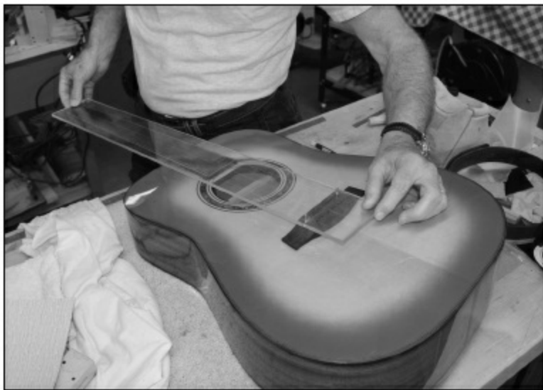
FIGURE 1.7.2. Next, we check the neck alignment with our neck template. This template allows us to check the centerline of the fingerboard with the center seam of the guitar top.
