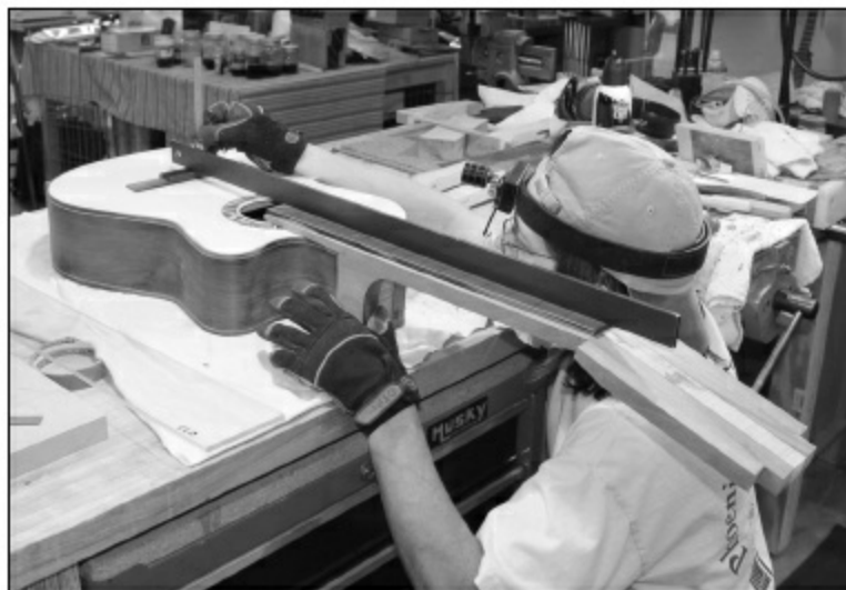
FIGURE 3.2.4. After initially shaping the fingerboard extension, we start to drop the dovetail into its slot. As we carve the dovetail, we continuously check the neck alignment from left to right (as we did on the steel string and the archtop) and vertically by putting the fingerboard down on the neck (it's not glued on yet), using a straightedge to check its height against the bridge. We want the height to align lower than it does with the steel string—about 1/8" below the top of the bridge in this case (without the saddle). The classical alignment is lower on the bridge, because typically, classical players like their action significantly higher than that of a steel string player. This will keep the saddle from being too high.
