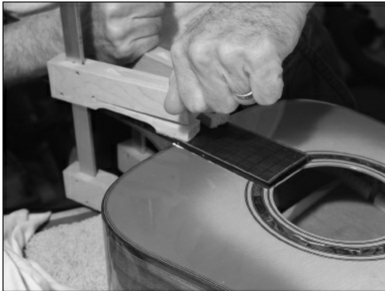
FIGURE 1.7.9. We apply two clamps at the edge of the guitar back to about the fourteenth fret slot. We want the clamping pressure to be as vertical as possible. You can see glue squeeze-out already starting to form under the clamps.
