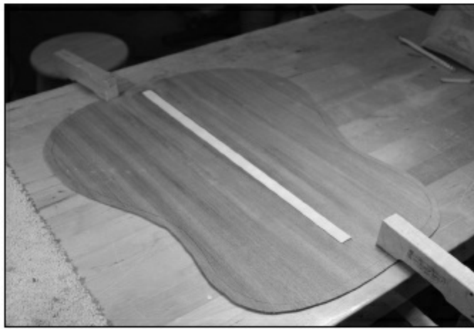
FIGURE 1.2.13. This photo shows the center strip, sanded and ready for back braces.
