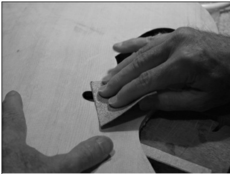
FIGURE 2.1.29. Once the two long legs of the F-hole (the ones with the loops) are bound and the glue is dry, sand them flush with the top and underside with sandpaper.
