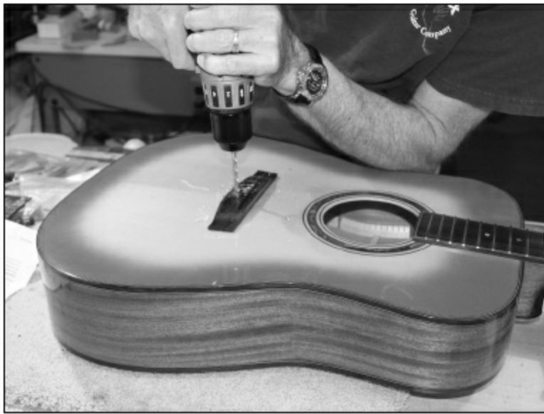
FIGURE 1.7.78. Now, we will prepare the bridge side. First, we finish drilling the bridge pin holes using a 3/16" drill bit.
