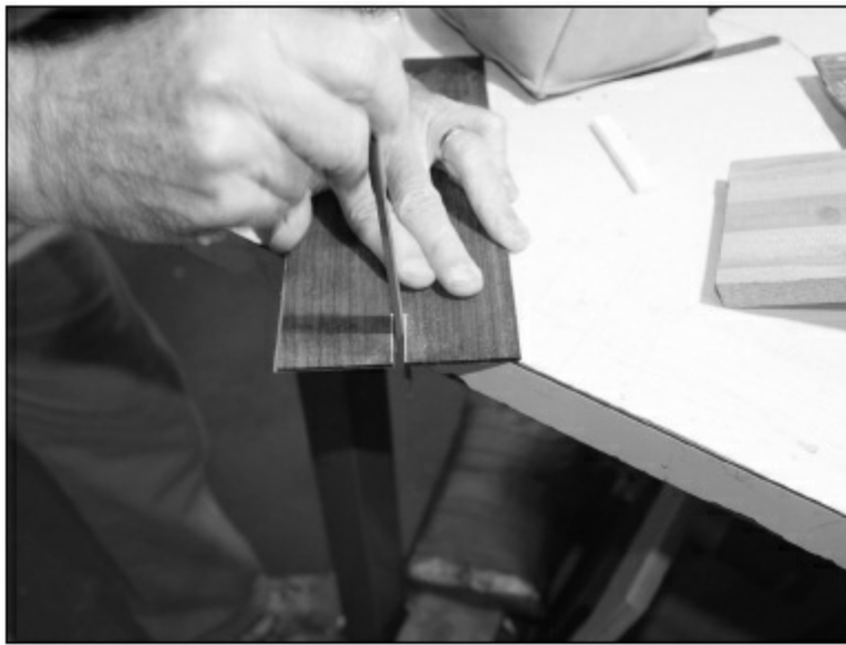
FIGURE 1.4.71. We file the band-sawn edges and check the headstock laminate frequently on the headstock to make sure we don't file too far.
