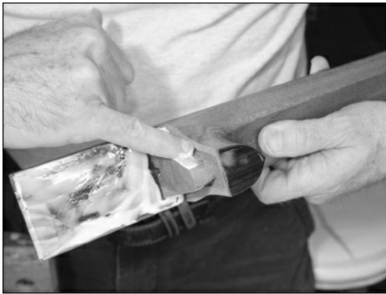
FIGURE 1.7.8. Now we're ready for gluing. The fingerboard overhang has glue already applied, and glue is being spread on the dovetails.
