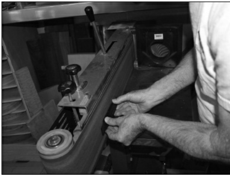
FIGURE 1.7.20. In the last view we had of the bridge, it still had sharp edges (just as it did when it came out of the final shaping jig as described in the chapter on the steel string bridge). Before we glue it down, we want to do some hand shaping and round the edges to soften the shape of the bridge. Here, we are using a belt sander to take off some of those sharp edges.
