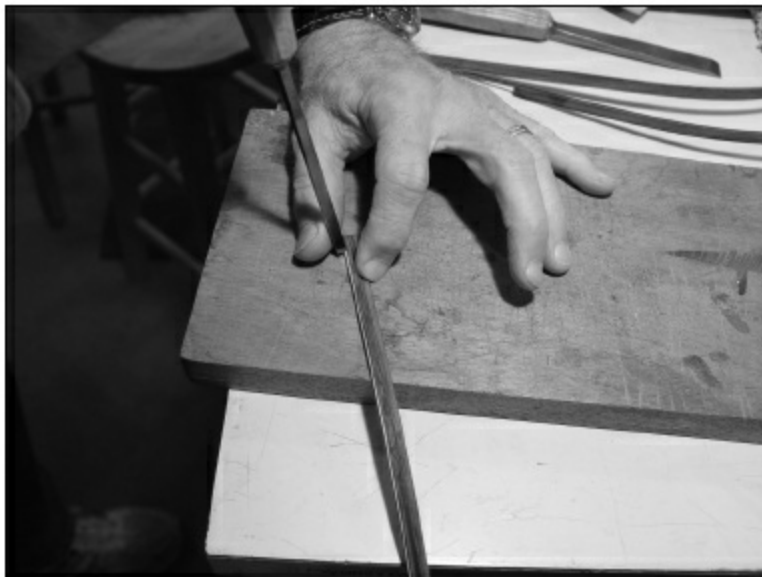
FIGURE 1.3.77. Now the purfling on the bottom edge of the binding is cut at nearly a 45-degree angle at the point where the end graft purfling meets the end graft purfling.
