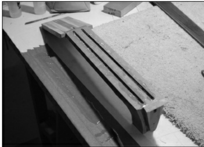
FIGURE 1.4.54. Here are the rods glued into place. We have put a few strips of masking tape down onto the bench to mix the epoxy. This tape will easily pull up after the glue is set up, and cleanup is easy.
