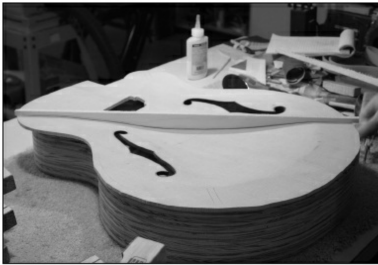
FIGURE 2.1.42. Here is the roughsawn brace placed into the top. The top is cradled in the work board where it will be clamped down, and the brace will be sanded to match the shape of the arch.
