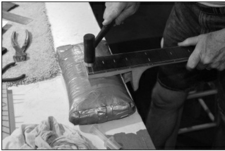
FIGURE 2.2.26. We use a bag filled with lead shot to stabilize the fingerboard extension as the frets are pounded in. For the rest of the neck, we will pound in the frets as we did for the steel string guitar.
