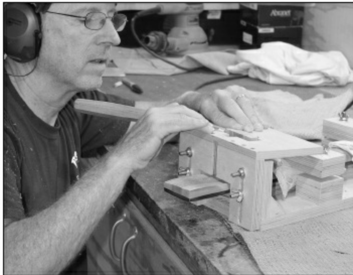
FIGURE 2.2.22. Here is the neck, put into our jig for cutting the heel in preparation for the heel cap. We are using the chisel to check when the alignment mark is directly aligned with the top of the jig (just as we did with the steel string heel cap cut).
