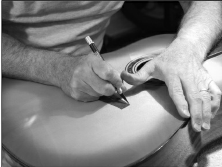
FIGURE 1.7.13. Once the neck and fingerboard have been clamped for about forty-five minutes, it's time to scribe for the bridge. Actually, Franklin—the maker of Titebond—says that you only need to leave the wood clamped for about twenty minutes. We tend to be conservative in this area. In this photo, we're scribing around the tape that marks the bridge location.
