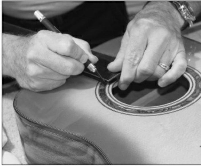
FIGURE 1.7.4. Once our alignment is correct and the neck is clamped down (not glued), we use an X-ACTO knife to scribe around the fingerboard, where it will be glued to the guitar top. Note: we like to use the back of the X-ACTO blade, because it gives us more control. Do not try to scribe with long strokes, since this is a good way to make a disastrous mistake. Make very short, controlled ( 1/4'' or so) strokes.
