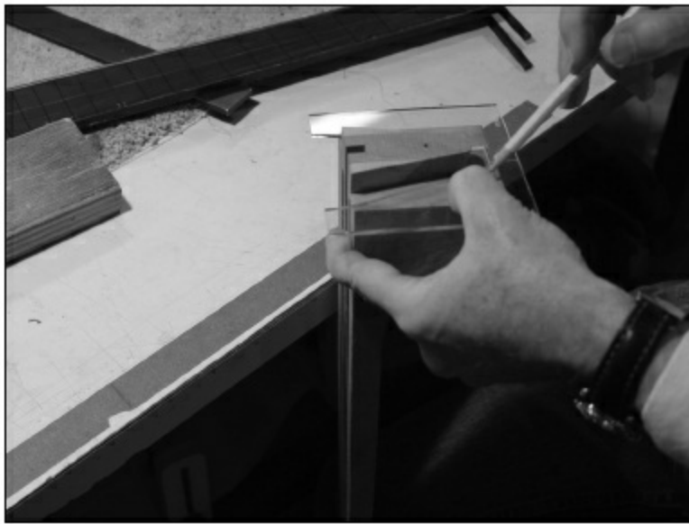
FIGURE 1.4.49. We are using a plexiglass template showing the shape of our neck heel. We will use this shape as we carve the heel.
