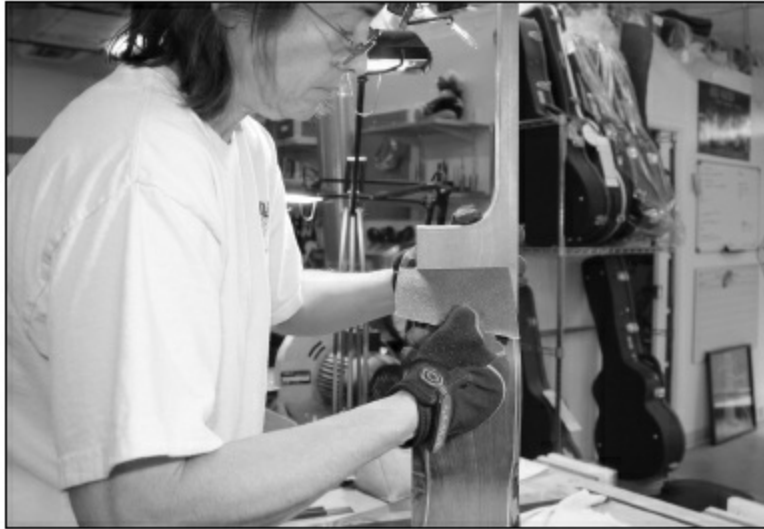
FIGURE 3.2.6. In addition, to be sure the left to right alignment is correct, we will pull some sandpaper on one side or the other, depending on the misalignment. We want to get this alignment as close as we can before we glue on the fingerboard.
