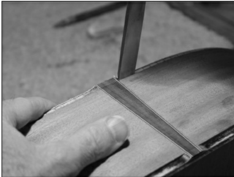
FIGURE 1.3.69. The curved section created by the bit diameter must be cleaned out with a chisel. First, use the flat part of the blade to extend the flat portion of the binding cut up to the end graft purfling.
