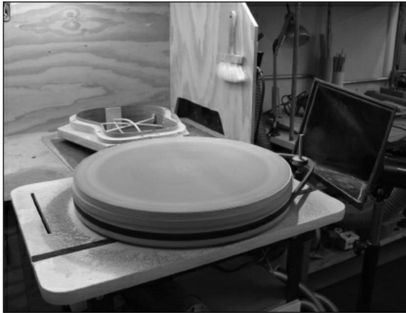
FIGURE 1.3.19. We use this is jig to sand down the sides to their proper profile. We got the idea for this jig from John Greven. Many thanks to John for his permission to show the jig here. We use different hollow form molds for the sanding surfaces. Since the back of the guitar has a 15' radius, we use a 15' hollow form, and for the top, we use a 25' form.
