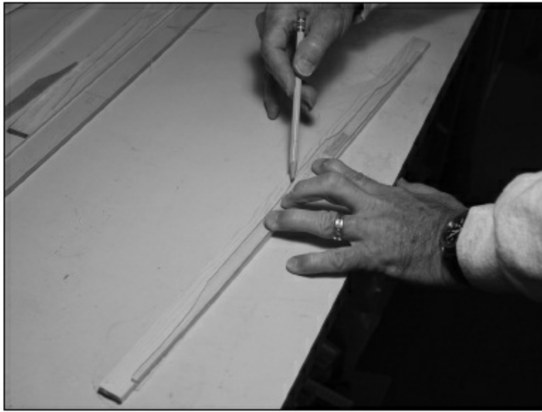
FIGURE 1.1.35. We have a template of the top of each of the braces. It is time to draw the top pattern onto each of the braces and cut it roughly on the band saw, leaving plenty of room for error.
