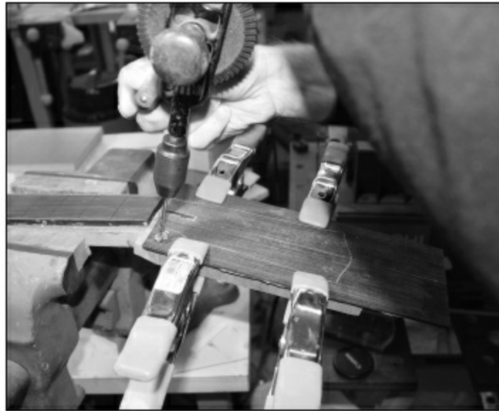
FIGURE 1.4.74. Now we clamp down the headstock laminate and drill a couple of holes on the outer corners of the headstock ears outside the area of the drawn headstock. You could also drill through the location of the tuning machines. The holes are 1/8'' .
