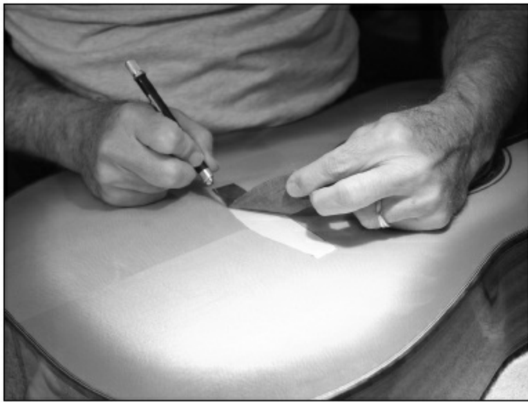
FIGURE 1.7.14. After you cut around the tape, lift a corner and start to peel the tape. You may need to cut more if you didn't cut all the way through the finish the first time. Remember to peel the tape toward the bare spot.
