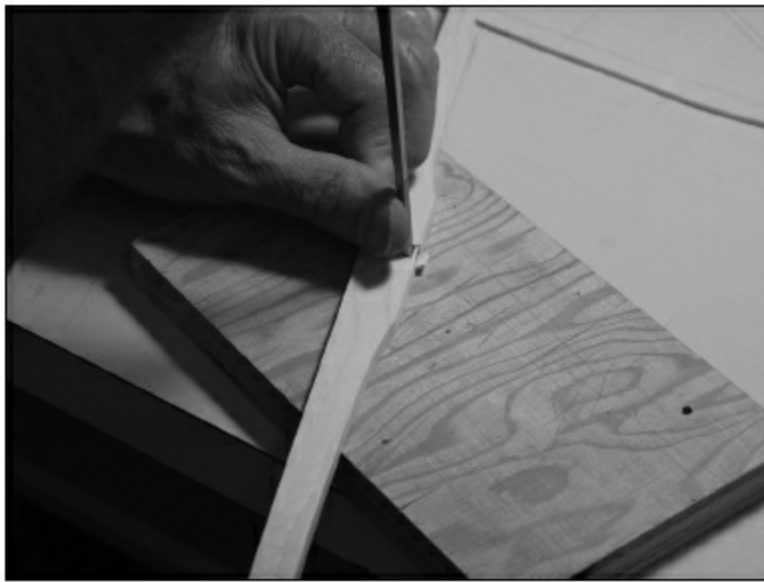
FIGURE 1.1.41. After cutting both lines, we use a chisel to cut out the center part.
