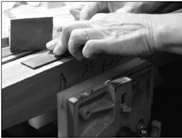
FIGURE 3.3.17. Next, we sand the 25' radius onto the bottom of the bridge using the same radius sanding block we used for the steel string bridge.
