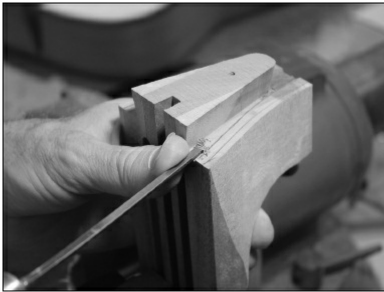
FIGURE 1.4.51. Here is the carved heel (slightly oversize). You can see that the outer drawing is the template tracing made above. The inner line is the point where we will carve away a shelf from the line up to the dovetail. This means we only have a thin shelf to meet the guitar side as the neck is fit. It would be a much more difficult fit if the entire flat area needed to be fit to the guitar sides.
