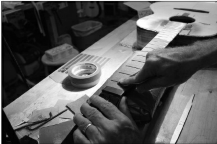
FIGURE 1.7.67. We now sand the frets with Micro-Mesh. We start with 1500 grit, then use 1800, 2400, and 3200. This will make the frets very shiny and ready for playing.
