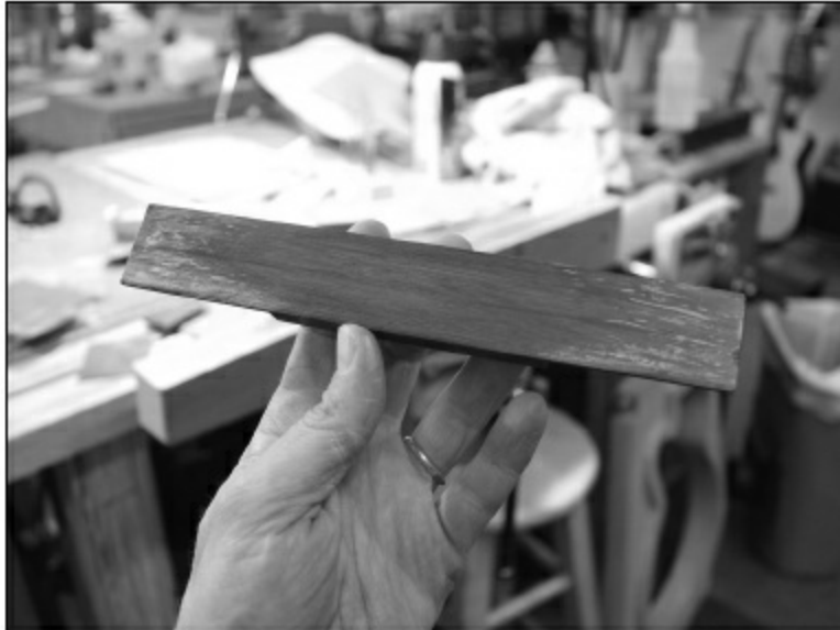
FIGURE 3.3.18. After some sanding, the bottom of the bridge is chalked and resanded to check progress. The photo shows there is more sanding to be done. Once the bottom of the bridge is completed, the top of the bridge is sanded from 220 grit to about 600 grit.
