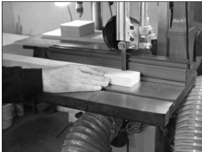
FIGURE 1.1.31. Next, we will saw off a few pieces of the brace stock—each a little over \frac{1}{4} " (actually, a little over \frac{5}{16} " to be safe). After sanding, we want the braces to be \frac{1}{4} " wide.
