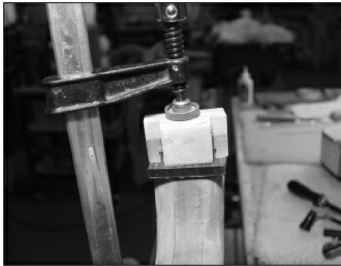
FIGURE 2.2.23. Here is the heel cap being glued down. Note the brads (the same type we use with the fingerboard) that hold the cap in place during gluing. These brads are placed so they are outside the area of the final heel, and the holes will be carved away. We also align the other side of the cap (that goes against the guitar) flush with the guitar side of the heel—though alignment is never absolutely perfect, and a few pulls of sandpaper are typically necessary to get the overall fit perfect. Also note the special caul made for this purpose that allows us to give pressure to the maximum area.
