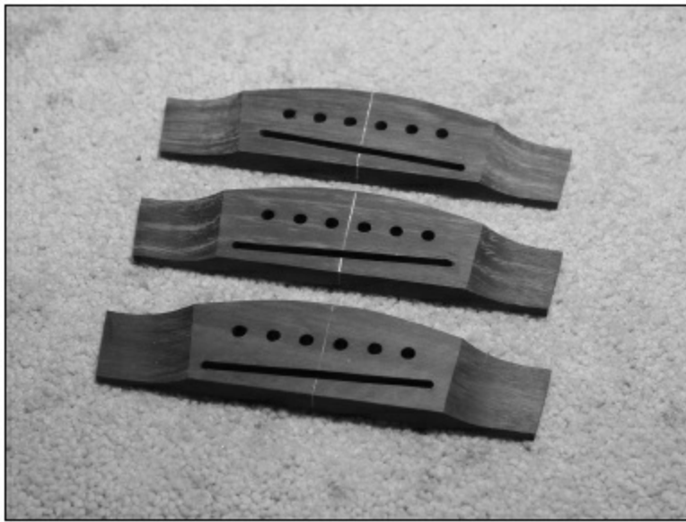
FIGURE 1.5.30. Here are the three bridges we started to make—two right-handed and one lefty—all virtually identical in dimensions. The final step for these bridges is to sand a 25' radius on the bottom of the bridges (since the guitar top will have a 25' radius), and soften the harsh edges created by the router and sander and do a little shaping of the bridge top.
