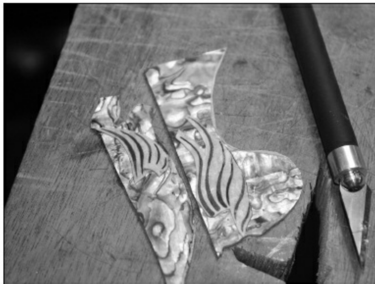
FIGURE 1.4.94. Here are all the pieces of the bird's body, cut out and filed. We have placed them on a board with masking tape, sticky side up, to keep the MOP pieces in place.
