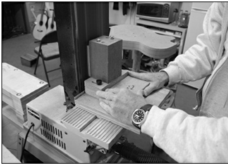
FIGURE 1.3.16. Here is the entire jig with an endblock blank tape with double-stick tape to the block on top of the jig. This block is rotated against the metal edge, and we'll sand the proper radius onto the endblock once the jig is properly set up.
