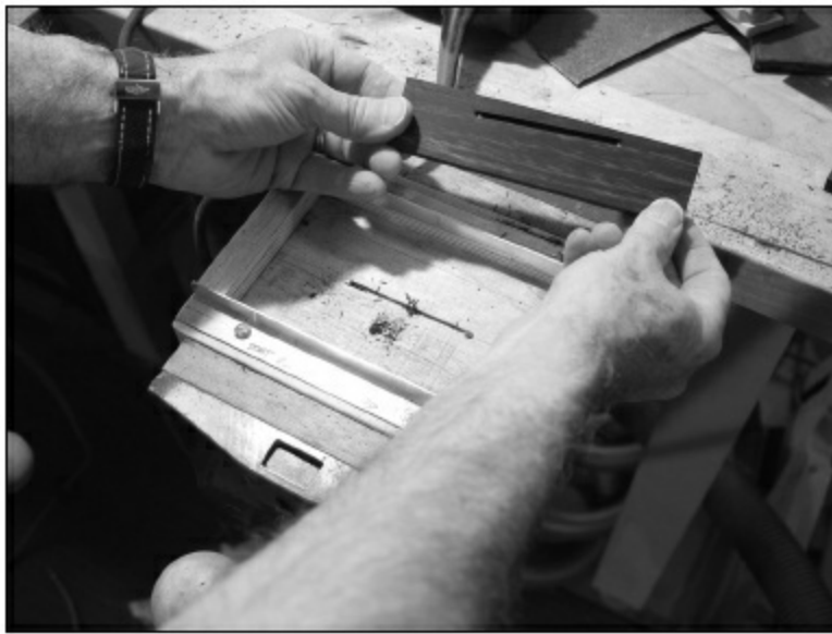
FIGURE 1.5.16. Here is the bridge blank with the slot. Note that the brass pins in the jig must not stick up very high, because the router bit is sticking down into the hole. You must leave some distance between them so you don't ruin either the brass pin or the bit. The depth of cut in this case is \frac{3}{16} ", and the total thickness of the bridge blank is \frac{3}{8} ". A little will be taken off this dimension as we radius the bottom of the bridge and shape the top. The final thickness should be a little over \frac{5}{16} ".
