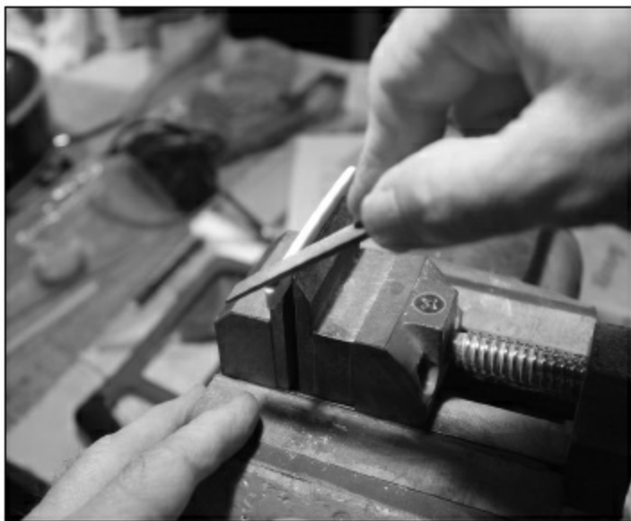
FIGURE 1.7.95. Next, we put the marked saddle into a small vise. Using our fine file, we file the saddle to a rounded point at the proper intonation point for each string. The points are filed as follows: the high E is filed to a point at the front edge of the saddle. The B string is filed to a point at the back edge of the saddle. Then an edge is filed diagonally from the front of the saddle for the G string to the back of the saddle for the low E string. Note: don't make the saddle points too sharp. Keep them slightly rounded. Sharp points will chip off.
