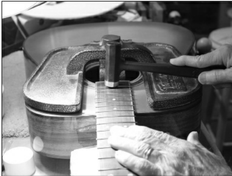
FIGURE 1.7.51. The fret buck holds the upper face brace very solidly so you easily can pound the final frets into the fingerboard without damaging the guitar top.
