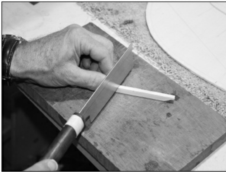
FIGURE 3.1.17. We now connect the marks on each side of the brace and saw a shallow cut into the brace on each of the lines.
