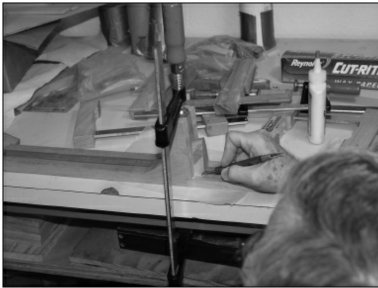
FIGURE 2.2.5. The glue-up for the fingerboard extension is very simple—don't forget to put some wax paper under the glue joint and clean up the squeeze-out.
