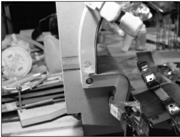
FIGURE 3.1.26. After the ends have been trimmed, they will fit tightly together before gluing the headblock and tailblock. Similar to the steel string, we use a similar jig to sand the proper radius onto the headblock. In addition, the cutaway is designed to come off the headblock at a 90-degree angle, so the headblock is fairly simple to make.
