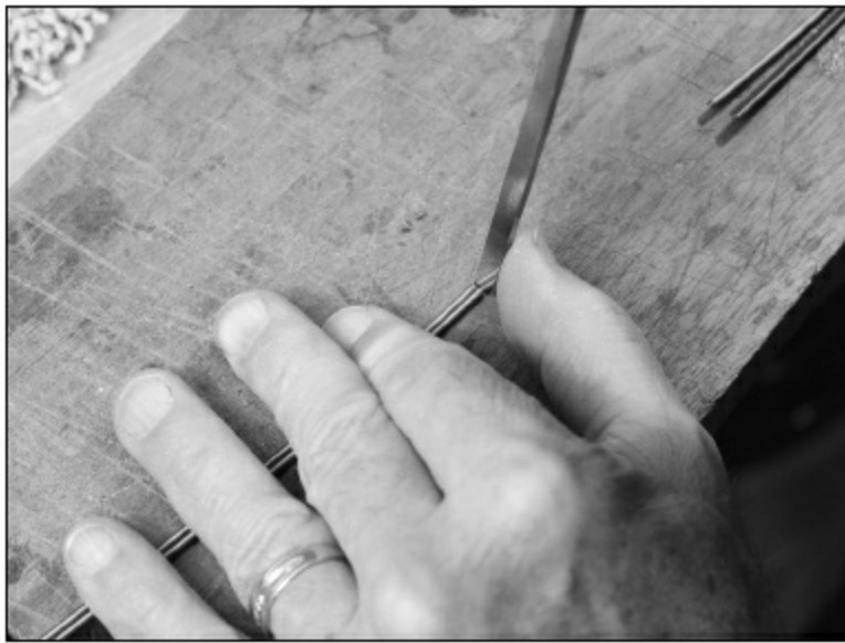
FIGURE 1.3.80. Now we must prepare the purflings that will go on the top of the guitar. First, we have to use a sharp chisel to miter the edges of the purflings so the right and left sides match up perfectly.
