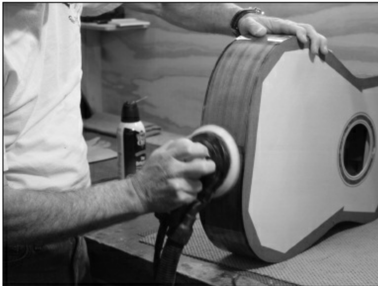
FIGURE 1.6.19. After reapplying epoxy, we sand again. The goal is to fill the grain but leave a very thin layer of epoxy. This will typically take two to three applications of the epoxy to get the results we need. If you jump too quickly to finish before the grain is truly filled, you will have to spray more coats, and since lacquer will sink over time, the grain will likely become visible.
