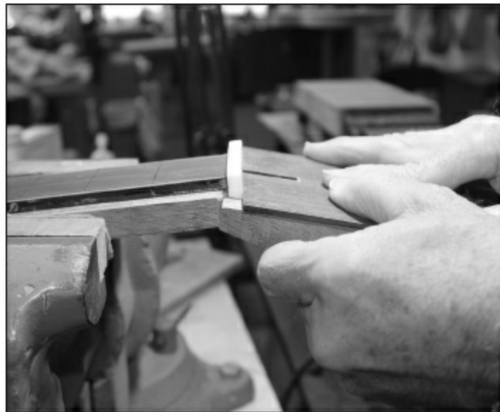
FIGURE 1.4.72. Here's a good shot of how it will all fit together. The front edge of the nut fits flush against the fingerboard, the bottom of the nut is flush against the face of the headstock, and the back of the nut will fit flush against the angled edge of the headstock laminate.
