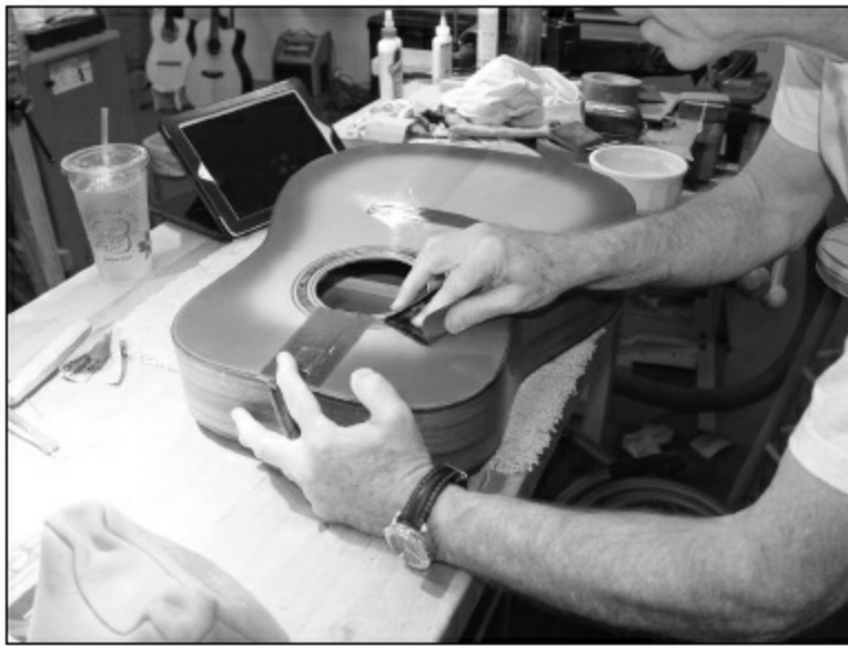
FIGURE 1.6.40. When you find a small bump or blemish, use a hard rubber pad and sand lightly with 2000-grit wet/dry paper (we use it wet in this case), then buff the area out. Note that if you sand too hard, you risk sanding a visible hollow into the surface (or sanding through).
