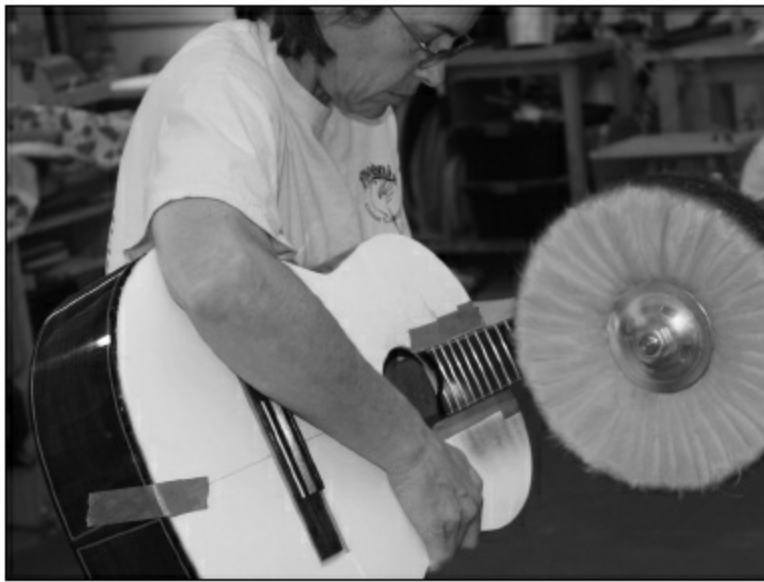
FIGURE 3.4.19. After the neck is dry, the remainder of the fret job is completed. Fret leveling, crowning, and polishing are done the same way as on the steel string. The neck is now buffed. Note that the top of the guitar is protected during these steps.
