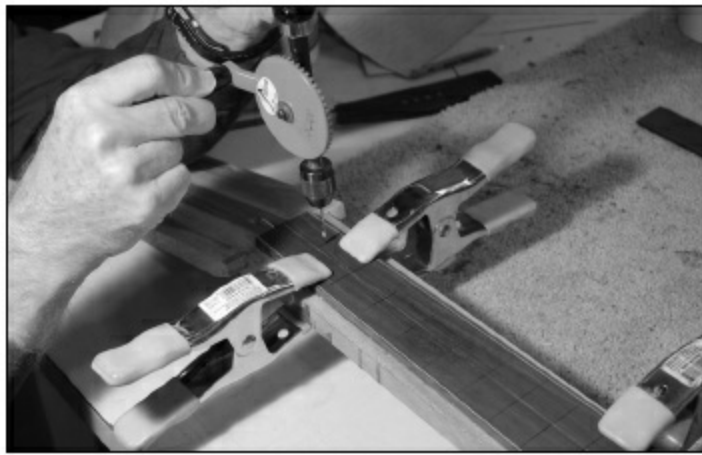
FIGURE 1.4.61. Now, we center the fingerboard onto the neck exactly where we want it and drill holes directly into the holes we drilled into the fingerboard. The tape on the drill bit is marked at the 1/2" line, so the holes will go completely through the fingerboard and 1/4" into the neck wood.
