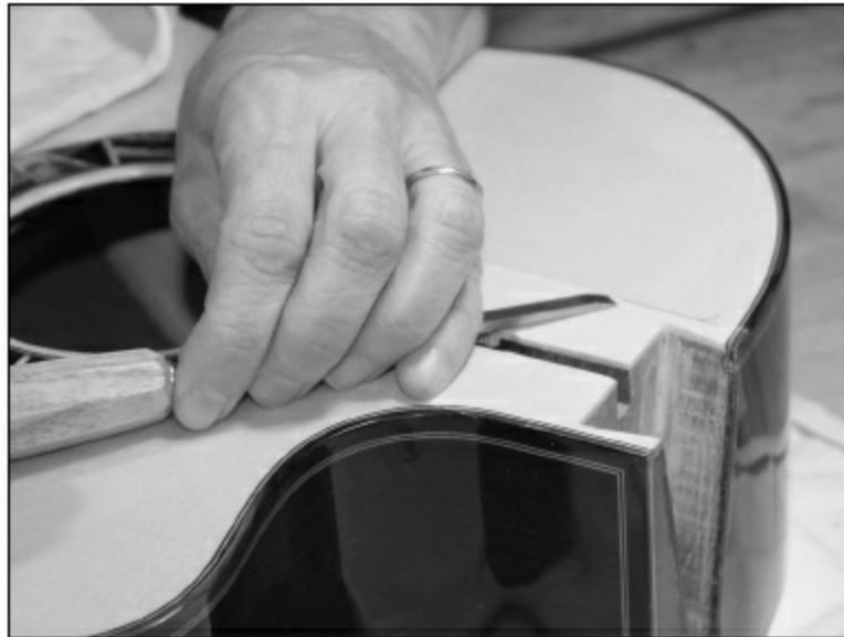
FIGURE 3.4.8. We now repeat the process of scribing and chiseling the finish under the fingerboard.
