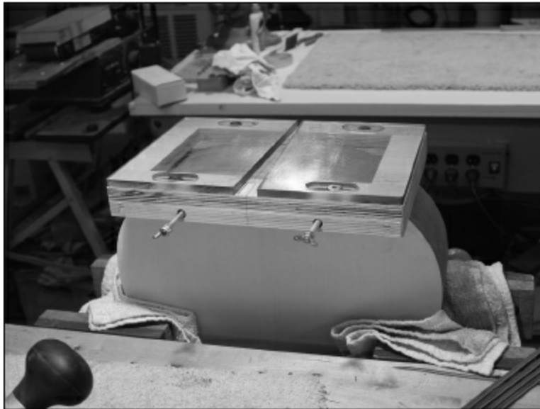
FIGURE 1.3.51. This jig enables us to accurately cut the channel for the end graft into the guitar body. The top of the jig is \frac{3}{8} " plexiglass, and with the wing screws (which are also on the other side), we can tighten the jig onto any of our guitar sizes. Again, thanks to Charles Fox for the idea for this jig.
