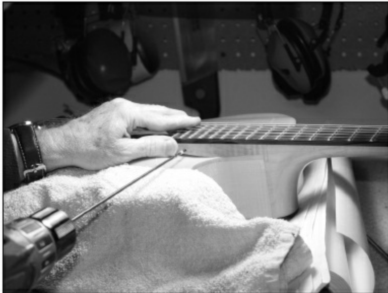
FIGURE 2.3.37. We now use a 1/8" aircraft bit to drill out the screw hole. The aircraft bit enables us to keep the drill far enough from the guitar to avoid scratches. Try to drill as straight as possible and perpendicular to the fingerboard edge. Note the tape on the bit, marking the depth.
