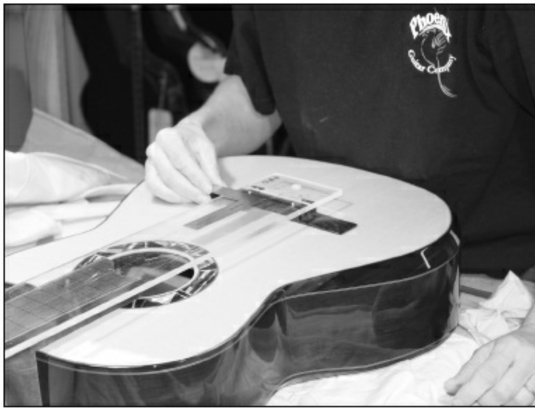
FIGURE 3.4.3. We place the bridge in position under the template with the holes aligned directly over the saddle slot, and check that the bridge is perpendicular to the template centerline with a small square.
