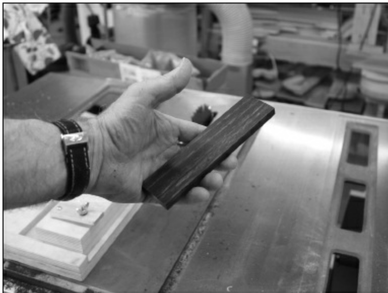
FIGURE 1.5.8. Here it is, a nearly perfect bridge blank. Length, width, and thickness were completed within a few minutes, and all the blanks are the same. This will also be true of the next batch we make, and we don't have to set up equipment every time we do a batch of bridges.
