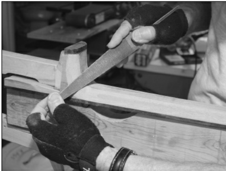
FIGURE 2.2.24. With the heel cap in place, we can complete the carving of the heel and the final fit of the neck to the body.
