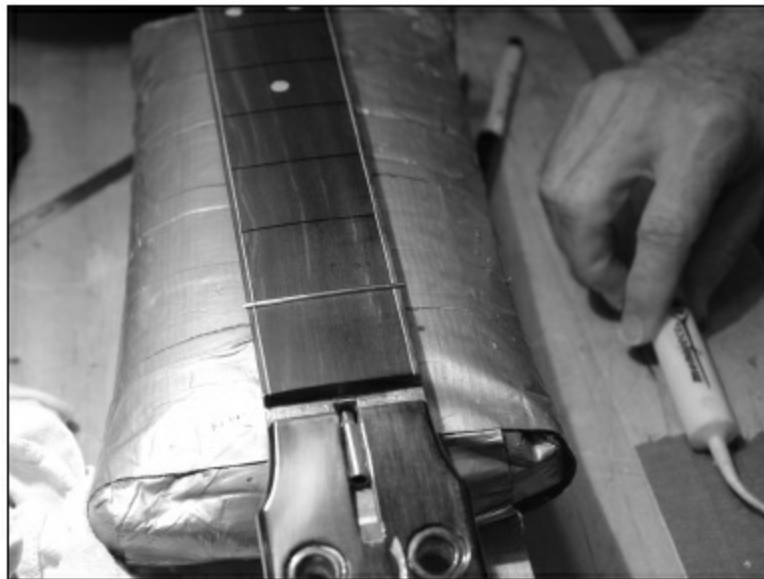
FIGURE 1.7.49. Here is the first fret in the slot. We will repeat this process through the sixteenth fret. Note the glue syringe on the right. We like to put a patch of masking tape on the corner of a bench so the glue does not drip onto the bench.
