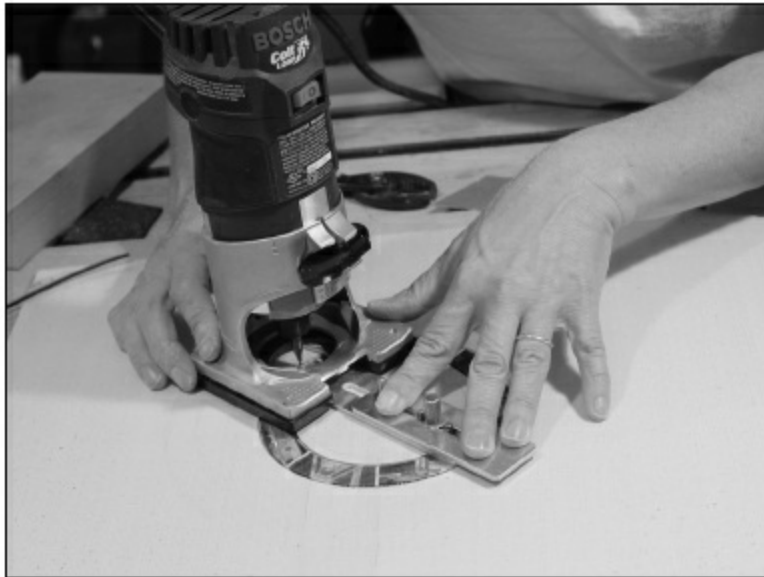
FIGURE 3.1.12. Once we're satisfied with the rosette fit, we cut a \frac{5}{8} " groove into the top (at the proper radius, of course), and glue the rosette in. After it dries, we take a \frac{1}{16} " router bit and cut a groove around the inside and outside radii of the rosette (cutting partially into the rosette and partially into the top).
