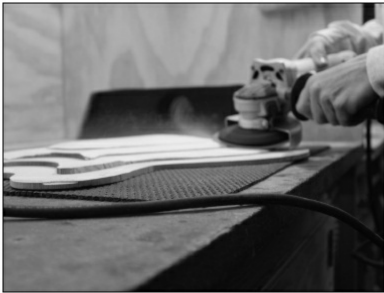
FIGURE 2.1.7. Here is another view of the process. Notice how the dust is swirling into the dust collector vent. It is critical to have good dust collection for a step like this.
