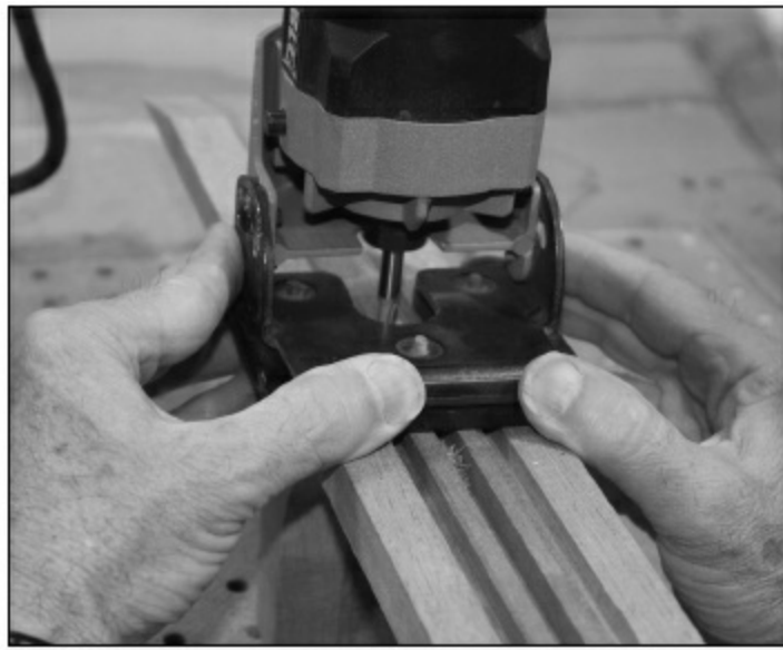
FIGURE 2.2.7. The laminate trimmer is set to the same depth as the truss rod slot and is carefully guided by hand until it is the proper length. Then the rounded end of the slot will be squared off with a chisel, until the truss rod fits properly into the slot.
