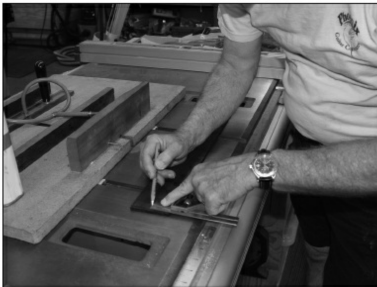
FIGURE 1.4.19. A centerline must now be drawn onto the fingerboard using a right angle from the good, straight-jointed edge. Since this is the side of the board that is perpendicular to the fret slots, the centerline must be parallel to this side. Draw the centerline on one side, then transfer it to the other side so it is visible on both the top and back of the board.
