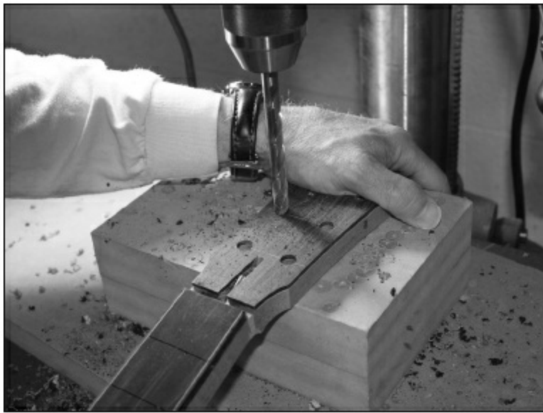
FIGURE 1.4.85. Time to drill the holes for the tuning machines. We will use a brad point bit 25/64 diameter ( 1/64 " larger than 3/8 "). The reason for this size choice will become evident in the next photo.
