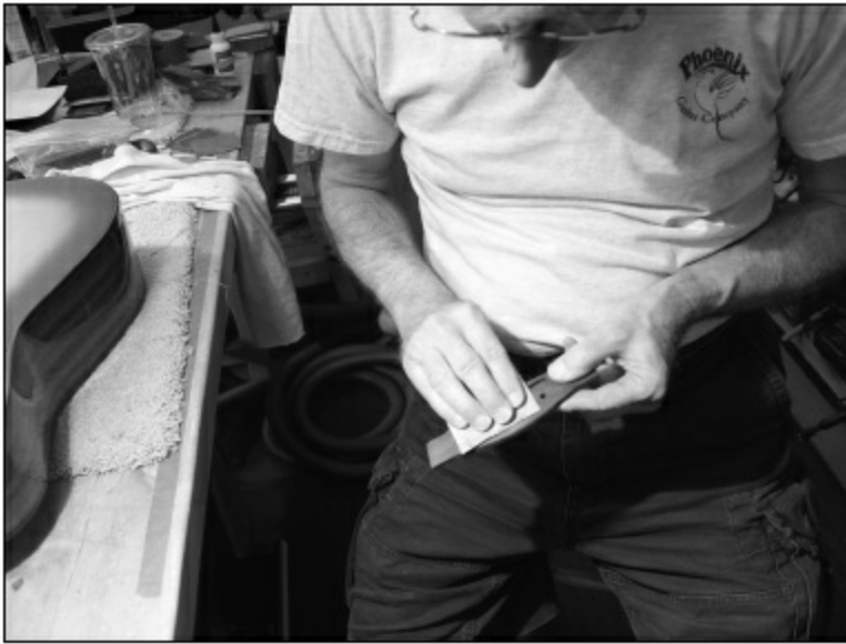
FIGURE 1.7.22. Once the desired shape is achieved, we will go up in sandpaper grits. Starting at 120, we go to 220, 320, 400, and 500 before buffing the bridge.
