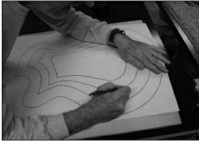
FIGURE 2.1.3. The completed rout plan, being transferred to the guitar top by tracing the drawing using carbon paper. Note that this is going to be a left-handed archtop.
