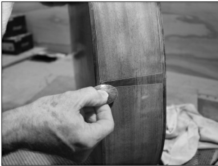
FIGURE 1.6.18. Here is a small oval scraper being used to scrape away the epoxy down to the glue spot. Once we have this and any other glue spots taken care of, we can reapply the epoxy. We will also sand the neck, but due to its curved surfaces, we have to sand by hand instead of using the random orbital sander.
