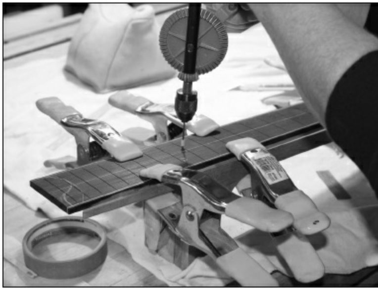
FIGURE 3.2.7. Once we have the alignment close, we're ready to glue down the fingerboard. We drill our pin alignment holes in the first and eleventh frets (as opposed to the first and thirteenth frets) and glue down the fingerboard, just as we did with the steel string.
