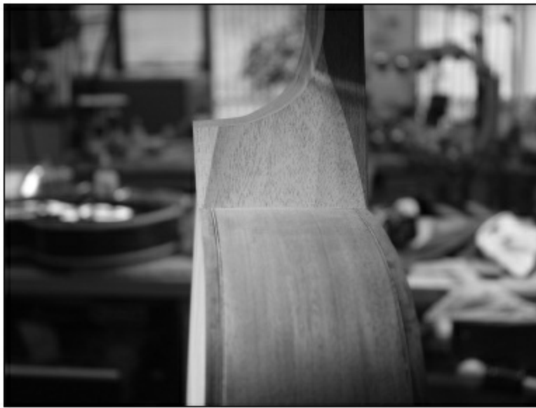
FIGURE 1.4.59. Here is the fit before we glue on the fingerboard. There will be some final fitting to do later, but this is pretty good for now.
