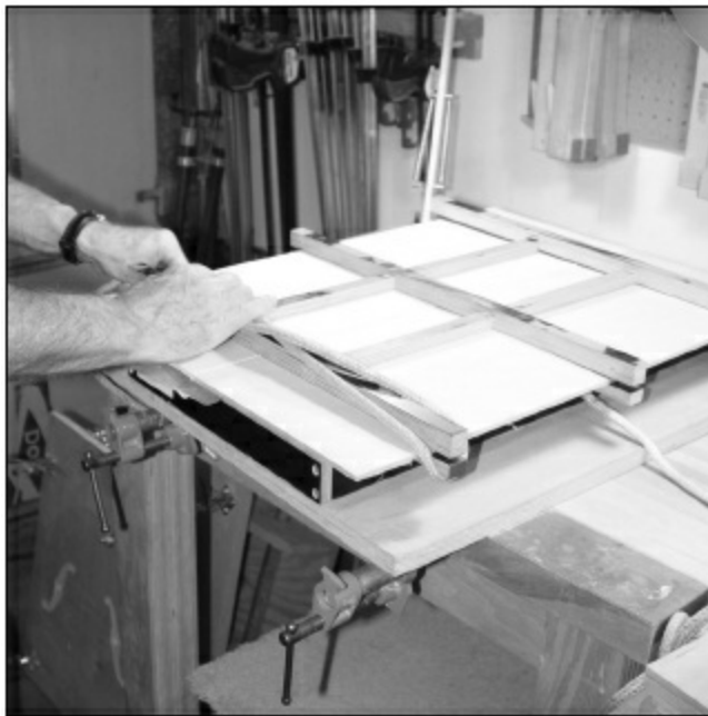
FIGURE 1.1.6. We place a strip of wax paper under the glue joint and then put the frame over the halves of the top, tying the ropes around the ends of the frame ends.
