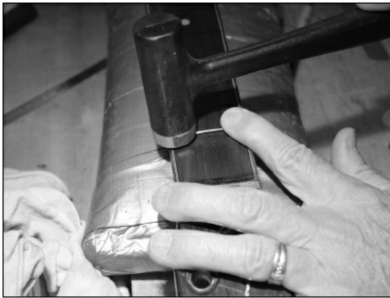
FIGURE 1.7.48. Before pounding in the fret, you must be sure the fret is properly seated in the slot. The tang must be vertical, and the fret must be aligned properly side-to-side in the slot. At this point, firmly tap the fret into the slot. Be sure you don't tip the hammer, or you'll likely hit the fingerboard and make crescent-shaped dents that will need to be sanded.
