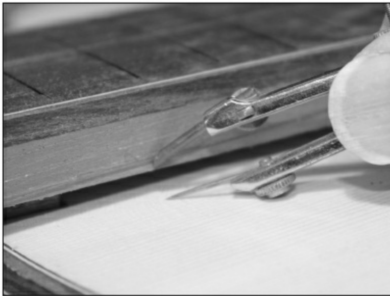
FIGURE 3.2.2. This shows the same method we used on the archtop to measure the fit between the guitar top and the fingerboard extension. Once the pencil line is made, the extension is trimmed down to the line with a chisel, a plane, or both. (Also check Figure 2.2.12 on the archtop neck fit to check the technique.)
