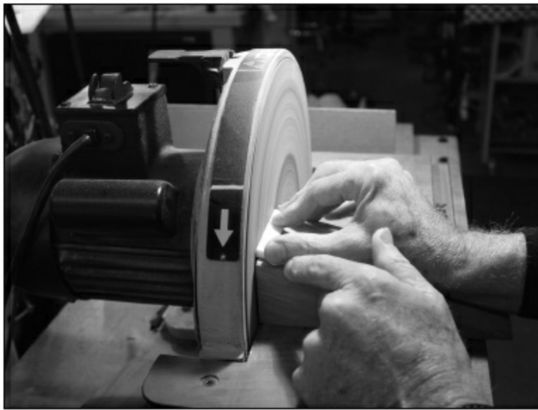
FIGURE 1.4.67. We now must prepare a rough nut for the guitar, so we take a piece of bone material \frac{1}{4} " thick, \frac{13}{32} " tall, and 2 \frac{1}{4} " wide. We are putting one edge of the nut on a jig that has the same angle as the headstock angle (15 degrees), and we will sand that angle onto the bottom of the nut.
