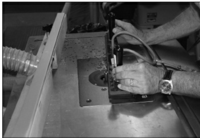
FIGURE 1.4.25. The fingerboard blank is now placed onto the vacuum template, shown above, with the fret slots down. The centerline on the fingerboard is aligned with the centerline drawn onto the vacuum template. We use a spiral, flush-cut bit used for this step. In addition, you absolutely must know the direction of your grain, as the router bit is cutting it. In the case of ebony, it is often difficult to tell what direction the grain is running, so we recommend what we call nibble cuts to do this step. We will start the cutting toward the far right side of the board and make a cut of about 1/4" (going against the direction of the spin of the bit). We will then repeat this procedure every 1/8" to 1/4" as we slowly cut toward the left side of the board. We have had cases where the grain has run out, and the bit has been able to dig directly into end grain and caused a tear-out instead of a clean cut. However, by using this nibble-cut method, we haven't had a problem. If you don't have vacuum capability in your shop, you can use double-sided tape to hold your fingerboard to the jig. Just be sure to put good handles on the jig. Keep your fingers away from the blade!
