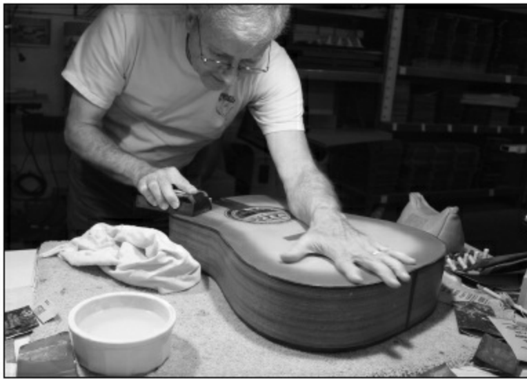
FIGURE 1.6.36. After the first sanding, four or five additional coats are sprayed. Then, we wet-sand the surface by hand using 600- to 800-grit sandpaper, followed by 1200-grit paper. This sand-out is easier than the first, since the final coats went onto a very smooth surface. Using the spraying and sanding schedule we've presented results in the final finish thickness being between .005" and .007".
