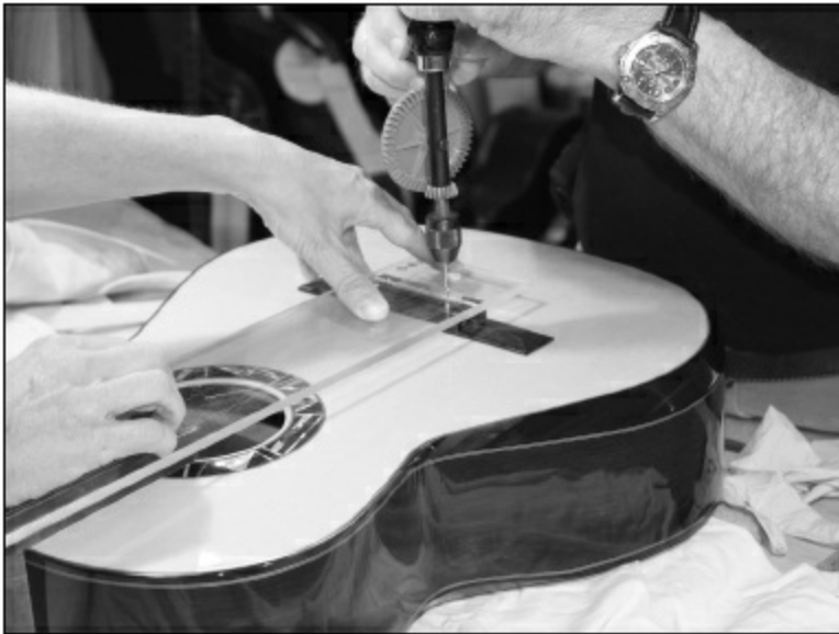
FIGURE 3.4.4. When the position of the bridge is right (meaning it's square to the centerline, and the holes line up correctly in the saddle slot), we drill holes directly through the template holes, through the saddle slot and through the guitar top.
