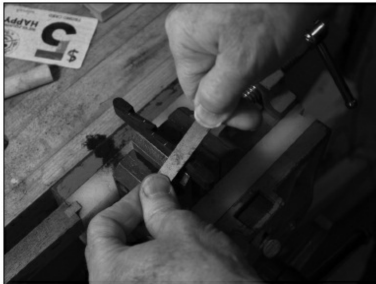
FIGURE 2.3.15. The top of the bridge is being filed to shape. Note the white marks on the top of the bridge, marking where the strings will go. The spacing of the outside strings on this archtop is 2 \frac{3}{16} ". The marks were made with the same Stew-Mac tool used to mark the string spacing on the nut on the steel string guitar.
