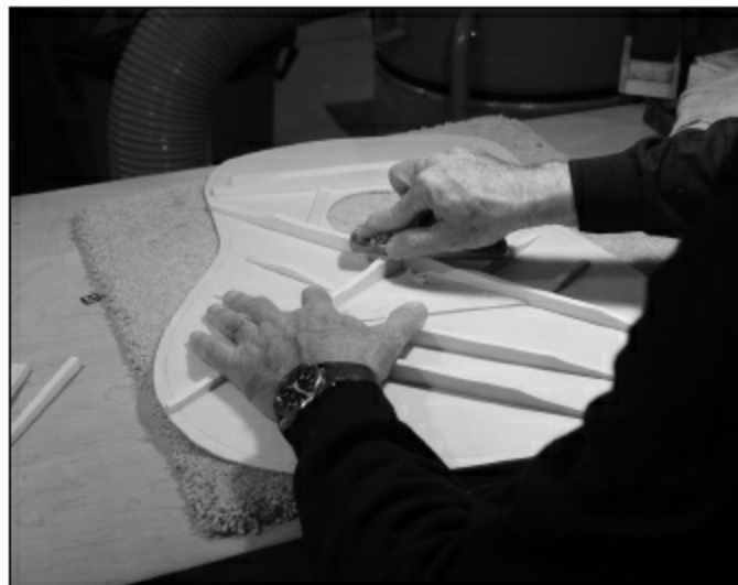
FIGURE 1.1.53. Finally, it is time to carve the braces. We have made the job much easier by pre-shaping much of the brace material before gluing the braces down. First, we carve the intersection of the X brace using a small flat-soled plane. As mentioned before, this brace will be \frac{5}{8} " tall at this point.
