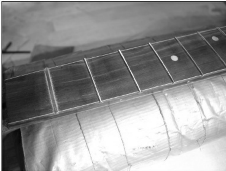
FIGURE 1.7.63. Here you can see the first fret, all crowned. The second fret is ready to be crowned.
