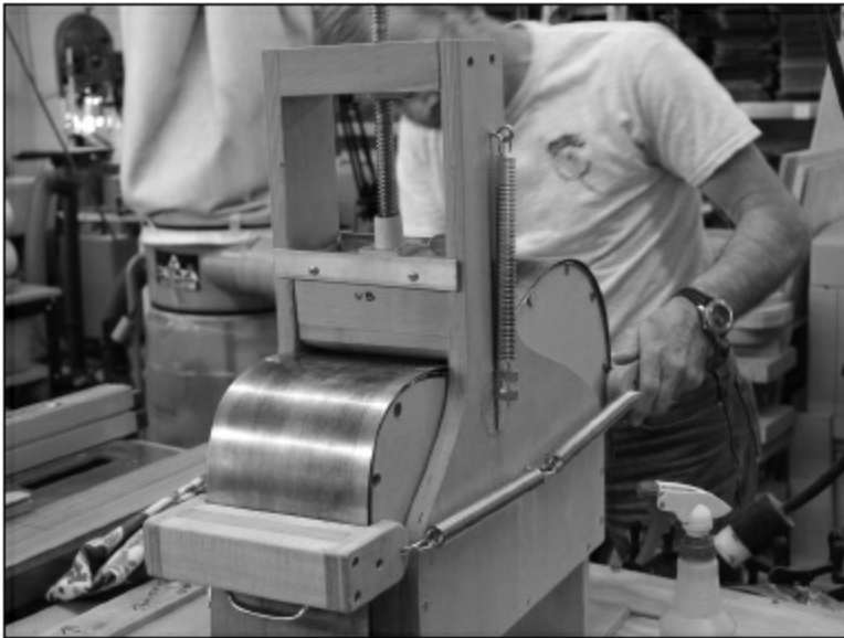
FIGURE 1.3.10. Once the heat blanket has gotten hot, the waist clamp is slowly screwed down all the way, and the upper and lower bout clamps are brought around to clamp the sides around the bouts. We will leave the side clamped in the bender until it cools. We will then reheat the side and wait until the sides are just cool enough to touch. We like to clamp the sides into the molds when they are still very warm and moist. After the sides are in the molds, they are left to dry, preferably a couple of days (if time permits).
