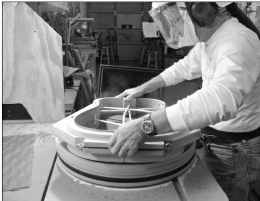
FIGURE 1.3.20. Here is the jig in use. It requires very little downward pressure to quickly sand away material, so much care must be used. Also, check each side often to be sure one side isn't getting shorter than the other. Also, we stop the jig when the sides are about 1/8" away from the mold. We don't want to damage the mold.
