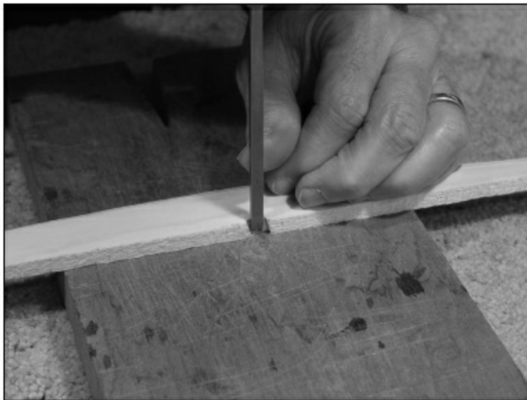
FIGURE 2.1.47. Once the edges of the notch are cut, use a thin chisel to get rid of the center of the notch. Be sure you don't use the chisel below the level of the saw line—you'll split your brace.
