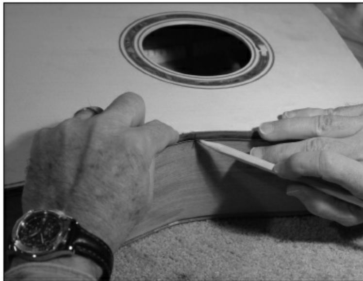
FIGURE 1.3.73. Each piece of binding is held up to the guitar, and we mark the guitar side and the binding so we can find the proper alignment. We make the mark at the waist.
