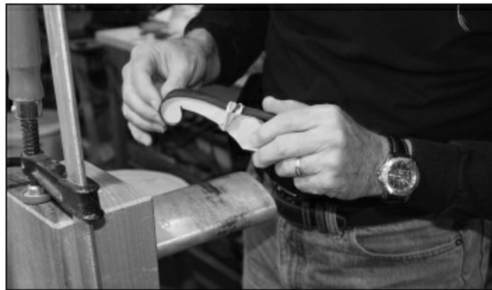
FIGURE 2.1.37. Once the veneer has been made pliable enough to bend around the caul, the free end is held down with a rubber band. After a few hours, it will be dried and will hold its shape well enough to be put into the F-hole so the contour of the hole can be drawn onto the veneer, and its final shape can be sanded down. This step helps keep the Indian rosewood from splitting.
