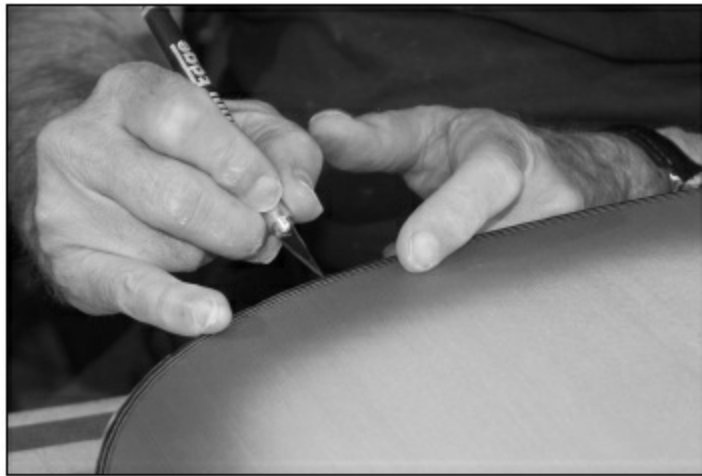
FIGURE 1.6.32. The color is being scraped off the purfling with an X-ACTO knife.
