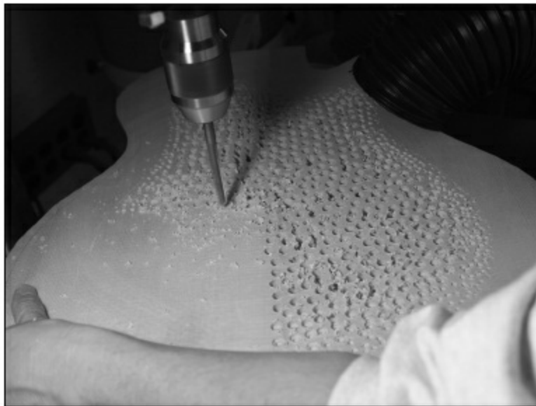
FIGURE 2.1.12. Next, a few hundred holes are drilled into the top, from the back side. Since the drill press has a depth stop, all the holes stop 1/4" from the top surface.
