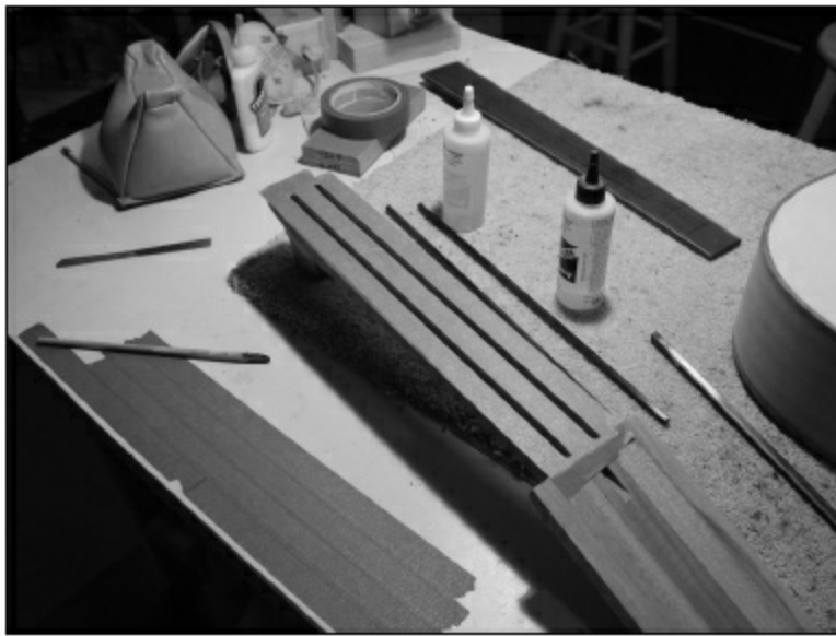
FIGURE 1.4.53. Now we will glue the carbon fiber rods into the neck. We will use epoxy for this step. First, we cover the neck surface that will be glued to the fingerboard with masking tape, and using an X-ACTO knife, we cut out the slots for the rods. Since this is a very sloppy job, we use the tape to keep the neck surface clean.
