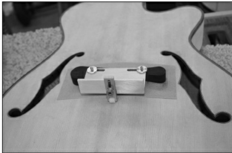
FIGURE 2.3.7. After the bridge posts are in, we use a piece of self-stick 120-grit sandpaper taped to the guitar top and a Stew-Mac archtop bridge fitting jig to sand the underside of the bridge to fit exactly to the top.
