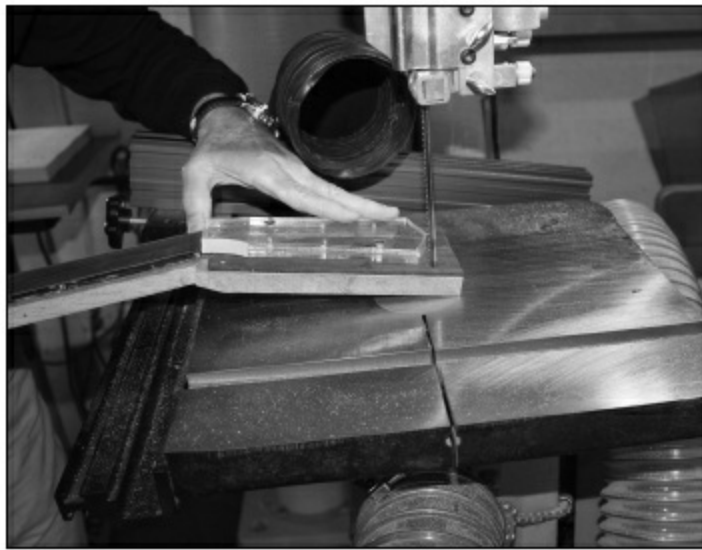
FIGURE 1.4.79. Next, we will cut around the template as closely as possible. It's always important to leave a comfortable margin so we don't cut up our template. Note that we have put some green masking tape on the hyoid portion of the headstock template. Since the template and the fingerboard are the same size, we want the headstock to be cut slightly larger so we can file it to size.
