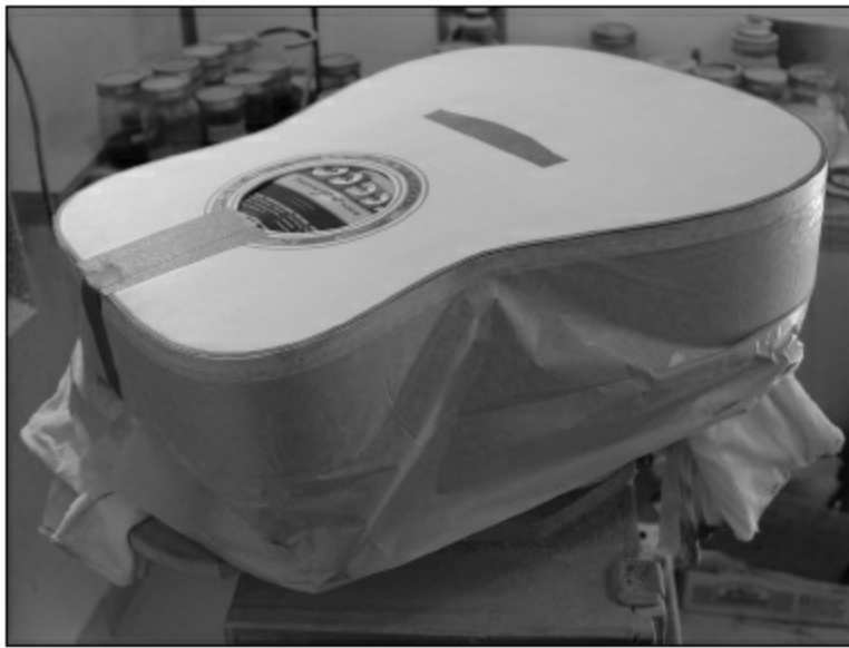
FIGURE 1.6.27. Now we tape off the sides of the guitar. This guitar will have a two-tone sunburst on the top, and we are going to do colors next.
