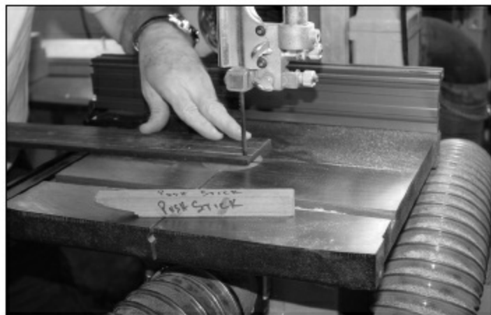
FIGURE 1.4.23. After the proper measurement has been reached, (in this case, through sizing of the bindings), the template is placed on the fingerboard and is drawn. Then we band saw the fingerboard shape, which is oversize by about \frac{1}{16} ".
