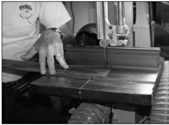
FIGURE 1.4.20. We now have to prepare the fingerboard bindings to complete the fingerboard. We are using Indian rosewood for the bindings for the steel string and Macassar ebony for the archtop and the classical, all with a thin veneer (approximately 0.020) of maple separating the bindings from the fingerboard. Since the next several steps are identical, we will only show them once. The photo shows us cutting binding strips from a board on the band saw.
