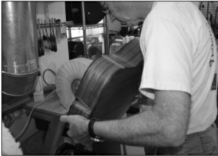
FIGURE 1.6.37. Once the sand-out is complete, we start the buffing process on the coarse buffing wheel. We use the coarse wheel both with and against the grain to get out as many scratches as possible.
