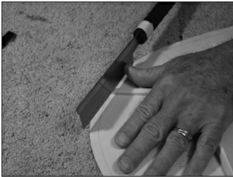
FIGURE 1.3.28. After marking the braces, the sides are moved, and we mark each brace 3/16 " outside the original mark. This is the thickness of the kerf. Then, as is shown in the photo, we will cut the brace down to the top wood. Take special care here; you don't want to damage the top.
