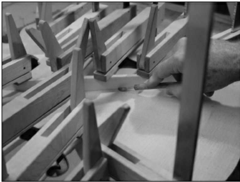
FIGURE 2.1.55. We use a small tool for clay sculpting for cleaning up glue. We buy them at an art supply shop. To get the squeeze-out on the other side of the braces, we must carefully go between the clamps to get the excess glue.
