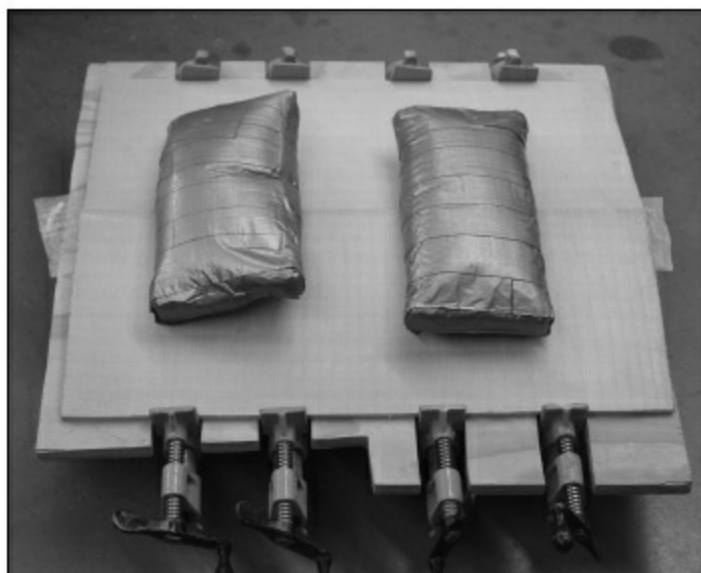
FIGURE 2.1.2. Here, two wedges of Sitka spruce being glued together in a simple jig comprised of a flat board and four pipe clamps. We have cleaned away the glue squeeze-out along the top of the glue joint and placed a couple of twenty-five-pound bags of lead shot on top to keep the boards
