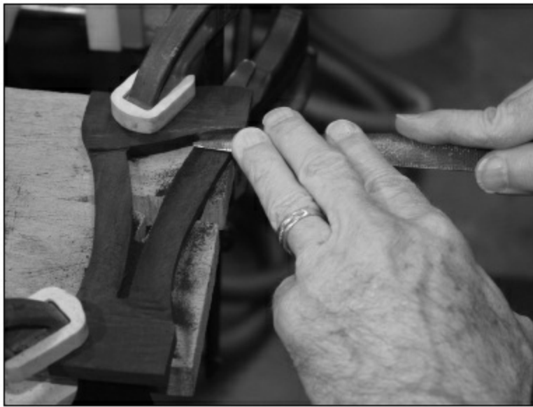
FIGURE 2.3.22. We use a file to give the top of the tailpiece some definition and styling.
