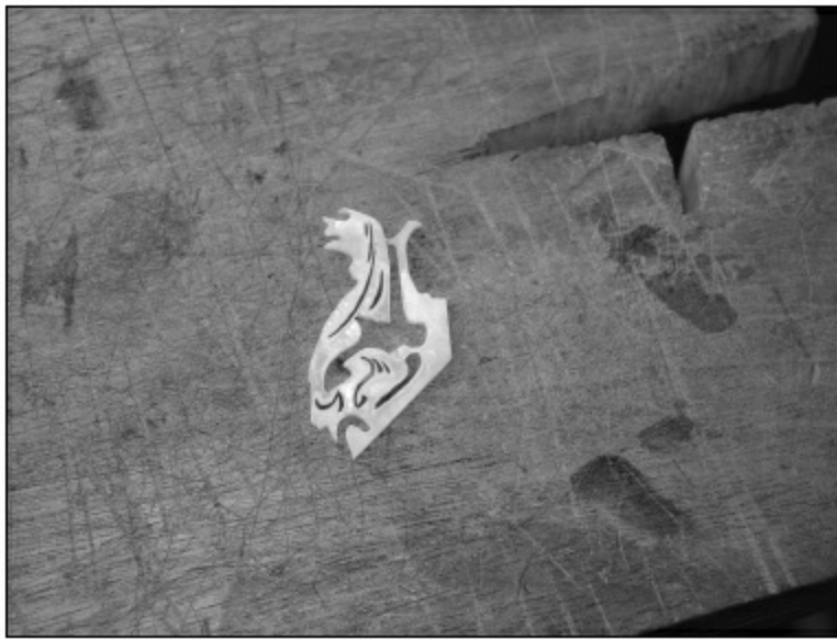
FIGURE 1.4.91. Here are all the paper pieces making up the body of the bird after they are glued to the scrap piece of MOP. We were lucky to be able to fit the bird's entire body onto the one MOP piece.
