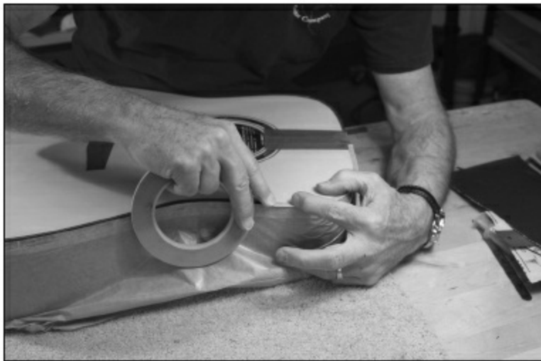
FIGURE 1.6.28. After spraying the first color (the amber shellac), we will tape off the purflings around the guitar edges with 1/4" masking tape. The next color will be a cherry red sunburst, and we want the purflings to remain their natural color. The red color is mixed in with blond shellac. We always spray our colors mixed in with shellac. It sprays well and looks good under our waterbase lacquer.
