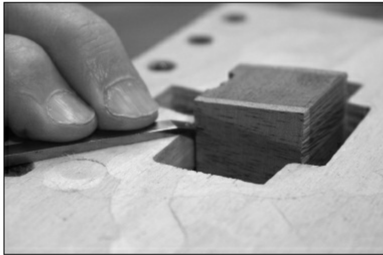
FIGURE 1.4.113. We are going to cut the heel off exactly at the level of the top of the plane of the jig. In this photo, we are checking with a chisel that the jig level lines up with the pencil mark we made above in Figure 1.4.111.
