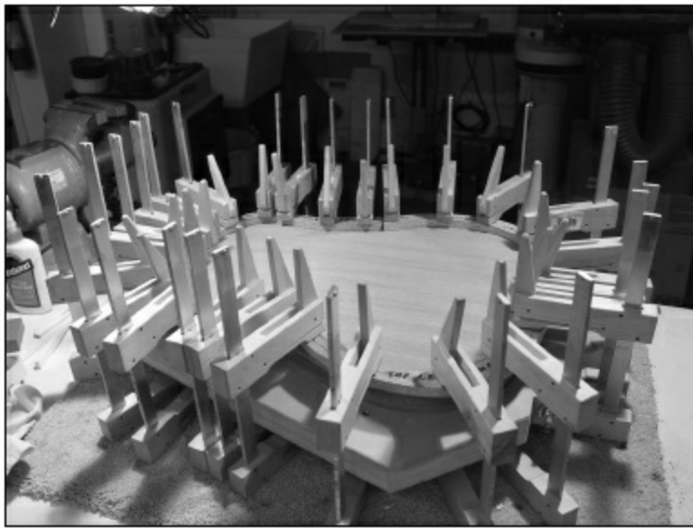
FIGURE 1.3.40. Now clamps are put around the guitar, using the cauls for even pressure distribution.
