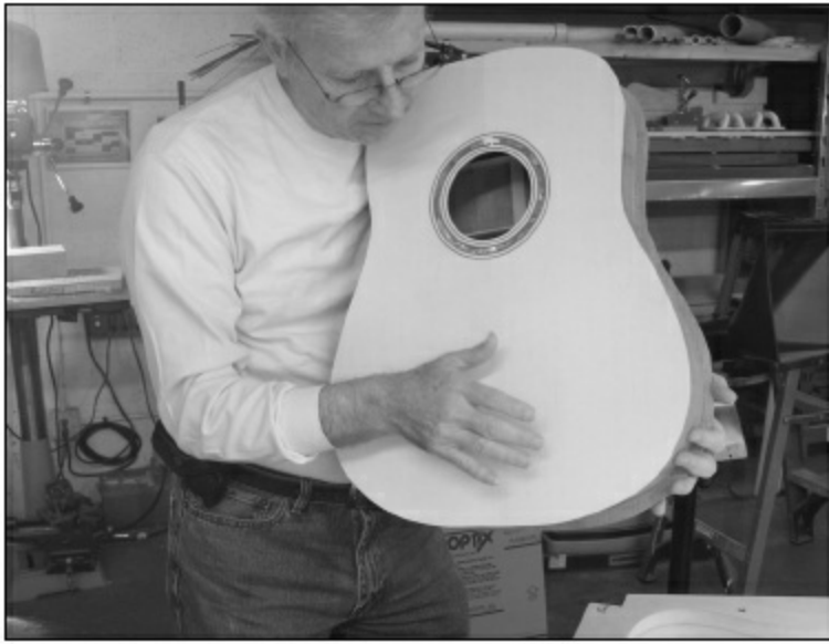
FIGURE 1.3.44. Once the guitar body is removed from the mold, we always tap the body to hear its response. A large body guitar like this should have a deep, clear ring. If the tap tone is muffled, like it's stuffed with a pillow, you have a serious problem. You will probably have to saw off the top and make another one, because the instrument will not have a good sound.
