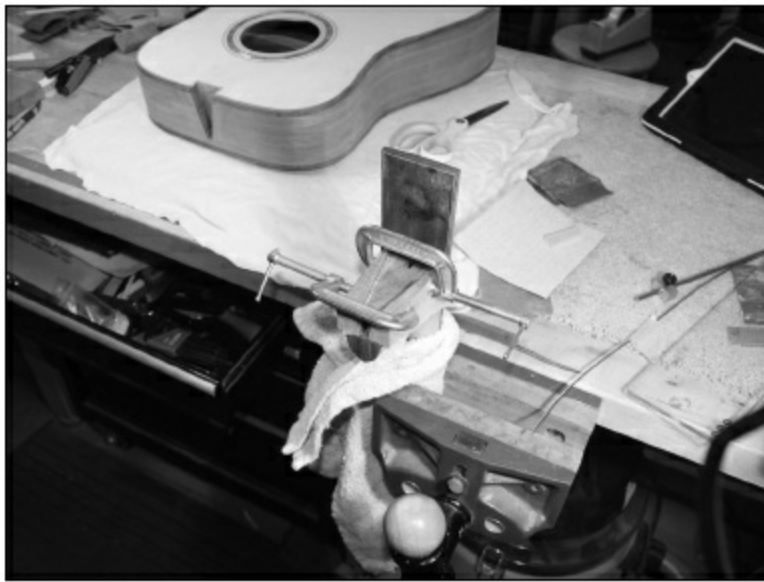
FIGURE 1.4.129. After making an initial check of the vertical alignment, we see that it looks very good, but once the side-to-side alignment is changed, the dovetail fit is slightly loose. We are going to shim the dovetail and refit it to be sure that it is tight and that the neck is perfectly aligned. When we're done, there will be almost nothing left of the shims. We'll almost completely carve them away as we make the final fit. In this photo, we're gluing on the new shims (small pieces of veneer).
