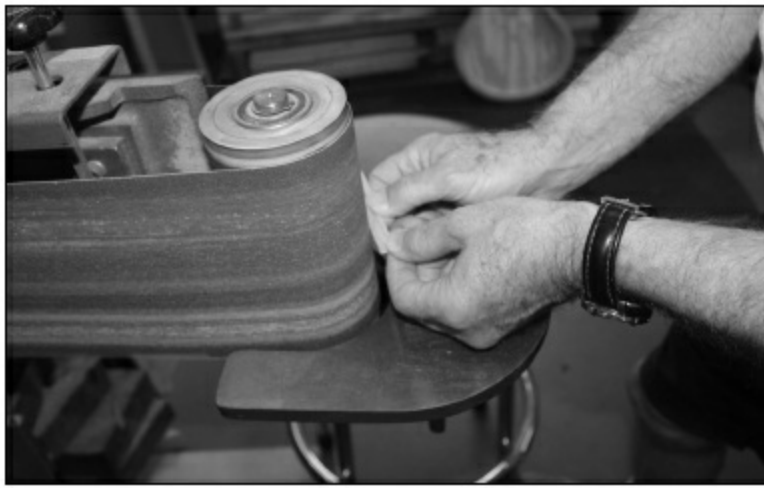
FIGURE 2.1.34. As mentioned above, don't try to cut the maple with scissors. Use a belt sander to sand away the excess and get down to the lines. Be sure not to sand your fingers during this step.
