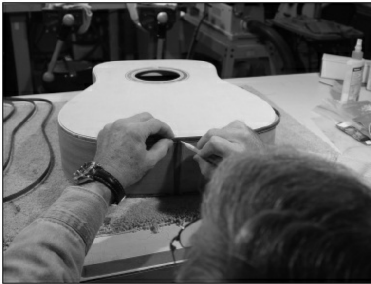
FIGURE 1.3.74. With the binding line aligned with the line on the side of the guitar, we bring the binding around to the end graft and mark the center. We will repeat this operation with the bindings on the other side and the back.
