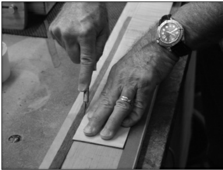
FIG, 2.1.61. After we get the thickness of the maple side, we glue a thin veneer (in this case, a .020 thick veneer of walnut) to the thinned down portion of the maple side. In this photo, we are trimming the veneer after it has been glued. With the veneer, the total thickness of the side will be very nearly equal to that of the rest of the side.
