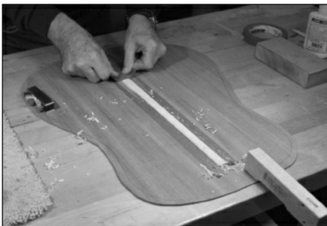
FIGURE 1.2.12. We use 120-grit sandpaper to smooth out the strip and shape it from a rectangle to an arc.
