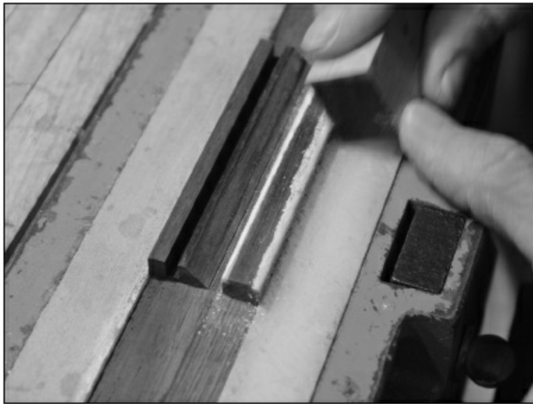
FIGURE 3.3.16. After sanding and filing the ends of the blocks, we sand the edges of the bone pieces to soften them so they will not break strings, since strings will certainly pull very hard across the top of the back block.
