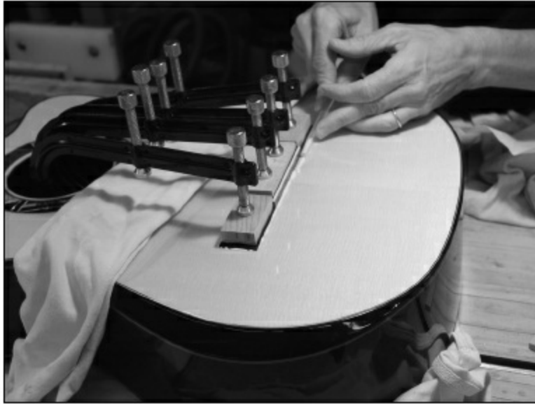
FIGURE 3.4.12. A plastic straw is being used to scrape up most of the glue squeeze-out.
