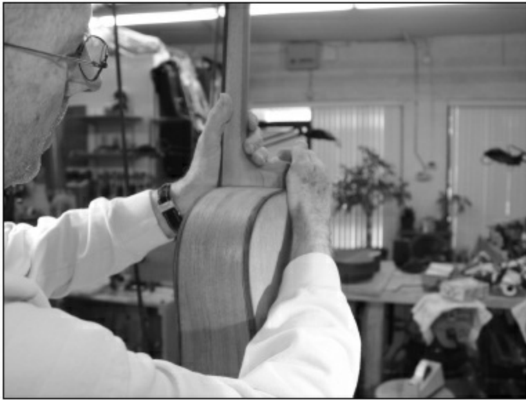
FIGURE 1.4.131. We put the neck into the dovetail to check the fit.
