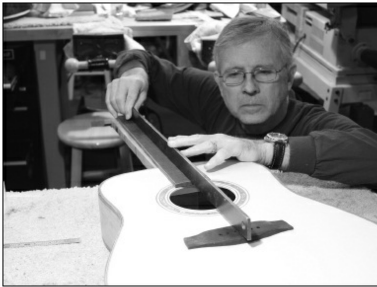
FIGURE 1.4.57. Once side-to-side alignment is checked, we need to check vertical neck alignment. For this, we place the fingerboard onto the neck (it's not glued yet) and place a sample bridge in its proper position on the soundboard. By placing a straightedge along the fingerboard, we can see how it lines up with the top of the fingerboard. We want it to just kiss the top of the bridge—up to about 1/32'' higher. If it is lower or higher than this, we need to adjust the neck angle. It is easiest to do this now, before we glue the fingerboard on.
