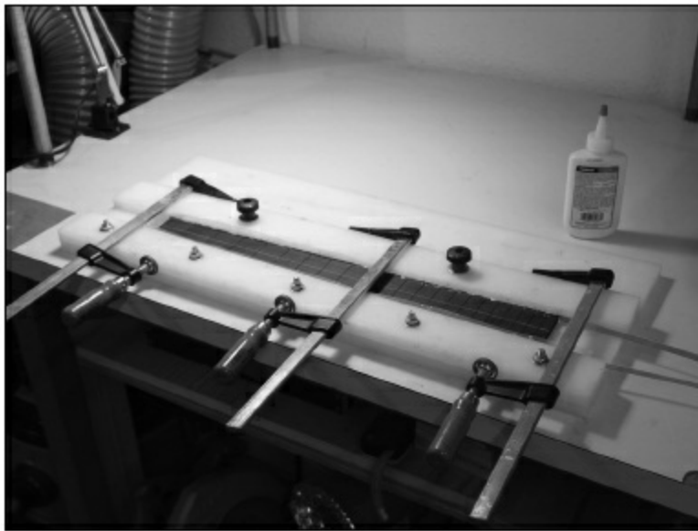
FIGURE 1.4.27. As shown in the photo, we have built a jig out of UHDPE (ultra-high-density polyethylene) to glue our purfling and bindings to the fingerboard. We use a small screwdriver blade to push the maple purfling down so it doesn't creep up. In addition, we will cut a couple of 1" wide pieces of wax paper to go around the glue-up to keep glue out of the jig.
