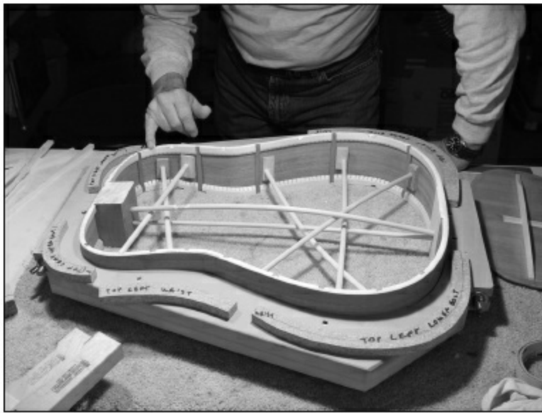
FIGURE 1.3.38. Now it's time to glue on the back. We glue the back first, since much of the back-to-kerf joint is visible through the sound hole. After clamping, we can clean this joint before gluing the top. In this photo, glue is being applied to the kerf.
