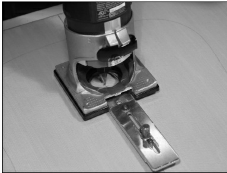
FIGURE 1.1.19. A 3/16" pin is put through the center hole, and extended down into the backing board shown in figure 1.1.18. A 1/16" bit is in the router and is set to cut to about 2/3 the height of the purfling. Now we set the bit at the point marked as the inner purfling ring and cut.
