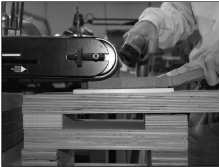
FIGURE 3.2.11. As with the steel string, we sand down the back of the headstock to final thickness. Note that the spacer under the headstock is thinner than the one for the steel string (Figure 1.4.106). This gives us a headstock thickness of about \frac{1}{32} " over \frac{3}{4} " ( \frac{29}{32} " )
