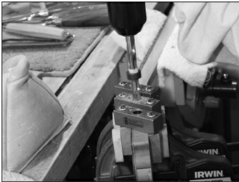
FIGURE 3.2.12. Now we drill the holes for the tuning machines. The jig shown is a tuning machine drill jig for slotted pegheads from Stew-Mac. Note that we have a depth stop on the bit, so we don't go too deep.
