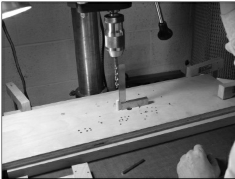
FIGURE 2.1.10. In preparation for carving the underside of the top, we set up the drill press. Note there is a 5/16" peg sticking up vertically in the base board. The right angle helps get the 5/16" drill bit perfectly aligned (as close as possible) over the peg.
