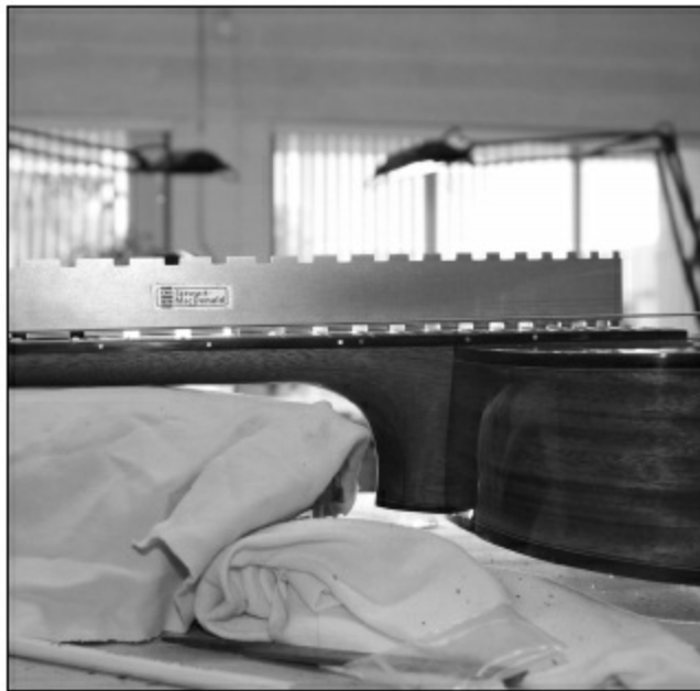
FIGURE 1.7.90. Once all the strings are on and tuned to pitch, we do a quick check of the “relief” in the neck. The relief is the amount of curvature in the neck. Note the light shining under the straightedge. In this case, it is approximately .012” high (not too bad). Relief is a desirable thing. When a string is plucked, it vibrates with a certain envelope. If the neck is dead straight, the vibrating envelope will cause the string to bottom out or buzz at some point along the fingerboard. Having the proper amount of relief helps lower the action to the best point, while allowing room for the string to vibrate without buzzing. The louder a player plays, the more relief, and higher action is needed. The softer he plays, the more action can come down; relief can be minimized but should not be eliminated.
