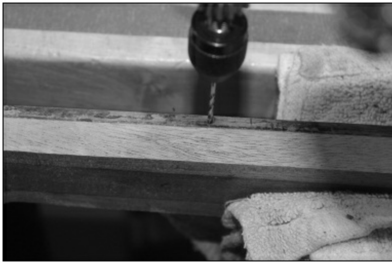
FIGURE 1.4.108. Now it is time to put in the side dots. We will use MOP side dots (2 mm). So we mark the position of the fret slots, mark the location for the dots (halfway between the frets), and drill a hole for each dot.
