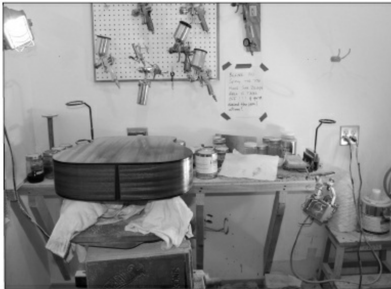
FIGURE 1.6.11. Once the epoxy is applied and smoothed out, we put the body into our spray booth, where we can turn on some lamps and heat the air by a few degrees to help the epoxy dry faster. The hardener we are using is a fast-cure hardener, but it still takes several hours before it can be sanded. Therefore, if we apply the first coat early in the day, we can get a second coat done before the end of the day. In most cases, at least two coats are needed. This mahogany has a lot of deep grains, so it will probably take three coats.
