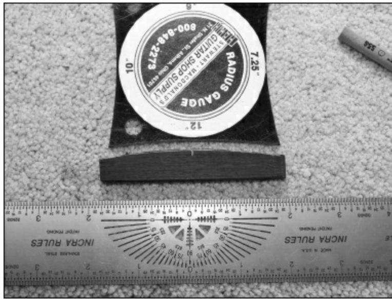
FIGURE 2.3.10. Now we start working on the top of the bridge. First, prepare a piece of ebony about \frac{1}{2} " tall, \frac{5}{16} " thick, and 3\frac{1}{2} " wide. On the top, as shown in the photo, draw an arc of the same radius as the fingerboard (in this case, 12") and sand the top to the drawn line.
