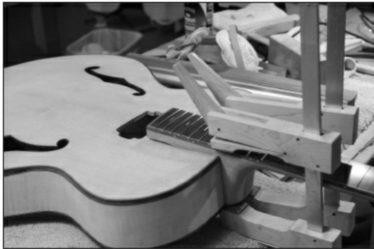
FIGURE 2.2.27. Once the fret job is at this point, we will do the final neck fit, then glue on the neck of the archtop. We will also file the fret ends now. Fret leveling, crowning, and polishing will happen after the finish is applied.
