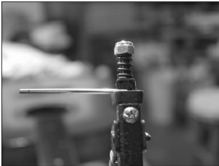
FIGURE 1.7.43. Using the Sharpie marks to align the fret with the fret tang nipper (another very handy tool from Stew-Mac), we cut the fret tangs.
