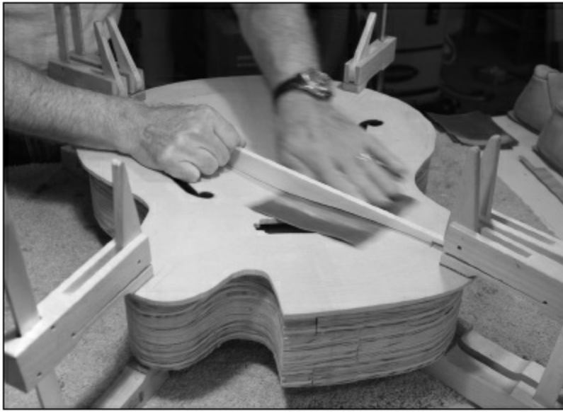
FIGURE 2.1.44. Here is another view of the brace being sanded. Note the notch on the far right (upper bout) side of the brace. This is put there to allow the sandpaper to get under the brace all the way to its end but still have an extension that can be held in place by the clamps. This extension will be sawed off after the brace is glued in place. Sand both braces to match the top profile.
