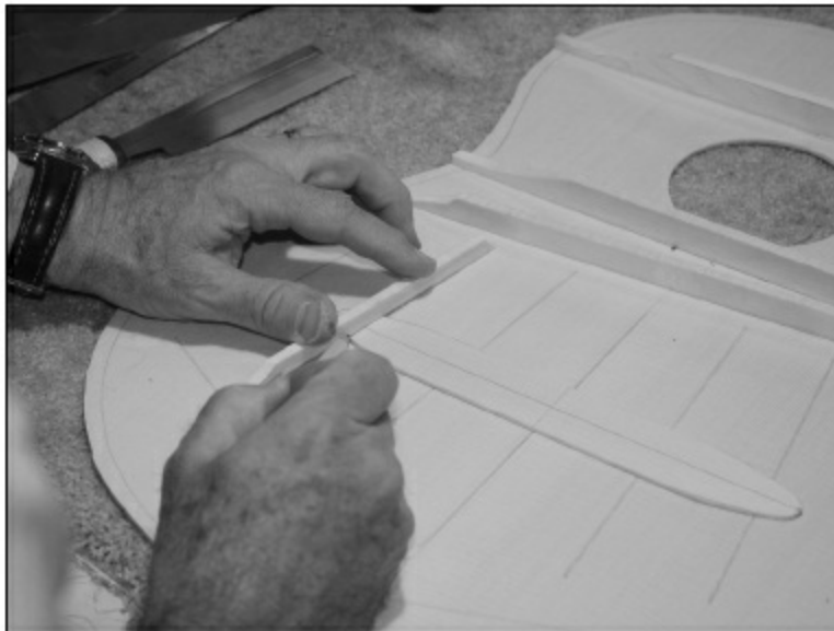
FIGURE 3.1.16. As you can see, we have given a shape to the ends of the braces using a belt sander. It's easier to do on the belt sander before gluing than with a chisel or plane after it's glued down. We then hold the brace on its respective line and mark where it crosses the bridge plate. Both sides must be marked.
