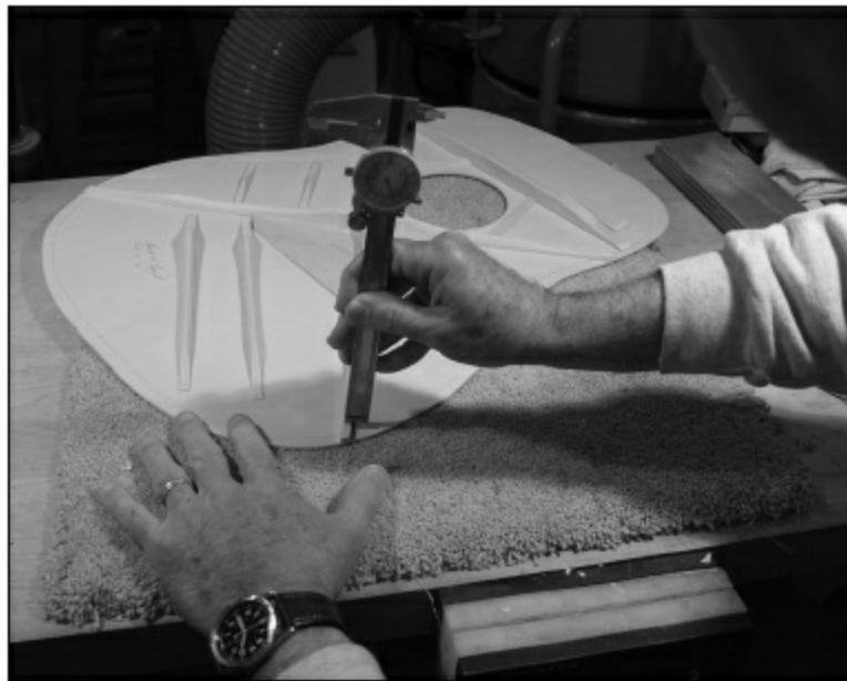
FIGURE 1.1.59. One very important point is to make sure the outer wings of the X braces, as well as those of the upper face brace, are planed down to no higher than 1/8". This will be important as we get the top fitted to the sides and kerf.
