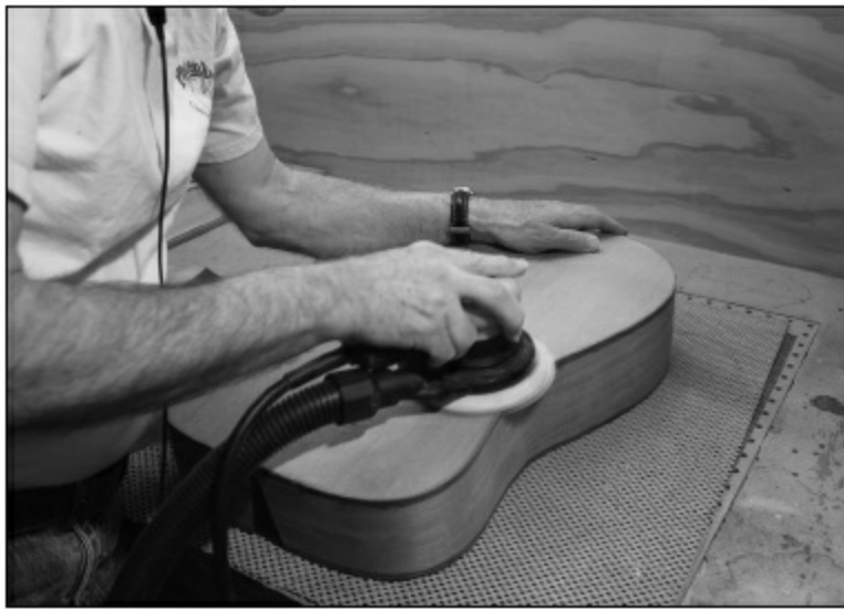
FIGURE 1.6.1. We start by using a random orbital sander to go over all surfaces, using 220-grit sandpaper. If your guitar has a cutaway, you won't be able to use the sander in the cutaway, so you will have to do that section by hand. Also, practice using the random orbital sander on scrap before you try it on your acoustic. It is easy to tilt the sander and create a divot in a critical surface that you cannot hide, so be sure you understand how to use the sander. You will be able to save time and create a smooth surface ready for finish.
