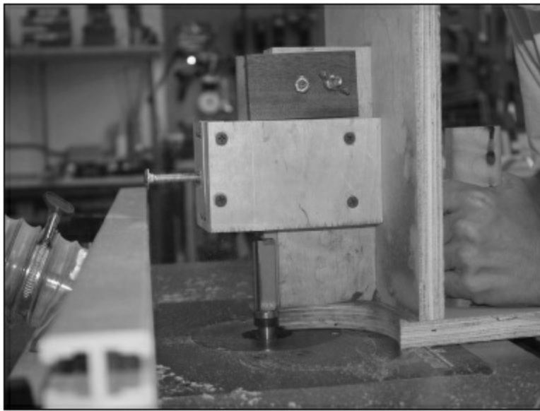
FIGURE 3.3.6. Here is the jig we use to cut the wings of the bridges. The wings are exactly 2" in length because the longest router bits that we can easily find (and for a reasonable price) are 2" long.
