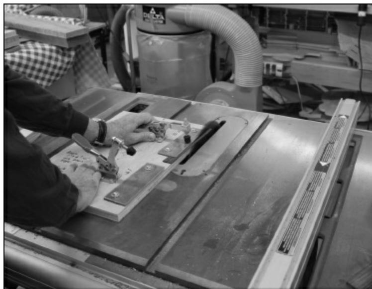
FIGURE 1.3.49. Here is the second part of the jig. After making the first cut, the graft is turned so that the freshly cut side is put inside, against the jig edge, and the rough side is outside, ready to be cut on the jig. You can see the rough sliver being cut off.
