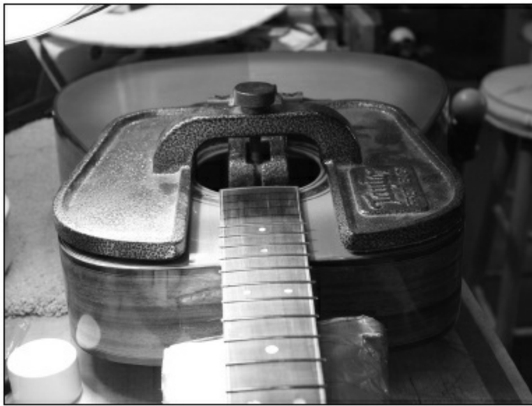
FIGURE 1.7.50. We use a Taylor fret buck to help pound in the final few frets over the guitar body. The fret buck helps disperse the hammer blows off the thin wood of the guitar top.
