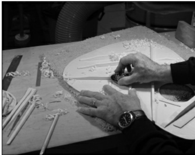
FIGURE 1.1.55. The braces must now be thinned by planing the upper corners. This takes away very little of the brace strength, but it does take away weight, which would otherwise just make the top work harder to move with the vibration of the strings. Making the braces thinner helps increase overtones that help in the overall tone of the instrument. After planing, we sand the tooling marks and make the brace smooth.
