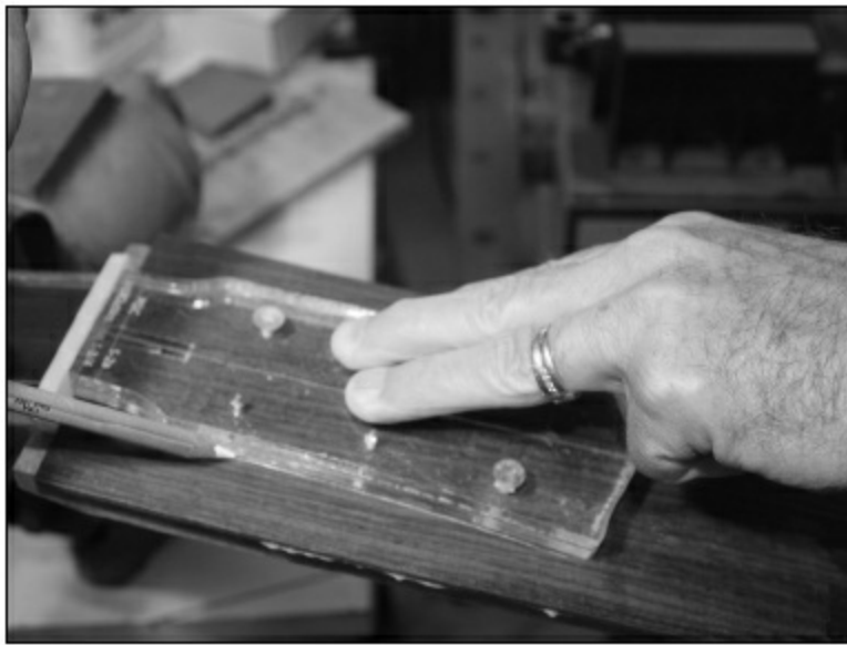
FIGURE 1.4.73. We now take our headstock template and trace its outline.
