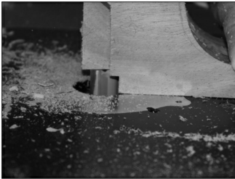
FIGURE 3.2.1. After the neck is shaped, the router table is used to cut out the ledge for the fingerboard extension. In our case, it will be \frac{3}{8} " tall. The other dimensions are set by the width of the neck and the length of the fingerboard.
