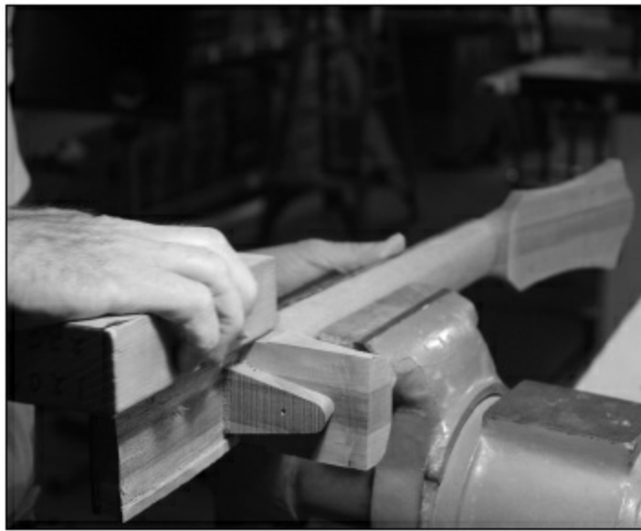
FIGURE 2.2.17. Once all the dots are put in, they are glued, and we use a sanding block to level them. Note that since we are using dark bindings, we can use superglue. However, if we were using maple or other light wood for the bindings, we recommend using a drop of Titebond to hold the dots.
