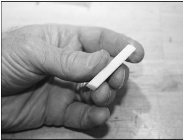
FIGURE 1.7.73. Using a sanding block and a fine file, we round off the back edge of the nut and file it smooth.
