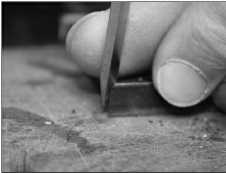
FIGURE 1.4.30. After the bindings have been glued to the fingerboard, cut them to within about 1/8" from the end of the fingerboard and use a chisel to cut a 45-degree miter cut.
