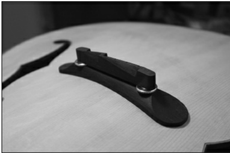
FIGURE 2.3.17. Here is a view of the final bridge that shows the carving on the top of the bridge for intonation.
