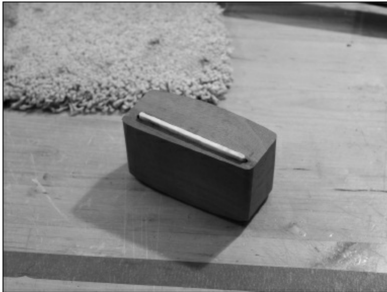
FIGURE 1.5.31. We will use this handle with a bone saddle blank that fits snugly into the bridge saddle slot.
