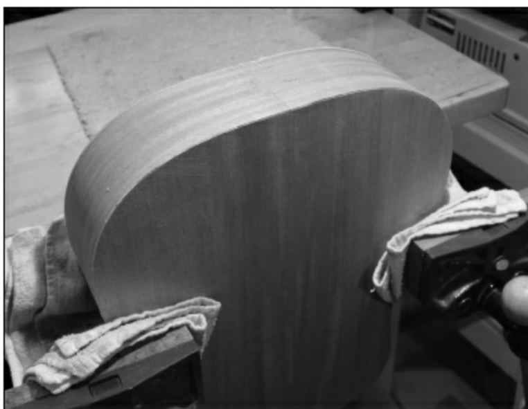
FIGURE 1.3.47. After the top and back overhangs are trimmed, the guitar is placed into a fixture we have on our benches to hold bodies while they are being worked on—two clamps, placed far enough apart for the upper bout to pass between but not so far that the lower bout passes. This way, the guitar cannot fall through and be damaged. We pad the guitar body with shop rags and make sure it is secure.
