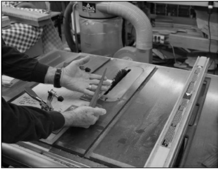
FIGURE 1.3.50. Here is the final graft. Note the grain is lengthwise on the graft. This will make it stand out and look better when it is inlaid.
