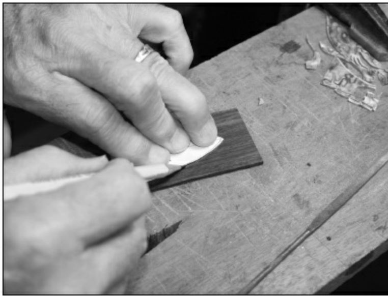
FIGURE 1.4.98. Before we complete the placement of the bird's tail, we must get the truss rod cover made. We are using a piece of scrap from the headstock laminate, so the match will be a good one.
