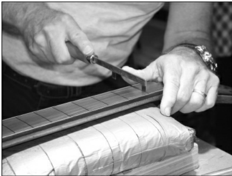
FIGURE 1.7.37. We now have to clean out the fret slots. First, we will get rid of any glue in the slots. We already know there is some glue in the first and thirteenth slots from when we used the pins for alignment when gluing the fingerboard to the neck. Shown is a Stew-Mac fret slotting tool—very handy for this job.
