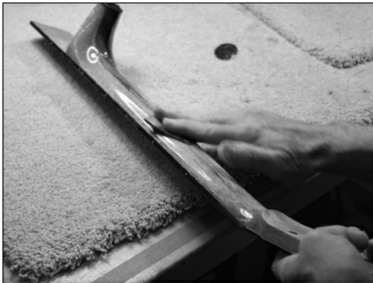
FIGURE 1.6.21. For the long, curved portion of the back of the neck, hand sanding is the best. At this point, which is probably the final sanding before spraying, we are using 600-grit wet/dry sandpaper. It is very easy to sand through, in which case, another coat would have to be applied.
