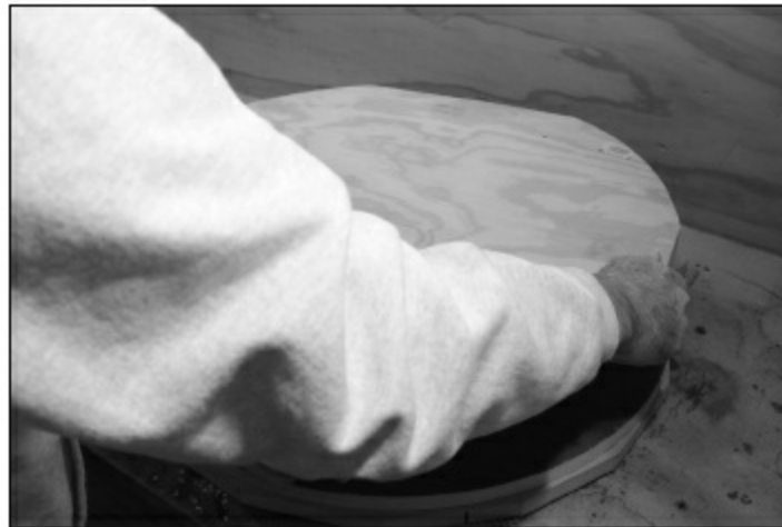
FIGURE 1.3.25. Now, we use the hollow mold forms to sand the kerf down to the level of the sides, endblock, and headblock. Remember to use the proper radius form—25' for the top and 15' for the back (in our case—many other guitar makers use different radii).
