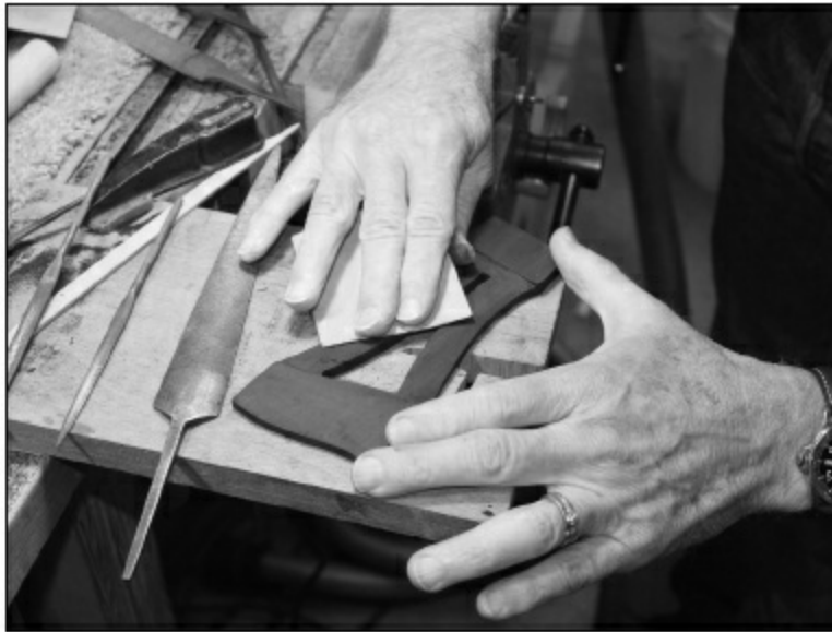
FIGURE 2.3.23. Once the shape is acceptable, we sand out all the tool marks.
