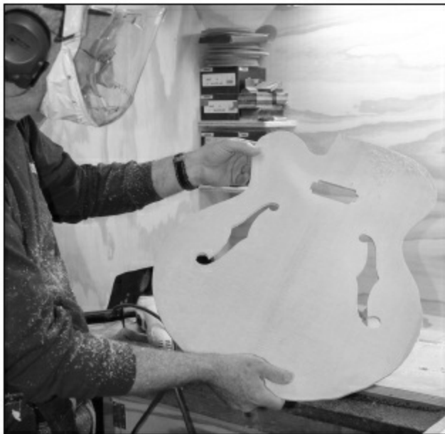
FIGURE 2.1.21. Here is the final cut of all the holes. This is a very dirty job. Notice all the sawdust on my shirt. This is the reason I use a 3M Breathe Easy system, since it has a good face shield and blows filtered air through the helmet. This also keeps the shield from fogging up. I'll usually keep this on until I've vacuumed myself off and have gotten most of the dust away from the area. We also have smaller, simpler face dust filters for jobs that don't generate as much dust.
