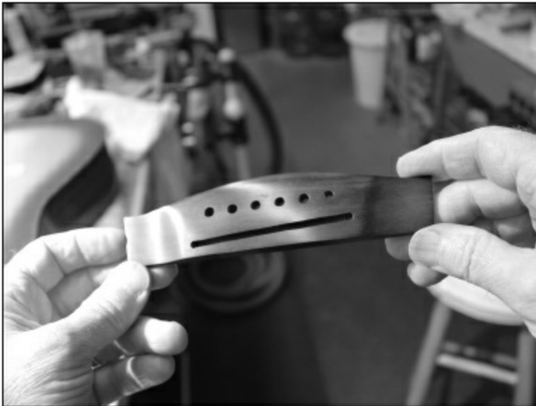
FIGURE 1.7.23. Here is the final bridge, sanded, buffed, and ready to glue.
