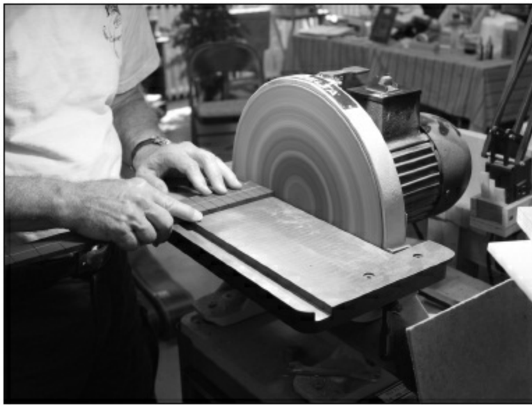
FIGURE 1.4.26. After both sides of the fingerboard are routed smooth, sand the board smooth on a disc sander at the twenty-second fret (assuming you have a twenty-one-fret fingerboard). The nut side of the fingerboard can be left alone for a while.
