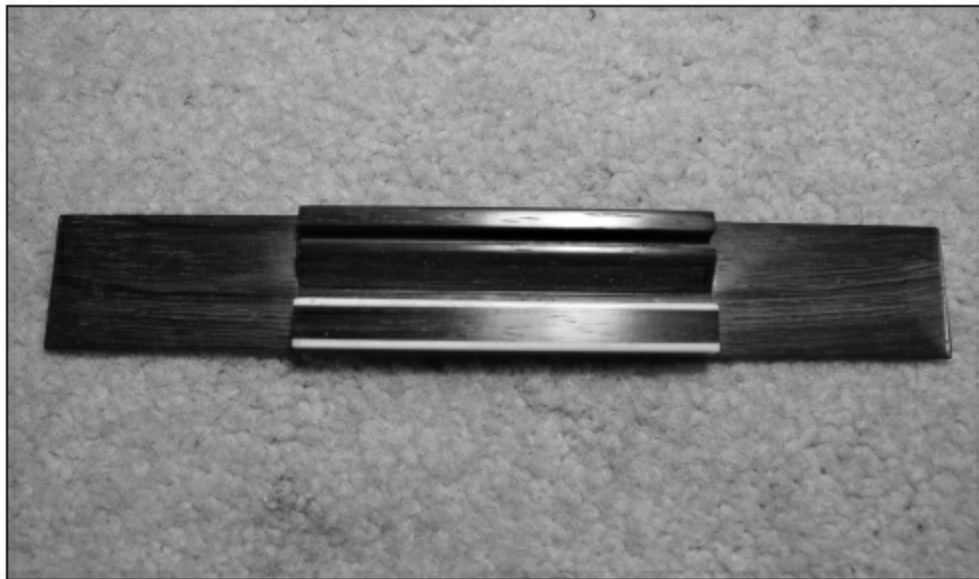
FIG, 3.3.20. Here is the final bridge. Note the taper at the edges of the wings (you can particularly see it on the right side). That taper was done by hand with a file and a sanding block.
