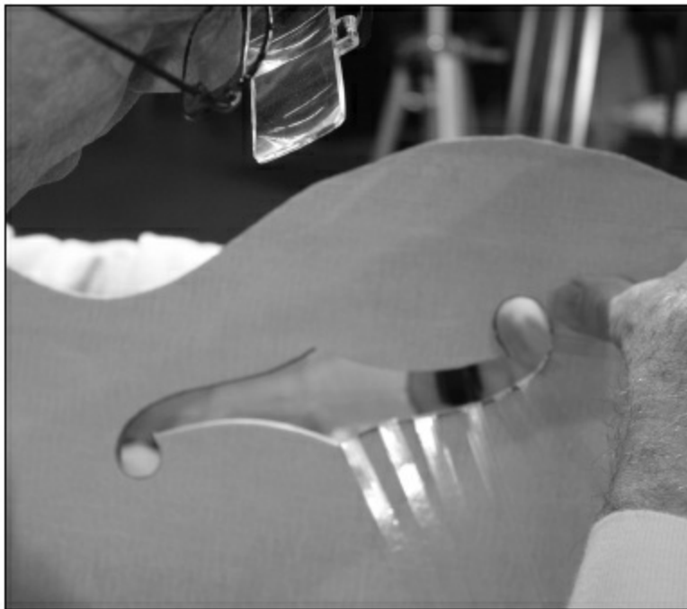
FIGURE 2.1.35. Here is the maple layer being taped over the black fiber.
