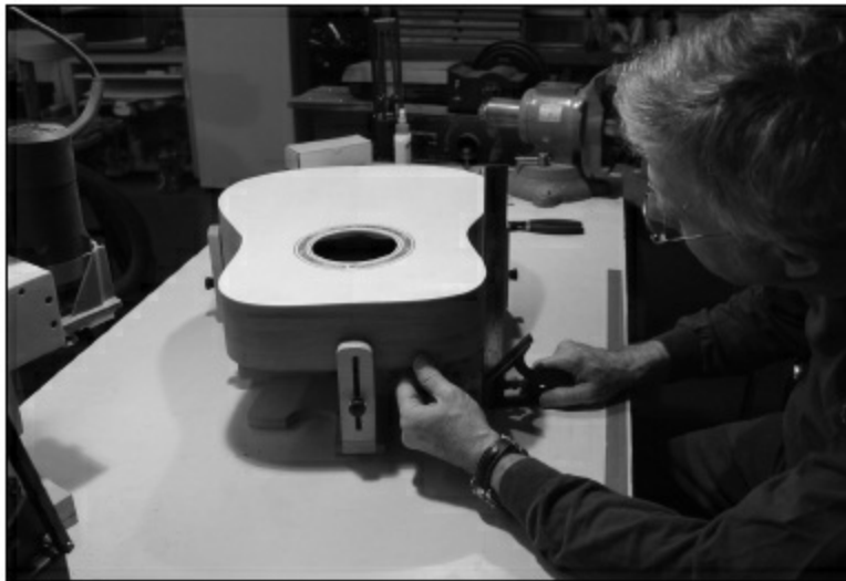
FIGURE 1.3.65. As the bindings are cooling, it's time to cut the binding and purfling slots in the body. We are using the LMI binding jig (originally designed by Tom Ribbecke), and first we must be sure the body sides are perpendicular to the table.
