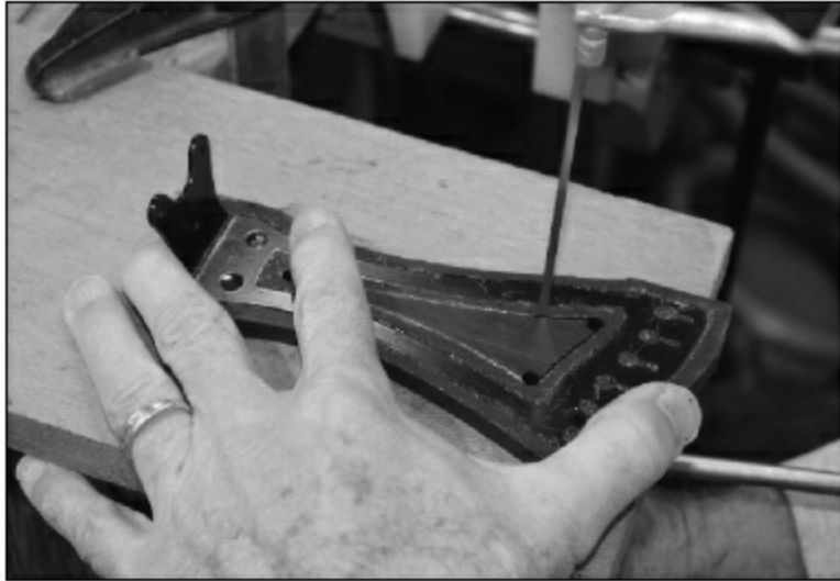
FIGURE 2.3.21. After epoxying the metal skeleton into the ebony slot, we have the option to leave the bridge as a solid piece or to cut out the center and create a trapeze-style tailpiece. In this case, we are creating the trapeze-style tailpiece. We drill three holes in the corners and draw a line where we will cut with a coping saw.
