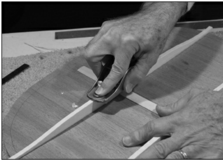
FIGURE 1.2.21. Using a small block plane, each brace is carved down using a plane to a height of 5/8'' in the center.
