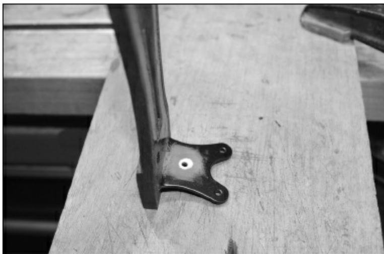
FIGURE 2.3.28. We have sanded off the powder coating where the balls of the strings will touch the bottom of the tailpiece. Earlier in this chapter, we mentioned that we designed this tailpiece so the strings could be grounded. This step and the next make that possible.
