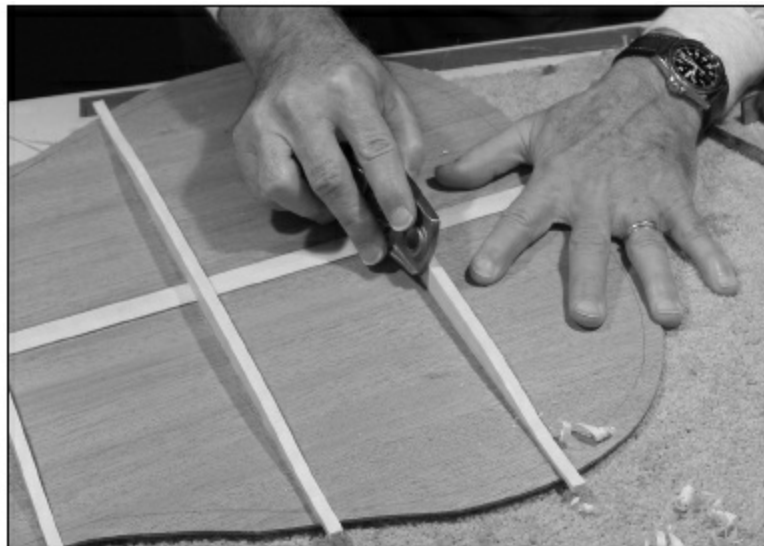
FIGURE 1.2.23. Finally, a plane is used to shave material off the sides of the braces, and after a little sanding, the back is ready.
