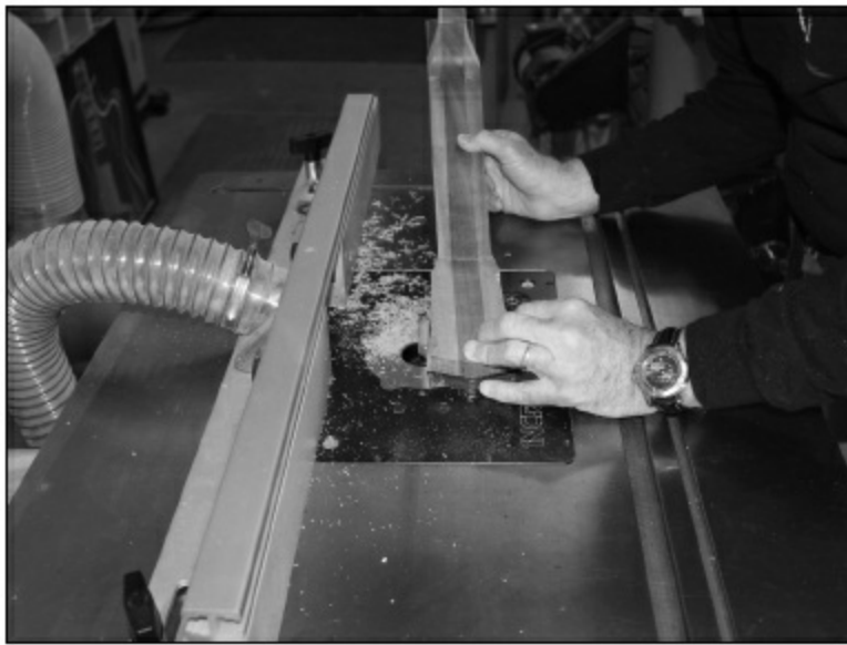
FIGURE 1.4.81. We then use the headstock template as the routing template and rout the headstock using a flush-trim bit. You must be certain to push against the direction of the router bit—especially along the very top of the headstock—or it could kick back and possibly ruin the headstock, or cause an injury
