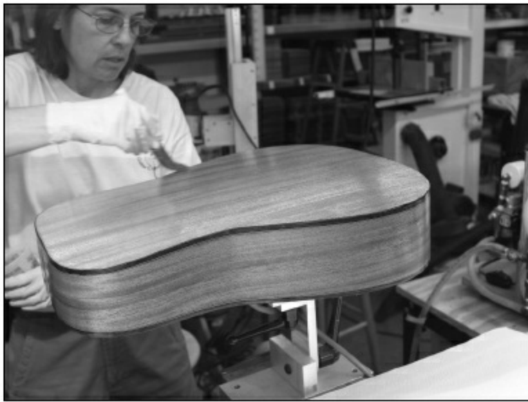
FIGURE 1.6.10. Next, we apply the epoxy to the back. After applying, you should use a credit card blank or squeegee to smooth the surface the best you can. Very thick or lumpy surfaces will be difficult to sand down later.
