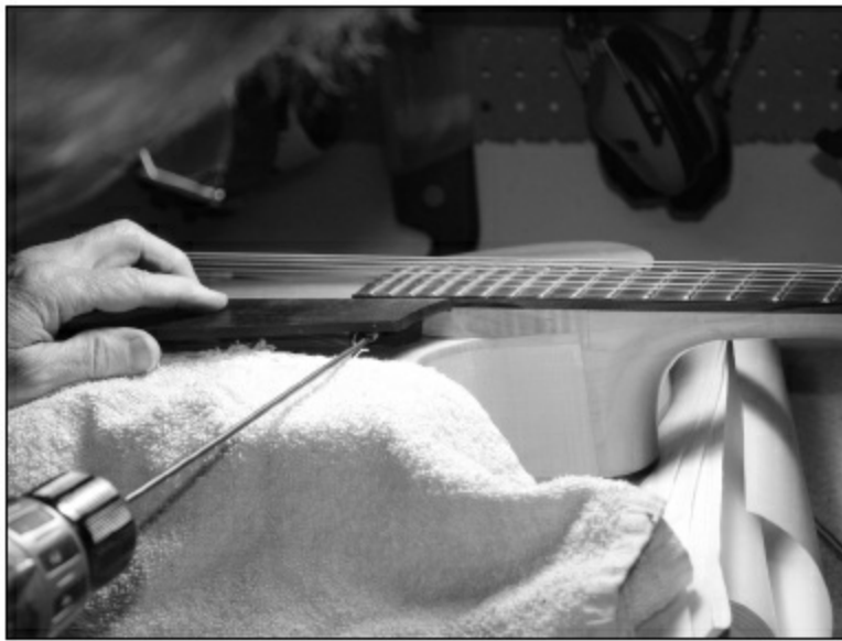
FIGURE 2.3.36. Using the same size drill bit (in this case, a long aircraft bit), drill through the hole in the block, just scoring the surface of the fingerboard. We will use a smaller bit to actually drill out the screw hole in the fingerboard. We want the screw to pass easily through the block, but bite into the fingerboard.
