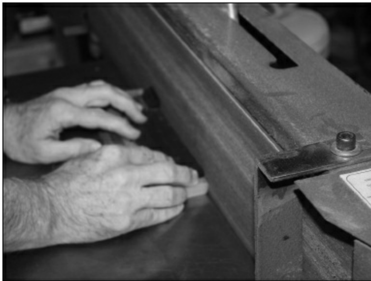
FIGURE 2.3.33. We use the angled block to sand the edge of the block (and the edge of the pickguard). With this angle sanded onto the edge, once the block is screwed to the fingerboard edge, the pickguard will angle down 3 degrees, making the fingerboard much more comfortable to use.
