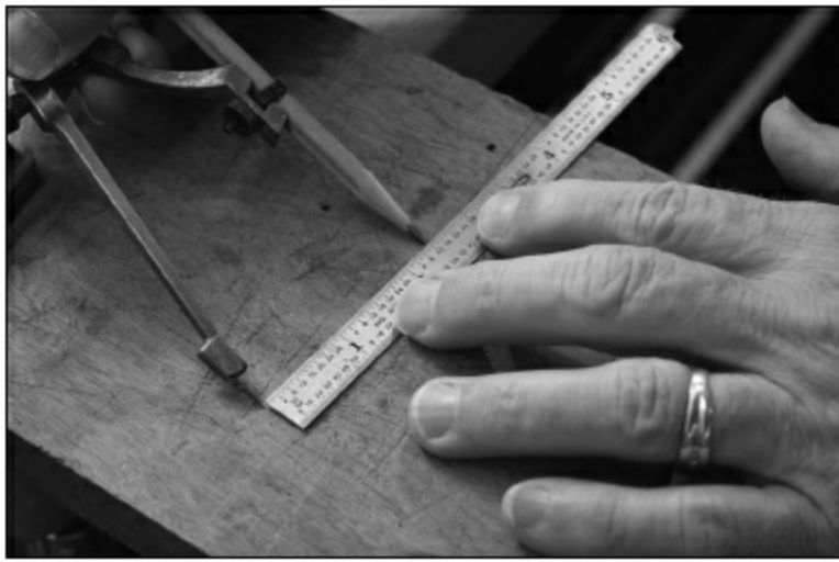
FIGURE 1.1.9. The inside radius of the abalone ring is 2 \frac{3}{8} ", so we set a compass for that radius.
