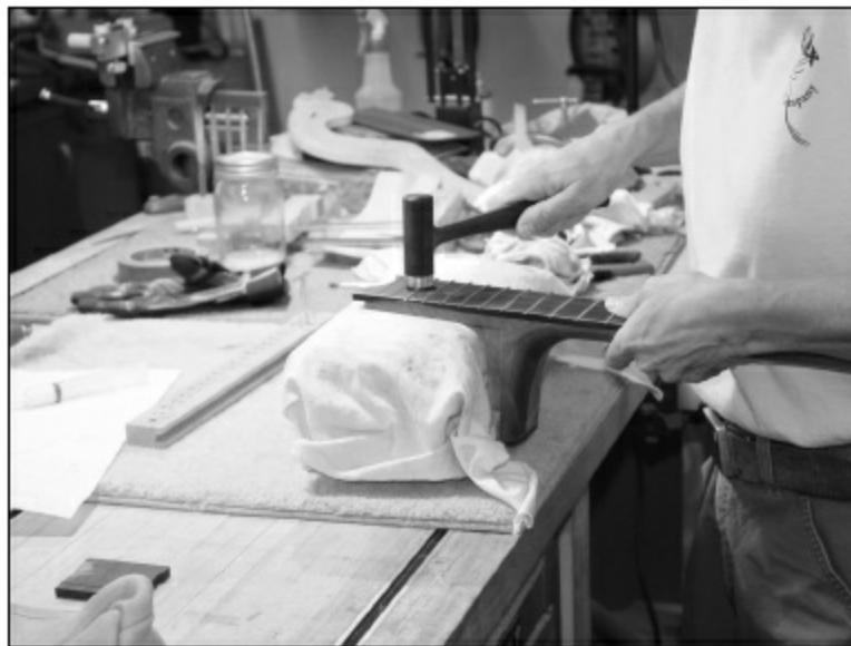
FIGURE 3.4.15. The frets over the fingerboard extension are pounded in using the bag of lead shot to stabilize the shock.
