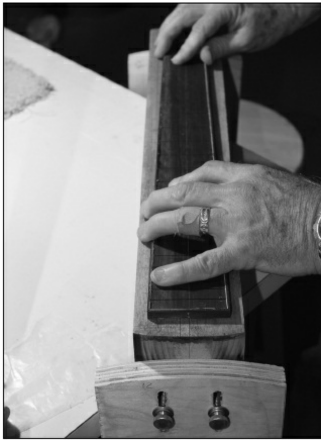
FIGURE 1.4.35. The fingerboard is secured with double- sided tape to the underside of our radius jig. Care must be taken to be sure the centerline on the fingerboard is properly aligned to the centerline on the jig. Also, be sure the back side of the fingerboard is taped to the jig. It would be a shame to sand the radius onto the wrong side of the fingerboard.
