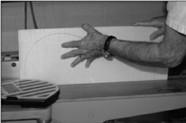
FIGURE 1.1.2 Next, we put both halves together. Make sure the edges that are to be glued are down against the jointer table. Then we joint the edges.
