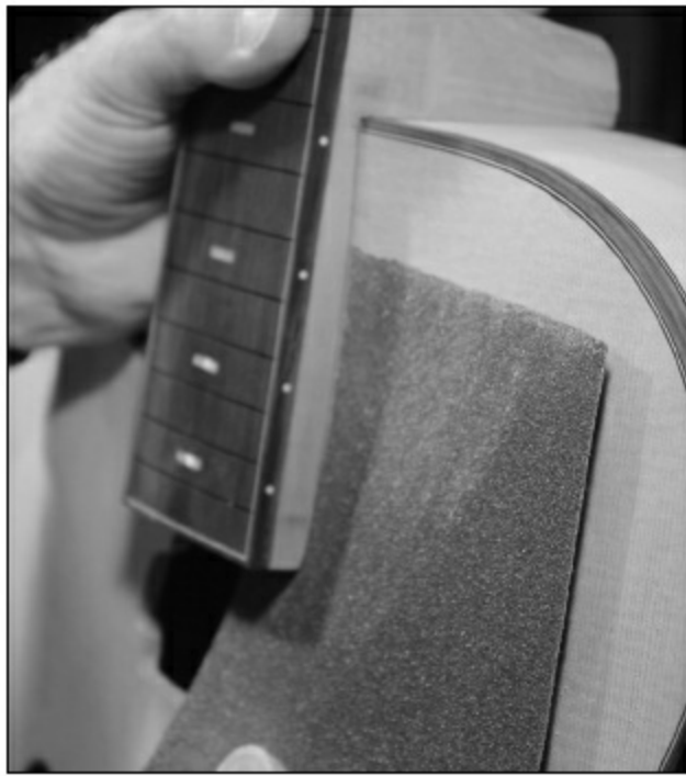
FIGURE 2.2.21. We also pull sandpaper to make the final fit on the fingerboard extension. Both the heel and the fingerboard extension must fit just right to the guitar body.
