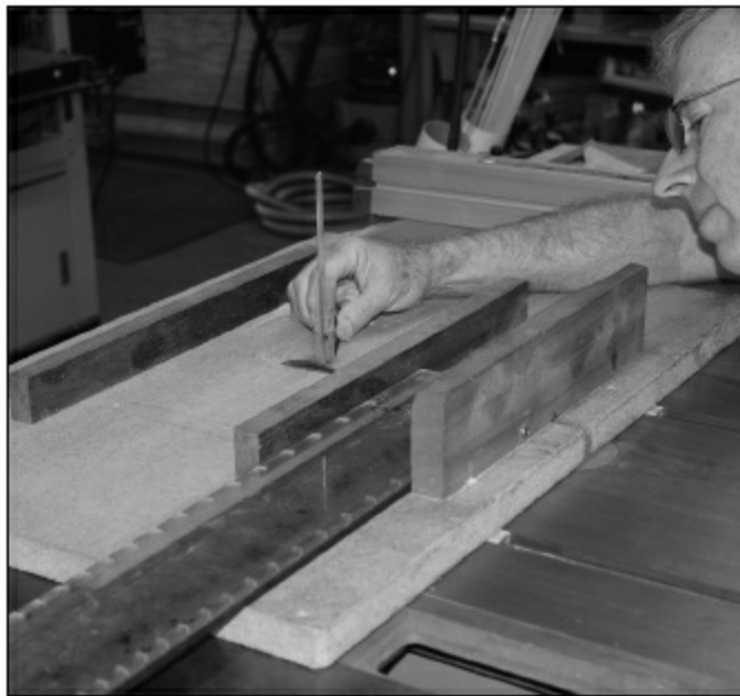
FIGURE 1.4.16. After the blade is in place, we put our sled onto the saw and measure the height of the blade above the sled table. This is how deep the blade will cut into the fingerboard. Ideally, it will cut at least halfway through the board, maybe just a little more. After we've made a measurement, we will try a test cut with a piece of scrap. Once we're happy with the depth of cut, it's time to actually cut the fret slots. Notice our fingerboard has been taped to our slotting template with double-sided tape. The jointed edge is perfectly aligned with the edge of the template being used for the fret slot measurements. In this case, it's a 25.31" scale length, and the 25.31" slotting template is the one on the right side of the template.
