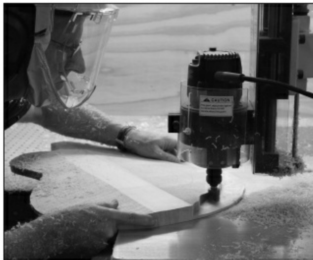
FIG 2.1.4. Here the rout plan is drawn onto the guitar top. Now, it is time to route the levels into the top.
