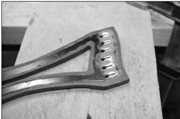
FIGURE 2.3.28. We have sanded off the powder coating where the balls of the strings will touch the bottom of the tailpiece. Earlier in this chapter, we mentioned that we designed this tailpiece so the strings could be grounded. This step and the next make that possible.
