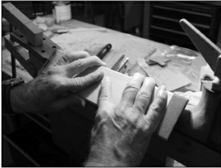
FIGURE 1.4.122. We like to use a flat sanding board with 80-grit sandpaper attached to it to be sure the entire board is level all the way across.
