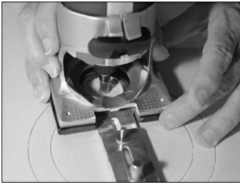
FIGURE 1.1.22. The section of the arc that will be directly under the fingerboard can be used to test the placement of the center circle. If it's slightly off, it can be adjusted and reset and retested. When it's right, we cut the inner circle. After cutting, we sand it to clean up our work.
