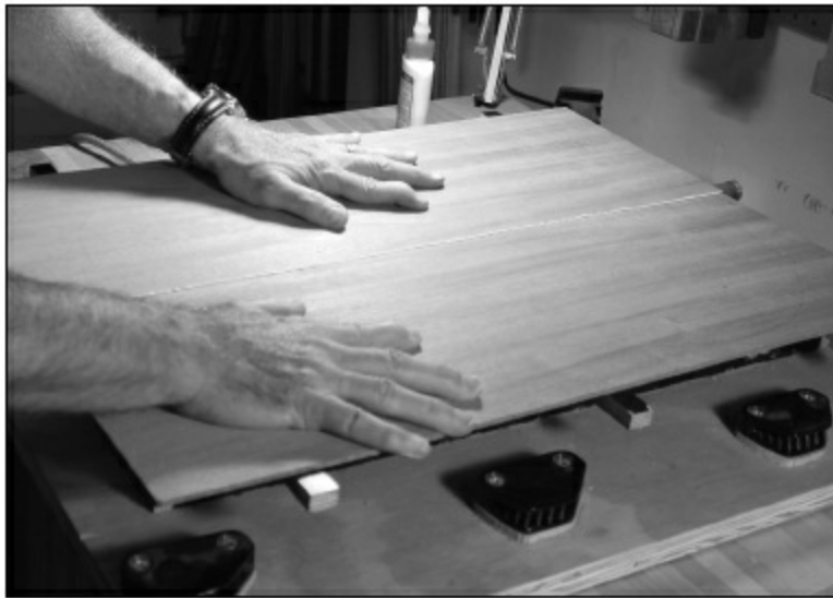
FIGURE 1.2.6. We use the plate-joining jig to glue the back together.
