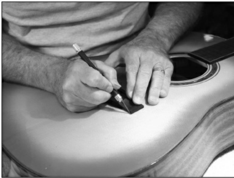
FIGURE 1.7.18. Now, while the pins are holding the bridge in place, we scribe around the bridge, exactly as we did with the fingerboard overhang.
