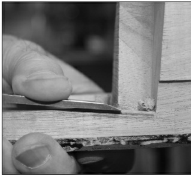
FIGURE 2.2.13. Now we use a chisel to carve away the material up to the pencil line. This makes for an initial fit of the neck. We will now take care of a couple of other items before the final fit is complete.
