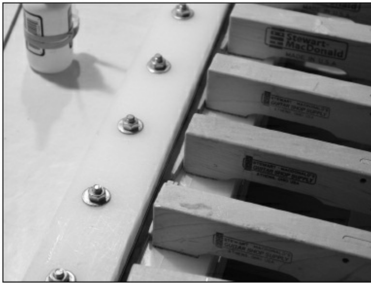
FIGURE 1.3.62. In this photo, you can see the Indian rosewood binding (sanded flat on one edge) being clamped against a strip of b/w/b purfling by a series of small wedges between the cam clamps and the jig. We will push both the binding and purfling down solidly against the bottom of the jig using a small flat-blade screwdriver.
