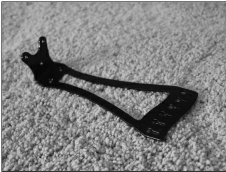
FIGURE 2.3.18. Our tailpieces are built around a stainless steel skeleton. We designed these pieces for a couple of reasons. First, we wanted to be sure that the tailpiece was strong. Even if the ebony gets dry and cracks, we want the tailpiece to hold. Second, we wanted to be able to ground the strings in case the guitar has a pickup (which is most of the time). We had our design built by a small manufacturing company and then had them powder coated.
