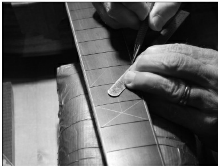
FIGURE 1.7.33. After the fingerboard is level, we inlay the fret markers. In this case, we’re putting in a basic pattern of MOP dots, which is what our customer ordered.
