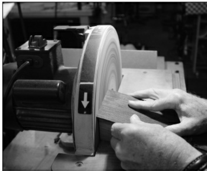
FIGURE 1.4.68. Now we put the same angle onto one edge of the headstock laminate (if it's not obvious, this is the edge that will go up against the nut).
