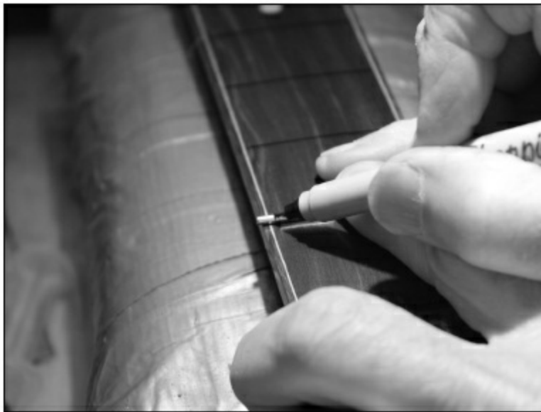
FIGURE 1.7.42. After all the frets are cut, we take each fret, hold it up to its respective slot, and, using a Sharpie, mark slightly inside the purflings on both sides, by about 1/32'' .
