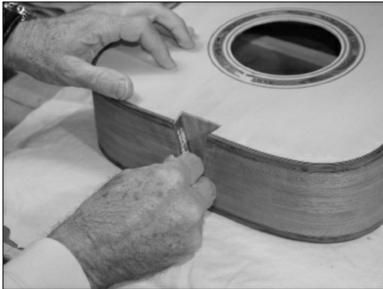
FIGURE 1.4.130. Once the shims are glued to the dovetail, we are marking the headblock side of the dovetail with chalk.
