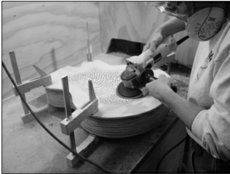
FIGURE 2.1.16. Now, as before, the angle grinder is used to take away the bulk of the excess. During steps like this, a lot of dust and wood chunks are thrown about (not to mention that an angle grinder along with a dust collector makes a lot of noise), so proper dust, eye, and ear protection must be used. Once the sanding gets close to the bottom of the drilled holes, switch from the angle grinder to the random orbital sander, just as we did on the top side above (see figure 2.1.8)
