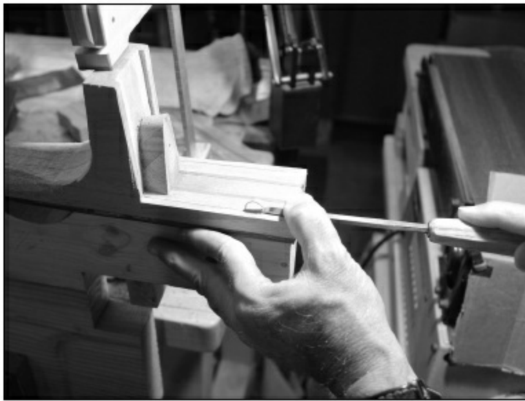
FIGURE 2.2.11. Now we will do the same thing to the underside of the fingerboard extension, for the same reason. We only want to fit the shoulders to the guitar top, rather than the entire surface of the fingerboard extension.
