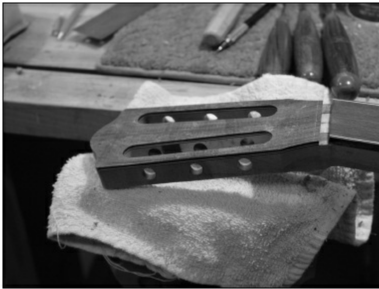
FIGURE 3.2.15. Here is the headstock after the holes and slots have been cut. The dark square on the inside of the slot is the veneer between the mahogany and the maple on the neck.
