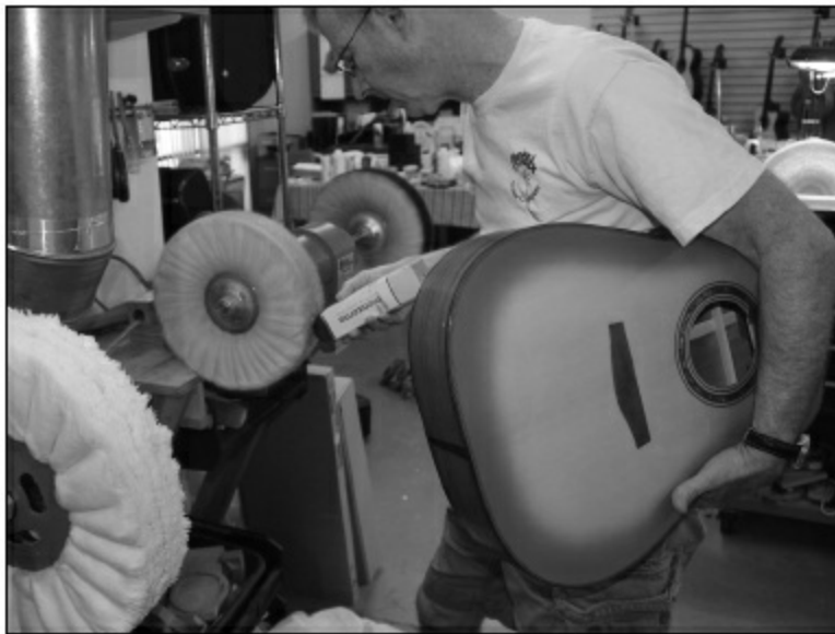
FIGURE 1.6.39. Be sure to put buffing compound onto the wheel every few minutes. This is yet another reason to practice finishing on a cheap piece of wood before you try on your nice acoustic. If you put too much buffing compound on the wheel, it will leave residue on the surface that is difficult to remove. If you use too little, the wheel will not be very effective.
