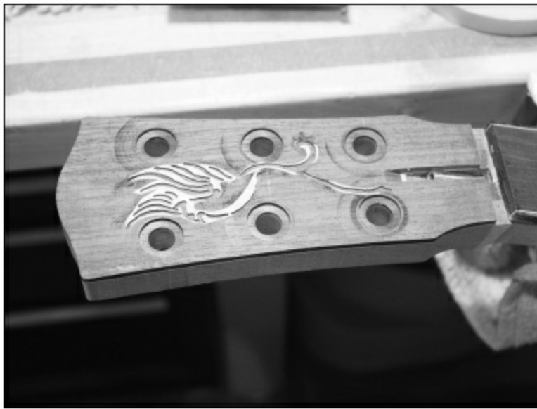
FIGURE 1.4.100. Once we have placed the truss rod cover, we can determine the best placement of the bird's tail. The entire logo is shown in the photo. It was cut out with the Dremel and is ready to inlay.
