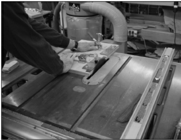
FIGURE 1.3.48. Now we are ready to make the end graft. First, we select a piece of Indian rosewood and cut it on the band saw to the approximate shape, only oversized. We place it in the first clamp-down of the jig, and one edge is cut clean on the table saw. This jig was the idea of Charles Fox. We want to thank Charles for permission to show the jig.
