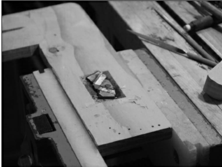
FIGURE 3.1.10. Here is one rosette piece with the inlay done. Since the inlay extends slightly beyond the Macassar ebony, it will have to be resanded with the same jigs originally used to create the inside and outside radii.
