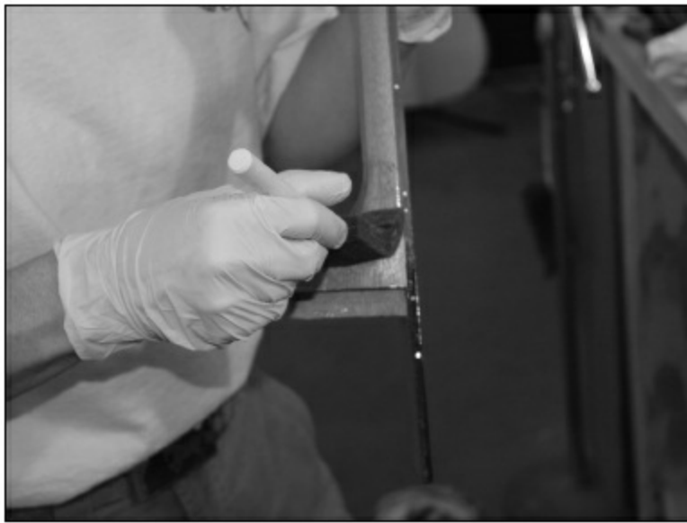
FIGURE 1.6.12. Next, we spread epoxy on the neck. First, we spread it on the front, back, and sides of the headstock, then on the heel and the fingerboard overhang.
