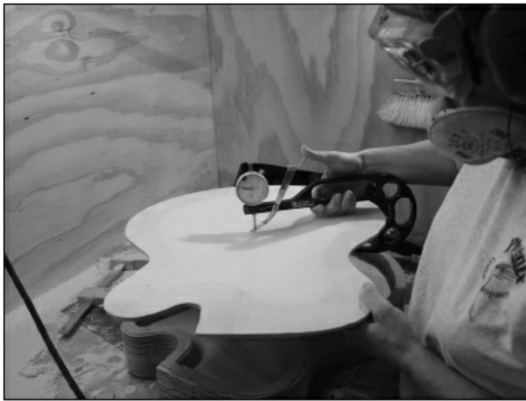
FIGURE 2.1.17. Here is the fully carved top. We check the thickness, and any areas are too thick, they are marked and either sanded or scraped down. This is another time that we will hold the underside of the top in the light to see if there are any shadows that show an uneven surface. Any traces of unevenness must be smoothed out prior to gluing braces to the top.
