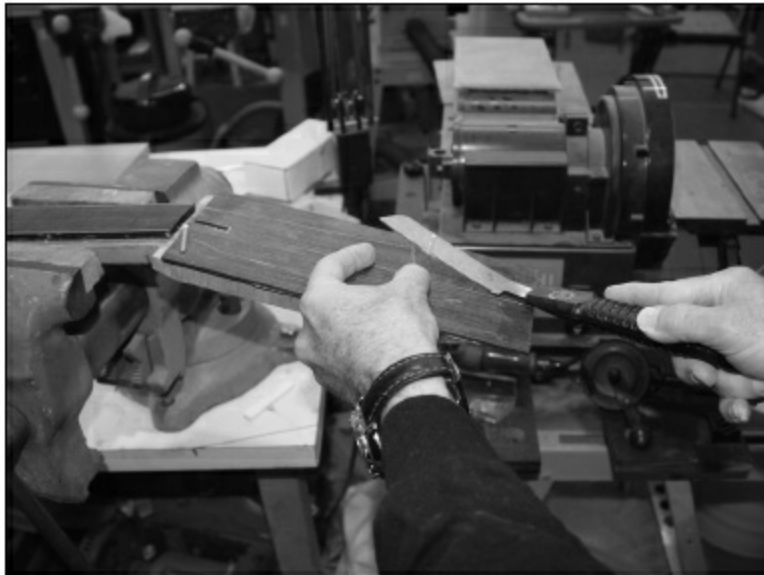
FIGURE 1.4.76. After we drill the holes, the alignment dowels are removed so glue can be applied to the surface of the headstock. Then the headstock laminate is placed back down where it belongs, and the dowels are put back in their holes. Once inserted, they are cut with a flush-trim saw.
