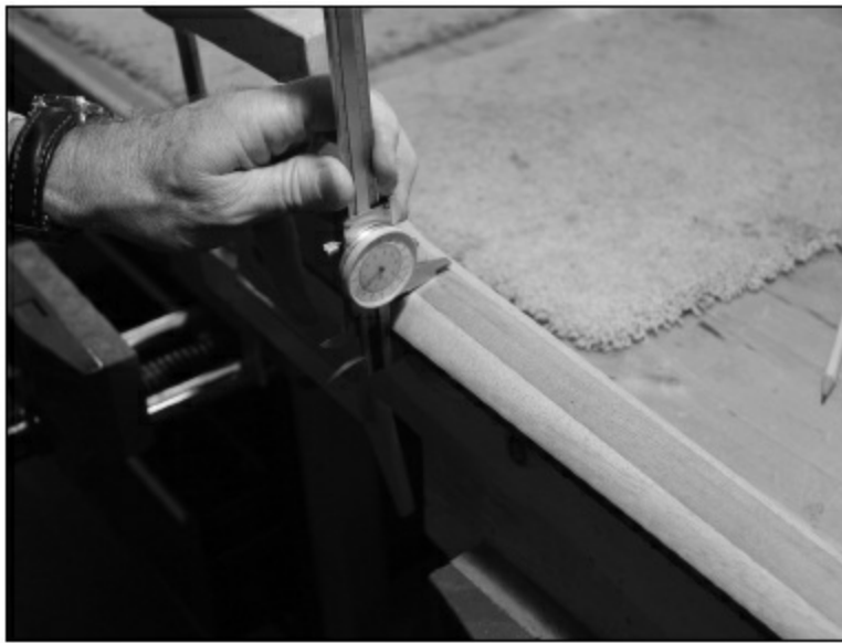
FIGURE 1.4.124. In addition to checking the radius of the neck, we check the neck thickness using a caliper. Typically, at the nut (or just in front of the nut), the thickness is \frac{13}{16} " and increases by about \frac{1}{16} " to \frac{7}{8} " as you move down the neck to about the ninth fret. Some guitars increase in thickness by more than \frac{1}{16} , but our customers tend to like this smaller increase.
