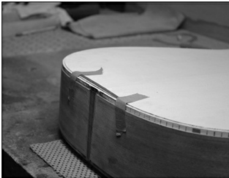
FIGURE 1.3.71. This photo shows how the ends of the end graft are trimmed by taping a piece of purfling against the guitar top (and back) and rerunning the binding cut. This will trim the end graft exactly the thickness of the purfling higher than the original binding cut.
