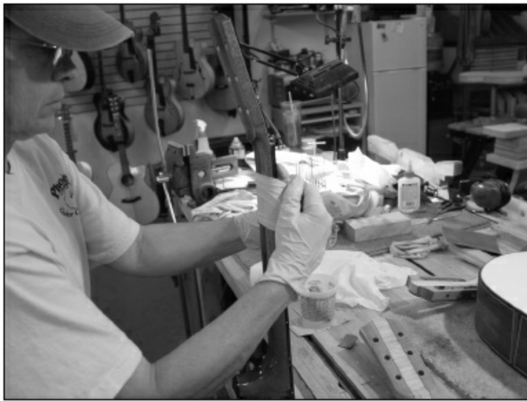
FIGURE 1.6.14. We will use a glove (like the ones being used in the photo) to help spread the epoxy down the neck to be sure the application is smooth. Be sure that you don't push against the neck, putting stress on the fingerboard overhang in the vise. Note that pressure is being applied on the back of the neck with the glove and on the front of the neck (with the fingers of both hands). The fingerboard is taped off for the epoxy step (and through finishing) to keep it clean.
