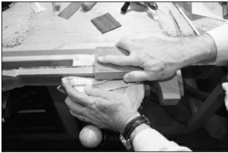
FIGURE 1.4.110. Last, we use a flat sanding board to sand the dots so they are level.
