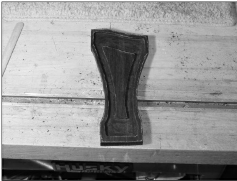
FIGURE 2.3.20. After routing out the shape of the metal skeleton, we cut around the shape with the band saw.
