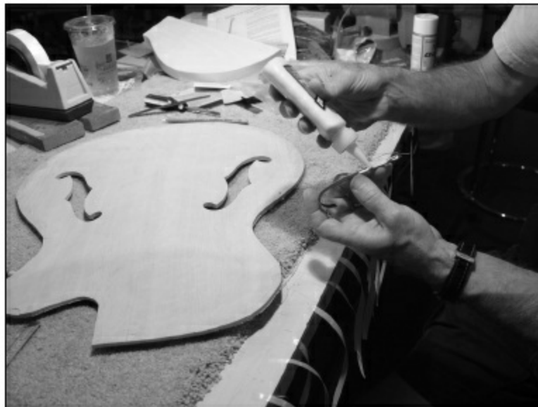
FIGURE 2.1.27. After the fiber has been cut, rebend the loop and apply glue. Don't use superglue in this case, or you risk the glue staining the light top a yellow color. We use Titebond for this step. If you use plastic bindings, Titebond may not be the best. There are good plastic glues for this. Note we have cut several strips of fiber tape ready to tape the binding down.
