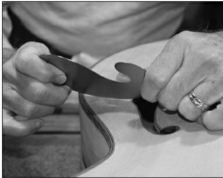
FIGURE 2.1.70. This photo shows using a curved scraper to carve the recurve. Drawing 2.1.3 shows what the recurve should look like. The groove made by the scraper must be smoothed out to look like the natural curve of the arch before final sanding is done. Note that if you are making an acoustic archtop, the recurve can be deeper, helping the top to flex farther. However, if you are making a guitar that will be played with a pickup, the recurve cannot be as drastic, or the guitar is likely to have a feedback problem. That is why we show the minimum thickness in the recurve area as being 3/16" , since this guitar (and most of the archtops we make) will have a pickup. We have found this recurve thickness to have a very pleasant acoustic tone (and add significant acoustic tone to the amplified sound) without a significant feedback issue. Note that you can always make an amplified instrument feedback with too much volume or if you're too close to the amp.
