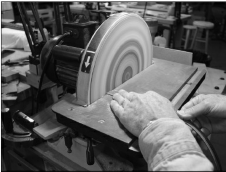
FIGURE 1.3.75. Once both topside bindings are marked, they are held together and the ends are sanded down to the marks (maybe shy by just a teeny little bit).
