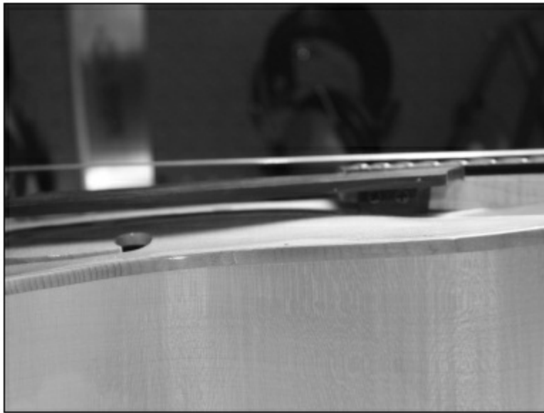
FIGURE 2.3.39. Here is the final pickguard. Note how the pickguard angles down from the end of the fingerboard to the end of the pickguard. We like to install the pickguard after the neck is on the guitar and the strings are on. This way, we can make sure the angle is right. If the angle of the pickguard is too shallow, the edge of the pickguard is too close to the strings, and most players find this problematic. Also, note that from this angle you can see that the pickguard block has been sanded to an angle to match the angle of the arch of the top.
