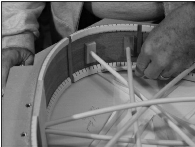
FIGURE 1.3.27. Each brace that crosses under the kerf must be marked at the point it touches the kerf. In addition, the kerf must be marked where the brace intersects it.
