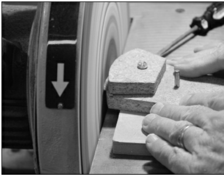
FIGURE 1.1.14. Here is the jig in use. The top two pieces of particleboard are clamped together with the screw on the top, and they pivot with the 3/16" pin. Once the jig is set up, it is very easy to make multiple pieces with the same outside radius.
