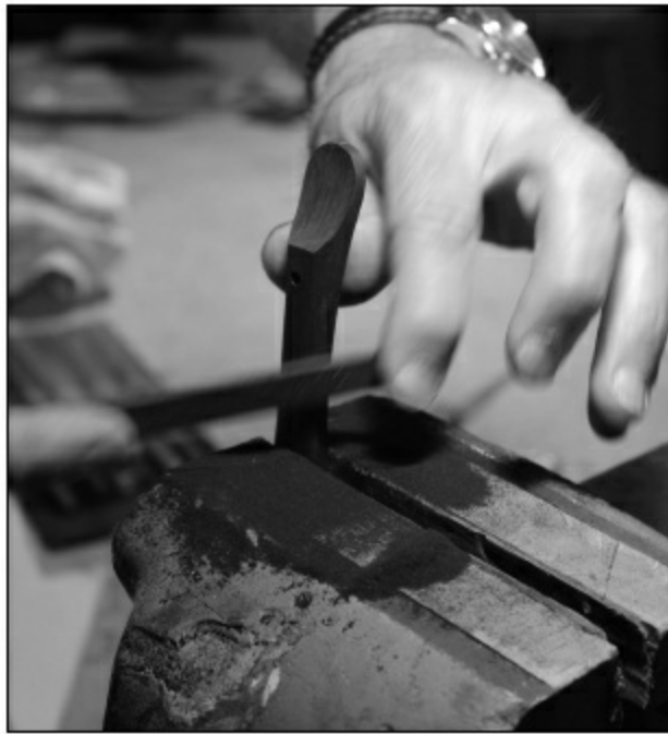
FIGURE 2.3.9. Once the wings are shaped, we put the bridge into a vise and taper the sides of the bridge. This makes the bridge look more streamlined and removes unnecessary weight.
