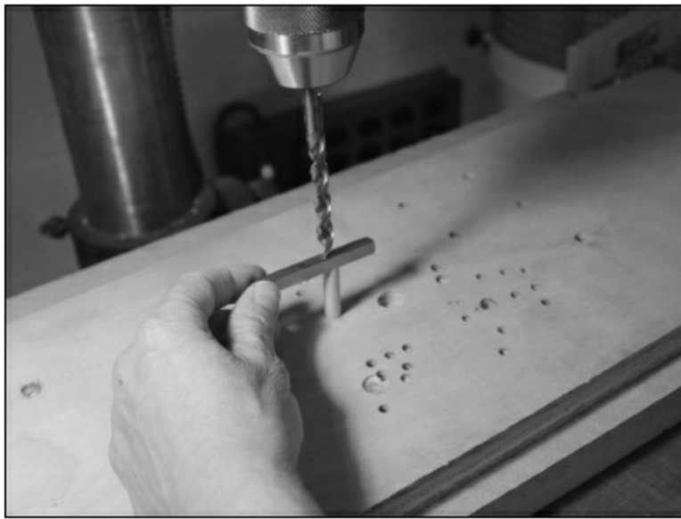
FIGURE 2.1.11. Since we're going to carve the top to be 1/4" thick, we will use a brass setup block and set the drill to stop at exactly 1/4" above the peg.
