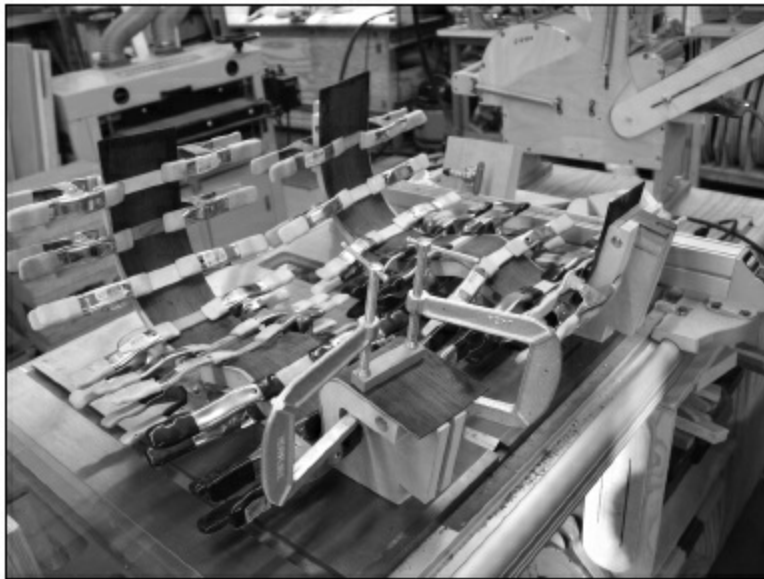
FIGURE 3.1.25. Here are both sides of the classical guitar. The cutaway is in the foreground, and the noncutaway is in the background. Note that if the sides do not fit comfortably into the molds, they may have to be heated over a hot pipe to make them fit. They should not be forced into the molds if they don't fit. For an excellent description of pipe bending, see Guitarmaking Tradition and Technology , by William R. Cumpiano and Jonathan D. Natelson
