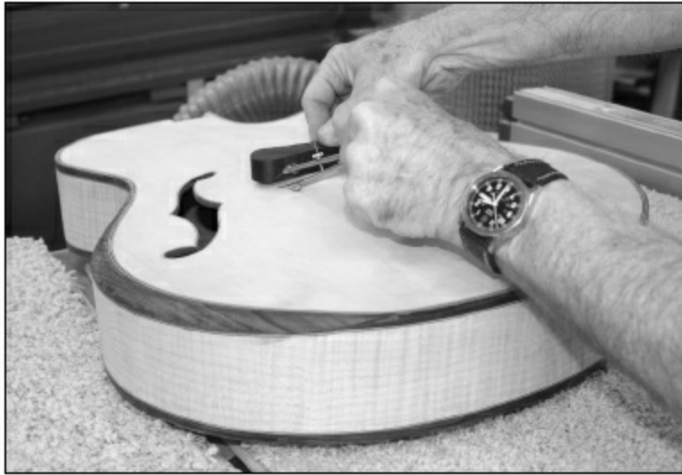
FIGURE 2.3.2. The bridge blank is placed between the points of the F-holes (very close to its final position), and a line is drawn on the blank with a compass, following the shape of the arch.
