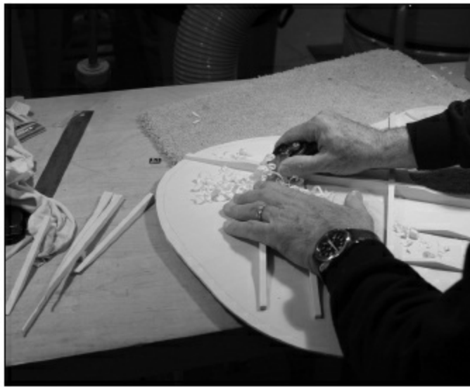
FIGURE 1.1.54. Now we carve the legs of the X braces using a curved-sole plane. A chisel can also be used, but our experience shows that we are more accurate using the plane. The brace will be 5/8 " tall at the center and remain flat for about 1.5" or so, slope down to 3/8 ", and remain at that height until about 3" from the edge of the top. At that point, we slope it down and keep it at 1/8 " until the guitar edge. Note that this is how we carve our braces. We do not scallop our braces as many builders do. We have had excellent tonal results from this method (having compared our sound with many other guitars) and have not had any issues with bellying.
