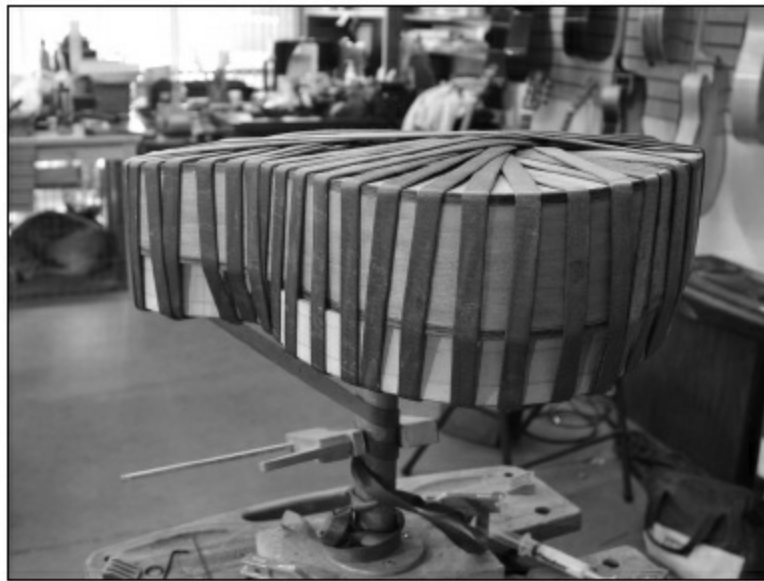
FIGURE 1.3.85. Here are all four pieces of binding, all strapped down. Note how we use a cam clamp to tie down the end of the nylon rope. Now for the details up at the neck end.
