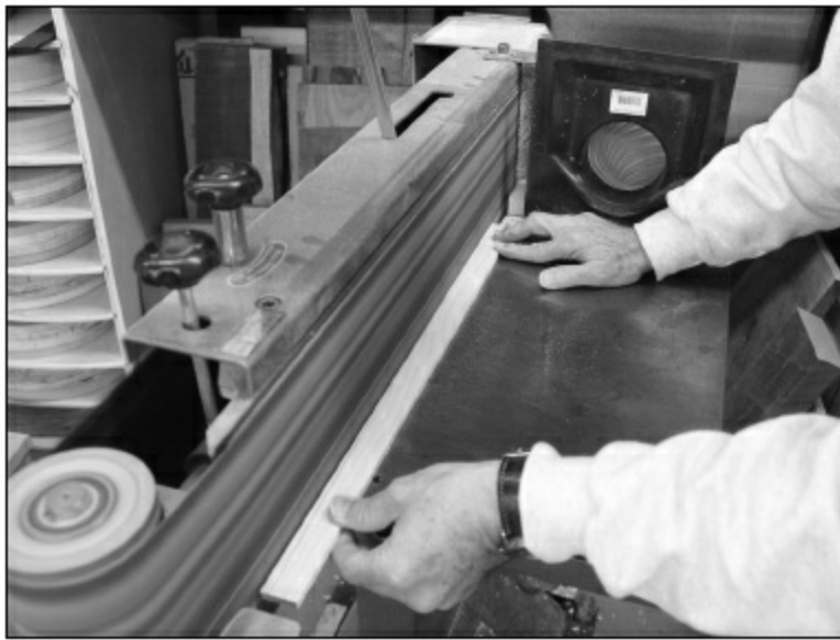
FIGURE 1.1.34. Now, we sand the drawn radius onto the bottom of the braces.
