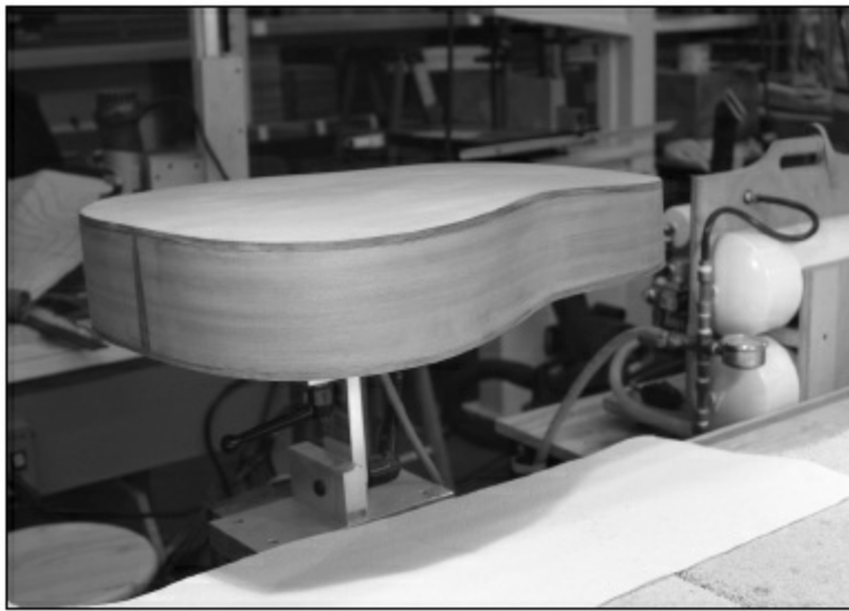
FIGURE 1.6.5. We now use a vacuum clamp from LMI to hold the body, using the same vacuum pump that we have shown before.
