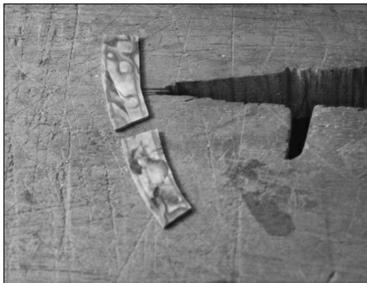
FIGURE 1.1.10. After drawing both the inside radius of 2 \frac{3}{8} " and the outside radius of 2 \frac{5}{8} " onto a piece of abalam (it's difficult to see the pencil lines in the photo), we will cut out multiple pieces to form the abalam arc. We will cut well outside the lines to allow for any error.
