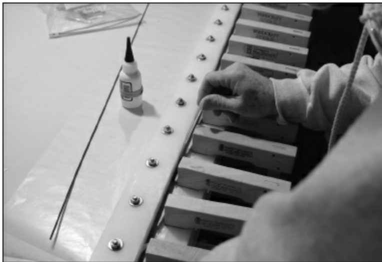
FIGURE 1.3.63. Once we're happy that the bindings and purflings are solidly down against the base of the jig, we will use a small pipette filled with superglue to run a bead of superglue between the binding and the purfling. Use the very thin superglue, and it will have no problem seeping between the clamped binding and purfling to form a good glue joint. Note: do not use superglue if you are using light bindings (like maple). Superglue can stain the very light woods yellow, and the stain will not sand out. If you use lighter woods, it's best to use epoxy for the glue step, then clamp the bindings and purflings together after gluing. You do not want to use regular wood glue, because we are going to put the bindings into a hot bender, and we don't want the glue joint to come apart.
