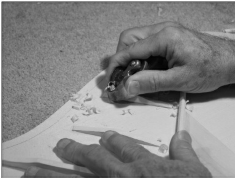
FIGURE 1.1.57. Finally, we will use the curved-sole plane to slightly scallop the straight edges of the finger braces—again, this is just removing unnecessary mass.
