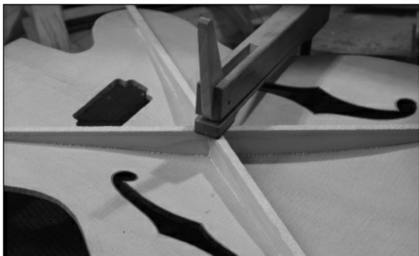
FIGURE 2.1.51. Here is the X brace, all fit together and ready for gluing.
