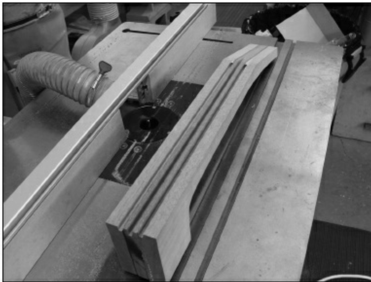
FIGURE 1.4.11. Next, we use a 6 mm metric bit to cut the slots for the carbon fiber rods. We put these rods as stiffeners on all our steel string and archtop guitars. They add very little weight but add a lot in strength. The rods are 5 mm wide and 1/4" deep, so a 5-mm cut is too small. We make this cut from about 1/4" from the nut to about the fourteenth fret. This is not necessarily a requirement for a steel string neck. Many manufacturers only use a truss rod; however, we have chosen to use the carbon fiber rods for our production guitars because of the additional stiffness and strength they offer.
