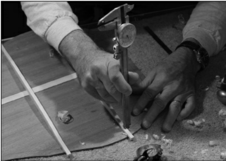
FIGURE 1.2.22. All the brace ends are carved down to 1/8'' , where they will tie into the kerf.
