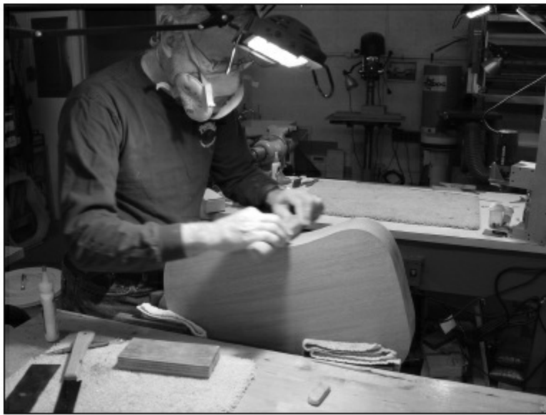
FIGURE 1.3.60. For the waist, we use a thick dowel (about 1 1/4") with self-stick sandpaper attached. Note that in each of the photos, a dust mask is used during the sanding process. Sanding creates a lot of very fine dust, and you need to protect your lungs. We also have an overhead dust collector on the ceiling to help reduce the airborne dust. Also note that we continue to use the same bench clamping fixture to hold the body that we used when cutting the end graft. As long as the body is put in from the top, it can't fall through (and never put the guitar in from the bottom).
