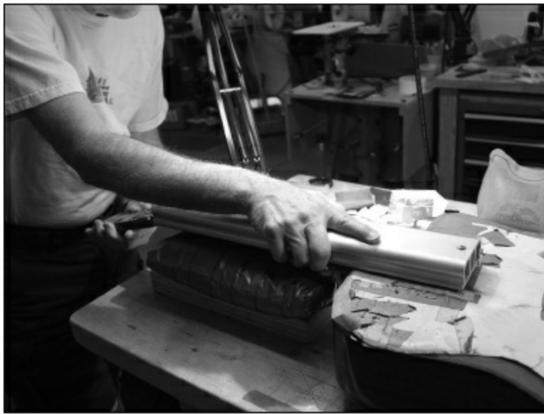
FIGURE 1.7.32. First, we chalk the fingerboard, and then we use a radiused fingerboard sander to get the fingerboard completely level from the nut to the twenty-first fret. We have always liked to level the board on the guitar. It helps eliminate the “hump” that is so common on many acoustic steel string guitars at the fourteenth fret.
