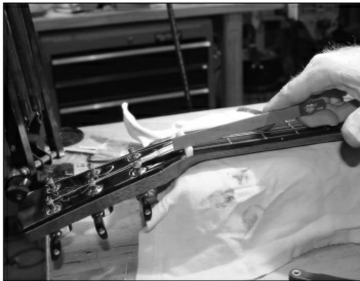
FIGURE 1.7.97. Now that the saddle is shaped and is at the proper height, we focus on the nut. First, hold the nut file so that you can easily file the same angle every time. If you hold your hand at a random height above the strings, you cannot be sure. We like to put the file over a finger as shown. Then that finger will be moved along the top of the strings to keep the file at a constant angle. This also just happens to be the angle about halfway between the fingerboard and the headstock. This means that the string will rest solidly along the entire length of the nut file slot, which is what you want.
