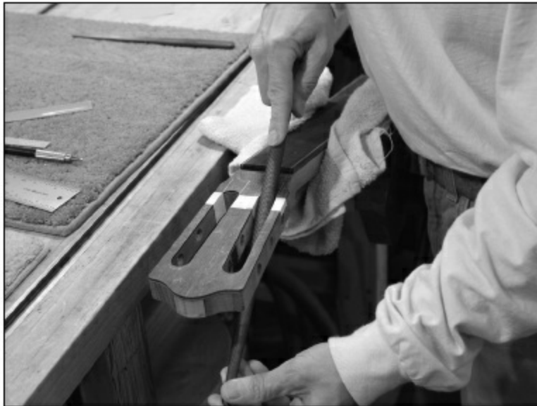
FIGURE 3.2.16. Now we have to file the slanted edges onto the slots. The slots are \frac{5}{8} " wide, and we are using a \frac{1}{2} " file. Note the tape on the inside edges of the slots. It is obviously there to protect the slots from file marks. However, you must be careful because it is still easy to scratch the wood through the tape.
