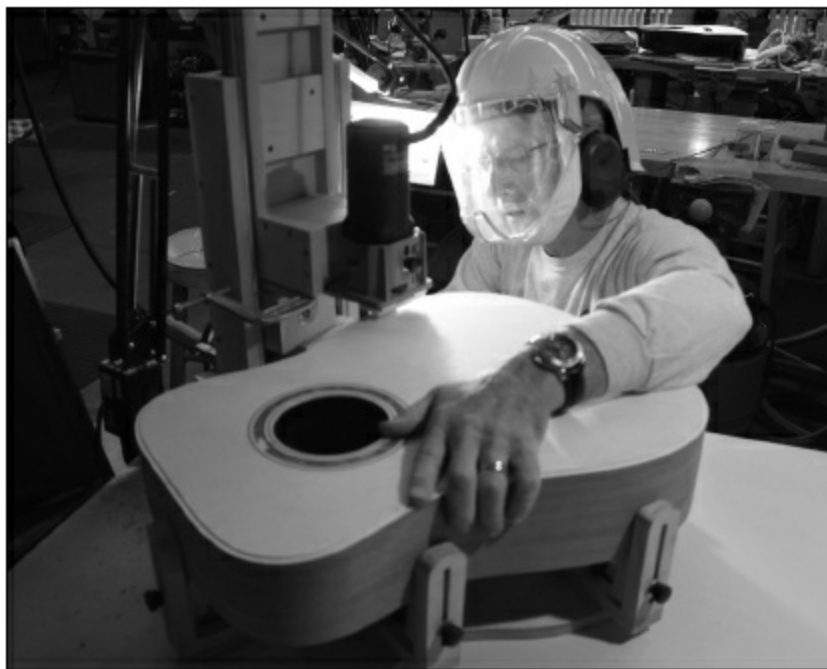
FIGURE 1.3.67. In this photo, the purfling cut has already been made, and we are making the binding cut. With this jig, we only have to change the bearing size and depth of cut to change between the different cuts, since the router (or laminate trimmer) is always held vertically.
