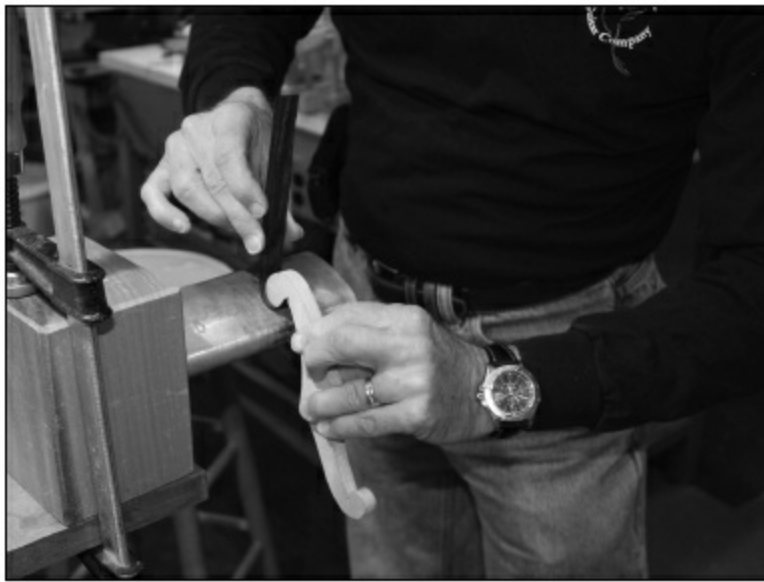
FIGURE 2.1.36. We use the same method for the initial bend on the Indian rosewood as we did above with the maple; however, we put this veneer into a homemade plywood caul the same shape but very slightly smaller than the actual F-hole. This caul will hold the veneer as it is shaped and cooled. You can see from this photo and the next that the curved end of the veneer fits into a small slot in the caul so it doesn't need anything special to hold it in place.
