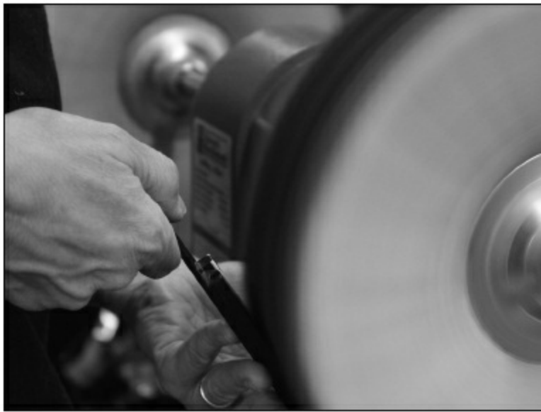
FIGURE 3.3.19. Once this level of fine sanding is done, we buff the bridge. We will not be putting a finish on the bridge, but sanding and buffing it will almost make it look finished.
