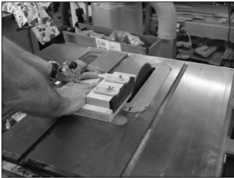
FIGURE 1.5.7. Last, we put the blank with the smooth side against the jig, reverse the side of the saw that we will use, and make the final cut for the blank thickness. We made the small clamps we are using by cutting and drilling pieces of 1/4" thick, 1" wide aluminum stock. A couple of small springs around the screws hold the clamps up when not in use.
