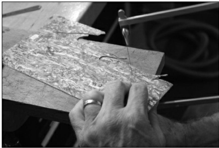
FIGURE 1.1.10. After drawing both the inside radius of 2 \frac{3}{8} " and the outside radius of 2 \frac{5}{8} " onto a piece of abalam (it's difficult to see the pencil lines in the photo), we will cut out multiple pieces to form the abalam arc. We will cut well outside the lines to allow for any error.
