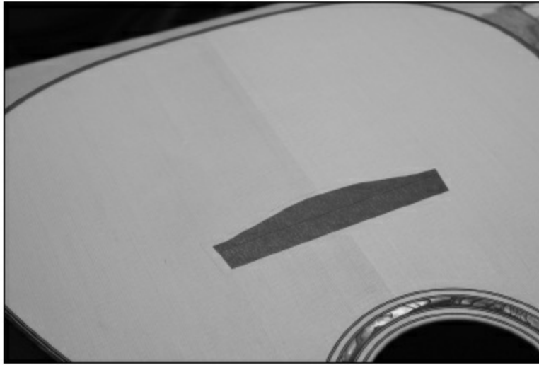
FIGURE 1.6.25. It is very difficult to see the pencil line that outlines the bridge location, but the tape is put right in the center (or as close as we can get—exactness is not critical here). Now, be sure to erase the pencil line, using a very soft eraser.
