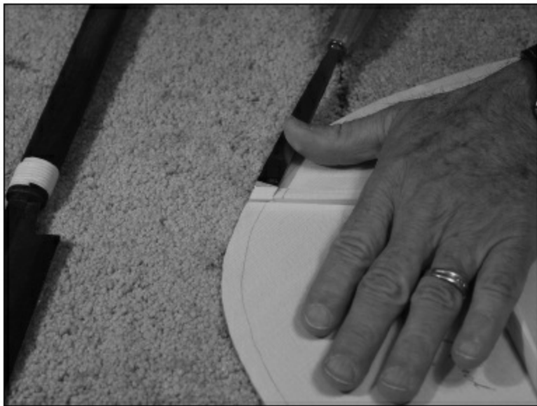
FIGURE 1.3.29. Next, we use a chisel to remove the excess length of the brace. It must be cleaned right down to the top wood.
