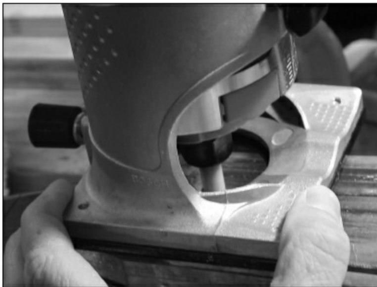
FIGURE 3.2.14. Using a small laminate trimmer with a 3/8" bit with a flush-trim bearing, we are able to follow the inside edges of the template and cut the slots for the tuning machines.
