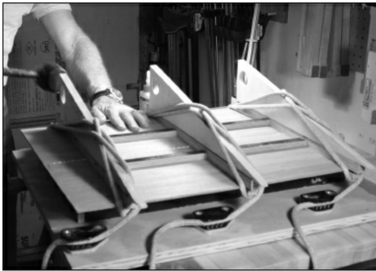
FIGURE 1.2.8. Wedges are slid between the ropes and the bracket and are lightly hammered in place with a rubber mallet. Now we wait until the glue is dry.
