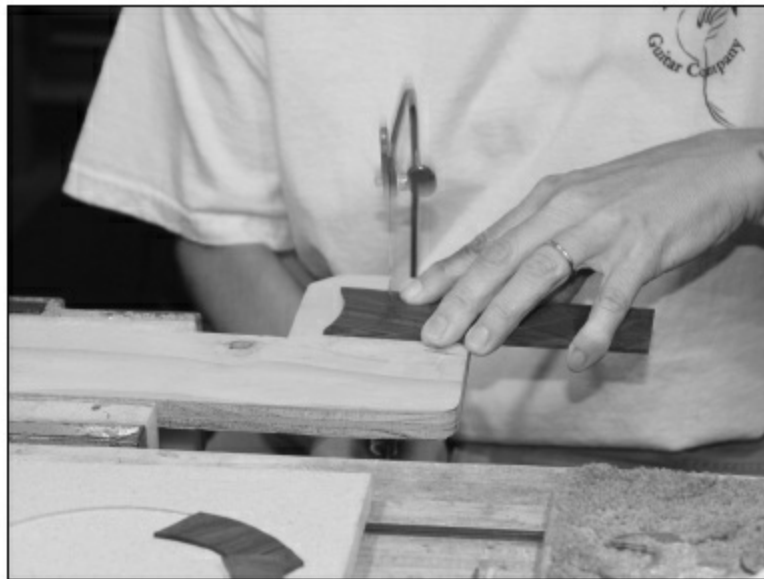
FIGURE 3.1.5. The Macassar ebony pieces are cut out slightly oversize using a jeweler's saw.
