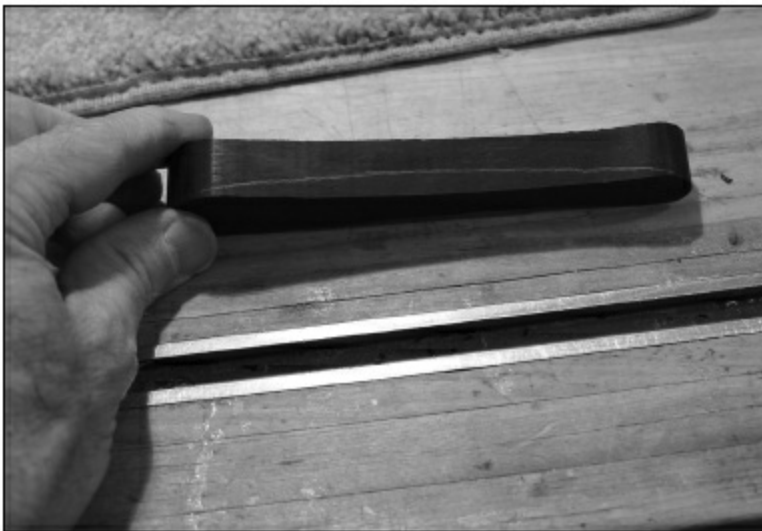
FIGURE 2.3.3. Here is a close-up of the shape we must carve into the base of the bridge. The bridge must be very snug against the top of the guitar.
