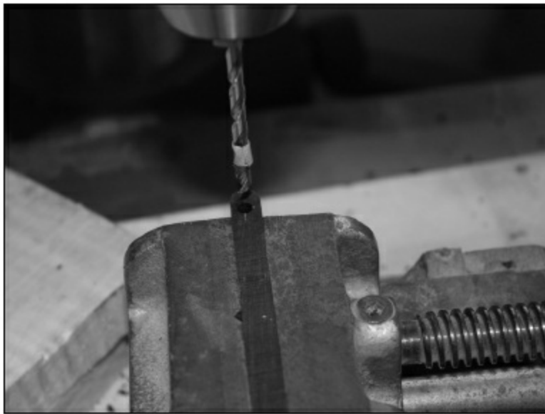
FIGURE 2.3.12. We now have to drill the holes in the underside of the bridge top. We will use a 5/32" brad point bit. These holes must line up exactly with the holes in the bridge base, so the bridge posts will fit right in. We put tape on the drill bit to mark the depth.
