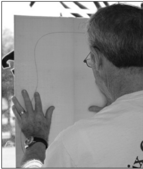
FIGURE 1.1.3 After the edges are jointed, they are “candled” or held up together to a window to check the edges for fit. Sometimes the edges have to be rejoined, but after candling, no light should shine between the halves of the top.
