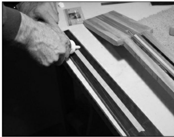
FIGURE 1.4.62. Now we will put a strip of 1/2" tape down the center of the underside of the fingerboard and apply Gorilla Glue to the portion of the board that will meet the neck. We are using a sample credit card blank for this purpose. We use Gorilla Glue for this step because we have found over the years that Titebond or other standard wood glues can inject water into the neck during gluing and often puts a slight warp into the neck. The Gorilla Glue has not caused this problem. We know several luthiers who use epoxy for this step, and there is no problem with epoxy. We just find it to be very messy, so the Gorilla Glue has been a good choice for us.
