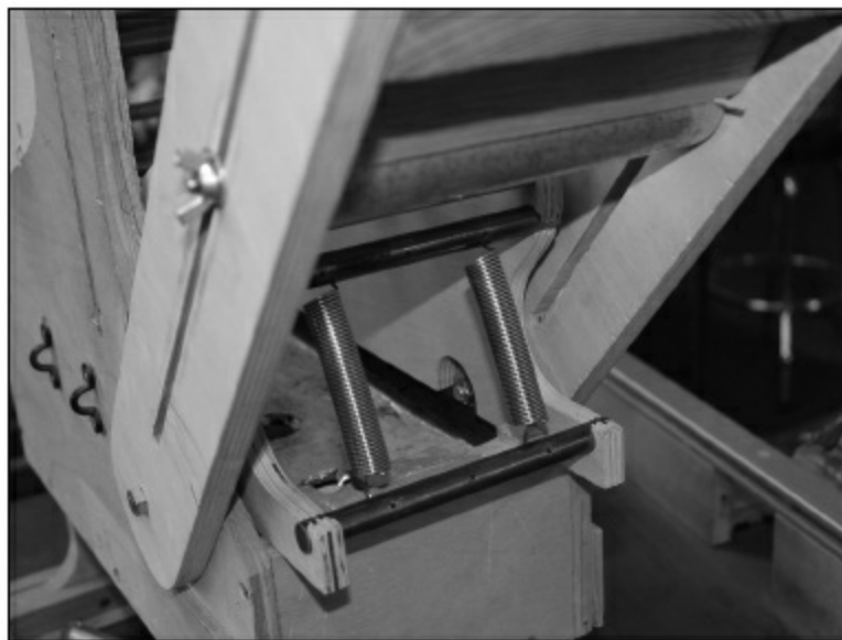
FIGURE 2.1.62. In this photo, we show the Fox bender with a cutaway attachment. However, by adding the springs between the last two posts, the area of the inward cutaway is given much more protection against splitting, since the board fibers are held together. This technique, along with gluing the veneer to the cutaway portion of the side, significantly prevents splitting, even with highly figured woods. Thanks to Michael Baranik for this idea.
