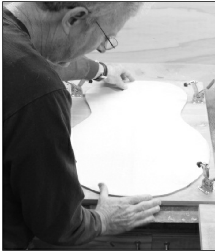
FIGURE 2.1.19. The top is being clamped into the jig. It must be aligned to marks on the jig. First the centerline must line up, and second, you must mark where the bridge will go on the top (for our scale length, it is approximately 11 1/4" from the mark at the heel to the bridge. Note that this is also where the inner points of the F-holes are).
