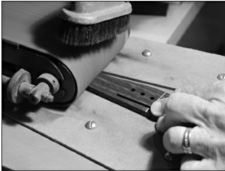
FIGURE 1.5.27. In order to cut the “wings” of the bridge, we use a small 4” belt sander purchased just for this step. We have put a platform on the base of the sander, which we use as a feeding table, and have screwed a couple of thin (1/8”) guides for the bridge. Now, we push the bridge into the belt sander to create the wing.
