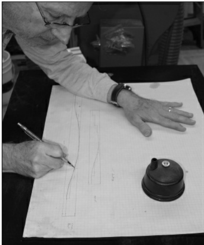
FIGURE 2.1.1. First, the desired arch for the top and back of the guitar must be designed. All dimensions must be accurate, and the curve of the arch should be smooth and graceful. As can be seen from the photo, the lower bout as well as the waist and upper bout must be planned. Leave nothing to surprise. We've been contacted many times by hobbyist first-time archtop builders who have bought expensive wood and started carving without a drawn plan, only to find that their dream guitar is a pile of scrap. The sketches shown in the photo show the arch across the lower bout and the waist; however, a sketch should also be made that shows the length of the guitar body and just how the builder wants the profile to look.
