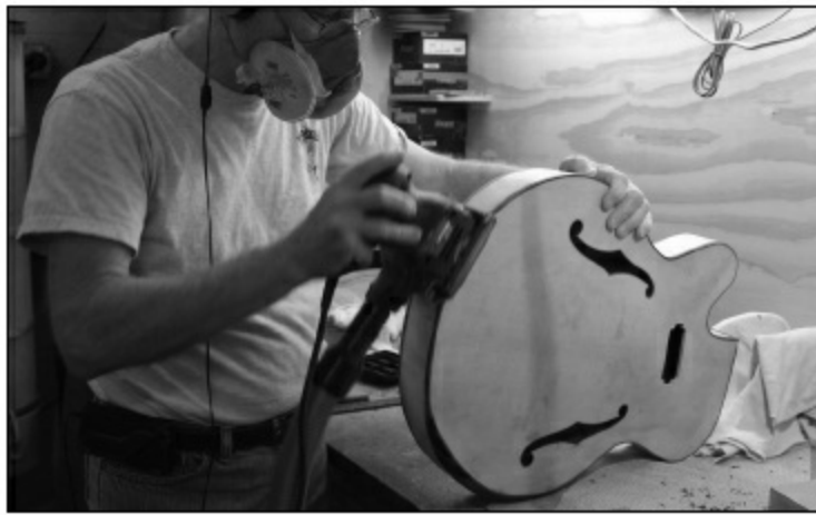
FIGURE 2.1.69. Here is the completed archtop body, after binding. We are not going into the binding steps here because they are identical to the binding of the steel string guitar. We use the same jig to hold the guitar and cut the binding slots and glue and strap the binding on in the same way. That's part of the purpose of this book—to show that most of the steps involved in building each of these very different types of guitars are very similar (or identical).
