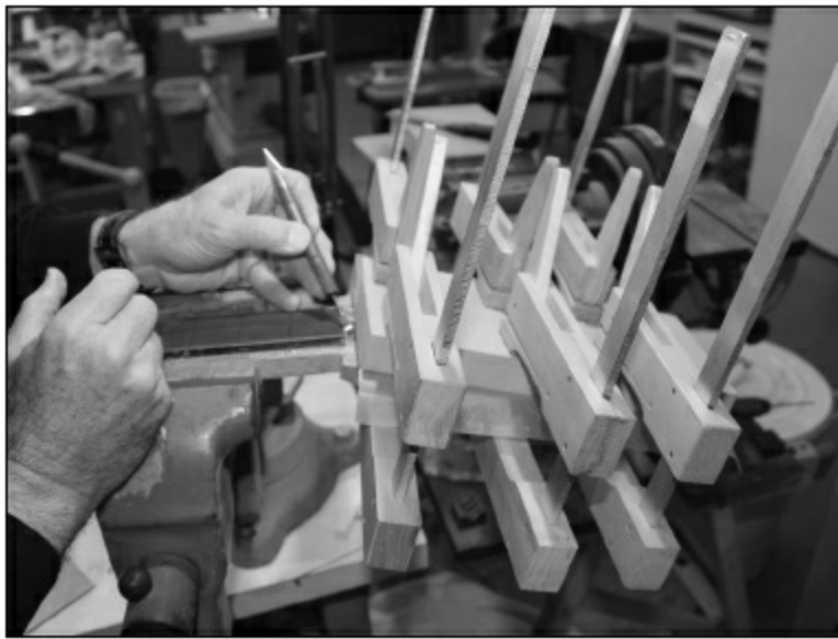
FIGURE 1.4.77. We use a 3/4" thick caul of MDF to evenly apply clamping pressure as we glue on the headstock laminate. We like to put the caul at the edge of the headstock laminate so any glue that squeezes out can be cleaned from the nut area.
