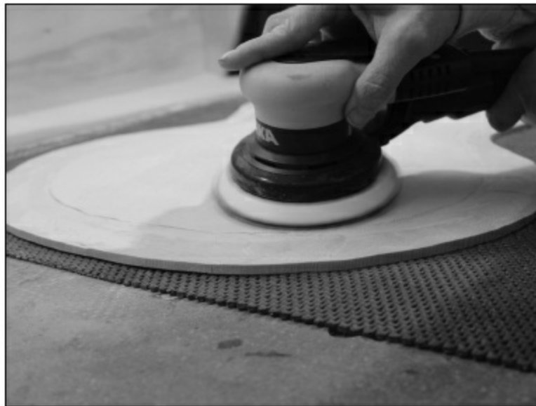
FIGURE 2.1.8. Since the angle grinder is very aggressive, we will switch over to a random orbital palm sander using about 60-grit paper to remove the remainder of the ridges after the grinder has gotten them very low. As the ridges continue to get smoother, we will switch to 100 grit, then move to 150. This is smooth enough for now, since final sanding will be done with 220, and we are not yet ready for that.
