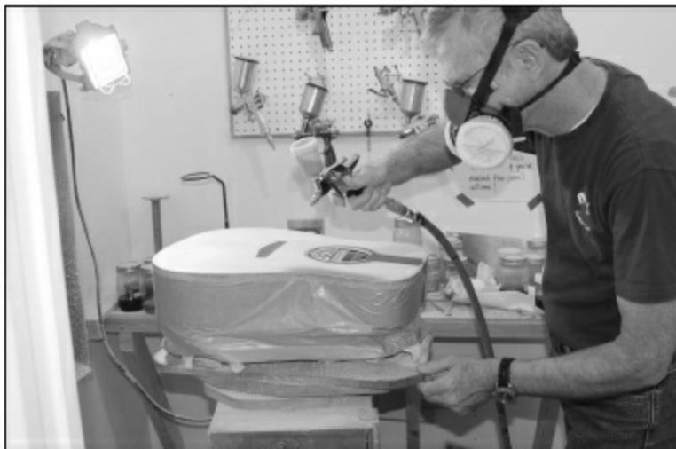
FIGURE 1.6.30. Next, we spray the sunburst along the edge of the guitar. We will typically have to spray at least two coats to be sure the color is dark enough and the band of color is wide enough. Also, it is imperative that you don't try to spray too dark a coat all at once. This could cause a drip to form, and this is a very difficult problem to fix, requiring sanding away all the color and starting over. Spray light and use multiple coats to get the best results.
