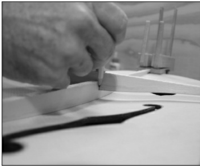
FIGURE 2.1.48. After the lower brace notch is done and at the right height, place the upper brace into the notch and mark on the side of the brace where it intersects with the lower brace.
