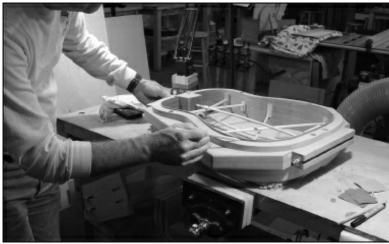
FIGURE 1.3.21. Once we've sanded to within about 1/8'' , we draw a line at the edge of the mold, which is at the height we want the sides to be.
