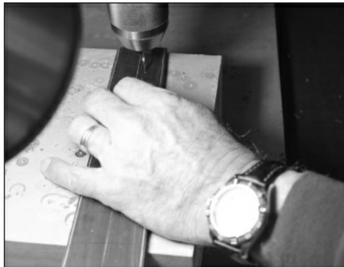
FIGURE 1.4.60. We are now ready to glue the fingerboard to the neck. First, we draw a centerline on the fingerboard and mark where we will drill two holes. The holes are drilled \frac{1}{4} " away from the centerline, directly in the fret slots of the first and thirteenth fret for the steel string and the archtop. In the case of the classical, the holes will be drilled at the first fret and the eleventh fret. The holes are \frac{1}{16} " in diameter.
