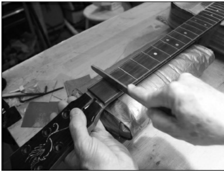
FIGURE 1.7.62. Here is the first fret being crowned with a diamond crowning file. It is critical that you check the fret many times with the light in different angles to verify that you have just barely filed up to and including the flat spot created by leveling. Don't file the fret too low in this step or you'll have to relevel it.
