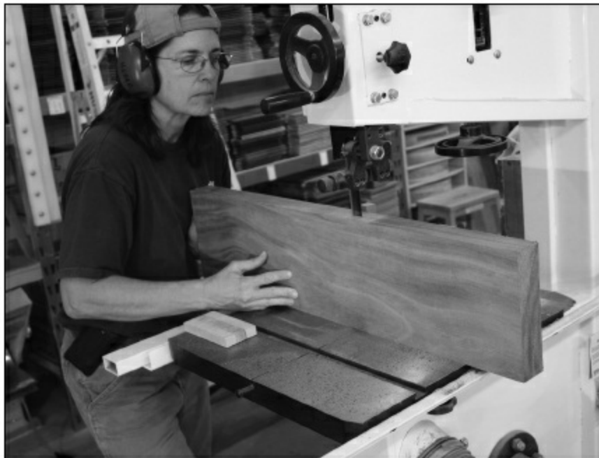
FIGURE 1.4.1. With our guitars, the steel string neck starts out very much like our archtop or classical necks. The main difference between any of the necks is the scale length and the neck width. Almost all our necks are a five-piece sandwich. The neck is three pieces of mahogany separated by veneers of walnut. If the mahogany slabs we have in stock are slightly too thin for the proper neck width at its widest point (the fourteenth fret for a steel string or archtop and the twelfth fret for a classical), then we have a choice: either get wider pieces of mahogany or resaw off wider slabs of walnut to make the proper width neck instead of using veneers of walnut. We like the neck at its widest to be at least 1/16'' oversize, just to be safe. In this photo, you can see a nice board of African mahogany being resawn, which will be the two outer sides and will make four necks. Also note that the grain is in the vertical or quartersawn direction.
