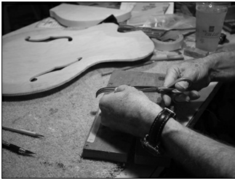
FIGURE 2.1.26. Scissors can be used to cut the fiber layer, but don't try this on the wood layers or they will split.
