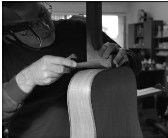
FIGURE 1.4.58. In our case, the side-to-side alignment was right on the money, but the neck angle was very slightly high. So to bring the angle down, we are pulling a strip of sandpaper along the thin shelves we created on each side of the dovetail, where the neck will rest on the sides of the guitar. To bring the angle down, we put the sandpaper between the neck and the side (with the sandpaper side up against the neck), push the neck down against the side, and pull the sandpaper up, toward the top of the guitar. To keep the side-to-side alignment true, we will do the same number of pulls on each side, checking our alignment every twenty or so pulls.
