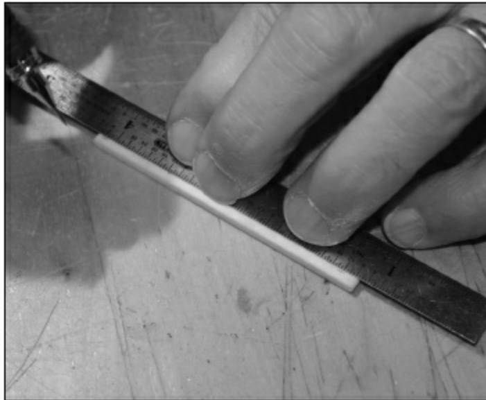
FIGURE 1.7.93. Since we need to take the action down by 3/64'' at the twelfth fret, we need to take the saddle down by double that amount or 6/64'' ( 3/32'' ). We mark this on the saddle and draw the line where we need to sand.
