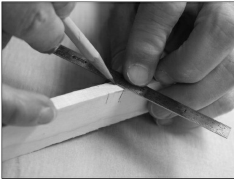
FIGURE 2.1.50. Now, transfer the points from each side of the brace and cut the notch as before. Since this is the upper brace, it will be much thinner over the notch than the lower brace; therefore, you will have a much deeper cut than before.
