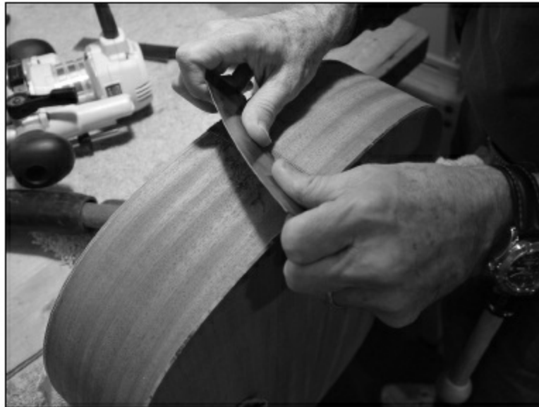
FIGURE 1.3.57. After trimming the ends of the graft, we use a cabinet scraper to level the graft with the sides.
