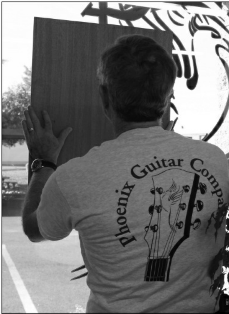
FIGURE 1.2.4. After jointing, the edges are held together and are candled, just as we did with the top.
