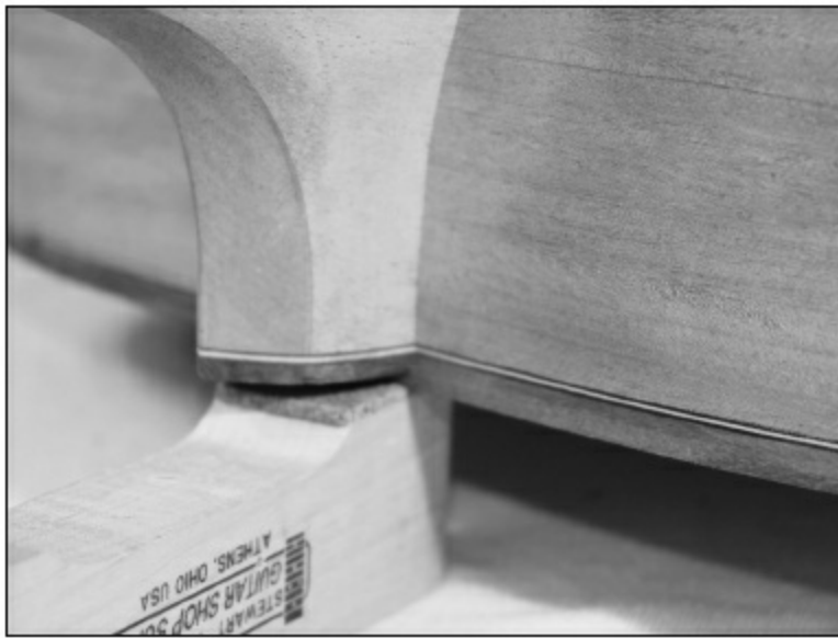
FIGURE 1.4.136. In this photo, the neck is perfectly fit into the dovetail joint. The neck overhang is touching the guitar top, and you can see that our heel cap purfling is lining up nicely with the purfling around the body.
