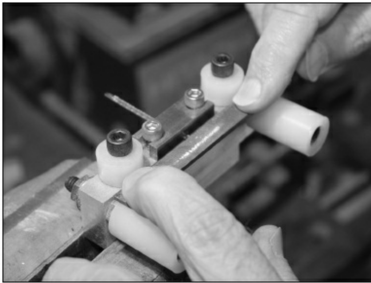
FIGURE 1.7.46. Here's the tool in action. Using a fine file, rolling it on the plastic rollers, and filing the fret tang residue flush with the underside of the fret bead.
