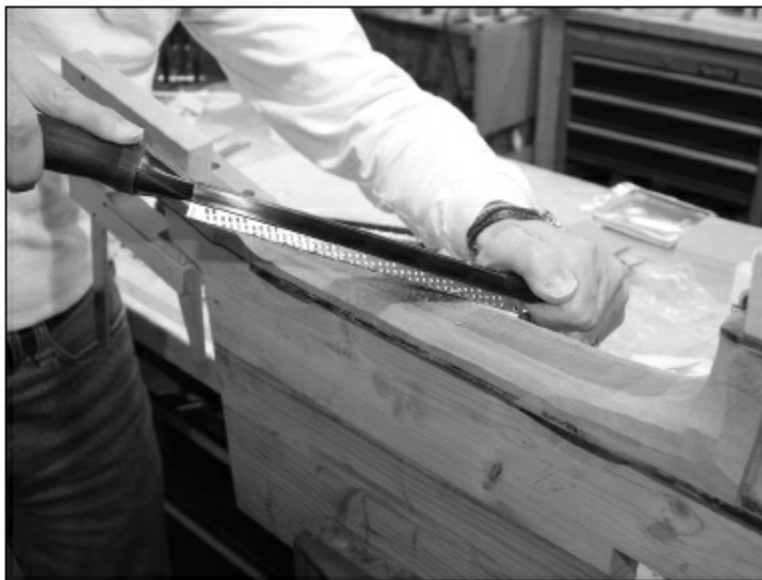
FIGURE 1.4.120. Next, we carve with a microplane. This tool works well because it does more cutting than grinding.
