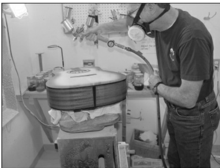
FIGURE 1.6.34. The top of the guitar is being sprayed. Note the reflective light in the upper left being used to be sure the spray is even all the way across. Also note that the first two coats right after the color has been applied are light, dry coats. If you spray too heavily right away, the color can bleed into the upper layers and look very bad. The coats sprayed on the sides must be lighter than those sprayed on the top to avoid dripping. It's OK because we will spray twice as many coats on the sides as we will on the top or the back.
