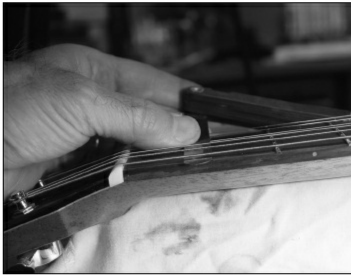
FIGURE 1.7.98. After filing the slot for the low E string, you can see that we're leaving the string a little high above the .010 feeler gauge—just a little. You definitely would rather be just a little high than a little low in this case.
