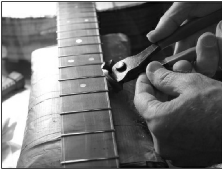
FIGURE 1.7.52. After all the frets are in, the next step is to use a fret nipper and cut off the fret ends. Don't push too hard on the fingerboard or the bindings or you'll leave marks that will be very difficult to sand out.
