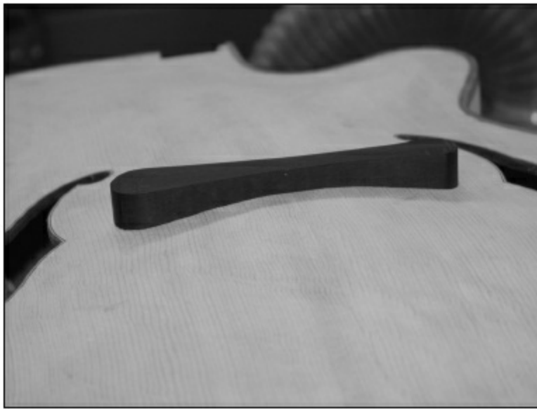
FIGURE 2.3.4. After using a band saw to cut just below the line, we can see that the bridge has a pretty close fit to the guitar top, but we have to make it fit exactly.
