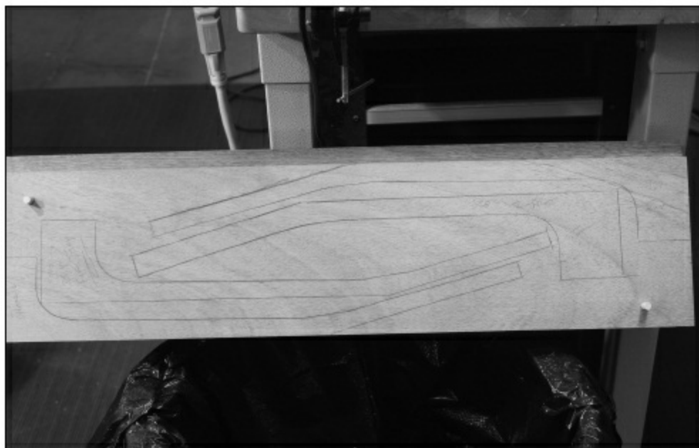
FIGURE 1.4.2. Here is the sandwich, ready for gluing. Note the two dowels in the corners for alignment. These will keep the boards from slipping during the clamping process.
