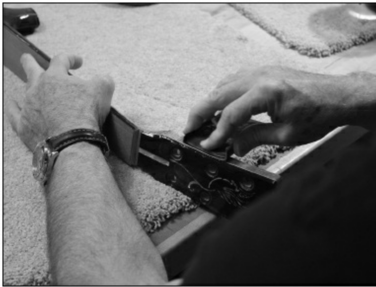
FIGURE 1.6.20. To sand the flat surfaces of the neck and headstock, we use a small, hard rubber sanding pad available at local auto paint stores.
