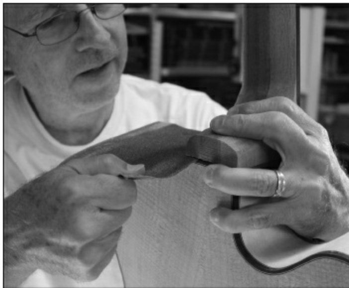
FIGURE 2.2.20. If the fit is close, and you can use sandpaper to make slight moves to the angles up/down or left/right. If you have a bad fit, you may need to use a chisel on the shoulders to make the angle right. Notice we have not yet put on the heel cap. The neck fit must be good before we do our heel cap, due to the critical nature of the measurements involved.
