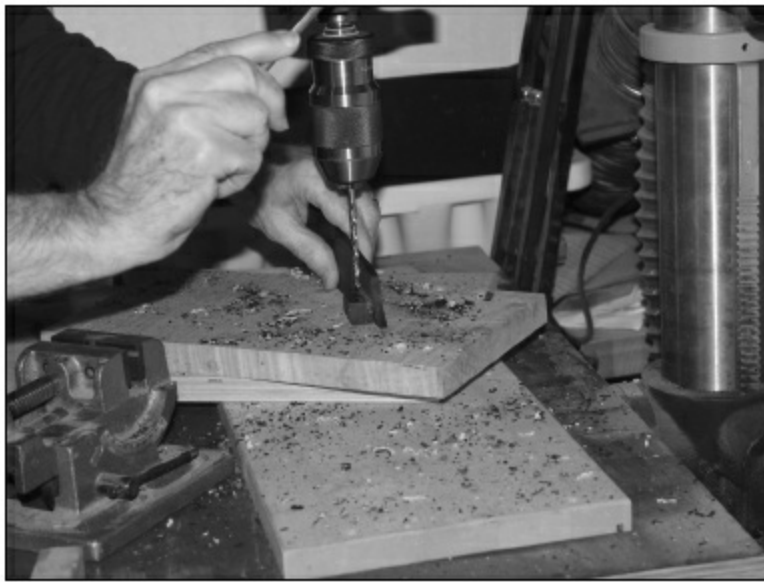
FIGURE 2.3.34. For the screws we are using, we drill through the block using a 3/16'' bit. Be sure the newly sanded edge is flat against the base so the rest of the pickguard is leaning at a 3-degree angle.
