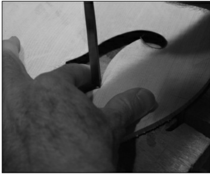
FIGURE 2.1.30. Once the binding is flush with the top and back, miter the corners and end of the loops with a sharp chisel.
