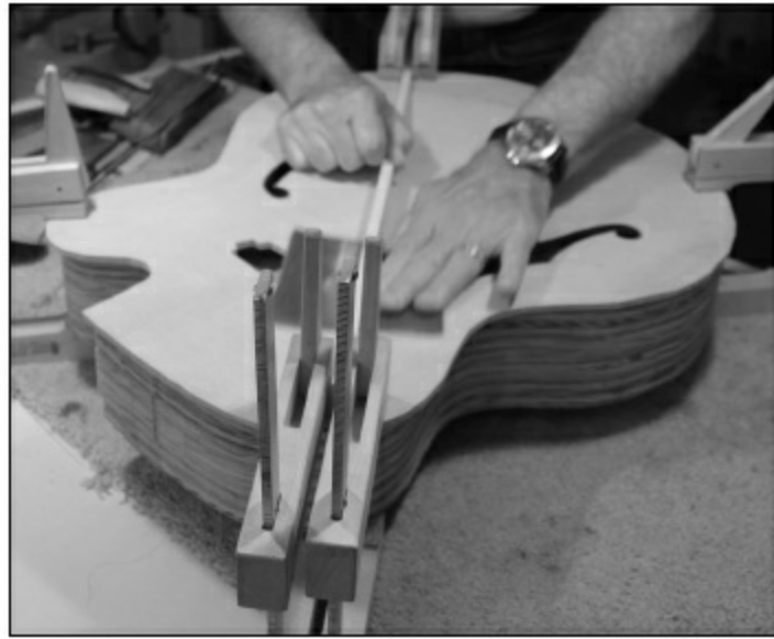
FIGURE 2.1.43. Now, we put two cam clamps on each end of the brace we want to work, so the brace aligns perfectly with the alignment marks we put onto the top. The remaining clamps are there for stability. Next, we take a piece of 80- to 100-grit sandpaper and put it under the rough brace with the sandpaper side up against the brace. We sand it until the face of the brace perfectly matches the surface of the arch. These two surfaces must match because they are about to be glued together, and we don't want any gaps between the surface of the brace and the surface of the top. It's a good idea to use a glove on the hand holding the sandpaper.
