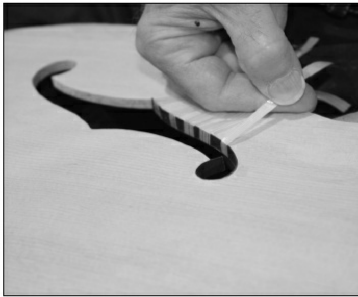
FIGURE 2.1.28. Once the binding has been put in place (with one side tightly against the corner of the F-hole, we use the tape to hold it in place. Note the overlap around the F-hole loop. We will cut this down to miter the joint later. When removing the tape, we never just pull it off—we use a small amount of naphtha, squirted from a pipette. This will allow the tape to pull off easily without tearing any of the soft wood fibers. It’s best not to get any of the naphtha on your skin, so either use gloves or hold the tape with tweezers or small pliers to pull it up.
