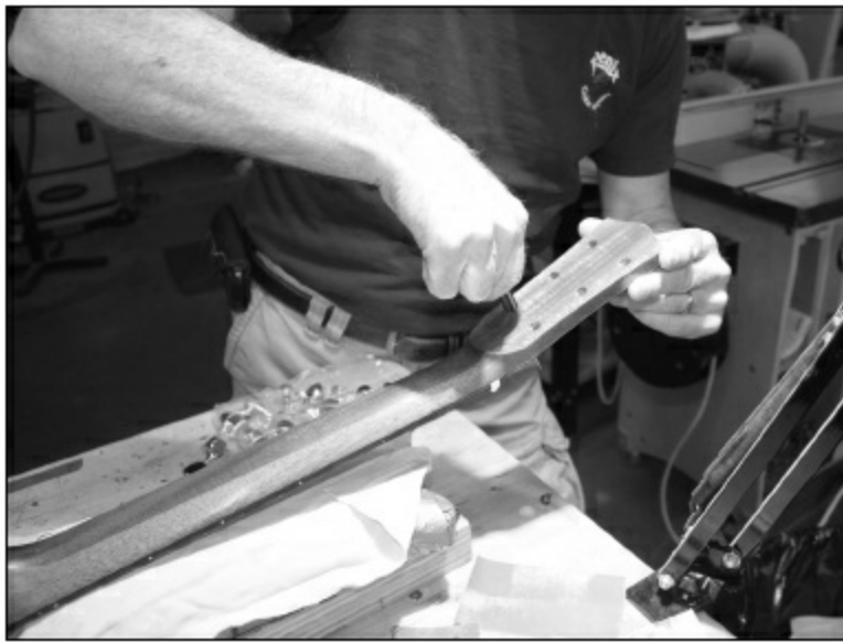
FIGURE 1.7.84. Now we put in the tuning machines. We need to use a reamer to fit the machines into the holes we originally drilled. Be careful here because it only takes a few gentle turns with the reamer to make the fit too loose. You want a slightly snug fit—but not a tight one. You can easily split the headstock if you push the tuning machines in too hard.
