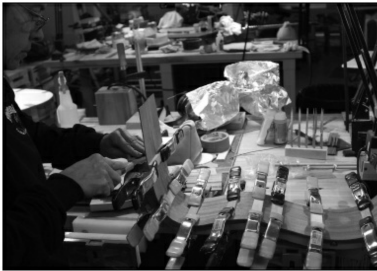
FIGURE 1.3.11. Here is one side, clamped into the mold. In this photo, the overlap at the neck joint is being trimmed flush to the mold using a flush-trim saw. We will also trim the overlap at the other end, in preparation for putting the mold together.
