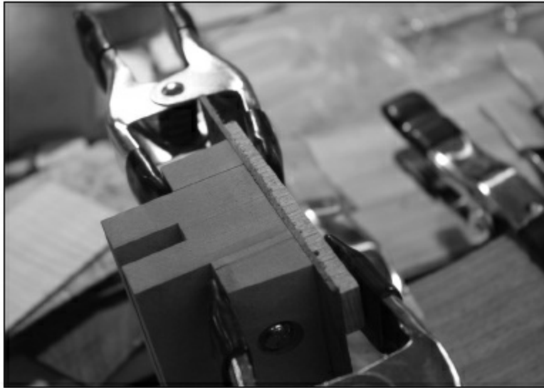
FIGURE 1.3.12. This is a close-up of the freshly cut joint. Now it is time to put the two halves of the mold (and sides) together.
