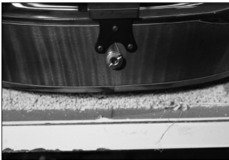
FIGURE 2.3.40. Here is the connection to the tailpiece on the finished guitar. This will effectively ground the strings.
