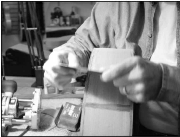
FIGURE 1.3.97. After scraping, sanding, and leveling all the bindings and purflings, the body is ready for the dovetail to be cut.
