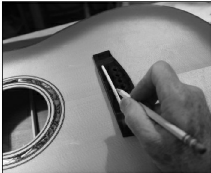
FIGURE 1.7.94. Once we have sanded the bottom of the saddle to the line on the disc sander, we put the saddle back into the saddle slot and mark between the strings (center the lines between the strings as closely as possible).
