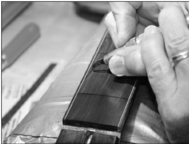
FIGURE 1.7.39. Here is another fret cleaning tool from Stew-Mac. This one does an excellent job of cleaning at the edges of the slots.
