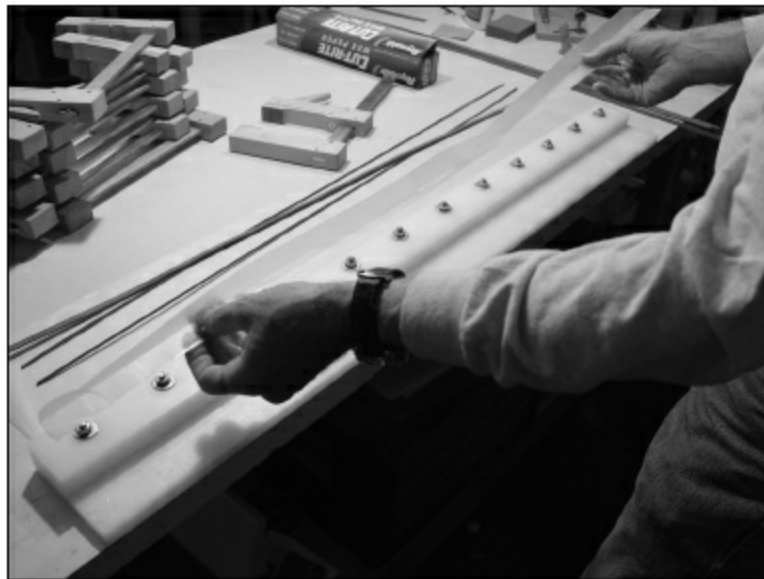
FIGURE 1.3.61. With the body sanded, it is time to prepare the bindings. We start with a jig we created that is made of ultra-high-density polyethylene. It simply creates a shelf to clamp the bindings against. Though this material is used to eliminate as much glue sticking to it as possible, unfortunately, it still does stick, so we have cut a piece of wax paper about 36" long and 1" wide and fold it lengthwise to fit against the wall of the jig.
