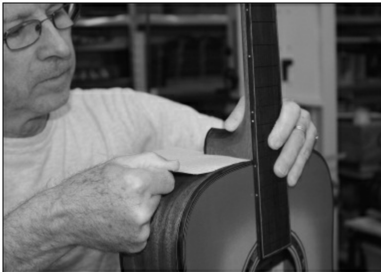
FIGURE 1.7.3. Even if the neck alignment is perfect, you will likely have to make a few pulls with
