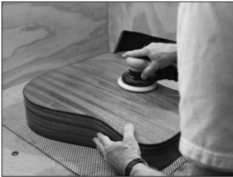
FIGURE 1.6.16. We use the same sander as before, and the Abranet shown above attaches to the sander with hook-and-loop.
