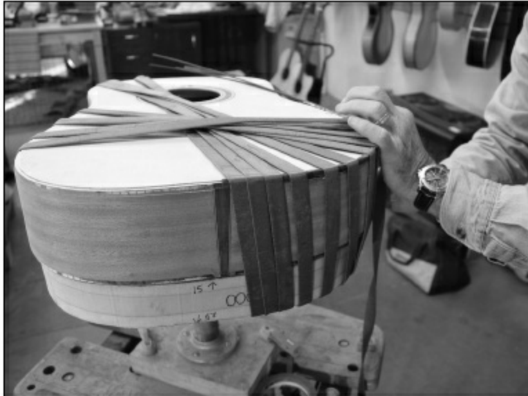
FIGURE 1.3.83. We will typically glue for a few inches, then bind the glued area with the flat nylon rope and repeat the process, gluing a few inches and then binding.
