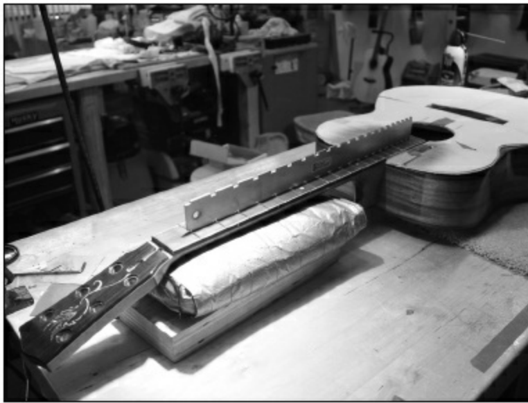
FIGURE 1.7.58. Before we go on, we must make sure the fingerboard is straight. For this, we use another Stew-Mac tool that fits over the frets and shows whether the board is straight. We will adjust the truss rod until the neck is straight. After a fret job, the fret tangs are likely to force the neck into a slight back bow.
