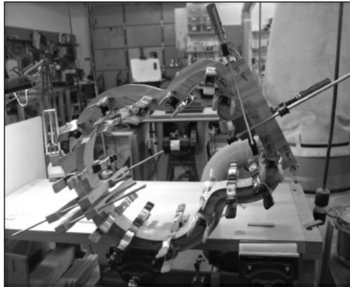
FIGURE 2.1.64. After the edges are trimmed, as we did in Figs. 1.3.11 and 1.3.12 for the steel string, we make the endblock and headblock and clamp them as shown.
