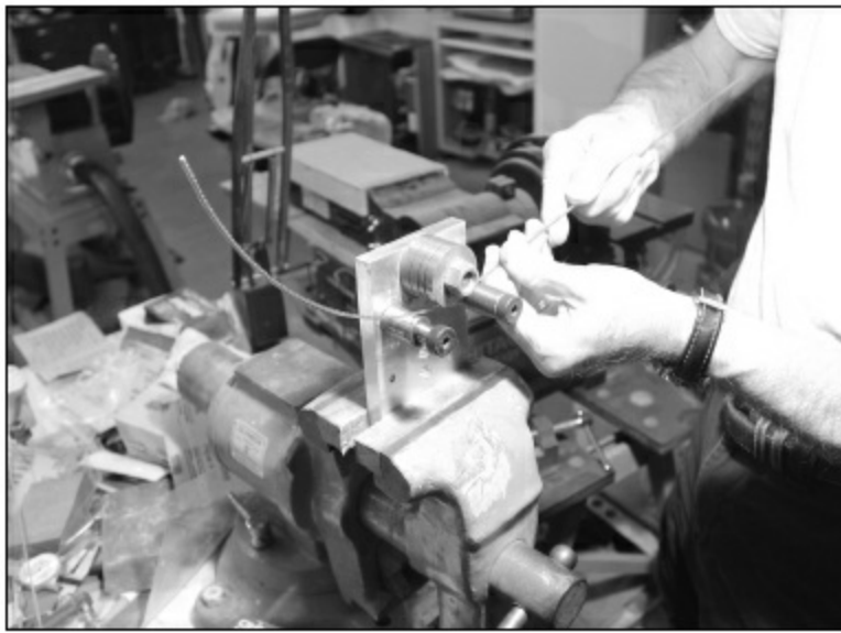
FIGURE 1.7.36. Now that the fingerboard is level, we bend our fretwire in our homemade bending machine. There is nothing very scientific about this job. We simply want the wire to be bent to a smaller radius than the fingerboard. Our fingerboard radius is 16", and our bender will bend the fretwire to about a 12" radius.
