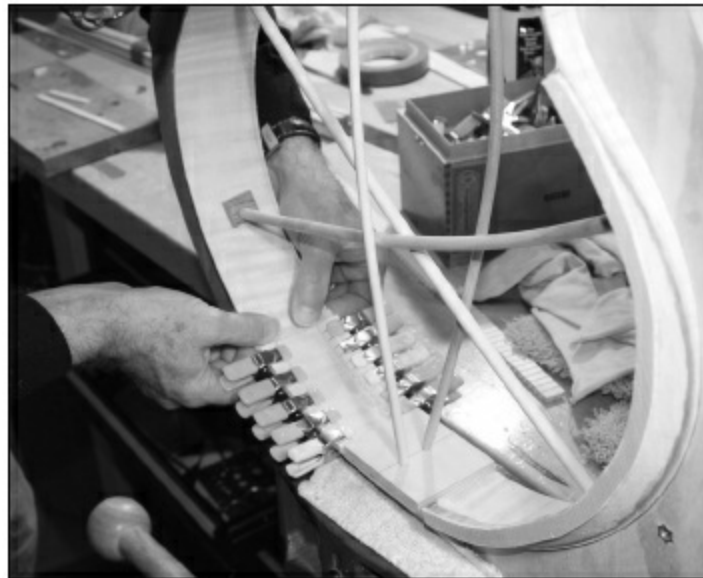
FIGURE 2.1.66. Here, the two lengths of kerf have been glued and clamped in, and we have cut a short piece of spruce (what we call a Popsicle stick) and get ready to glue it in perpendicular to the kerf. We always cut two identical pieces of kerf so we can glue the Popsicle sticks evenly around the side. The purpose of the Popsicle sticks is to stop a split in case the player hits his guitar, and the side starts to crack.
