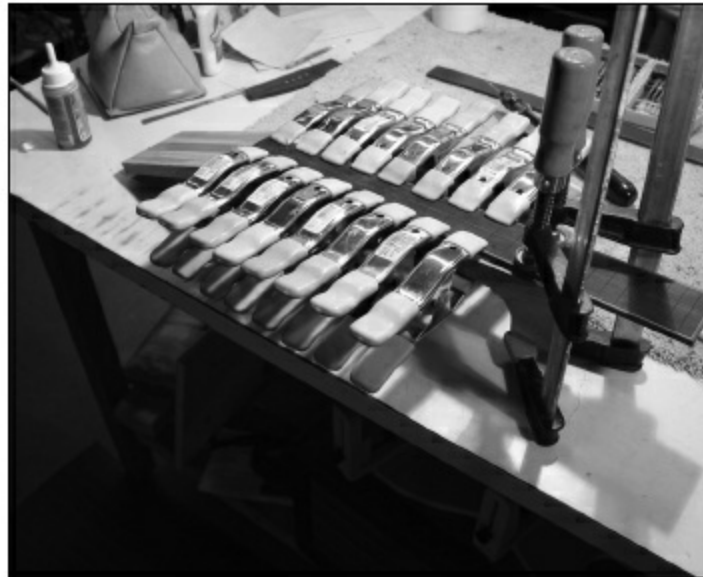
FIGURE 1.4.64. Once the fingerboard is put down against the neck, brads are put into the holes to ensure proper alignment. Next, we put several spring clamps on the fingerboard and two screw-down clamps to hold the fingerboard against the neck heel. The Gorilla Glue will expand to glue the wood over the truss rod to the fingerboard, but if we had left the center section of the fingerboard fully glued, the Gorilla Glue could seep down and impact the action of the truss rod. Using this technique, we have not had this problem. Right after gluing, we remove one clamp at a time and clean the glue squeeze-out.
