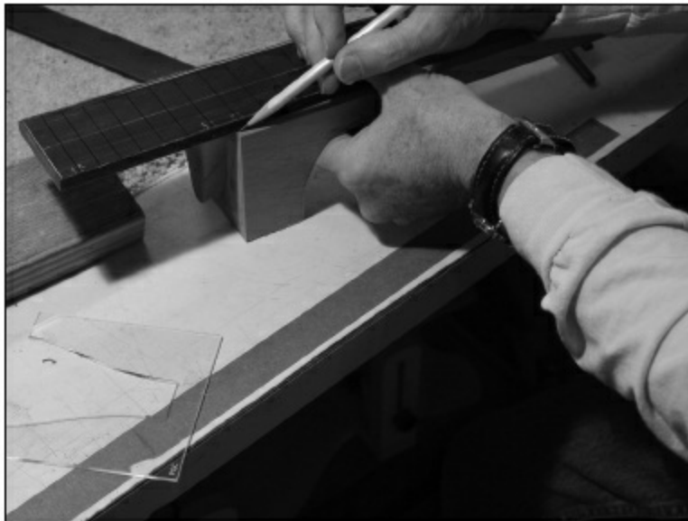
FIGURE 1.4.48. We are marking the position of the fingerboard on the neck. Each fingerboard edge is measured and marked to be equidistant from the edges of the neck.
