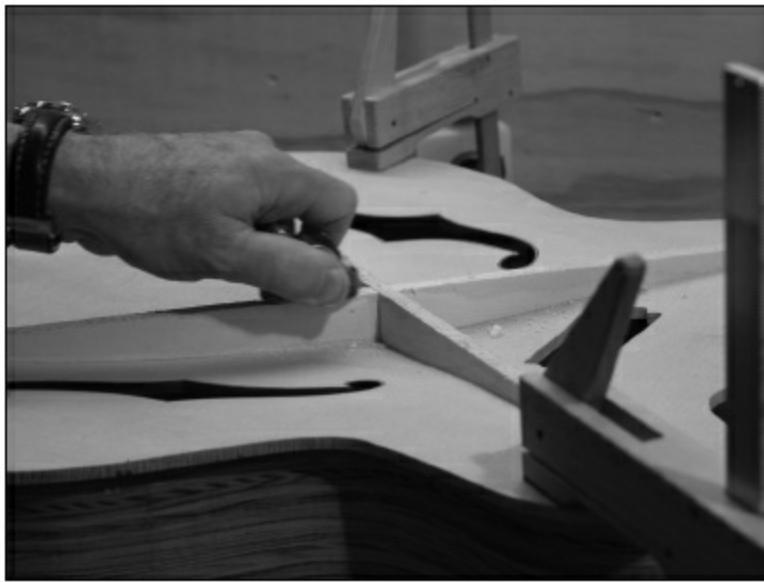
FIGURE 2.1.57. The braces are carved with a small, curved-sole plane. Sometimes the spruce of the brace wants to chip and tear out as you carve. When this happens, turn the work around and go in the other direction. This will usually solve the problem.
