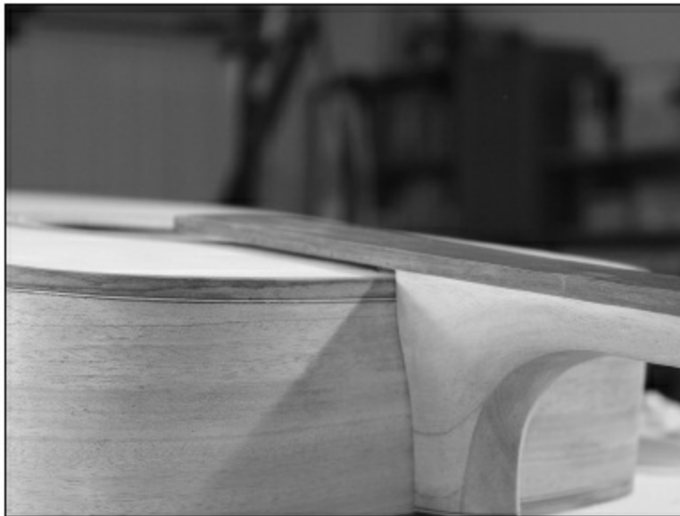
FIGURE 1.4.132. Here is the first fit of the neck after the shims are glued on. It is sitting too high, and we need to start shaving down the shims to make it fit.
