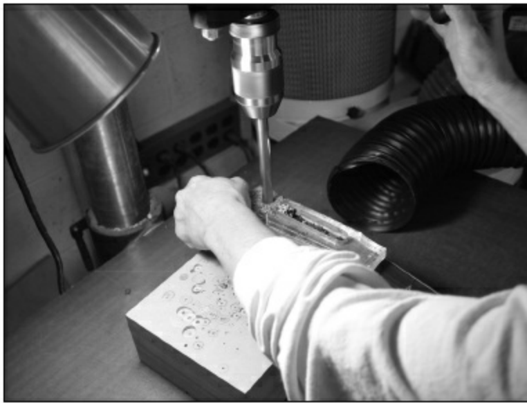
FIGURE 3.2.13. We have put a new template onto the headstock that is the same size as the one we used to cut it originally to shape. This template is put down with double-sided tape. In the figure, multiple holes are being drilled into what will become the headstock slots to make routing the slots easier.
