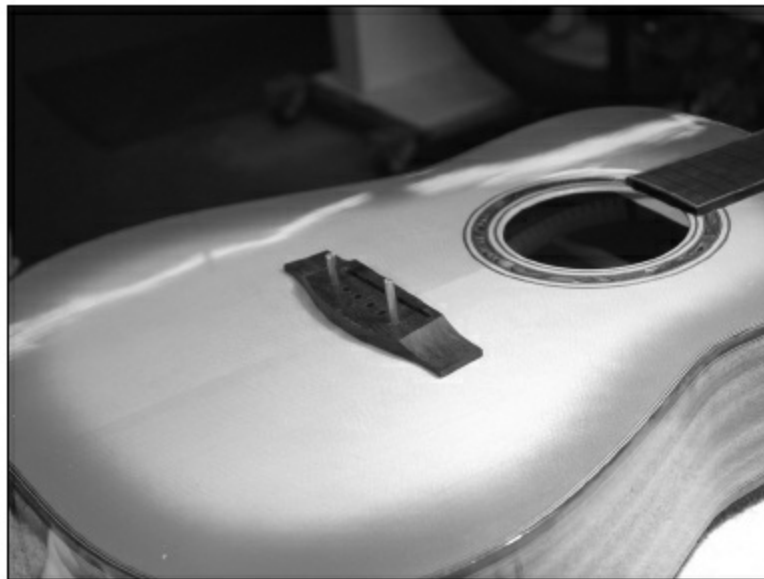
FIGURE 1.7.17. Once the holes are drilled, we place two 3/16'' brass pins into the holes to hold the bridge in place very tightly while we perform the next step: scribing around the bridge.
