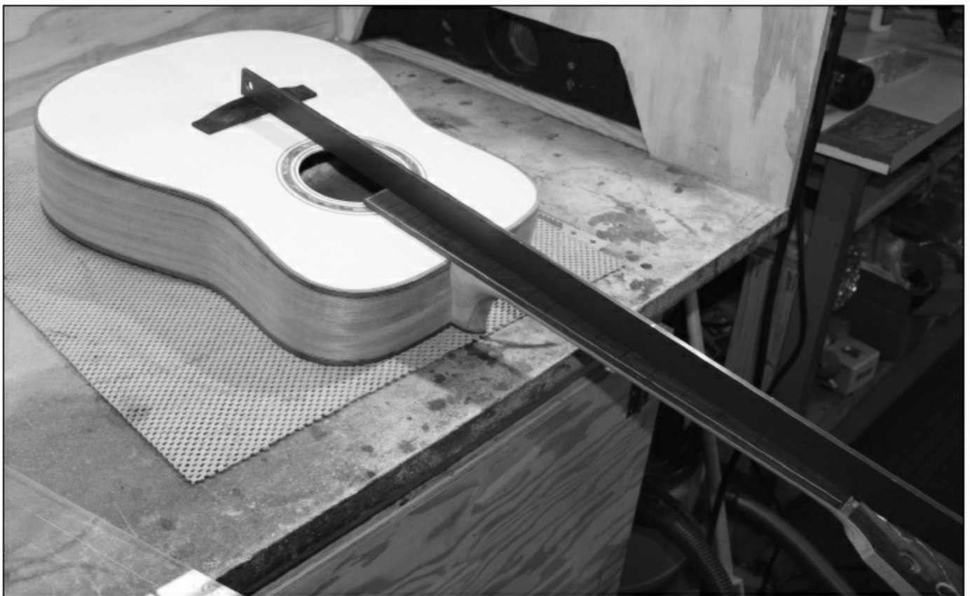
FIGURE 1.4.137. We do one final neck alignment check, both side-to-side and vertical. In this photo, we are measuring the vertical neck alignment using a test bridge and a straightedge. The neck aligns to a point about 1/32'' above the bridge—just about perfect.
