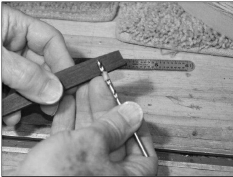
FIGURE 2.3.12. We now have to drill the holes in the underside of the bridge top. We will use a 5/32" brad point bit. These holes must line up exactly with the holes in the bridge base, so the bridge posts will fit right in. We put tape on the drill bit to mark the depth.
