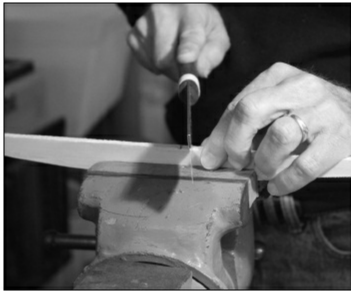
FIGURE 2.1.46. After the position of the X is marked on the lower brace, it is put into a vise, and we use a thin kerf saw to cut the edges.
