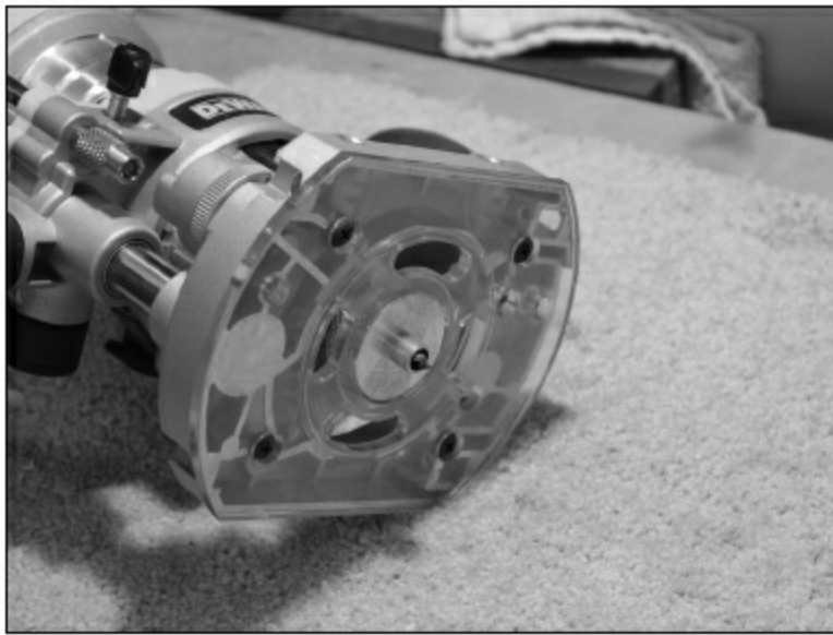
FIGURE 1.3.52. For the cut, we use a small plunge router with a collar screwed into the base. A 1/4" spiral bit makes the actual cut.
