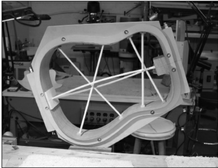
FIGURE 1.3.18. While the blocks were being glued, we removed the clamps we had holding the sides to the mold and replaced them with go-bars. We have used this method for years to hold the sides in place while we are gluing on the kerf in the next step. Note that we don't take off all the clamps before putting on the go-bars. We only do a couple at a time to keep the sides exactly in place.
