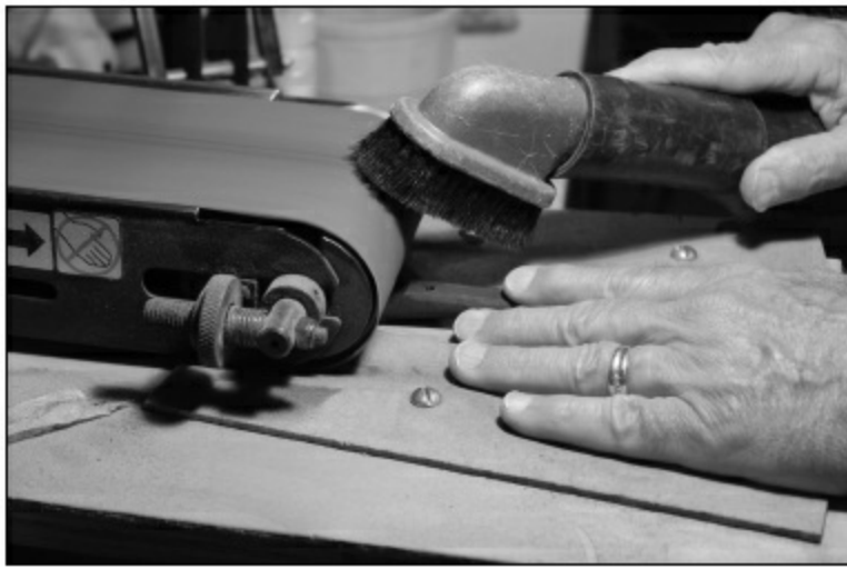
FIGURE 2.3.8. To shape the ends of the bridge, we use the same jig that we used to shape the wings of the steel string bridge. We simply let the radius of the belt sander wheel shape the wing of our archtop bridge. We'll have the new wing stop about \frac{3}{16} " outside the bridge postholes.
