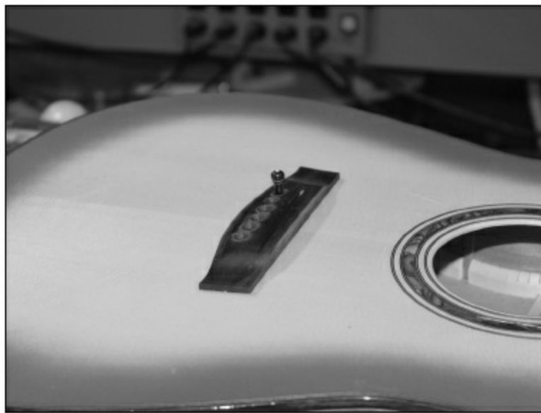
FIGURE 1.7.81. It's time to put in the bridge pins. However, they won't fit until we ream the proper taper into the existing holes.
