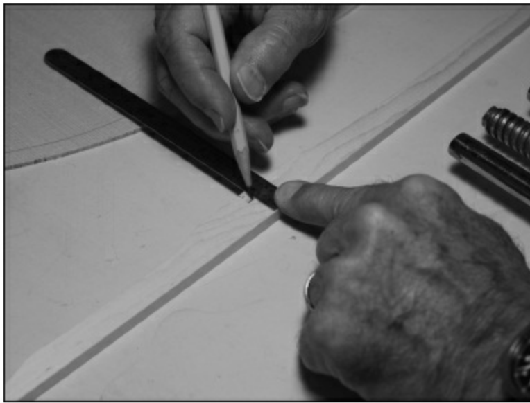
FIGURE 1.1.39. The final height at the intersection of the X brace will be \frac{5}{8} ". We will mark the brace at the \frac{5}{8} " point, and we will also mark it at about \frac{15}{32} ". This is the point where we notch the brace to keep the bottom brace about three-quarters of the total height and therefore as strong as possible at the X.
