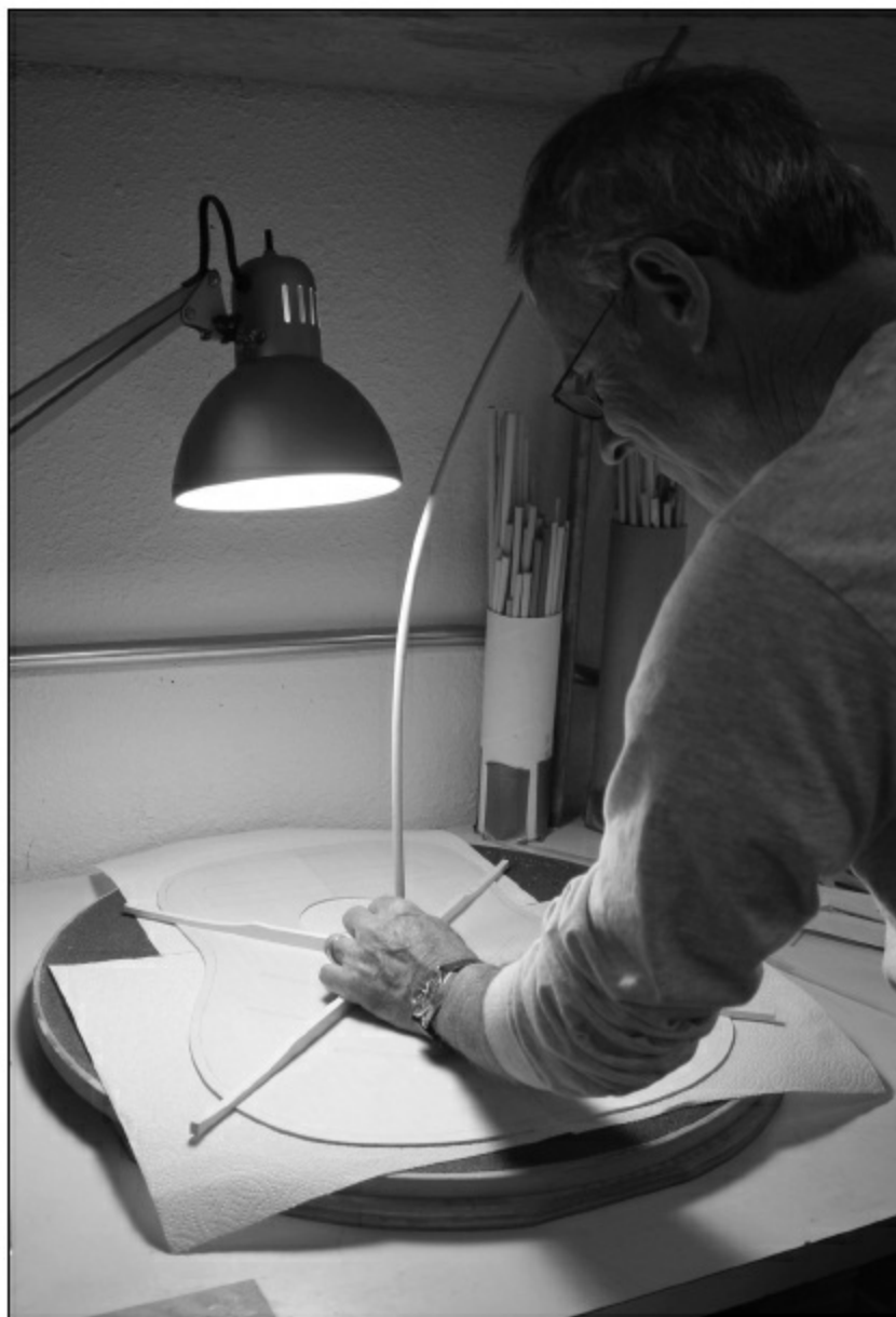
FIGURE 1.1.47. The first go-bar goes in the center of the X.
