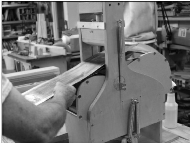
FIGURE 1.3.8. The sandwich consisting of the sides, paper, foil, steel, and heat blanket are inserted into a Fox bender. This bender was developed by Charles Fox and has become an industry standard, especially among small builders.
