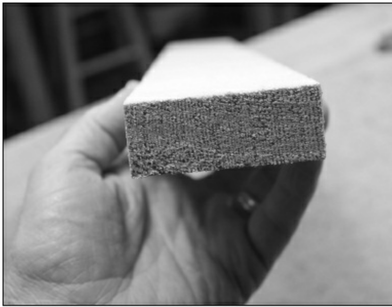
FIGURE 1.1.30. Now, we focus on the top braces. We start with a piece of very nicely quartersawn Engelmann spruce that matches the top wood.
