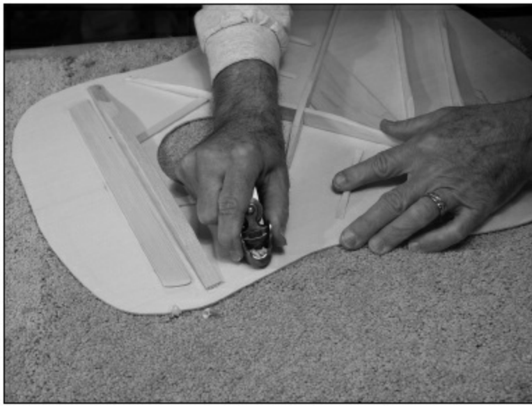
FIGURE 1.3.34. After fitting the top, any braces that are slightly over 1/8'' high at the ends must be planed down now or the top will not fit flush with the sides and kerf.
