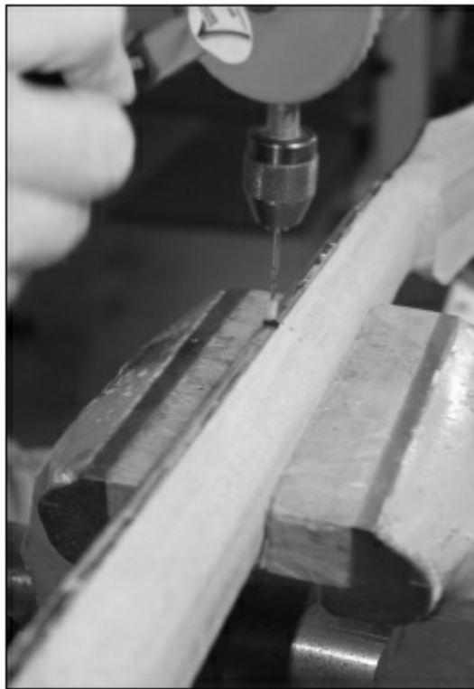
FIGURE 2.2.14. For the steel string guitar, we used 2 mm MOP dots for the fingerboard side dots. In this case, we are using plastic dots cut from a small plastic rod with a 1/16'' diameter. Note the masking tape on the drill bit as a stop marker. After measuring the position for each of the side dots, we drill a 1/16'' hole approximately 1/8'' deep.
