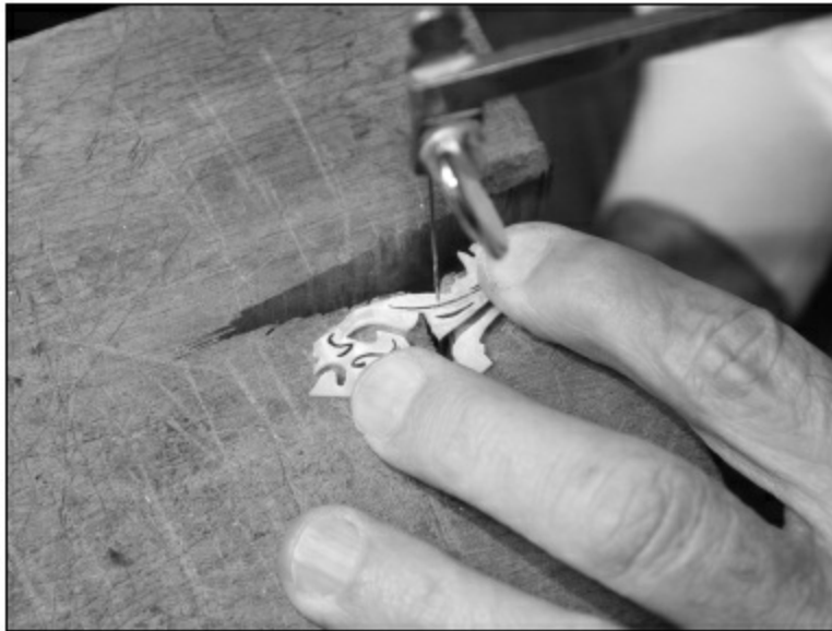
FIGURE 1.4.92. Now we cut out each of the pieces. We are staying slightly outside the lines, and we will file any uneven sections.
