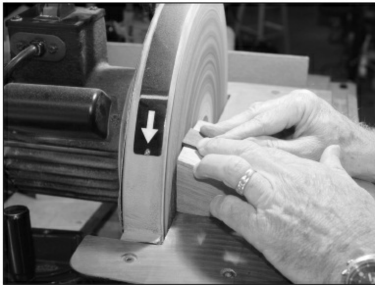
FIGURE 1.4.99. After shaping the truss rod cover, we sand the same angle onto the nut edge as we did on the headstock laminate.
