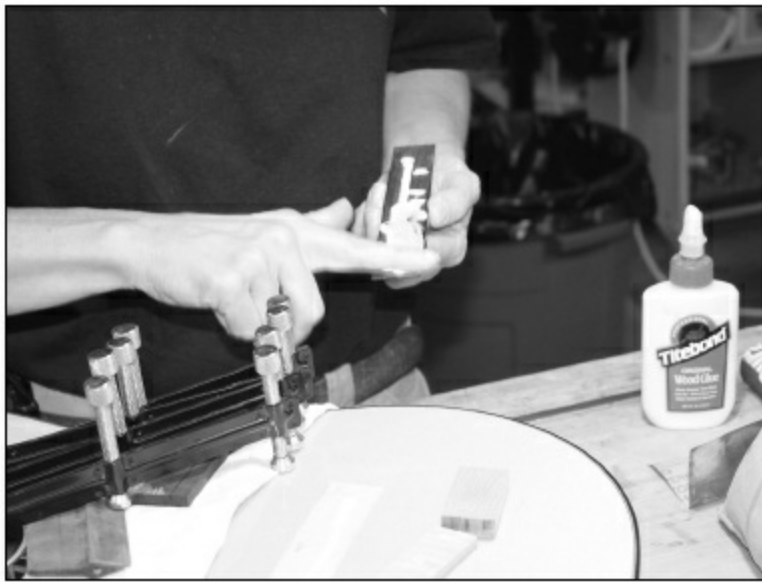
FIGURE 3.4.9. Glue is being put onto the bridge.
