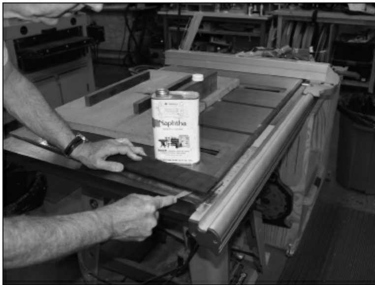
FIGURE 1.4.18. To remove the fingerboard from the template, use some naphtha in a pipette and carefully lift the board with a thin knife edge. We use an artist's pallet knife for this. You must be patient and let the naphtha do its job loosening the tape. If you force it, you could crack the fingerboard—particularly at a fret slot.
