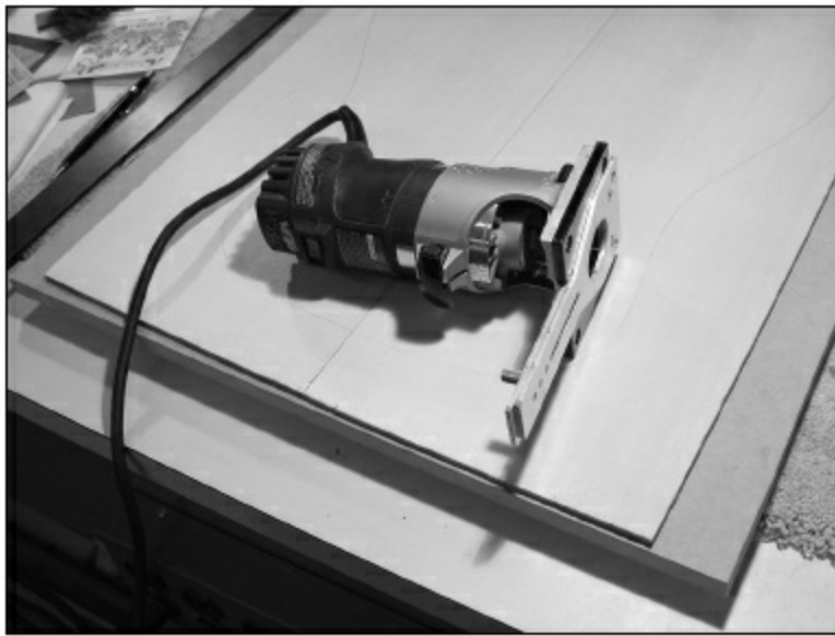
FIGURE 1.1.18. We will now cut the grooves into the top using a laminate trimmer attached to a Stew-Mac circle cutter. The laminate trimmer base had to be slightly modified so the holes in the circle cutter screw properly into its base.
