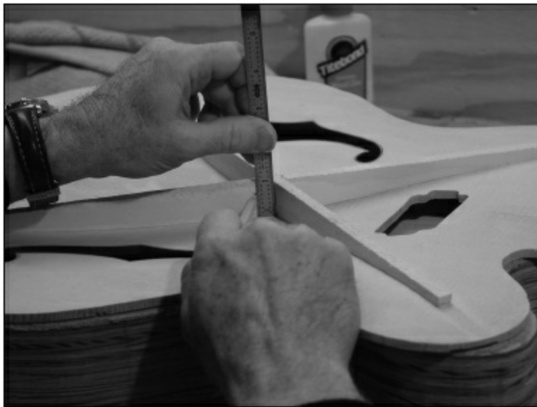
FIGURE 2.1.56. After the glue is dry, we cut off the extensions of the braces and measure exactly how tall we want the braces to be. This guitar is a 17" (lower bout), so we will make the braces 5/8 " tall (at the X ). For a smaller guitar, we will make the braces shorter.
