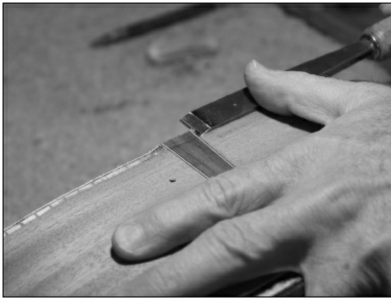
FIGURE 1.3.70. Next, put the chisel blade directly in the binding slot and clean out the necessary wood.
