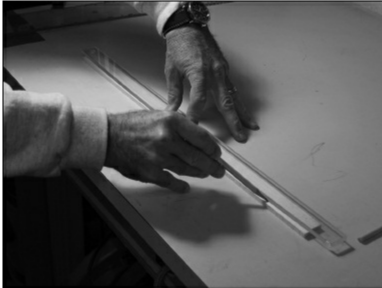
FIGURE 1.1.33. Once the braces have been thickness sanded down to 1/4" (which is the desired width of our braces), we begin preparing the X braces by first drawing a 25' radius onto one edge of the braces. The top of this guitar will have a sphere with a 25' radius, which, from our experience, helps in tone and structural integrity.
