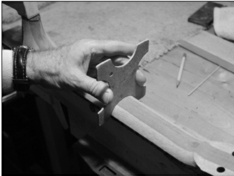
FIGURE 1.4.123. As the neck is being carved, we will use the template shown to check the radius of the neck as it slowly increases from the nut to the heel. The template is simply a square of fiberboard with a different arc cut on each side: 1", 1 1/16", 1 1/8", and 1 3/16".
