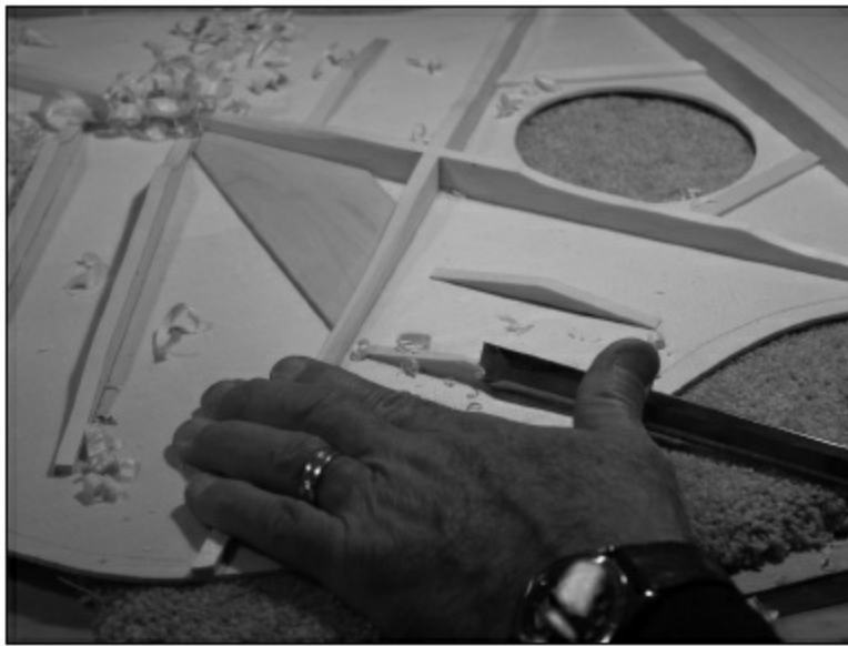
FIGURE 1.1.56. We use a chisel to thin the edges of the finger braces. Again, this is not removing much strength but is removing a lot of the mass of the brace.
