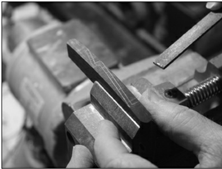
FIGURE 2.3.14. The lines are drawn on the top of the bridge top, showing where we want to carve away excess material, leaving the proper intonation points for our bridge.
