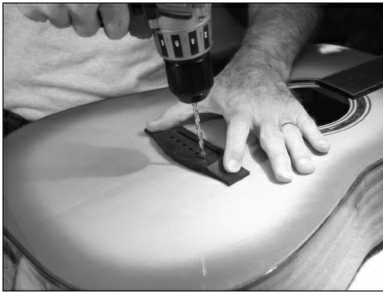
FIGURE 1.7.16. The next step is to remove the template while leaving the bridge in its correct location. Then, 3/16'' holes through the two bridge pinholes on the ends.
