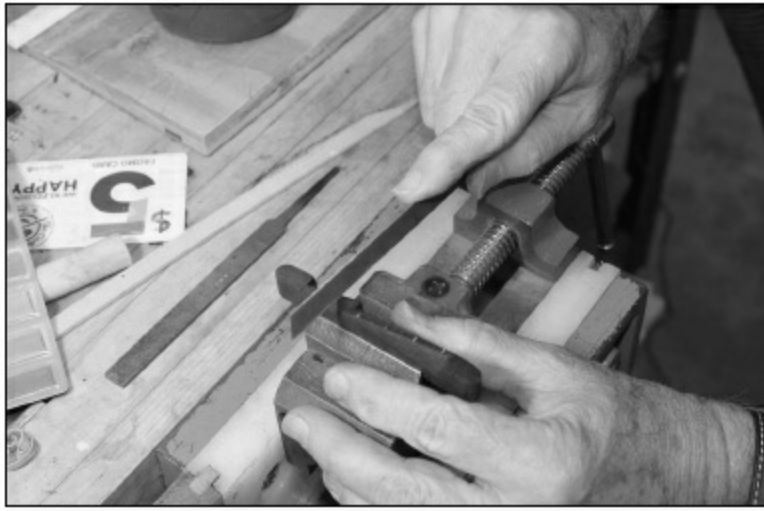
FIGURE 2.3.16. Now, we must file a notch where we want each string to cross the bridge, which is marked by the white lines. We will use the same files that we use on the nut for the strings. Tilt the file so the string will intonate on the front edge of the slot.
