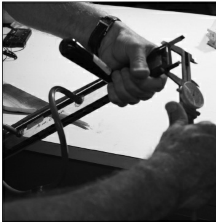
FIGURE 1.4.22. Here is the template with both bindings and both maple purflings being measured. At this point, if the measurement is too large (and we typically start with very thick bindings to make sure the measurement is too large), we have two choices. First, we can put the bindings through the thickness sander to reduce their thickness. Second, we can joint very small amounts from each side of the fingerboard (you must joint both sides). Our template was made to make the fingerboard come out at exactly 1 \frac{3}{4} " at the nut, using two 0.020 purflings, and two 0.080 bindings. From our experience, it's much easier to sand off very slight amounts from the bindings than to joint off the same very small amounts from the fingerboard.
