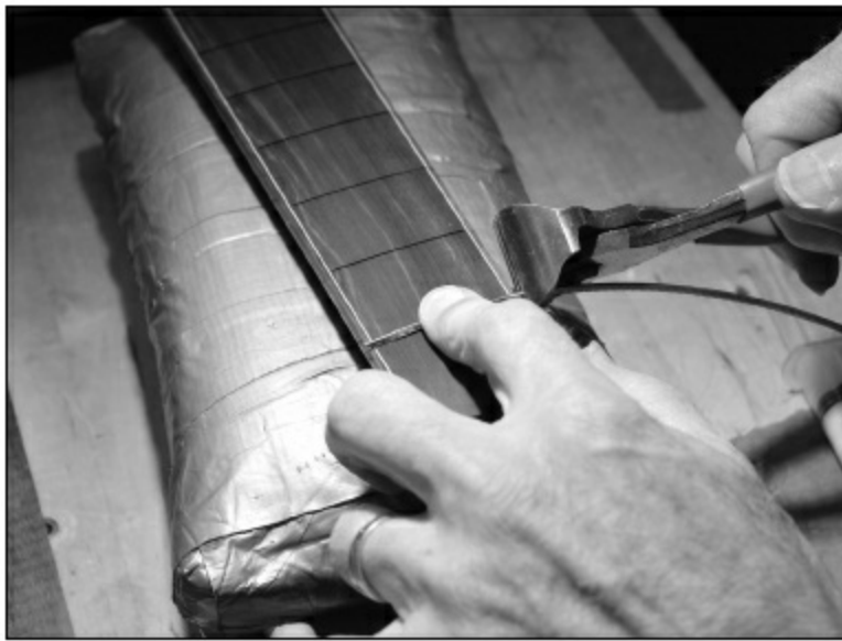
FIGURE 1.7.40. Now, we take our fretwire, lay it across the first fret, and cut—with a little overlap on each side. We repeat this for each fret all the way up the fingerboard.
