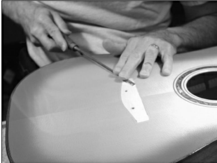
FIGURE 1.7.19. Next, we use a chisel to lift and scrape away the lacquer up to the scribe line. This is a step where a long-neck chisel works very well. It's easier to hold the chisel flat against the surface.
