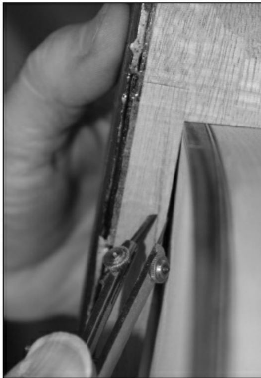
FIGURE 2.2.12. Now we start fitting the neck to the body. Put the neck dovetail into the body dovetail, and using a small compass, let the point of the compass follow the guitar top profile, while the pencil draws the profile onto the fingerboard extension.
