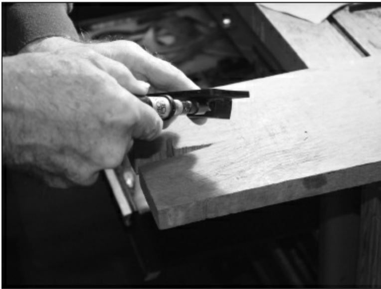
FIGURE 2.3.35. Using a hand chamfer tool, we chamfer the edges of the holes so the screw heads will be flush with the block when screwed in.
