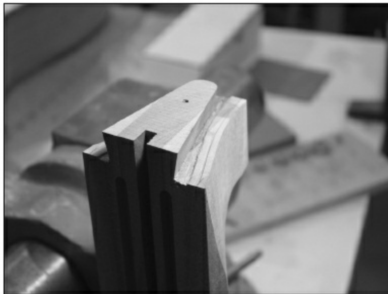
FIGURE 1.4.52. Here is the heel with the shelf carved out. It is about \frac{1}{32} " deep. As the final neck carve is done, the dimension will approach the original line from the template.
