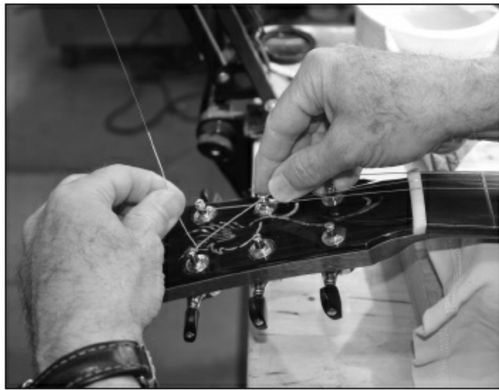
FIGURE 1.7.88. We put the string under itself and pull up on the string. We now start to tighten the tuning machine, and the string will tighten on itself, locking itself onto the tuning peg. The strings will not slip if you use this technique to string your guitar.
