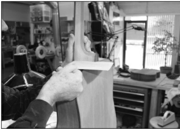
FIGURE 1.4.127. If the neck is pointing to the left, the sandpaper must be pulled straight to the left side to realign the neck. Once we get the alignment correct, we'll check the vertical angle. We don't want to adjust two angles at once. In this case, it took about fifty pulls of the sandpaper to get the alignment right.
