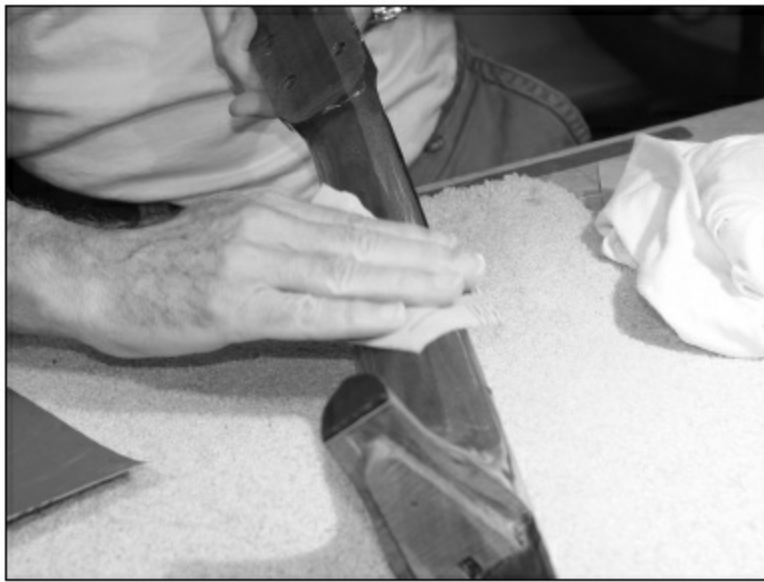
FIGURE 1.6.44. Once we're happy with the body, it's time to sand the neck. We will start with 600-grit sandpaper, then use 1000-grit sandpaper to sand the shaft of the neck. We will not buff the neck shaft unless requested to do so, because most of our customers like the feel of the neck with a satin finish instead of a gloss finish. However, we will sand the back and top of the headstock with 1200- to 2000-grit and buff them.
