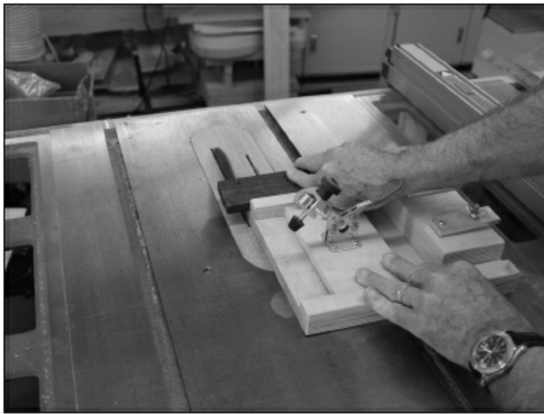
FIGURE 1.5.5. Next, we flip down the hinge, place the freshly cut end against it, and cut the other end. With that, we have a blank that is the proper length. We don't have to measure it, since we had measured when the jig was made. Our bridge blank is 6" long.
