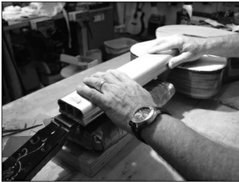
FIGURE 1.7.60. Next, we use the same curved sanding block that we used to sand the fingerboard to sand the tops of the frets. We use 220-grit sandpaper for this step and sand very lightly. This step is called fret leveling.
