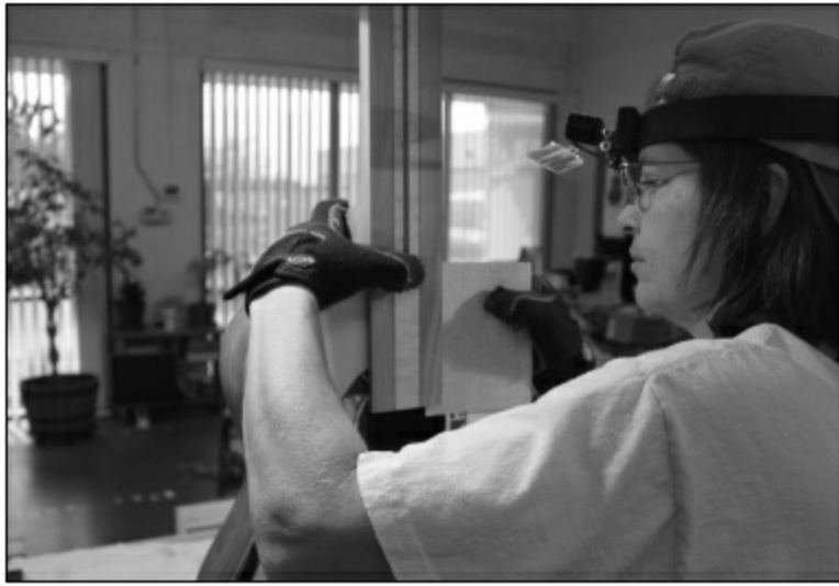
FIGURE 3.2.5. As the neck gets down into the dovetail, sandpaper is used to get the underside of the fingerboard extension to meet exactly with the top.
