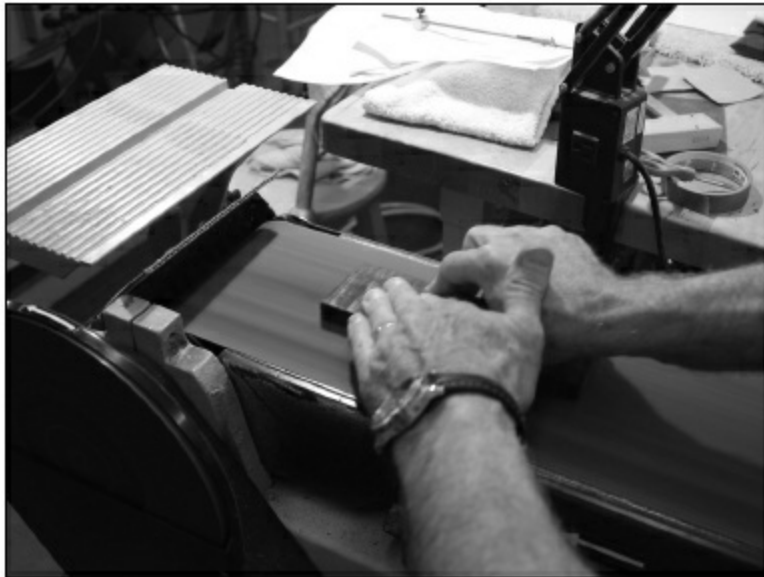
FIGURE 1.5.2. First, we will sand one side flat and put one of the long sides through the jointer. This leaves us with two smooth sides at 90 degrees from each other.
