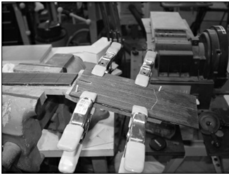
FIGURE 1.4.75. We have placed 1/8" dowels into the alignment holes. This helps ensure that we can get the headstock in the same position when we glue it down.
