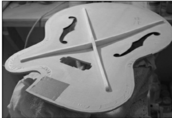
FIGURE 2.1.58. Here is the top, braces carved, in the spray booth ready for a seal coat of shellac. You can see that the rim of the top where it will glue to the guitar sides and kerf has been taped off as have the areas of the head block and tail block.
