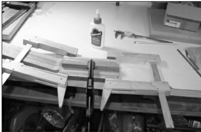
FIGURE 1.4.47. After cutting the dovetail, we glue the ears onto the headstock. We will try to use some cutoff pieces from the same neck block that the neck came from so the ears will match as closely as possible to the neck itself.
