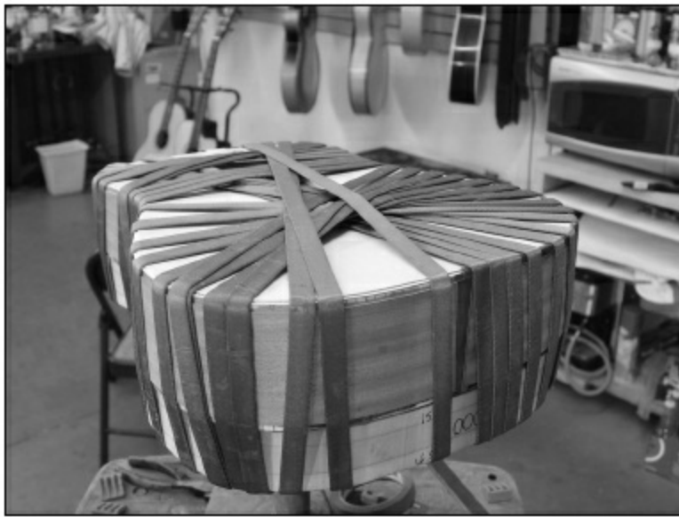
FIGURE 1.3.84. Here is the first piece of binding, all strapped down. After this piece of binding, we will put on the other piece of the top binding, then turn the guitar body over and do each side of the back binding.
