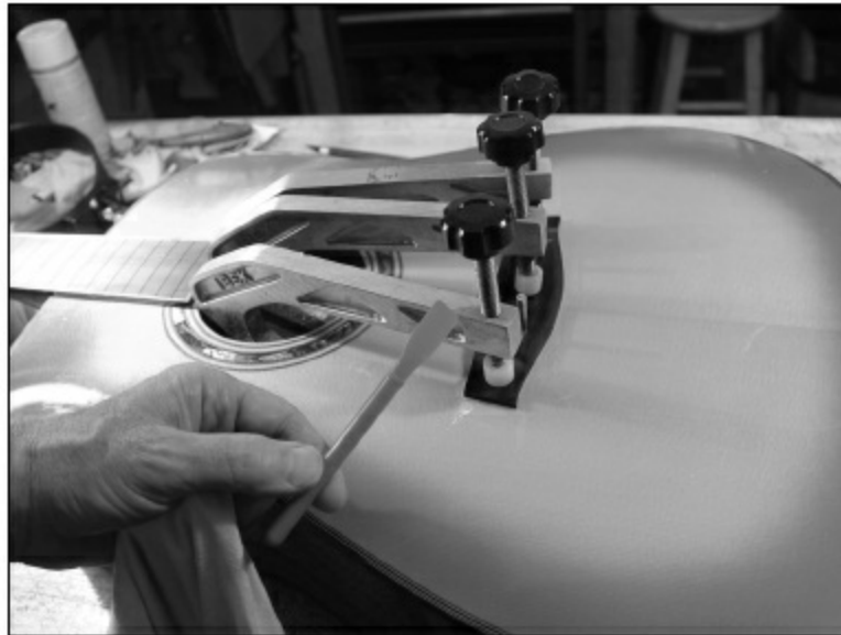
FIGURE 1.7.28. We often use a small plastic spatula as shown to help clean up glue squeeze-out.
