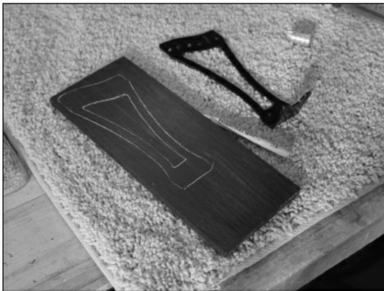
FIGURE 2.3.19. We start with a piece of ebony about 1/4" thick and big enough to trace the tailpiece skeleton.
