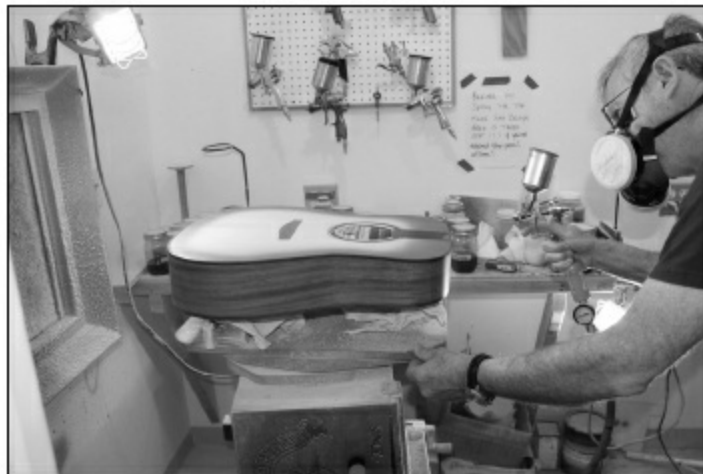
FIGURE 1.6.33. This is a pretty good angle showing our spray booth. Clear coats are being sprayed on the sides and top (first day of spraying). Note the light to the lower right—the reflection of this light can be seen as the sides are sprayed. The guitar is rotated on the lazy Susan, keeping the reflection in view as the sides are sprayed all the way around. The light at the upper left is used to see the reflection as the top is sprayed. You must keep these reflections in view as the spraying is done. If you try to spray without the reflection in view, you really can't see how good and even a job of spraying you are doing. On the far left is the exhaust, which is a filter in front of an explosion-proof fan. Even though we spray mostly water-based lacquer, the colors, mixed in shellac, are flammable because the shellac is mixed with alcohol.
