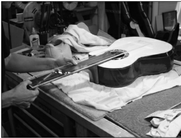
FIGURE 3.4.1. We start by clamping on the neck and checking the alignment. We use a homemade template made of plexiglass 1/4" thick, 3" wide, and about 30" long. It has a centerline scratched on it, and two other lines that approximate the position of the two outside strings. Two holes ( 5/64 " in diameter) are drilled in the template exactly where the two outer strings intersect the saddle.
