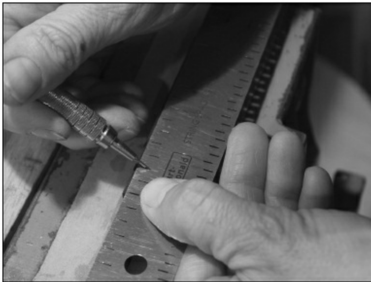
FIGURE 3.3.10. Using a Stew-Mac string spacing ruler, Diana finds the outer string position and then marks the position of the rest of the strings. We then make a mark 1/8'' to the bass side of each string since we are making a two-hole tie system for this guitar. We also mark the centerline horizontally along the back of the tie block. Figure 3.3.11. We are now ready to drill. In this photo, the depth stop for the drill press is being set to allow the bit to pass through the tie block but not touch the angle.
