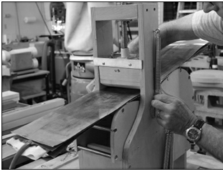
FIGURE 1.3.9. The main waist clamp is lowered until it is snug with the side sandwich. Next, the springs are connected to the waist crossbar. This crossbar is critical, especially for narrow-waisted guitars with figured woods. It helps prevent the wood from splitting at the waist bend.
