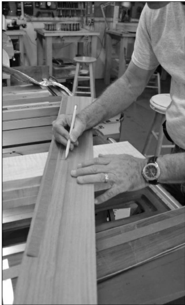
FIGURE 1.3.3. Put the tape on one side that is already cut a little longer than the tape and thickness sanded (or “thickened”) to 0.085”. Then we transfer the lines from the tape to the side.
