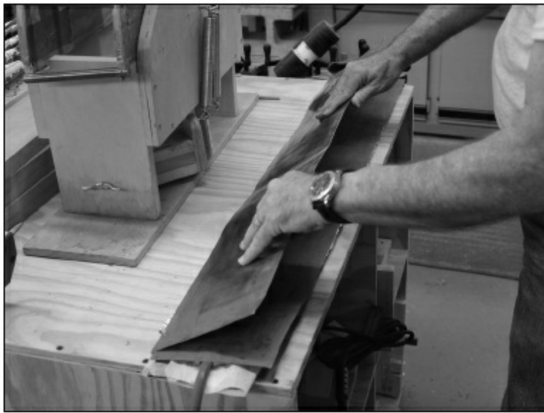
FIGURE 1.3.7. We create a sandwich with the foil between the two pieces of spring steel, using a heat blanket directly against the foil. Again, we mark the position of the waist.
