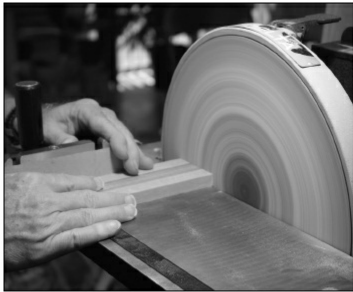
FIGURE 2.2.1. This is the first step to make the fingerboard extension. A piece of wood from the leftover neck material scrap is chosen for the extension. It is cut to approximate length (about 6") and is sanded to 1/2" thick for this guitar. This archtop has a built-in pickup. If this had been an acoustic archtop or if it had a floating pickup, the fingerboard extension would be thicker (about 5/8"), therefore making the fingerboard sit higher off the body of the guitar. In this case, we want the strings to be closer to the body and the built-in pickup.
