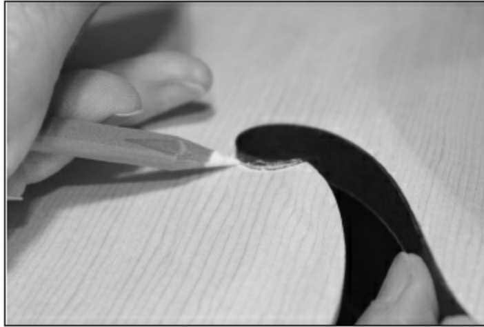
FIGURE 2.1.24. The fiber is easy to bend, so just bend it around your finger and fit it into the F-hole. Then, using a white pencil (or any pencil that will show up on the black layer), mark the binding overlap as shown on both the top and back side of the guitar top.
