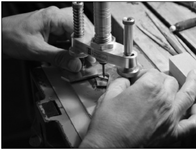
FIGURE 3.1.9. After the pieces are cut, the patterns are cut into the Macassar ebony with a Dremel tool.
