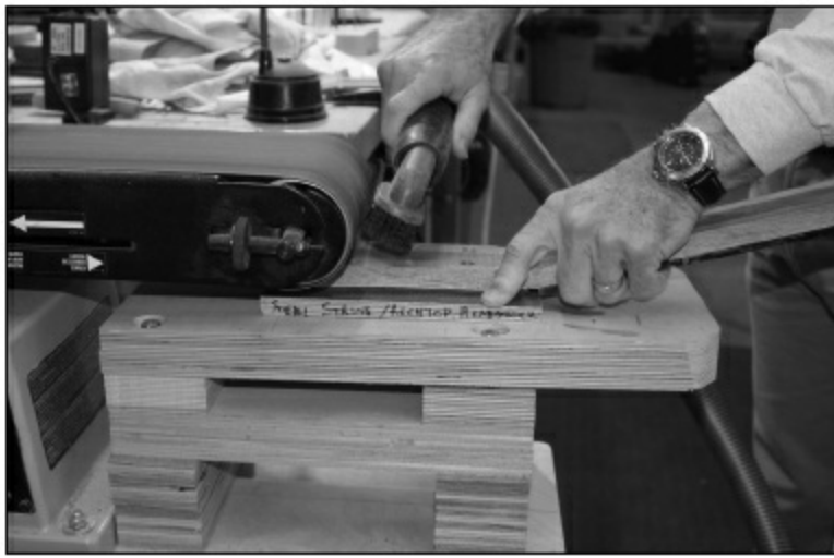
FIGURE 1.4.106. Here is the jig we use to thickness the headstock of our steel string and archtop guitars. The classical guitar uses the same basic jig but with a different size spacer to make its headstock the proper thickness.
