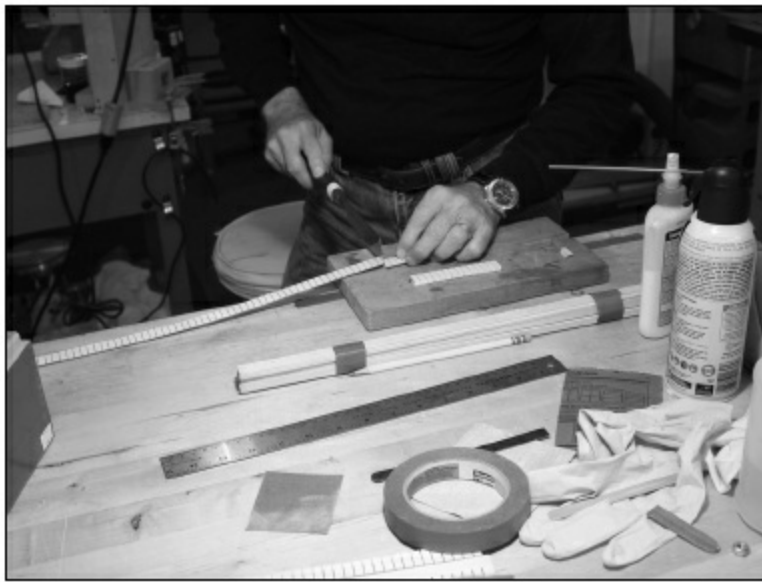
FIGURE 2.1.65. Once the headblock and endblock are glued in, we first replace all the clamps with go-bars, just as we did with the steel string (and all of our guitars). We profile the edges of the sides with a flat sanding board. Then we start cutting kerf. We cut two identical pieces at a time as shown, using a cutting board to keep from damaging the bench.
