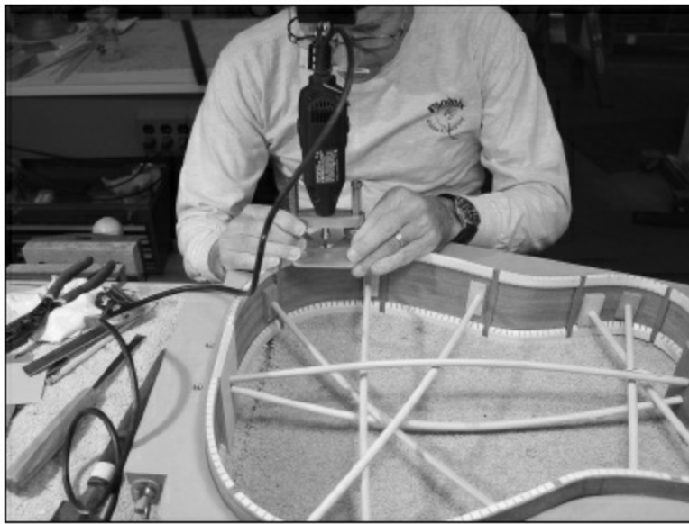
FIGURE 1.3.32. Now we will use a Dremel tool and carve a 1/8" deep slot where we made the marks.
