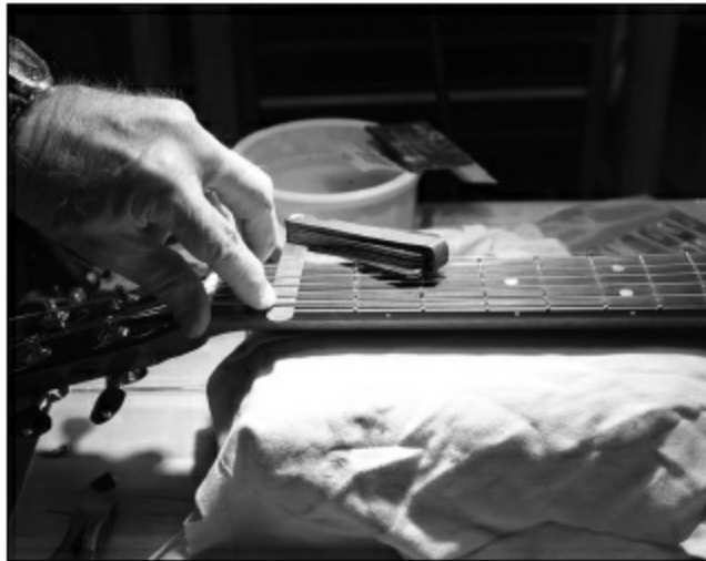
FIGURE 1.7.91. To set the heights of the strings, we put a feeler gauge under the strings at the first fret and push the string down, touching the gauge. Note, we use a .010 gauge for the low E and A strings, a .009 for the D and G strings, and a .008 for the B and high E strings.
