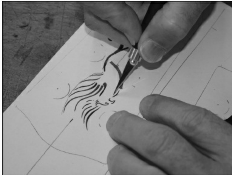
FIGURE 1.4.90. We are now cutting out the body of the bird and will glue the individual pieces to a scrap of mother-of-pearl (MOP).
