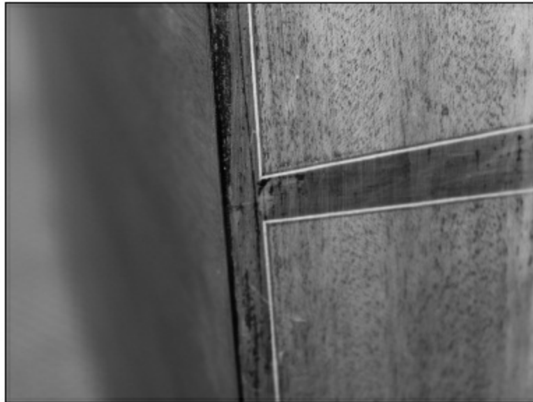
FIGURE 1.6.17. As you can see here, we have encountered a glue spot. It shows up as a light discoloration, this time on the Indian rosewood on the end graft. We will have to scrape down to the wood and sand the glue spot down. There is really nothing lost here, since we have to put on at least one more coat of epoxy. However, it is a good idea to carefully look at the entire surface and check for any more spots.
