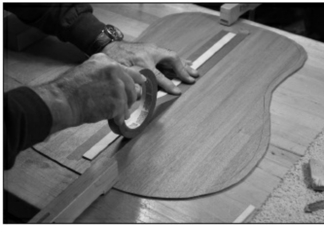
FIGURE 1.2.10. After the center strip is glued, the back is clamped to a bench and double-thick masking tape is put down each side of the strip.
