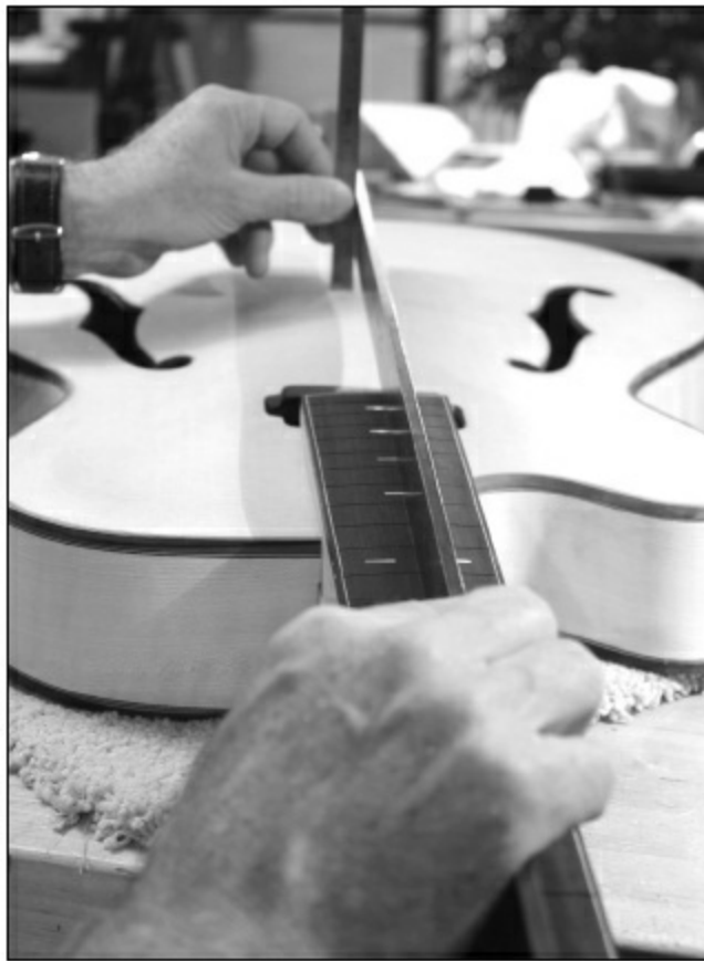
FIGURE 2.2.19. Now we start aligning the neck and finish the fit. We check left to right alignment to the centerline (drawn on the top of the guitar), and we check alignment up and down (the neck angle) by measuring the plane of the neck with a straightedge as shown and by measuring the height of the straightedge above the guitar body at the point of the bridge (between the points of the F-holes). This height should be about 3/4'' at this point. This is the measurement for the height measured when the pickup is built in. For a floating pickup, the measurement is closer to 1'' .
