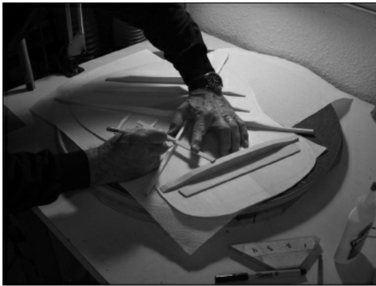
FIGURE 1.1.52. Finally, the sound hole braces are being made. These small braces strengthen the area under the rosette. They are made from scrap left over from the top. We glue one on each side of the sound hole, forming a pentagon shape with the X braces and the upper face brace.
