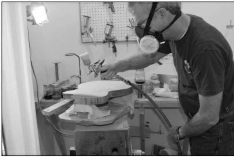
FIGURE 1.6.29. Before we actually spray the color on the guitar, we spray it on a test board. We want to check how the gun is spraying and make sure there is no spitting or dripping from the gun before we spray the guitar—any gun malfunction would be a disaster at this point. Since the body will be sitting on a lazy Susan so we can rotate it as we spray, we want to be sure it is also functioning smoothly.
