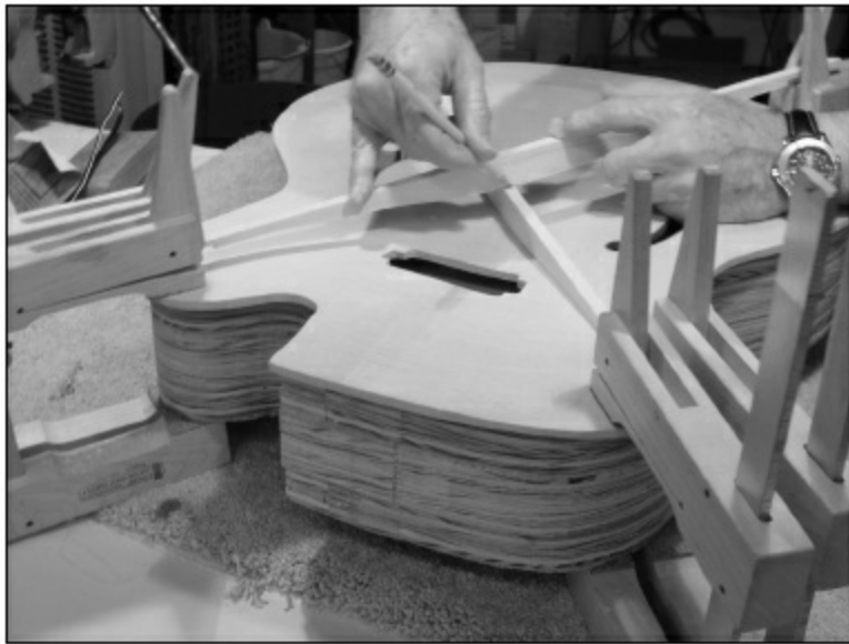
FIGURE 2.1.45. Now it's time to carve the notch and fit the X together. The photo shows that we have put cam clamps to align both braces, so we can mark the intersection point of the X .
