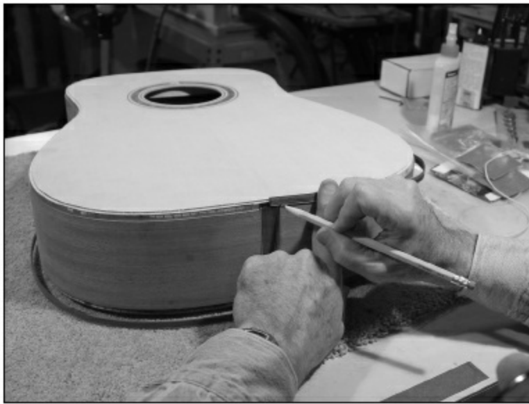
FIGURE 1.3.76. Now we put each binding back onto its respective binding slot and mark where the purfling will be mitered with the purfling of the end graft.
