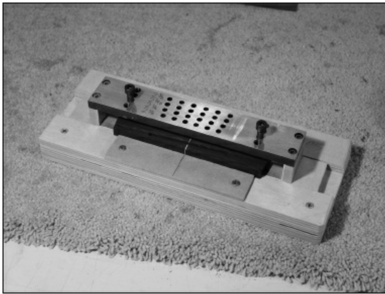
FIGURE 1.5.24. This is a great jig we bought from LMI. Frank Ford designed it. It allows you to drill your bridge pinholes very accurately at several different pin spacings. We put this jig into a fixture that allows us to place our bridge against a block, center it against the centerline, and drill our holes (2 1/4" spacing). This is how we make most of our bridges.
