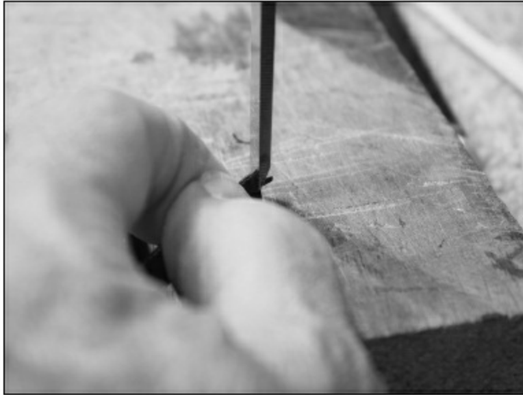
FIGURE 2.1.31. Prepare the short legs just as we did before, cut them to length, and carefully miter both ends with a chisel as shown. You may have to repeat this step a couple of times to get it just right—but it's worth it to get the fit you need.
