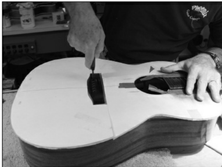
FIGURE 1.7.83. We will now use a tiny saw for cutting slots in the bridge pinholes to make room for the strings. Even though we are using slotted bridge pins, the slots are not wide enough for the A and low E strings to fit. Therefore, we saw a shallow slot in the pinhole to allow for the string to fit while the bridge pin can go completely down.
