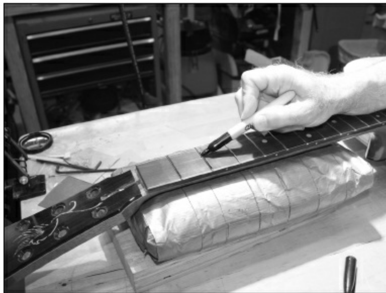
FIGURE 1.7.59. After the neck is straightened, a black marker is used to mark the tops of all the frets.
