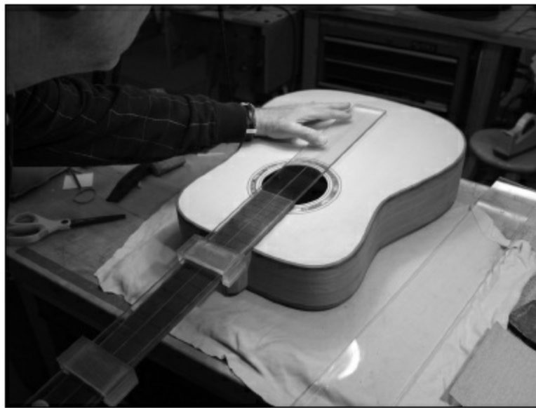
FIGURE 1.4.128. Now, we'll recheck the side-to-side alignment using a different alignment tool that is a little more accurate than the template. Now, the alignment is right on.
