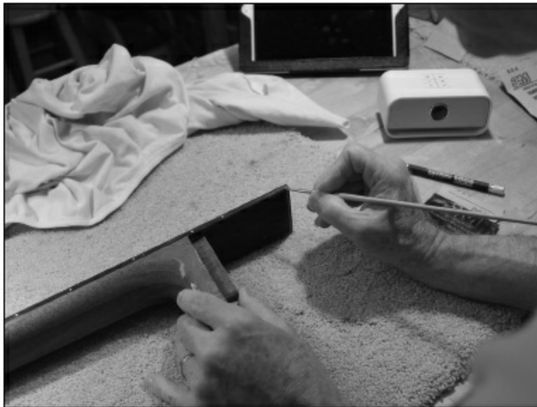
FIGURE 1.6.47. Now, we apply the finish to the area of the sand-through. It could take several applications to get enough finish on the spot to be able to sand it flat. Once that is done, and the rest of the neck is sanded out, we will buff the headstock and the heel. We like to buff the heel, because it will be next to the guitar body, which has a high gloss, and we think the neck heel looks better with the same degree of gloss as the body.
