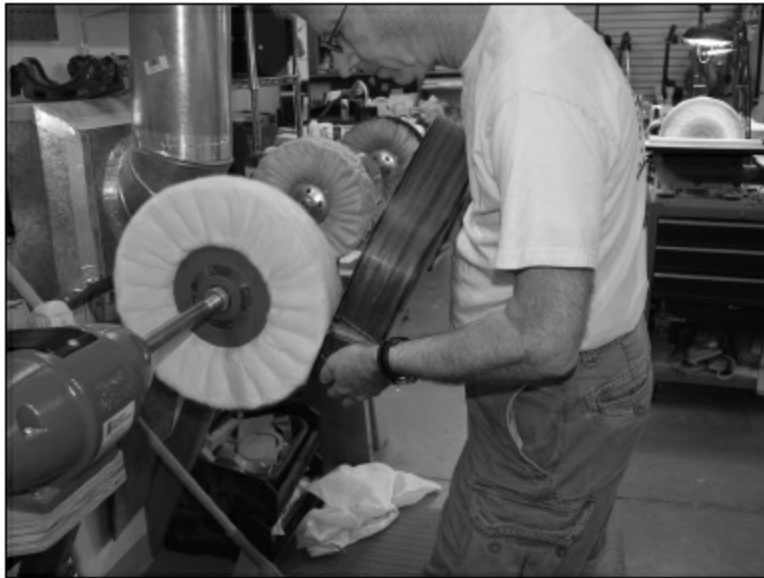
FIGURE 1.6.41. After buffing with the coarse wheel, we then buff with the medium and fine wheels. Be sure that your final run on the buffer is with the grain.
