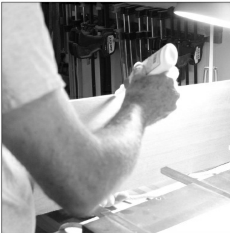
FIGURE 1.2.4. After jointing, the edges are held together and are candled, just as we did with the top.
