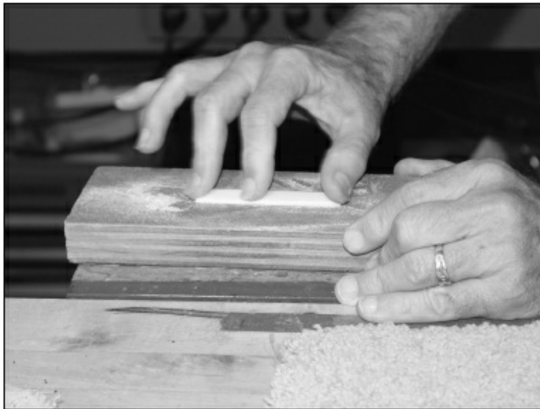
FIGURE 1.7.85. We will now fit the saddle. Upon first check, the saddle we have ( 1/8'' ) is slightly too wide for the slot, so we are sanding it using a block.
