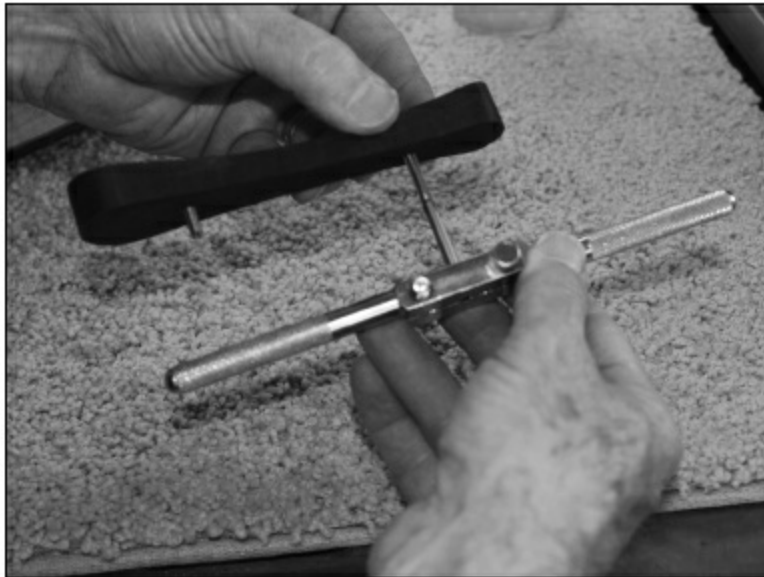
FIGURE 2.3.5. Now we must place the bridge posts. First, we establish a centerline on the bridge, then mark the posts 1.5" on each side of the center. This will place the posts 3" apart.
