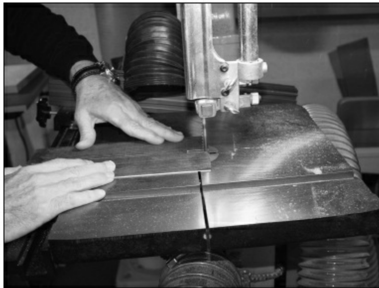
FIGURE 1.4.70. With the truss rod measurements transferred to the headstock laminate, we make a rough cut on the band saw. We cut well inside the lines on this step because we want to file to the lines to make them look good.
