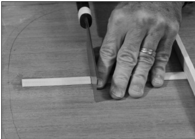
FIGURE 1.2.17. Using a thin kerf saw, we cut just inside the lines. If you cut exactly on or outside the lines, you will have gaps between the braces and the center strip.
