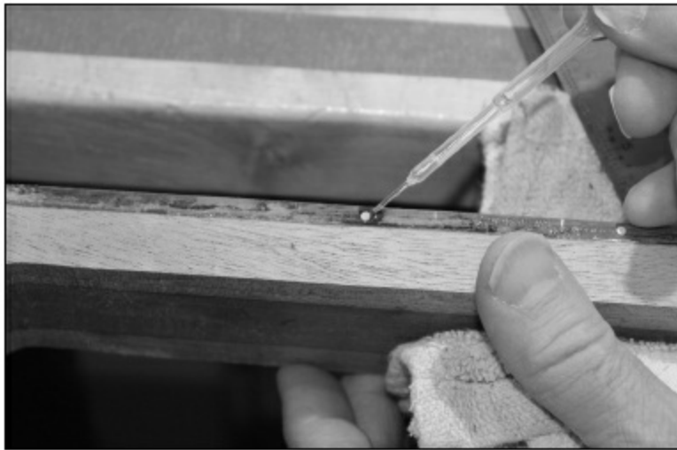
FIGURE 1.4.109. With all the holes drilled and the side dots properly placed in the holes, we use a drop of superglue to affix the dots. For this fingerboard, we can use superglue since the binding is a dark wood (Indian rosewood). If it were a light wood, like maple, the superglue could stain the maple a yellow color. In that case, we would use a drop of Titebond in each hole before we put in the dots. Remember, the dots should stick out slightly from the level of the binding.
