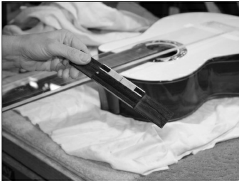
FIGURE 3.4.2. Once we're happy that the neck is straight by checking the centerline of the template with the center seam of the top, we put a piece of tape on the bridge as shown and mark a centerline on it.
