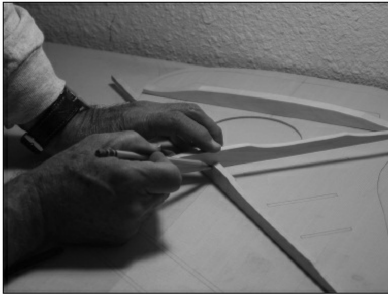
FIGURE 1.1.42. We set the upper brace into the lower brace slot and mark the sides of the top brace in preparation for notching.
