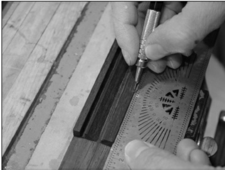
FIGURE 3.3.9. Now, Diana finds the center point of the bridge. In addition, knowing that the outer string spacing will be 2 \frac{5}{16} " (based on the neck width), she will mark the points where the outer strings are located.
