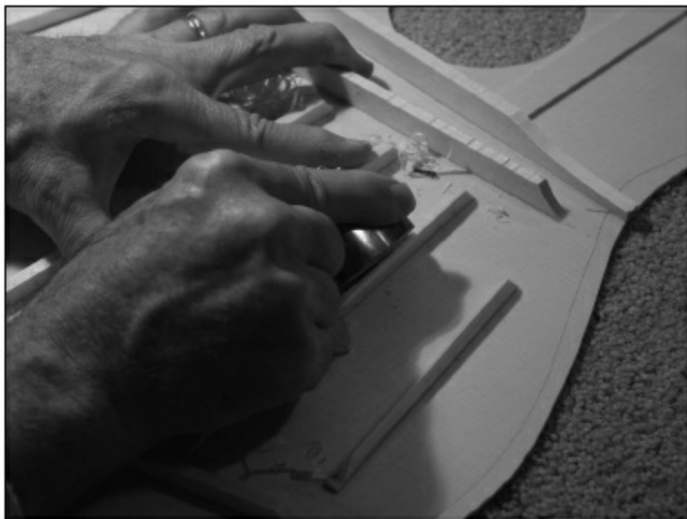
FIGURE 3.1.20. All the fan braces are glued down and all the pencil lines have been erased.
