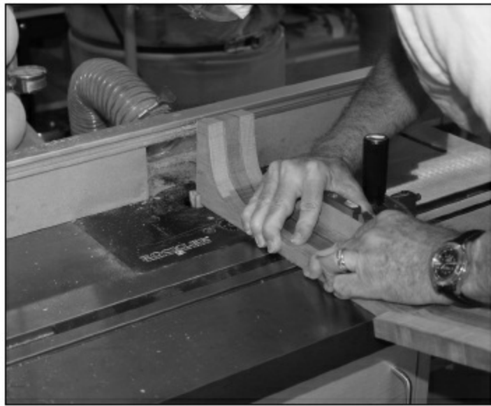
FIGURE 2.2.3. Next, the slot is cut into the end of the fingerboard and dovetail for the fingerboard extension. Note that we do not make the whole cut at once. We only cut about \frac{3}{16} " at a time to keep the cut very smooth. We will end up cutting about \frac{1}{4} " beyond the dovetail into the fingerboard itself.
