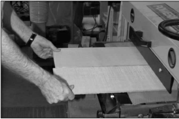
FIG. 1.1.1 We start with a beautiful book-matched set of Engelmann spruce and sand its thickness down to about .150".
