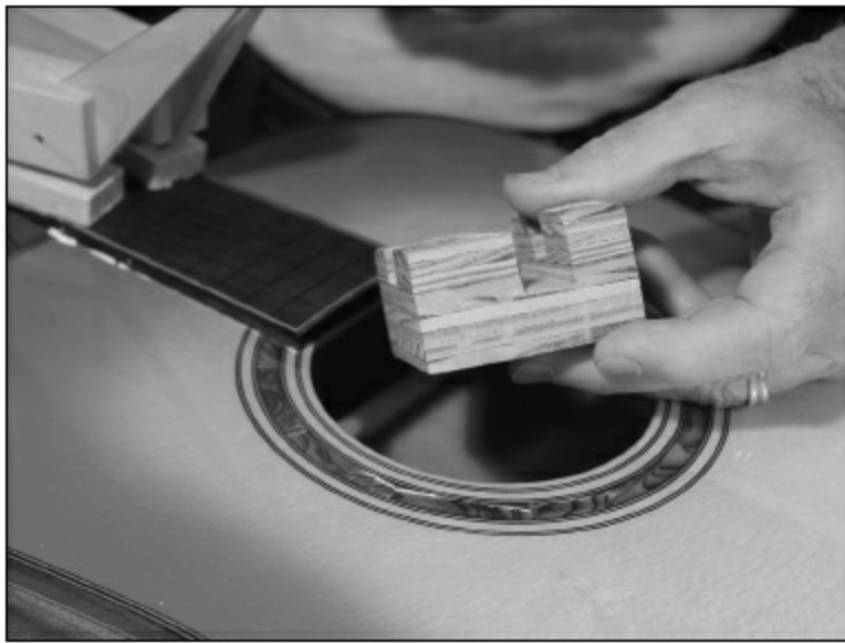
FIGURE 1.7.10. Next, we put a clamping caul in the sound hole under the fingerboard overhang. The caul is designed to go around the upper face brace and allow us to clamp directly onto the underside of the guitar top.
