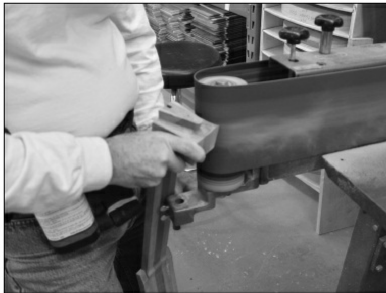
FIGURE 1.4.50. We use our large belt sander to carve away the excess material and get the final heel shape.
