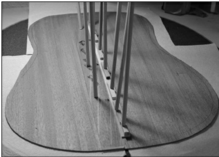
FIGURE 1.2.9. After it is glued, the back is thickness sanded to between .100" and .105" (Note that this is our preference. Some luthiers use different dimensions.) This should give us a final dimension of about .090" to .095". We roughly cut the shape on a band saw—about 3/8" oversized. Next, we use a piece of scrap from the guitar top to make the back strip, which is being shown here in the go-bar deck. Note that the grain of the back strip must be perpendicular to that of the back. Its strength should be in holding the back joint together, and if the grain is in the same direction as the back grain, its purpose would be defeated. We use a back strip that is 5/8" wide and long enough to reach from the headblock to the endblock. In the photo, you can see that we go-bar down a piece of plexiglass and then glue down the center strip against it. The plexiglass holds the center strip in the correct position. In addition, we draw a centerline directly down the glue line of the back to ensure that the center strip is exactly on the centerline.
