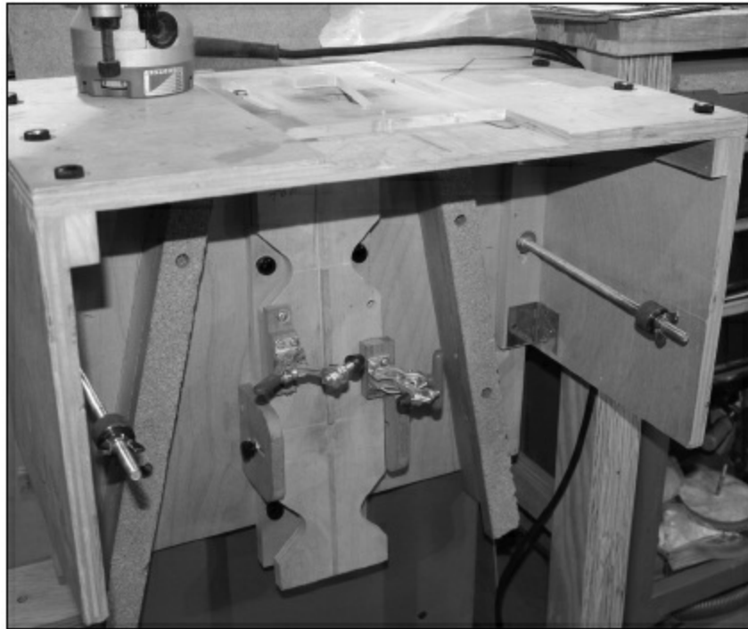
FIGURE 1.4.40. This is the jig that we use for cutting dovetails (thanks to Tom Ribbecke for this idea). The truss rod slot fits into the 1/4" extension in the center of the vertical board and is clamped into place using the two clamps. The hinge at the top of the board allows the angle of the cut to be easily changed, depending on the type of guitar we are making. For the steel string, the angle will be approximately 2 degrees. For an archtop, the angle is approximately 4 degrees, matching the angle of the end of the dovetail above.
