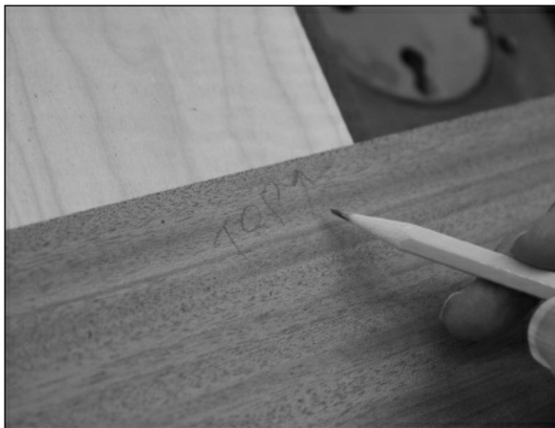
FIGURE 1.3.4. The outside face and the guitar top are marked with pencil. This is repeated on the other side. It is a bad mistake to discover that you didn’t pay proper attention to the book-match of
