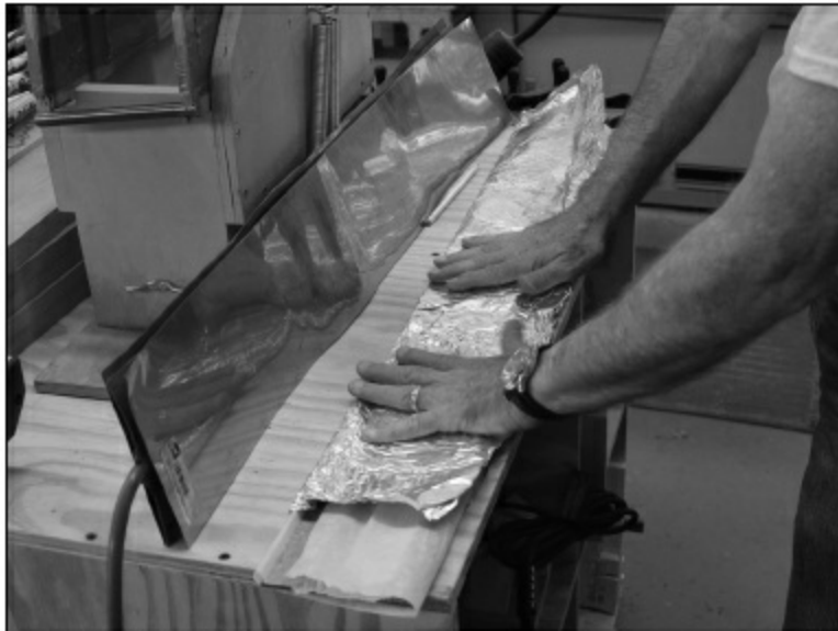
FIGURE 1.3.6. We now fold aluminum foil around the parchment paper. Again, the exact position of the waist is marked clearly on the foil.
