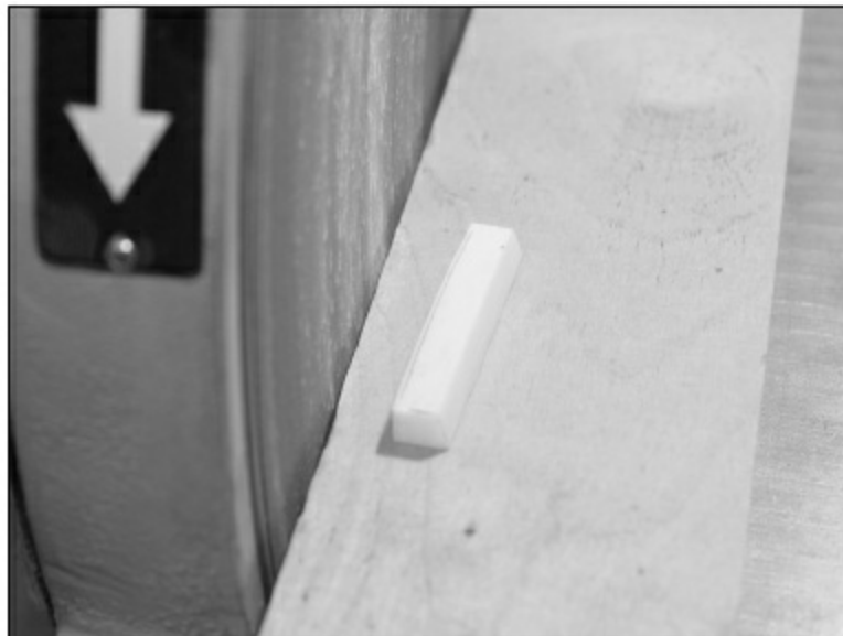
FIGURE 1.7.72. Using the disc sander, we sand the top of the nut to about \frac{1}{32} " above the line drawn by the half-pencil.
