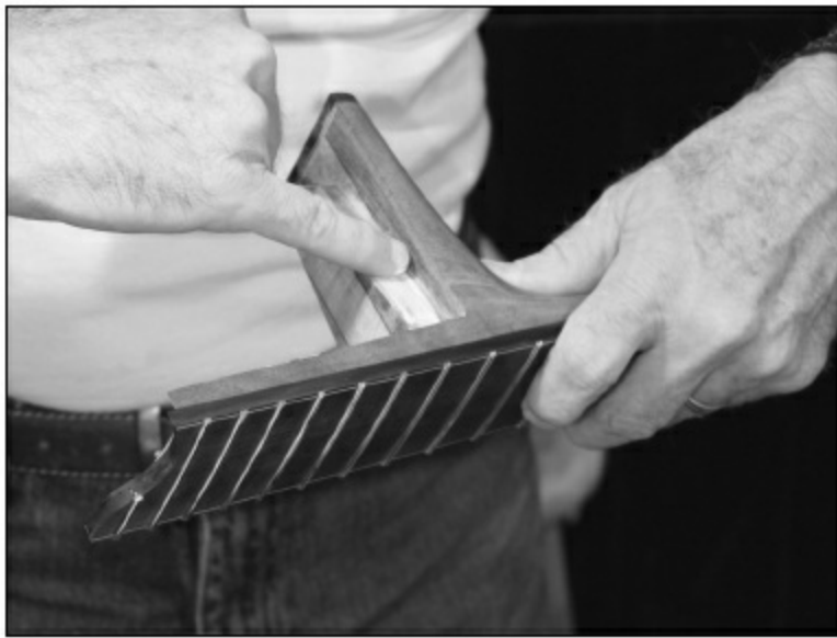
FIGS. 3.4.16 AND 3.4.17. Now it's time to glue on the neck. Glue is spread on the fingerboard extension (note only the outer edges will be in contact with the top) and the dovetail surfaces.
