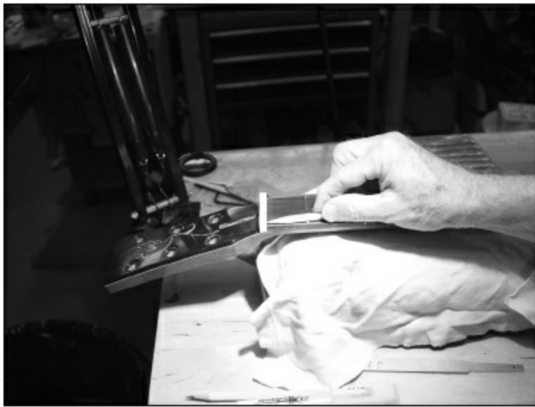
FIGURE 1.7.71. Now, draw a line on the front edge of the nut with the half-pencil resting on the first couple of frets. This will establish approximately how deep the string slots will be cut (but not exactly). It's an approximation only.
