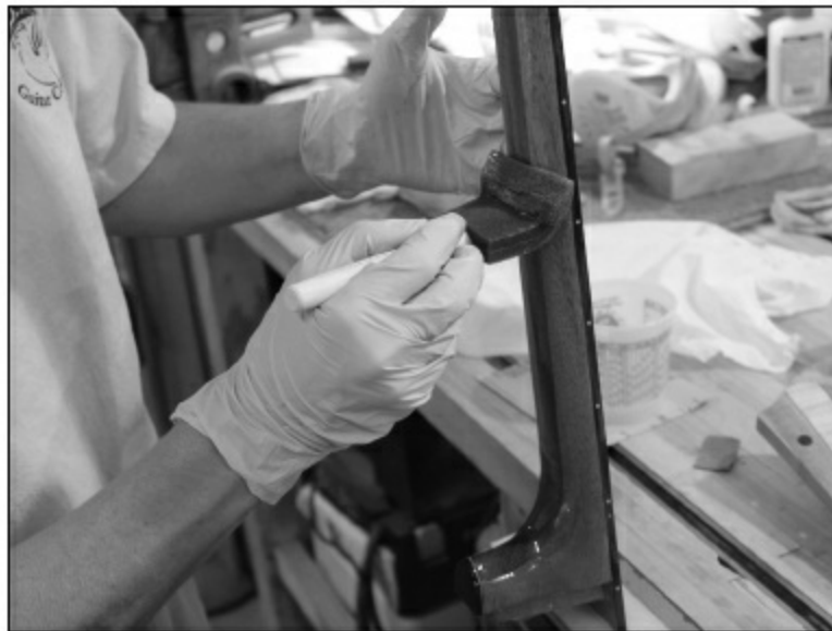
FIGURE 1.6.13. Now, we clamp the fingerboard overhang into a bench vise and apply epoxy to the rest of the neck.
