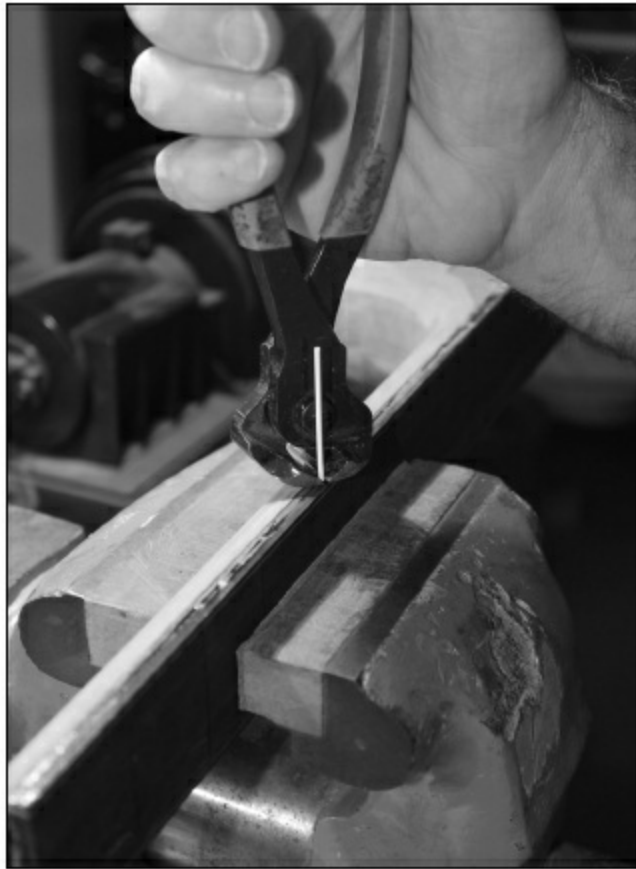
FIGURE 2.2.16. Cut off the plastic rod flush with the fingerboard edge.
