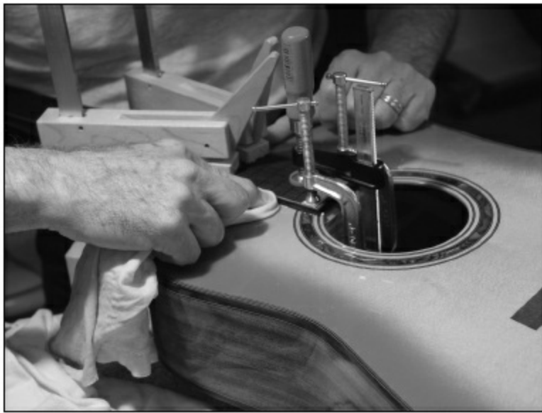
FIGURE 1.7.12. We use a very soft, wet cloth and lightly wipe off the excess glue all the way around the fingerboard overhang.
