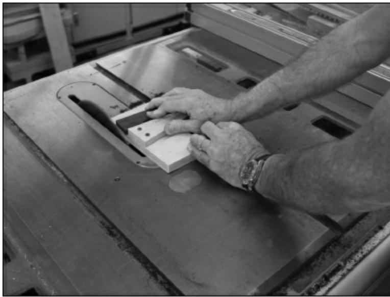
FIGURE 1.5.18. Here is the blank end being cut. The corner of the bridge blank is put directly on the edge of the jig, just where the cut is made. To make the cut on the other end, rotate the blank 180 degrees and flip it over. If you forget to flip it, you will end up having two parallel cuts for the bridge ends—probably not what you want.
