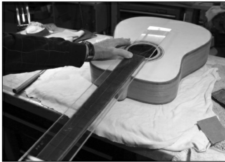
FIGURE 1.4.126. After the neck carving is complete, we will recheck the neck alignment with a template that shows the neck centerline. We use the center seam of the guitar top to check this. In this case, we see that the neck is very slightly pointing off to the left by about \frac{1}{16} " at the bridge. Now we will adjust the neck alignment.
