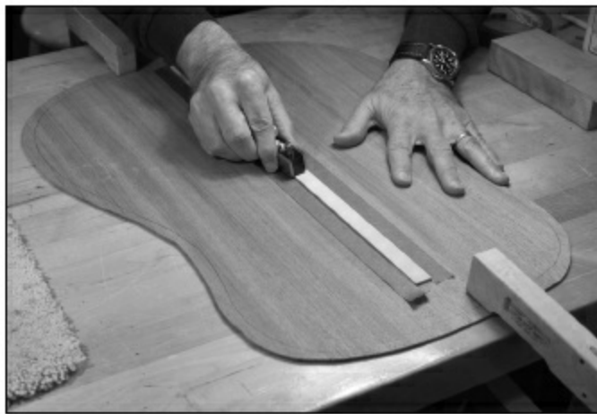
FIGURE 1.2.11. We use a very small hand plane to plane down the edges of the center strip. This step will tear out many facets in the strip that will be sanded out in the next step.
