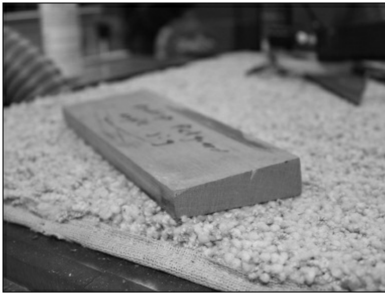
FIGURE 2.3.32. Next, we will use a block made for this purpose. It has a 3-degree bevel on the top edge. Some archtop pickguards come out from the fingerboard at a 90-degree angle. I find this uncomfortable and prefer the pickguard that tilts down slightly.
