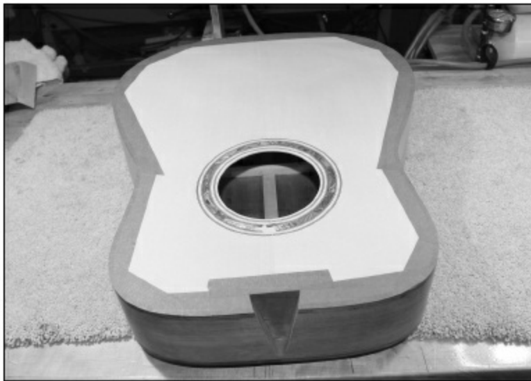
FIGURE 1.6.4. Once the sanding is done, we tape off the edge of the top. We are going to fill the grain of the sides and back with epoxy, and we don't want anything getting on the top. There are many good ways to fill the grain, but this has worked out very well for us. I want to thank John Greven for walking us through this process. It was very helpful.
