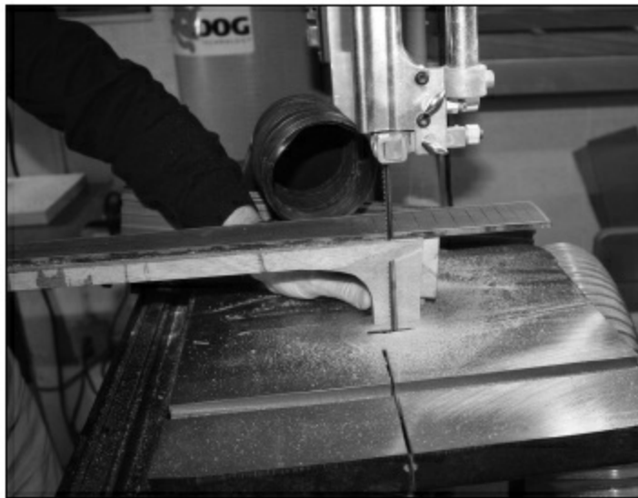
FIGURE 1.4.80. We also cut the edges outside the fingerboard as closely as possible. Again, we want to leave a good margin because cutting the fingerboard or its binding would be a disaster at this point.
