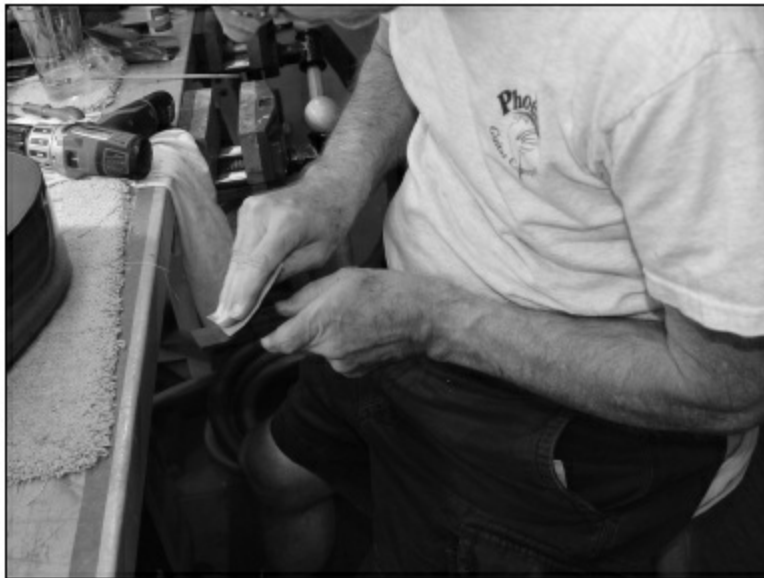
FIGURE 1.7.21. After sanding away as much material as possible on the belt sander, we will then use a coarse grit of sandpaper and shape the remainder by hand.
