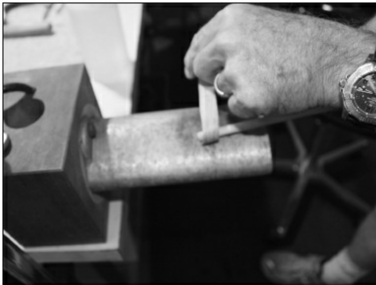
FIGURE 2.1.33. Once the black fiber layer is completed, it's time to work on the maple layer. First, cut the pieces to size as before, but then you must bend the maple on a hot iron. We use a spray bottle to wet the maple veneer, then heat it on the bender and curl it around a dowel. Be careful not to curl it too tightly too quickly, but this method will work very well. Then place the maple piece into the F-hole and mark it with a pencil—just as you did with the black fiber.
