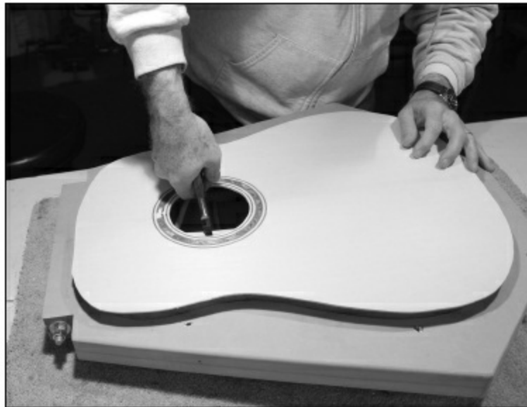
FIGURE 1.3.43. After the glue dries, we must remove the go-bars before the box is removed from the mold. The long go-bars between the endblock and headblock must be cut with nippers. The rest can be removed simply by pulling them out.
