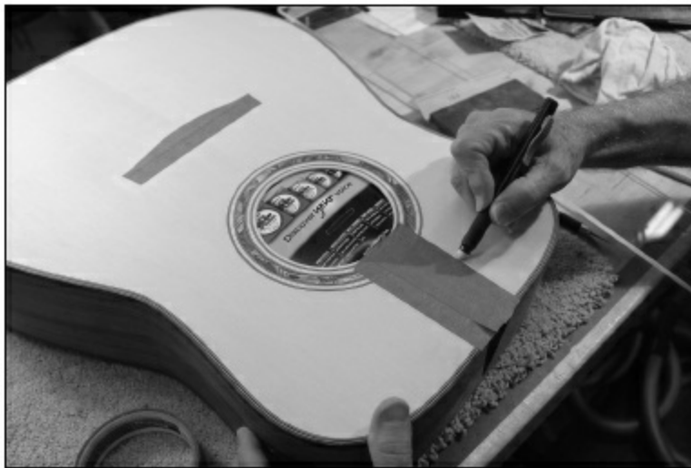
FIGURE 1.6.26. Next, we put the neck back on, trace around the fingerboard onto the body, and put tape about 1/16" inside that line. Note that the sound hole has been stuffed with paper, and a string box lid has been put over the paper. All residual pencil lines must be erased. We like to use a white eraser since it leaves less residue on the guitar top.
