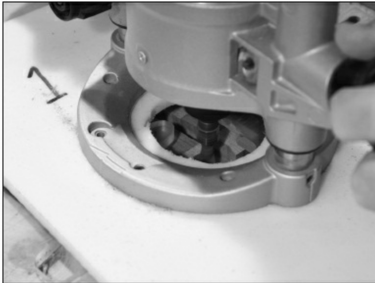
FIGURE 1.4.45. Here is the router bit making the dovetail cut in the neck. The template extends approximately \frac{1}{4} " less down the neck heel versus the cut in the body (remember, the dovetail cut in the body extends 2\frac{3}{4} " ), and the depth of the cut is \frac{5}{8} ".
