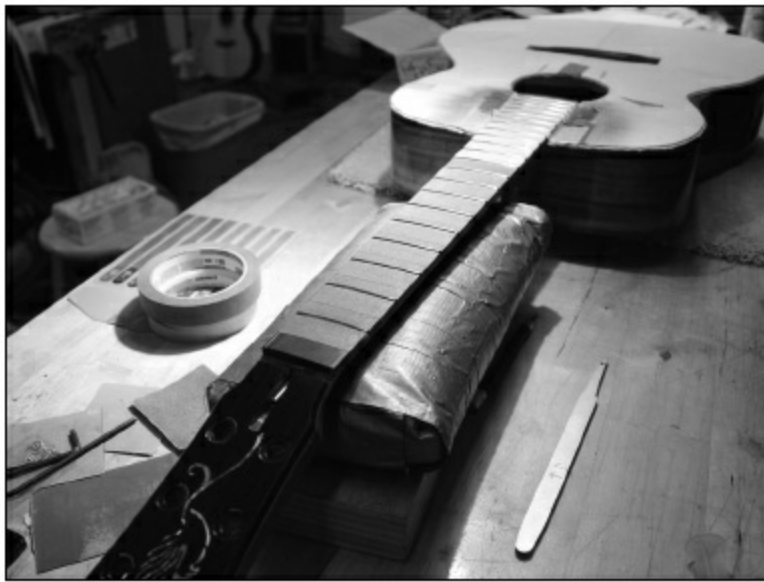
FIGURE 1.7.66. Once all the frets have been crowned, they must be polished because they are still very rough. For this step, we tape off the fingerboard, leaving the frets accessible for sanding.
