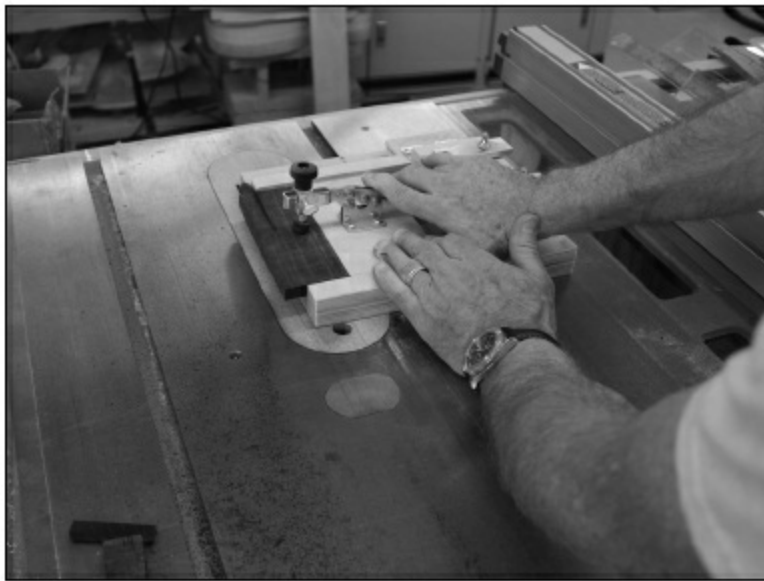
FIGURE 1.5.6. Next, we put the blank into its slot under the toggle clamp with the previously jointed edge against the jig and the rough edge up, and make another cut. This establishes the exact width of the bridge blank.
