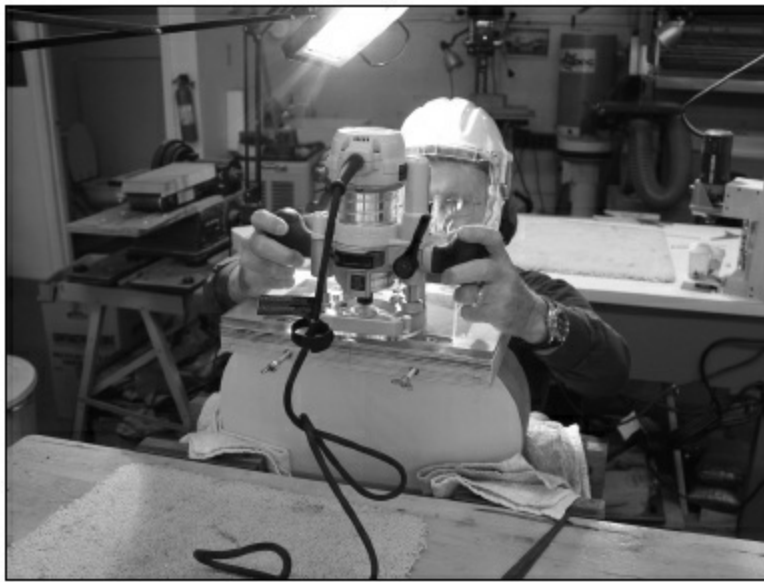
FIGURE 1.3.54. The collar on the router base follows the edge of the jig. It is important to bring the cutter into the guitar top and back rather than to start in the middle of the pattern and push the cutter out. This will help avoid tear-out on the top and back.
