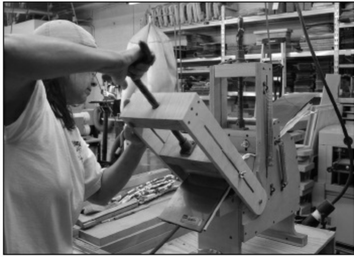
FIGURE 3.1.24. Diana is pressing in the cutaway. This is done very slowly, after the heat blanket has been brought to full temperature. The waist is done first, then the cutaway, and lastly, the lower bout.
