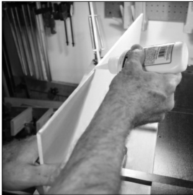
FIGURE 1.1.4. Once we are happy with the candling results, we put glue (in our case, we are using the red label Titebond Original Wood Glue) on one edge as shown.
