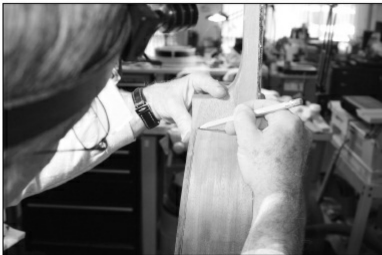
FIGURE 1.4.111. Now we will cut the heel. We cut our heel at the point that's level with the top stripe of the side purfling. In this case, we are going to put purfling under the heel cap to match the position of the side purfling. In this photo, we are marking the location where we will make the cut. We will make this mark on both sides of the heel.
