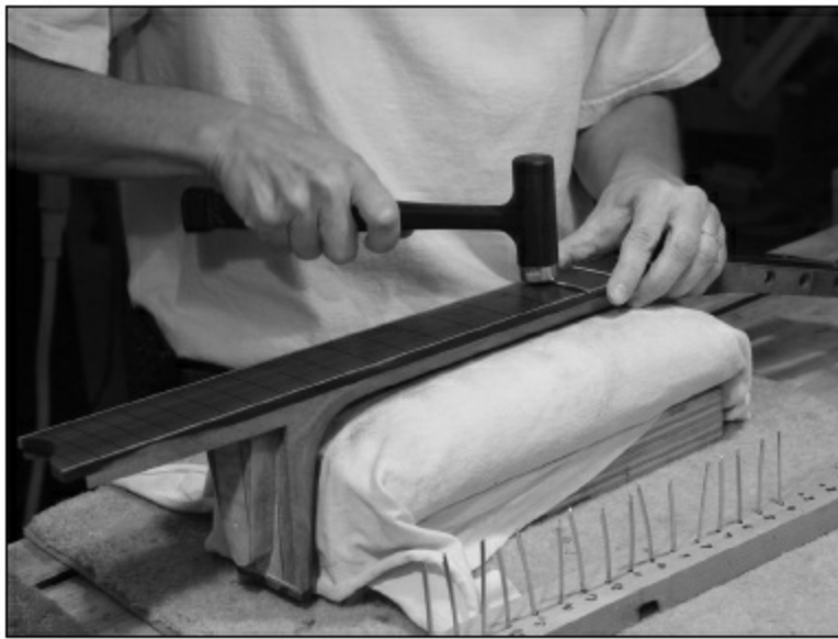
FIGURE 3.4.14. While the bridge dries, we start on the fret job. Just like with the archtop, we're going to fret the fingerboard off the guitar. We could wait and do it on the guitar, as we did with the steel string, but this is easier to do. Since this top is significantly thinner than the top of the steel string, we don't want to risk pounding frets on the guitar.
