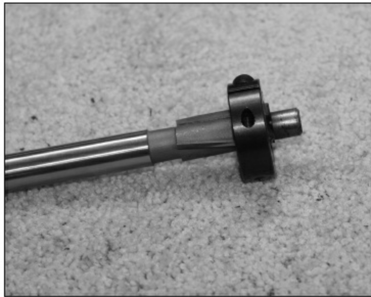
FIGURE 1.4.86. We are going to use a 5/8 " counterbore with a 3/8 " pilot bit to bore out a 5/8 " diameter area around each tuning machine hole. Once the finish is applied, screwing the machines down while the finish is not completely cured causes ripples in the finish on the top of the headstock. The counterbore makes a break in the finish and prevents this problem. The reason we predrill a 25/64 hole is that a 3/8 " pilot bit will not fit into a 3/8 " hole, so we have to drill a slightly larger hole to use the 3/8 " pilot bit. The hole is still perfectly good for the tuning machines we will be using.
