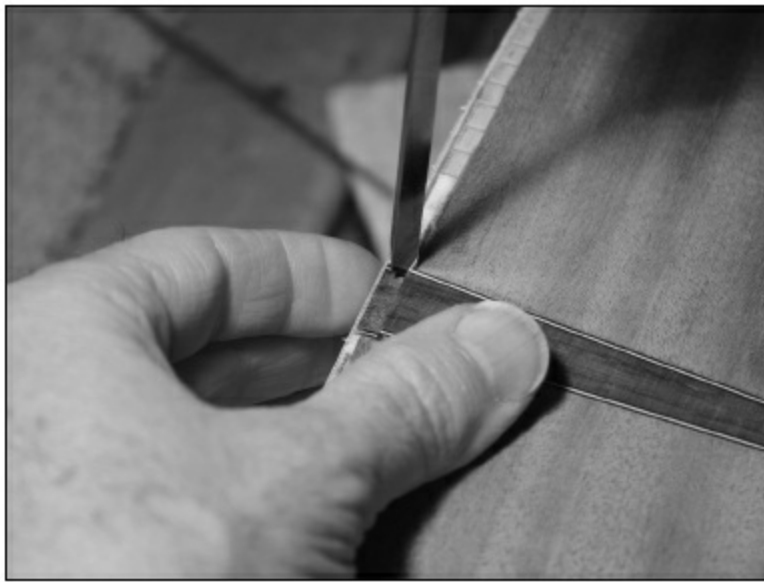
FIGURE 1.3.78. We trim the purfling edge of the endgraft to about a 45-degree angle. It may be just slightly different than an actual 45-degree angle, but not much. The angle is not as important as making the ends match each other.
