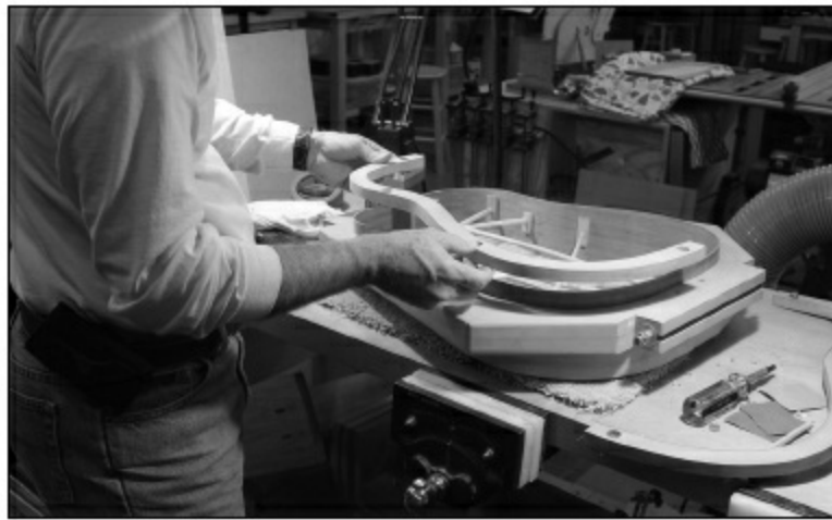
FIGURE 1.3.22. Now we remove the screws holding on the mold ribs. With the ribs removed, we can put the sides back onto the sander and sand them down to the profile line.
