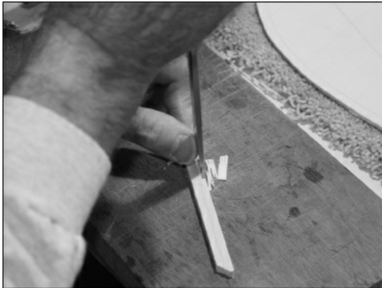
FIGURE 3.1.18. Now we use the chisel to cut out the notch. If it's not deep enough, we will extend the cut lines on each side slightly and make it deeper. Try not to make the notch too deep—we want the brace to fit exactly on the guitar top and the notch exactly on the bridge plate.
