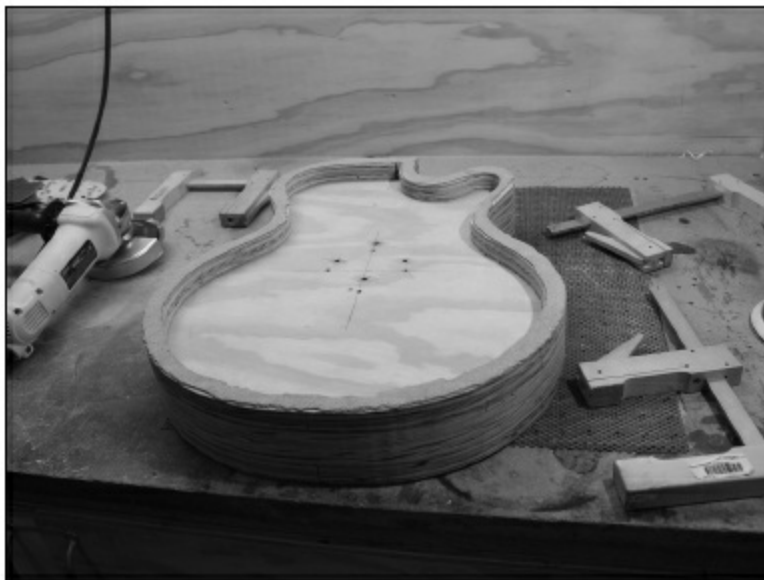
FIGURE 2.1.14. This is our work board. It is used to hold the archtop body around the edges and allows the arch to go in the recessed area. It is a critical part of building our archtops and is used in several steps.
