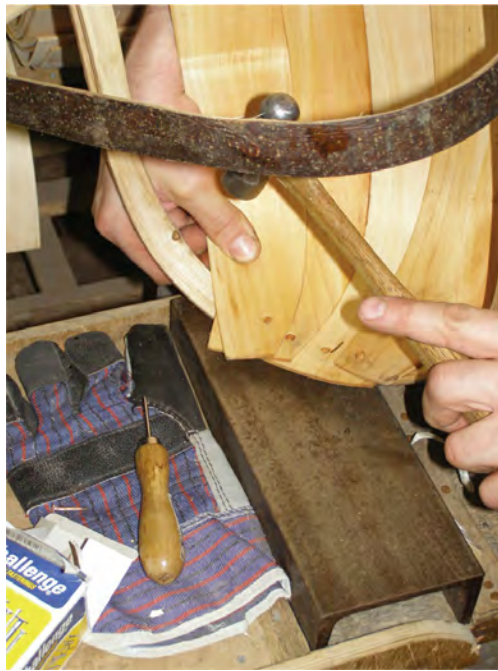
Fig. 5.40 Nailing the boards to the rim.
