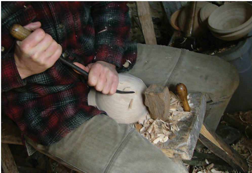
Fig. 3.23 Trimming the base with a long-handled knife.
