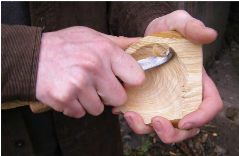
Fig. 3.32 a 'Thumb push' carving; b 'potato-peel' technique with a crook knife.
