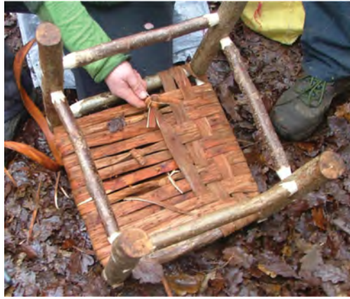
Fig. 4.34 When you run out of bark join in a new piece underneath as previously described.
