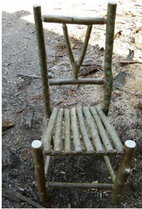
Fig. 4.43 Using forked wood to good advantage.
