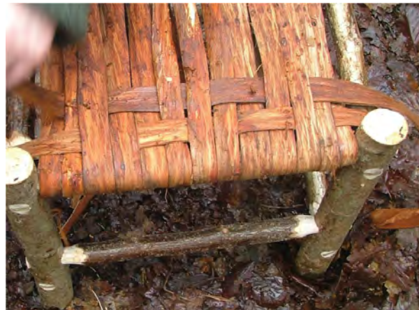
Fig. 4.33 The second row start 'over one, under two', and so on. Press the bark tight up against the first row and keep pulling it tight.
