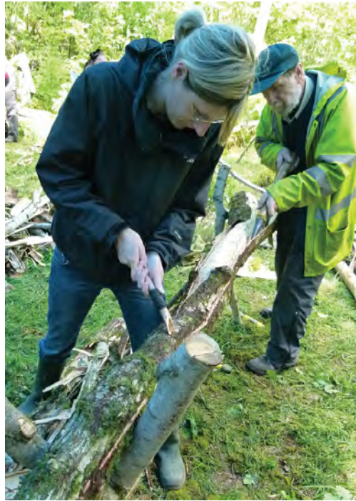
Fig. 6.9 Bark peeling using a homemade copper pipe peeling iron.
