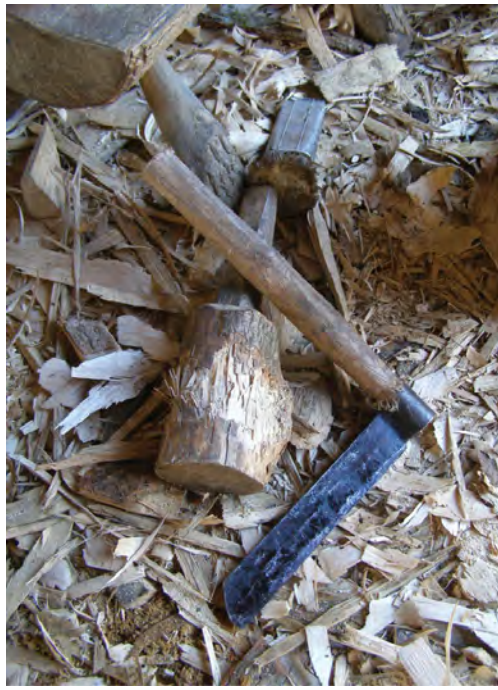
Fig. 2.29 Well-used shake-making froe and mallet.
