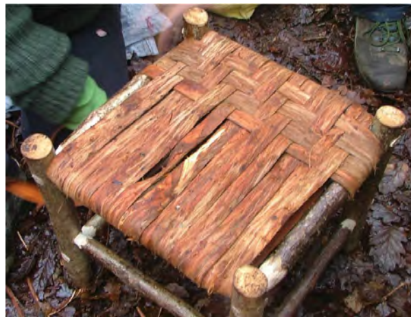
Fig. 4.35 The third row is 'under two, over two', and the fourth, 'under one, over two'. Repeat the pattern until you can fit no more rows in.
