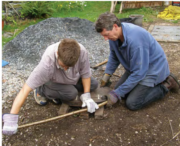
Fig. 5.33 Forming the bool with steamed hazel.
