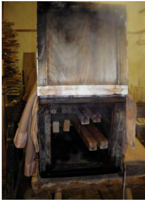
Fig. 2.47 The interior of the steam box.
