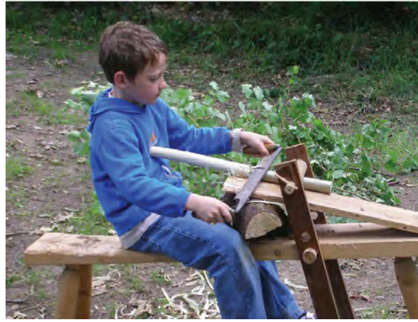
Fig. 2.19 Ensure the shave horse is the right proportions for the end user.
