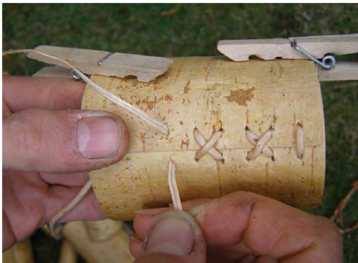
Fig. 5.28 a Making holes in the bark with a bradawl prior to stitching; b Stitching with the spruce root.
