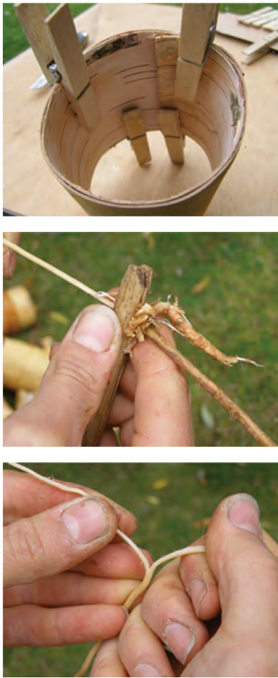
Fig. 5.27 a Coil of birch bark pegged together; b Stripping the bark off the spruce root; c Riving the spruce root into two.
