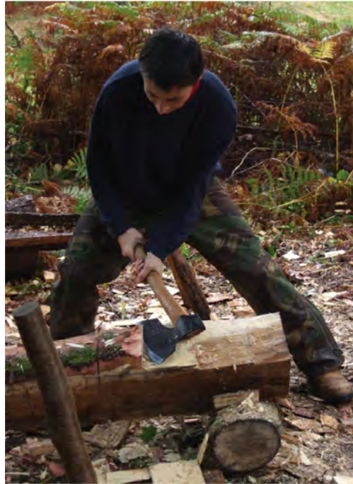
Fig. 7.11 Cut away the waste wood either with axe or chainsaw.
