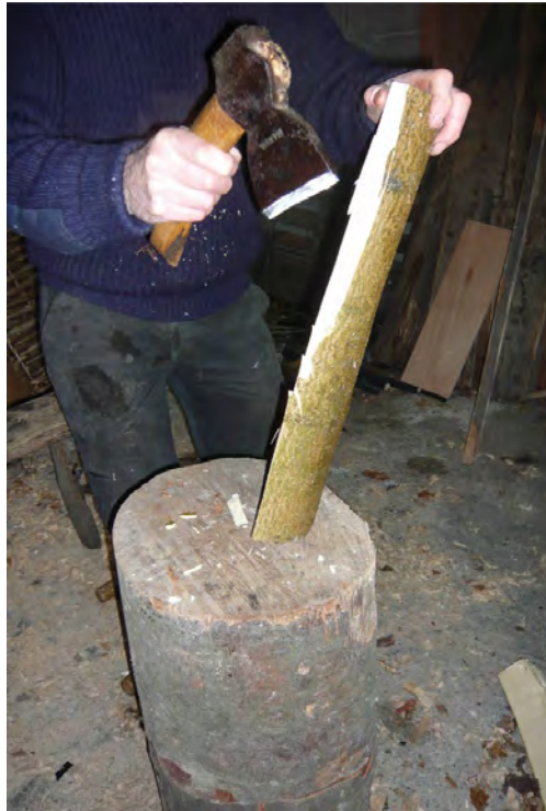
Fig. 4.19 Roughing out with a side axe.
