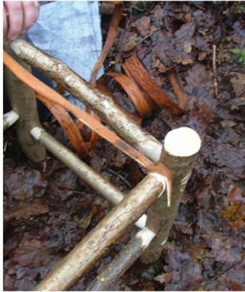
Fig. 4.26 Keep tension on the bark while winding it around the stool, making sure there are no gaps.
