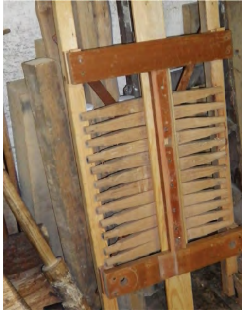
Fig. 2.26 Chair parts (back rails) left to set in a jig.
