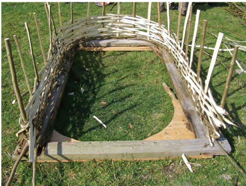
Fig. 6.20 Making your arch in a purpose-made jig will mean less damage to your lawn and will help with consistency of product. This is one that Alan Waters uses to make archways.
