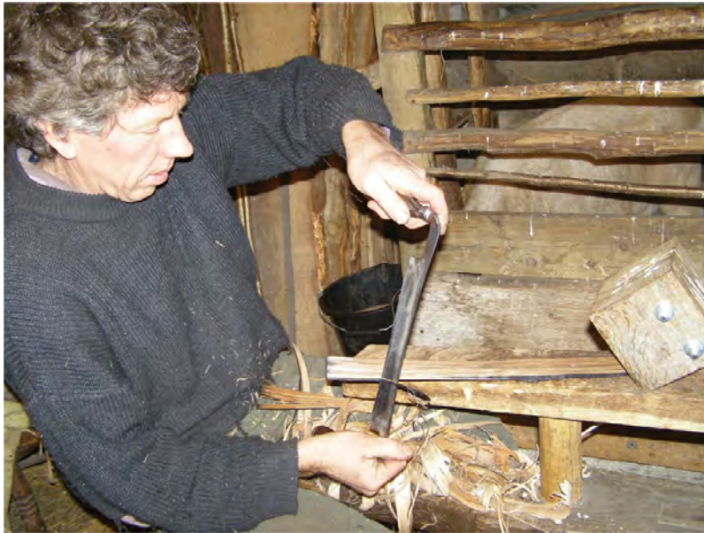
Fig. 5.31 Shaping the taws on a swiller's mare.
