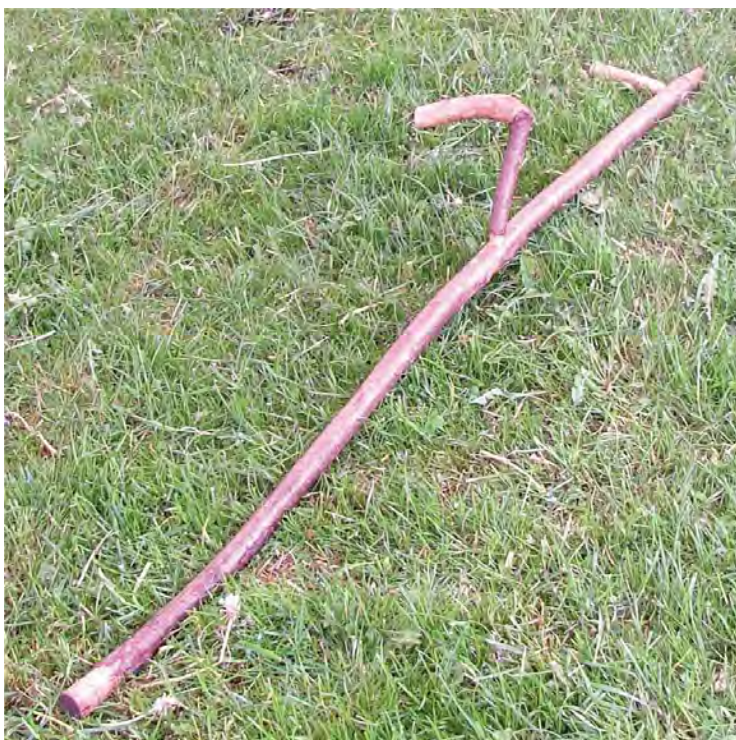
Fig. 8.27 This is a snaith made from a roundwood pole. It might utilize a natural fork or have the side handles attached.
