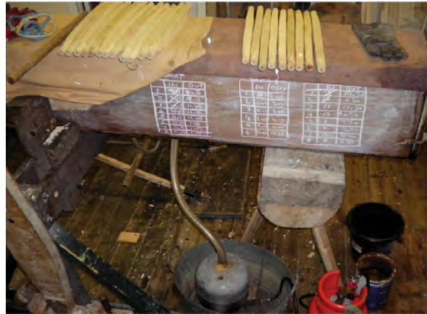
Fig. 2.48 Paul Girling's steambox with a record of what is being steamed written on the side.
