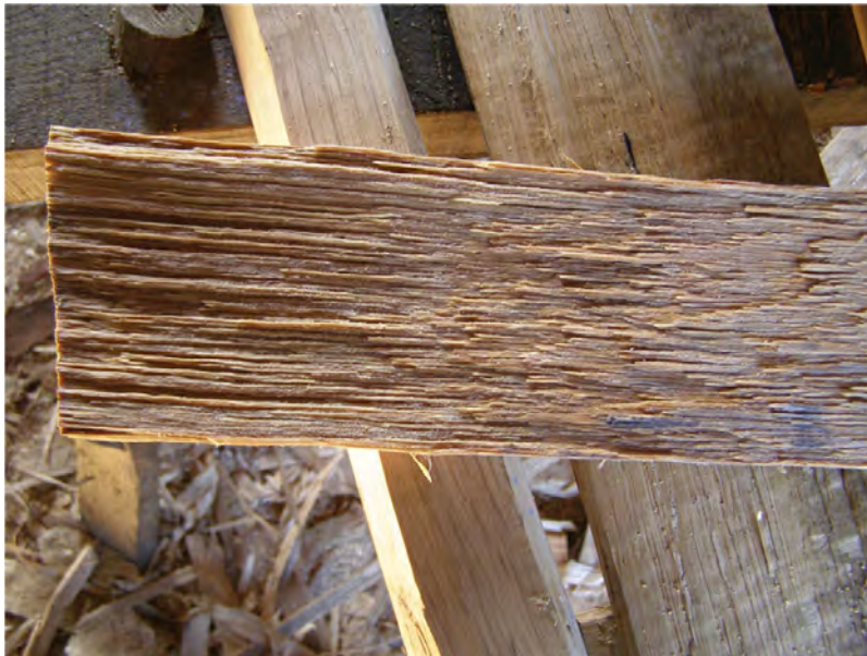
Fig. 7.43 Finished oak shake (this is a narrow one).
