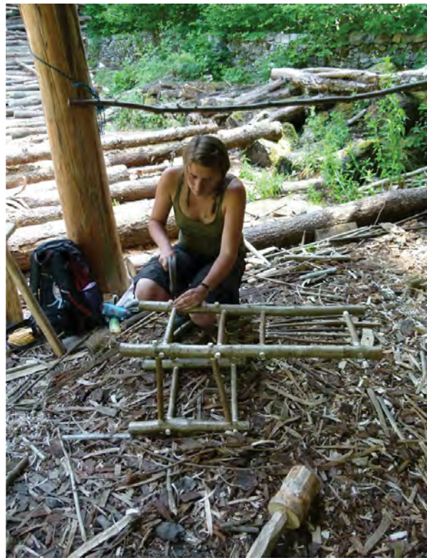
Fig. 4.47 Assembly of the chair with judicious use of a hammer.
