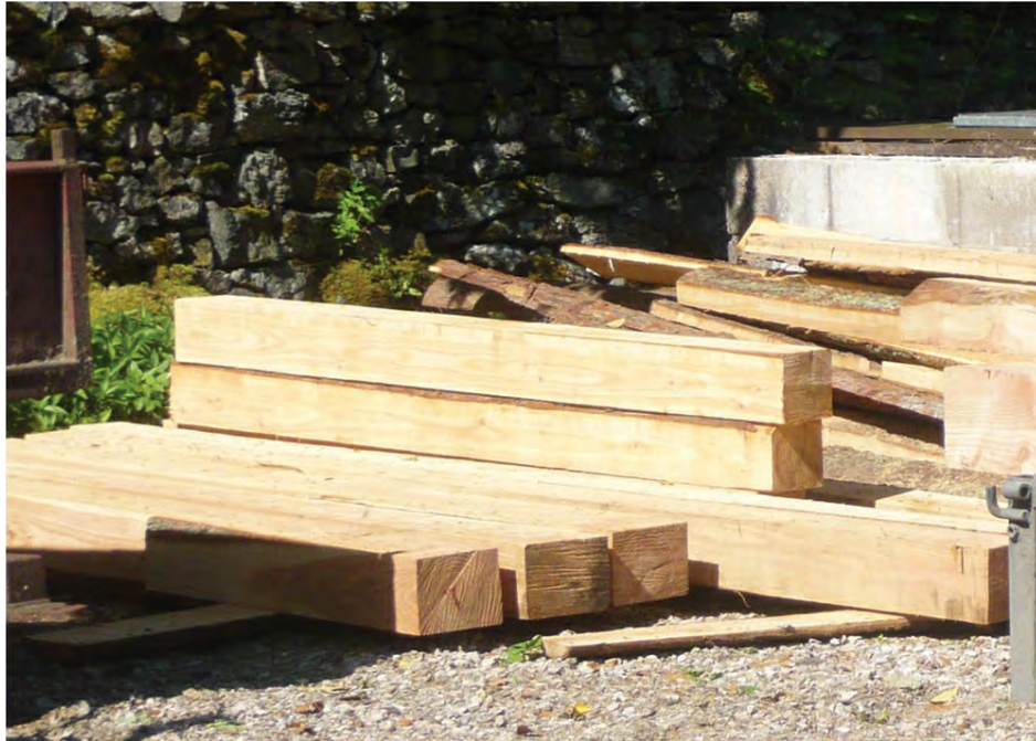
Fig. 7.30 The larch converted to beams with a chainsaw mill.
