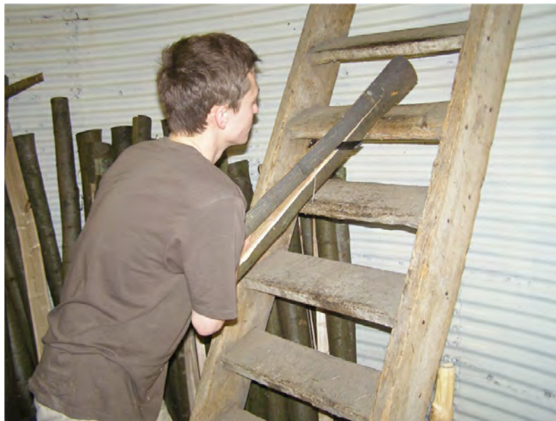
Fig. 5.38 Cleaving the trug bats.
