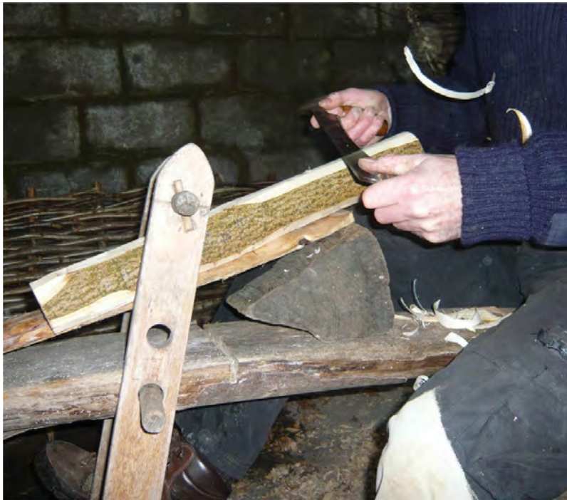
Fig. 4.20 Using a drawknife and shave horse.
