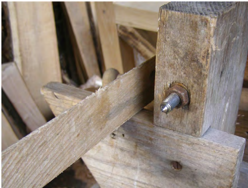
Fig. 2.8a and 2.8b Two views of how the crank fits into the head.
