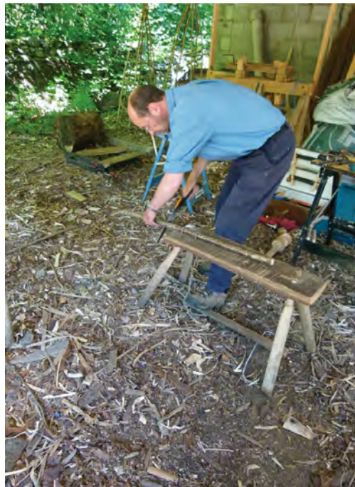
Fig. 4.45 Using a greenwood vice to hold the wood steady while cutting.
