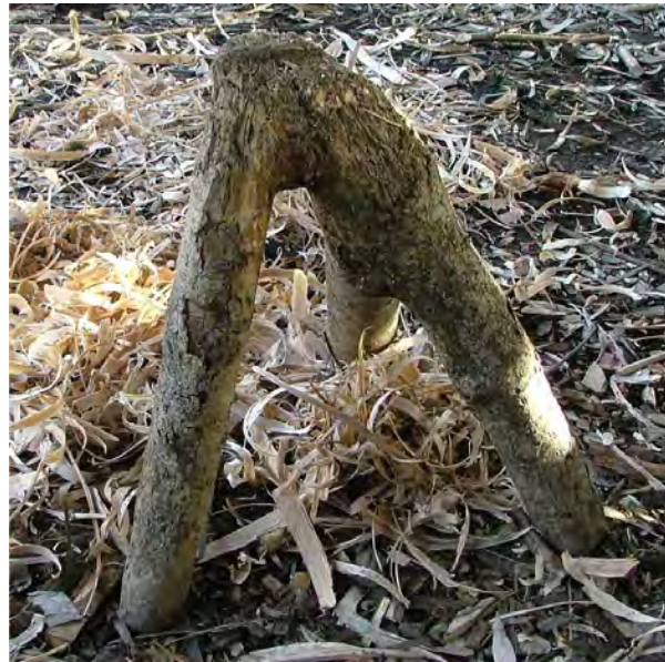
Fig. 2.1 A three-legged chopping block from a natural ash fork.
