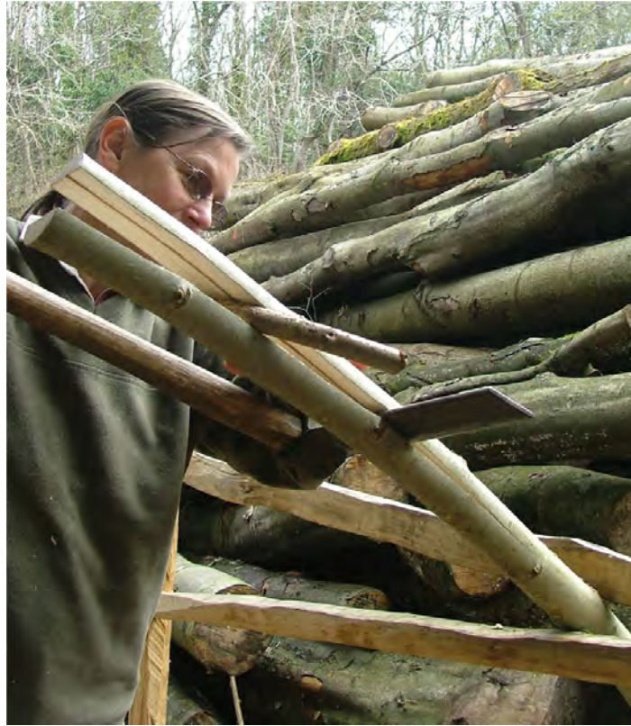
Fig. 8.4 Using the cleaving break and froe to produce two evenly cleft rails.
