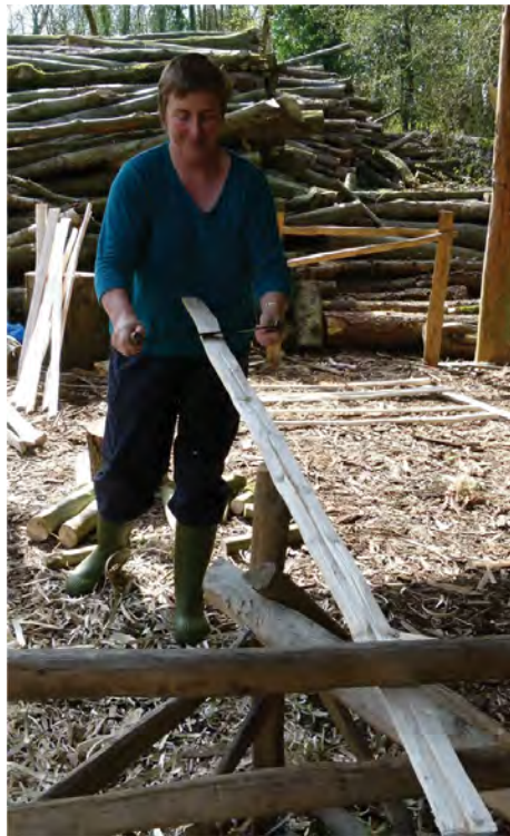
Fig. 8.5 (Left) Using a break to hold the rail while shaving it smooth with the drawknife.
