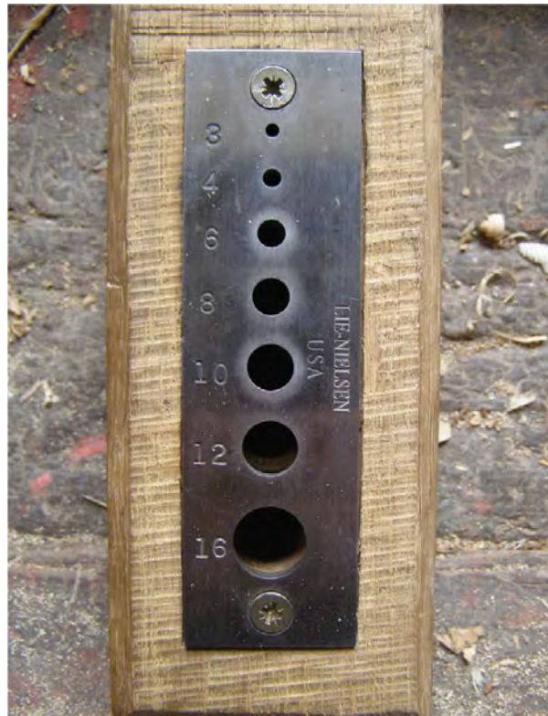
Fig. 2.46 Dowel plate – an alternative to the tine-former, used to make tines or dowels.
