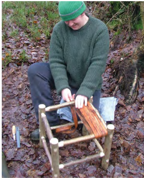
Fig. 4.27 When you get to the end of the piece of bark you will have to join a new piece with what is known as a weaver's knot on the underside of the stool.
