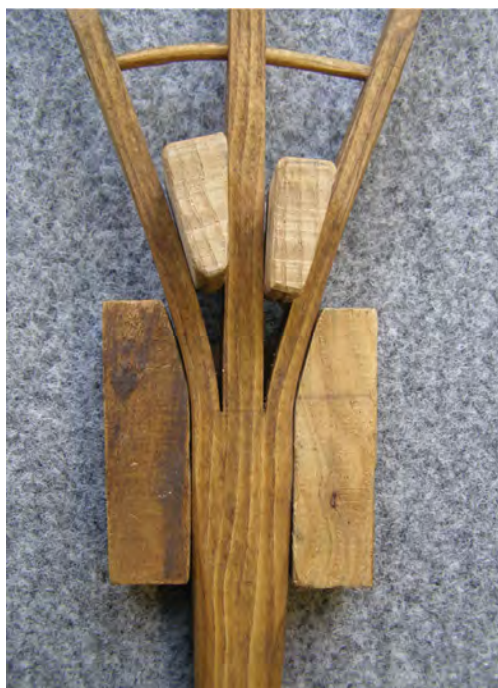
Fig. 8.22 Small jig to hold fork prongs apart at steaming.
