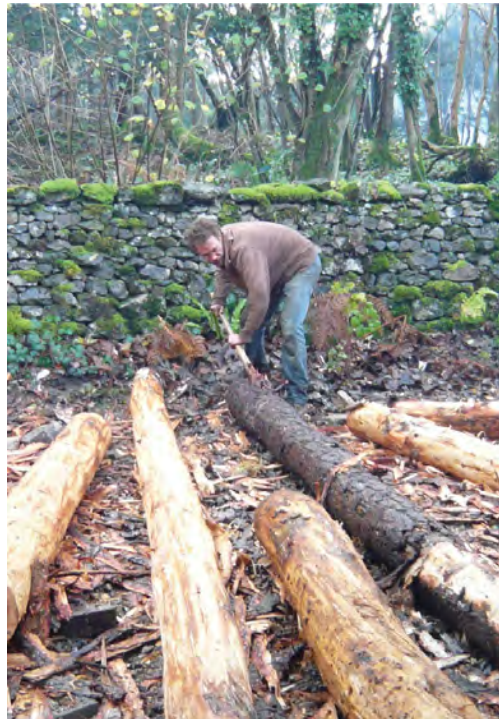
Fig. 7.6 Removing the bark with a bark stripping spade.
