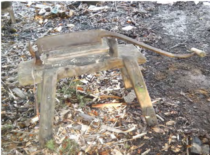
Fig. 2.37 Stock knife mounted on a low bench for maximum leverage.
