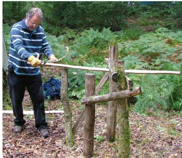
Fig. 2.22 A cleaving break with an extra post allowing the wood to be held under tension.
