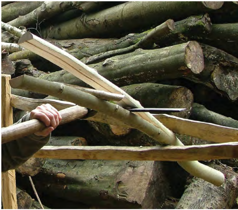
Fig. 2.21 Cleaving break in action.
