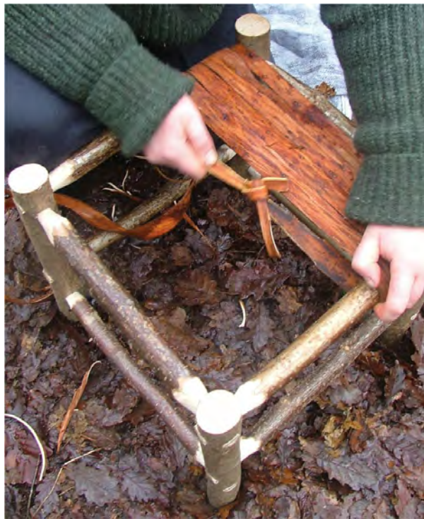
Fig. 4.31 The knot should be flat and hidden away. Continue like this until you have covered the stool completely, then take the bark around the side rail and head back the other way.
