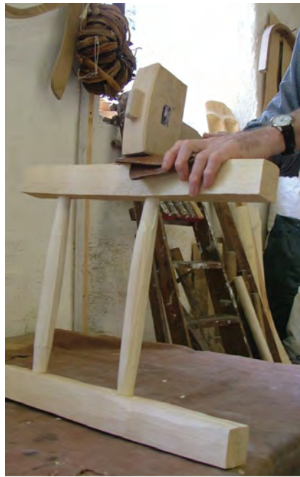
Fig. 4.22 Fitting the components together.
