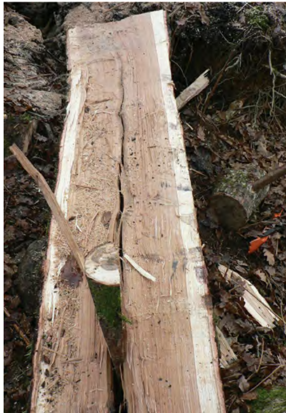
Fig. 8.11 Splitting an oak log lengthways with the help of a wedge.
