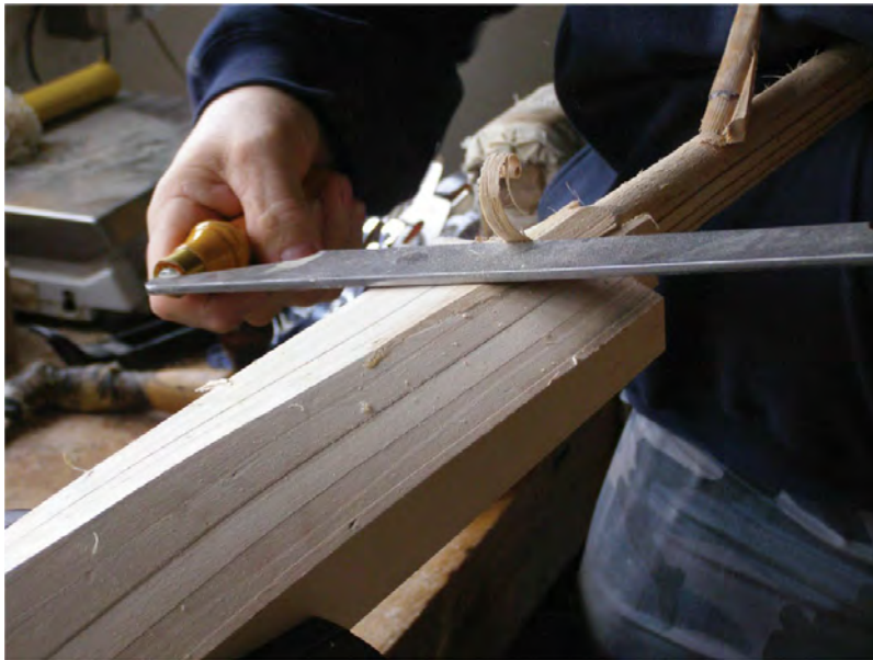
Fig. 3.18 The handle and bat are finished by shaving with a drawknife.
