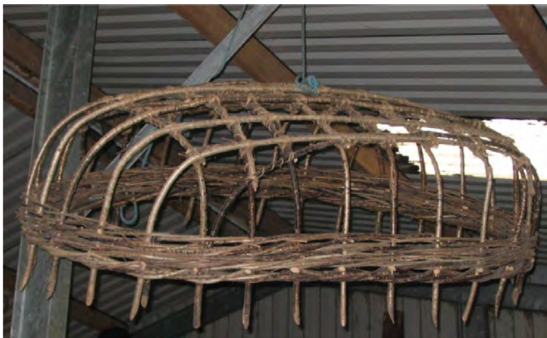
Fig. 5.11 Hazel frame Boyne coracle made by Joe Hogan. (Photo: Joe Hogan)
