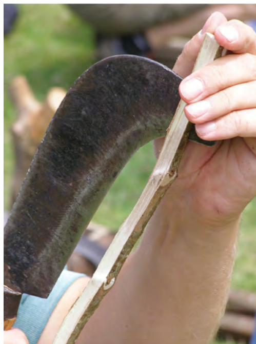
Fig. 7.46 a, b and c Three different methods of riving to make thatching
