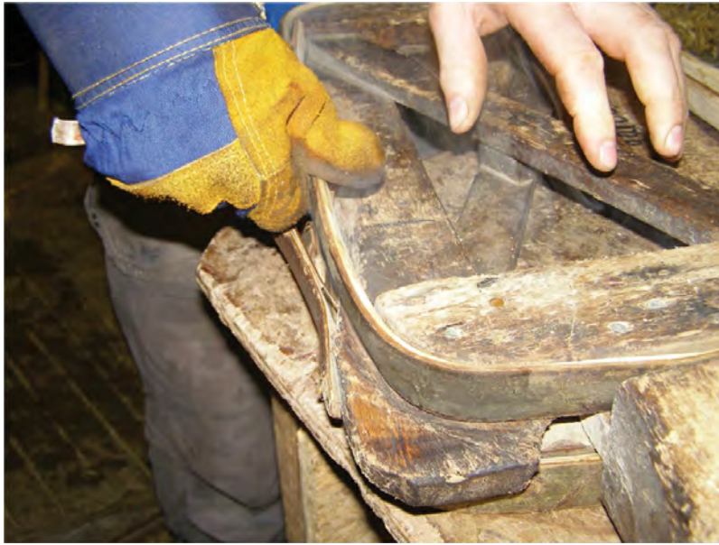
Fig. 5.39 Making the handle with steamed chestnut being bent around a former.
