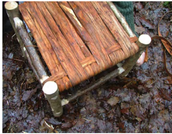
Fig. 4.32 For a lovely herringbone weave pattern you should start with 'over two, under two' all the way across the seat. Do the same back again underneath the seat as well.
