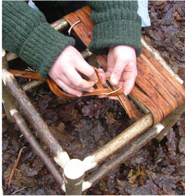
Fig. 4.30 Draw up the knot tight with gentle pressure and pushing as well as pulling; although strong, elm bark can snap if there is a bit of a fault caused by knots in the wood.
