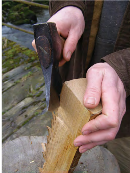
Fig. 3.30 Safe carving technique with the thumb well out of the way.
