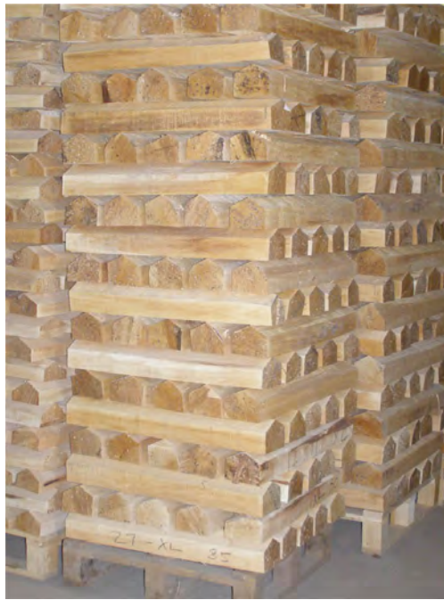
Fig. 3.17 Cricket bat blanks stacked in the kiln for drying.
