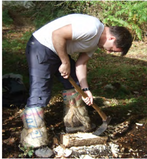
Fig. 2.34 Using an adze with lower leg protection.
