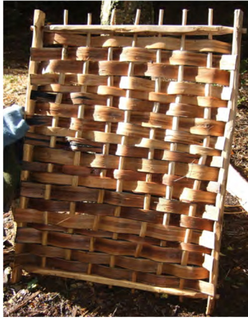
Fig. 6.18 The hard part is the last few strips, which must be coaxed through with a mixture of pushing and pulling.
