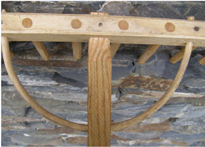
Fig. 8.28 This rake uses an ash bow for support. Maker: Steve Tomlin.
