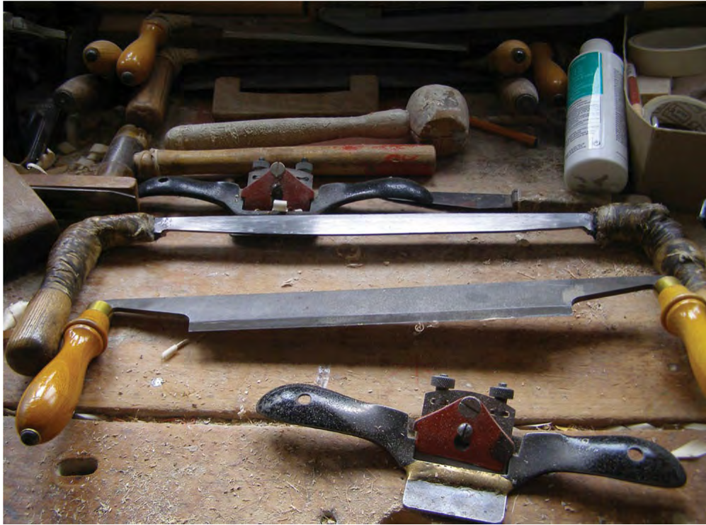
Fig. 2.33 Drawknives and a spoke shave at the Gray Nicolls cricket bat workshop.
