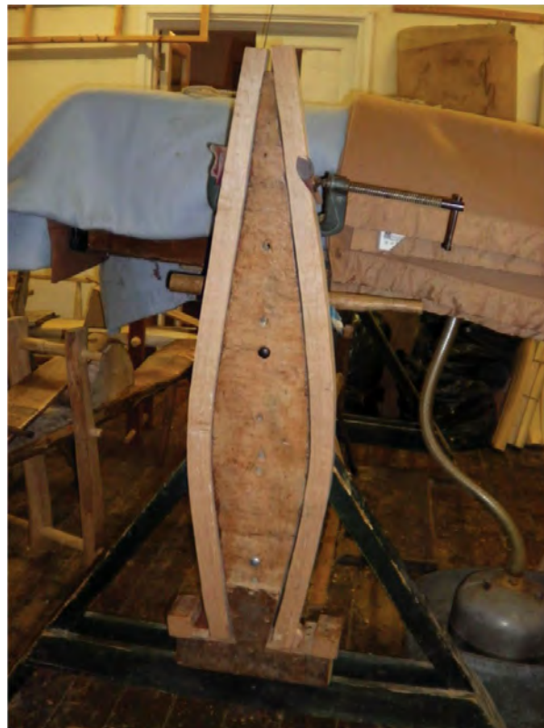
Fig. 2.27 The back legs of a chair clamped to a jig.
