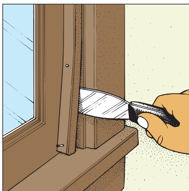
A. Gently loosen the stop bead before pulling out the nails. (Step 2)
